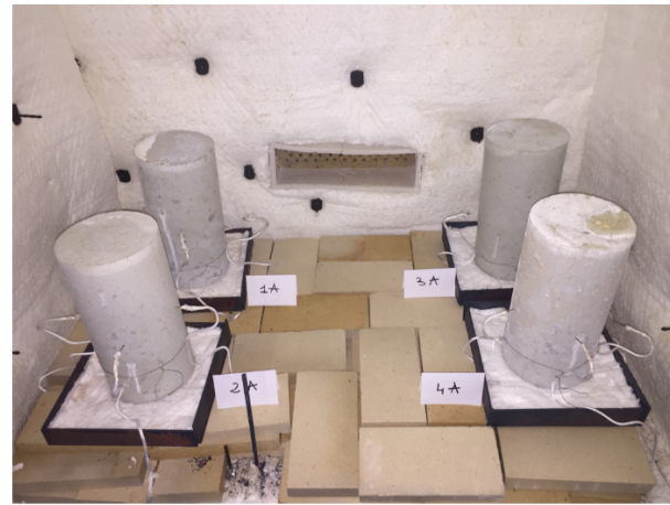
b) The test set up and samples configuration and data collection, before and after the fire test
