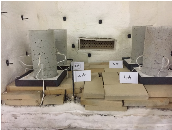
b) The test set up and samples configuration and data collection, before and after the fire test
