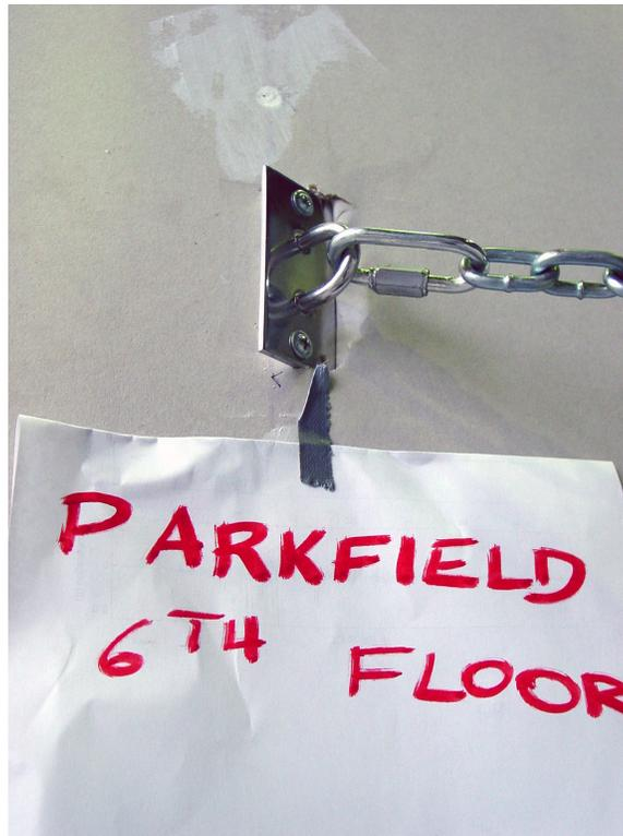
**Figure 9.2** The top photograph shows how the equipment is typically cross-chained to anchors that are screwed into the light steel framing of the wall. The bottom photograph shows the minor damage of the connection even under the very violent shaking induced by the UC Science Building 6th Floor Motion for the Cholome Array #8 record of the 1966 Parkfield, California, earthquake.
