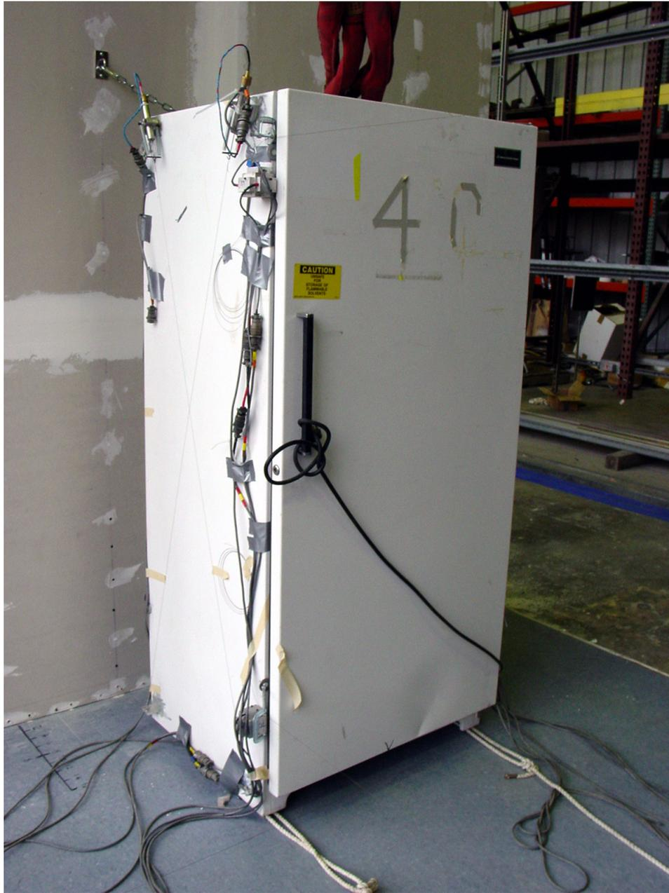
**Figure 9.1** The ASP refrigerator anchored to the mock non-structural wall that is nearly identical to those present at the UC Science laboratories.
