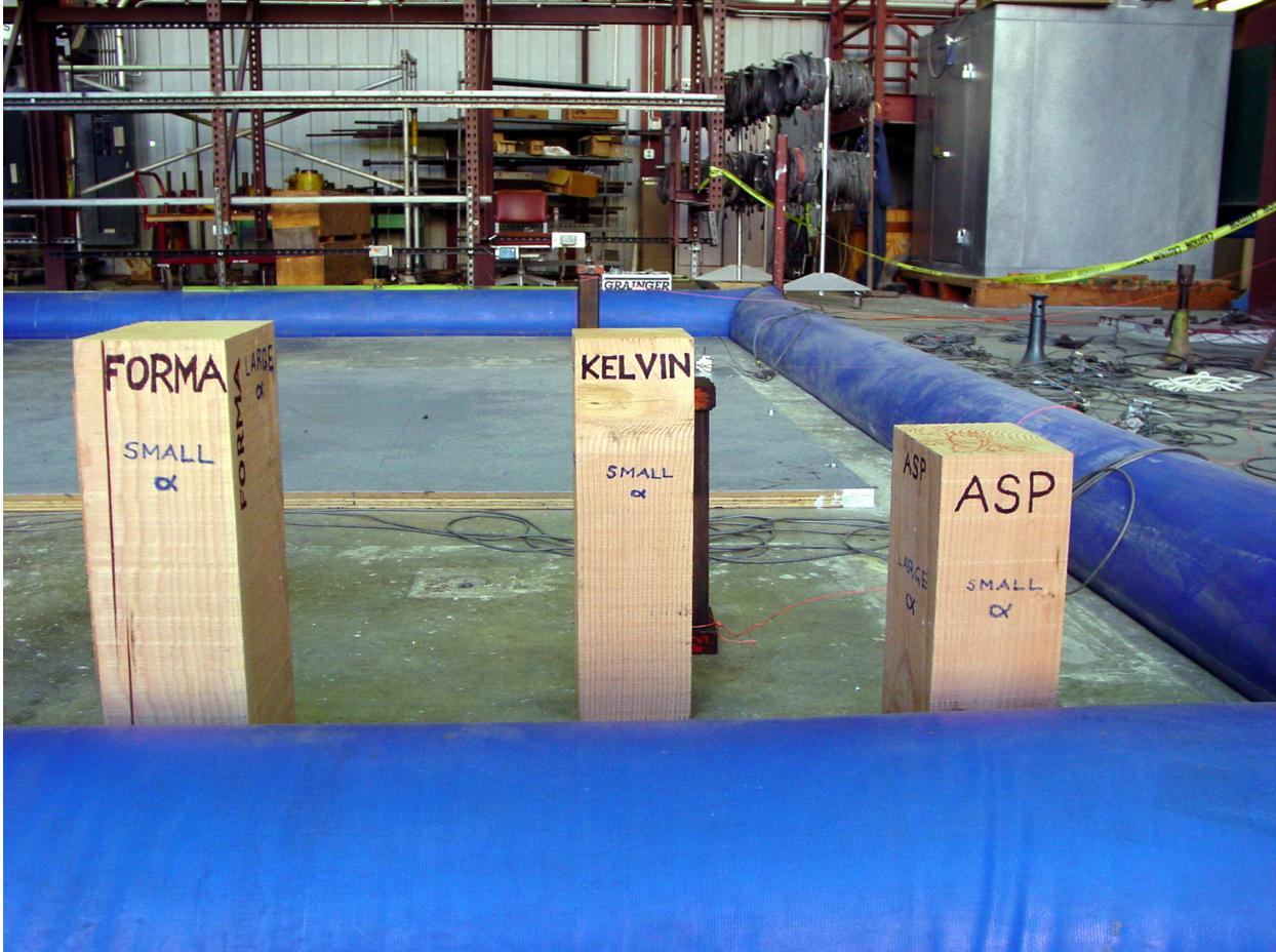
**Figure 7.1** Quarter-scale wooden block models of the full-scale prototype equipment (pictured in Fig. 3.1) resting on the shaking table at the Richmond Field Station Earthquake Simulation Laboratory, UC Berkeley. The excitation of the table is parallel to the more slender face of the models (labelled “SMALL  $\alpha$ ”).
