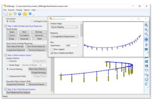
within a unified framework. Systematic evaluation of the global system response is conducted under a wide range of earthquake input shaking scenarios. The analysis options available in the new user interface MSBridge include: (1) pushover analysis; (2) mode-shape analysis; (3) single
