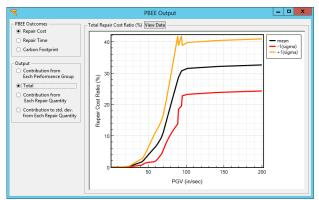
carbon emission) modeling; and (5) calculation of hazard curves. Once the time history results are computed, the user can view the PBEE results against any Intensity Measure (IM) and perform what-if scenarios by changing any parameter of the intermediate probabilistic models without recomputing the time history results.
