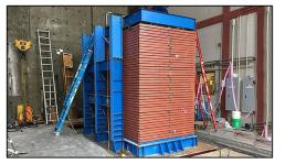
PEER announced the 2018 Blind Prediction Competition on the numerical simulation of a recently completed largescale liquefaction shaking table experiment. As a part of this PEER-funded project, a large-scale shaking table test was conducted at UCSD's Powell Structures Lab using a 2.9-m-tall soil laminar box that was the basis for this blind prediction competition. The experiment focused on the response of shallow foundations in liquefied soils. Both
