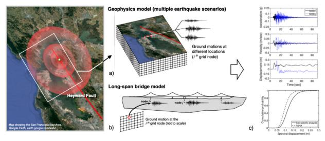
a) Geophysics model of the San Francisco Bay Area b) Representative long-period bridge c) Demonstrative model results for the evaluation of seismic risk variability
