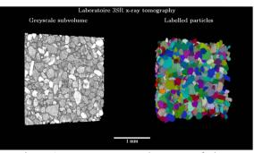
Figure 1. X-Ray Tomography Scans of Fine Sand Fabric
