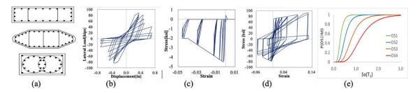
Figure 1: (a) Sample pre-1990 cross-sections; (b) Force-deformation response; (c) Material response: concrete; (d) Material response: reinforcing steel; (e) Sample fragility functions
