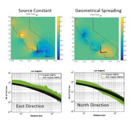
limitation, we will develop a complete non-ergodic GMPEs for California, with the coefficients of the GMPE that depend on the longitude and latitude of the earthquake and the site.
