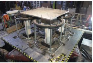
Shaking Table Test of a Rocking Podium Structure (2019)
