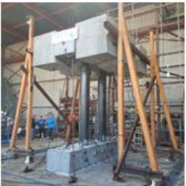
Shaking Table Test of a Self-Centering Bridge Bent (2017)
