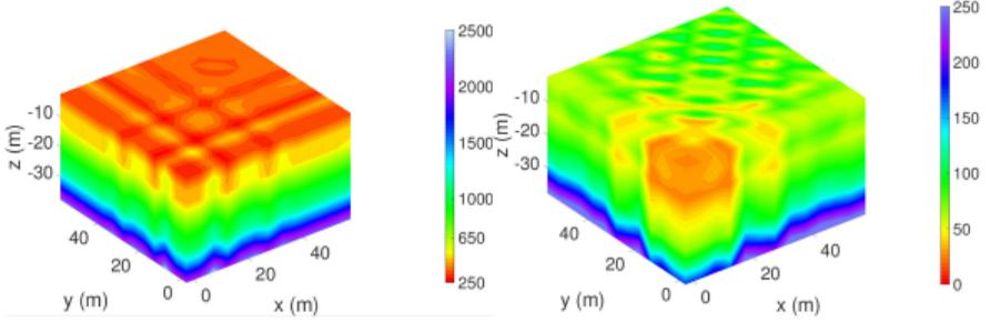
$V_P$  (m/s): mean (left) and standard deviation (right)
