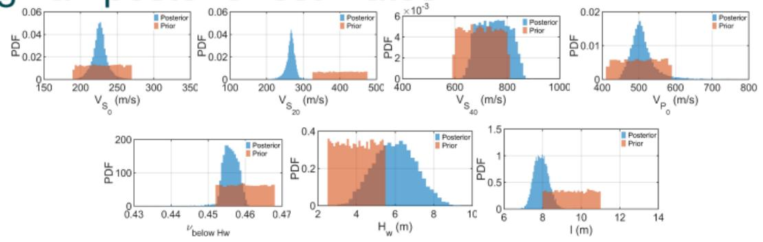
$V_{S0}$  ( $\uparrow$ ) and  $V_{P0}$  ( $\downarrow$ ) moved the most
