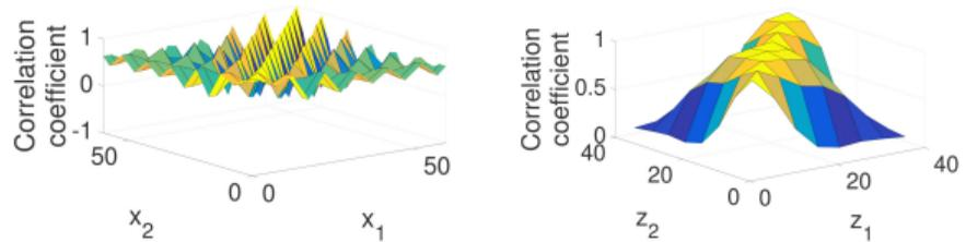
$V_S$  correlation structure: (left) x-direction at  $(y,z) = (30,0)$  and (right) z-direction at  $(x,y) = (20,30)$
