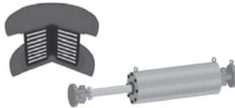
Figure 2.17 Thick laminated rubber bearings and oil dampers used in the FaCT reactor facility [Okamura et al. 2011].
