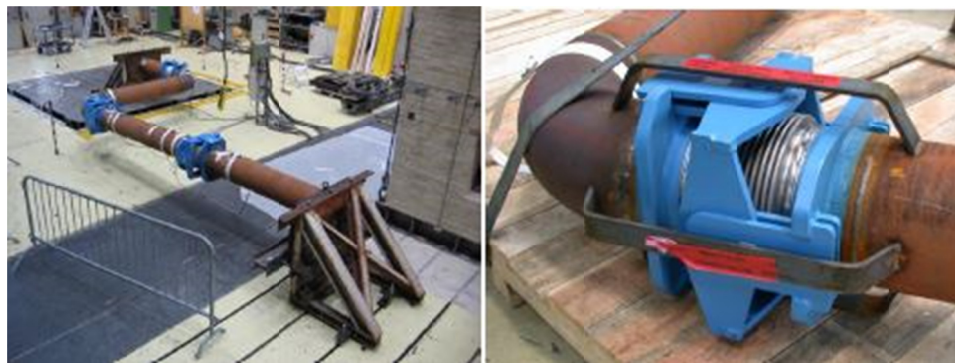
Figure 2.25 Pipeline expansion joints being tested for SILER.
