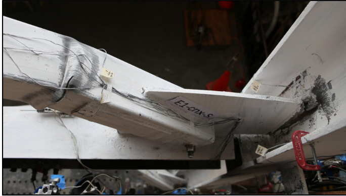
Figure 5.35 Local buckling and crack initiation of the second-story east brace.
