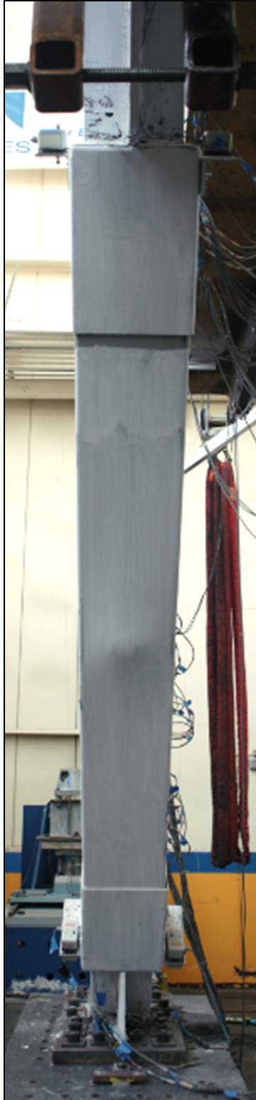
Figure 5.61 Final bulging of BRB casing.
