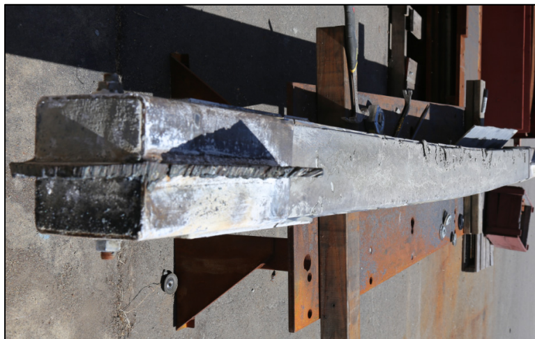
Figure 6.24 Inner concrete after test after global buckling of first-story west brace.
