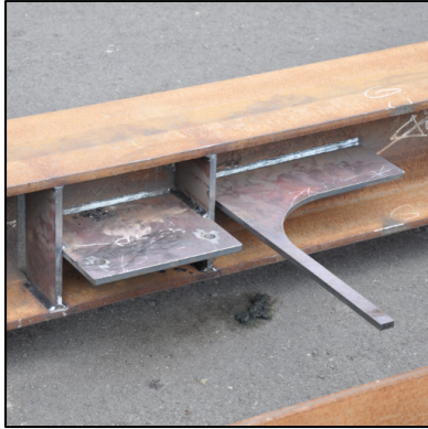
Figure 3.19 Original gusset plate “remnants” from NCBF-B-1 at first floor west connection of NCBF-B-3SB.
