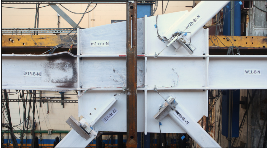
Figure 5.56 Final damage state of center connection and plastic hinging at first-floor east beam.
