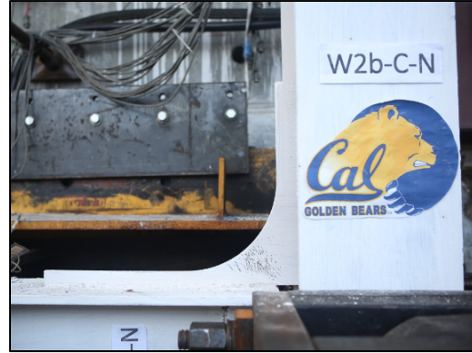
Figure 3.19 Original gusset plate “remnants” from NCBF-B-1 at first floor west connection of NCBF-B-3SB.
