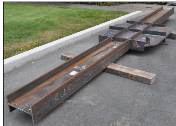
Figure 3.20 Erection of NCBF-B-3SB: parts after final shop fabrication.
