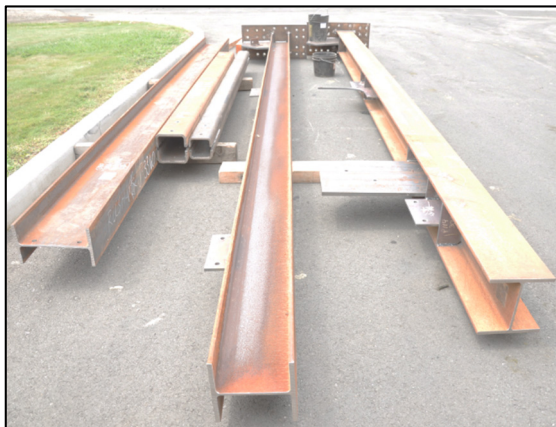
Figure 3.20 Erection of NCBF-B-3SB: parts after final shop fabrication.
