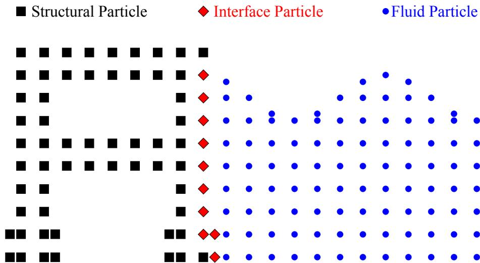
Figure 2.2: A cloud of FSI particles.
