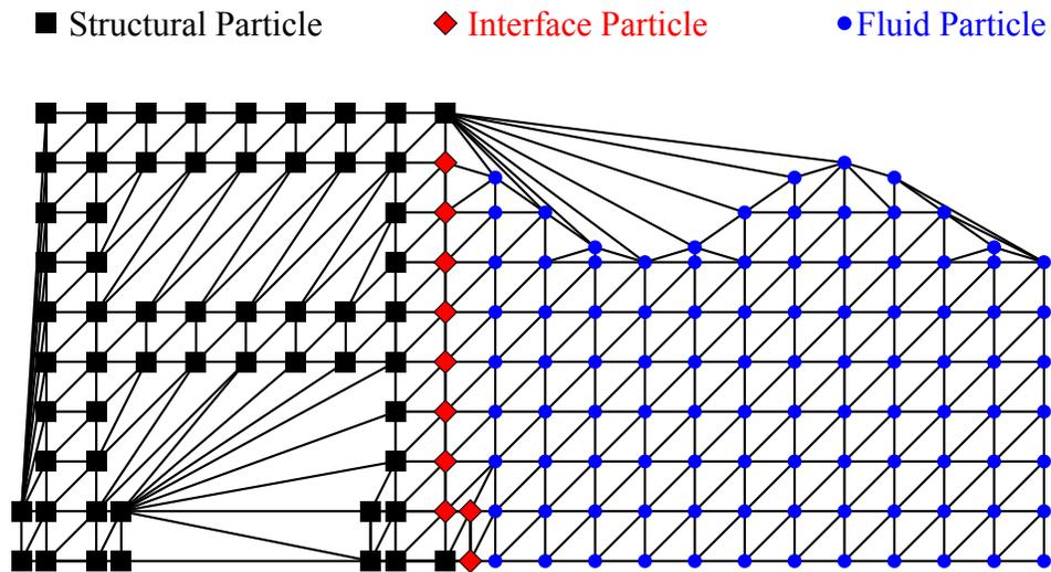
Figure 2.3: Delaunay Triangulation of the cloud of FSI particles.
