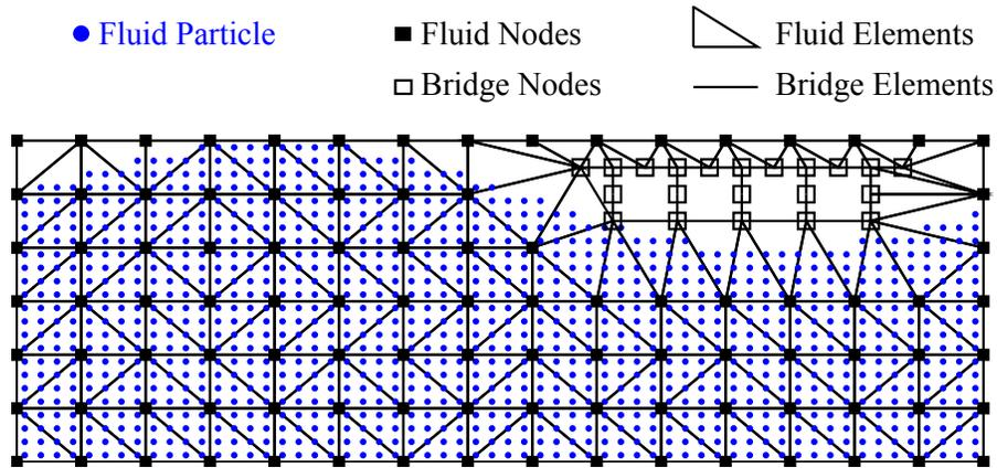
Figure 2.8: The Delaunay Triangulation between fixed-fluid mesh and structure.
