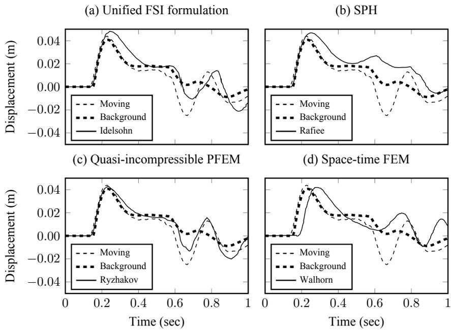
Figure 3.7: Comparison of the displacements of the free end of the elastic obstacle with different numerical approaches.
