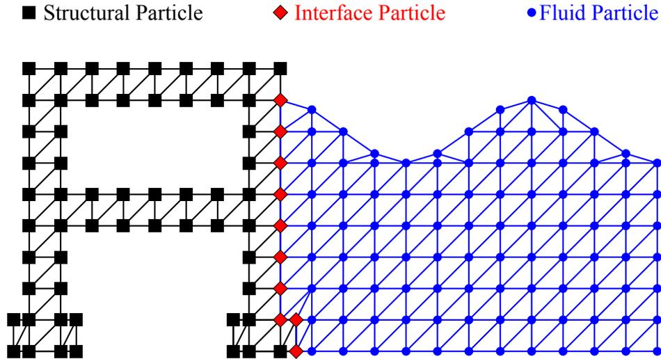
Figure 2.4: Moving mesh of the cloud of FSI particles.
