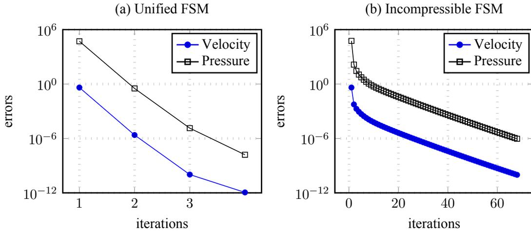
Figure 3.14: Convergence of velocity and pressure using unified FSM and incompressible FSM with viscosity  $\mu = 50$  Pa-s and time step  $\Delta t = 10^{-3}$  sec.
