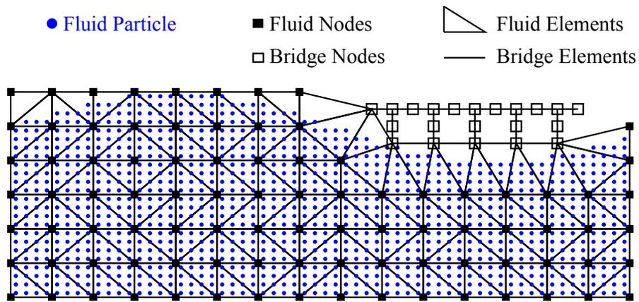
Figure 2.9: The background mesh with fixed fluid mesh and structure.
