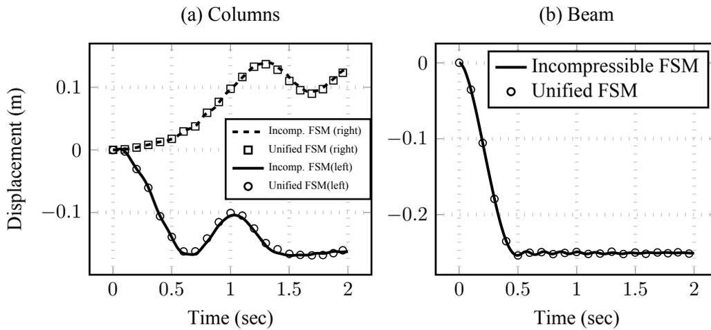
Figure 3.11: Tip deflection of left and right columns and middle deflection of the bottom beam using the unified FSM and the incompressible FSM with viscosity  $\mu = 10^{-3}$  Pa-s and  $\Delta t = 10^{-3}$  sec.
