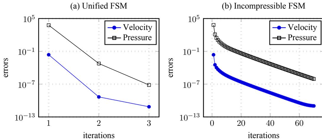
Figure 3.17: Convergence of velocity and pressure using unified FSM and incompressible with viscosity  $\mu = 10^3$  Pa-s and time step  $\Delta t = 5 \times 10^{-5}$  sec.
