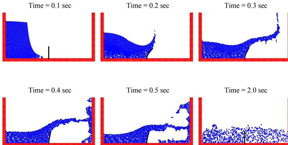
Figure 3.5: Snapshots of a dam break as an elastic obstacle with moving mesh.
