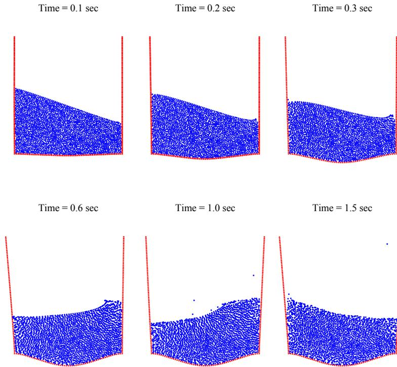
Figure 3.10: Snapshots of water sloshing in a flexible tank using the unified FSM and the incompressible FSM with viscosity  $\mu = 10^{-3}$  Pa-s and  $\Delta t = 10^{-3}$  sec.
