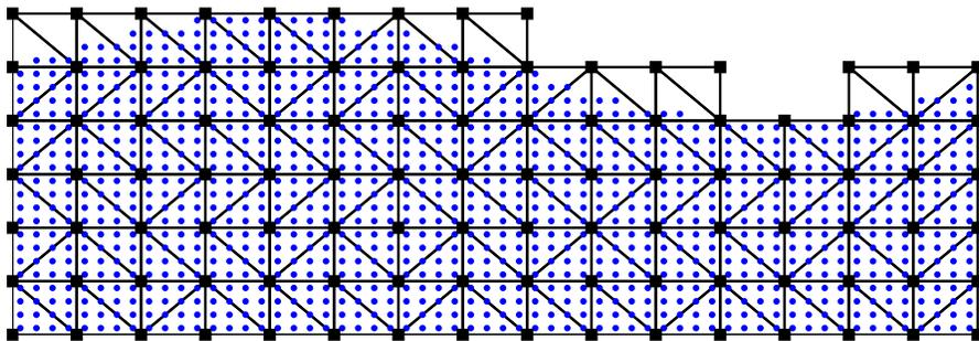
Figure 2.6: The fixed fluid mesh based on the fluid particles.
