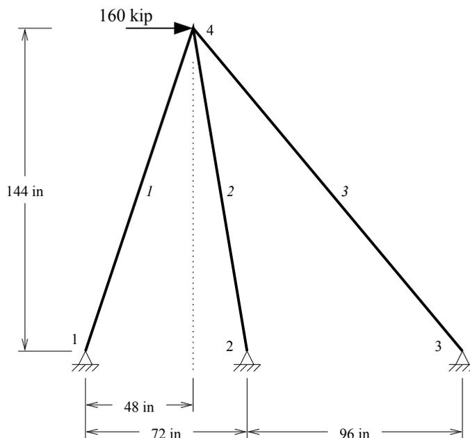
Figure 4.5: Truss model for the Python interpreter.
