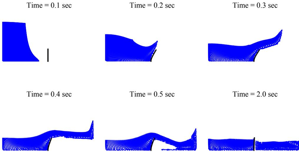
Figure 3.6: Snapshots of a dam break as an elastic obstacle with background mesh.
