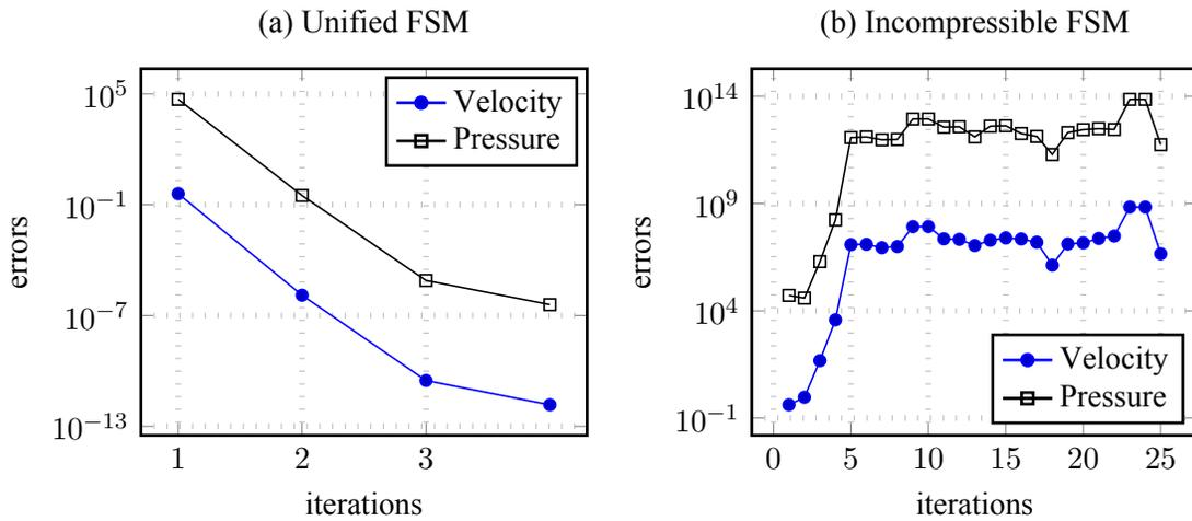
Figure 3.16: Convergence of velocity and pressure using unified FSM and incompressible FSM with viscosity  $\mu = 10^4$  Pa-s and time step  $\Delta t = 10^{-3}$  sec.
