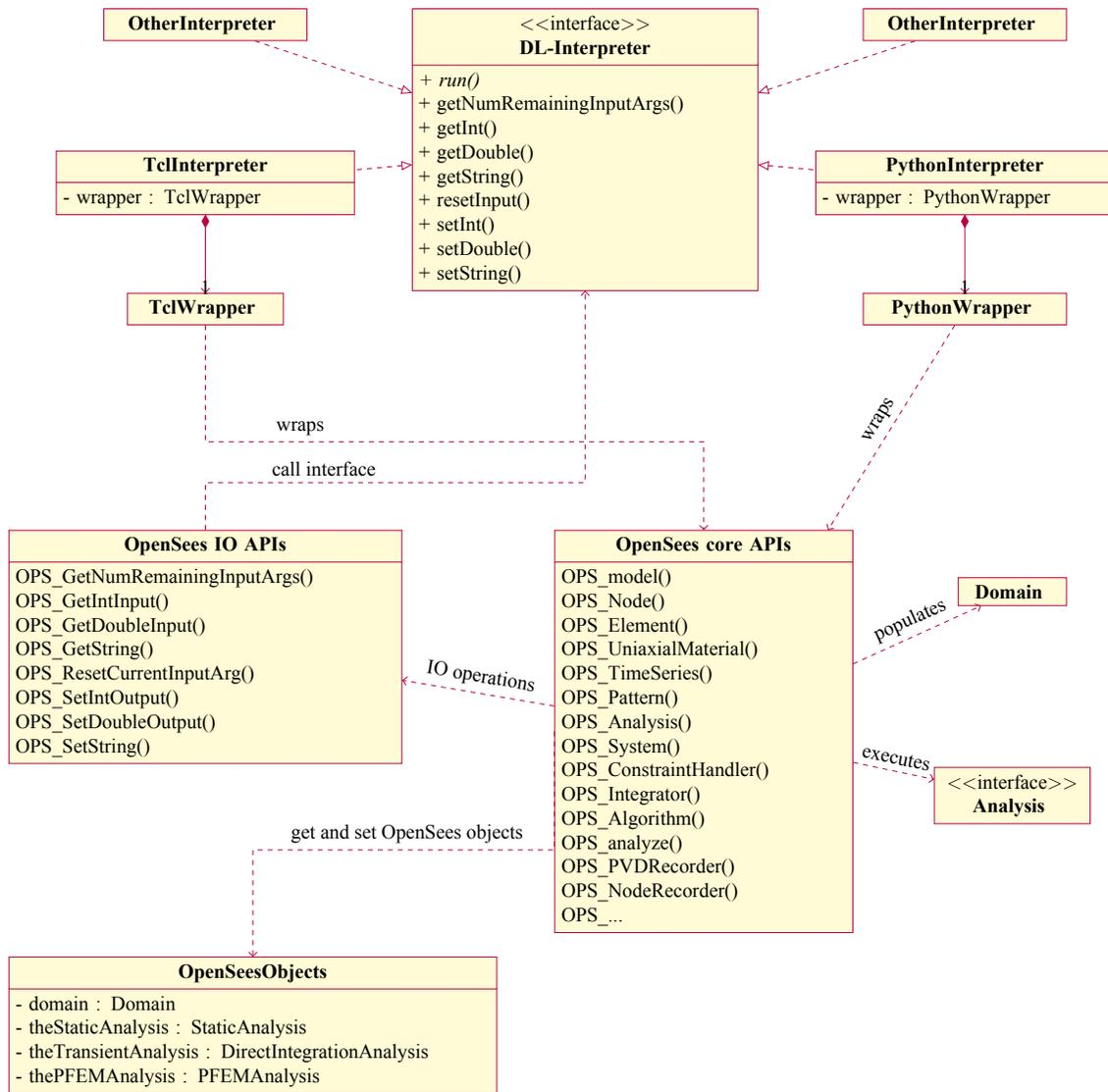
Figure 4.1: Class diagram of multi-interpreter interface.
