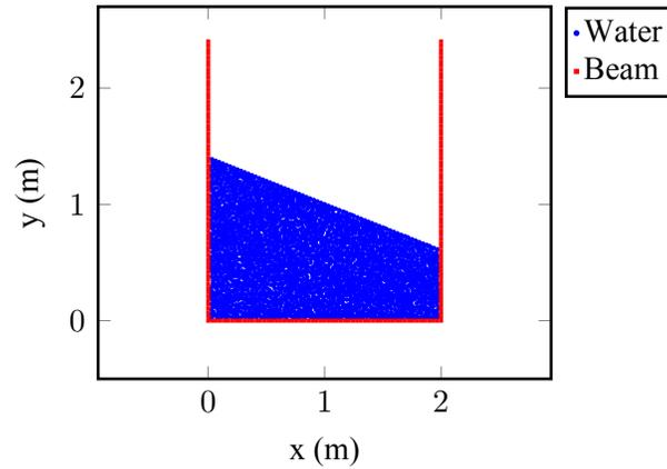
Figure 3.9: Model of 2D water sloshing analysis in a rectangular tank.
