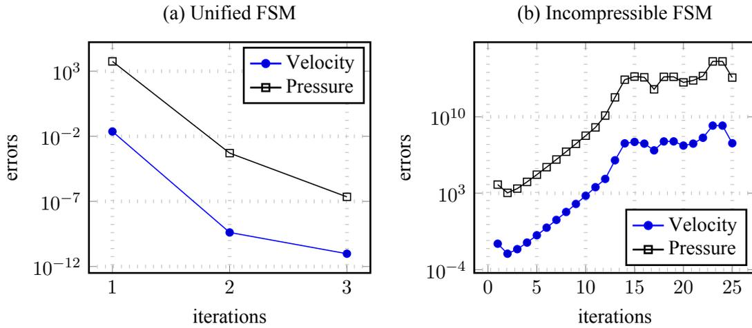
Figure 3.18: Convergence of velocity and pressure using unified FSM and incompressible FSM with viscosity  $\mu = 10^4$  Pa-s and time step  $\Delta t = 5 \times 10^{-5}$  sec.
