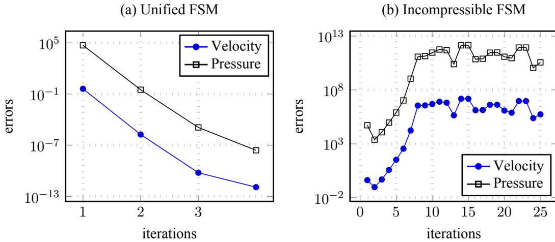
Figure 3.15: Convergence of velocity and pressure using unified FSM and incompressible FSM with viscosity  $\mu = 10^3$  Pa-s and time step  $\Delta t = 10^{-3}$  sec.
