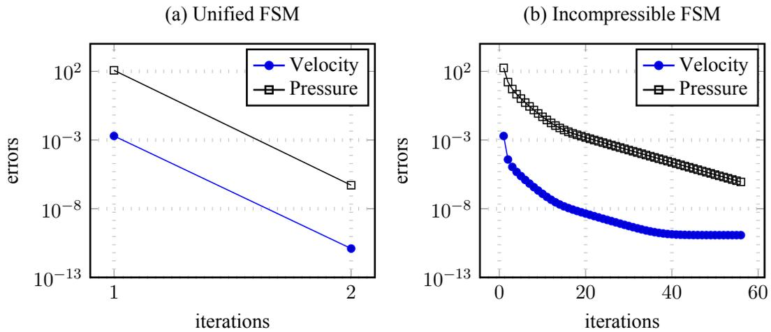
Figure 3.19: Convergence of velocity and pressure using unified FSM and incompressible FSM with viscosity  $\mu = 10^4$  Pa-s and time step  $\Delta t = 4 \times 10^{-6}$  sec.
