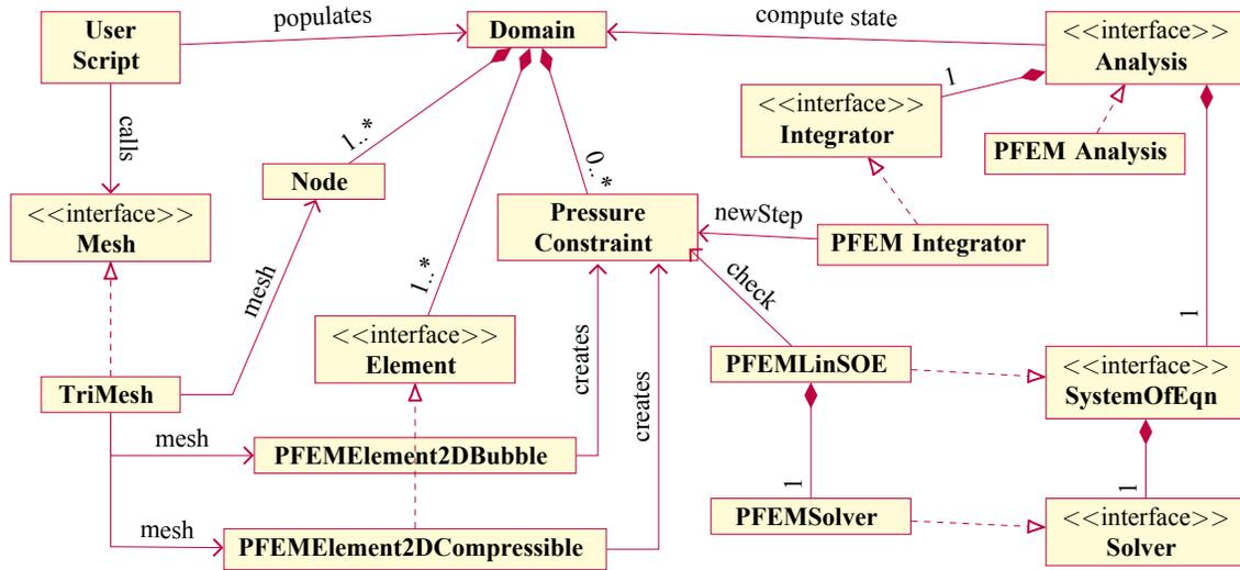
Figure 3.1: Class diagram of the FSI implementation in OpenSees framework.
