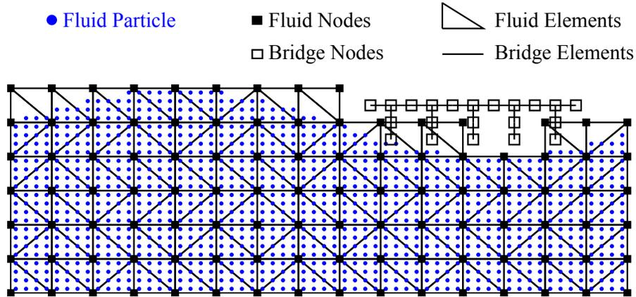
Figure 2.7: The fixed-fluid mesh with structure.
