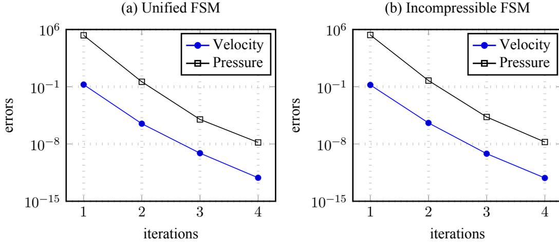
Figure 3.12: Convergence of velocity and pressure using unified FSM and incompressible FSM with viscosity  $\mu = 10^{-3}$  Pa-s and time step  $\Delta t = 10^{-3}$  sec.
