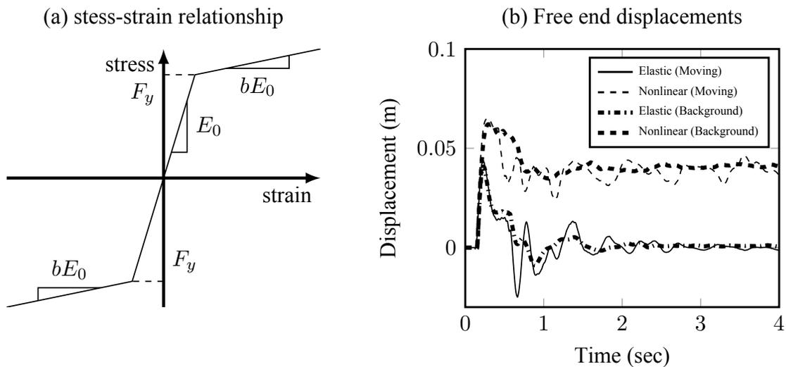
Figure 3.8: Nonlinear material for obstacle in dam-break problem and comparison of free-end displacements with elastic material.
