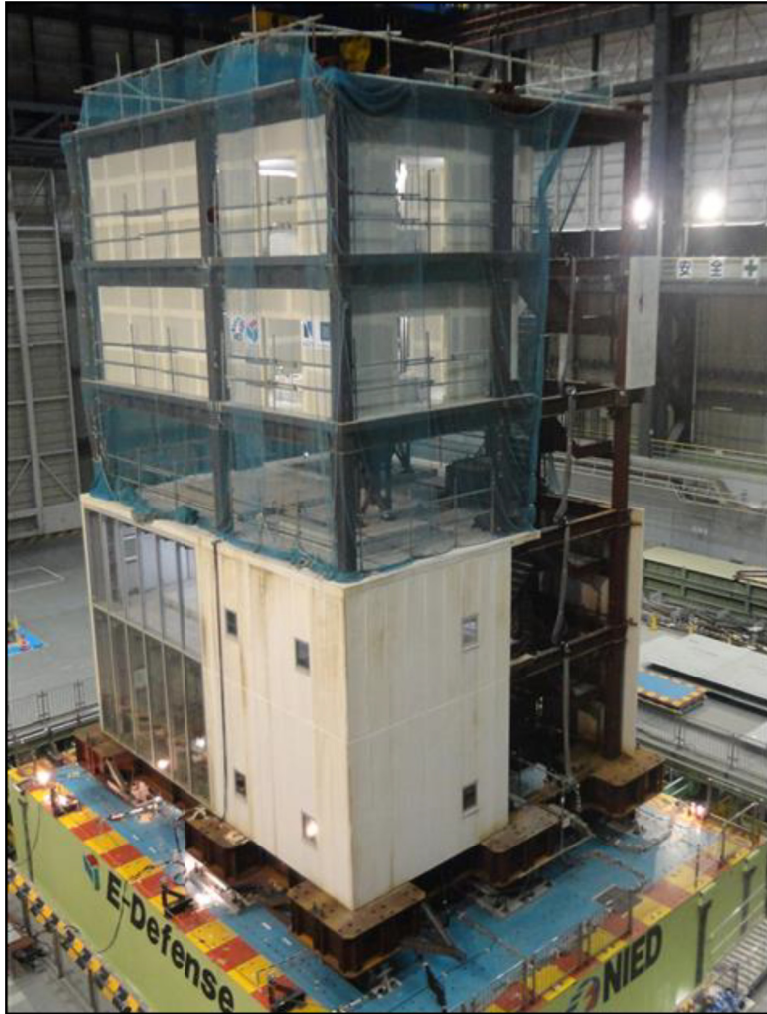
Figure 1.6 Full-scale five-story steel moment frame test specimen [Dao and Ryan 2015].
