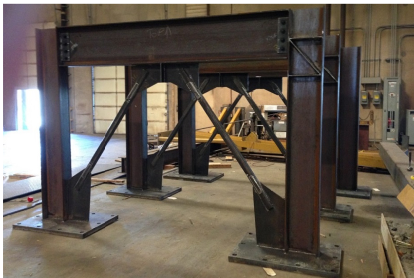
Figure 4.10 The three fully fabricated test specimens before shipping to UNR.
