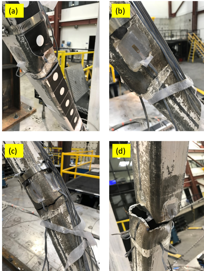
Figure 5.22 Stages of brace failure: (a) local buckling, (b) crack initiation, (c) crack propagation, and (d) fracture.
