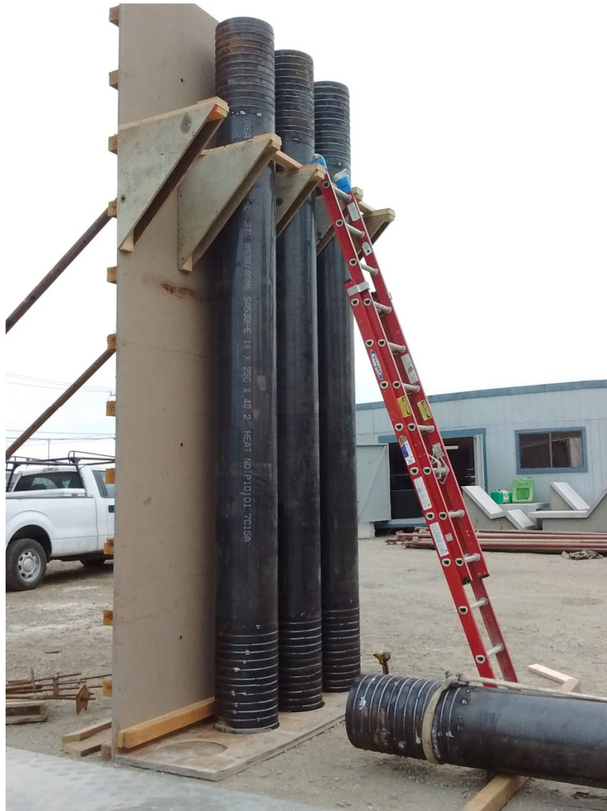
Figure 4.3 Column casting setup.
