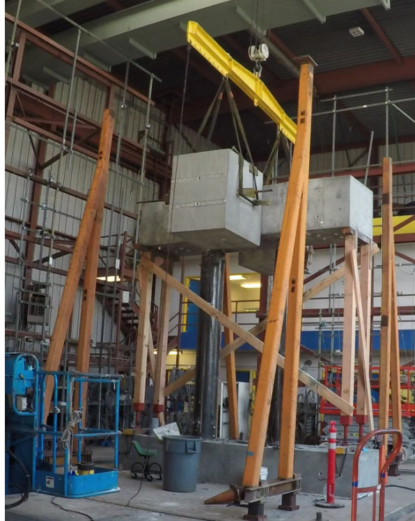
Figure 4.11 Superstructure mass block installation.
