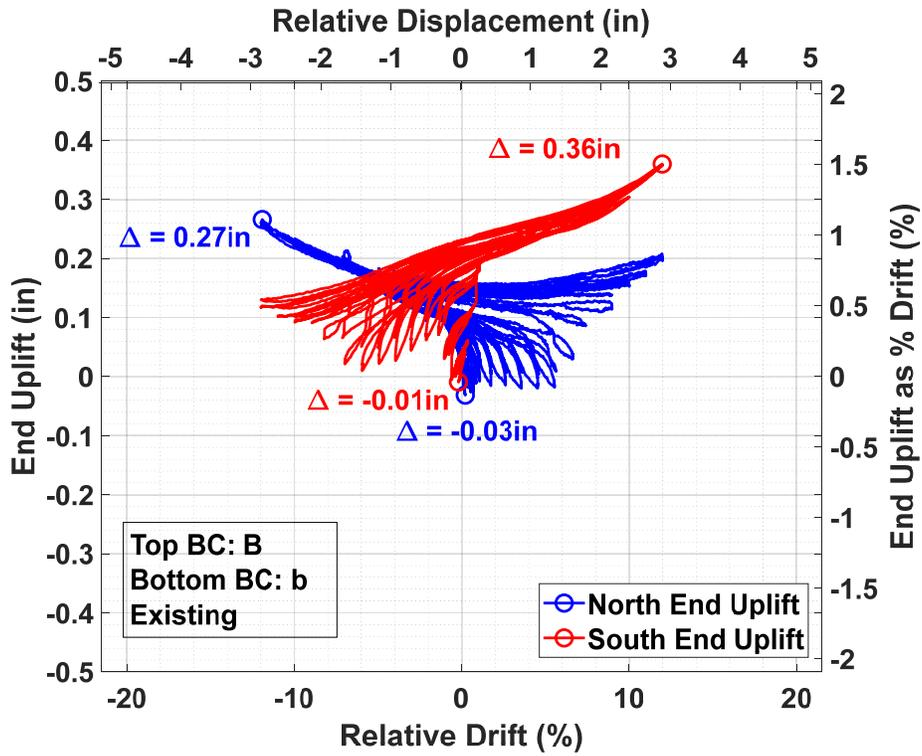
Figure C.24 Specimen A-4 end uplift versus relative drift.
