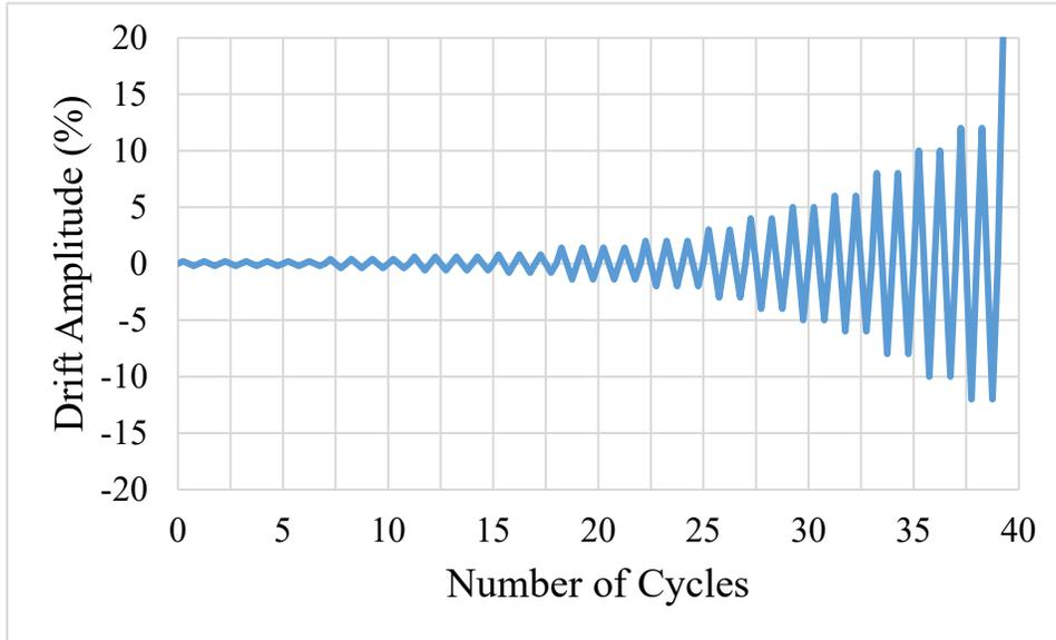
**Figure A.4 Specimen A-3 loading protocol.**
