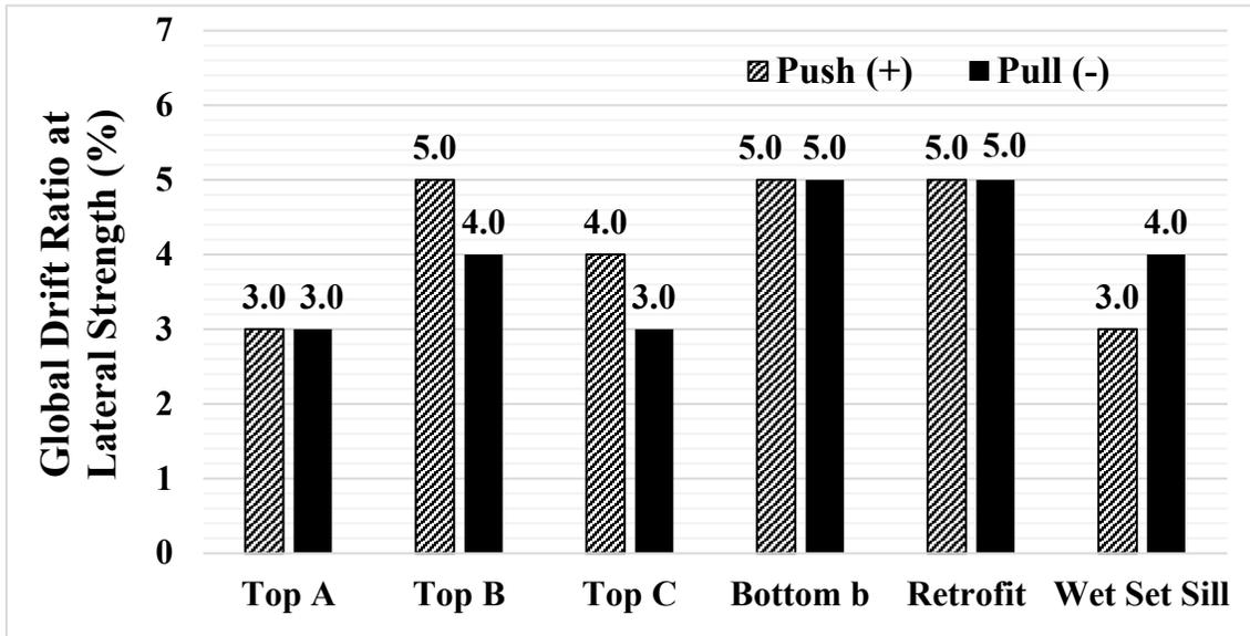
Figure 4.19 Comparison of *global* drift ratio at lateral strength.
