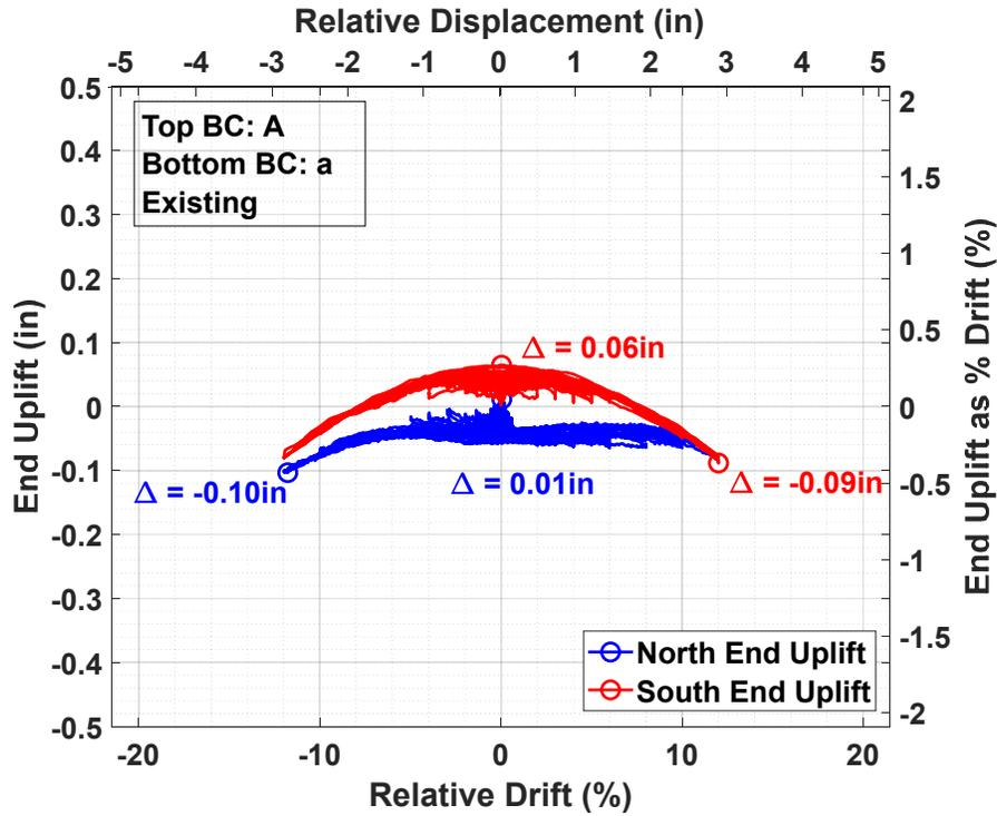
Figure C.21 Specimen A-1 end uplift versus relative drift.
