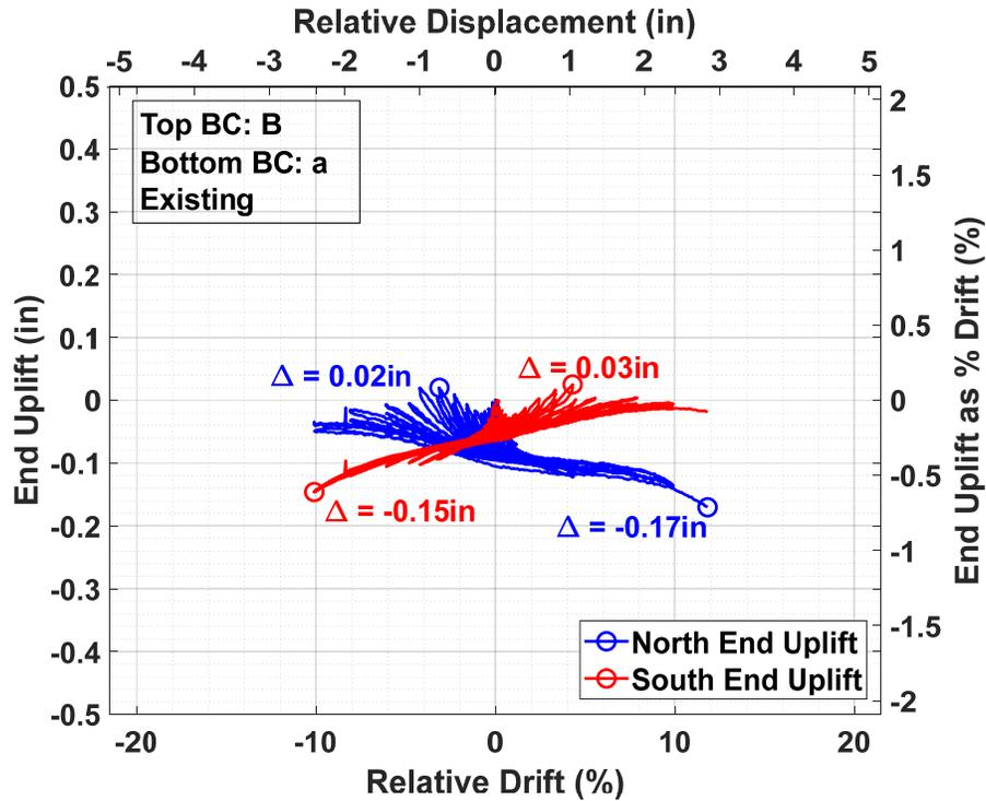
Figure C.22 Specimen A-3 end uplift versus relative drift.
