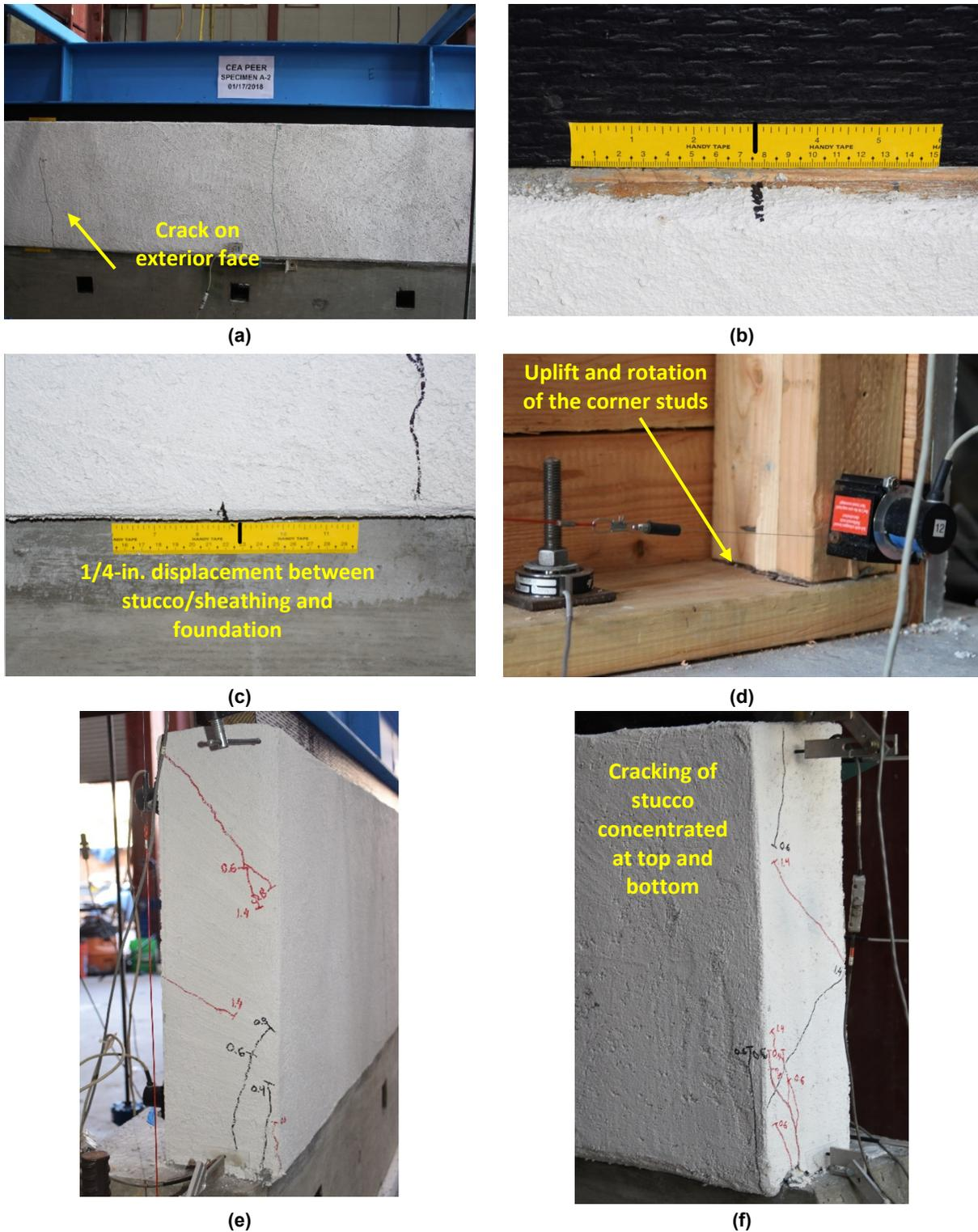
**Figure 5.4** Specimen A-2 damage state at -1.4% drift @  $\Delta = -0.336$  in.: (a) exterior elevation; (b) top of exterior wall; (c) bottom of exterior wall; (d) bottom corner of south-end interior; (e) north-end exterior corner view; and (f) north-end interior corner view.
