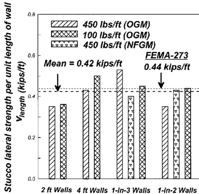
**Figure 1.14** Lateral strength contribution for walls with stucco finish (tests performed at UC Davis within the CUREE-Caltech Woodframe project) [Chai et al. 2003].
