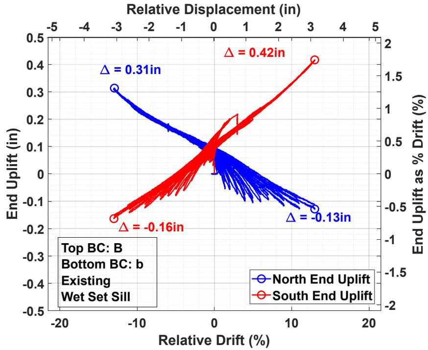
Figure C.26 Specimen A-6 end uplift versus relative drift.
