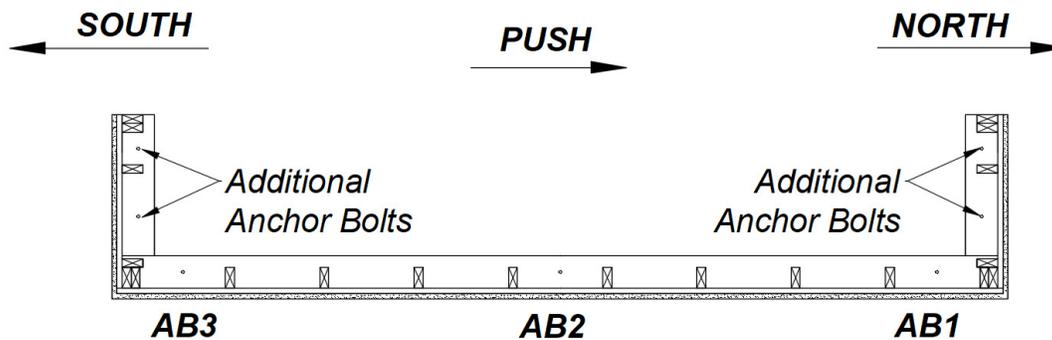
Figure 4.36 Specimen A-3: plan view anchor bolt layout.
