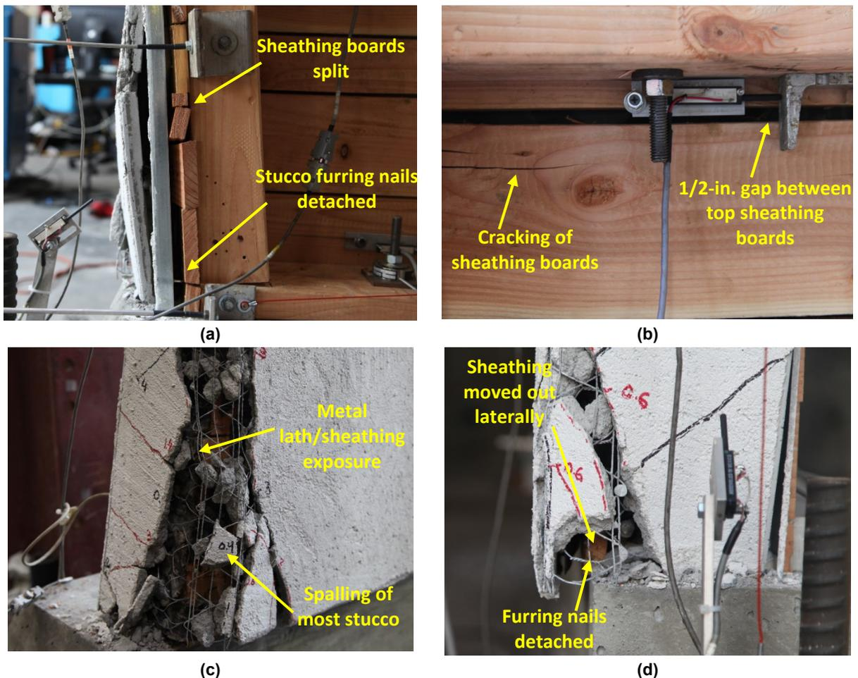
**Figure 5.21** Specimen A-2 damage state at 70% post-peak reduction of lateral strength @ +12% drift,  $\Delta = +2.88$  in.: (a) north-end of interior corner bottom; (b) close-up of top of interior wall; (c) south-end of exterior bottom corner; and (d) north-end of bottom corner.
