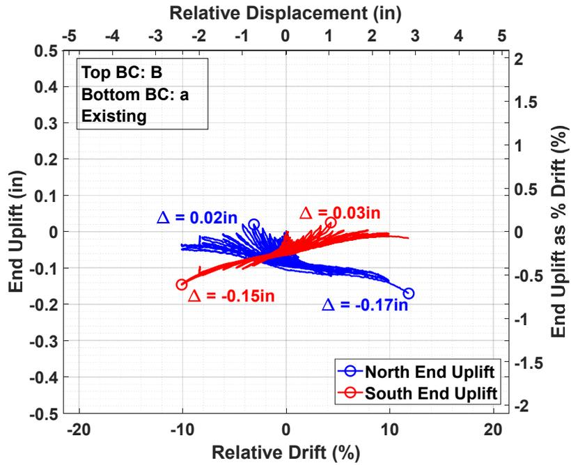
Figure 4.49 Specimen A-2 end uplift versus *relative* drift.
