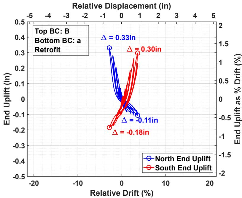
Figure 4.50 Specimen A-5 end uplift versus *relative* drift.
