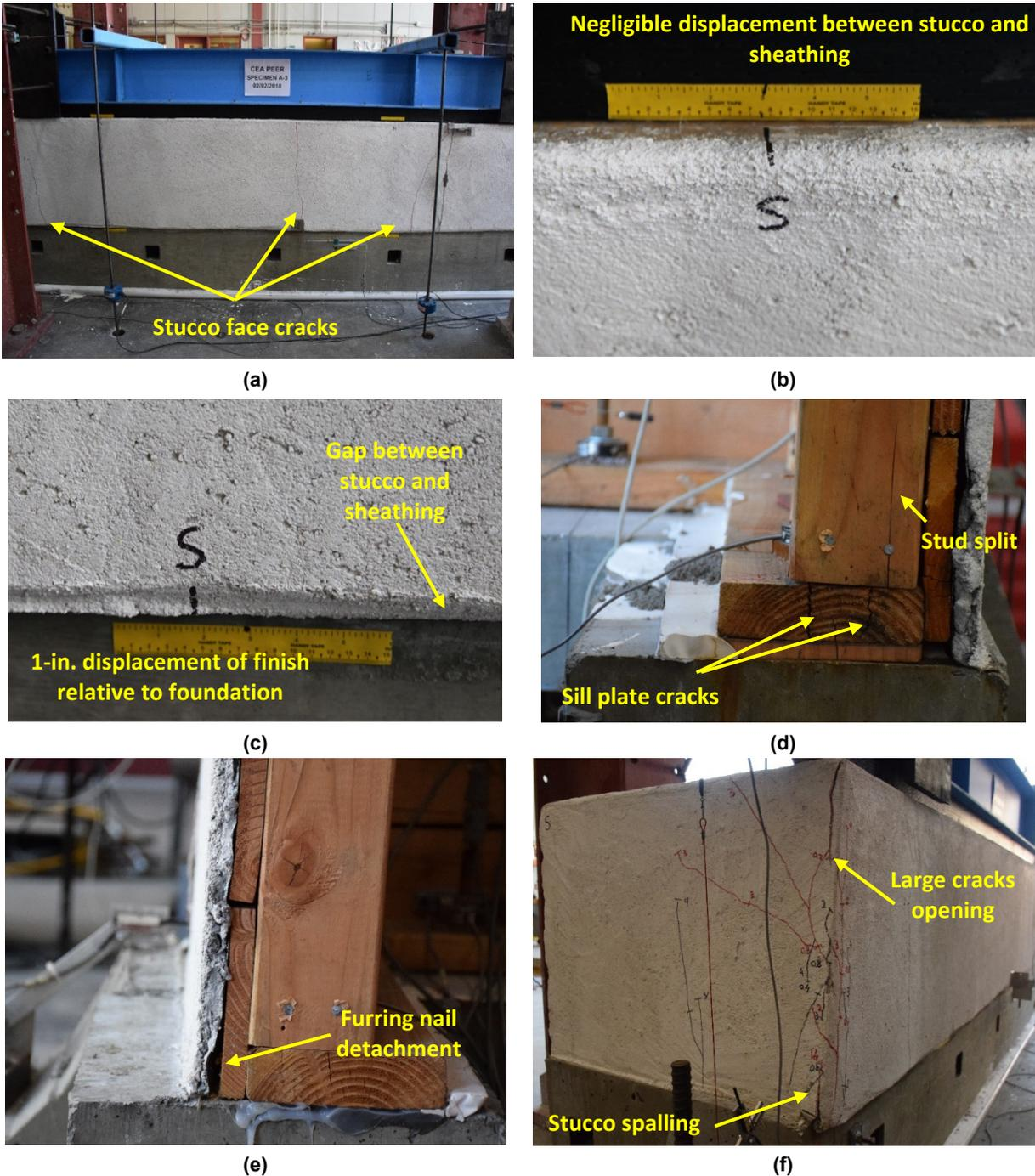
**Figure 5.15** Specimen A-3 damage state at lateral strength @ +4% drift,  $\Delta = +0.96$ : (a) exterior elevation; (b) top of exterior wall (c) bottom of exterior wall; (d) close-up of south-end wall; (e) close-up of north-end corner of wall; and (f) north-end exterior corner.
