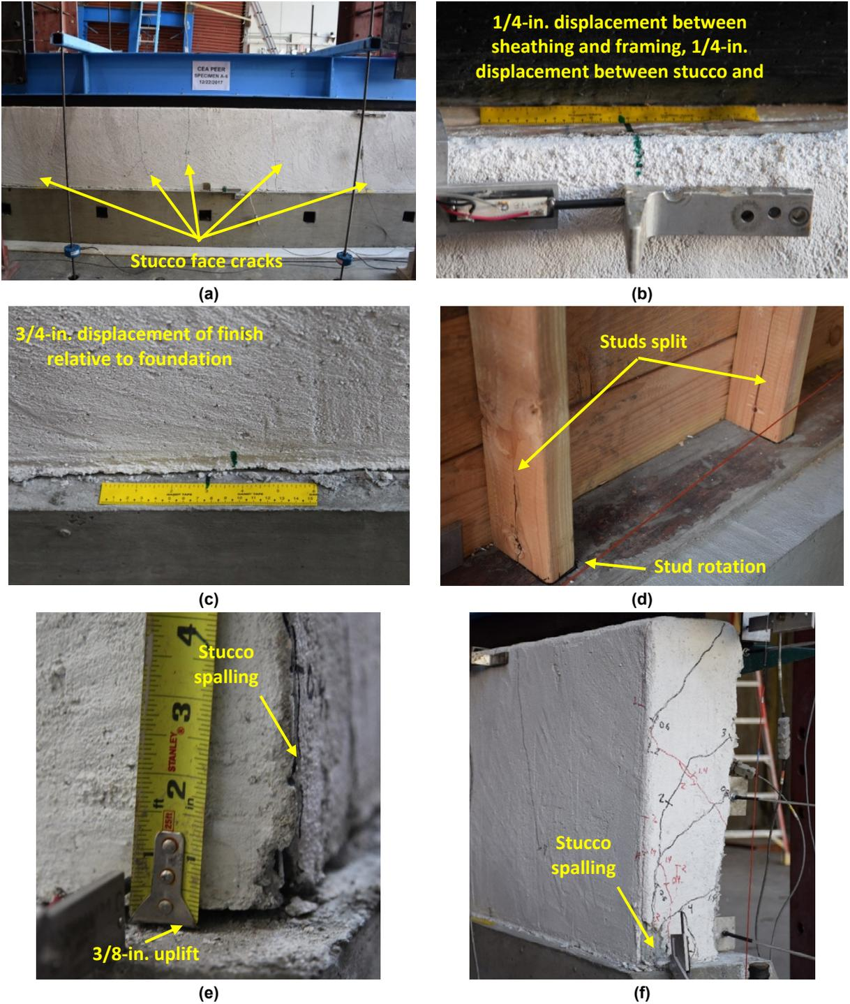
**Figure 5.18** Specimen A-6 damage state at lateral strength @ +3% drift,  $\Delta = +0.72$  in.: (a) exterior elevation; (b) top of exterior wall; (c) bottom of exterior wall; (d) close-up of studs and sill plate; (e) close-up of south-end of exterior corner; and (f) north-end exterior corner.
