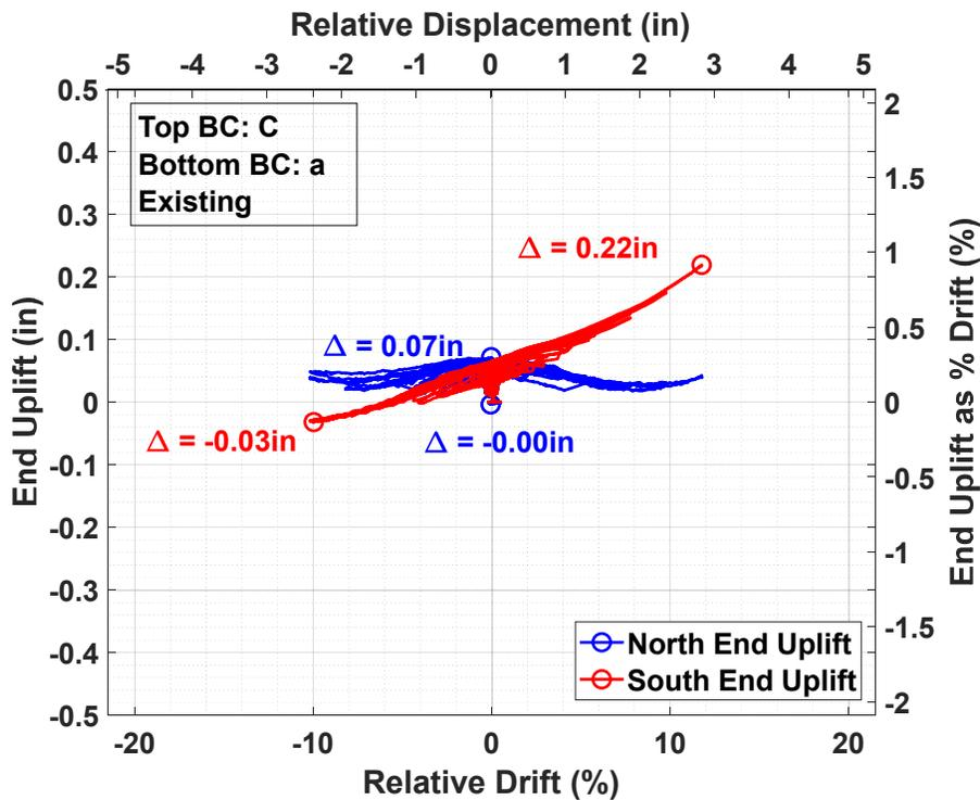
Figure C.23 Specimen A-3 end uplift versus relative drift.
