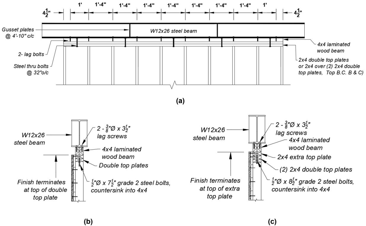
**Figure 3.34 Steel beam connections: (a) elevation of steel beam connection; (b) top of wall detail for stucco over horizontal sheathing for top boundary condition A; and (c) top of wall detail for stucco over horizontal sheathing for top boundary condition B and top boundary condition C Horizontal steel beam to cripple wall connection details.**
