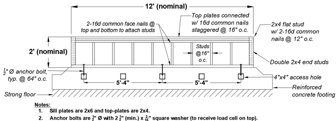
**Figure 3.1** Elevation of framing details of the interior face of the 2-ft-tall cripple wall Phase 1 test specimens. Note: the specimen height and length vary slightly due to modifications in the boundary conditions, which was a variable in Phase 1.
