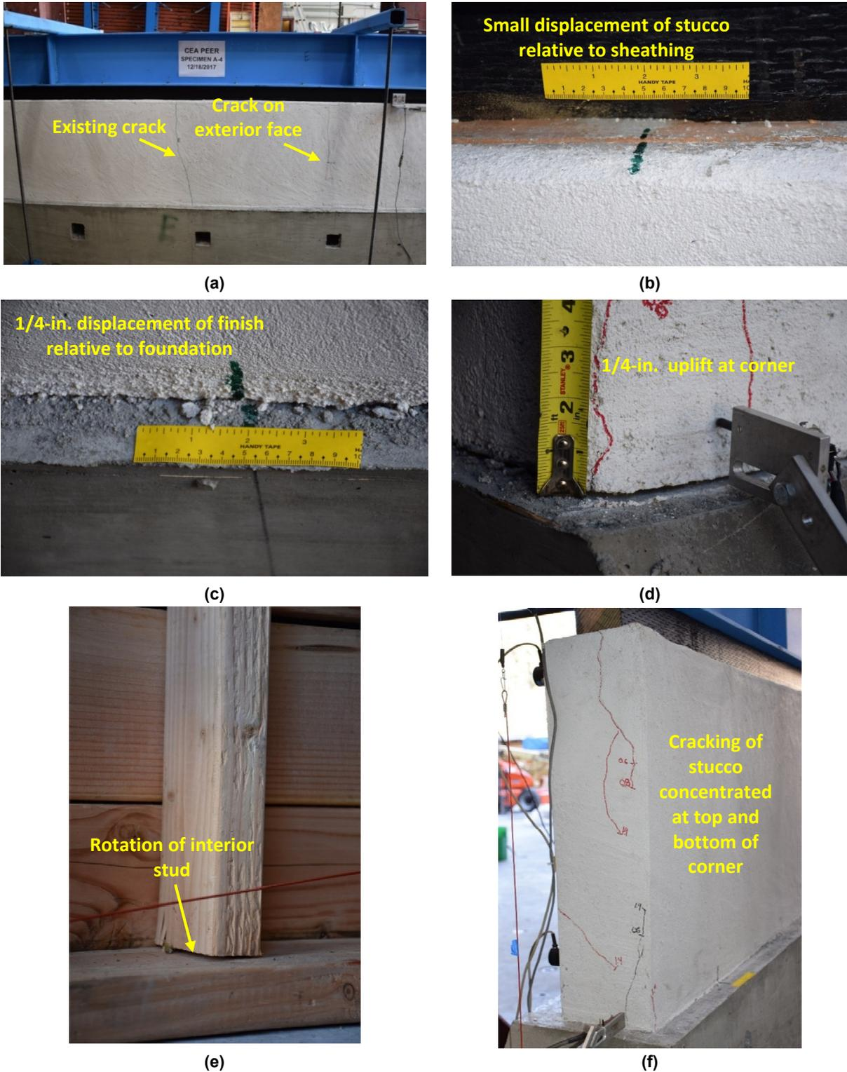
**Figure 5.8** Specimen A-4 damage state at -1.4% drift ( $\Delta = -0.336$  in.): (a) exterior elevation; (b) top of exterior wall; (c) bottom of exterior wall; (d) bottom of north-end exterior corner; (e) bottom of interior wall; and (f) north-end of exterior corner.
