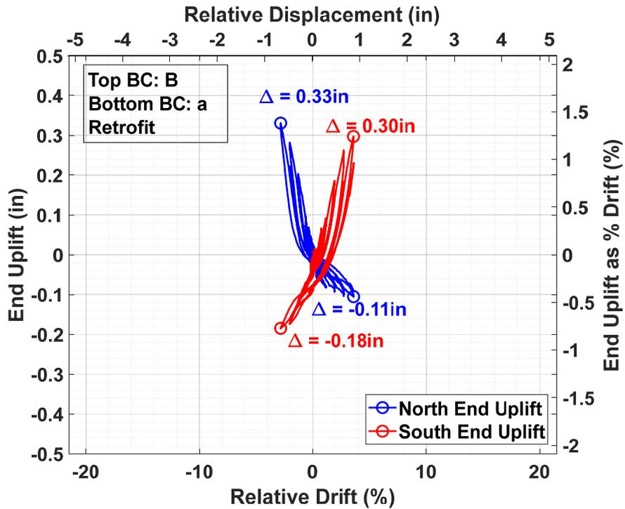
Figure C.25 Specimen A-5 end uplift versus relative drift.
