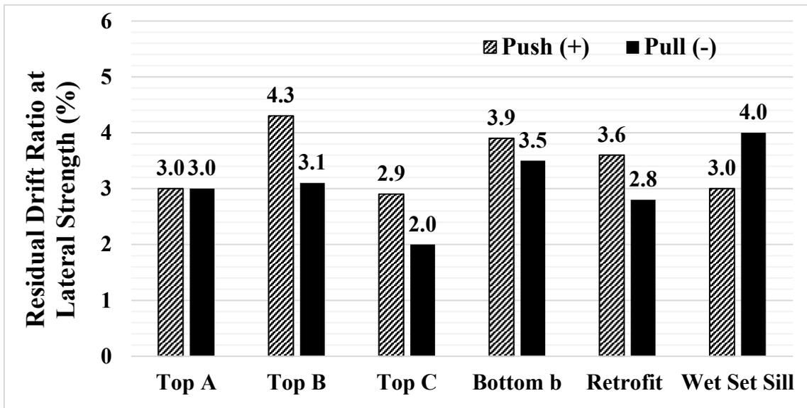
Figure 4.20 Comparison of *relative* drift ratio at lateral strength.
