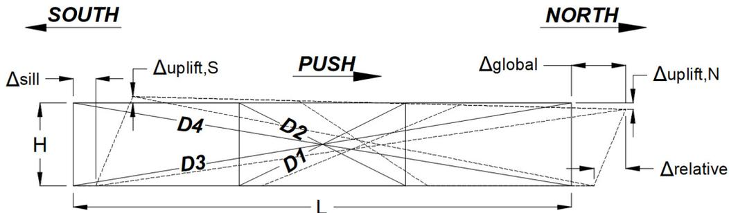
Figure 4.40 Deformed cripple wall with measurements used for resolving lateral displacement from diagonal and uplift measurements.
