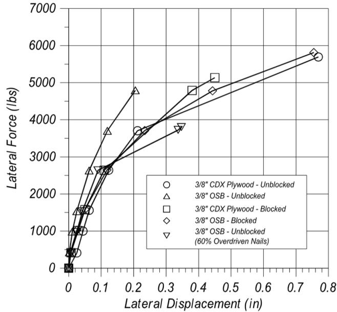
**Figure 1.9** Lateral strength envelopes for five level cripple walls tested by Steiner [1993] (figure courtesy of Chai et al. [2002]).
