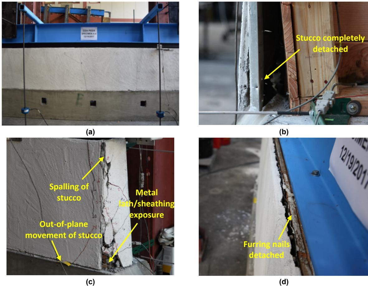
**Figure 5.25** Specimen A-4 damage state at 80% post-peak reduction of lateral strength @ -12% drift,  $\Delta = -2.88$  in.: (a) exterior elevation; (b) bottom of north-end interior corner; (c) north-end exterior corner; and (d) bottom of north-end corner.
