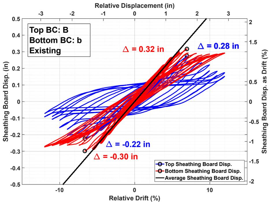
Figure C.30 Specimen A-4 top and bottom sheathing board displacements versus relative drift.
