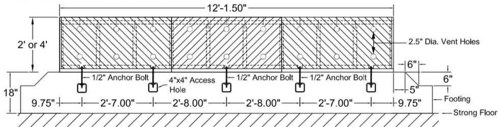
**Figure 1.10 Level cripple wall details tested at UC Davis within the CUREE-Caltech Woodframe project [Chai et al. 2002].**
