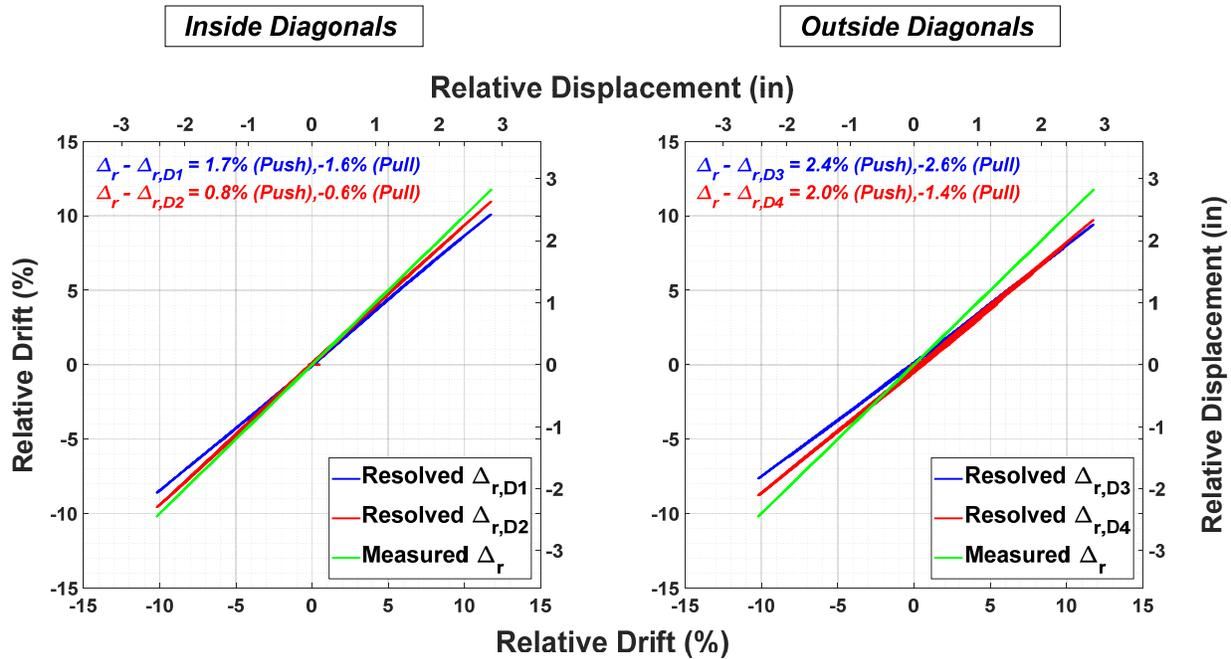
Figure C.14 Specimen A-3 resolved relative drift from diagonal measurements (outside and inside diagonals) versus measured relative drift.
