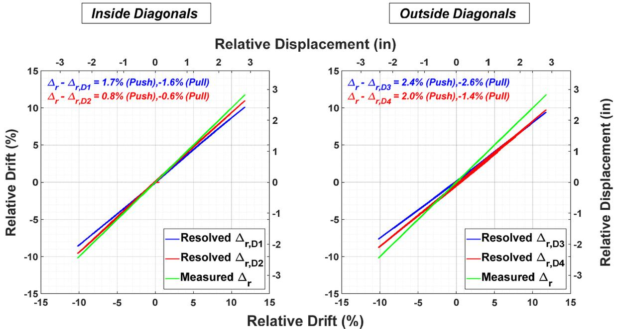
**Figure 4.46** Specimen A-3 (unretrofitted, top boundary condition C): resolved *relative drift* from diagonal measurements (outside and inside diagonals) versus measured *relative drift*.
