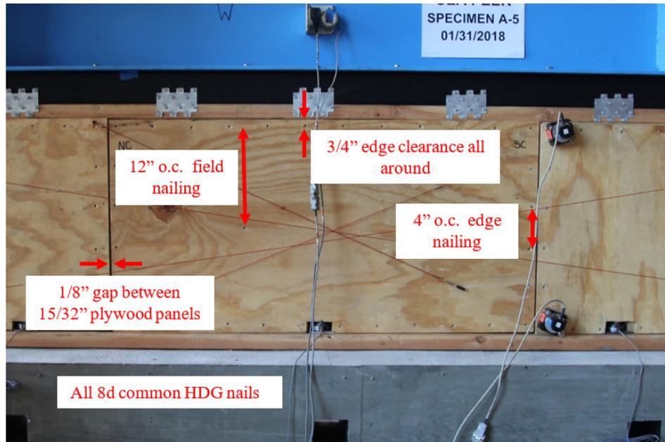
**Figure 3.31 Specimen A-5 retrofit plywood panel attachment.**
