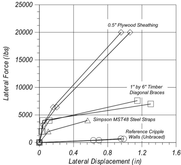
**Figure 1.7** Lateral load-deflection results from testing of [Sheperd and Delos-Santos 1991] five retrofitted and two “as-built” 2-ft-tall × 16-ft-long cripple walls (figure courtesy of Chai et al. [2002]).
