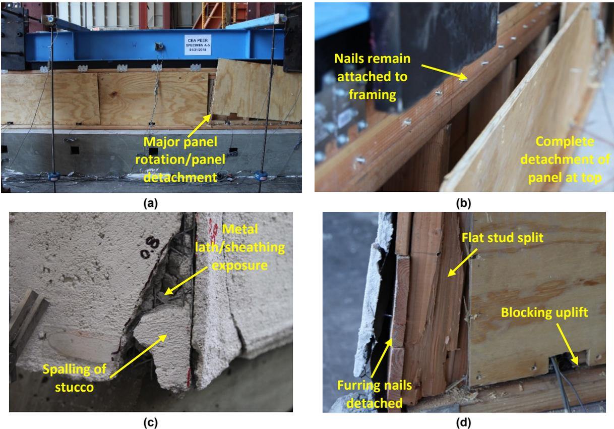
**Figure 5.27** Specimen A-5 damage state at 80% post-peak reduction of lateral strength @ -11% drift,  $\Delta = -2.64$  in.: (a) interior elevation; (b) top-down view of interior; (c) close-up of exterior south-end corner; and (d) close-up of interior north-end corner.
