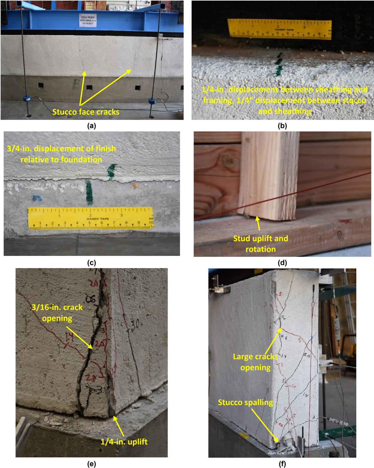
**Figure 5.16** Specimen A-4 damage state at lateral strength @-5% drift,  $\Delta = -1.20$  in.: (a) exterior elevation; (b) top of exterior wall; (c) bottom of exterior wall; (d) close-up of stud; (e) close-up of exterior south-end corner; and (f) north-end exterior corner.
