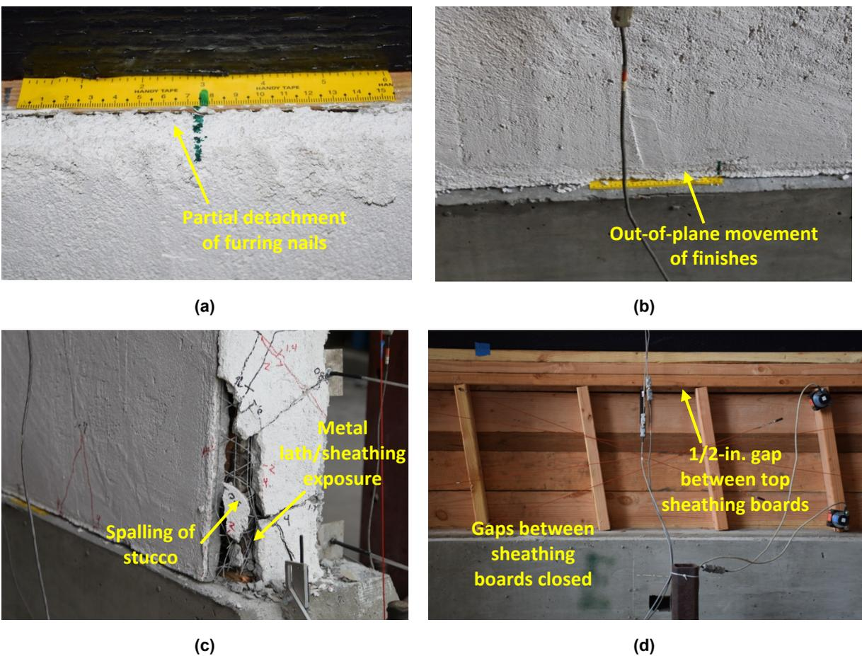
**Figure 5.29** Specimen A-6 damage state at 40% post-peak reduction of lateral strength @ +13% drift,  $\Delta = +3.12$  in.: (a) close-up of top of exterior wall; (b) close-up of the bottom of the exterior wall; (c) the north-end bottom of the exterior corner; and (d) the interior of the wall.
