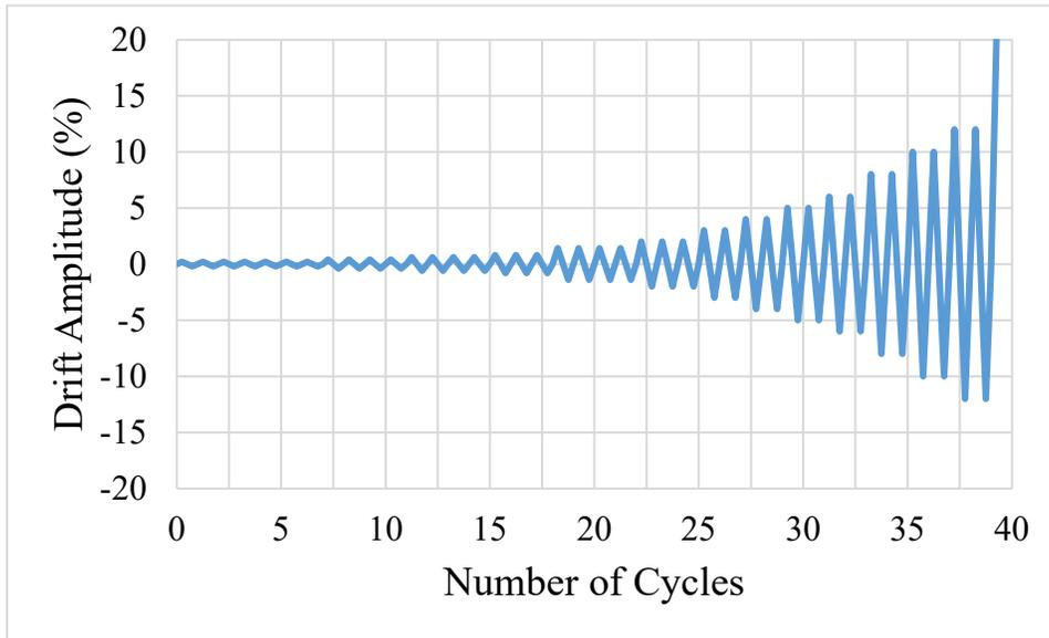
**Figure A.3 Specimen A-2 loading protocol.**
