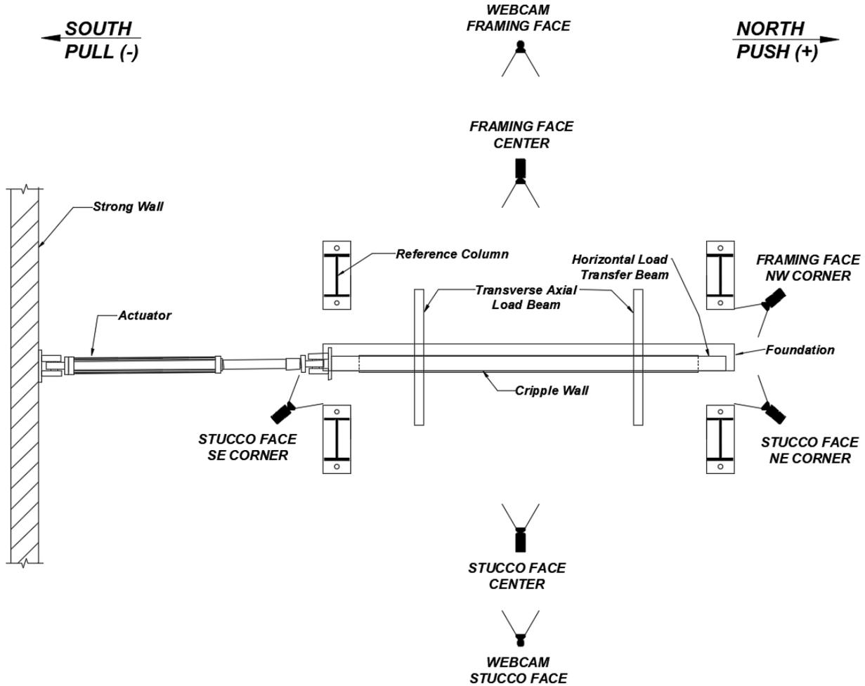
Figure 3.37 Plan view of typical camera layout.
