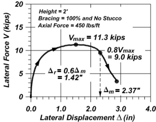
**Figure 1.12** Reference displacements from the monotonic tests of a 2-ft-tall level cripple wall: tests performed at UC Davis within the CUREE-Caltech Woodframe project [Chai et al. 2002] (specimen M, per Table 1.2).
