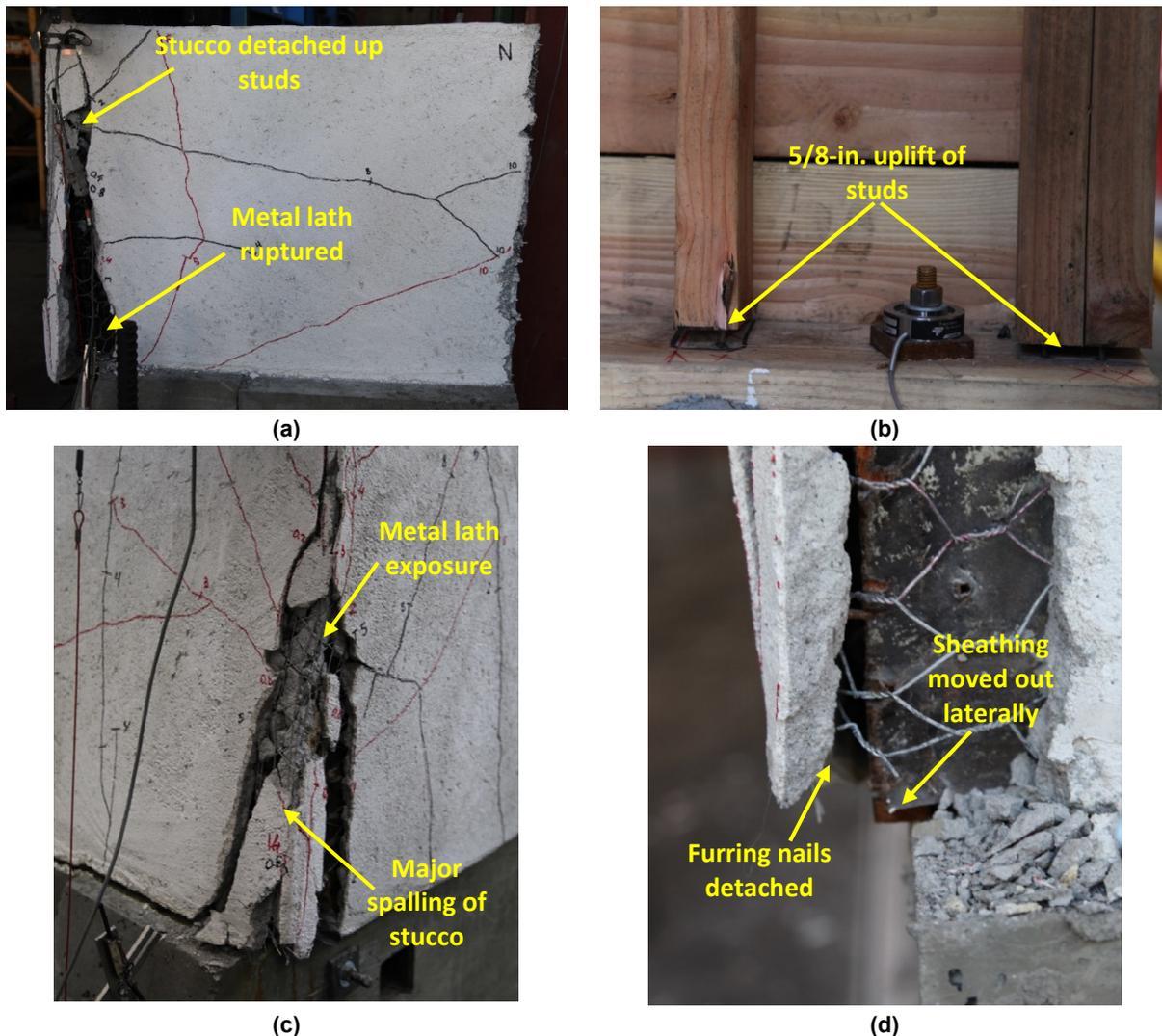
**Figure 5.23** Specimen A-3 damage state at 60% post-peak reduction of lateral strength @ -12% drift,  $\Delta = -2.88$  in.: (a) exterior view of north-end return wall; (b) interior of bottom of south-end return wall; (c) bottom of south-end exterior corner; and (d) bottom of north-end corner.
