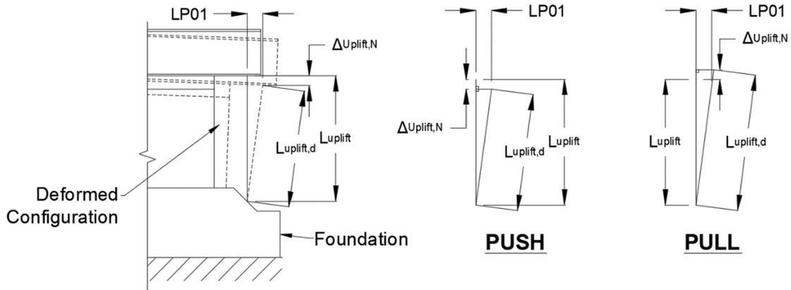
**Figure C.8 Schematic for resolving end of wall uplift.**
