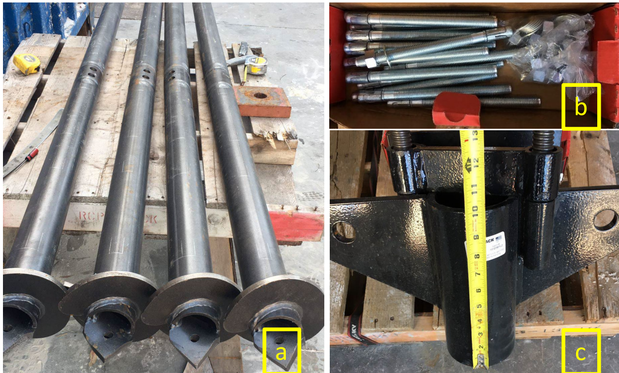
Figure 2.13 Photo of (a) single-helix helical piles, (b) bolts and nuts, and (c) side bracket used in Helical Pile tests.
