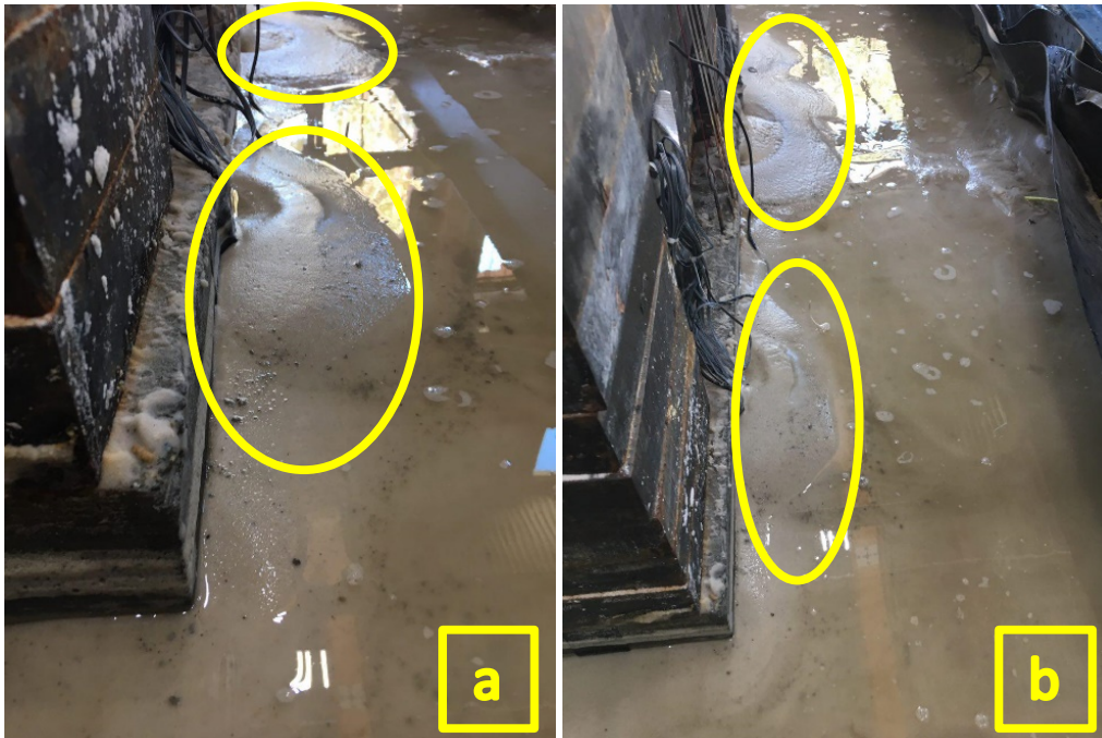
Figure 3.23 Observed sand ejecta in both (a) eastern and (b) western side of the soil box in the Helical Pile test after Shake 1.
