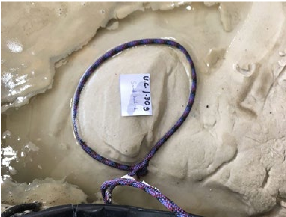
Figure 3.6 Observed sand ejecta after Shake 1-1 (Baseline test).
