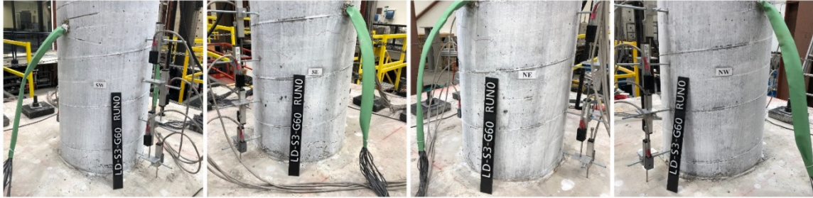
Figure 4.1 Column LD-S3-G60 before starting the test.
