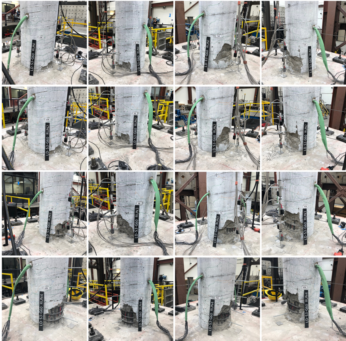
Figure 4.4 Column LD-S3-G60: progression of damage after each run.
