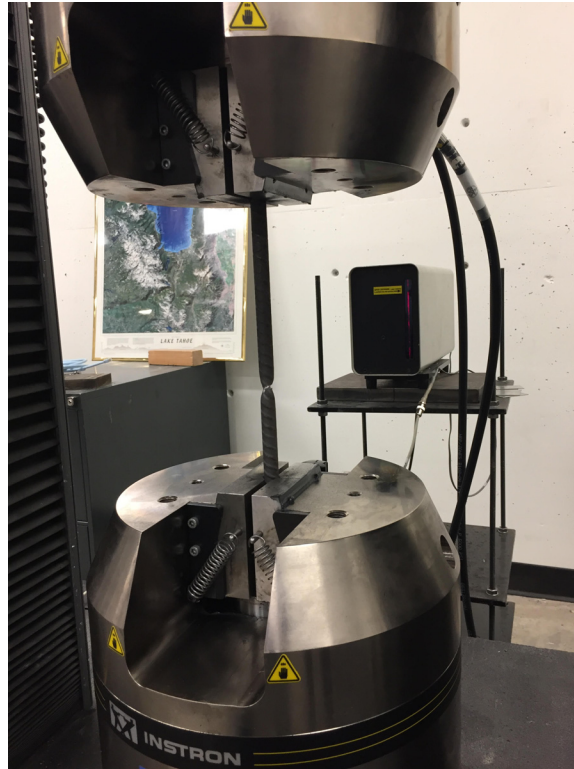
Figure 3.3 Reinforcing bar tensile test setup.
