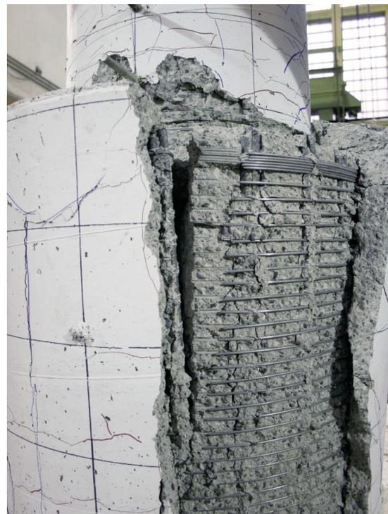
**Figure E.3** Close-up photographs of shaft transverse reinforcement fracture (at end of test): (a) uppermost spiral fracture on southwest side; and (b) Line of spiral fracture on southside.
