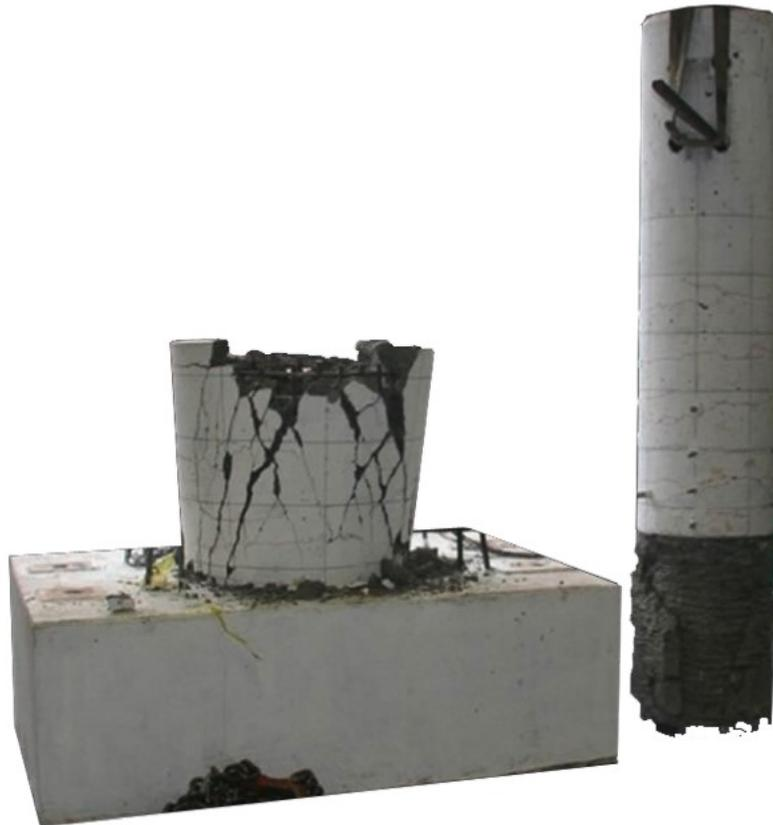
**Figure 2.10** Photograph of post-test damage in Specimen DS-2 [Tran 2015].
