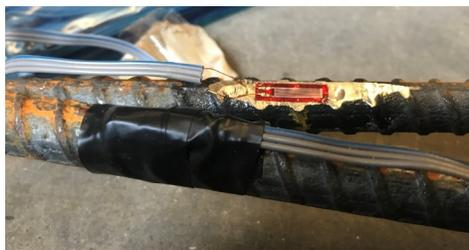
Figure 4.5 Photograph of two strain gauges at different stages of installation.
