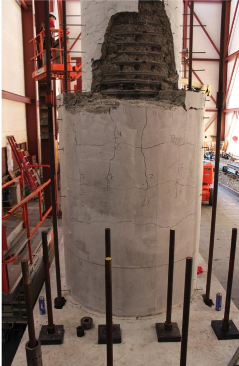
Figure 2.6 Photograph of post-test damage in Specimen UCSD-2 [Murcia-Delso et al. 2013].
