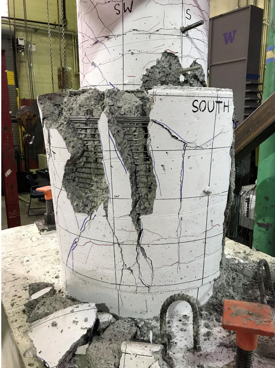
**Figure E.4** Southwest view of specimen (at end of test).
