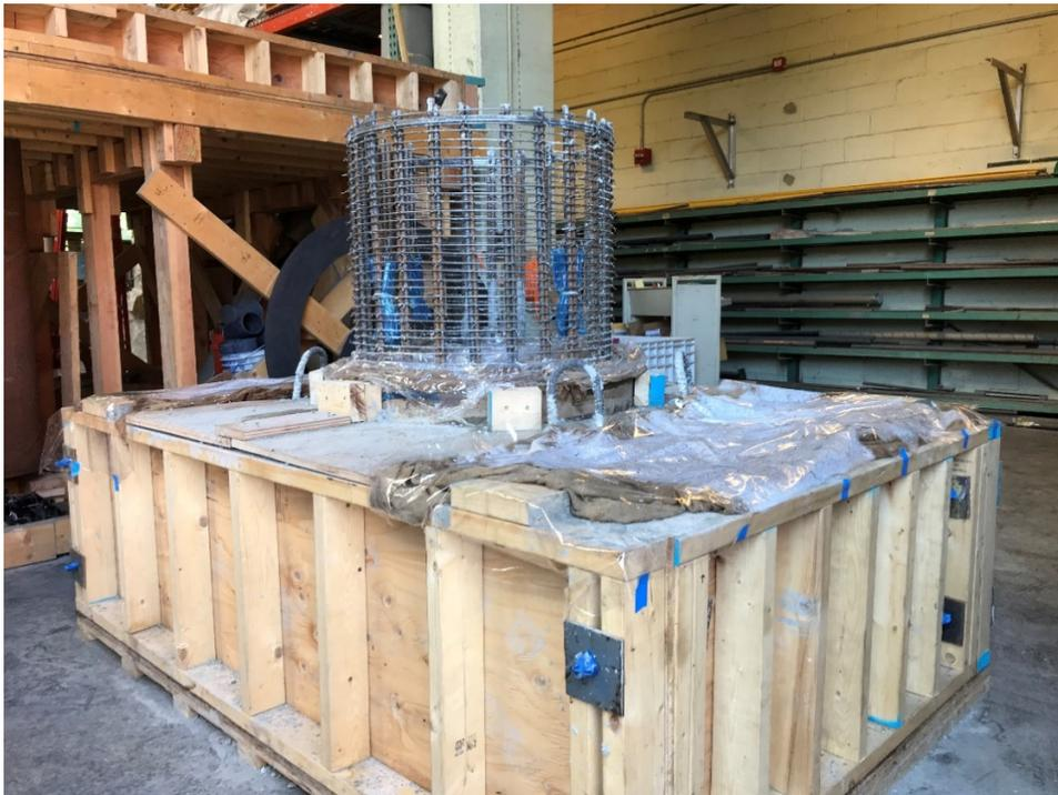
**Figure B.3** End of first concrete placement (base and shaft starter stub).
