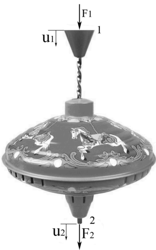
Figure 1.1: A physical realization of the inerter in which the force output is proportional only to the relative acceleration between nodes 1 and 2.
