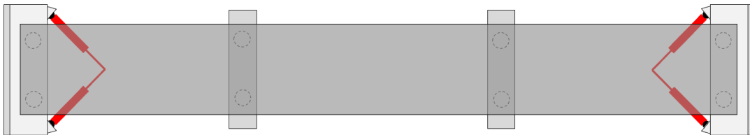
Figure 4.9 Plan view of viscous dampers location
