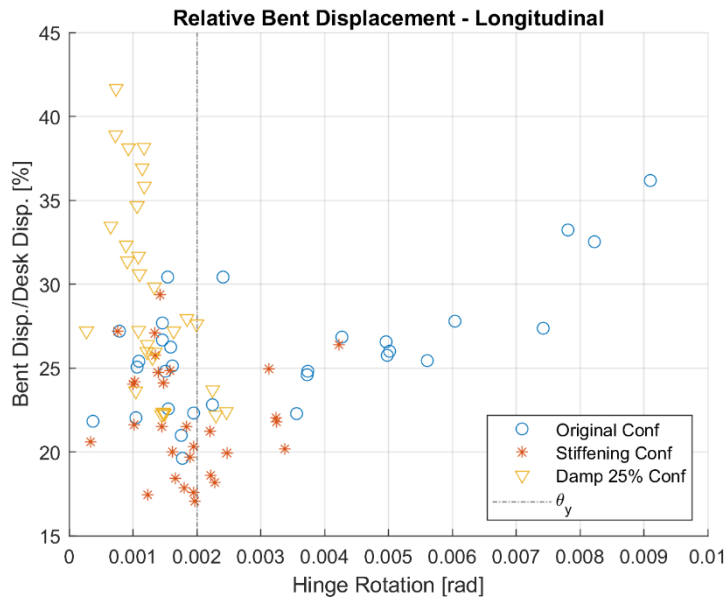
Figure 4.21 Relative bent deformation respect to the deck displacement for the three cases
