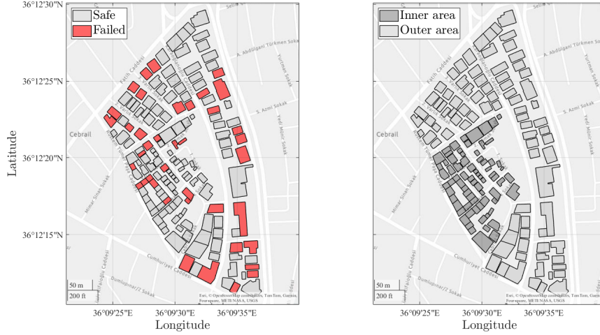
Figure 3: The building damage in a region of Antakya, Turkey, following the 2023 Turkey–Syria earthquake. Out of 156 buildings, 40 failed, including 14 out of 72 failing in the inner area and 26 out of 84 failing in the outer area. The inner and outer areas are defined in the right panel; this definition will facilitate the verification of the Ising model predictions.
