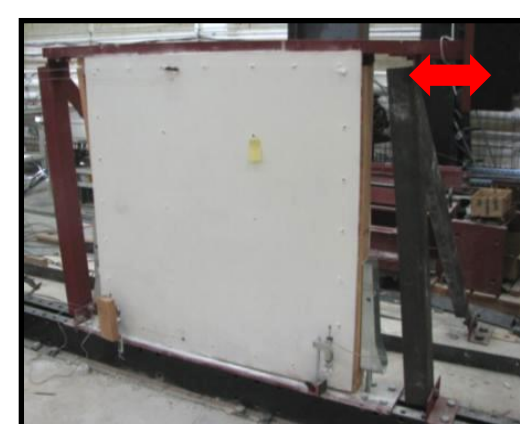
1.) 4ft x 4ft Wall Tests Setup
