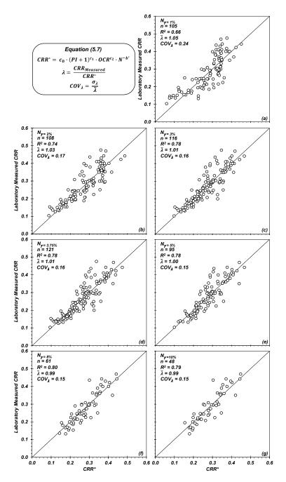
**Conclusions**: The models developed in this study may be used by practitioners and researchers to estimate cyclic resistance of intact non-plastic and plastic silt soils and corresponding factor of safety against cyclic failure for a range in cyclic shear strain failure criteria, to plan cyclic laboratory testing programs, and to calibrate models for use in site response and nonlinear deformation analyses in the absence of site-specific cyclic test data.
