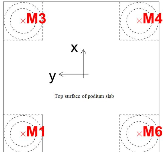
Figure 1. Specimen with markers for displacement measurements.
