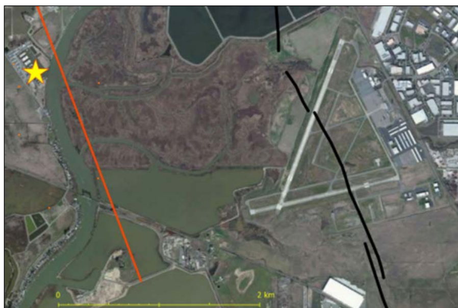
Figure 38 Napa airport with inferred fault trace in red (epicenter star), and mapped trace of W. Napa fault in black.
