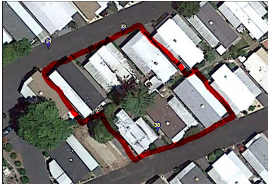
Figure 47 (l) NVMHP Park and locations of fires, 24 Aug 2014 S. Napa M_w 6.0 Earthquake; (r) 317 Patty Way fireground, showing locations of photos 31, 33, 38 in Figs. 3 and 4 (damaged buildings outlined in red)
