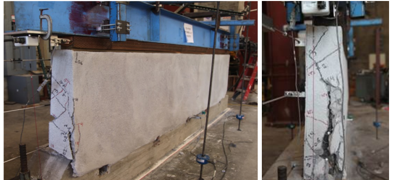
Figure 8. Laboratory tests for assessing the strength and flexibility of a stucco-covered crawlspace wall.
