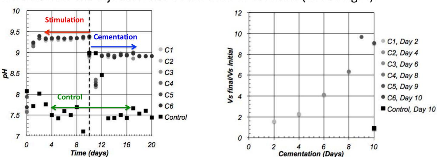
The pH of effluent solutions were shown to reach 9.0 within 2 days of treatment indicating high ureolytic activity. Effluent pH was also shown to decrease following the addition of calcium during cementation (above left). Normalized shear wave velocity increased with time as expected (above right).
