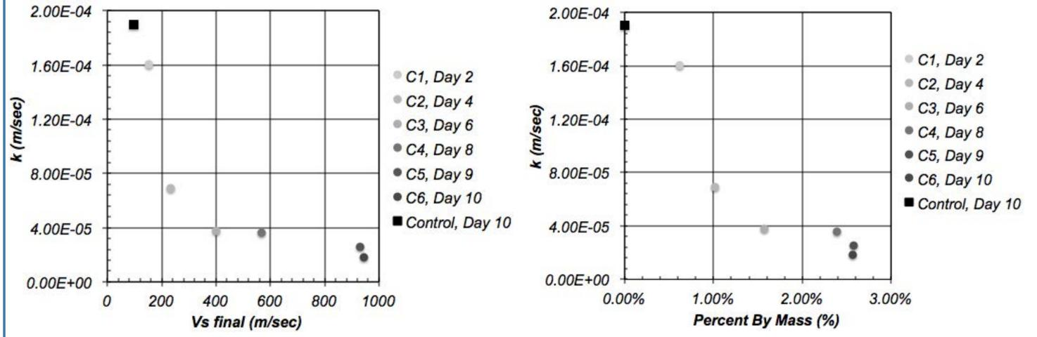
Permeability was shown to reduce with Vs due to calcite precipitation which reduced porosity (above left). As was expected the permeability also decreased with increased calcite mass (above right).
