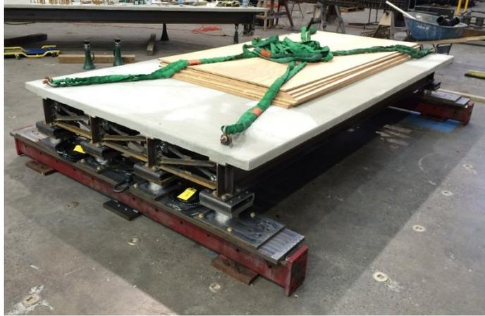
**Figure 2.1: Bridge with steel-bearings connected to the bent caps during the pre-assembly in the Large-Scale Structures Laboratory at the University of Nevada, Reno**
