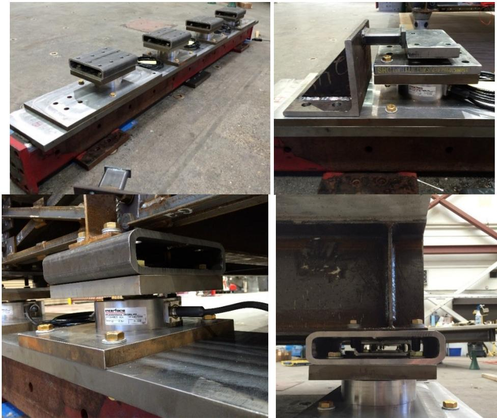
**Figure 1.5: Four steel bearings connected to the bent cap (top-left), shear-key in contact with the top plate of the elastomeric bearings (top-right), and details of the connections between the girders, steel bearings, load cells and bent cap (bottom), during the pre-test assembly in the Large-Scale Structures Laboratory at the University of Nevada, Reno**
