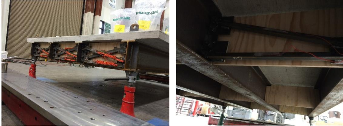
**Figure 4.2: I-girder Bridge with plywood diaphragms during the assembly in the Large-Scale Structures Laboratory at the University of Nevada, Reno**
