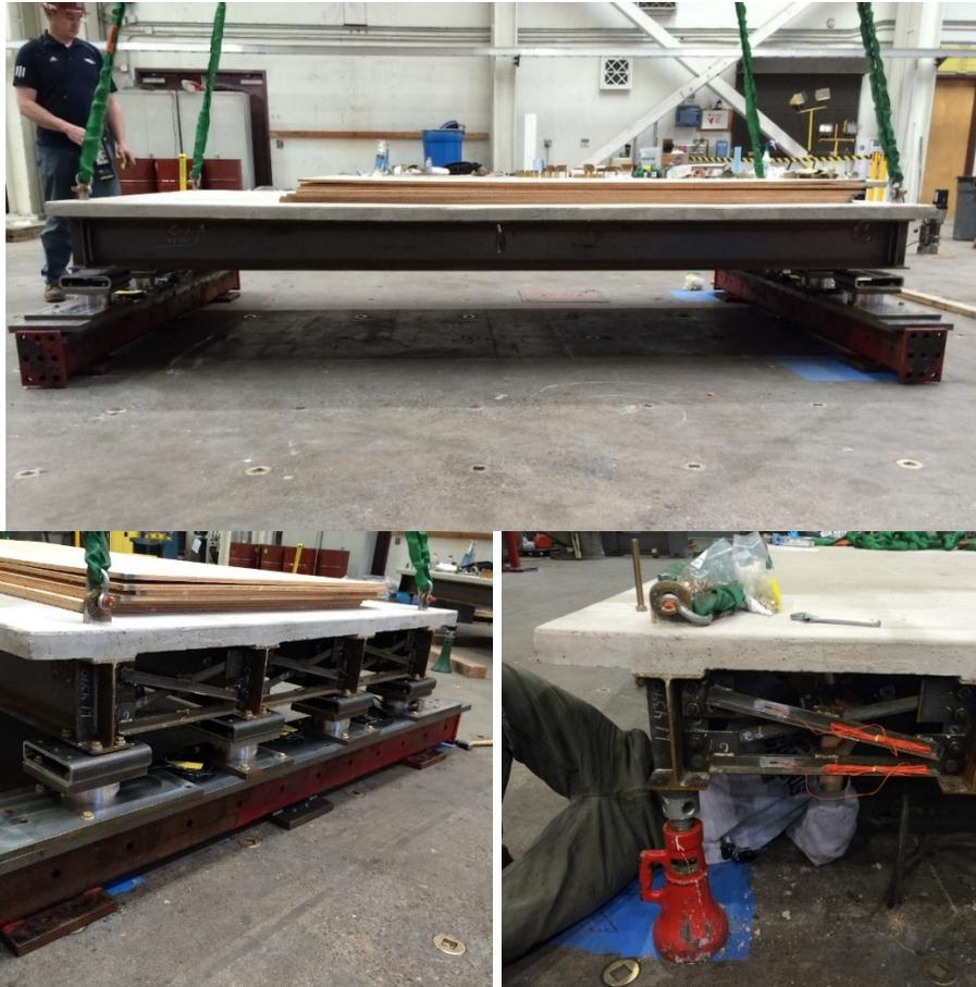
**Figure 1.6: I-girder bridge connected to the steel bent caps during the pre-test assembly (top and bottom-left) and instrumentation of cross-frames with strain gages**
