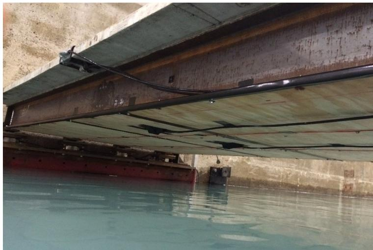
**Figure 5.3: Box-girder Bridge with attached instrumentation ready for testing in the O.H. Hinsdale Large Wave Flume at Oregon State University**
