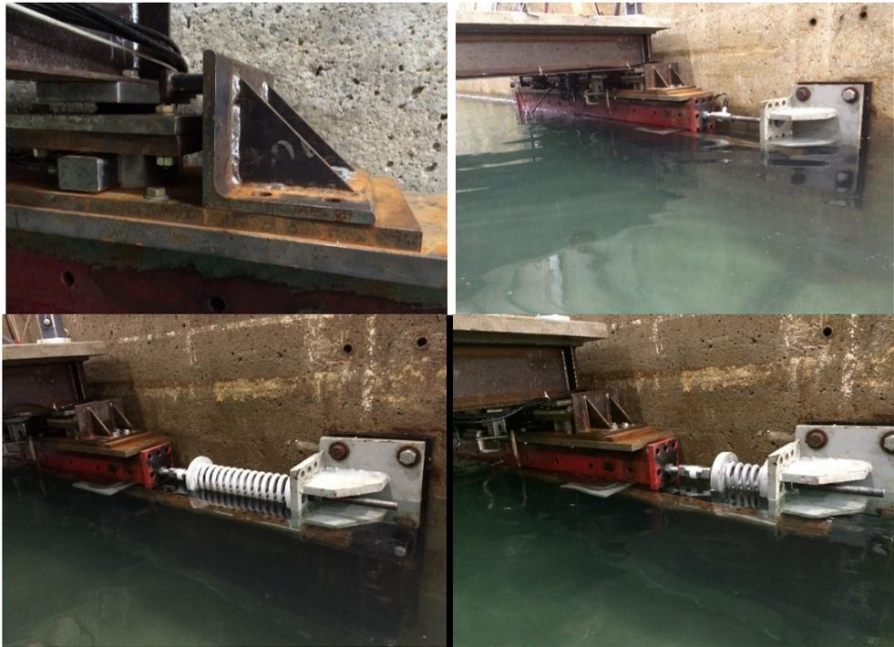
Figure 3.1: Details of the bearings, shear keys and substructure links used to study the effect of bridge flexibility and the role of dynamic FSI
