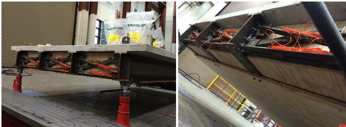
**Figure 5.1: Box-girder bridge during the pre-test assembly phase in the Large-Scale Structures Laboratory at the University of Nevada, Reno**
