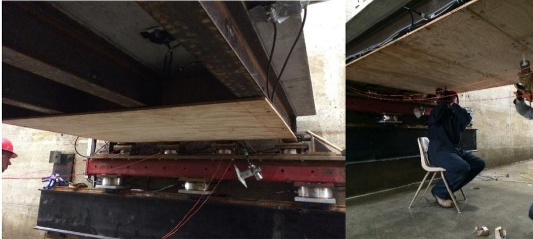
**Figure 5.2: Assembly of the box-girder bridge in the O.H. Hinsdale Large Wave Flume at Oregon State University**
