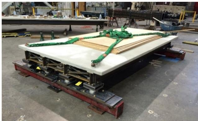
**Figure 4.1: I-girder Bridge with cross-frames during the assembly in the Large-Scale Structures Laboratory at the University of Nevada, Reno**
