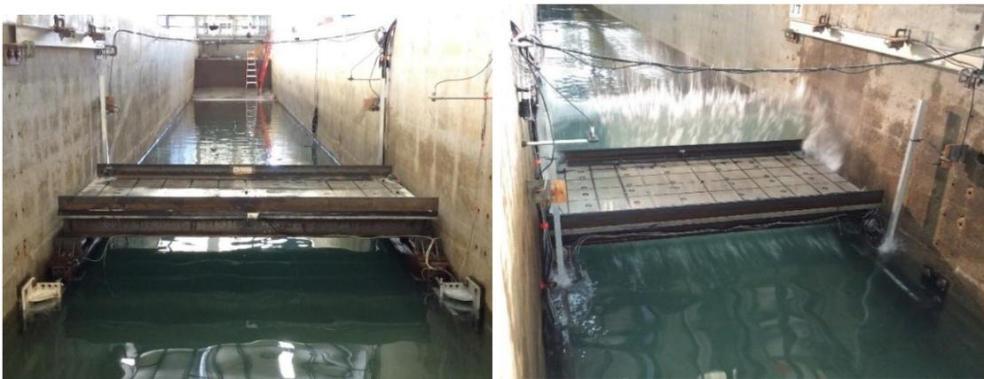
**Figure 7.1: Bridge with solid barriers during the hydrodynamic testing**
