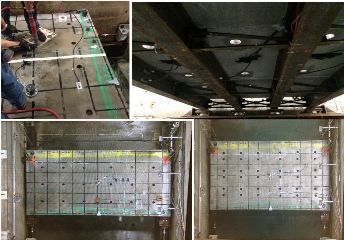
**Figure 6.1: Drilling of holes in the deck of the bridge (top-left), view of the bridge deck with air-vents (ST7) before the installation of the diaphragms, and plan view of the bridge case ST7 with 0.85% vented area (bottom-left) and bridge case ST9 with 1.70% vented area (bottom right)**
