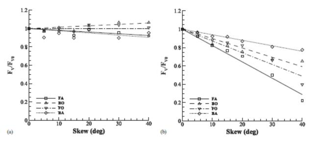
Figure 5.5: Effect of skew angle on vertical tsunami forces: (a) uplift impact and (b) downward steady state. (Image from Motley et al (2016)).
