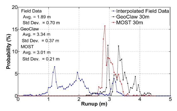
Figure 2.3: Comparison of the runup heights probability density functions between the interpolated field data, MOST and GeoClaw models.
