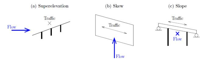
Figure 5.2: Three descriptors of bridge deck orientation: (a) superelevation, (b) skew, and (c) slope.
