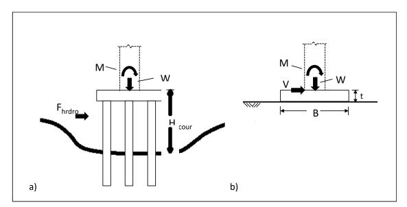
Figure 6.1: Tsunami induced foundation loading on a) deep foundations and b) shallow foundations.
