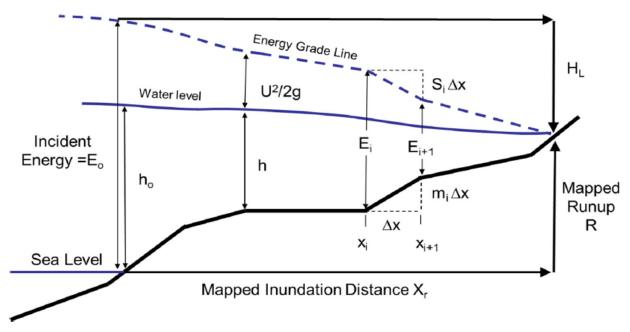
Figure 3.1: Illustration of energy method across inundated transect; incident tsunami flow is from left to right (from Kriebel et al., 2017).
