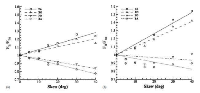
Figure 5.4: Effect of skew angle on horizontal tsunami forces: (a) impact and (b) steady state. (Image from Motley et al (2016)).
