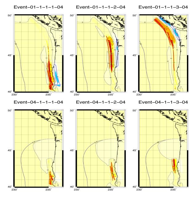
Figure 1.2: Vertical displacement field (res=uplift) for two scenarios. Top is a full rupture earthquake, bottom is a partial rupture, each shown three times with different asperity locations.
