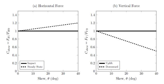
Figure 5.6: Modification of total bridge force, compared to the non-skew case, based on skew angle: (a) horizontal force, (b) vertical force.
