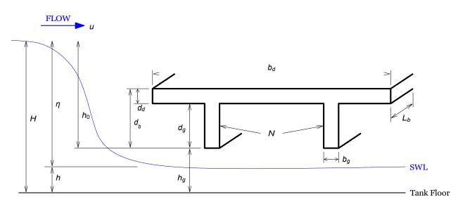
Figure 5.1: Variables that describe load estimation equations for deck-girder bridges.
