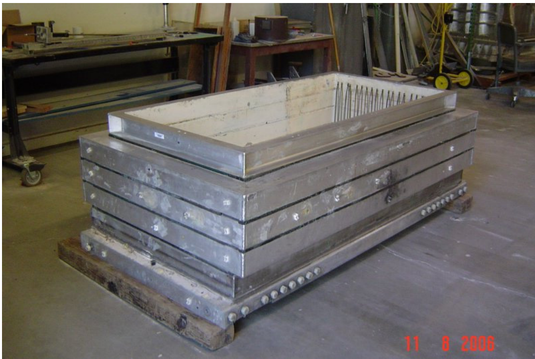
Fig. 3.1 Model container FSB2.
