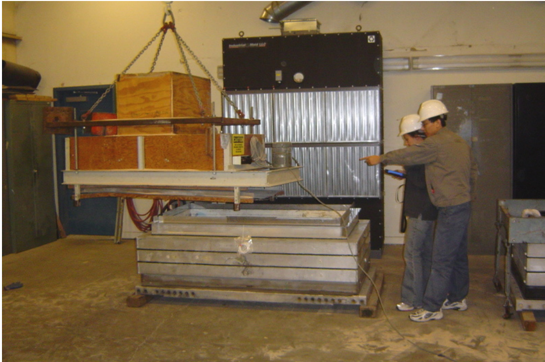
Fig. 3.9 Pluviation of sand inside model container.
