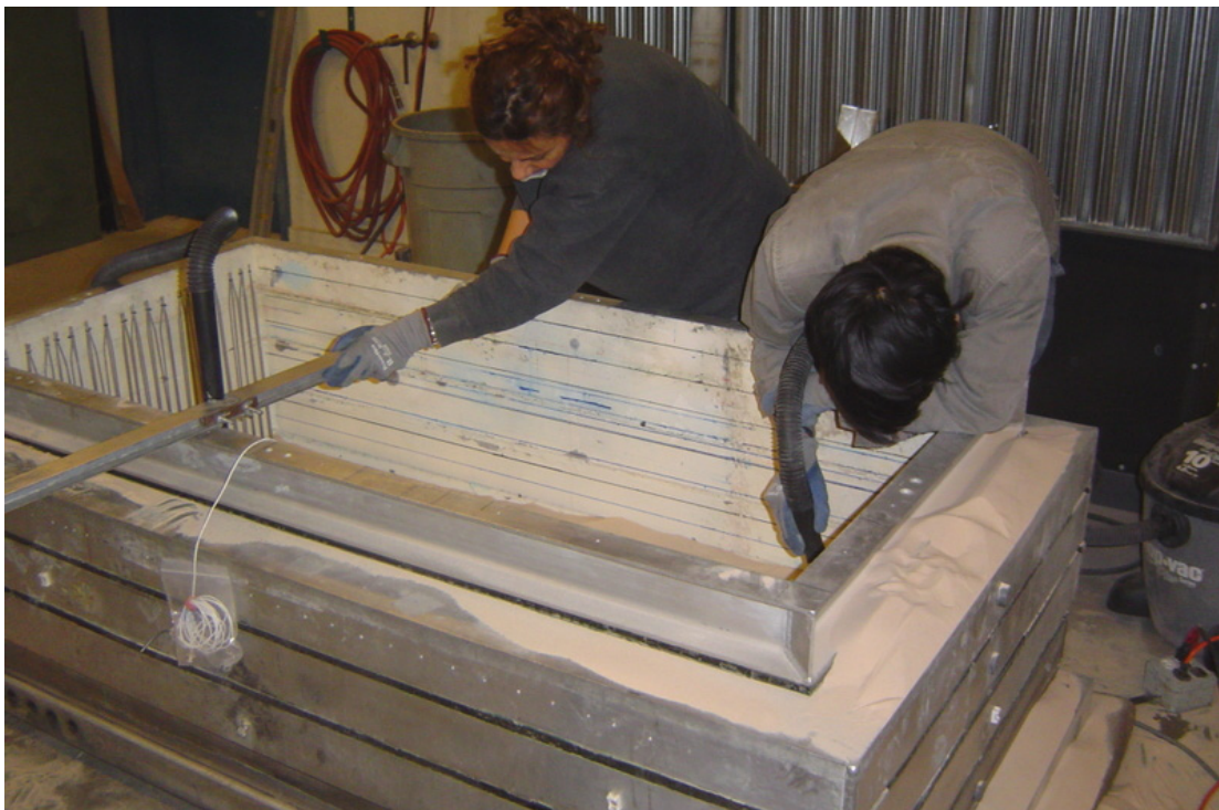
Fig. 3.10 Leveling sand surface with a vacuum.
