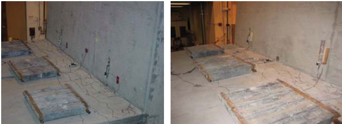
Figure 4-60 Observed cracking at 2.5% drift in Specimen 1 (left) and Specimen 2 (right).
