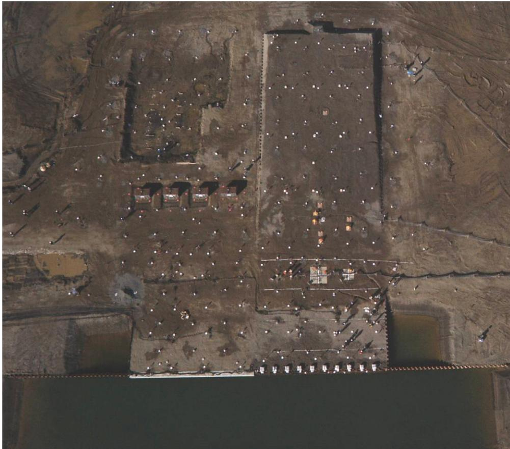
**Fig. 4.3 Aerial photo of first full-scale lateral spreading experiment (PARI 2002)**
