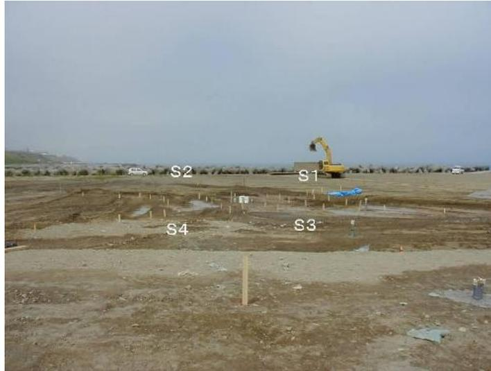
**Fig. 3.4 Photograph showing borehole locations for single borehole tests**
