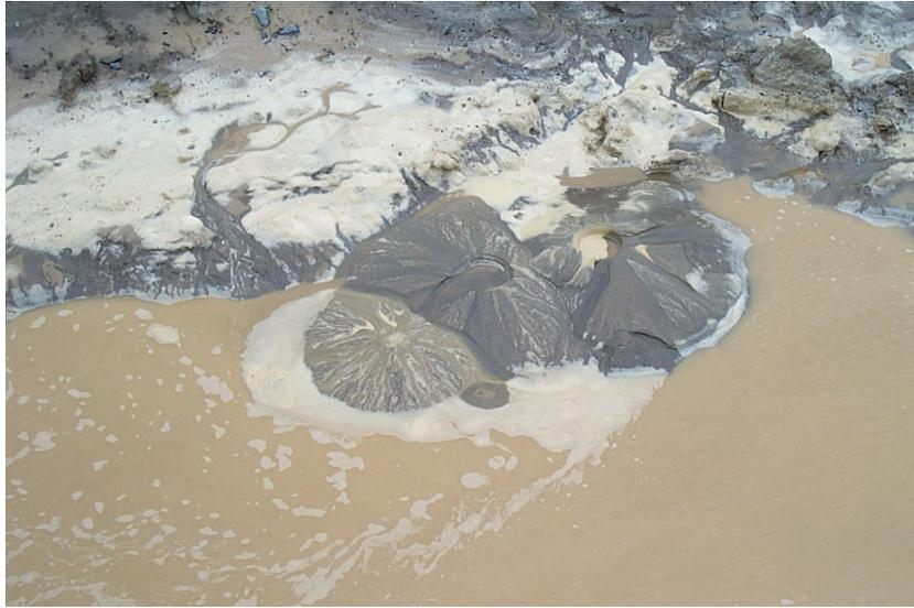
**Fig. 3.17 Sand boils observed following second pilot test**
