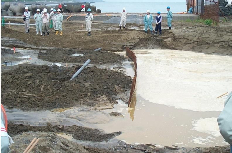
**Fig. 3.19 Lateral movement of sheet pile wall after the test**
