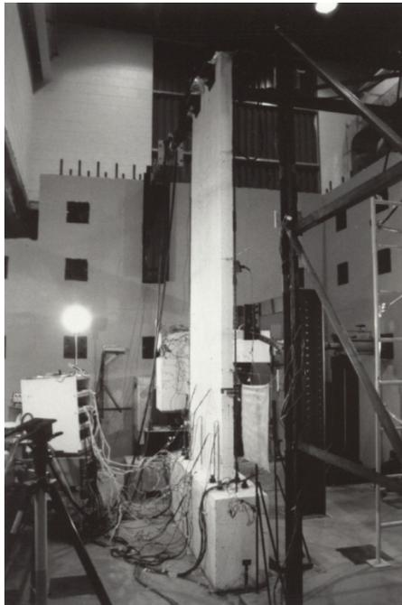
**Fig. 7.7 Photograph of test setup (Thomsen and Wallace, 1995)**
