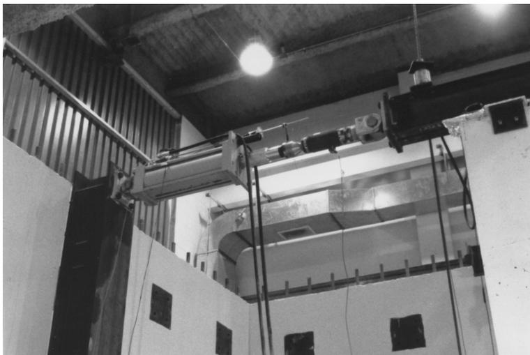
**Fig. 7.9 Hydraulic actuator**
