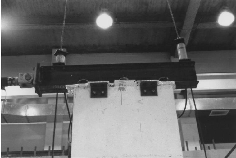
**Fig. 7.8 Load transfer assembly**
