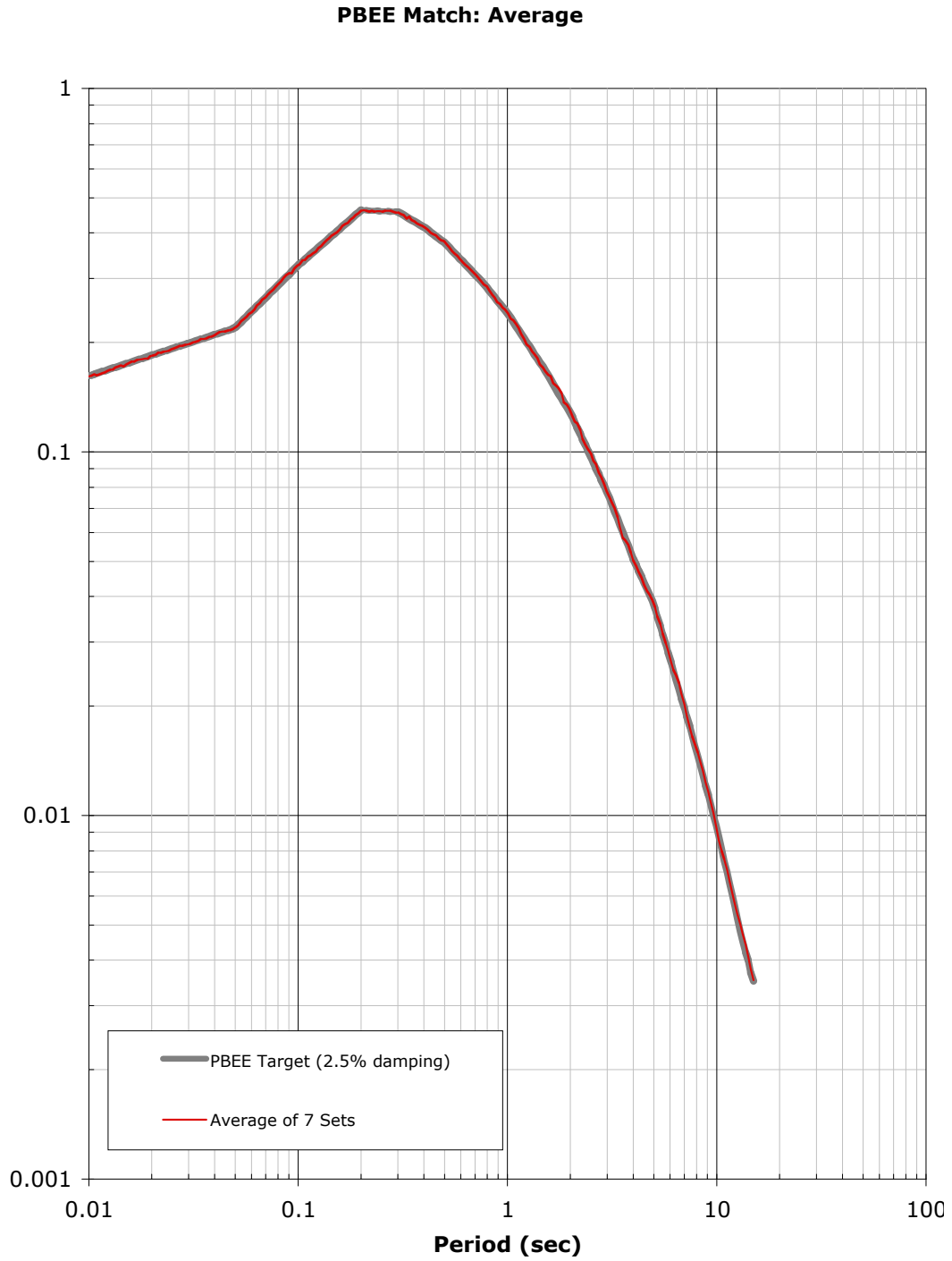
Figure 2.8 Comparison between the average modified spectrum compatible acceleration histories response spectrum for all 14 spectrum compatible histories and the target design response spectrum.
