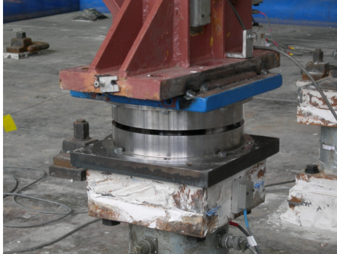
Figure 4.8: Photograph showing bearing connection at base of column, typical for all four columns and both DP and TP bearings
