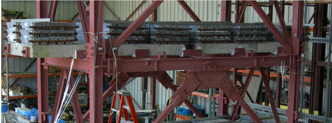
Figure 4.2: Photograph depicting attachment of floor ballast
