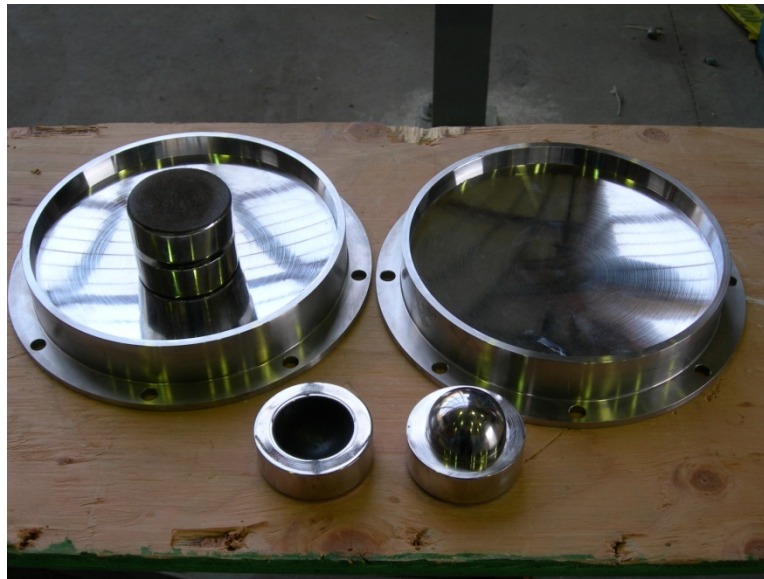
Figure 4.5: Photograph of a scale DP bearing, disassembled for clarification of each component
