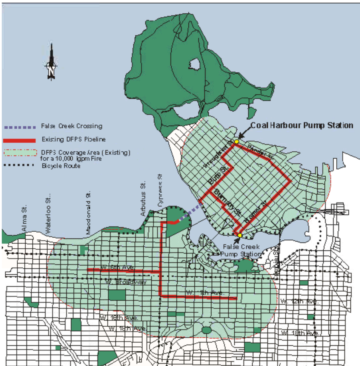
Figure 3.8 Plan of Vancouver, B.C. Dedicated Fire Protection System.
