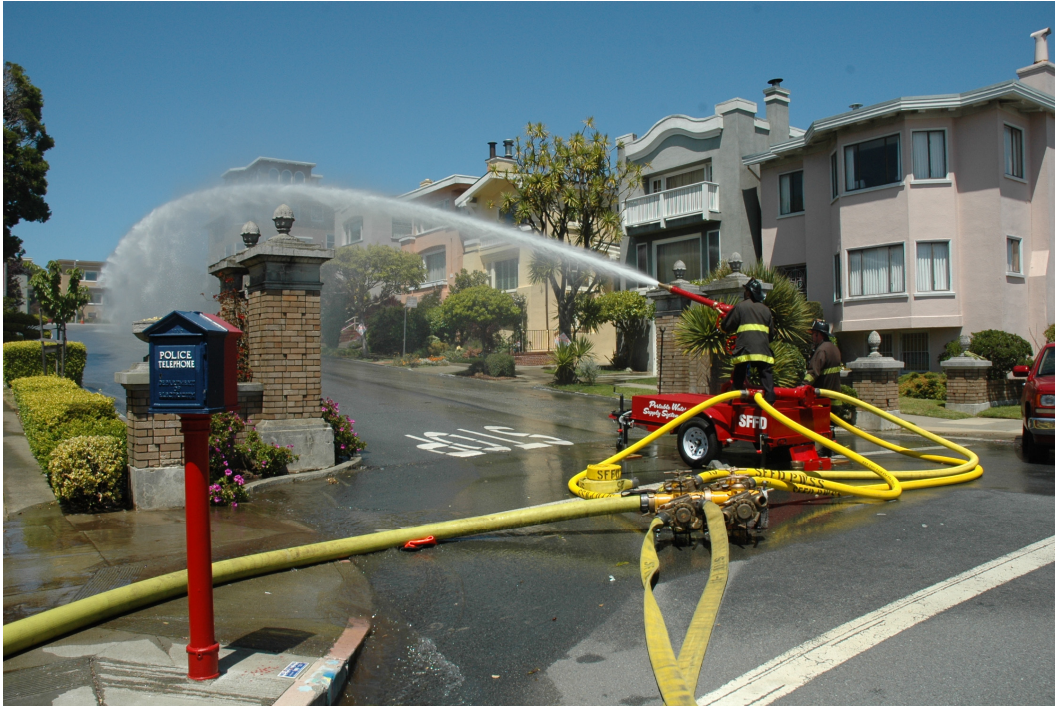
Figure C.1 SFFD portable monitor deploying a water curtain (source: http://sfearthquakesafety.org/the-bond/firefighting-water-supply-system/ ).
