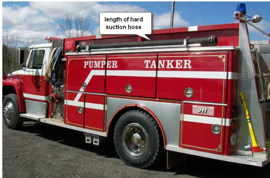
Figure 3.1 Illustration of a hard-suction hose.
