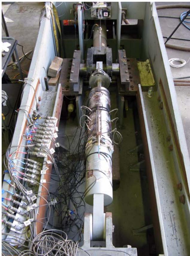
**Fig. 1.1 View of 250-kip damper tested at the Pacific Earthquake Engineering Research Center, U.C. Berkeley. The damper shown mounted on the testing machine is one of the fluid dampers from the 91/5 overcrossing tested during the viscous heating investigation by Black and Makris (2005, 2007).**
