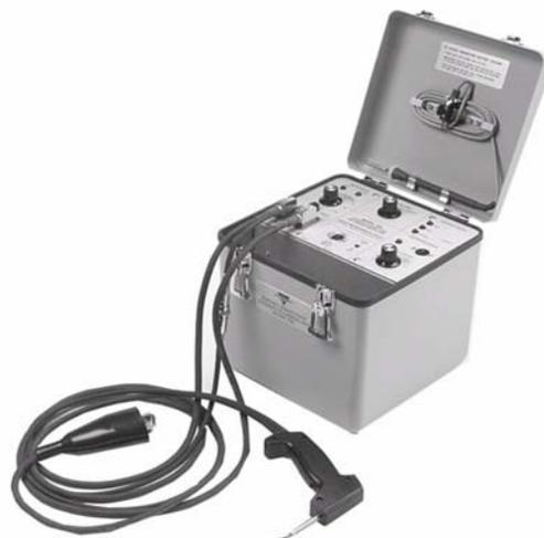
**Fig. 2.9 Vishay Micro-Measurements 700 portable strain-gauge welding and soldering unit.**
