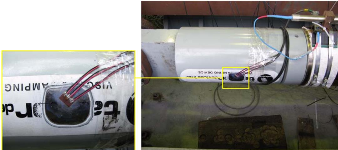
**Fig. 2.8** Strain-gauge rosette on the extender of the 250-kip damper.
