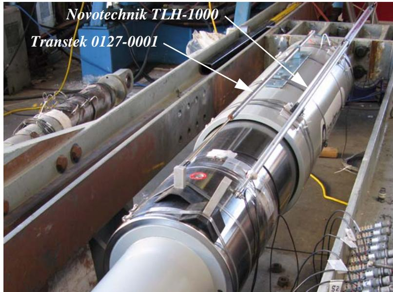
**Fig. 2.13 Transtek 0127-0001 linear velocity transducer and Novotechnik TLH-1000 position transducer.**
