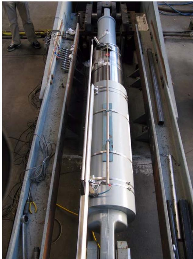
**Fig. 2.5 450-kip damper in the damper testing machine at the Pacific Earthquake Engineering Research Center laboratory, UC Berkeley.**
