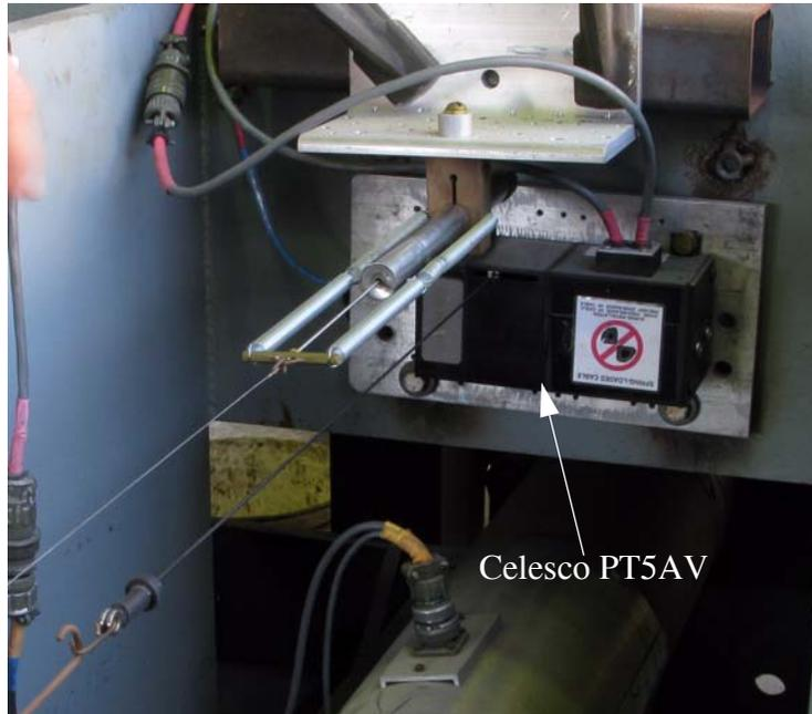
**Fig. 2.12 Celesco PT5AV position and velocity transducer.**
