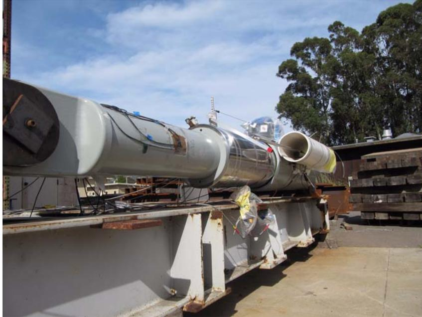
**Fig. 1.2 View of 450-kip damper tested in an outdoor setting at the Pacific Earthquake Engineering Research Center, U.C. Berkeley.**
