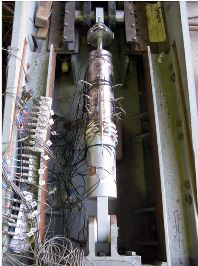
**Fig. 2.3 250-kip damper in the damper testing machine at the Pacific Earthquake Engineering Research Center laboratory, UC Berkeley.**
