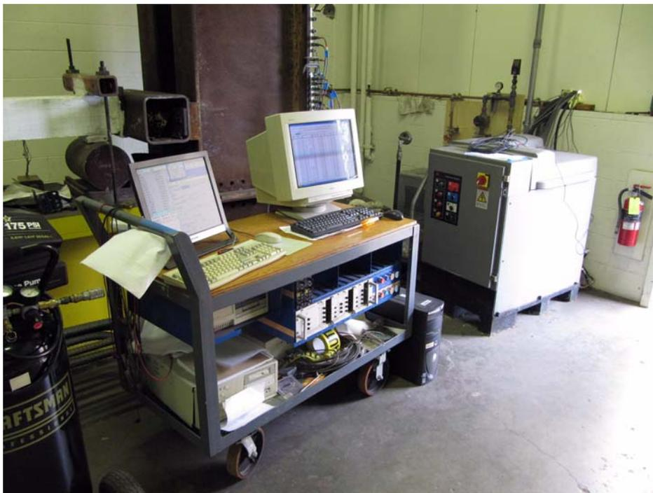
**Fig. 3.4 ATS controller and data acquisition cart; portable hydraulic pump.**
