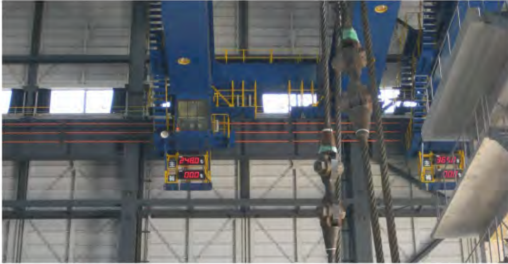
Photo 3. RC Specimen Hanging on Cranes ( 248+365-25=588 t) (Total weight of hanging wires is 25 t)
