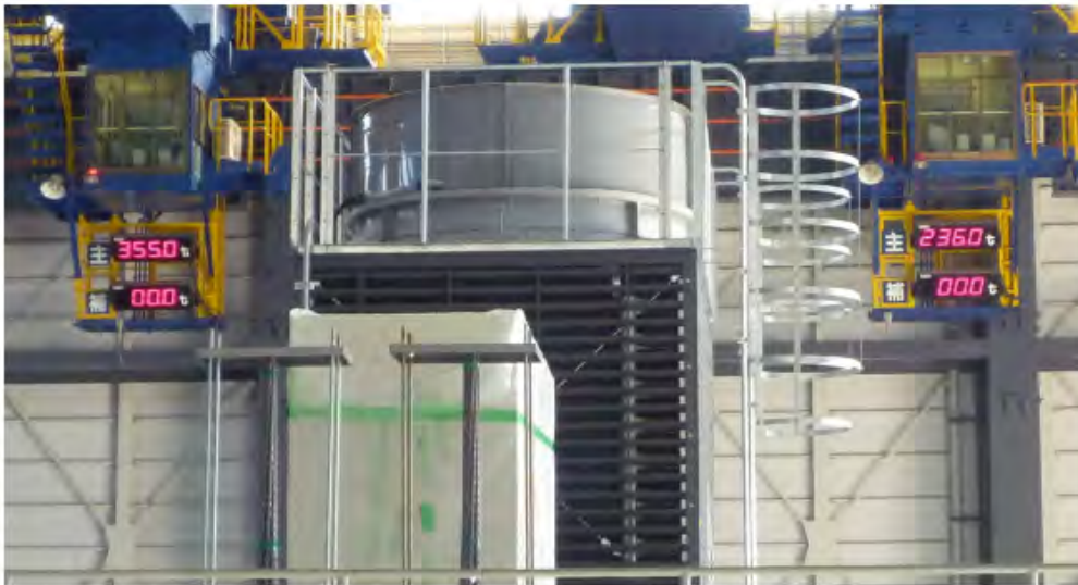
Photo 4. Weight of PT Specimen Hanging on Cranes: 335+236-25=546 t (Total weight of hanging wires is 25 t)
