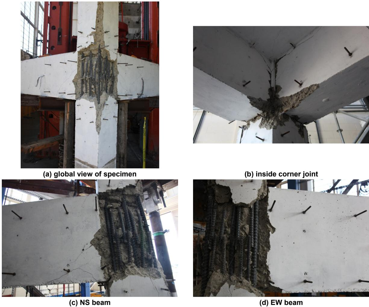
Figure 4.52 Failure of SP4 after removing concrete fragments.
