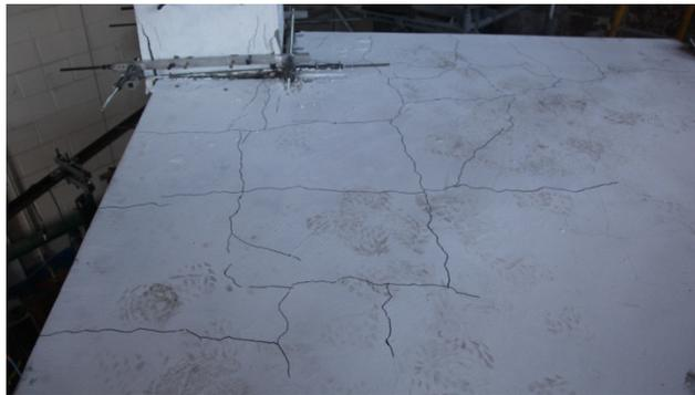
**Figure 5.5 Flexural cracks in the slab of SP3.**
