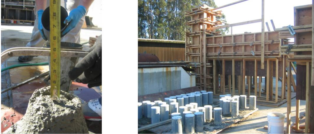
**Figure B.1 Slump test and curing.**
