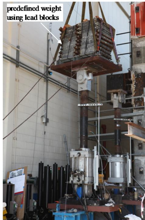
Figure 3.13 Calibration of load cell of the column axial loading actuator.
