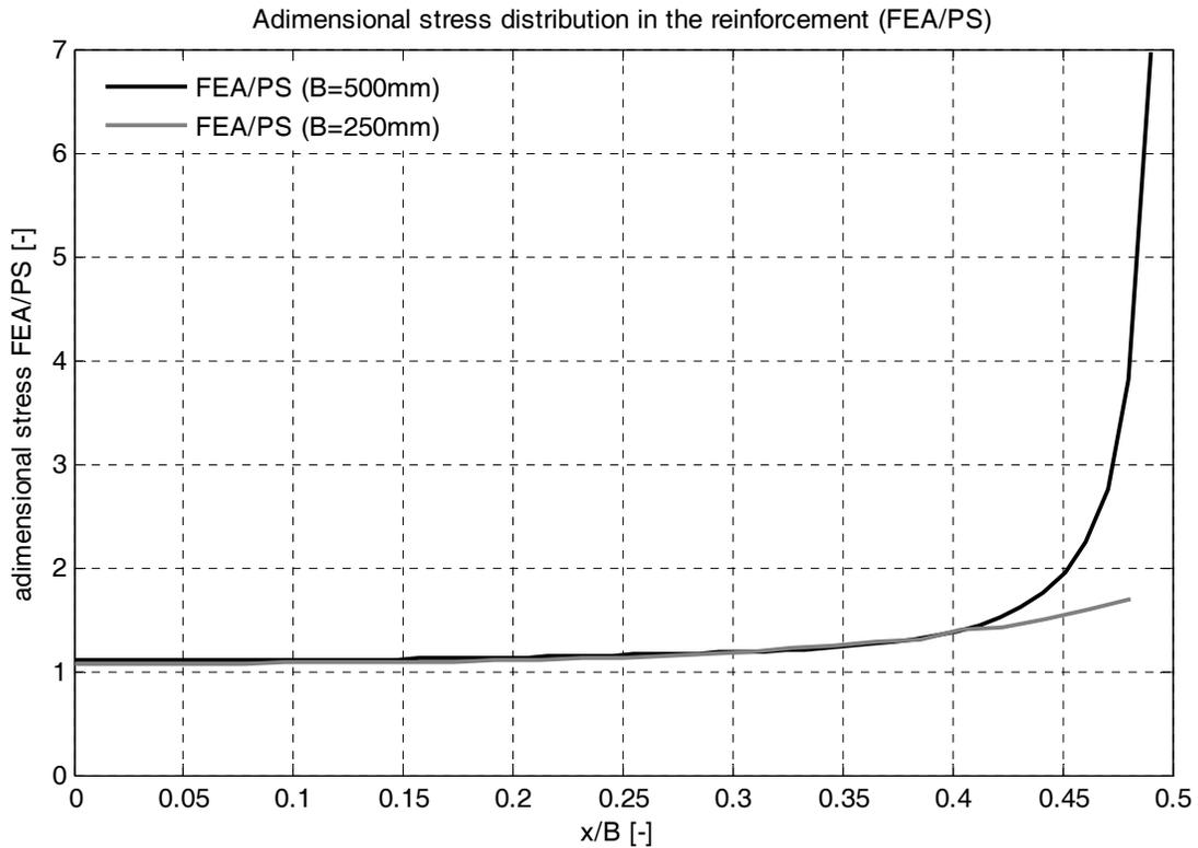
Figure 3.11 Non-dimensional stress (FE/pressure solution) against non-dimensional length ( $x/B$ ).
