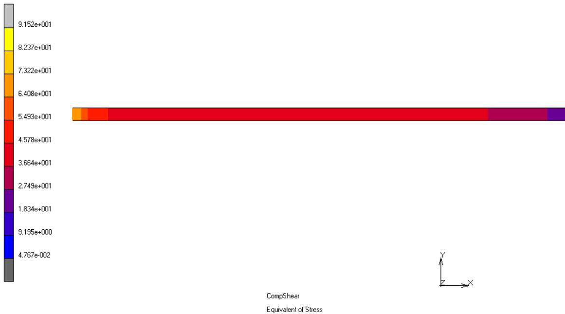
**Figure 3.22** Von Mises stress contours at peak vertical force in a cross section of a circular bearing ( $\Phi=500$  mm–SET1  $t_f=0.07$  mm).
