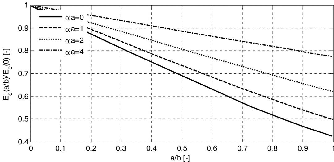
**Figure 2.17** Ratio of effective compressive modulus of rectangular pad to infinitely long strip pad ( $a/b = 0$ ) versus aspect ratio.
