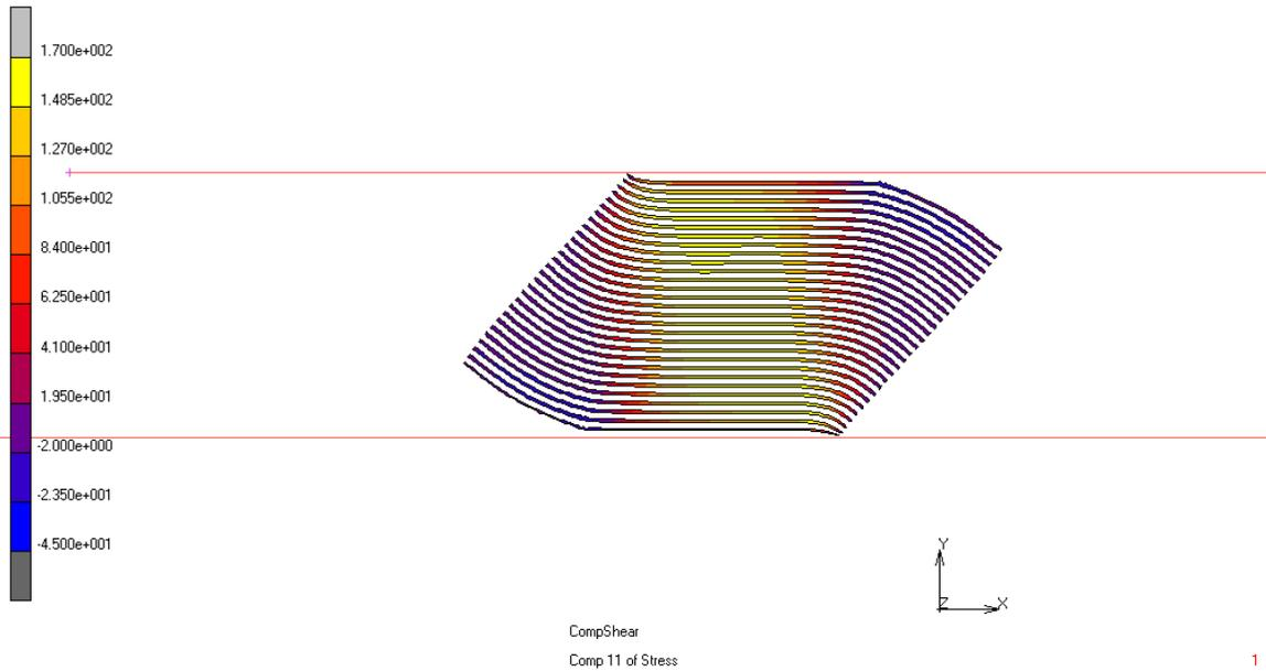
**Figure 3.14** Tension contours in the fiber reinforcement at maximum shear (B=250 mm).
