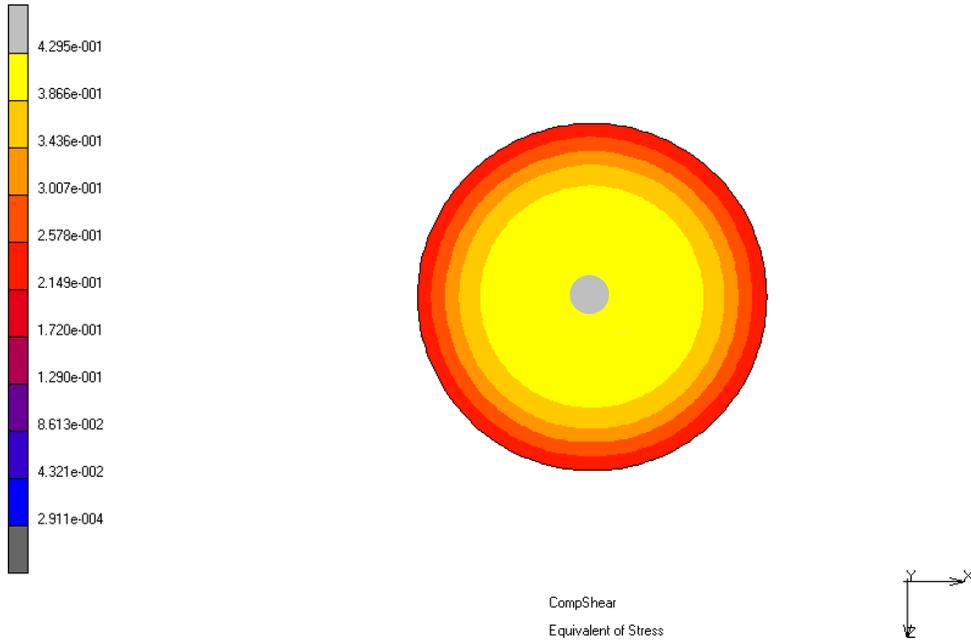
**Figure 3.25** Tension contours in the fiber reinforcement ( $\Phi=250$  mm–SET1  $t_f=0.07$  mm,  $S_V=3.45$  MPa).
