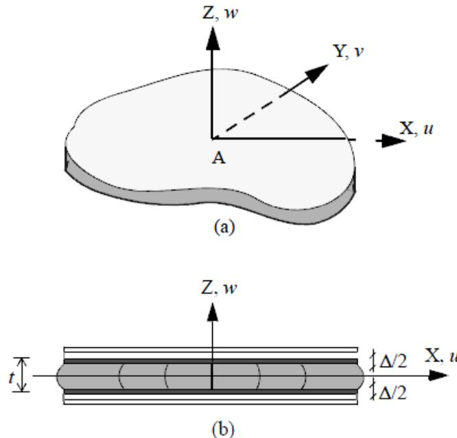
Figure 2.18 Constrained rubber pad and coordinate system.
