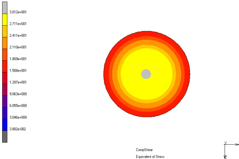
**Figure 3.27** Tension contours in the fiber reinforcement ( $\Phi=250$  mm–SET2  $t_f=0.25$  mm  $S_v=3.45$  MPa).
