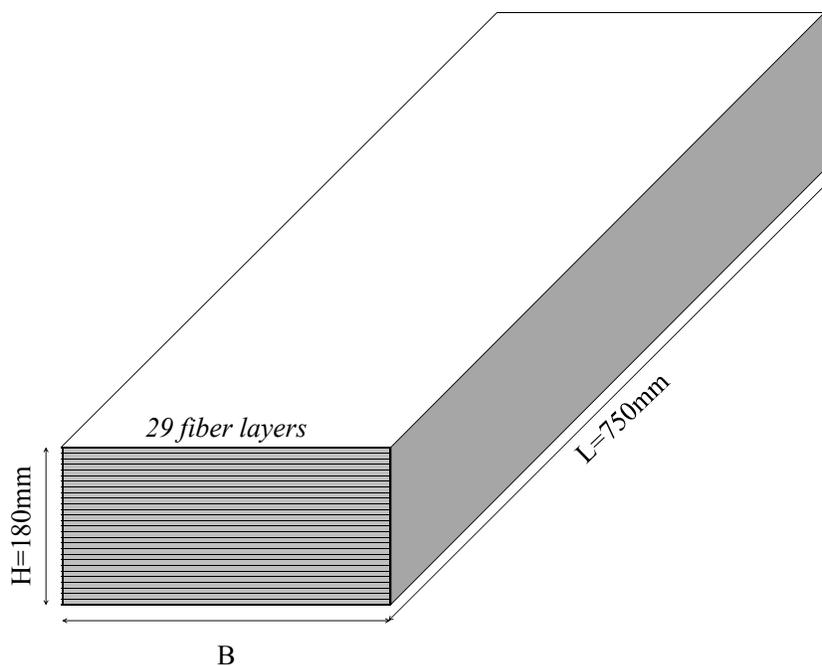
Figure 3.2 Strip type bearing showing reinforcements and dimensions.
