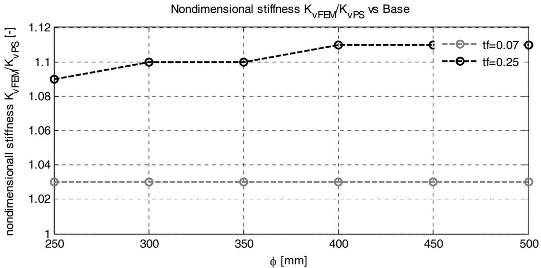
Figure 3.32  $K_{vFEM}/K_{vPS}$  as a function of the diameter.
