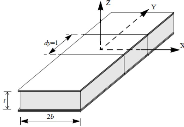
**Figure 2.1** Infinitely long rectangular pad showing dimensions.
