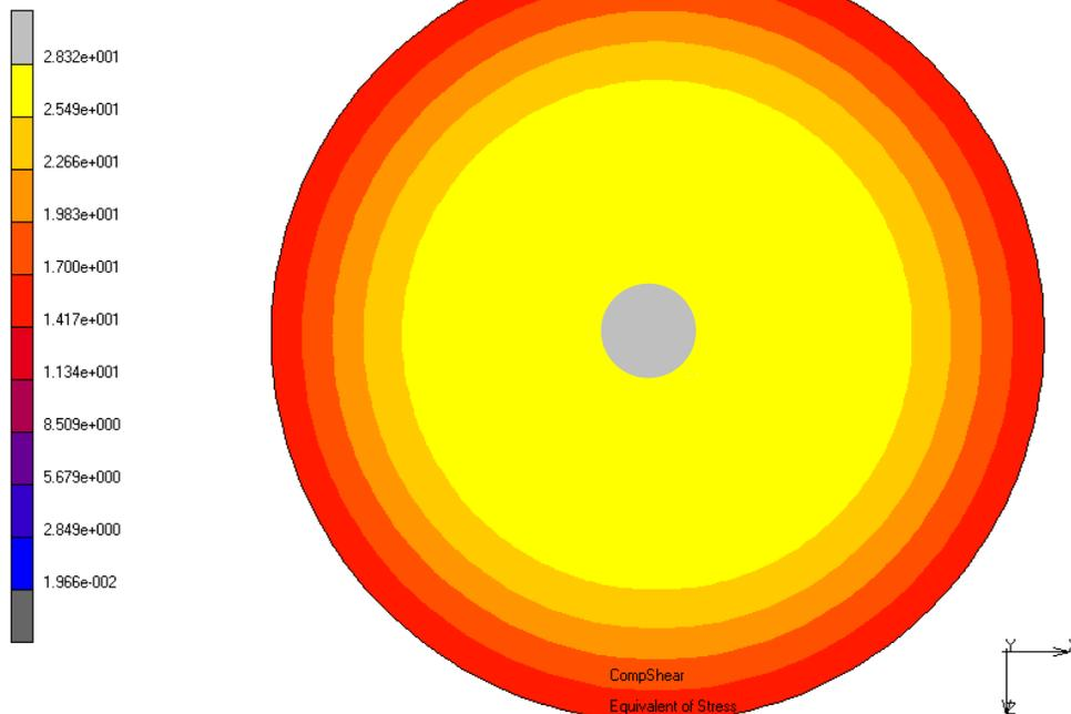
**Figure 3.28** Tension contours in the fiber reinforcement ( $\Phi=500$  mm–SET2  $t_f=0.25$  mm  $S_v=3.45$  MPa).
