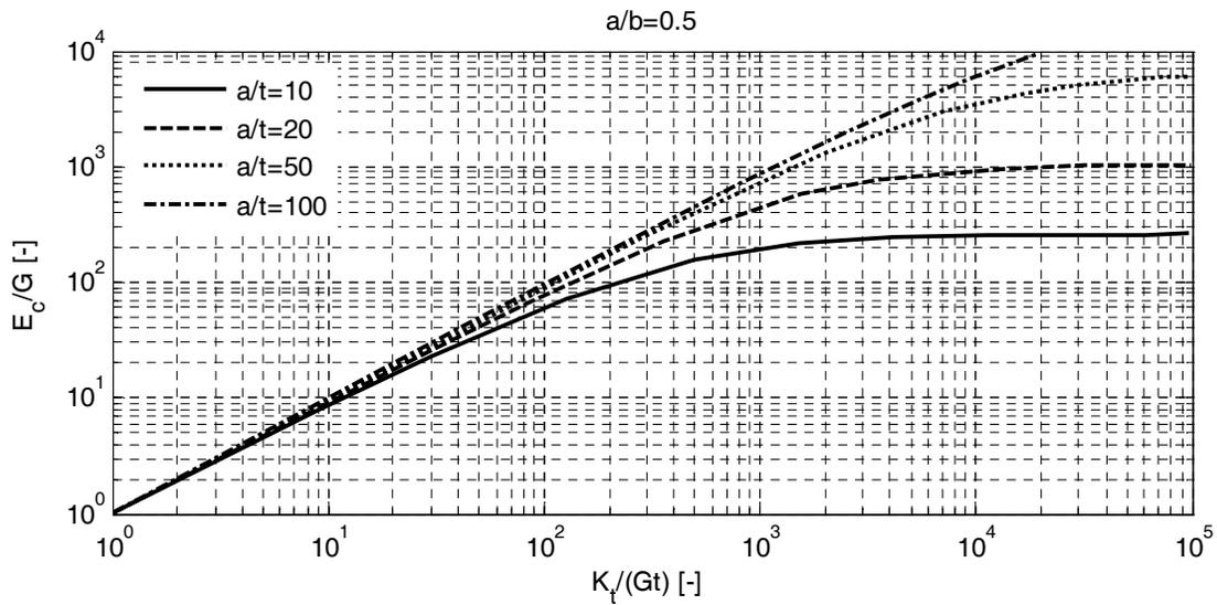
**Figure 2.15** Variation of effective compressive modulus with reinforcement stiffness in rectangular pad ( $a/b = 0.5$ ).
