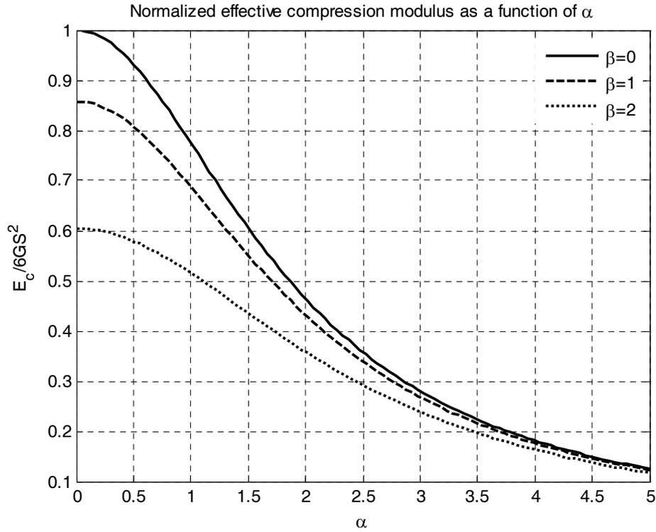
Figure 2.10 Normalized effective modulus as a function of  $\alpha$  for different values of  $\beta$ .
