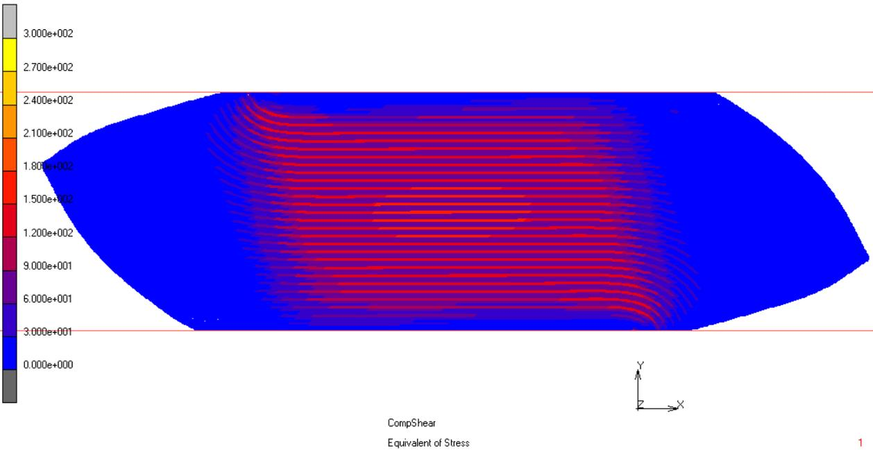
**Figure 3.13 Von Mises stress contours at peak horizontal force in a bearing of base B=500 mm.**
