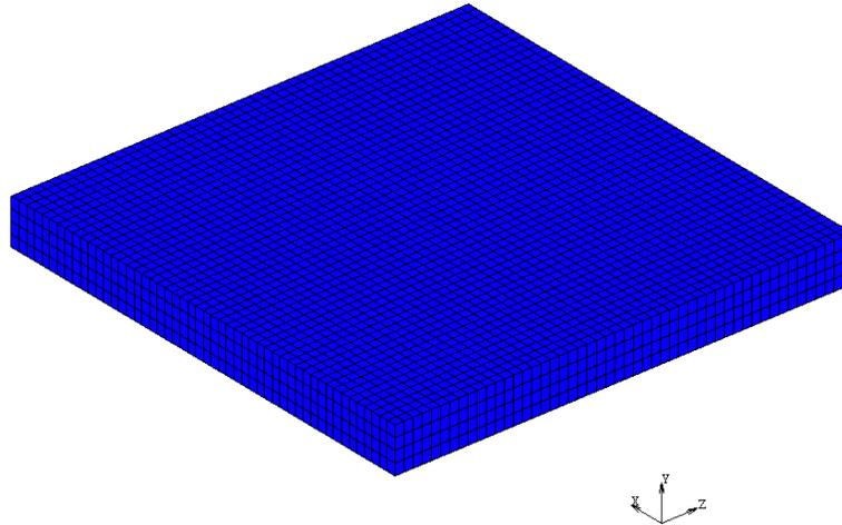
Figure 3.34 Model mesh for a single pad (element type 84).
