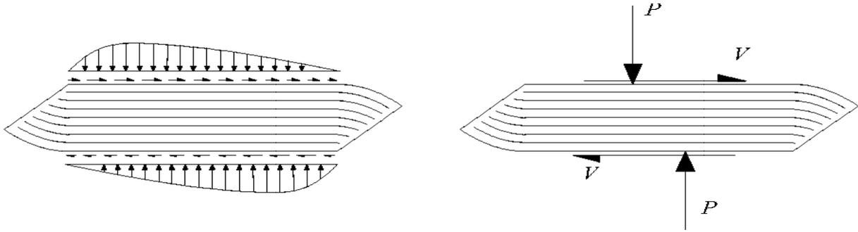
**Figure 4.2** Normal and shear stress distributions on the top and bottom faces of the unbonded bearing in its deformed shape.
