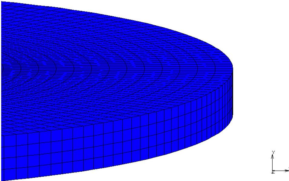
**Figure 3.20** Model mesh and layout of the reinforcement layers (elements 143).
