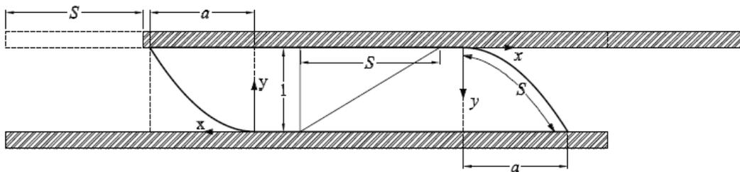
Figure 4.4 Schematic of the deformed bearing.
