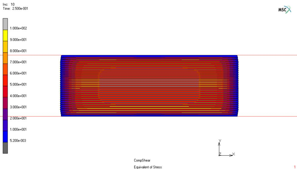
**Figure 3.5** Von Mises stress contours at peak vertical force in a bearing of base  $B=500$  mm [SET2 ( $t_f = 0.07$  mm)].
