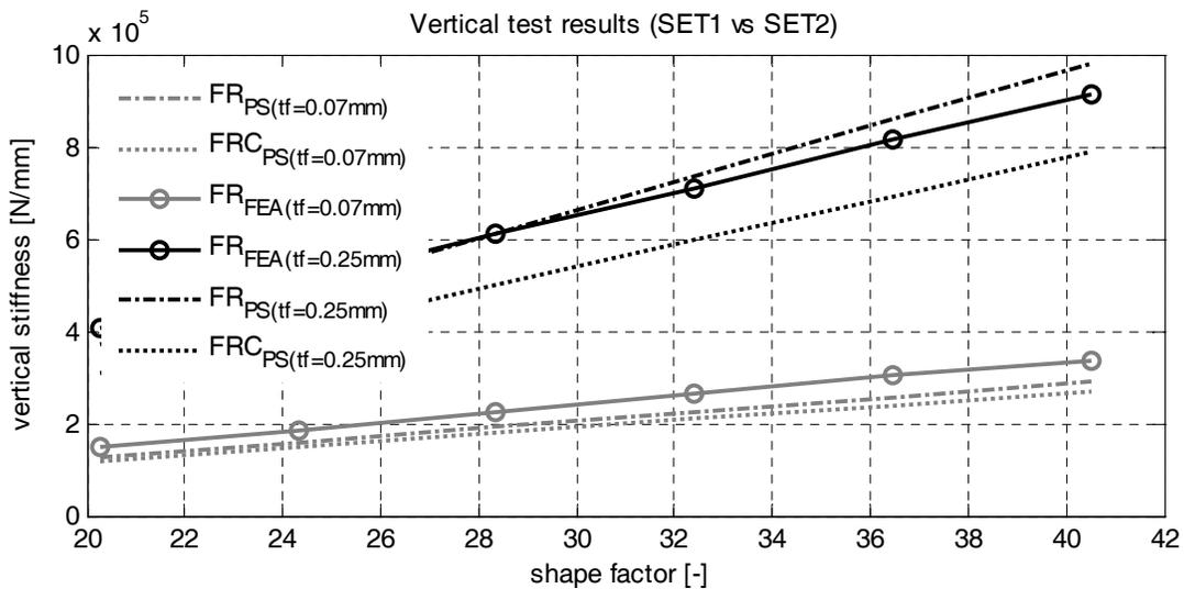
**Figure 3.8 Vertical stiffness (FE analysis versus pressure solution).**
