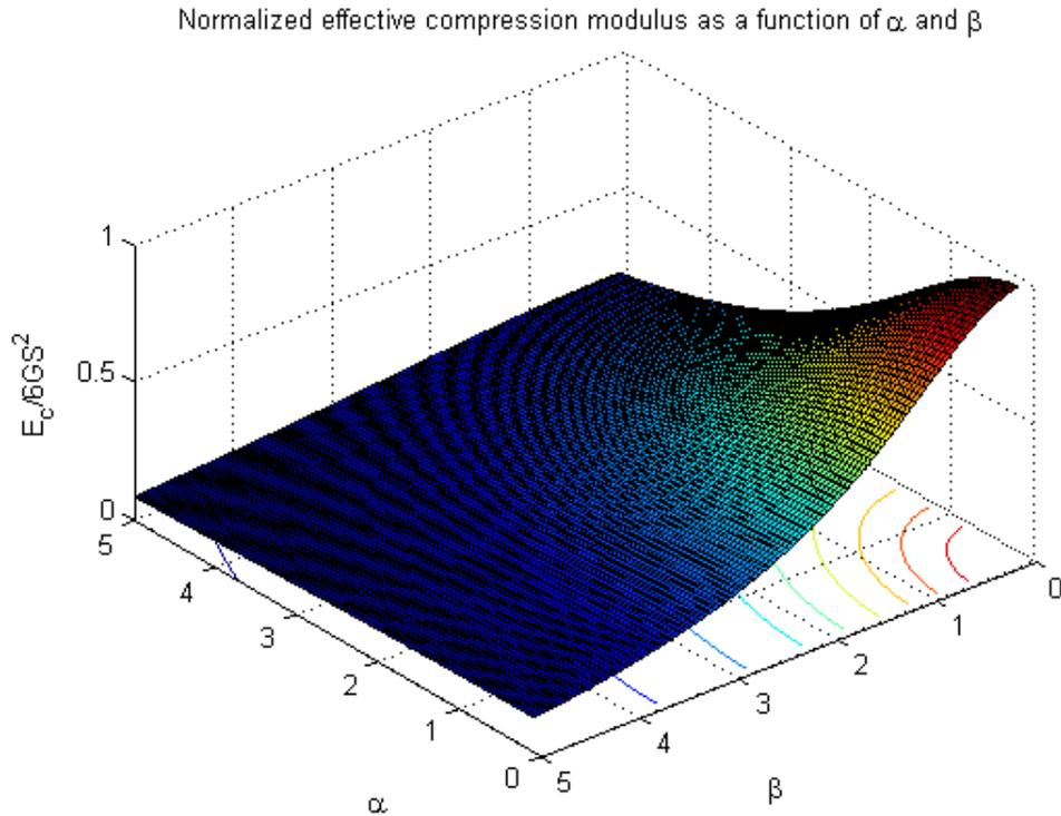
**Figure 2.9** Normalized effective modulus as a function of  $\alpha$  and  $\beta$ .
