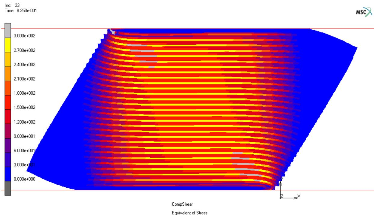
**Figure 3.12** Von Mises stress contours at peak horizontal force in a bearing of base  $B=250$  mm.
