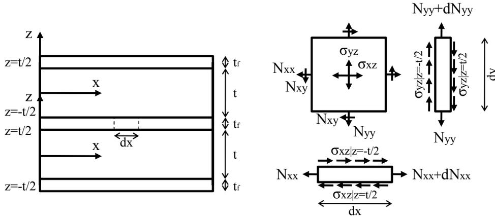
**Figure 2.13** Forces in reinforcing sheet bonded to rectangular layers of elastomers.
