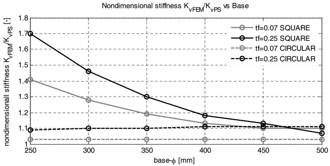
**Figure 3.38**  $K_{vFEM}/K_{vPS}$  as a function of the base-diameter for square and circular bearings.
