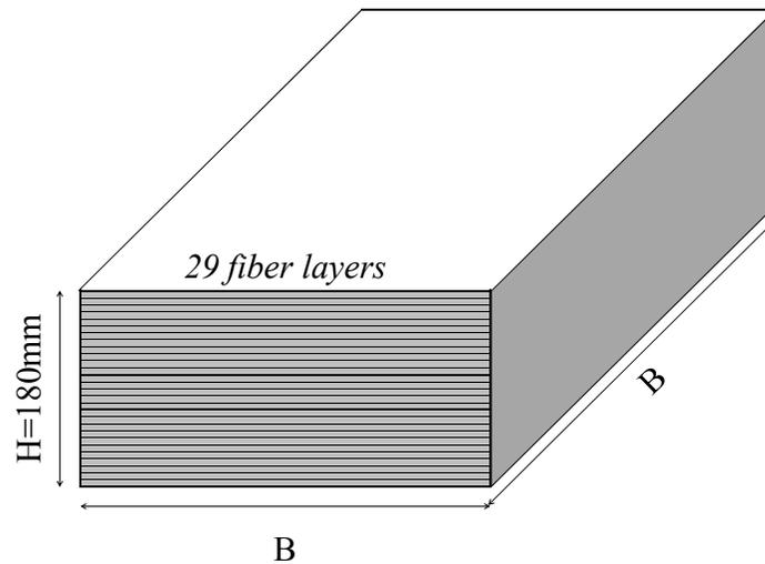
**Figure 3.33 Square type bearing showing reinforcements and dimensions.**
