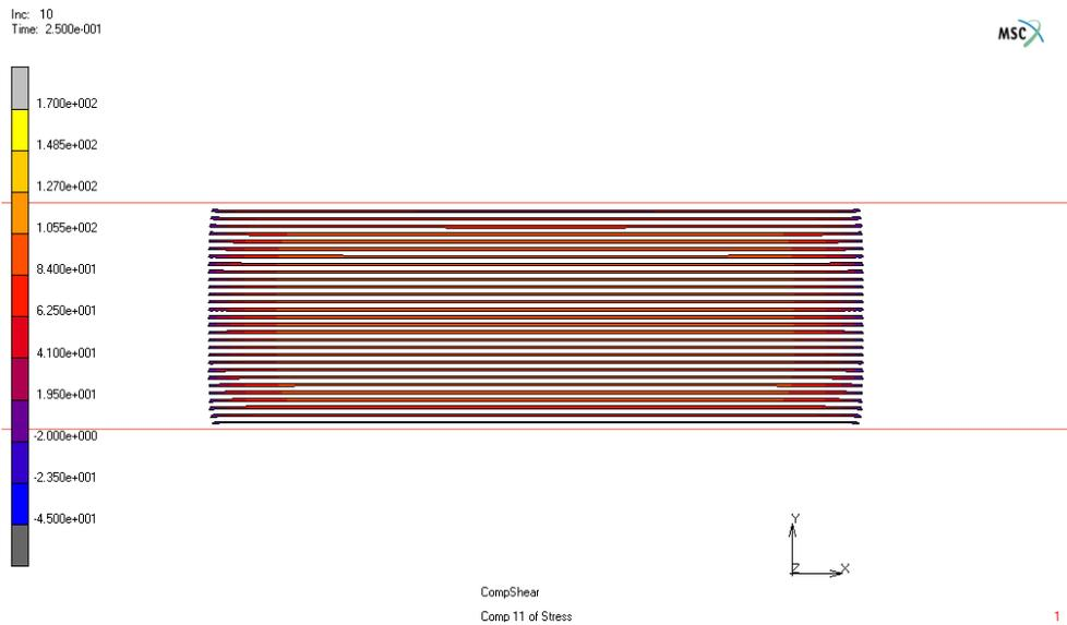
**Figure 3.7** Tension contours in the fiber reinforcement ( $B=500$  mm;  $S_v=3.45$  MPa; SET2).
