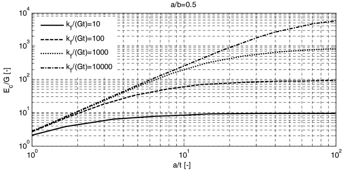
**Figure 2.16** Variation of effective compressive modulus with width thickness in rectangular pad ( $a/b = 0.5$ ).
