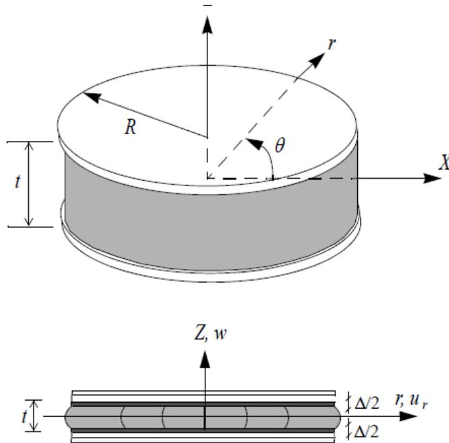
Figure 2.8 Coordinate system for a circular pad of radius  $R$ .
