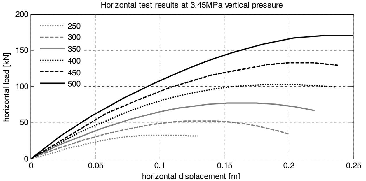
**Figure 3.16 Force-displacement curves.**
