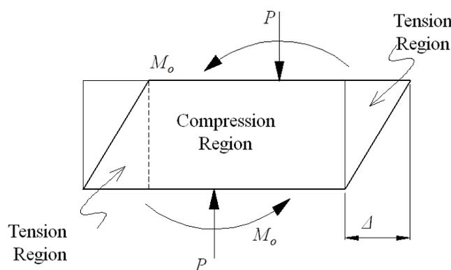
Figure 4.1 Bonded bearing under compression and shear.
