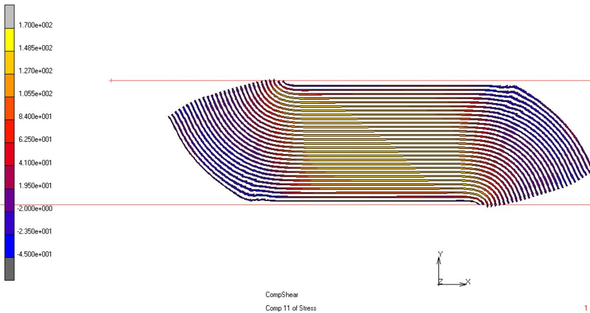
**Figure 3.15** Tension contours in the fiber reinforcement at maximum shear (B=500 mm).
