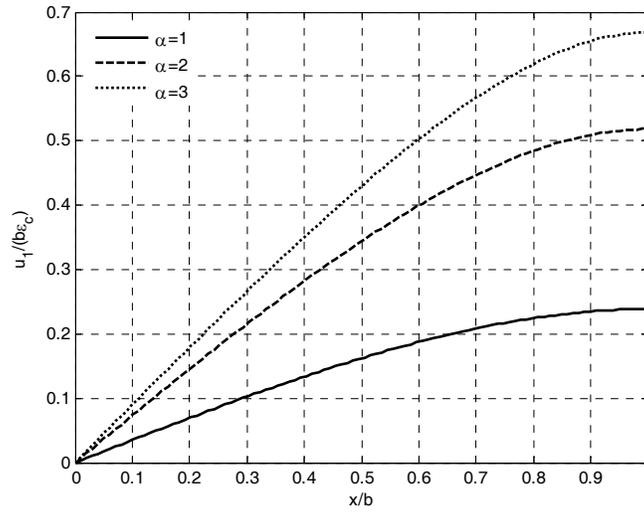
Figure 2.4 Displacement pattern for fiber reinforcement for various values of  $\alpha$ .
