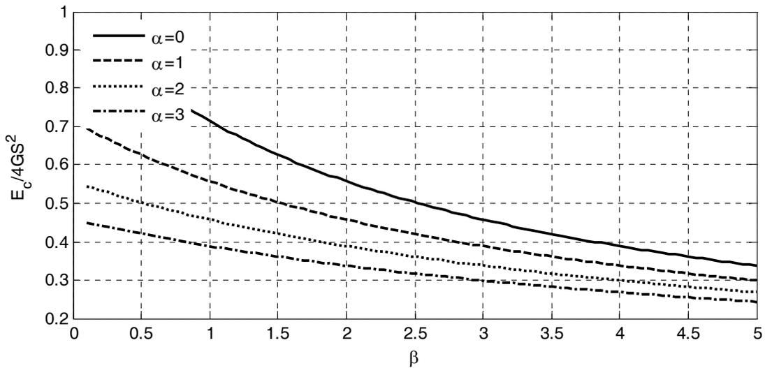
**Figure 2.7** Variation of normalized effective compression modulus with  $\beta$  for  $\alpha = 0 - 3$ .
