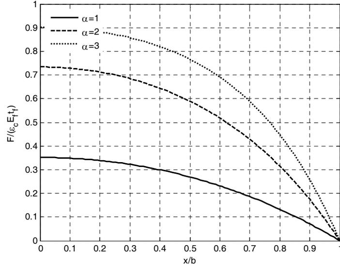
Figure 2.3 Normalized force pattern in reinforcement.
