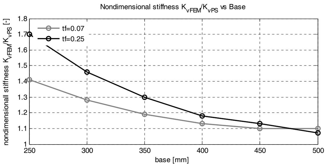
Figure 3.37  $K_{vFEM}/K_{vPS}$  as a function of the base.
