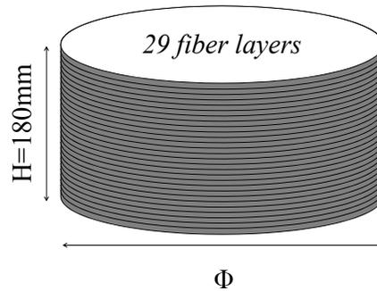
Figure 3.19 Circular type bearing showing reinforcements and dimensions.
