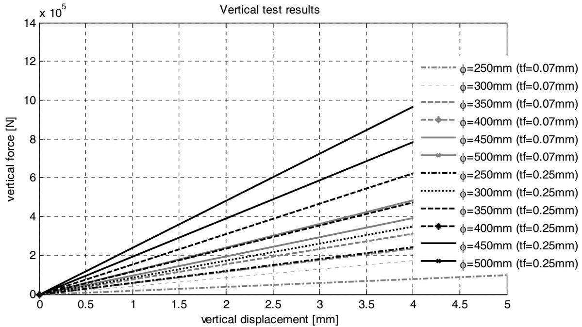
Figure 3.29 Vertical test results (FE analysis versus pressure solution).
