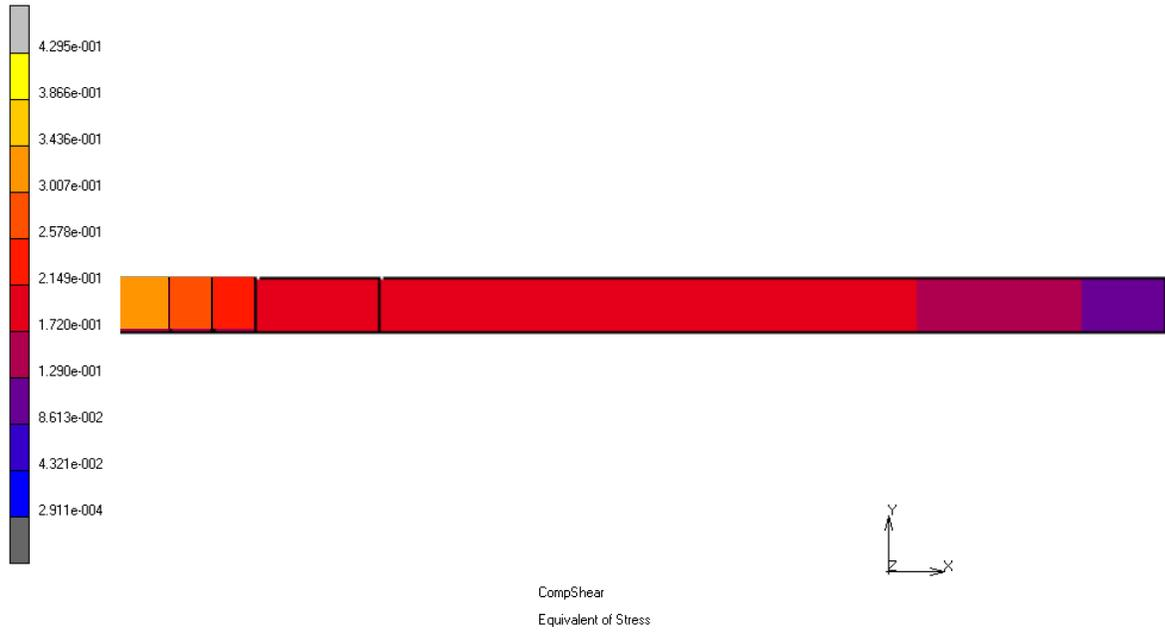
**Figure 3.21** Von Mises stress contours at peak vertical force in a cross section of a circular bearing ( $\Phi=250$  mm–SET1  $t_f=0.07$  mm).
