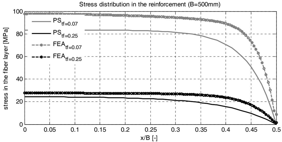
Figure 3.10 Stress distributions in the reinforcement (analyses versus pressure solution) for B=500 mm.
