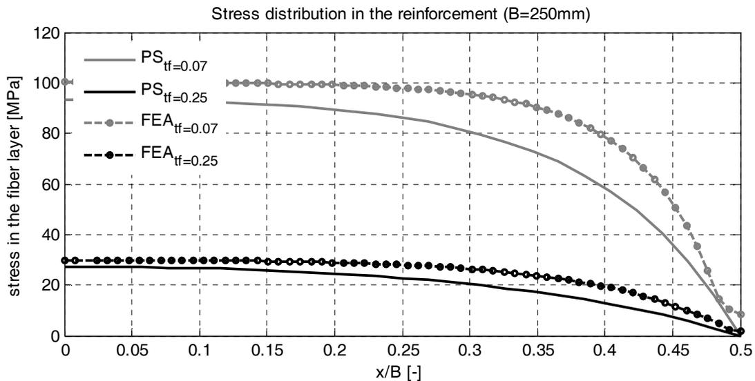
**Figure 3.9** Stress distributions in the reinforcement (FE analysis versus pressure solution) for  $B=250$  mm.
