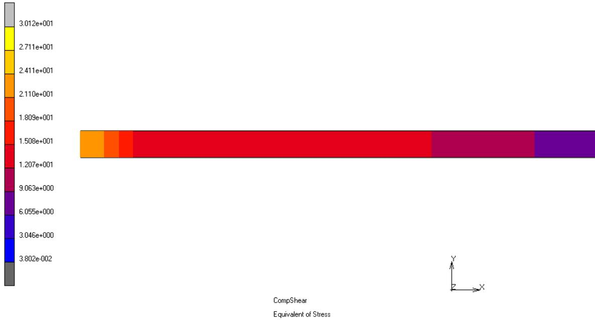
**Figure 3.23** Von Mises stress contours at peak vertical force in a cross section of a circular bearing ( $\Phi=250$  mm–SET1  $t_f=0.25$  mm).
