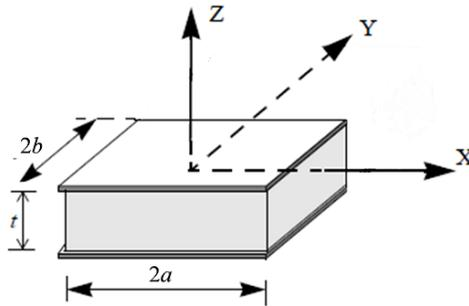
**Figure 2.12** Reference system for a rectangular pad showing dimensions.
