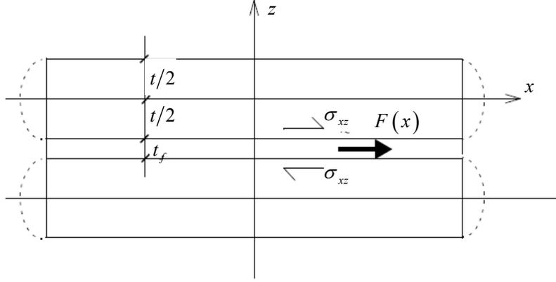
**Figure 2.2 Forces in reinforcing sheet bonded to layers of elastomers.**
