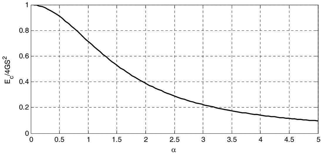
**Figure 2.5** Variation of effective compression modulus with  $\alpha b$  in infinitely long strip pad.
