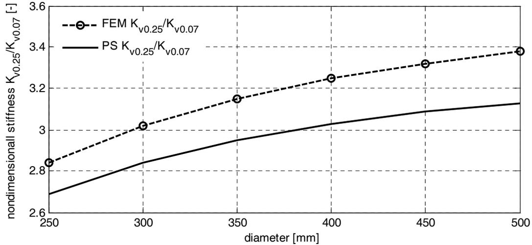
Figure 3.31 Non-dimensional stiffness versus diameter.
