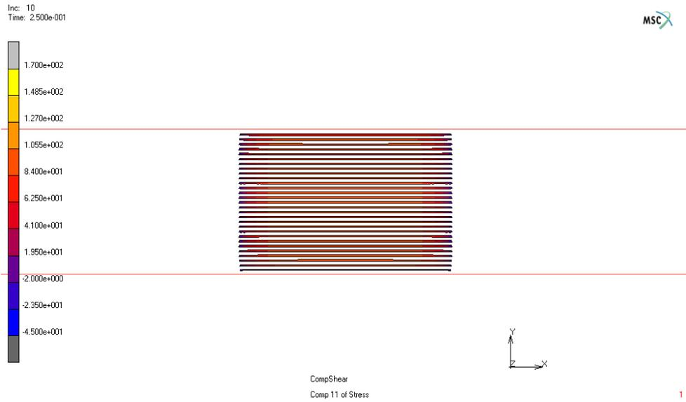
**Figure 3.6** Tension contours in the fiber reinforcement ( $B=250$  mm;  $S_v=3.45$  MPa; SET2).
