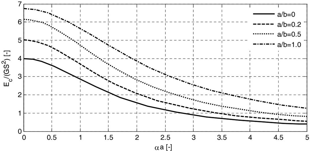
**Figure 2.14** Variation of effective compressive modulus with  $\alpha a$  in rectangular pad.
