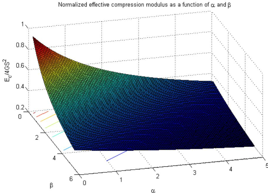
**Figure 2.6** Variation of normalized effective compression modulus with  $\alpha$  and  $\beta$ , in an infinitely long strip pad.
