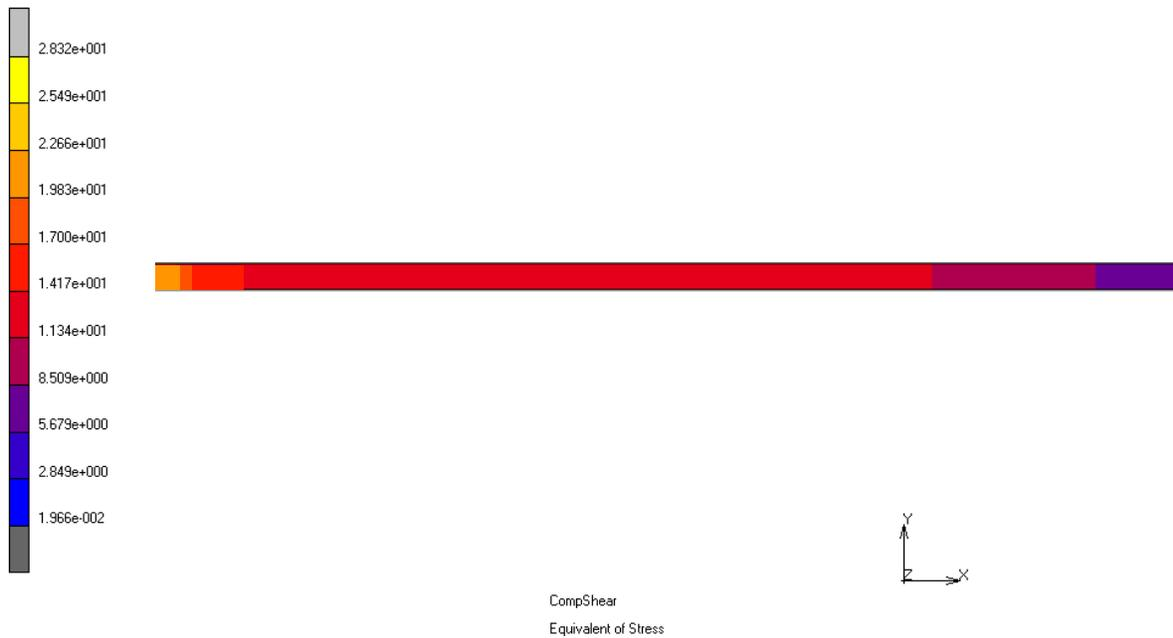
**Figure 3.24** Von Mises stress contours at peak vertical force in a cross section of a circular bearing ( $\Phi=500$  mm - SET2  $t_f=0.25$  mm).
