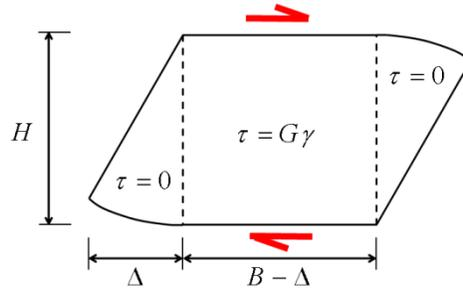
Figure 4.3 Unbonded bearing under shear load.
