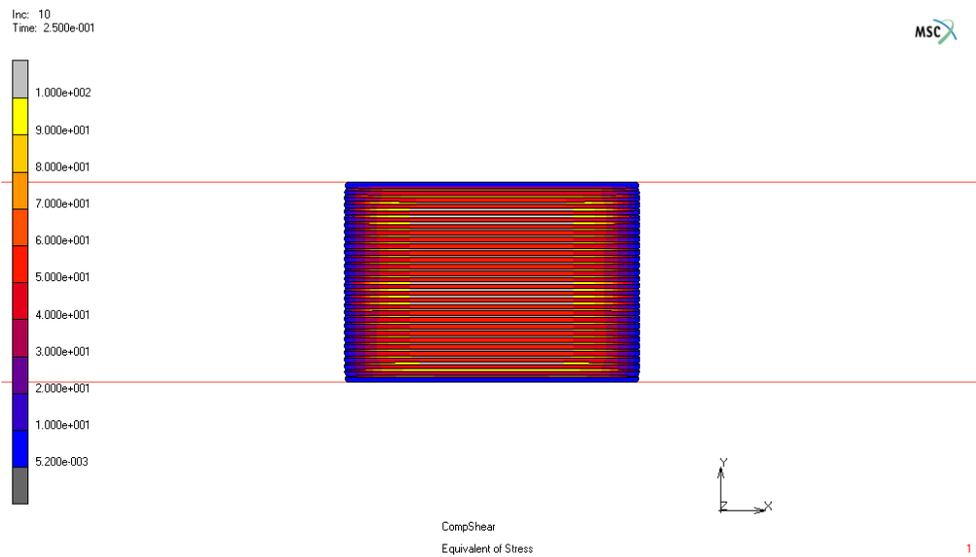
**Figure 3.4** Von Mises stress contours at peak vertical force in a bearing of base  $B=250$  mm [SET2 ( $t_f = 0.07$  mm)].
