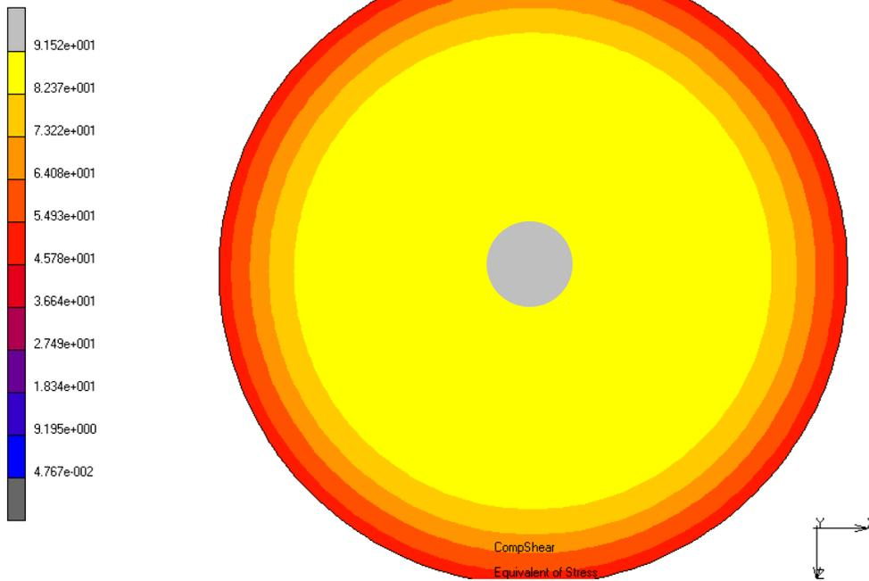
**Figure 3.26** Tension contours in the fiber reinforcement ( $\Phi=500$  mm–SET1  $t_f=0.07$  mm  $S_V=3.45$  MPa).
