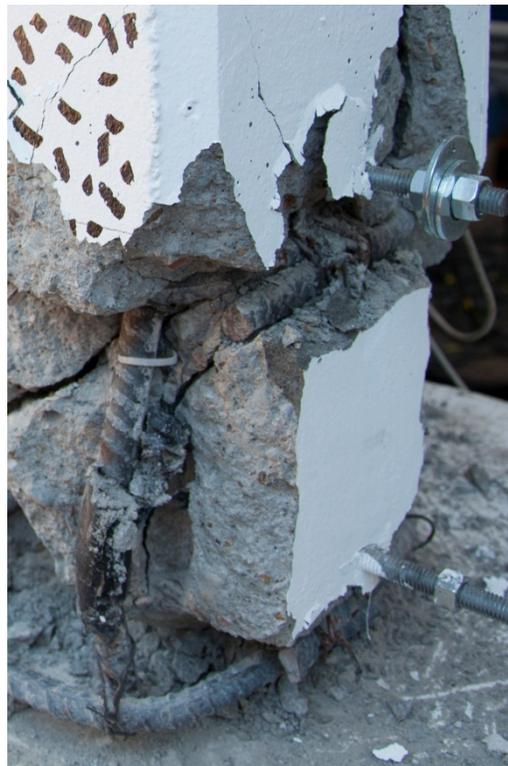
**Figure 6.50** Wall 2 west side reinforcing bars.
