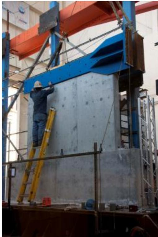
**Figure A.16** Attaching loading plate to wall.
