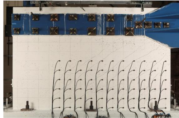
**Figure 6.8 Wall 1 BDBE shear cracks.**
