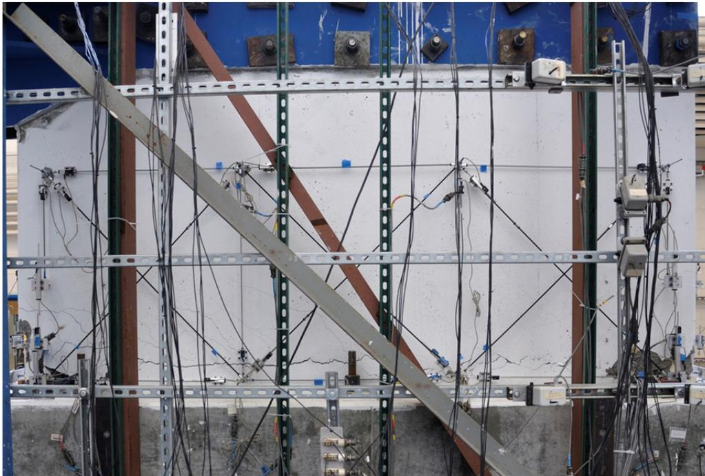
**Figure 5.10** Photograph of Novotechnik instrumentation to measure shear.
