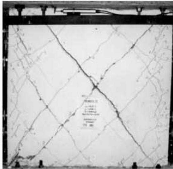
Figure 2.1 Diagonal tension failure (Gulec [2009] from Hildago [2001]).
