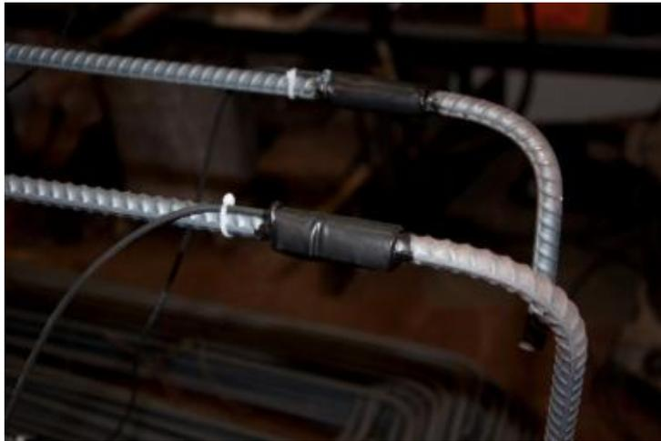
**Figure A.6** Mastic tape over strain gages.
