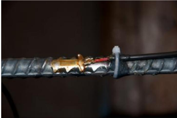
**Figure A.5** Strain gage.
