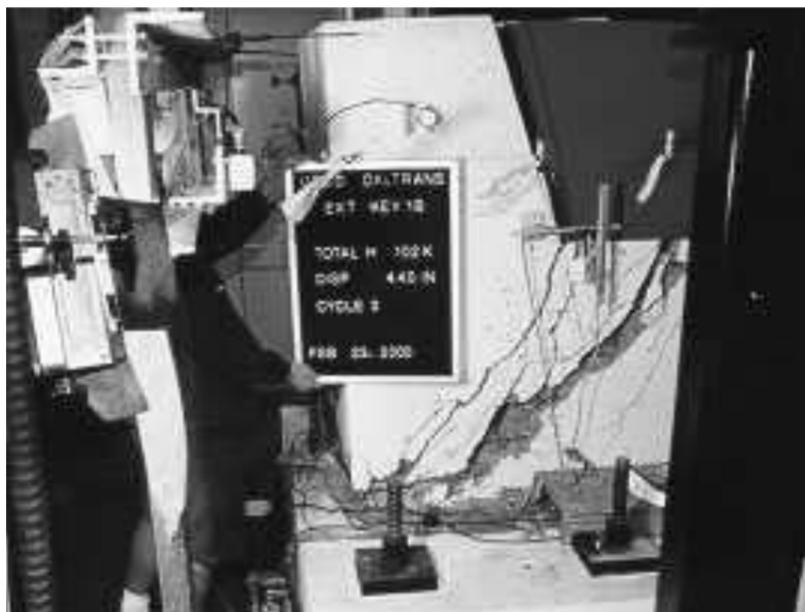
**Figure 3.14** Cracking pattern at the end of Shear Key testing (Test 1B; Megally et al. [2002]).
