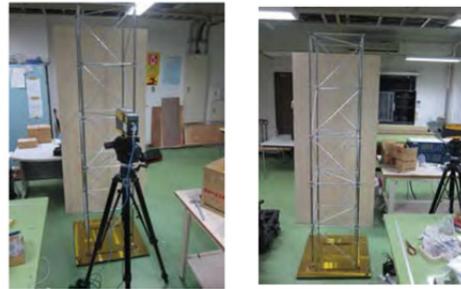
First model (non-continuous longitudinal members)
