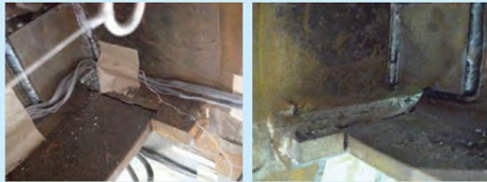
Fracture on Sensor 1 location
