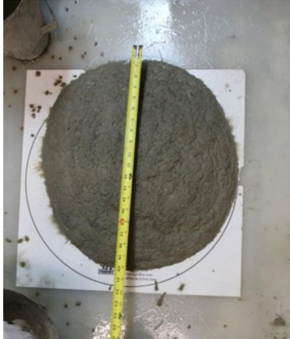
**Figure 2.3** Slump flow test of tube HyFRC.
