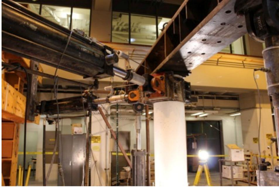
**Figure 3.2** Detail photograph of horizontal actuators.
