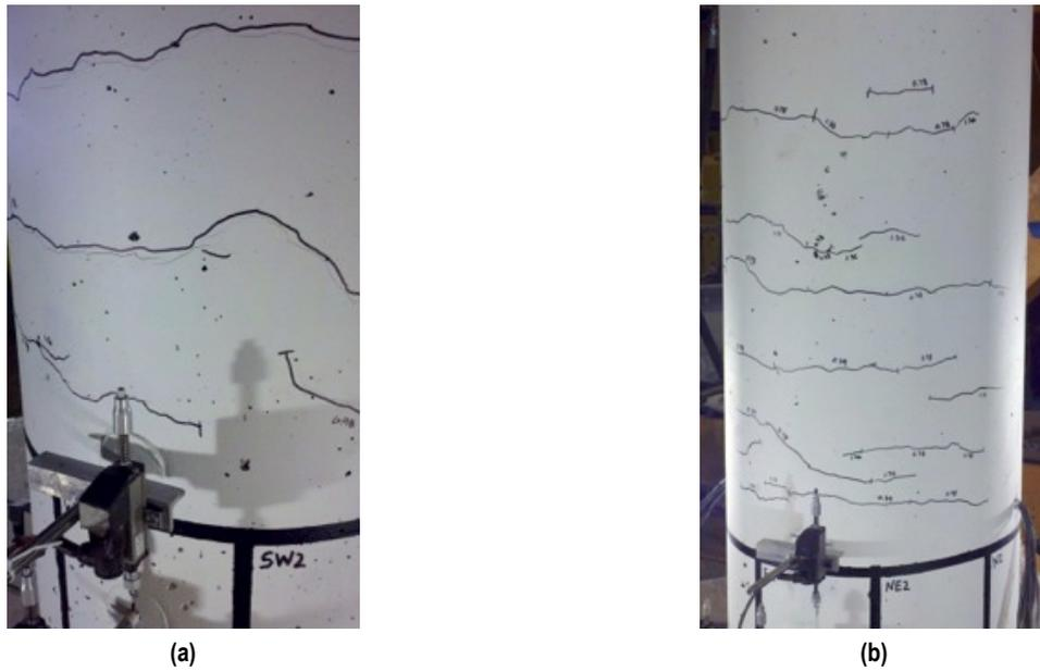
**Figure 4.5** Elevation view of column: (a) West face in extreme tension,  $\theta_r=2.4\%$ ; and (b) East face in neutral position,  $\theta_r=2.4\%$ .
