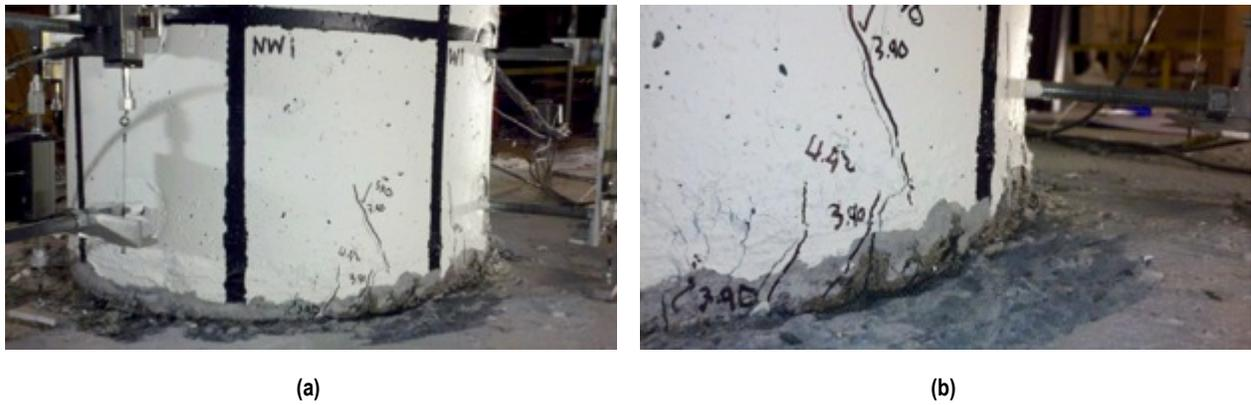
**Figure 4.13 Northwest face of column at extreme westward loading: (a)  $\theta_r=8.3\%$ ; and (b)  $\theta_r=9.5\%$ .**
