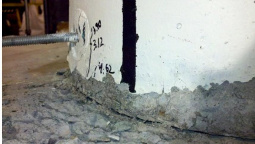
Figure 4.10 East face of column at neutral position,  $\theta_r=8.3\%$ . Permanent vertical displacement can be observed between the column–foundation interface.
