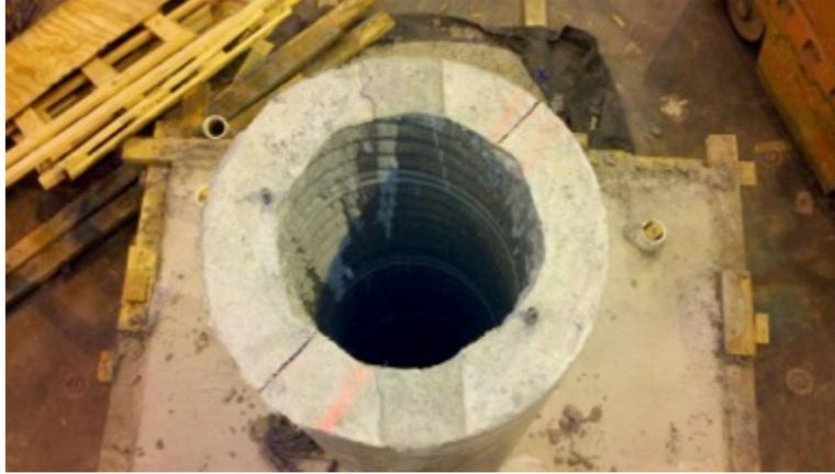
**Figure 2.11** Top view of column prior to core casting.
