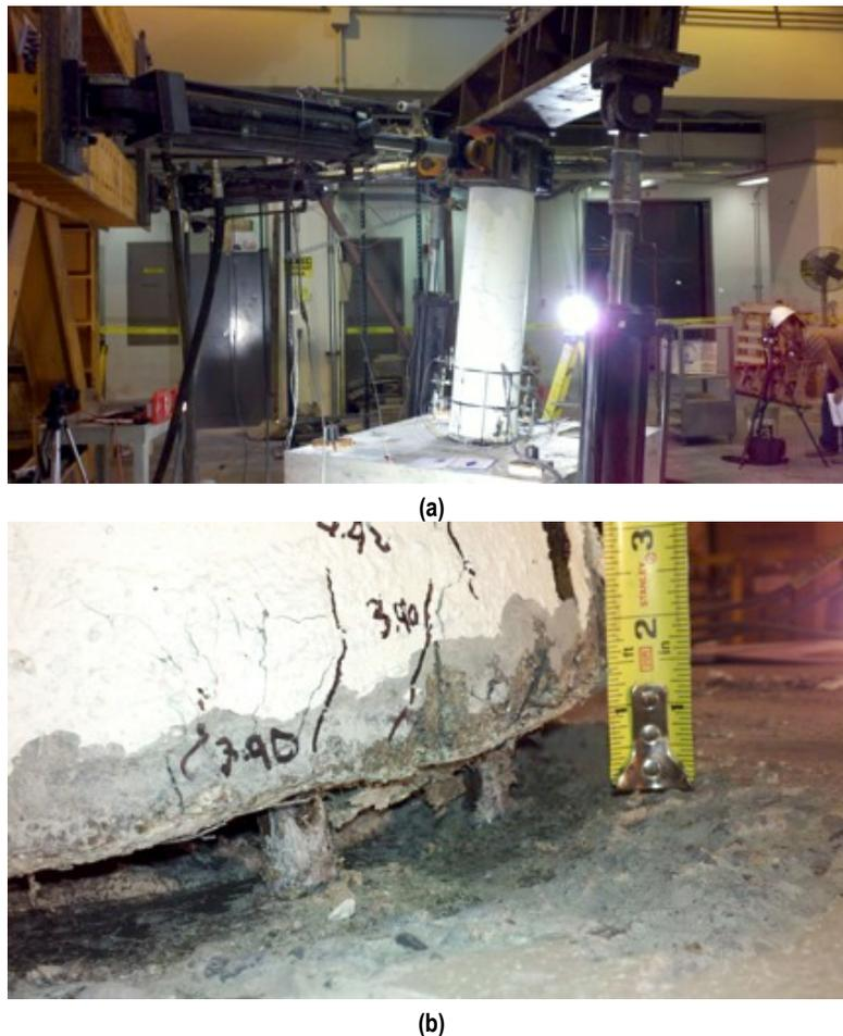
**Figure 4.6** Column during extreme eastern drift, at  $\theta_r=11.3\%$ : (a) global view, viewing from southern side; and (b) close-up at western face, viewing from northern side, showing exposed longitudinal rebar.
