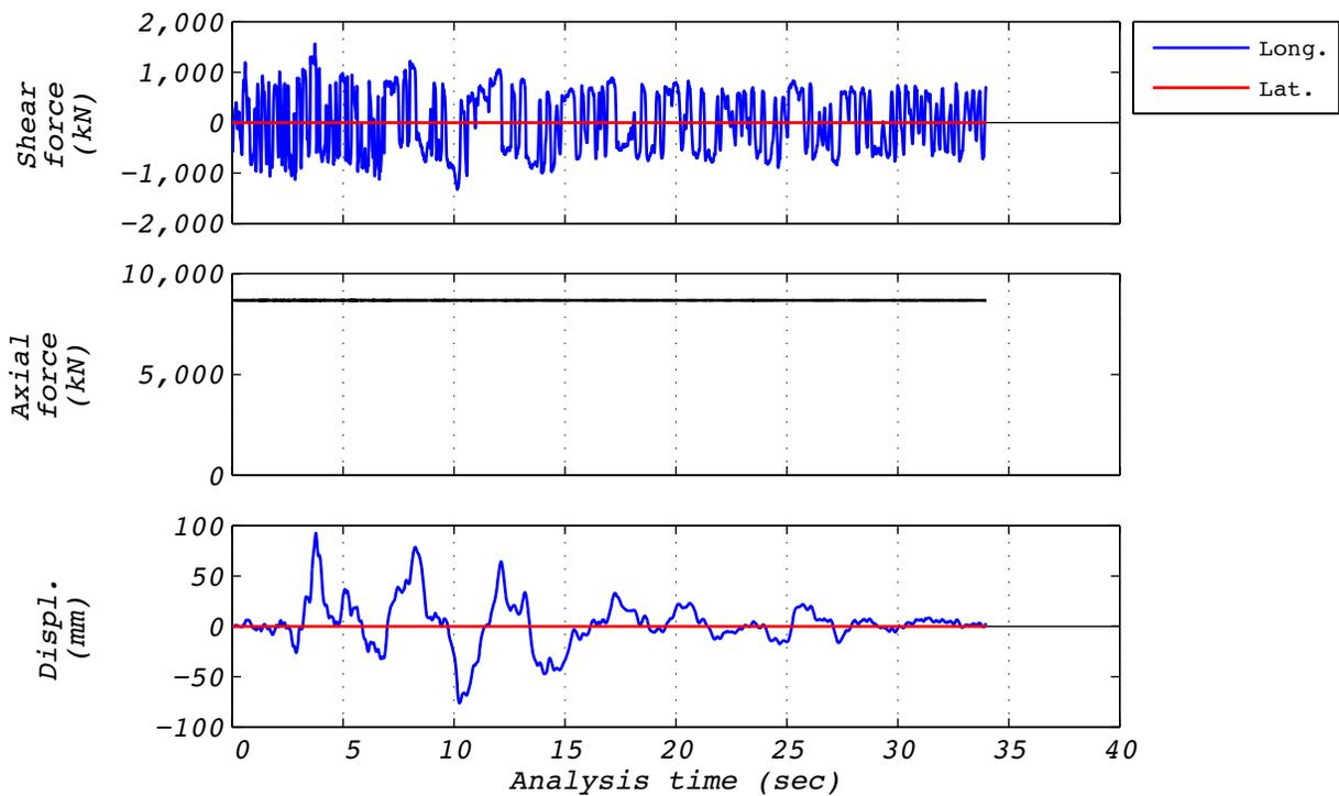
**Figure C.16-3 Hybrid test time history responses for run 52: NRC2, 1D with experimental bearing representing all bearings.**
