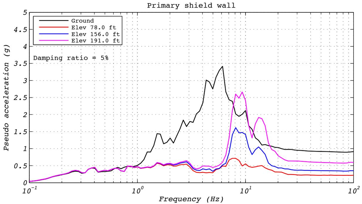
**Figure C.9-4 Hybrid test floor spectra for run 44: NRC2, 3D with 5 groups of bearings and the experimental bearing representing the center group.**
