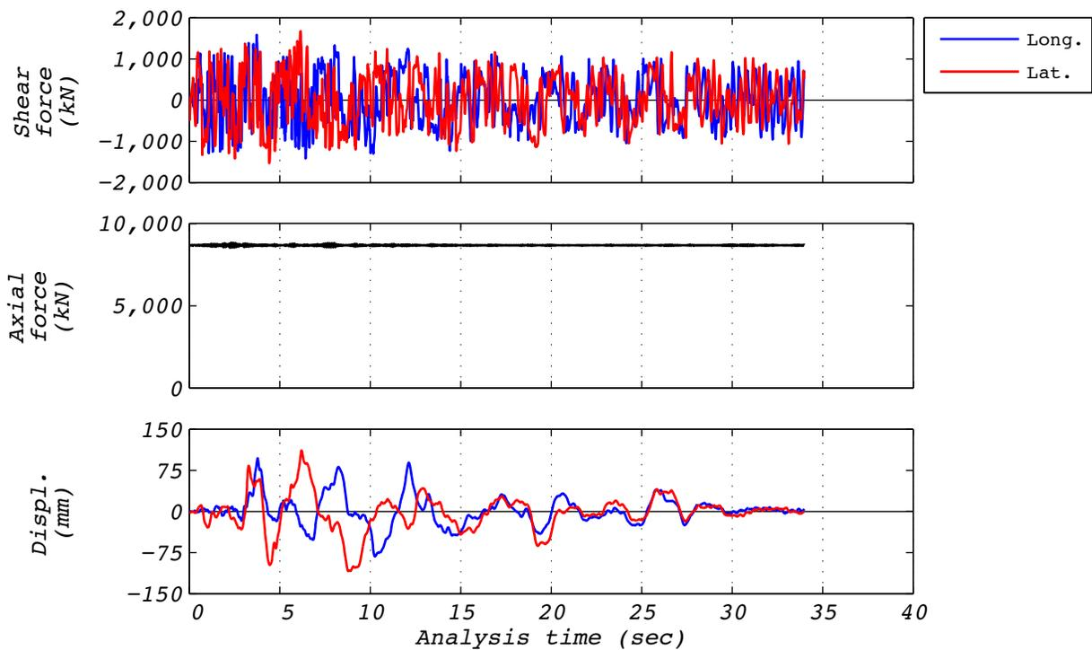
Figure C.20-3 Hybrid test time history responses for run 54: NRC2, 2D with experimental bearing representing all bearings.
