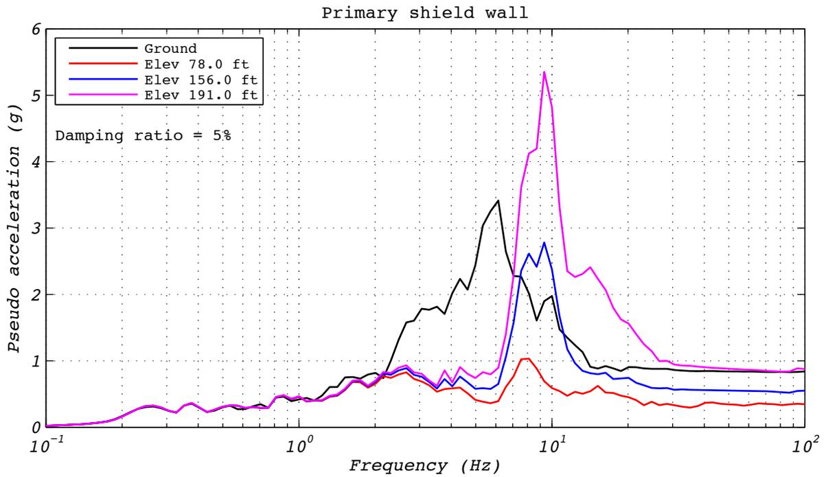
**Figure C.6-4 Hybrid test floor spectra for run 22: NRC2, 1D with experimental bearing representing all bearings.**
