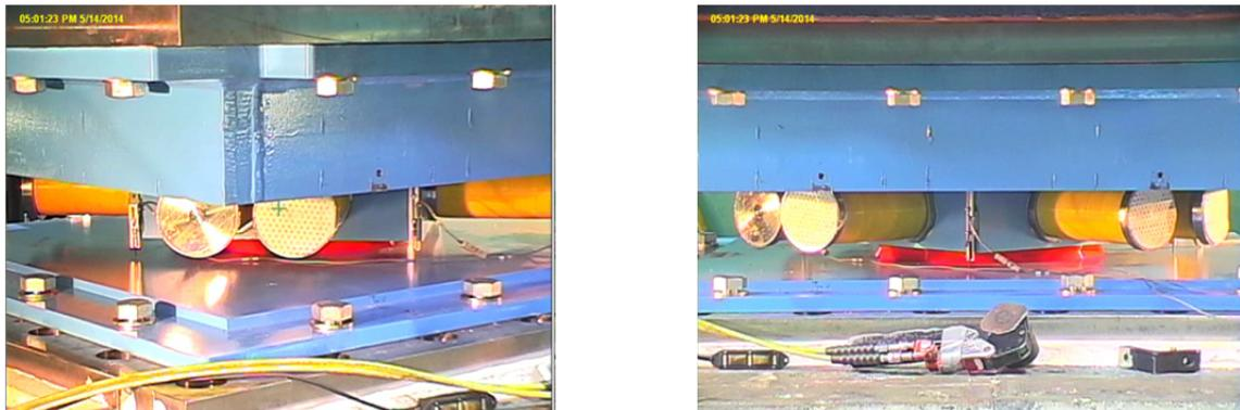
**Figure 3.87 Failure of the EQS-1 bearing.**
