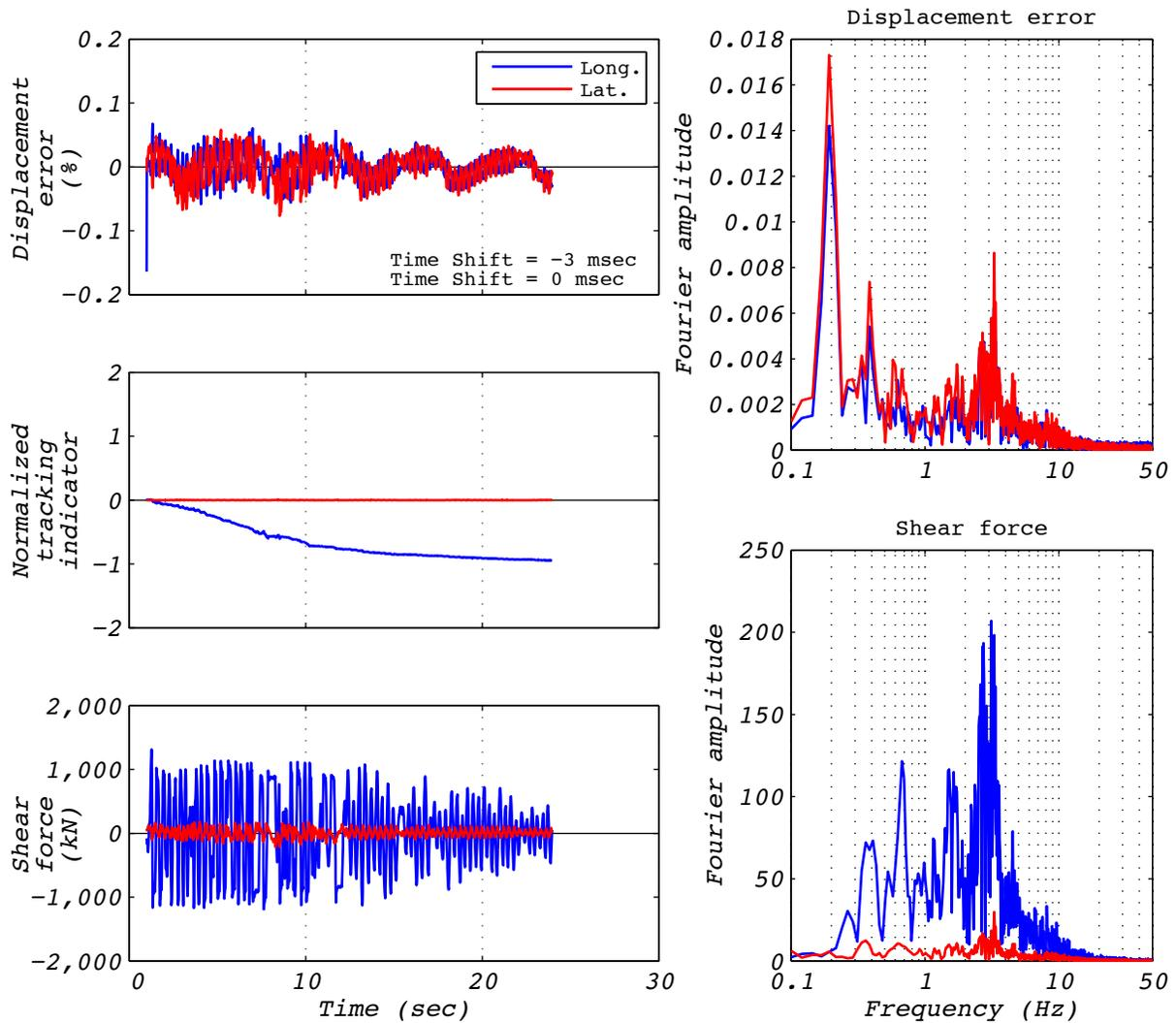
Figure C.1-1 Hybrid test performance metrics for run 17: EUR5, 1D with experimental bearing representing all bearings.
