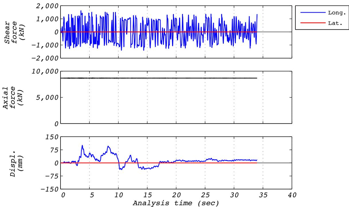
**Figure C.6-3 Hybrid test time history responses for run 22: NRC2, 1D with experimental bearing representing all bearings.**
