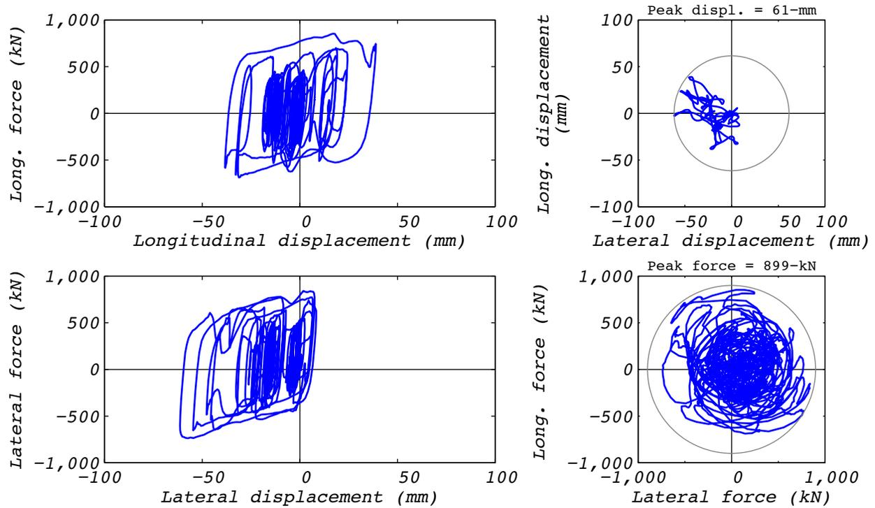
**Figure A.2-2 Hybrid test bearing response for run 25: EUR5, 2D with experimental bearing representing all bearings.**
