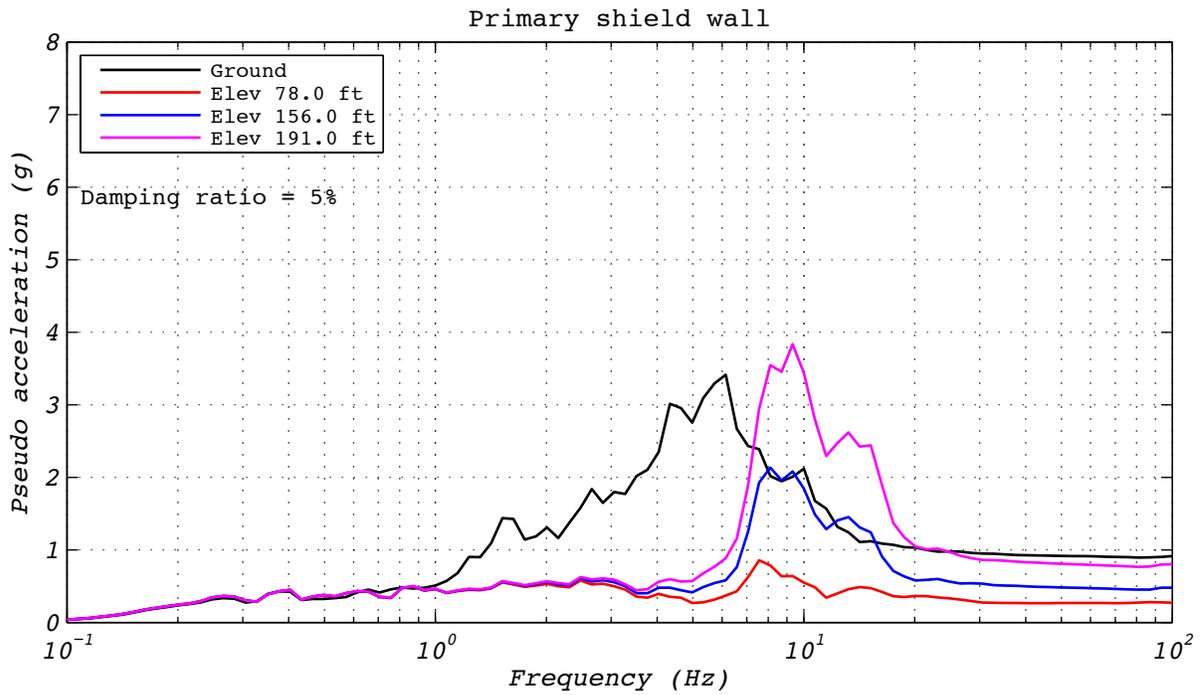
**Figure C.21-3 Floor spectra for analytical run 54A: NRC2, 2D with a single analytical bearing.**
