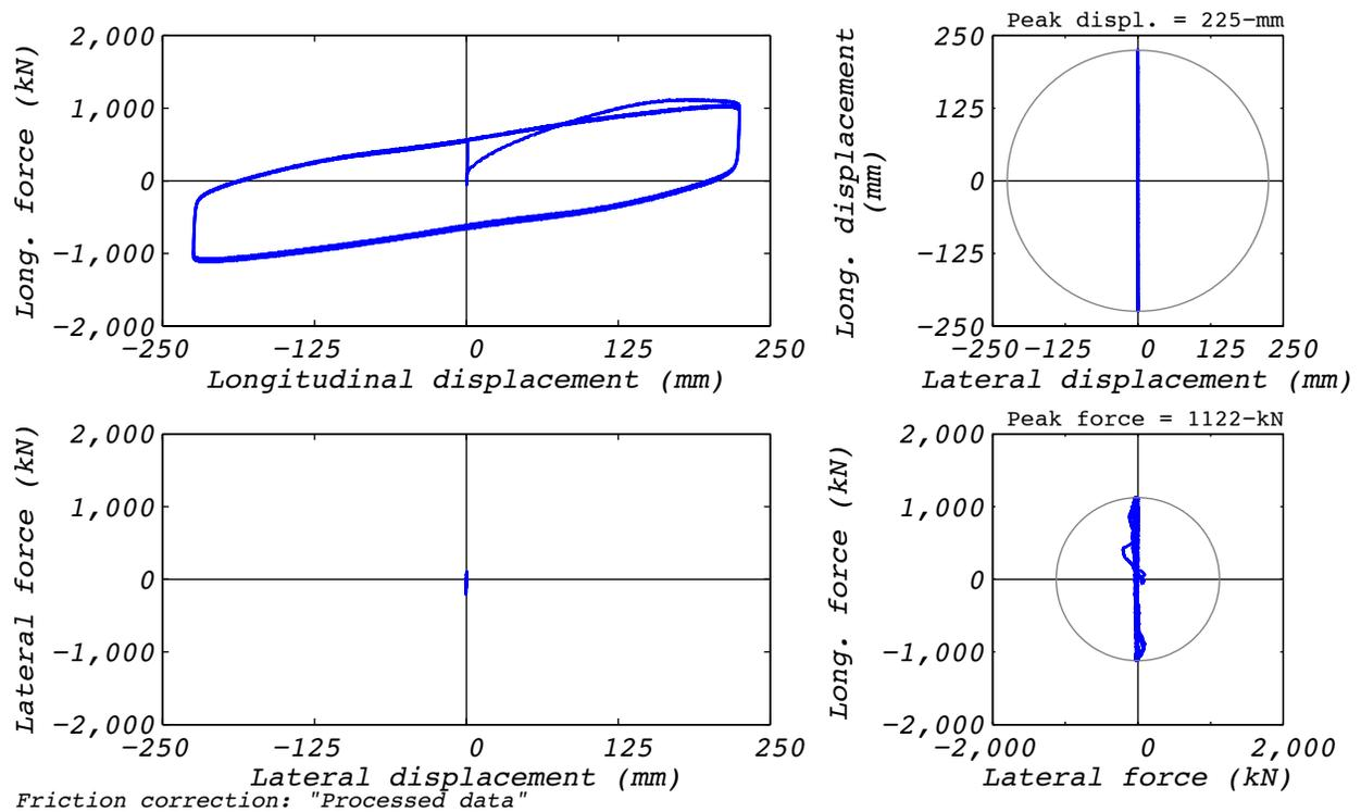
Figure B.31-2 Test run no. 74 hysteresis: Longitudinal (224 mm amplitude, 21,927 kN axial load, and 7 mm/s velocity).
