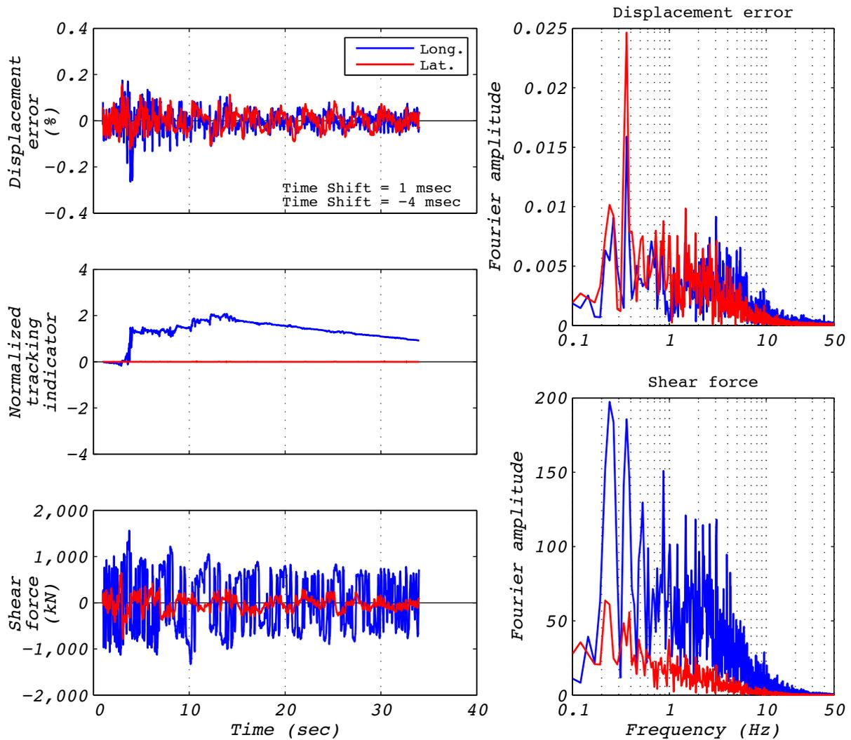
Figure C.16-1 Hybrid test performance metrics for run 52: NRC2, 1D with experimental bearing representing all bearings.
