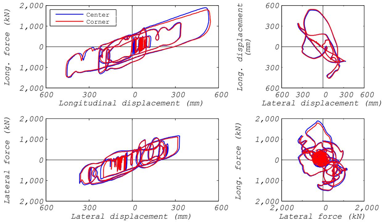
**Figure 3.48** LPRB bearing: comparison of bearing responses depending on the location of the bearing (ground motion NRC15, 3D analysis).
