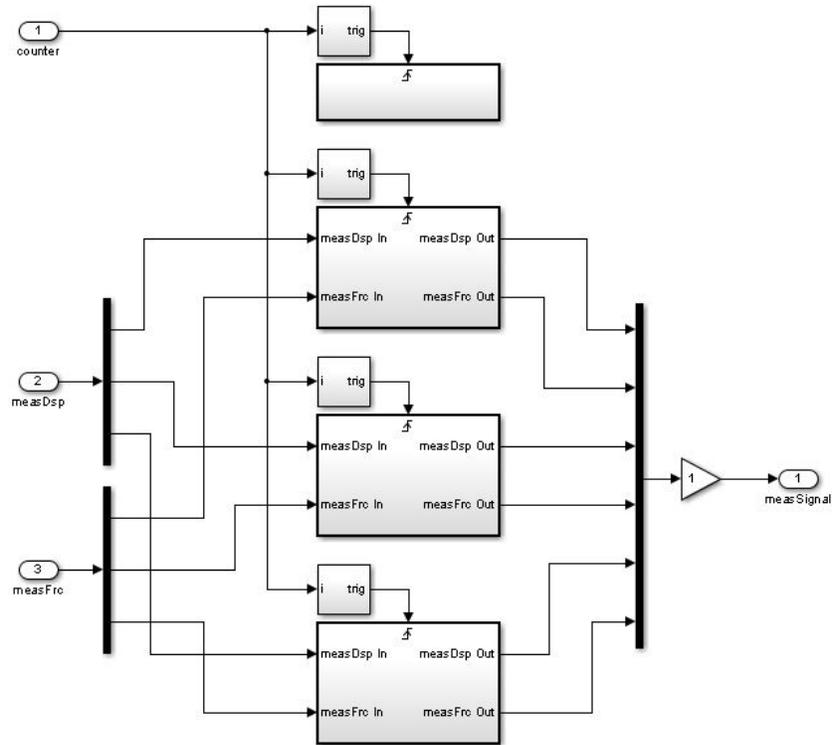
Figure 3.10 Delay model in simulink.
