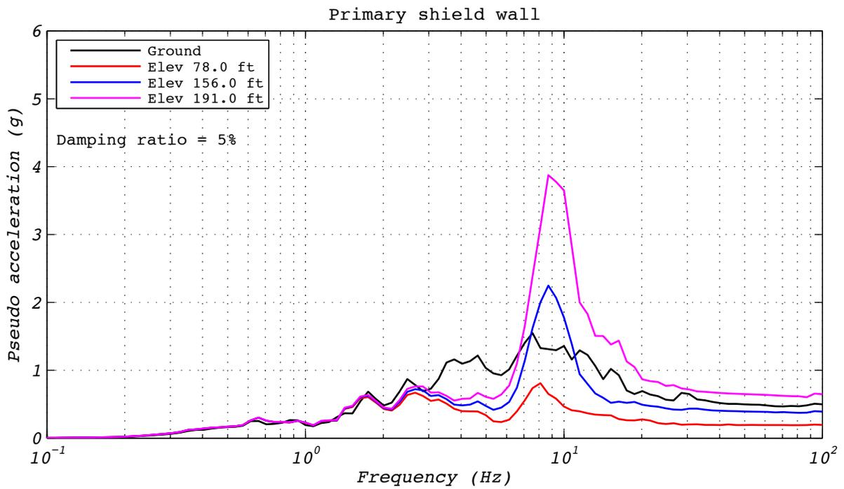
**Figure C.19-3 Floor spectra for analytical run 53A: EUR5, 1D with a single analytical bearing.**
