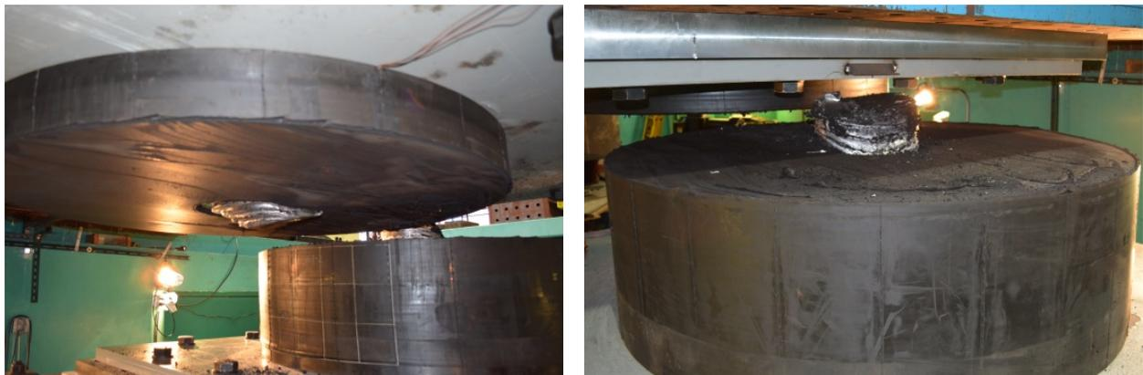
Figure 3.84 Failure of the LPRB (UET-2).
