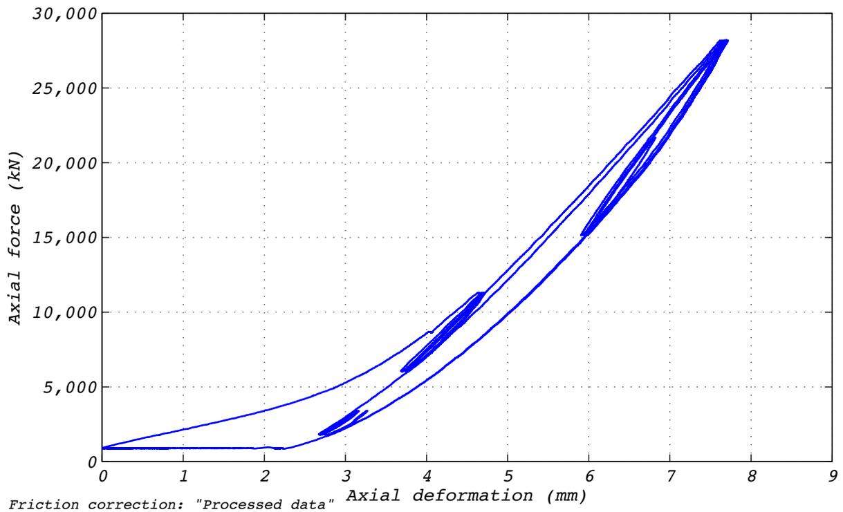
Figure B.8-2 Test run no. 17 hysteresis: Axial (224 mm amplitude and varying axial load).
