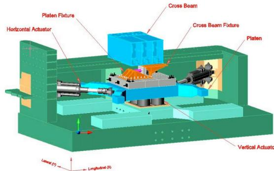
**Figure 3.15 Schematic of SRMD machine for the calibration.**
