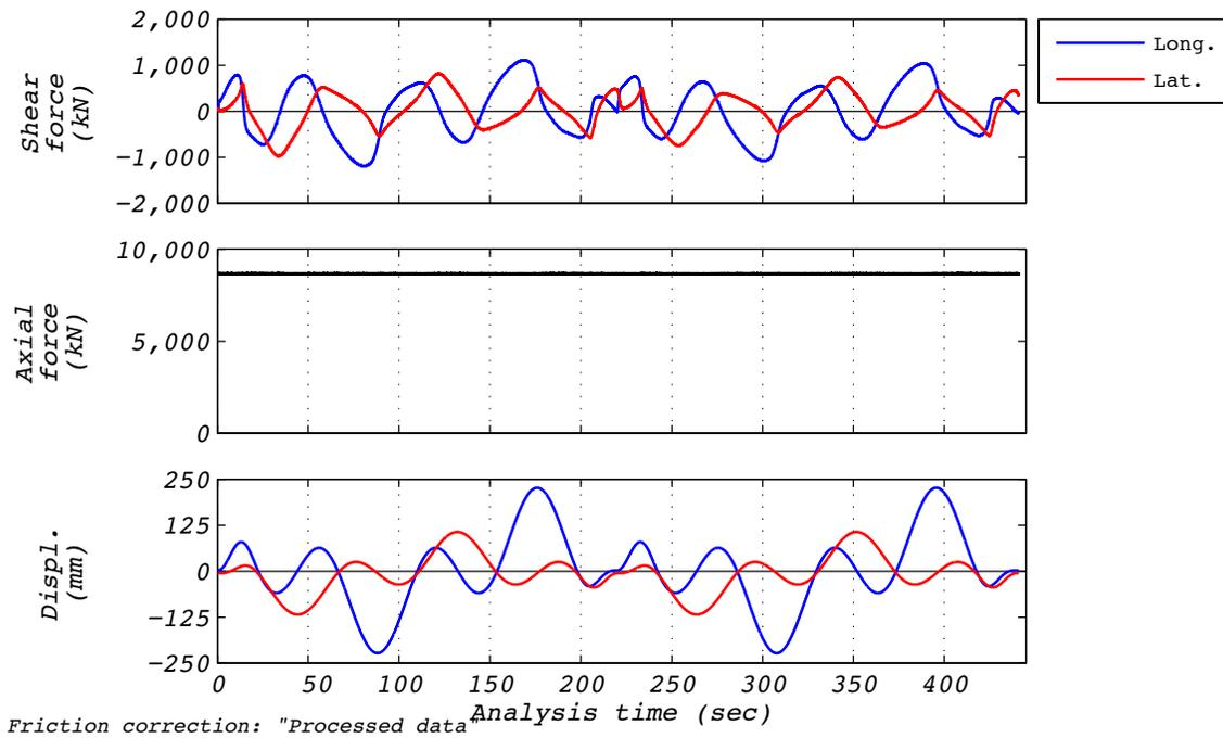
Figure B.18-1 Test run no. 57 time history: Clover leaf orbit (224 mm amplitude, 8,664 kN axial load, and varying velocity).
