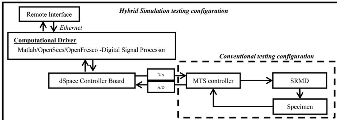
Figure 3.3 Hybrid simulation hardware configuration.
