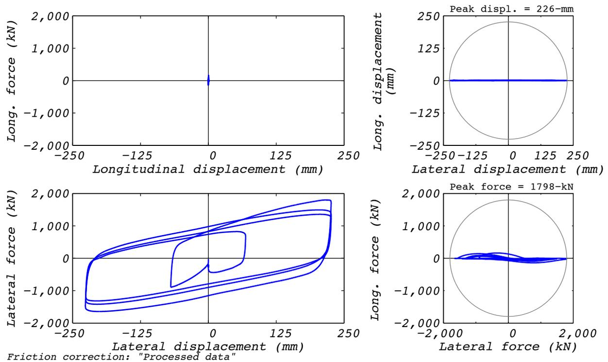
Figure B.27-2 Test run no. 70 hysteresis: Transverse (224 mm amplitude, 8,663 kN axial load, and 586 mm/s velocity).
