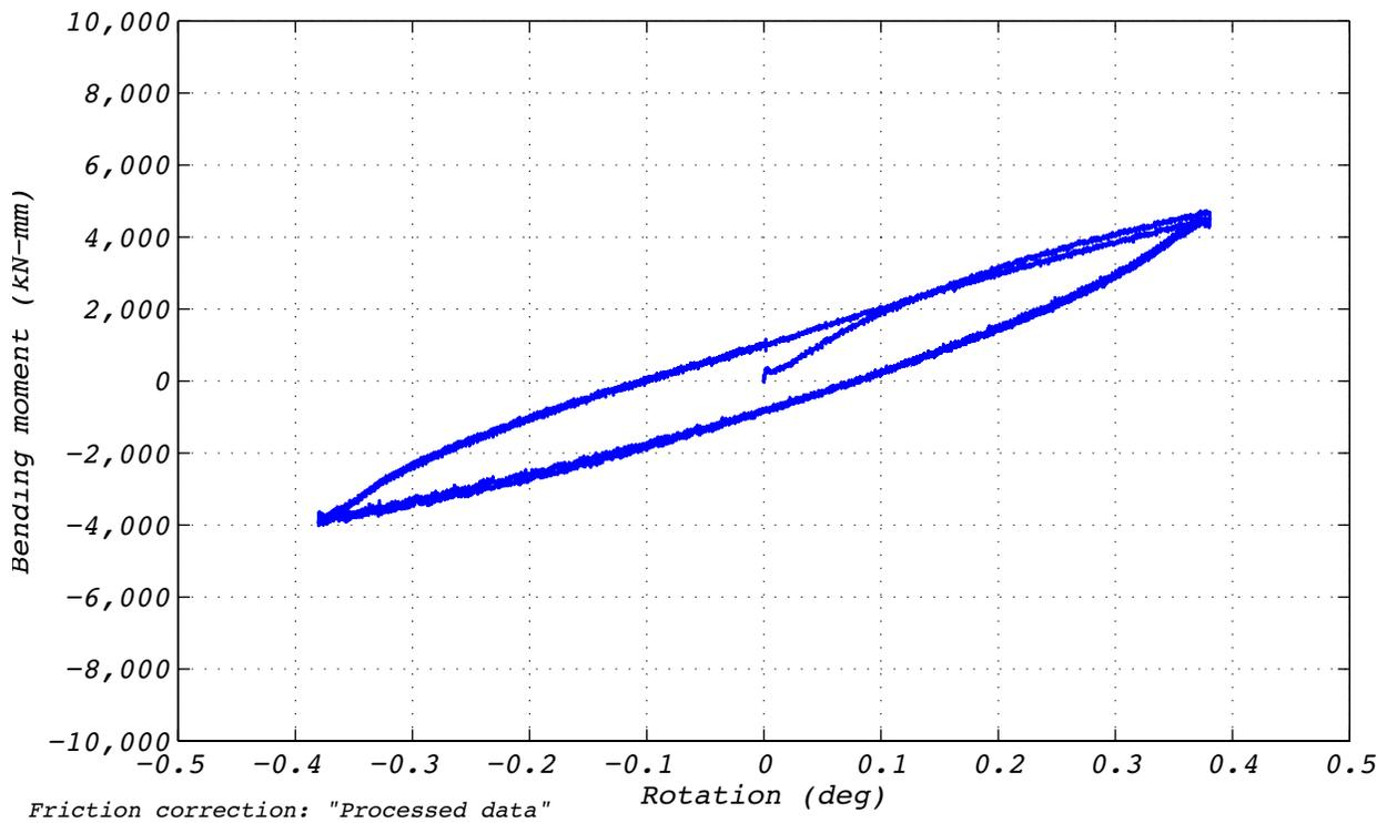
Figure D.7-2 Test run no. 7 hysteresis: Longitudinal rotation (0 mm displacement and 8,663 kN axial load).
