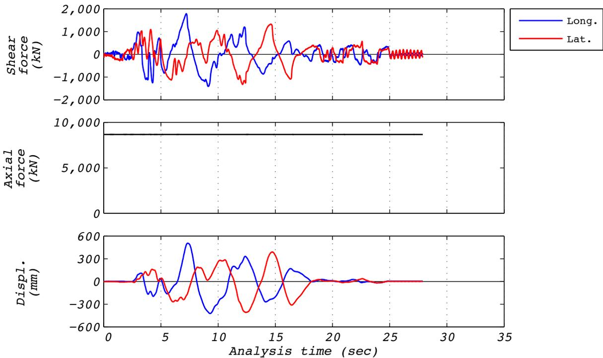
**Figure A.15-3 Hybrid test time history responses for run 55: NRC15, 2D with experimental bearing representing all bearings.**
