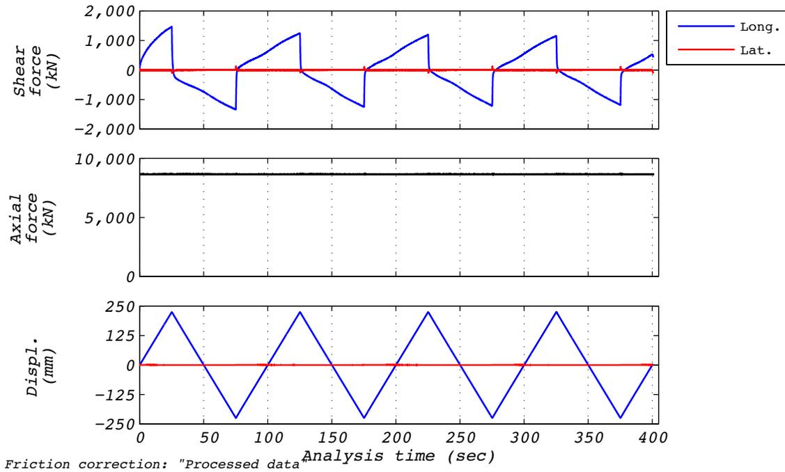
Figure B.29-1 Test run no. 72 time history: Longitudinal (224 mm amplitude, 8,663 kN axial load, and 9 mm/s velocity).
