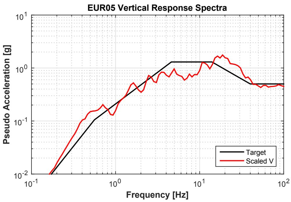
Figure 3.36 Response spectra of the EUR05 ground motion characterizing the EUR hazard level [2012]
