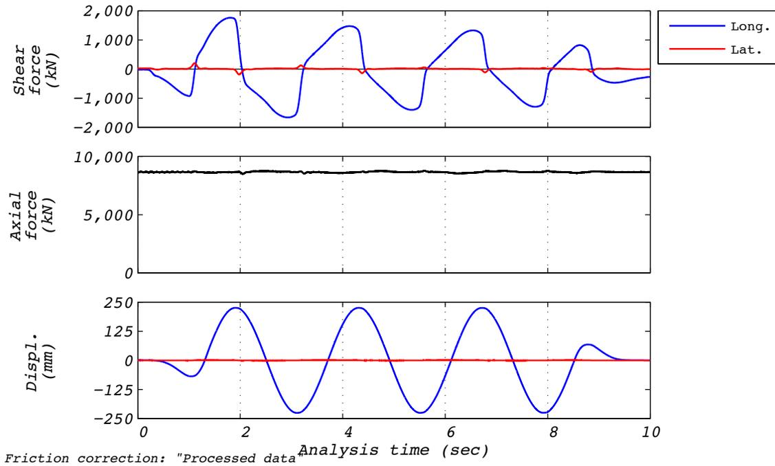
Figure B.19-1 Test run no. 59 time history: Longitudinal (224 mm amplitude, 8,663 kN axial load, and 586 mm/s velocity).
