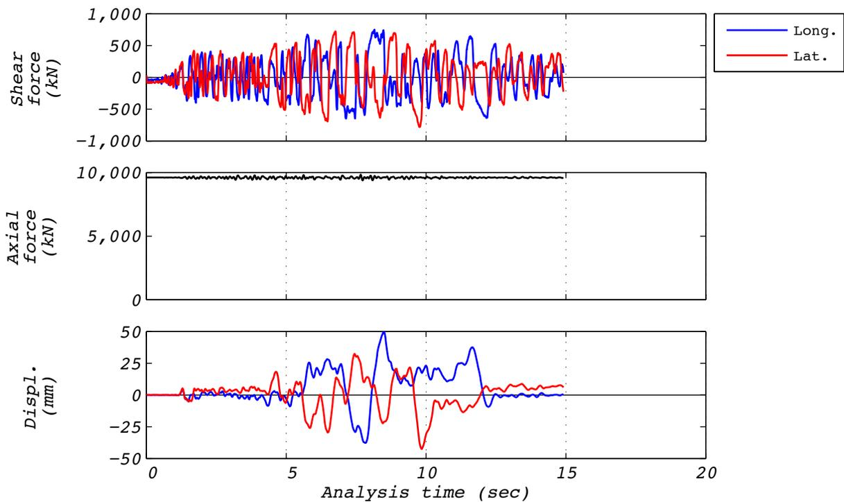
**Figure A.17-3 Hybrid test time history responses for run 58: EUR5, 2D with experimental bearing representing one of 527 bearings.**
