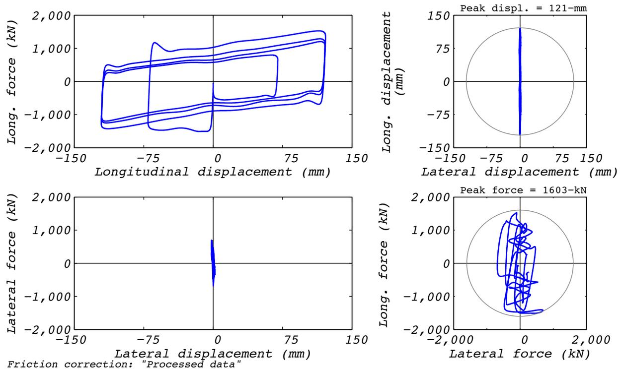
Figure D.17-2 Test run no. 20 hysteresis: Longitudinal (120 mm amplitude, 8,663 kN axial load, and 410 mm/s velocity).
