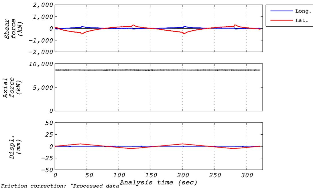
Figure D.7-1 Test run no. 7 time history: Longitudinal rotation (0 mm displacement and 8,663 kN axial load).
