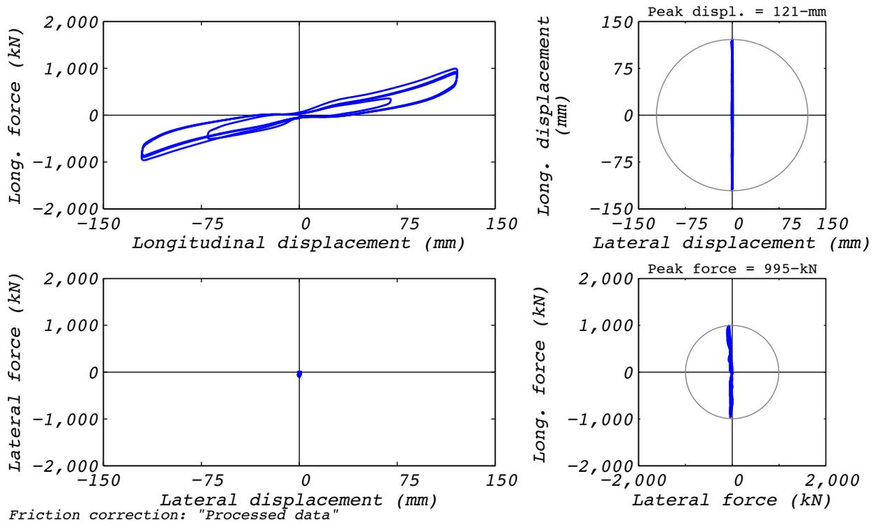
Figure D.11-2 Test run no. 11 hysteresis: Longitudinal (120 mm amplitude, 0 kN axial load, and 410 mm/s velocity).
