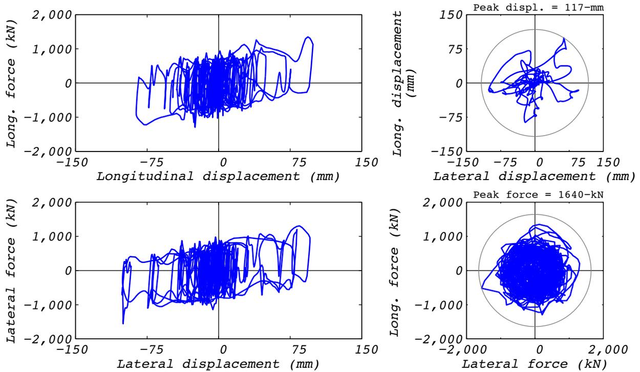
Figure C.12-2 Hybrid test bearing response for run 48: NRC2, 3D with 5 groups and the experimental bearing representing the no. 3 corner group.
