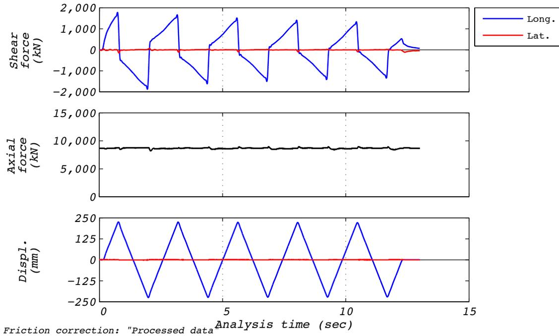
Figure B.28-1 Test run no. 71 time history: Longitudinal (224 mm amplitude, 8,663 kN axial load, and 373 mm/s velocity).
