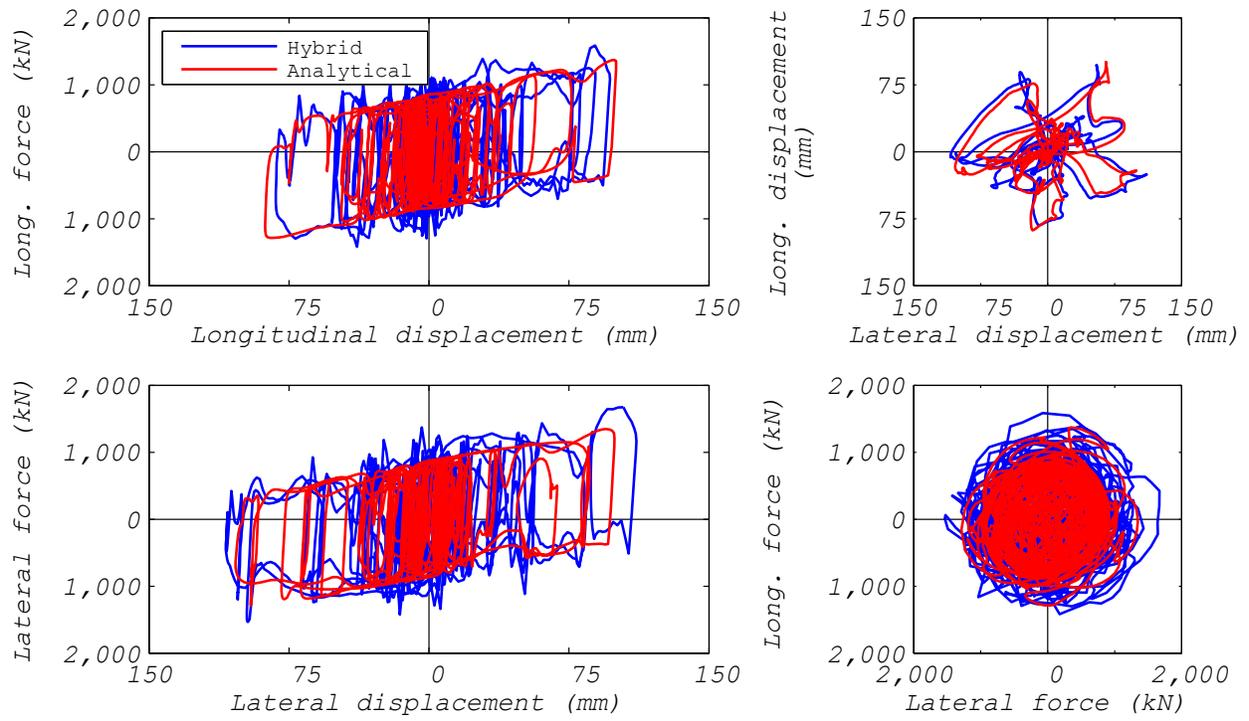
**Figure 3.82** EQS bearing: comparison of hybrid simulation and analytical estimation responses (ground motion NRC2, 2D analysis).
