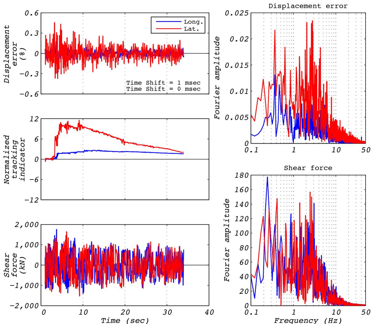
Figure C.8-1 Hybrid test performance metrics for run 43: NRC2, 3D with 5 groups of bearings and the experimental bearing representing the center group.
