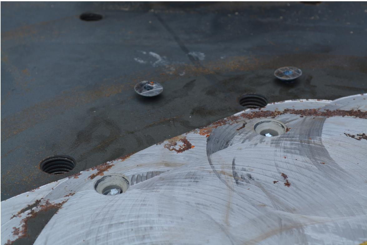
**Figure 3.26** Unison bearing cover plate bolt failure.
