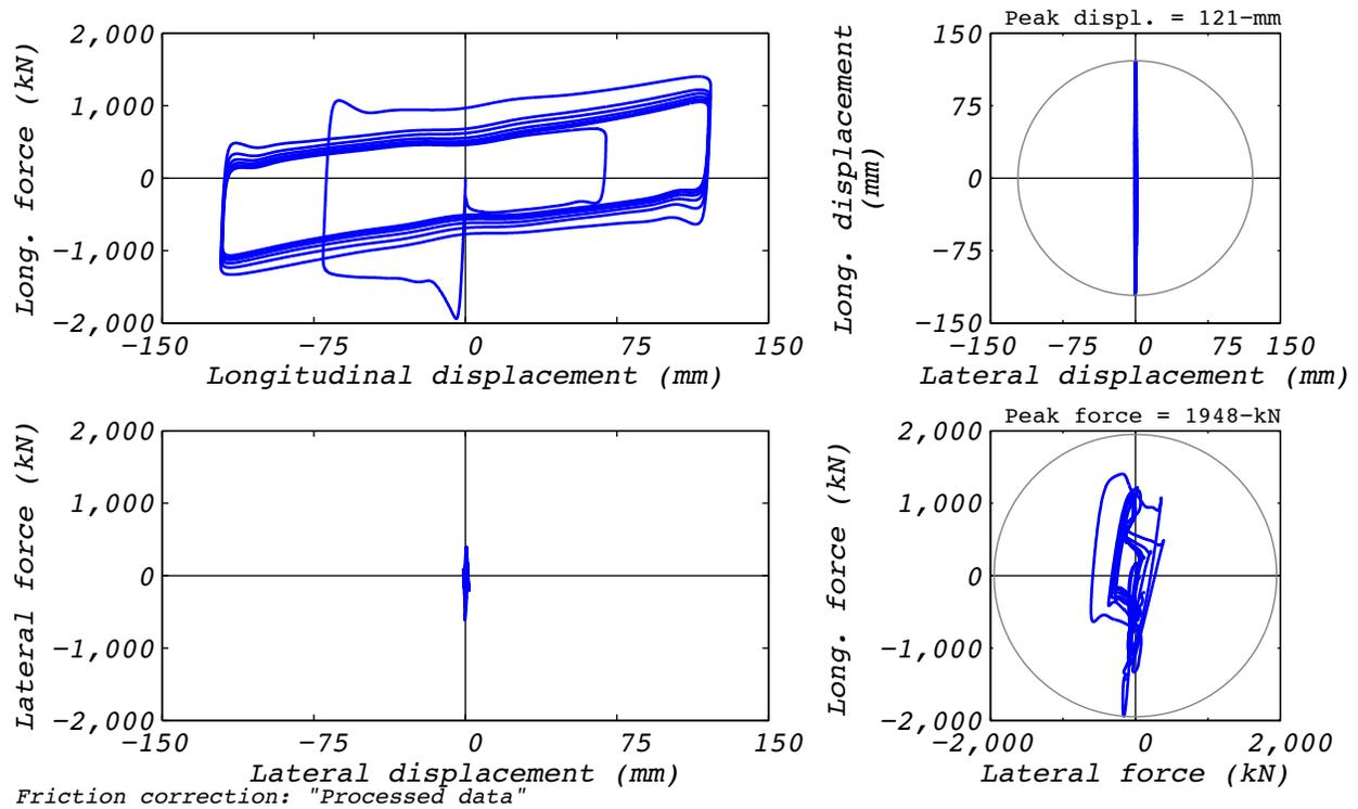
Figure D.20-2 Test run no. 26 hysteresis: Longitudinal (120 mm amplitude, 8,663 kN axial load, and 410 mm/s velocity).
