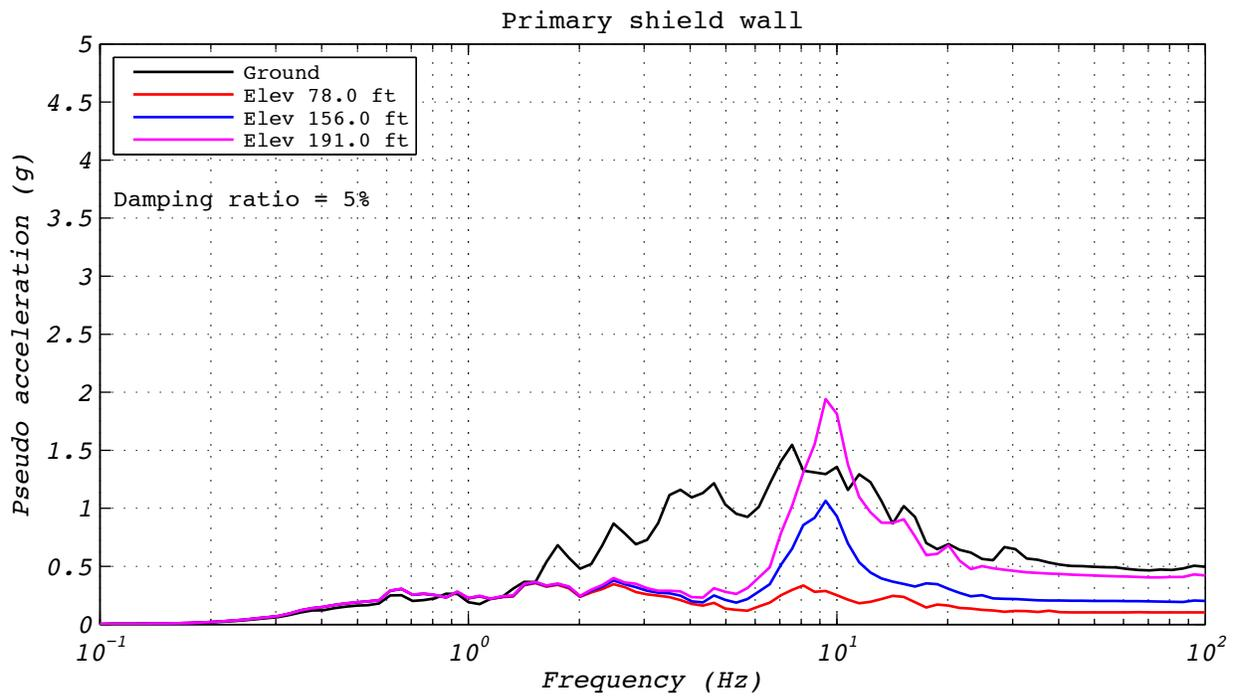
**Figure A.8-4 Hybrid test floor spectra for run 44: EUR5, 1D with experimental bearing representing all bearings.**
