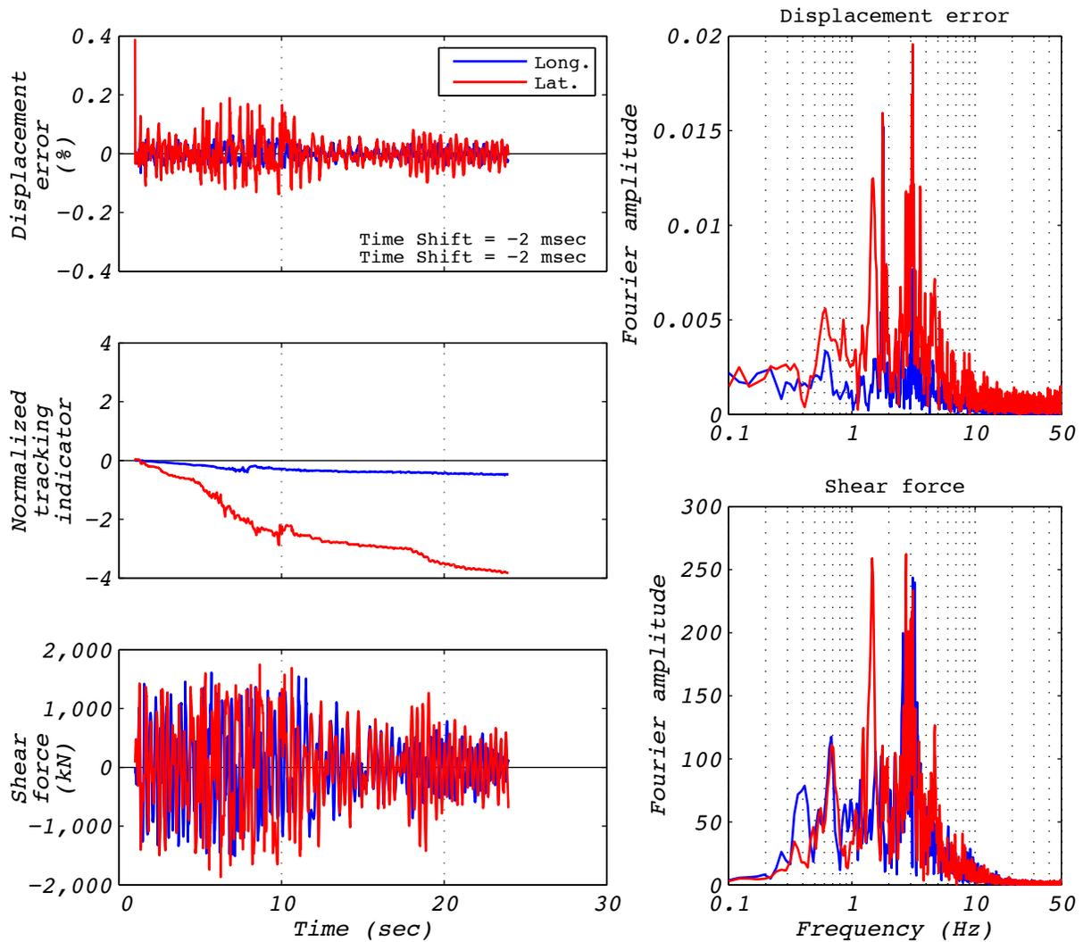
Figure C.2-1 Hybrid test performance metrics for run 18: EUR5, 2D with experimental bearing representing all bearings.
