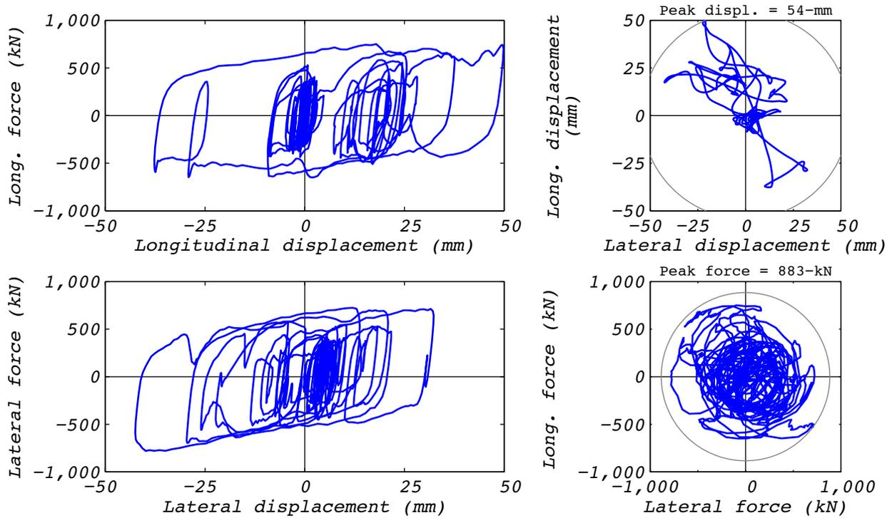
**Figure A.17-2 Hybrid test bearing response for run 58: EUR5, 2D with experimental bearing representing one of 527 bearings.**
