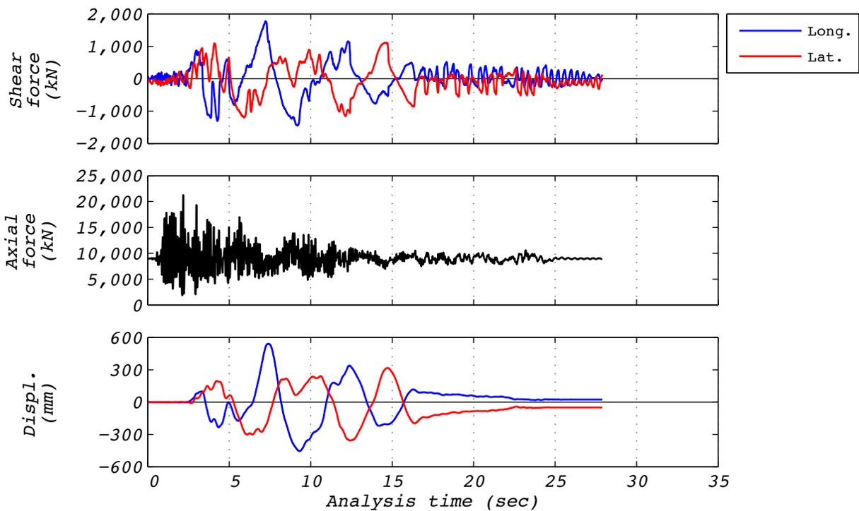
Figure A.30-3 Hybrid test time history responses for run 89: NRC15, 3D with 5 groups and the experimental bearing representing the no. 3 corner group.
