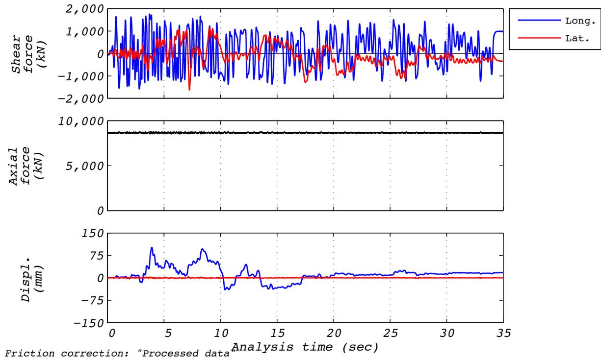
**Figure C.7-2 Time history responses for real-time reproduction of hybrid test run 22: NRC2, 1D with experimental bearing representing all bearings.**
