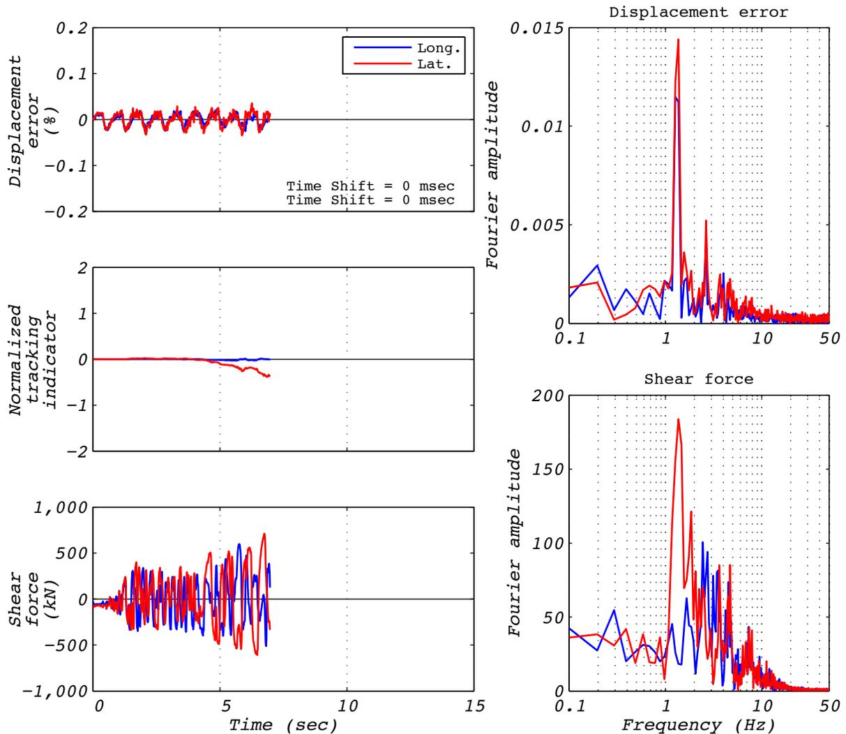
Figure A.18-1 Hybrid test performance metrics for run 60: EUR5, 2D with experimental bearing representing one of 527 bearings.
