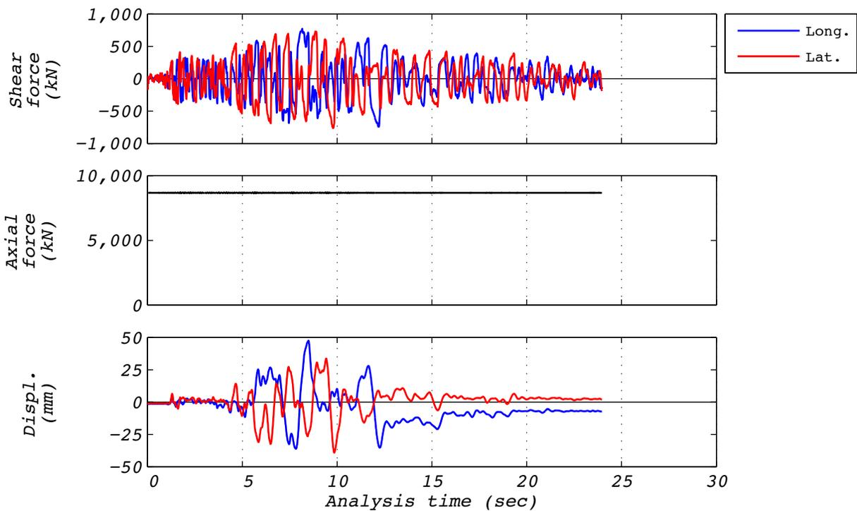
**Figure A.10-3 Hybrid test time history responses for run 45: EUR5, 2D with experimental bearing representing all bearings.**
