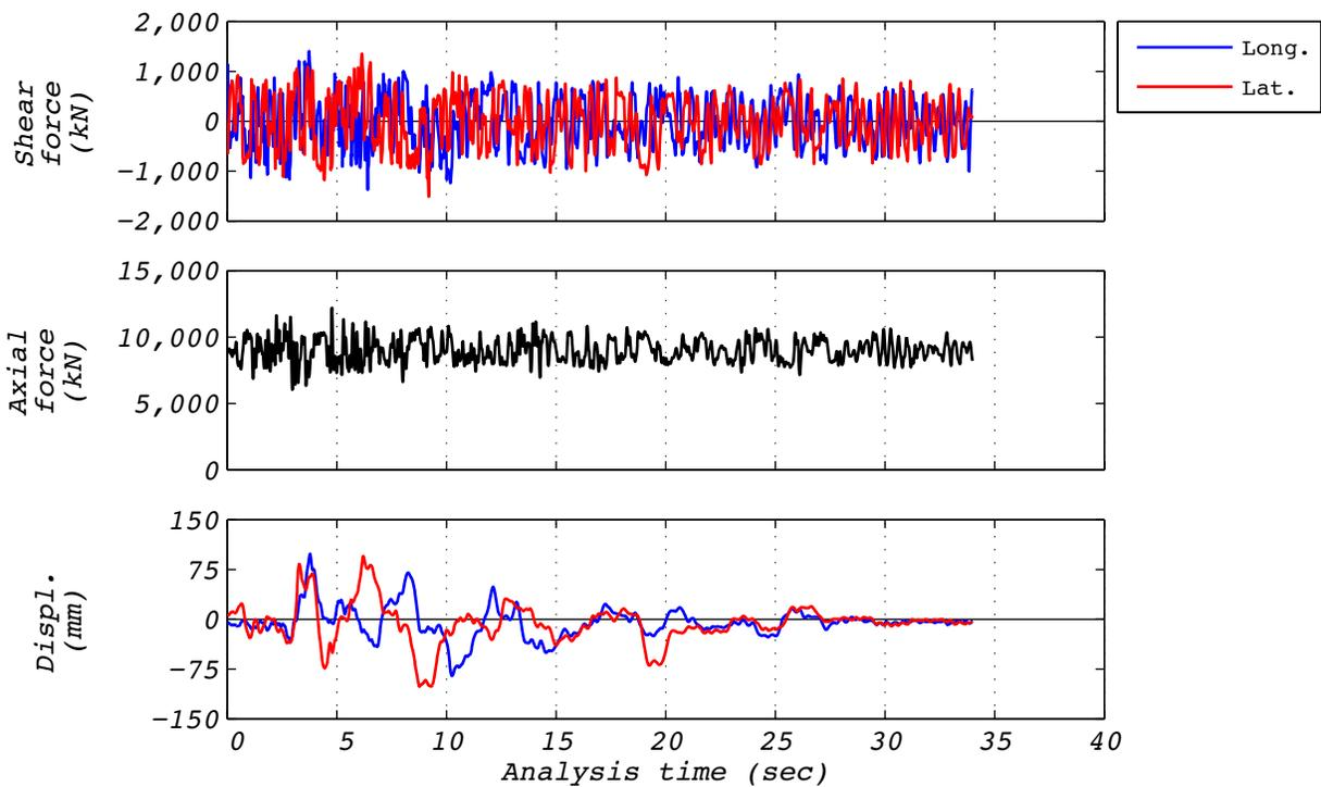
**Figure C.13-3 Hybrid test time history responses for run 49: NRC2, 3D with 5 groups and the experimental bearing representing the no. 3 corner group.**
