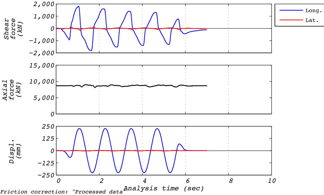
Figure B.30-1 Test run no. 73 time history: Longitudinal (224 mm amplitude, 8,663 kN axial load, and 1,173 mm/s velocity).
