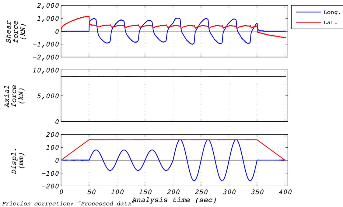
Figure B.20-1 Test run no. 62 time history: Bidirectional (224 mm amplitude, 8,663 kN axial load, and 28 mm/s velocity).
