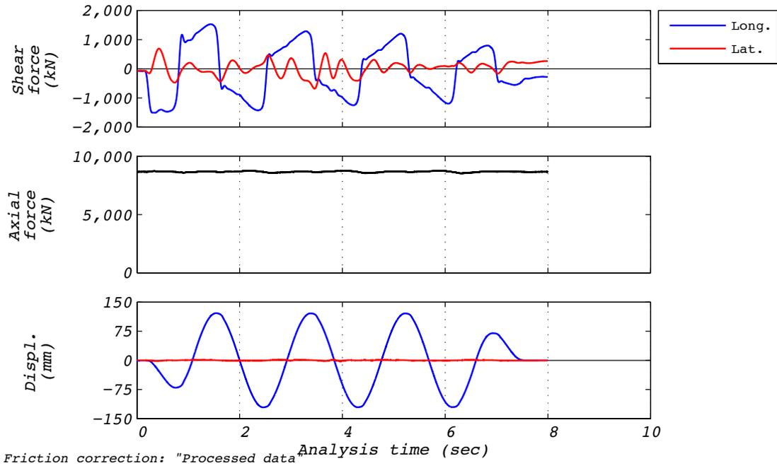
Figure D.17-1 Test run no. 20 time history: Longitudinal (120 mm amplitude, 8,663 kN axial load, and 410 mm/s velocity).
