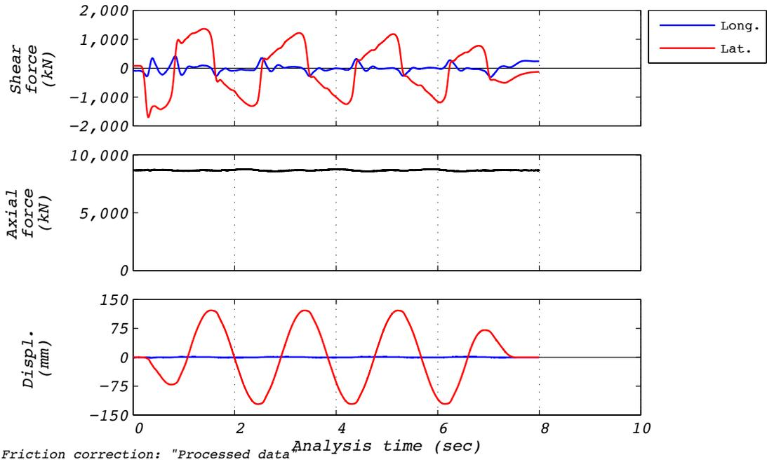
Figure D.32-1 Test run no. 60 time history: Transverse (120 mm amplitude, 8,663 kN axial load, and 410 mm/s velocity).
