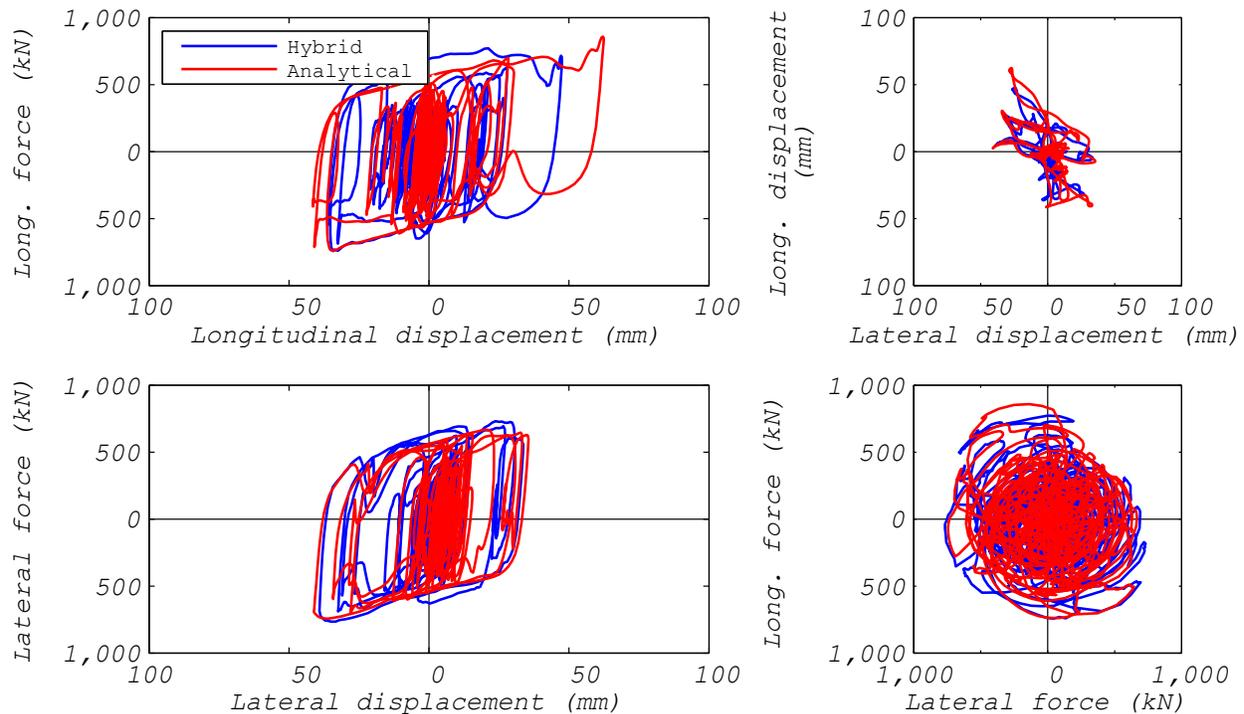
**Figure 3.56 LPRB bearing: comparison of hybrid simulation and analytical estimation bearing responses (ground motion EUR5, 2D analysis).**
