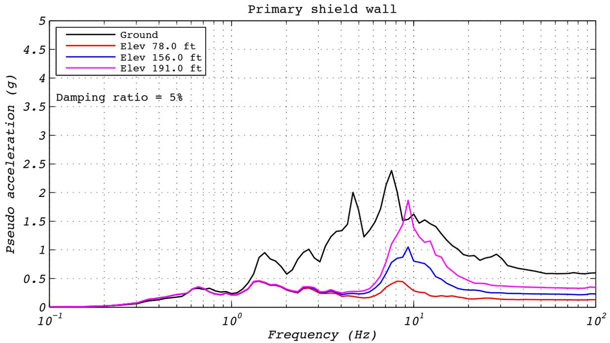
**Figure A.11-3 Floor spectra for analytical run 45A: EUR5, 2D with a single analytical bearing.**
