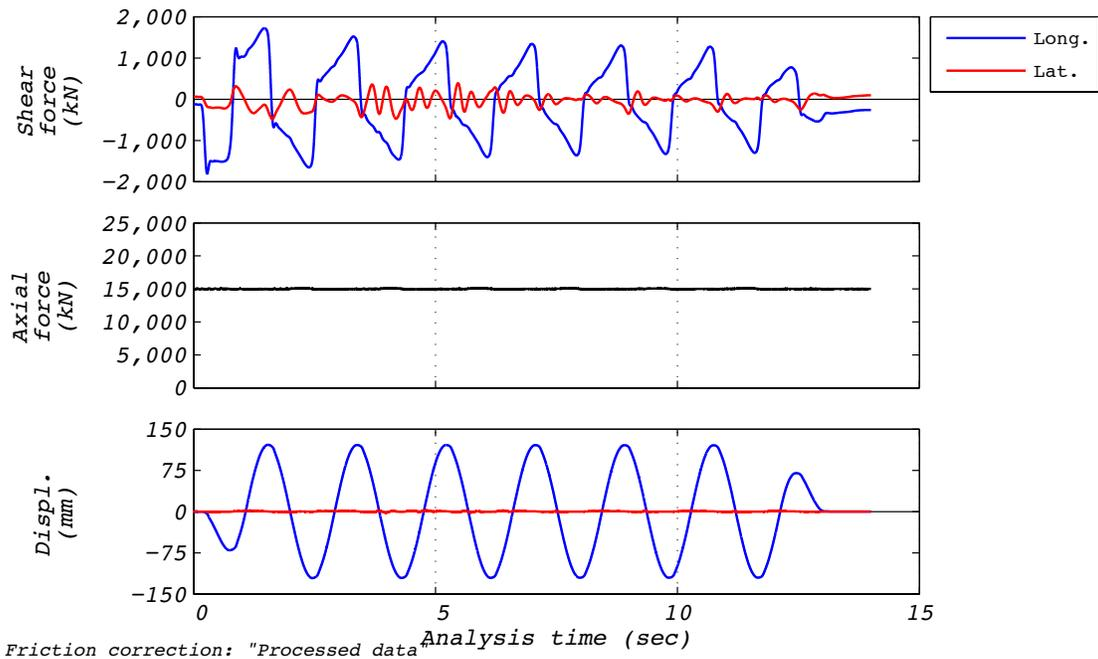
Figure D.14-1 Test run no. 14 time history: Longitudinal (120 mm amplitude, 15,000 kN axial load, and 410 mm/s velocity).
