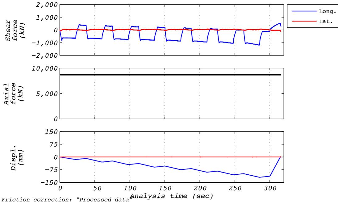
Figure D.28-1 Test run no. 34 time history: Longitudinal (120 mm amplitude, 8,663 kN axial load).
