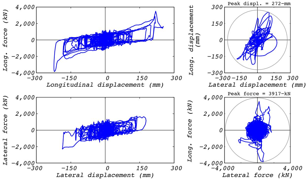
**Figure C.24-2 Hybrid test bearing response for run 58: NRC10, 2D with experimental bearing representing all bearings.**
