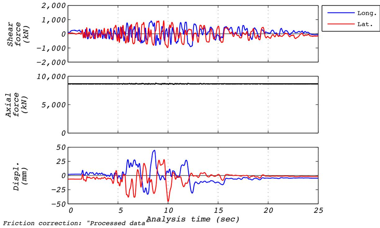
**Figure A.5-2 Time history responses for real-time reproduction of hybrid test run 26: EUR5, 2D with experimental bearing representing all bearings.**
