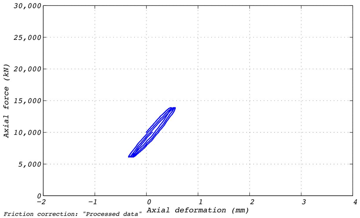
Figure D.4-2 Test run no. 4 hysteresis: Axial (0 mm displacement and varying axial load).
