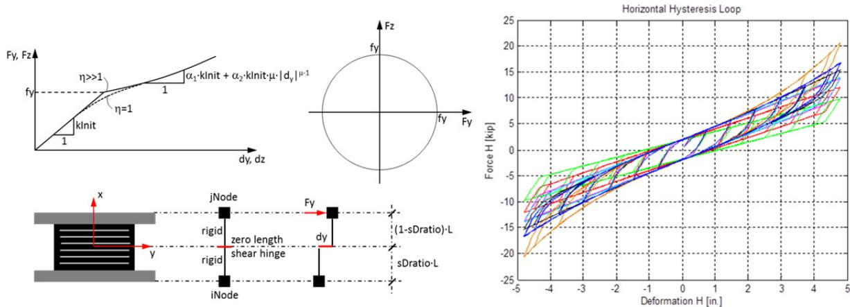
Figure 3.17 New OpenSees elastomeric isolator based on enhanced Bouc-Wen material properties.
