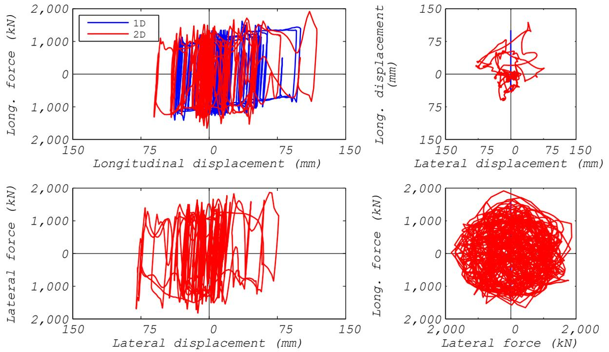
**Figure 3.62** EQS bearing: comparison of bearing responses to ground motion NRC2 executed 25 times slower than real time (1D and 2D analyses).
