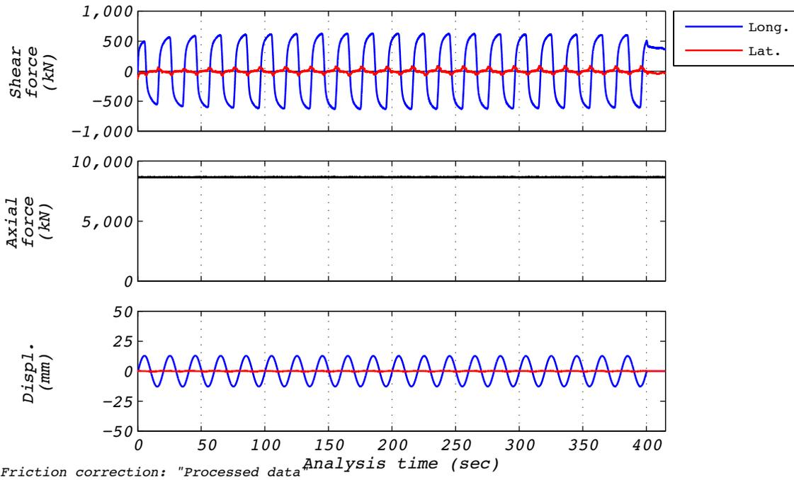
Figure B.34-1 Test run no. 81 time history: Longitudinal (13 mm amplitude, 8,663 kN axial load, and 4 mm/s velocity).
