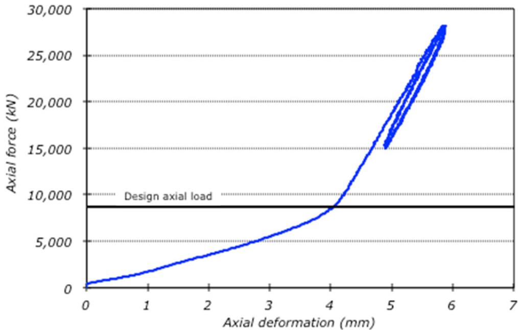
Figure 2.3 LPRB axial quality-control test.
