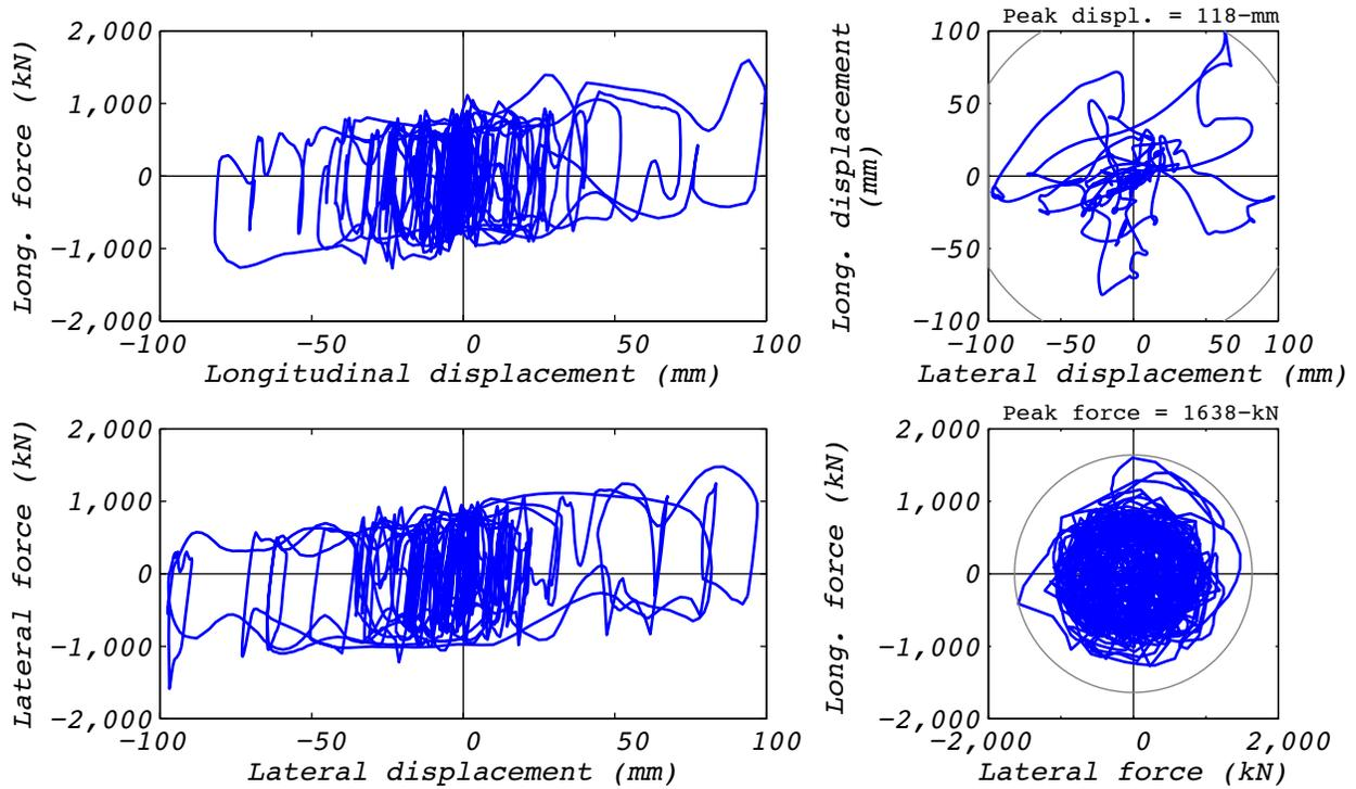
**Figure C.11-2 Hybrid test bearing response for run 47: NRC2, 3D with 5 groups of bearings and the experimental bearing representing the center group.**
