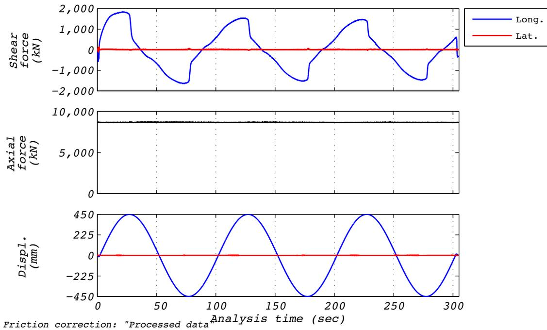
Figure B.21-1 Test run no. 64 time history: Longitudinal (448 mm amplitude, 8,663 kN axial load, and 28 mm/s velocity).
