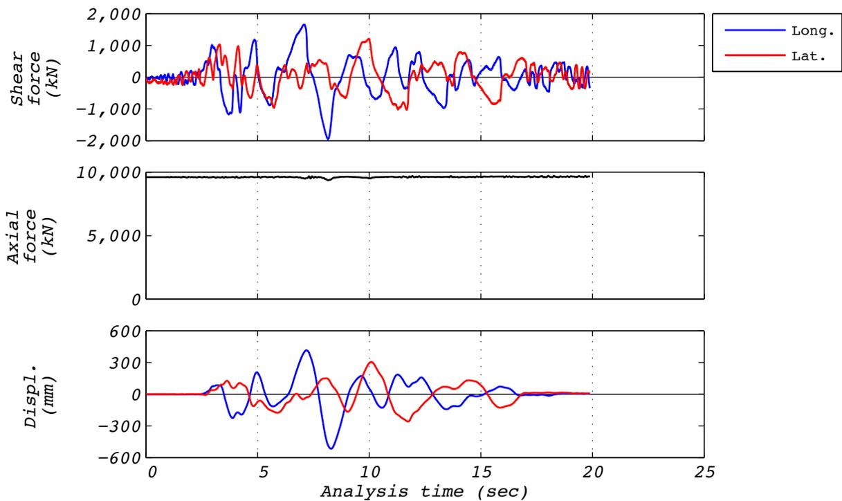
Figure A.19-3 Hybrid test time history responses for run 61: NRC15, 2D with experimental bearing representing one of 527.
