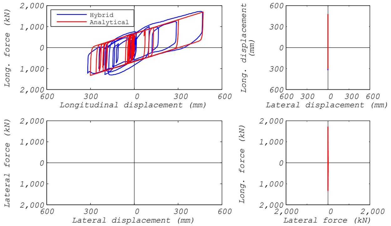
**Figure 3.54** LPRB bearing: comparison of hybrid simulation and analytical estimation bearing responses (ground motion NRC15, 1D analysis).
