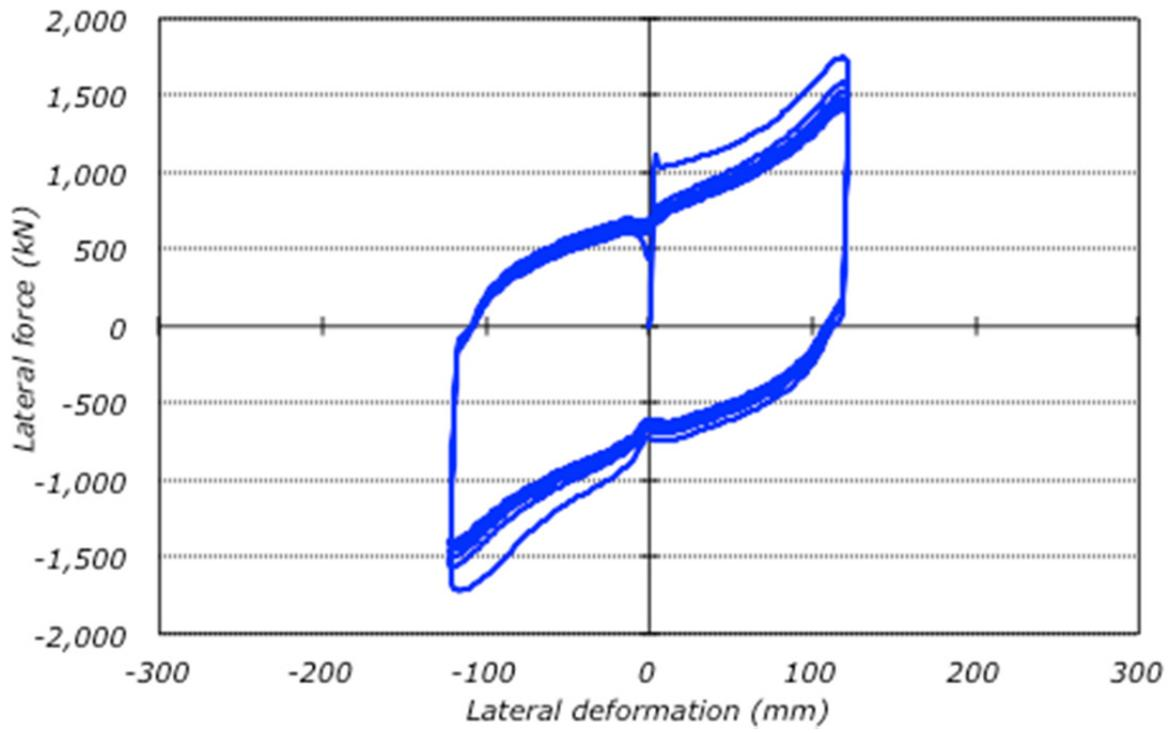
Figure 2.5 EQS lateral quality control test.
