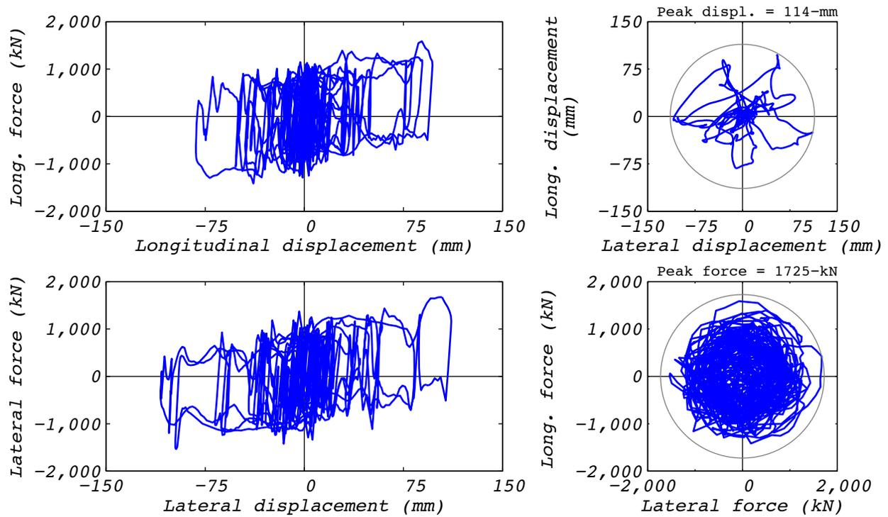
Figure C.20-2 Hybrid test bearing response for run 54: NRC2, 2D with experimental bearing representing all bearings.
