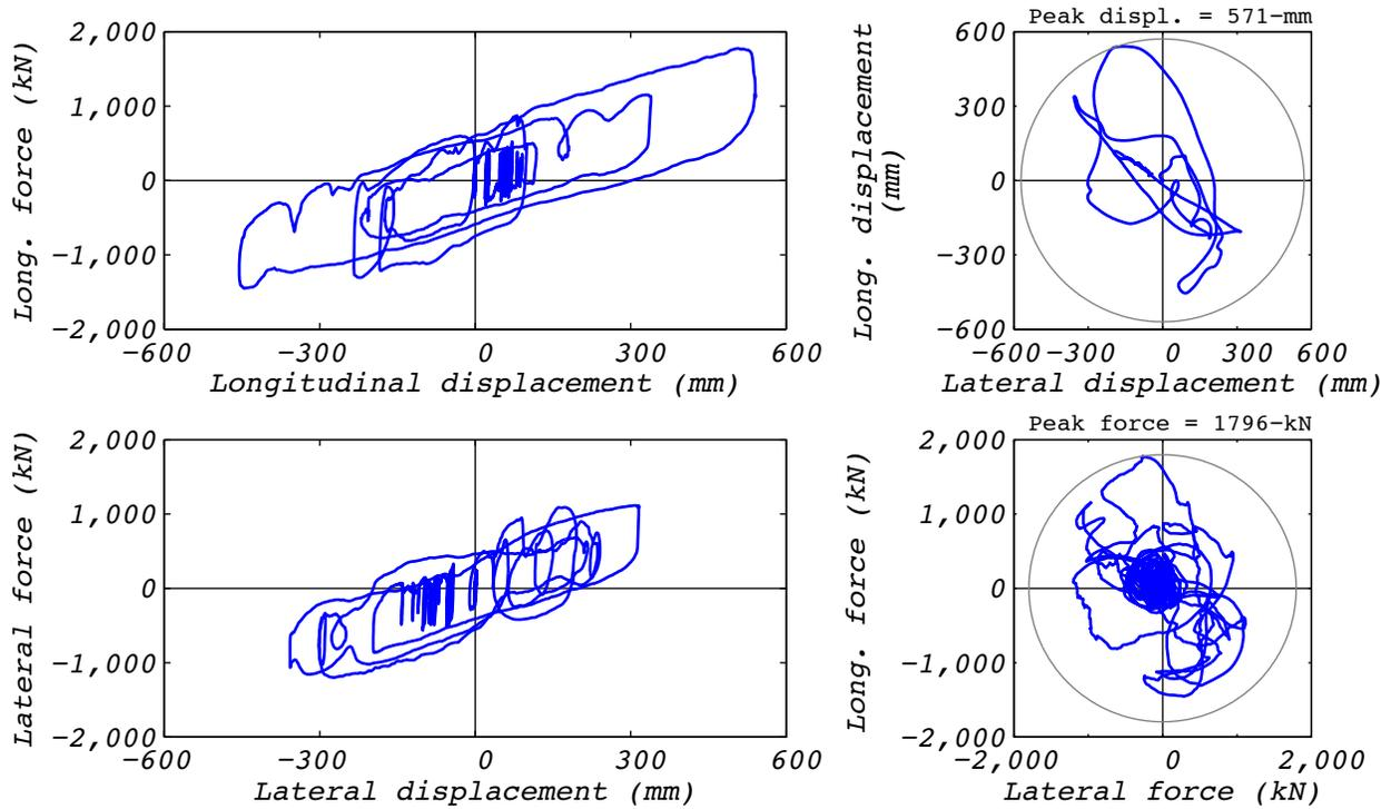
Figure A.30-2 Hybrid test bearing response for run 89: NRC15, 3D with 5 groups and the experimental bearing representing the no. 3 corner group.
