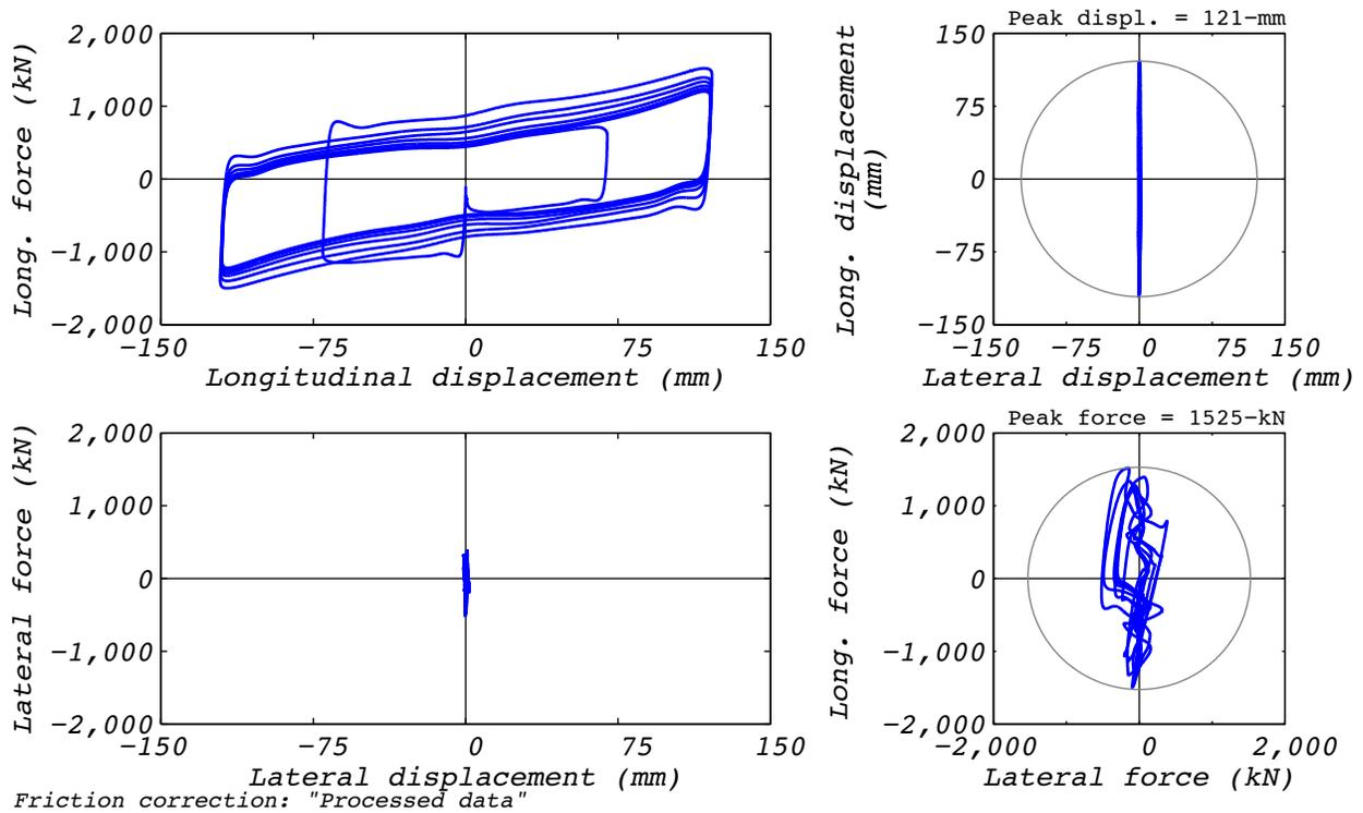
Figure D.13-2 Test run no. 13 hysteresis: Longitudinal (120 mm amplitude, 5,000 kN axial load, and 410 mm/s velocity).
