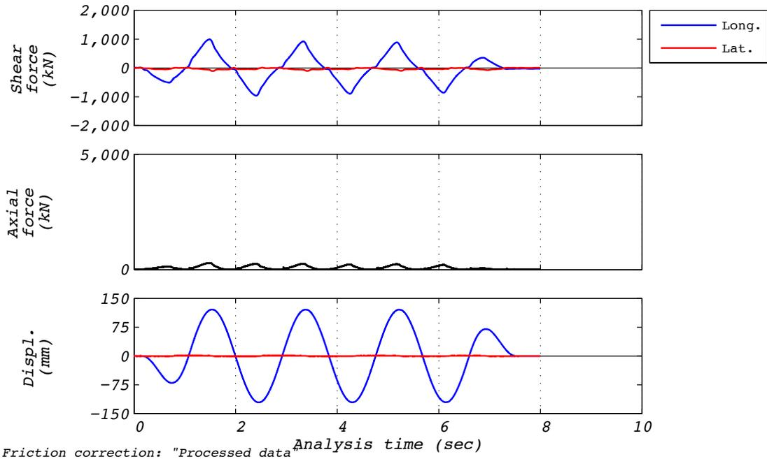
Figure D.11-1 Test run no. 11 time history: Longitudinal (120 mm amplitude, 0 kN axial load, and 410 mm/s velocity).
