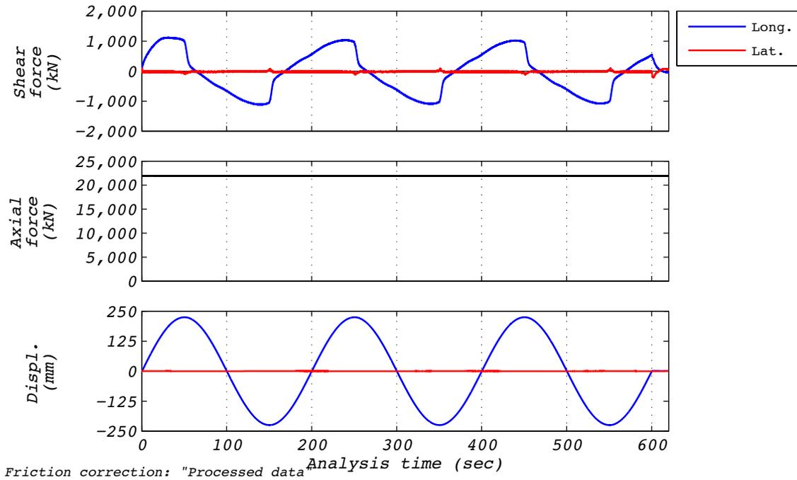
Figure B.31-1 Test run no. 74 time history: Longitudinal (224 mm amplitude, 21,927 kN axial load, and 7 mm/s velocity).
