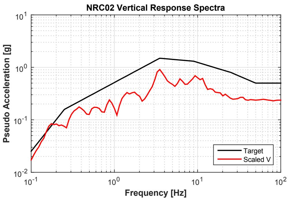
Figure 3.37 Response spectra of the NRC02 ground motion characterizing the NRC hazard level [1973].
