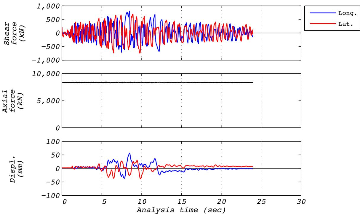
**Figure A.23-3 Hybrid test time history responses for run 80: EUR5, 3D with 5 groups of bearings and the experimental bearing representing the center group.**
