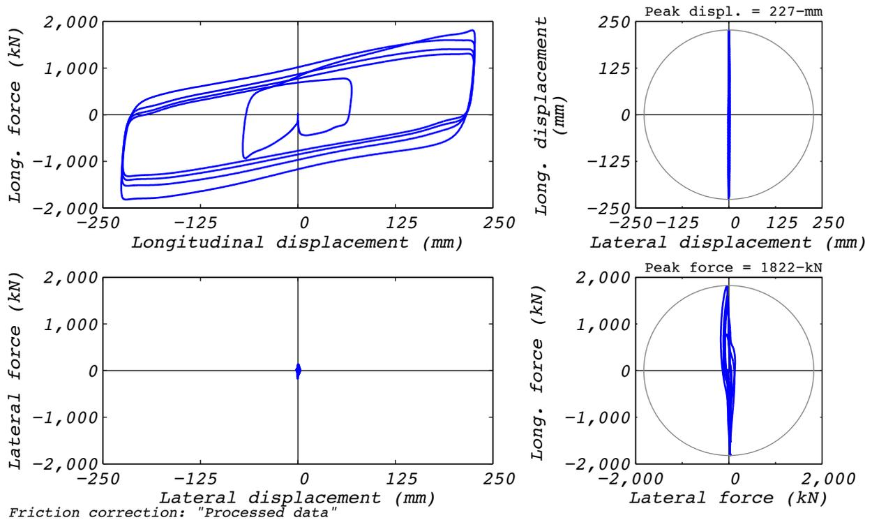
Figure B.30-2 Test run no. 73 hysteresis: Longitudinal (224 mm amplitude, 8,663 kN axial load, and 1,173 mm/s velocity).
