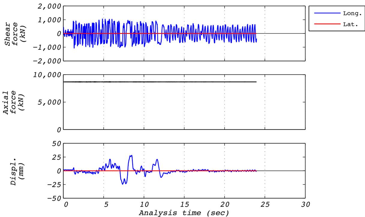
**Figure C.18-3 Hybrid test time history responses for run 53: EUR5, 1D with experimental bearing representing all bearings.**
