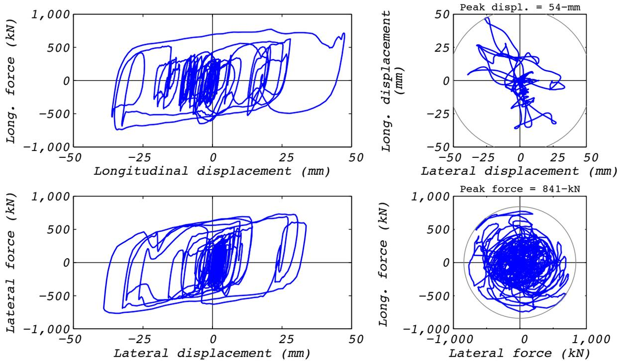
**Figure A.10-2 Hybrid test bearing response for run 45: EUR5, 2D with experimental bearing representing all bearings.**
