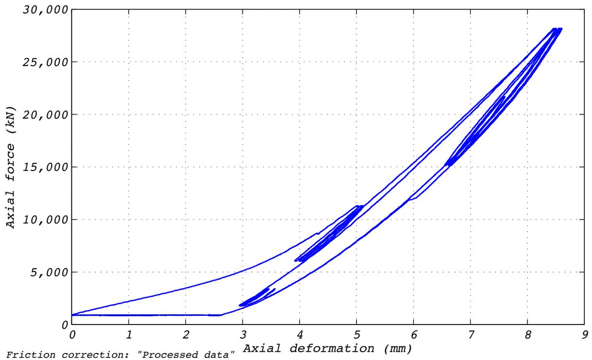
Figure B.9-2 Test run no. 18 hysteresis: Axial (336 mm amplitude and varying axial load).
