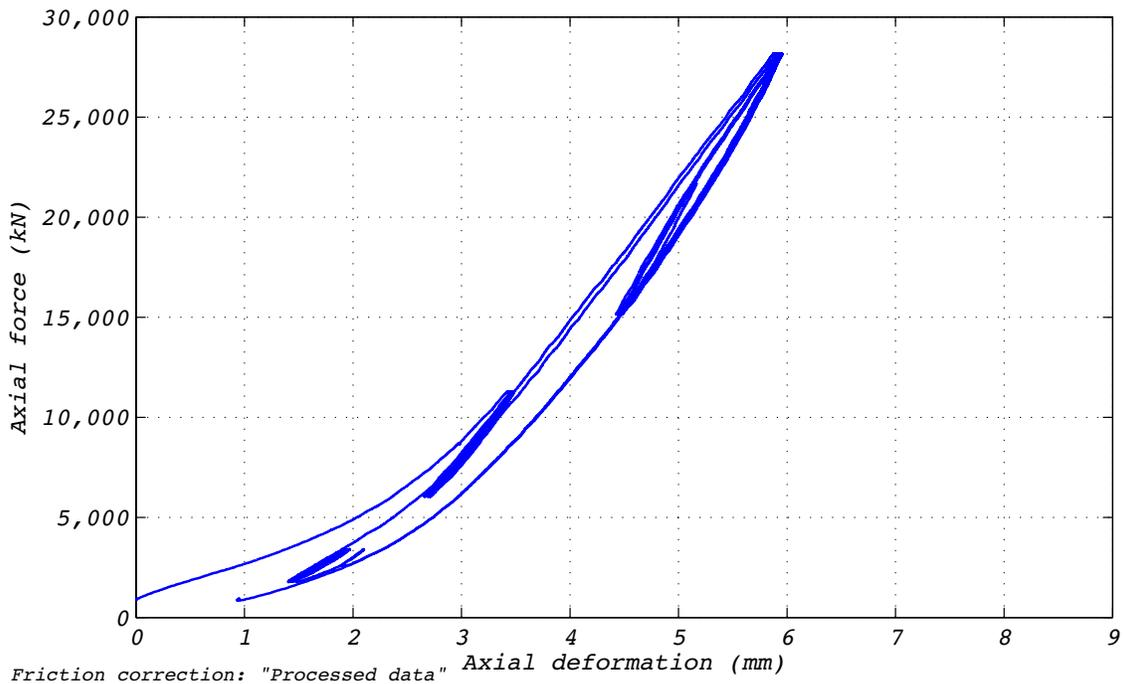
Figure B.1-2 Test run no. 8 hysteresis: Axial compression (0 mm amplitude and varying axial load).
