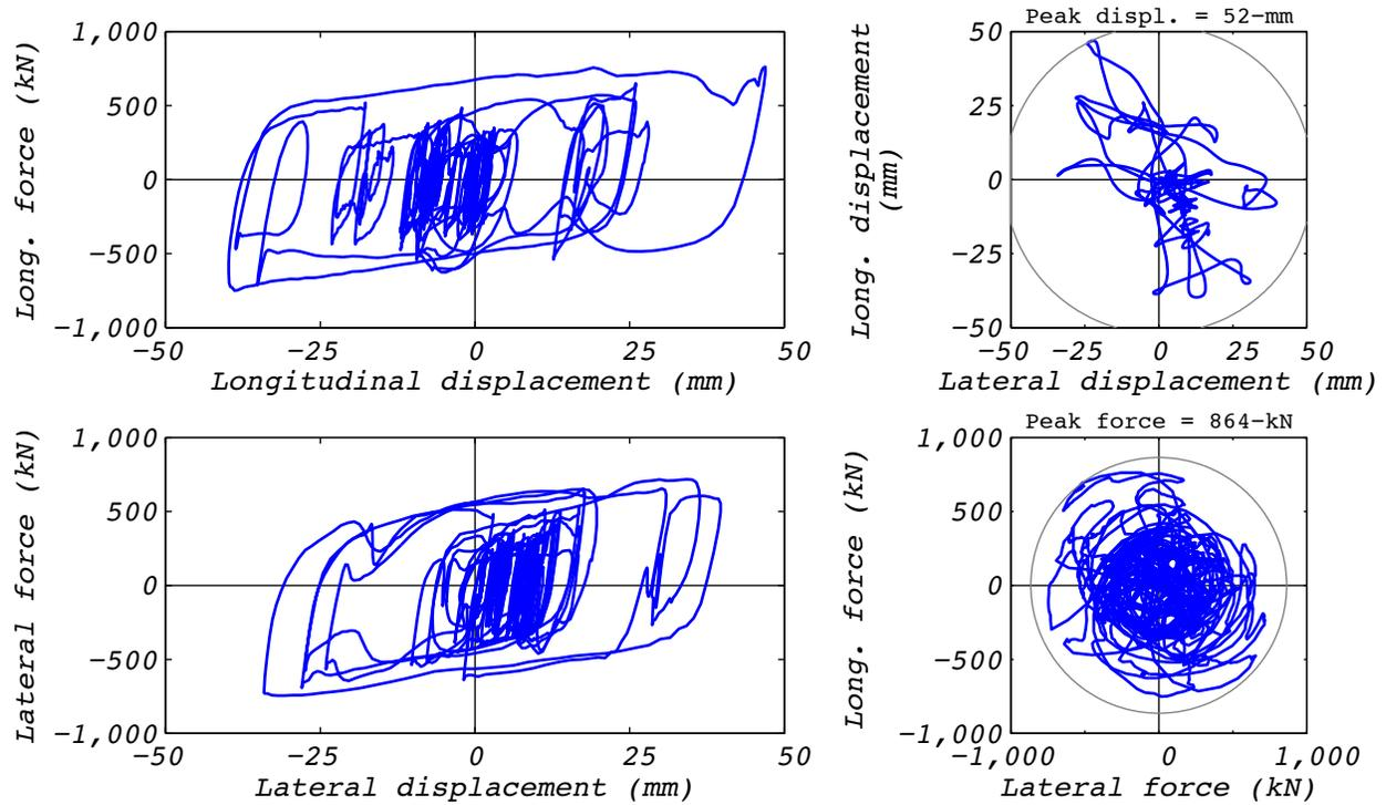
**Figure A.21-2 Hybrid test bearing response for run 78: EUR5, 3D with experimental bearing representing all bearings.**
