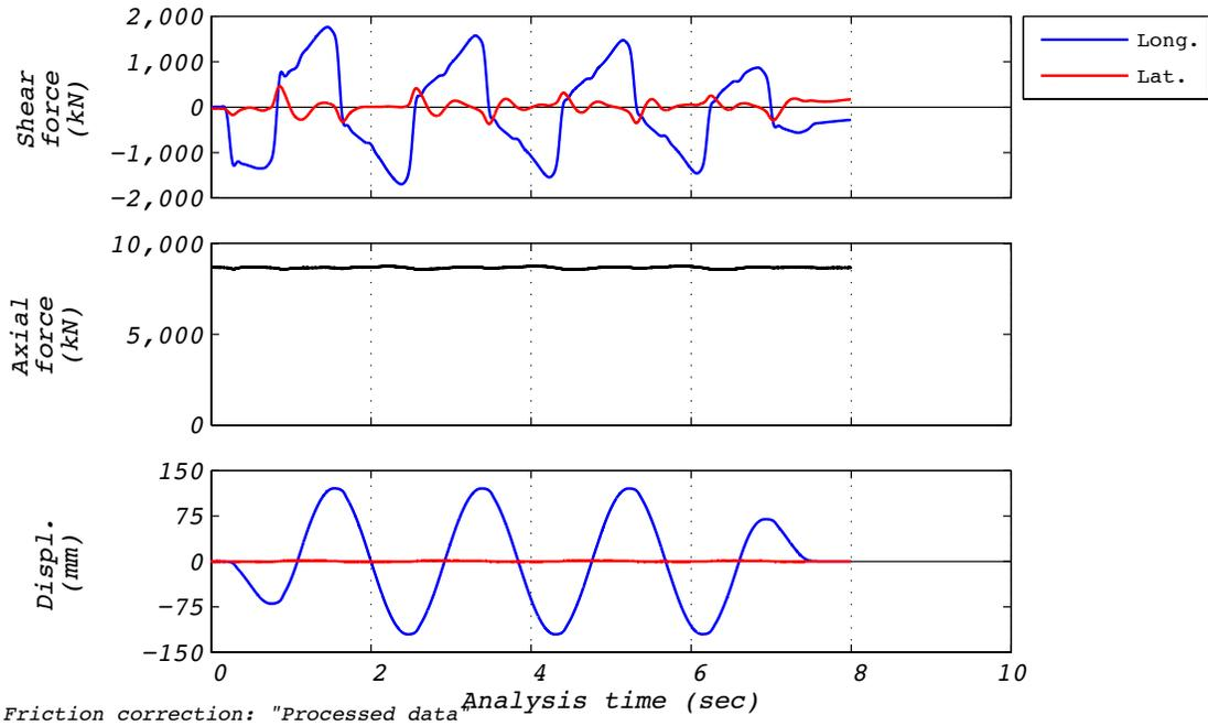
Figure D.1-1 Test run no. 1 time history: Longitudinal (120 mm amplitude, 8,663 kN axial load, and 410 mm/s velocity).
