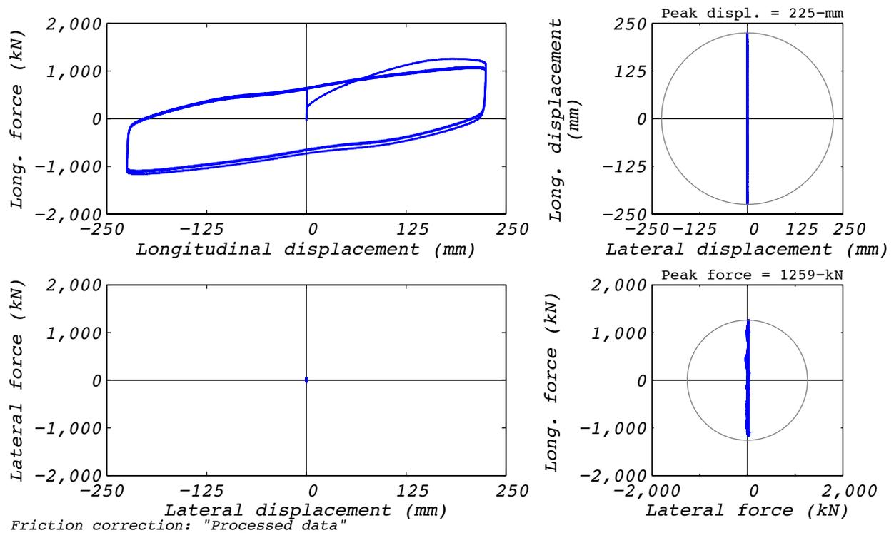
Figure B.12-2 Test run no. 41 hysteresis: Longitudinal (224 mm amplitude, 8,663 kN axial load, and 7 mm/s velocity).
