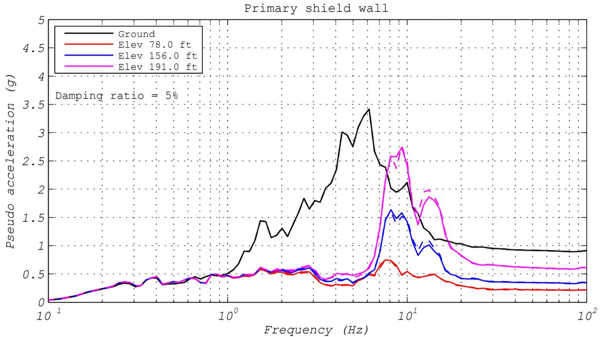
**Figure 3.69** EQS bearing: response spectra comparison of responses depending on the location of the bearing (ground motion NRC2, 2D analysis).
