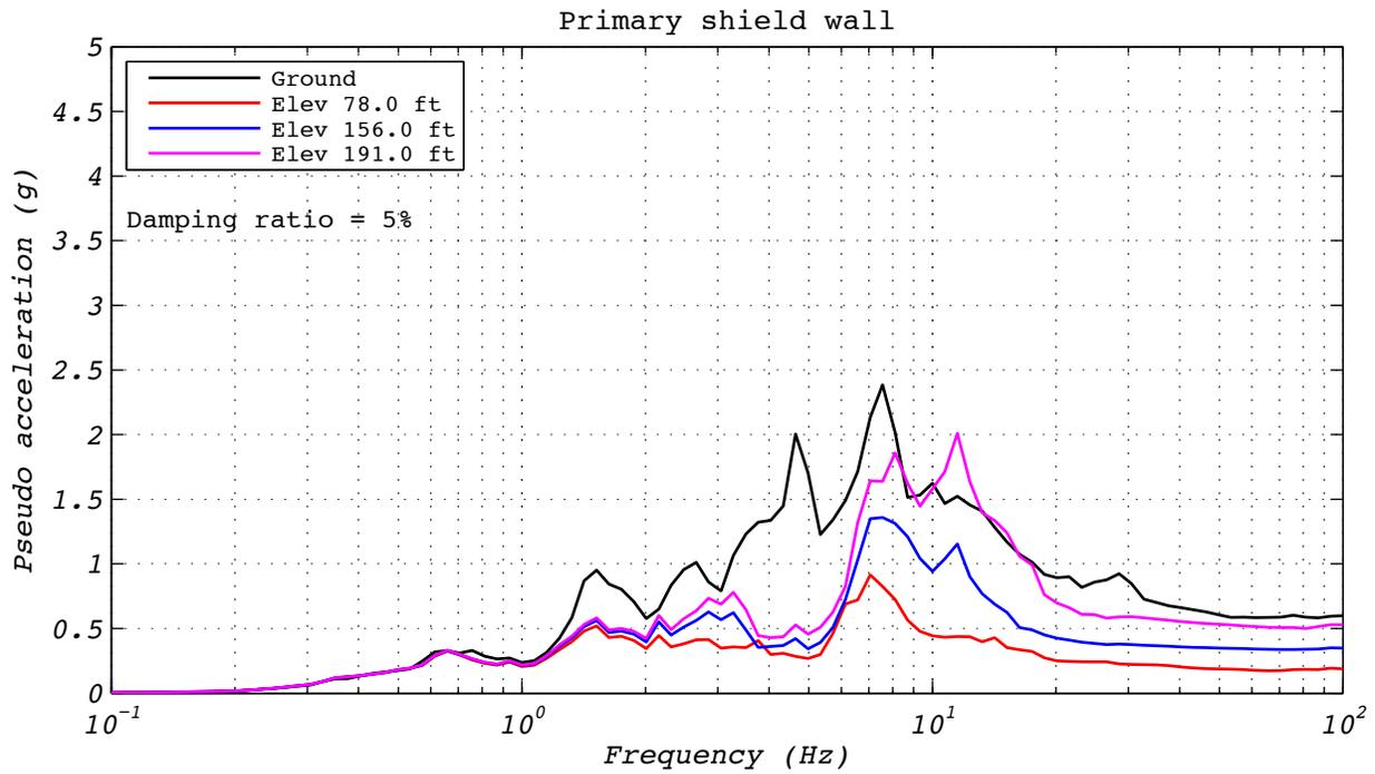
**Figure A.17-4 Hybrid test floor spectra for run 58: EUR5, 2D with experimental bearing representing one of 527 bearings.**
