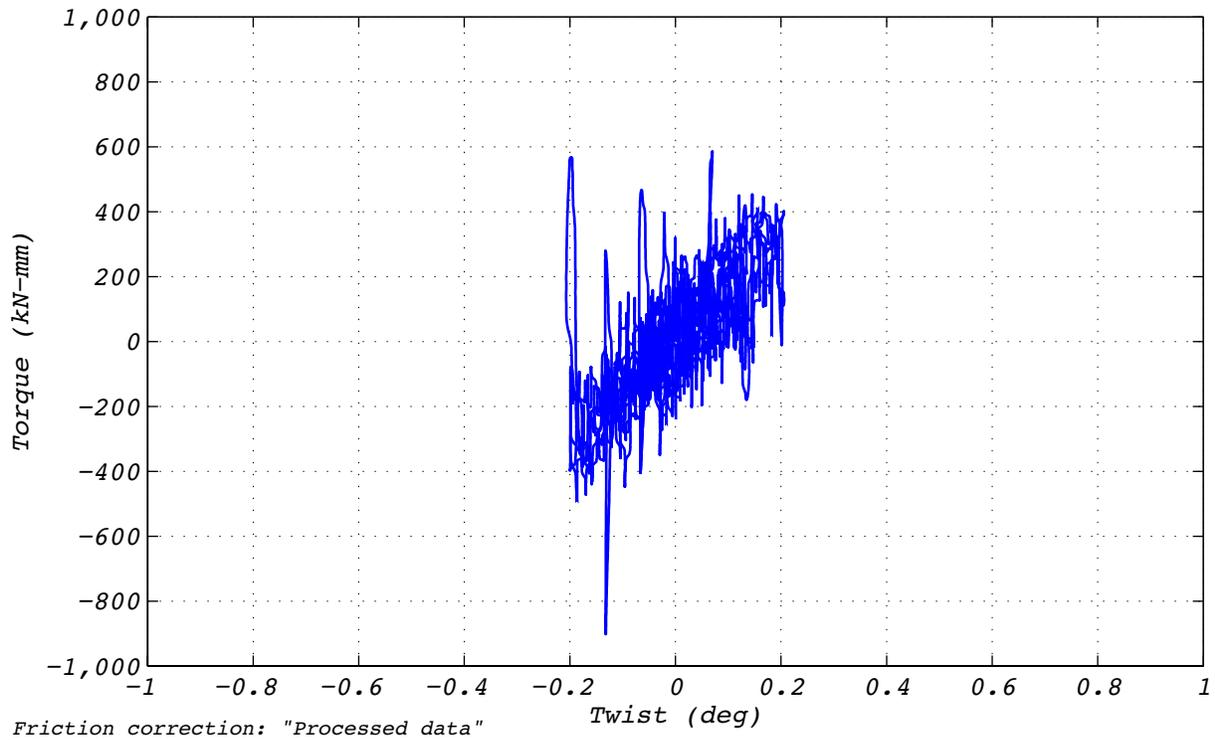
Figure D.8-2 Test run no. 8 hysteresis: Twist (0 mm displacement and 8,663 kN axial load).
