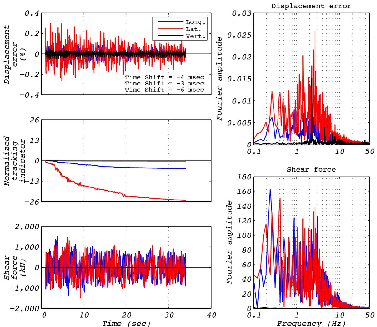
Figure C.9-1 Hybrid test performance metrics for run 44: NRC2, 3D with 5 groups of bearings and the experimental bearing representing the center group.
