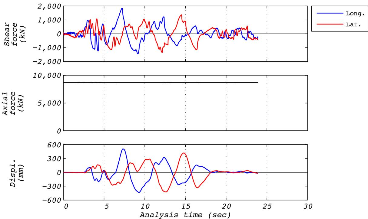
**Figure A.12-3 Hybrid test time history responses for run 46: NRC15, 2D with experimental bearing representing all bearings.**
