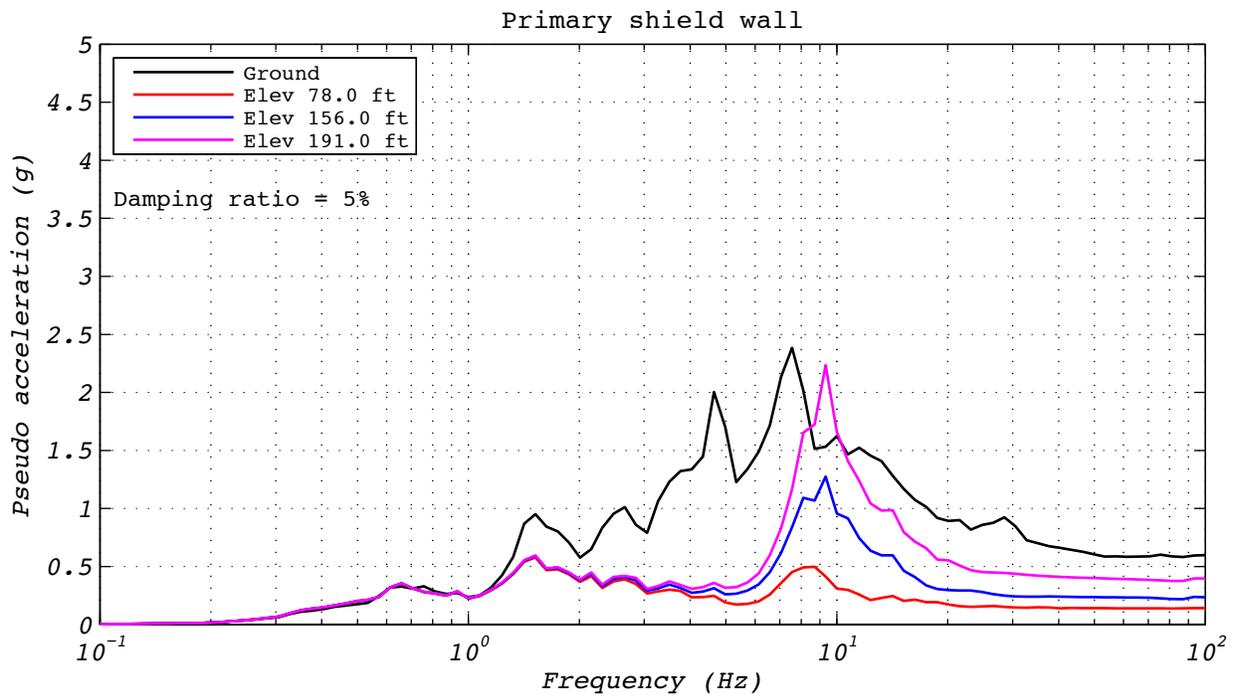
**Figure A.2-4 Hybrid test floor spectra for run 25: EUR5, 2D with experimental bearing representing all bearings.**
