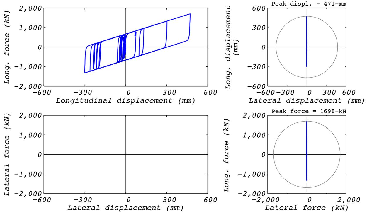
Figure A.14-1 Analytical bearing response for run 47A: NRC15, 1D with a single analytical bearing.
