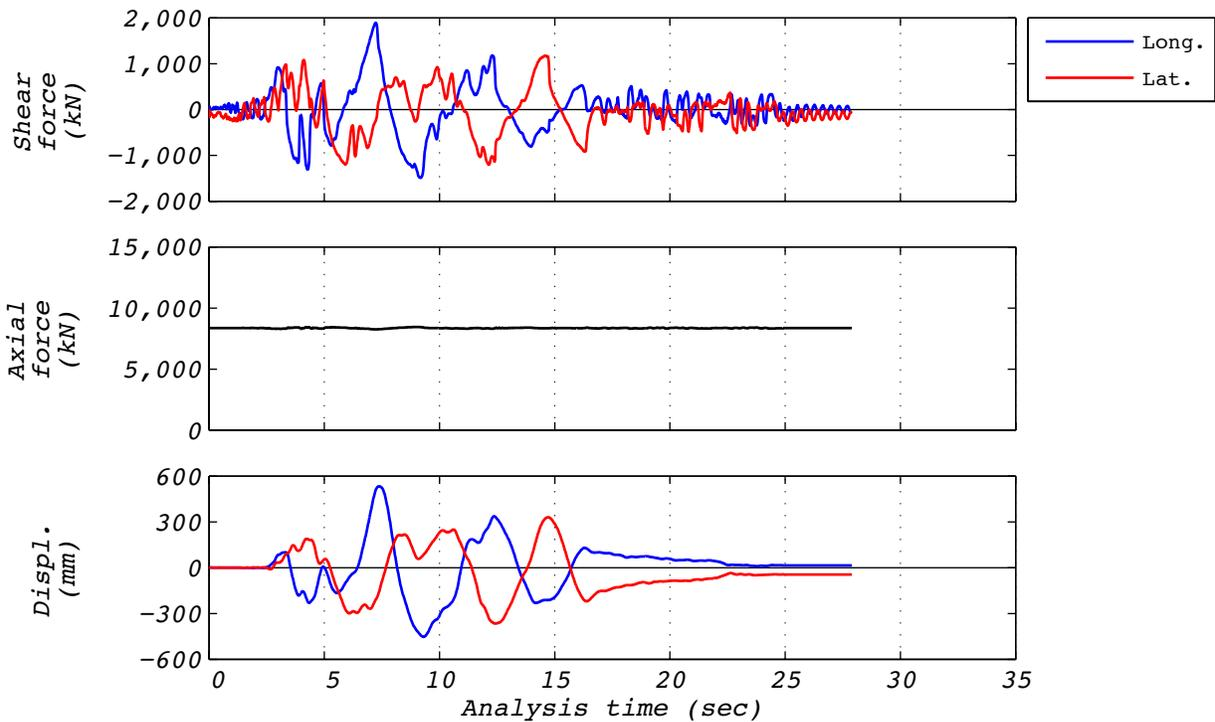
**Figure A.26-3 Hybrid test time history responses for run 84: NRC15, 3D with 5 groups of bearings and the experimental bearing representing the center group.**
