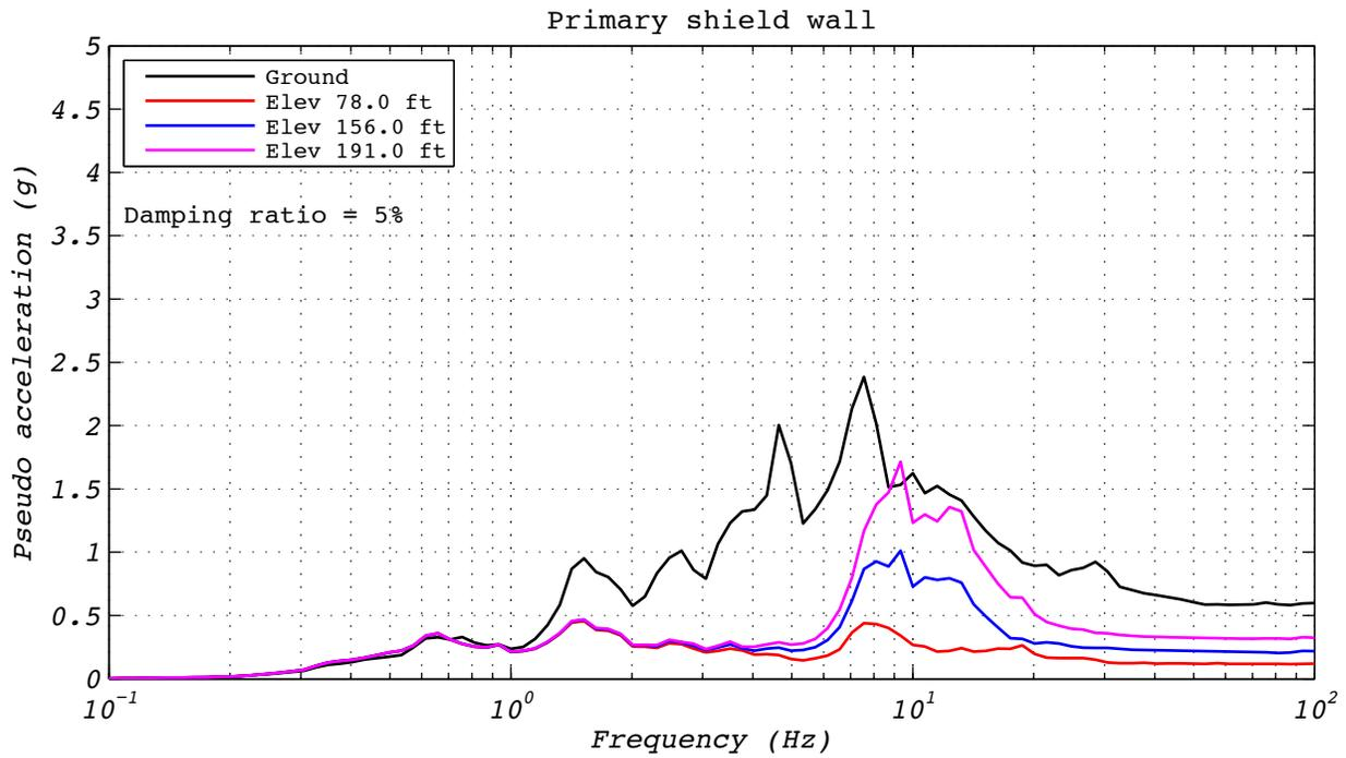
**Figure A.21-4 Hybrid test floor spectra for run 78: EUR5, 3D with experimental bearing representing all bearings.**
