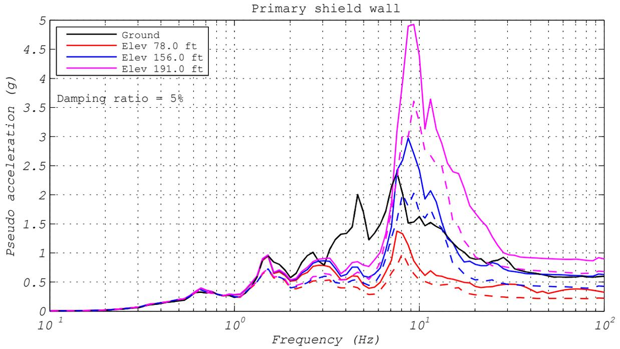
**Figure 3.81 EQS bearing: response spectra comparison of hybrid simulation and analytical estimation responses (ground motion EUR5, 2D analysis).**
