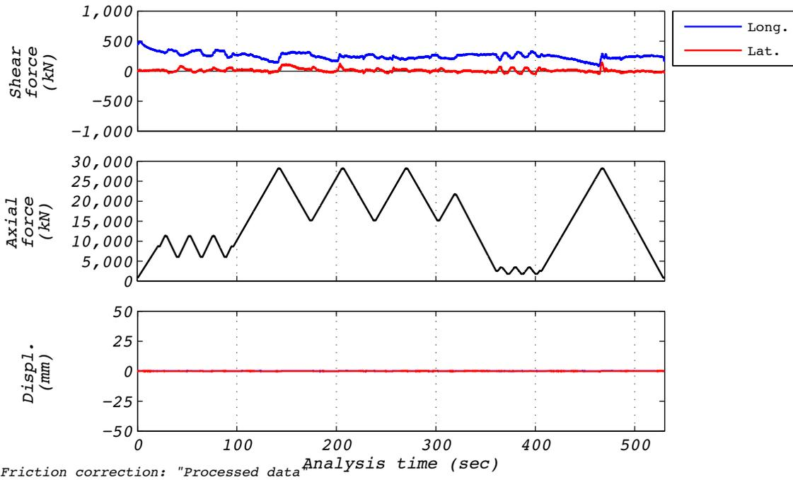
Figure B.6-1 Test run no. 15 time history: Axial (56 mm amplitude and varying axial load).
