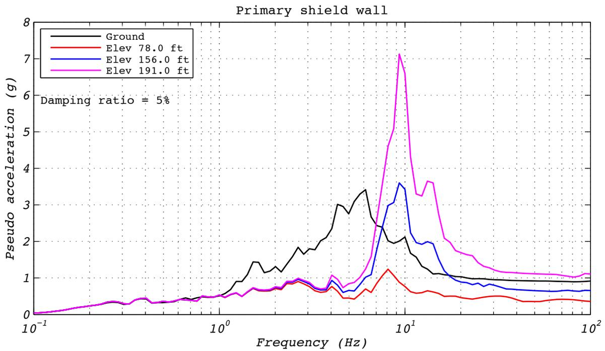
**Figure C.5-4 Hybrid test floor spectra for run 21 NRC2, 2D with experimental bearing representing all bearings.**
