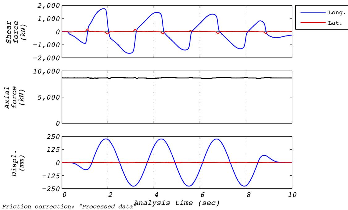
Figure B.11-1 Test run no. 35 time history: Longitudinal (224 mm amplitude, 8,663 kN axial load, and 586 mm/s velocity).
