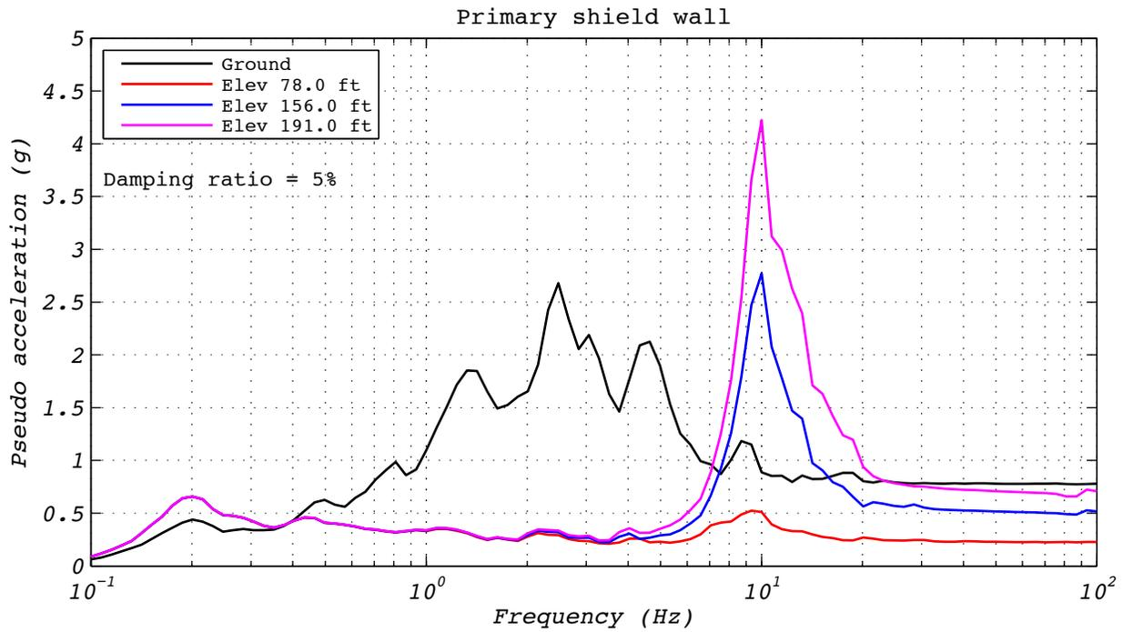
**Figure A.29-4 Hybrid test floor spectra for run 88: NRC15, 3D with 5 groups of bearings and the experimental bearing representing the no. 3 corner group.**
