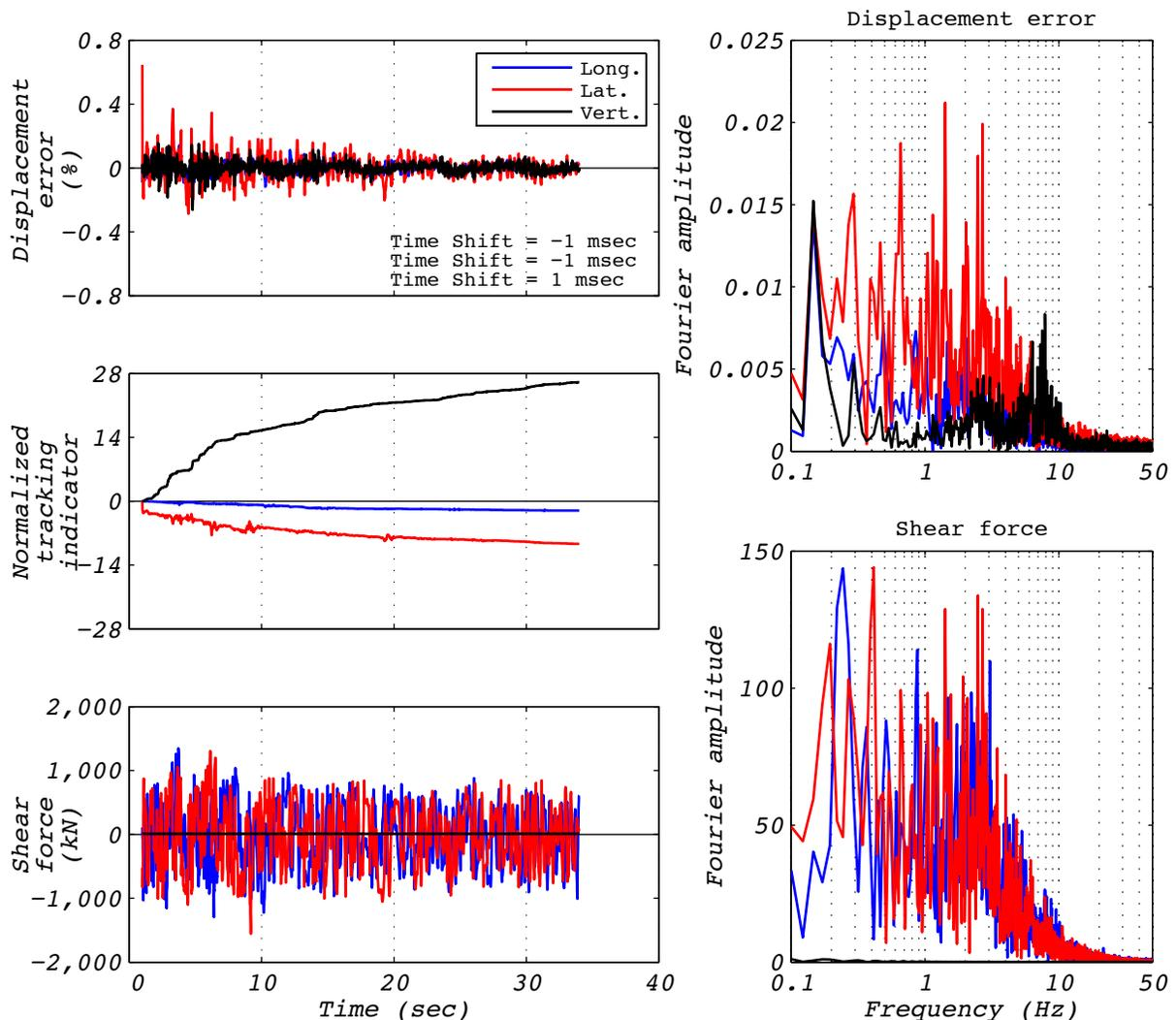
Figure C.12-1 Hybrid test performance metrics for run 48: NRC2, 3D with 5 groups of bearings and the experimental bearing representing the no. 3 corner group.
