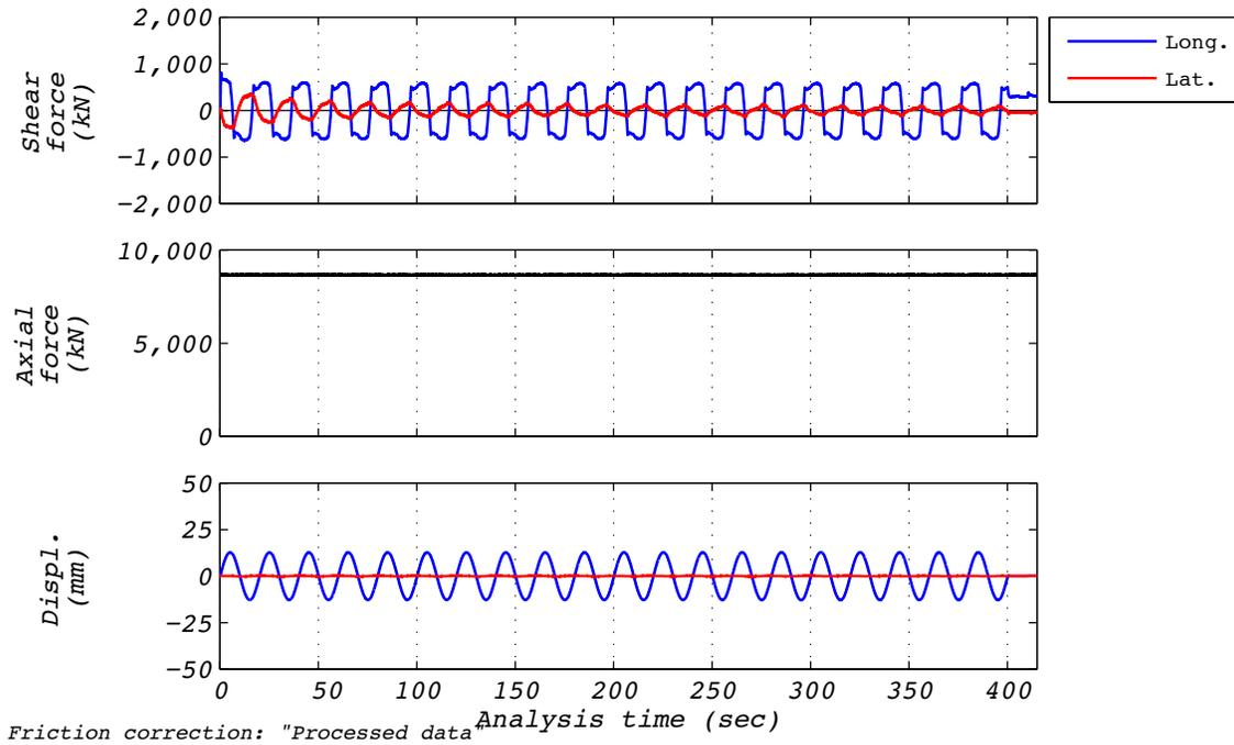
Figure D.30-1 Test run no. 36 time history: Longitudinal (13 mm amplitude, 8,663 kN axial load, and 4 mm/s velocity).
