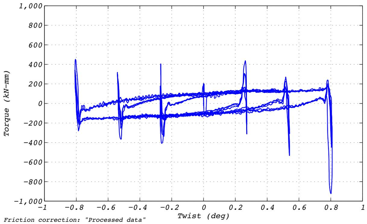
Figure B.15-2 Test run no. 53 hysteresis: Twist (0 mm amplitude and 8,663 kN axial load).
