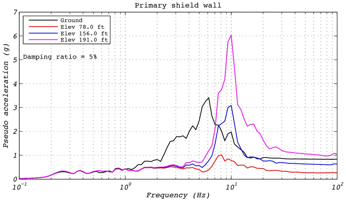
**Figure C.16-4 Hybrid test floor spectra for run 52: NRC2, 1D with experimental bearing representing all bearings.**
