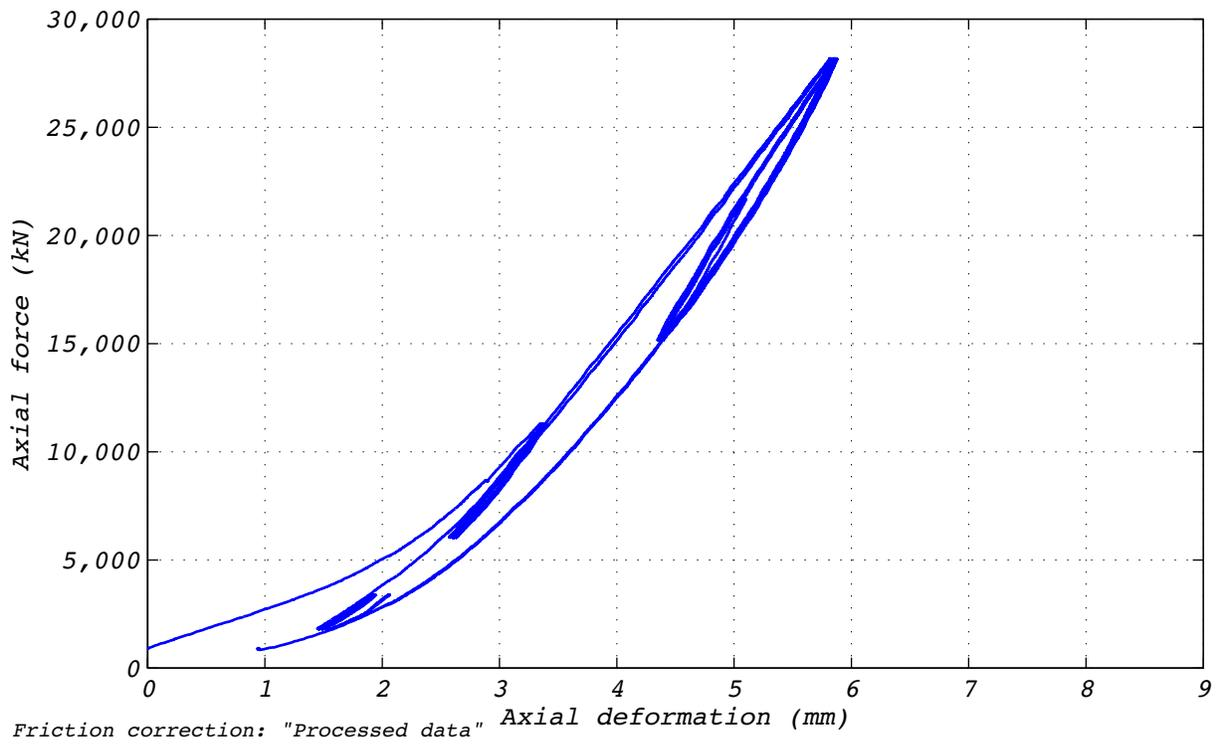
Figure B.6-2 Test run no. 15 hysteresis: Axial (56 mm amplitude and varying axial load).
