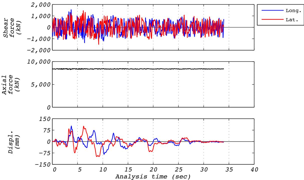
**Figure C.9-3 Hybrid test time history responses for run 44: NRC2, 3D with 5 groups of bearings and the experimental bearing representing the center group.**
