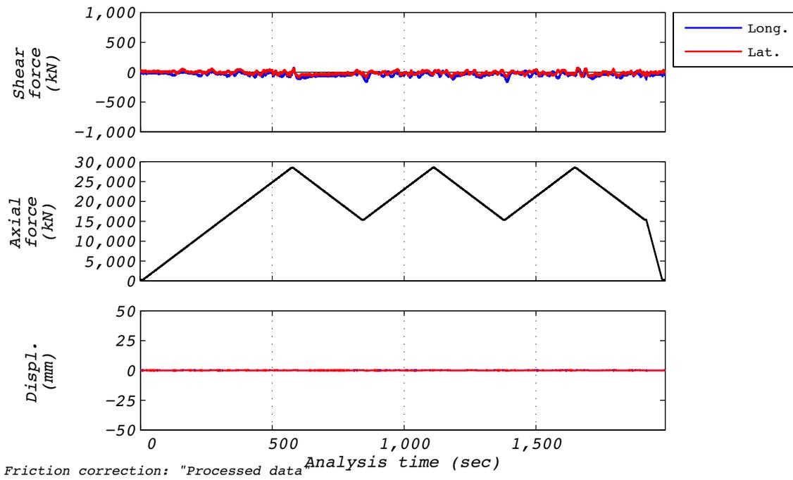
Figure B.25-1 Test run no. 68 time history: Axial (0 mm amplitude, varying axial load).
