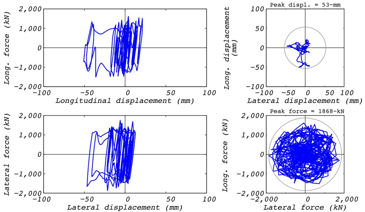
**Figure C.2-2 Hybrid test bearing response for run 18: EUR5, 2D with experimental bearing representing all bearings.**
