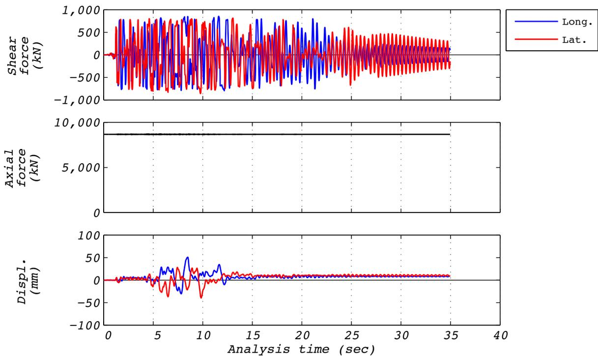
**Figure A.3 Hybrid test time history responses for run 24: EUR5, 2D with experimental bearing representing all bearings.**
