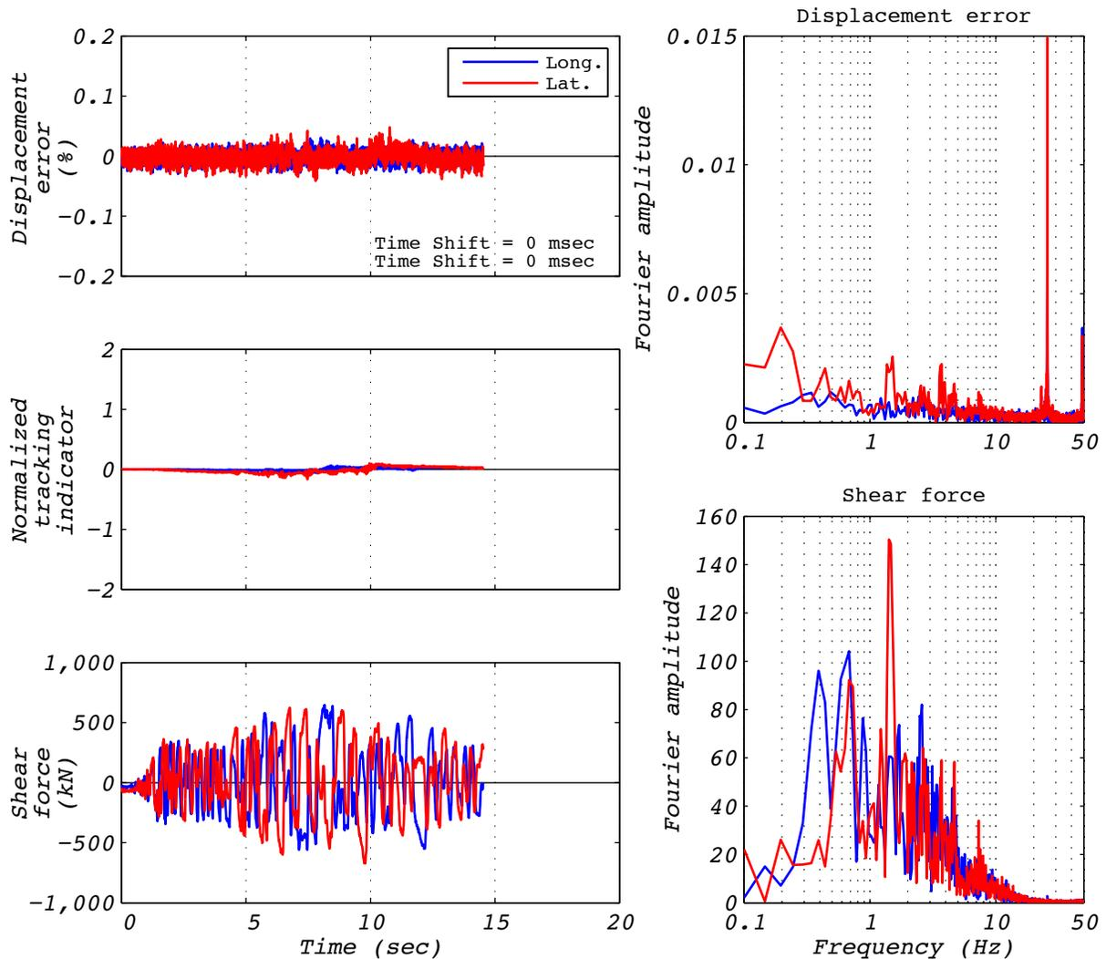
Figure A.17-1 Hybrid test performance metrics for run 58: EUR5, 2D with experimental bearing representing one of 527 bearings.
