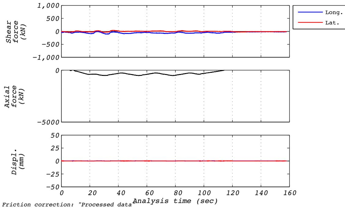
Figure B.5-1 Test run no. 14 time history: Axial (0mm amplitude and tensile axial load).
