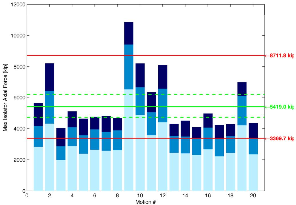
**Figure 3.33** Analytically determined peak axial force demands for the EUR hazard level [2012] based on an FPSB isolator (green lines = median with 95% confidence interval, red lines = 5<sup>th</sup> and 95<sup>th</sup> percentile).
