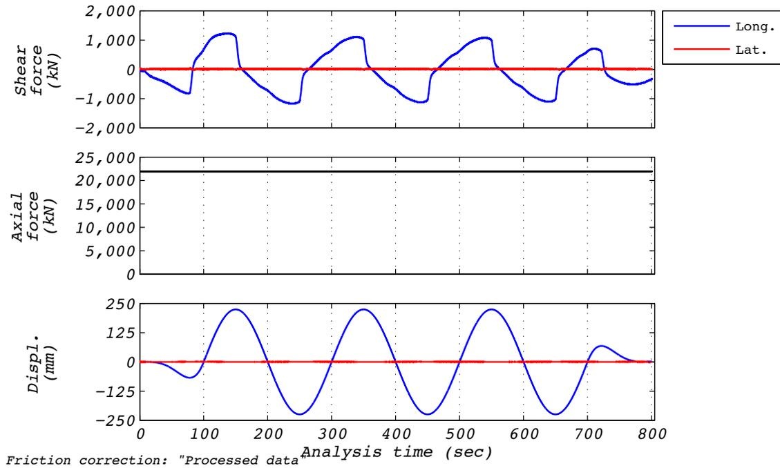
Figure B.3-1 Test run no. 12 time history: Longitudinal (224 mm amplitude, 21,927 kN axial load, and 7 mm/s velocity).
