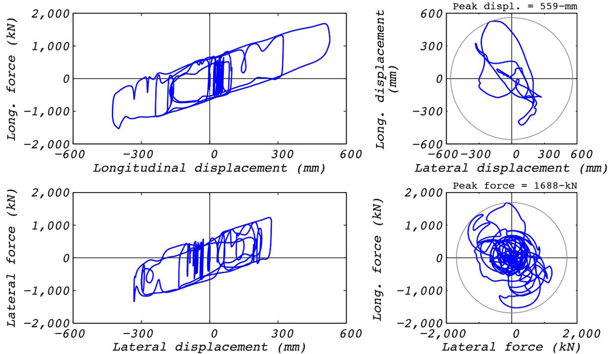
Figure A.16-1 Analytical bearing response for run 55A: NRC15, 2D with a single analytical bearing.
