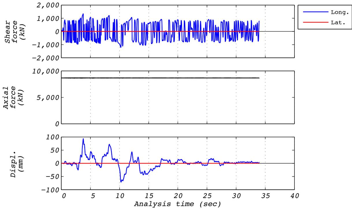
**Figure C.17-2 Analytical time history responses for run 52A: NRC2, 1D with a single analytical bearing.**
