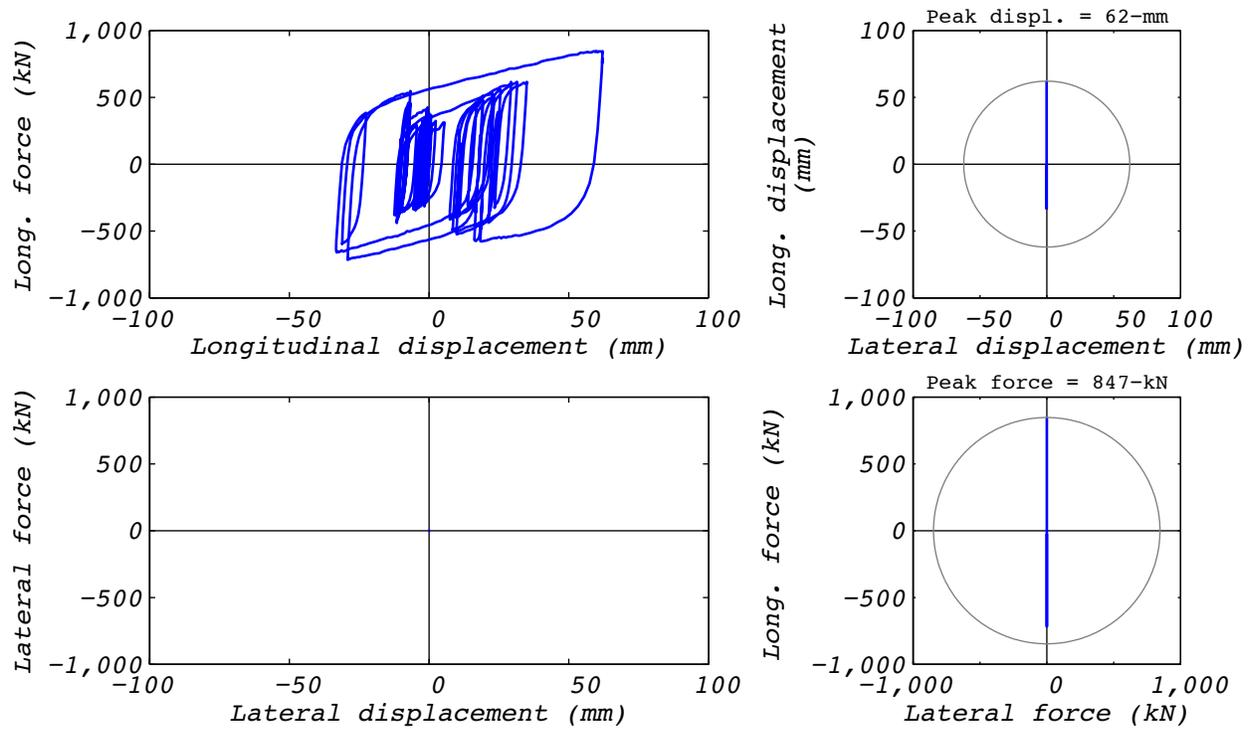
**Figure A.7-2 Hybrid test bearing response for run 43: EUR5, 1D with experimental bearing representing all bearings.**
