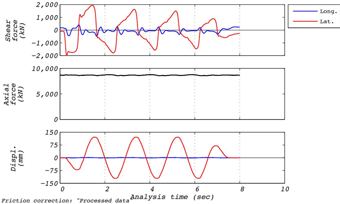
Figure D.10-1 Test run no. 10 time history: Transverse (120 mm amplitude, 8,663 kN axial load, and 410 mm/s velocity).
