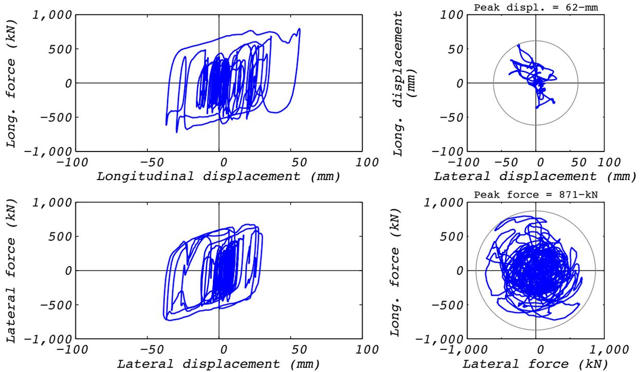
**Figure A.24-2 Hybrid test bearing response for run 82: EUR5, 3D with 5 groups of bearings and the experimental bearing representing the center group.**
