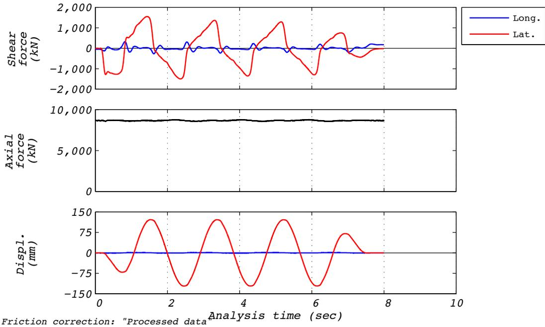
Figure D.26-1 Test run no. 32 time history: Transverse (120 mm amplitude, 8,663 kN axial load, and 410 mm/s velocity).
