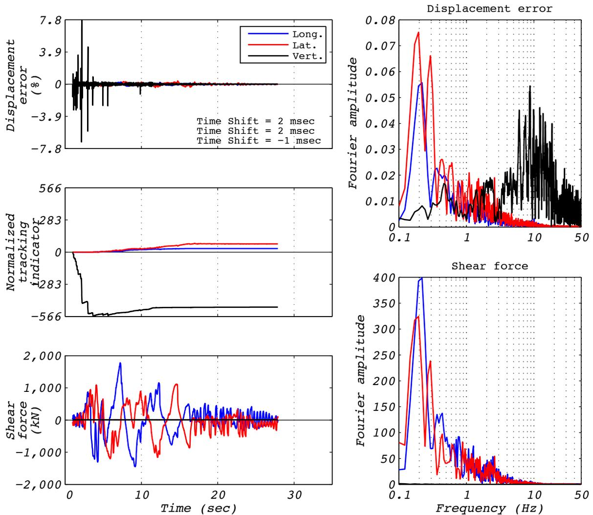
Figure A.30-1 Hybrid test performance metrics for run 89: NRC15, 3D with 5 groups of bearings and the experimental bearing representing the no. 3 corner group.
