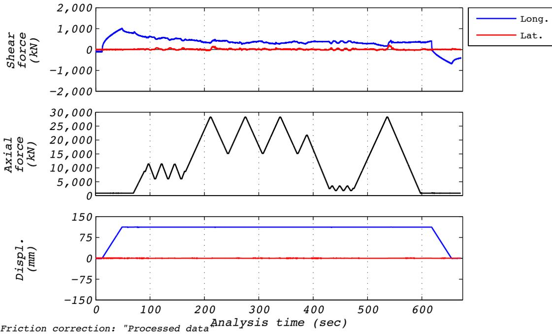
Figure B.7-1 Test run no. 16 time history: Axial (112 mm amplitude and varying axial load).
