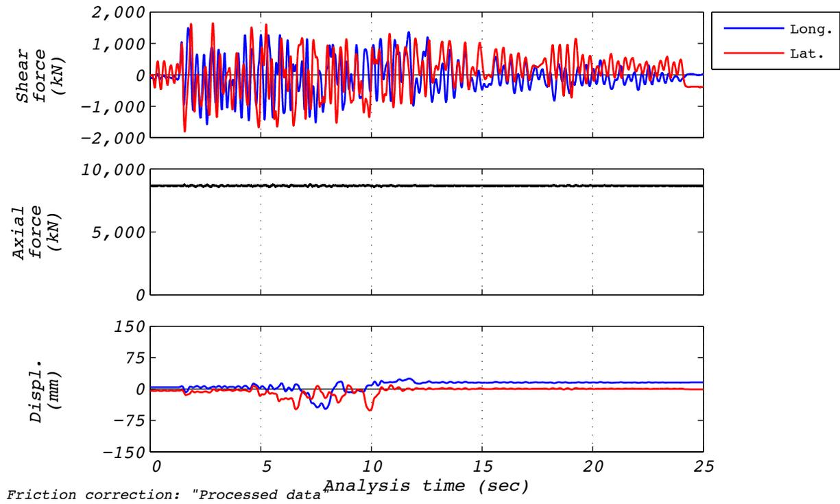
**Figure C.4-2 Time history responses for real-time reproduction of hybrid test run 18: EUR5, 2D with experimental bearing representing all bearings.**
