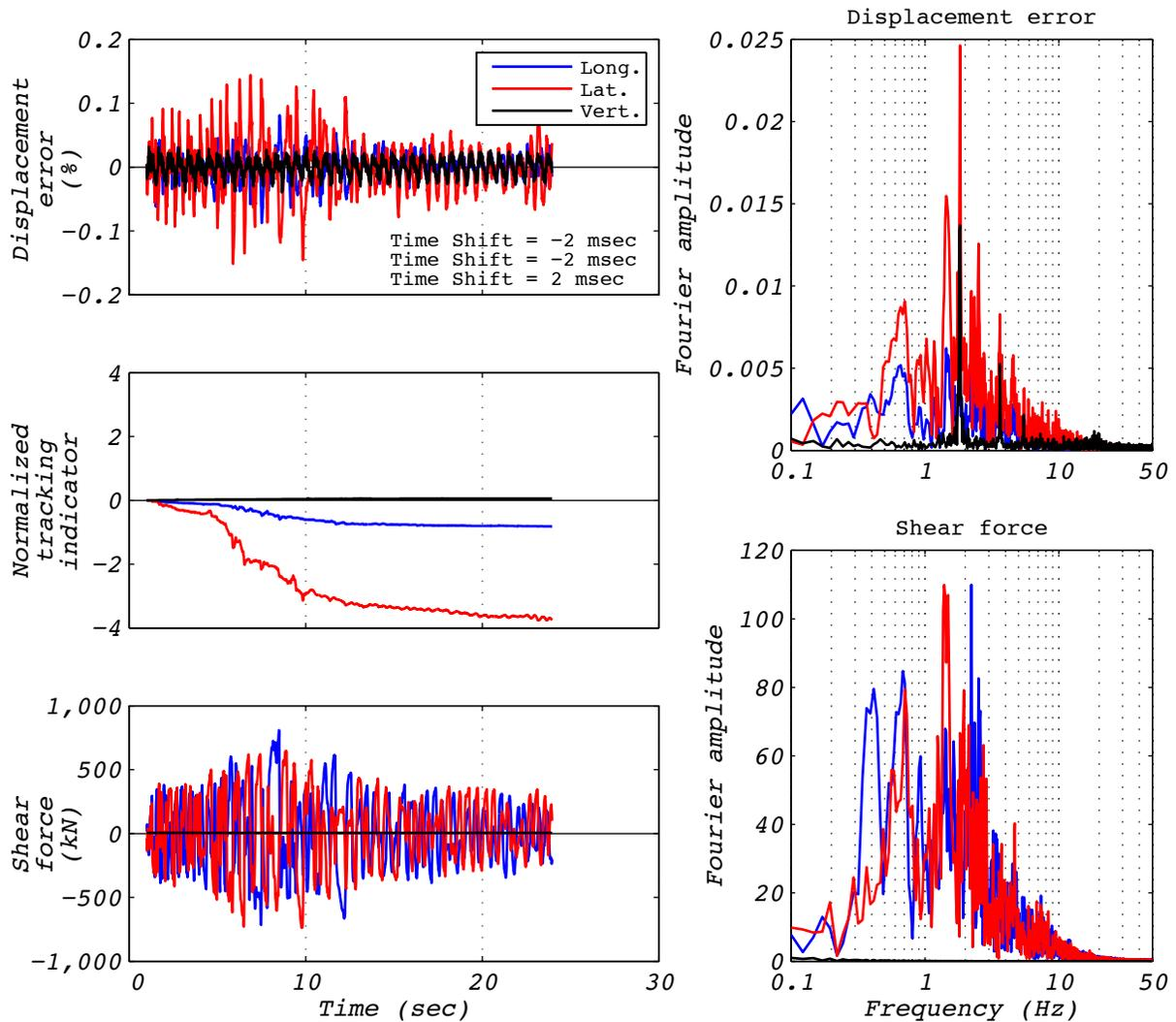
Figure A.22-1 Hybrid test performance metrics for run 79: EUR5, 3D with 5 groups of bearings and the experimental bearing representing the center group.
