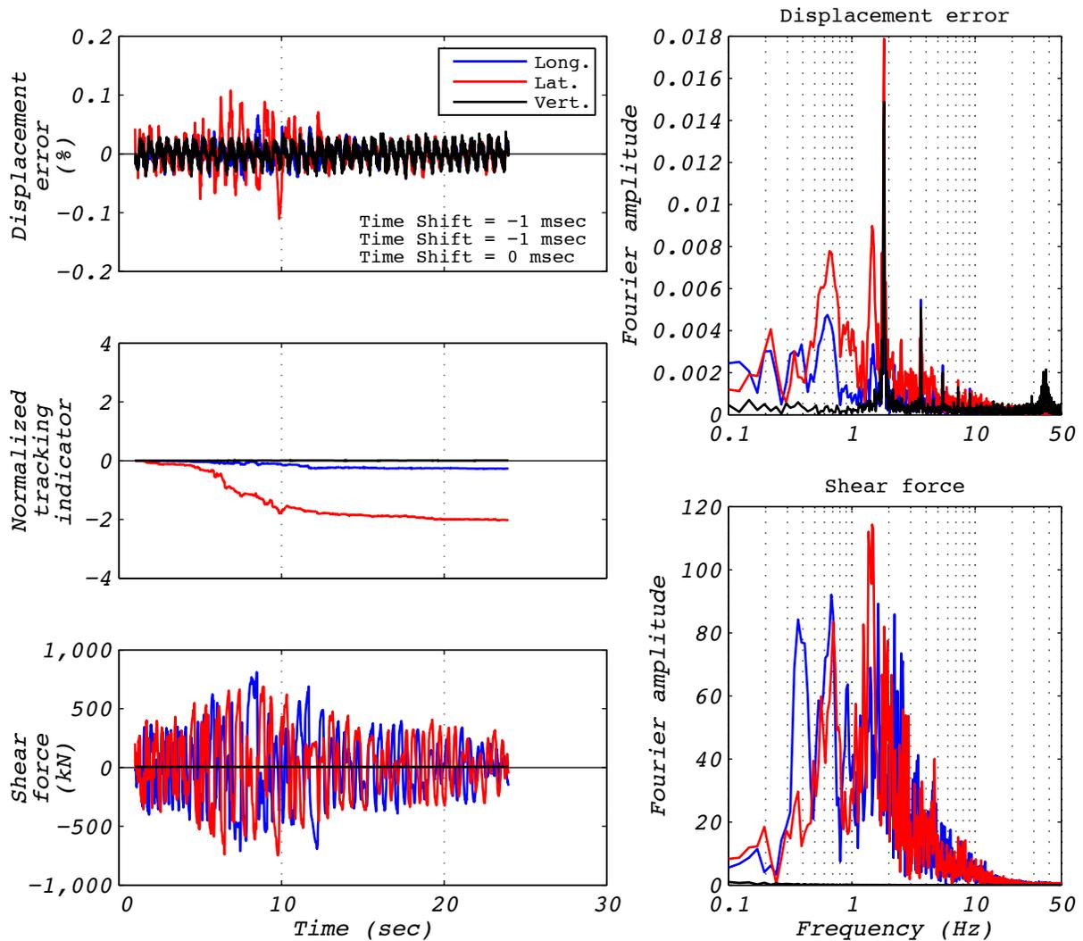
Figure A.23-1 Hybrid test performance metrics for run 80: EUR5, 3D with 5 groups of bearings and the experimental bearing representing the center group.
