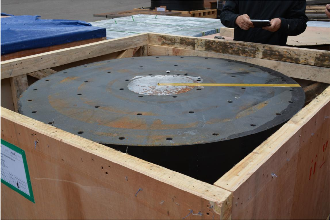
**Figure 3.25** Unison bearing pre-test condition.
