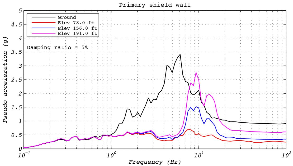
**Figure C.12-4 Hybrid test floor spectra for run 48: NRC2, 3D with 5 groups of bearings and the experimental bearing representing the no. 3 corner group.**
