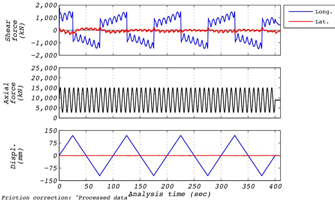
Figure D.21-1 Test run no. 27 time history: Longitudinal (120 mm amplitude, varying axial load, and 410 mm/s velocity).
