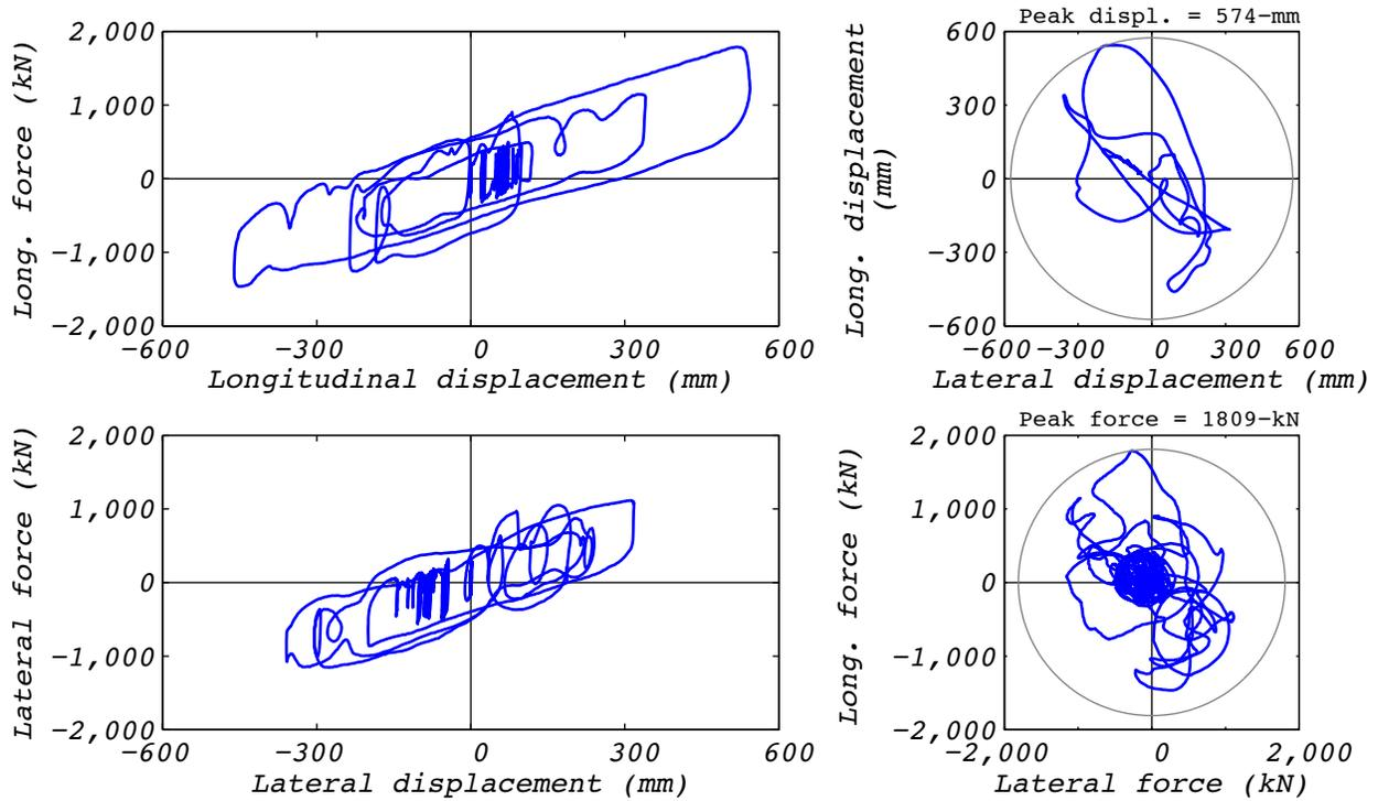
**Figure A.27-2 Hybrid test bearing response for run 85: NRC15, 3D with 5 groups and the experimental bearing representing the no. 3 corner group.**
