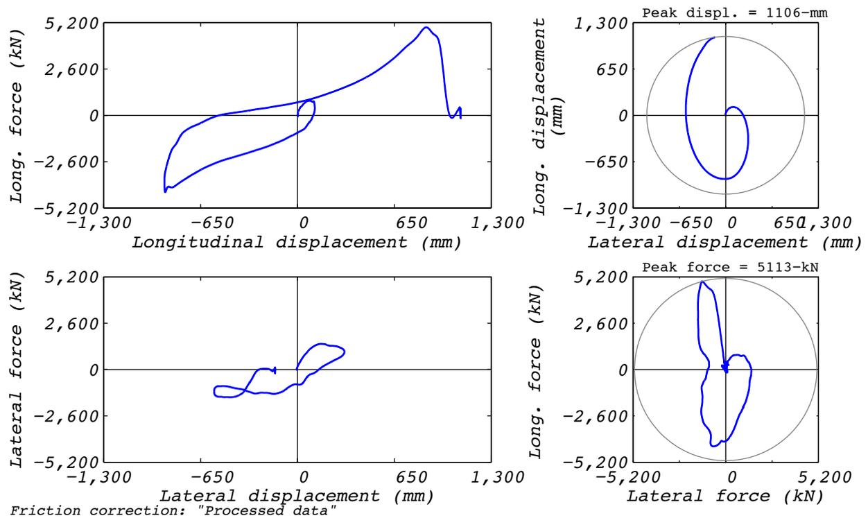
Figure B.23-2 Test run no. 66 hysteresis: Bearing response during failure test (varying amplitude and 8,663 kN axial load).
