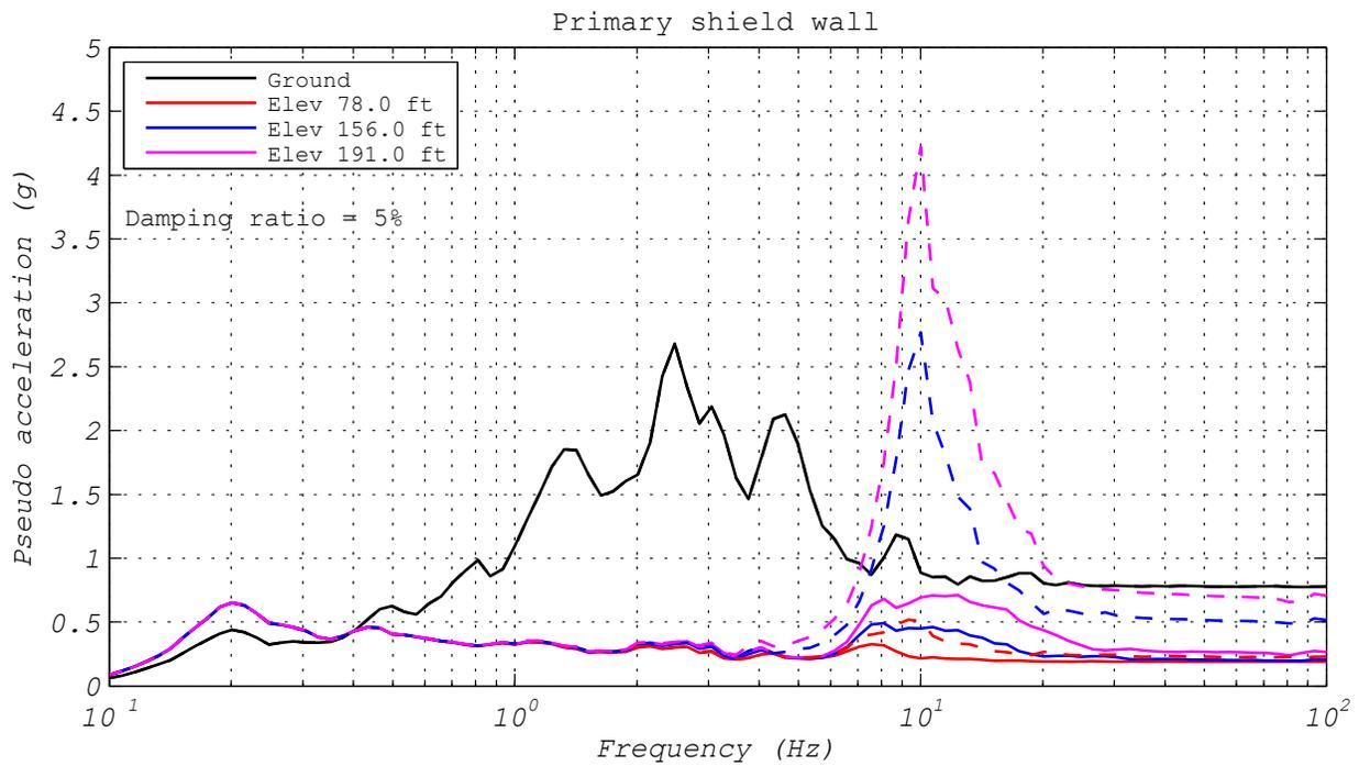
**Figure 3.45** LPRB bearing: response spectra comparison of responses to a ground motion with and without vertical excitation (ground motion NRC15, 2D and 3D analyses).
