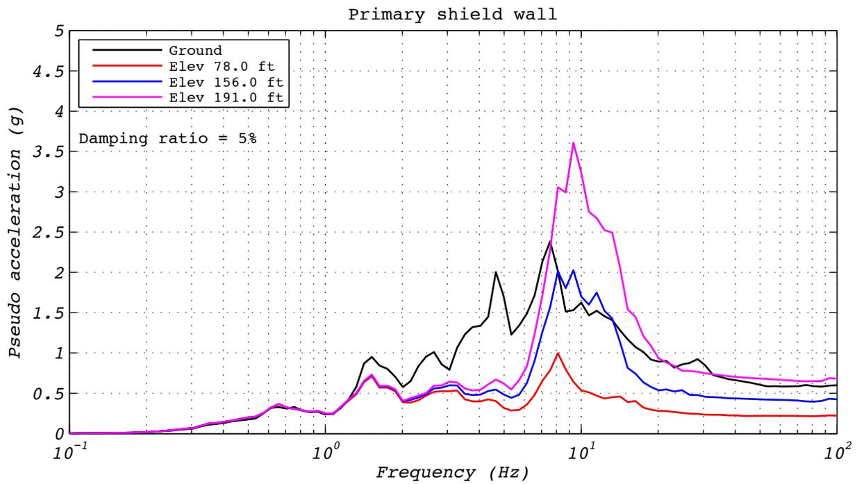
**Figure C.3-3 Floor spectra for analytical run 18A: EUR5, 2D with a single analytical bearing.**
