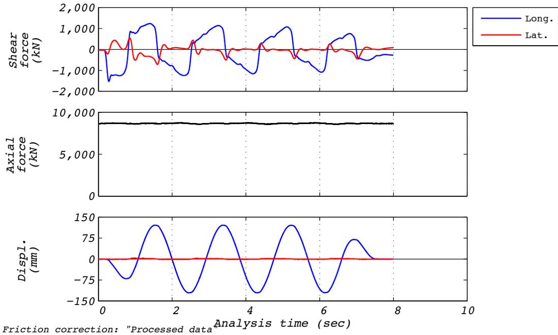
Figure D.31-1 Test run no. 59 time history: Longitudinal (120 mm amplitude, 8,663 kN axial load, and 410 mm/s velocity).
