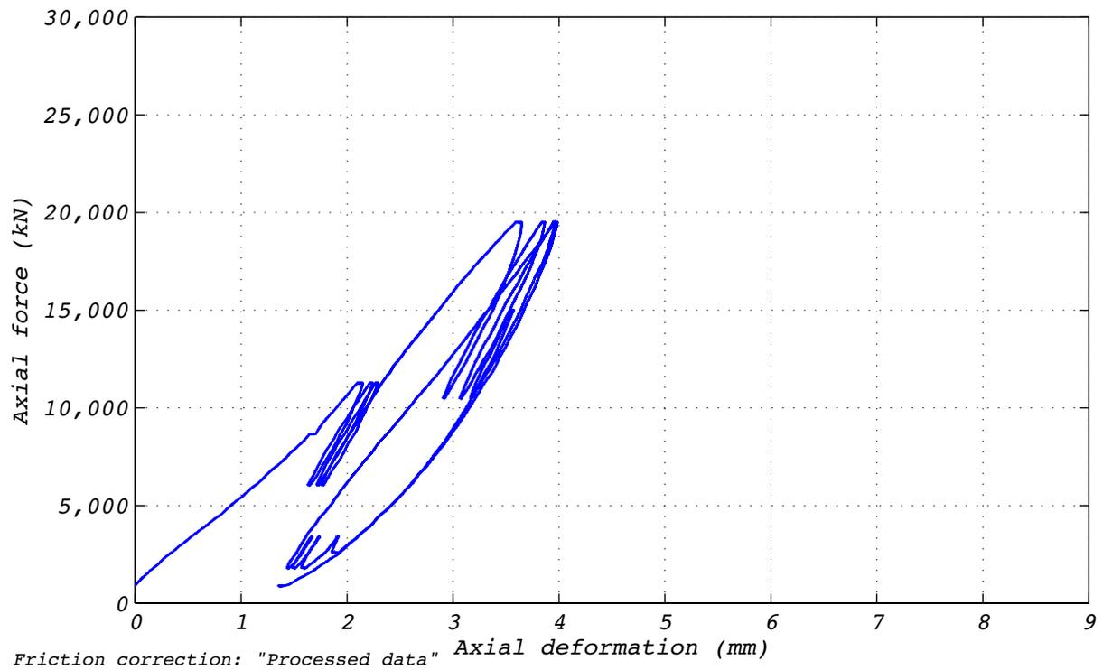
Figure D.2-2 Test run no. 2 hysteresis: Axial (0 mm displacement and varying axial load).
