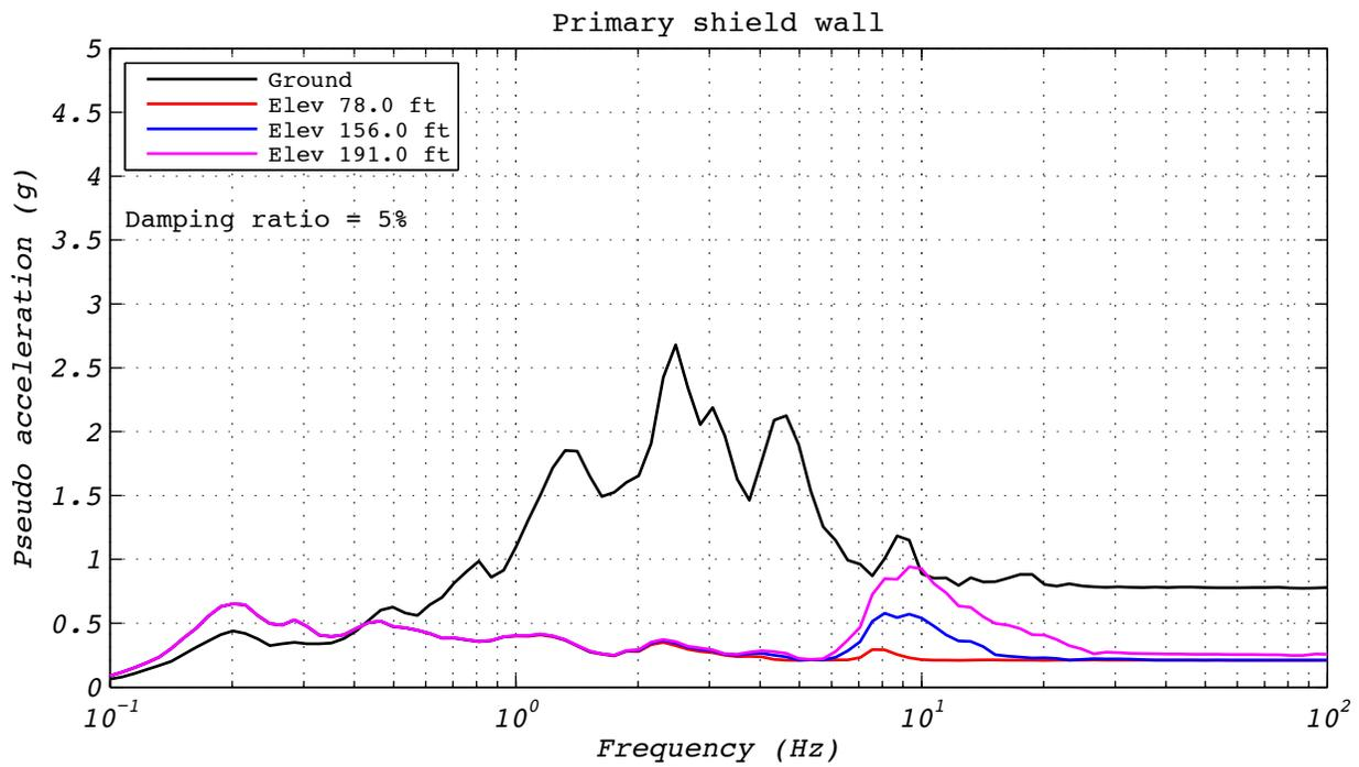
**Figure A.12-4 Hybrid test floor spectra for run 46: NRC15, 2D with experimental bearing representing all bearings.**
