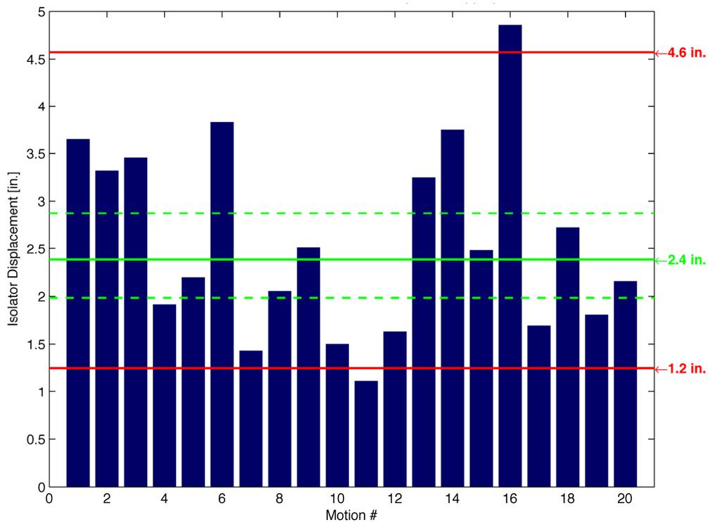
**Figure 3.28** Analytically determined peak lateral displacement demands per the EUR hazard level [2012] based on an LPRB isolator (green lines = median with 95% confidence interval, red lines = 5<sup>th</sup> and 95<sup>th</sup> percentile).
