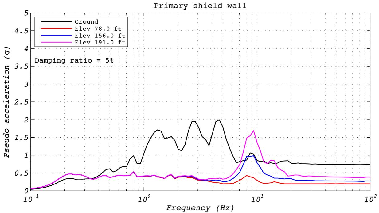
**Figure A.14-3 Floor spectra for analytical run 47A: NRC15, 1D with a single analytical bearing.**
