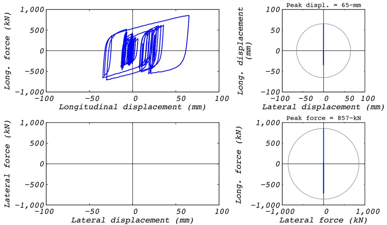
**Figure A.4-2 Hybrid test structural response for run 37: EUR5, 1D with experimental bearing representing all bearings.**
