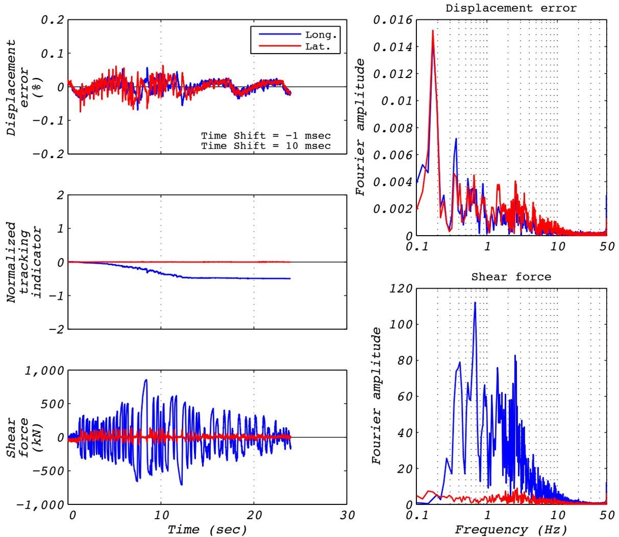
Figure A.4-1 Hybrid test performance metrics for run 37: EUR5, 1D with experimental bearing representing all bearings.
