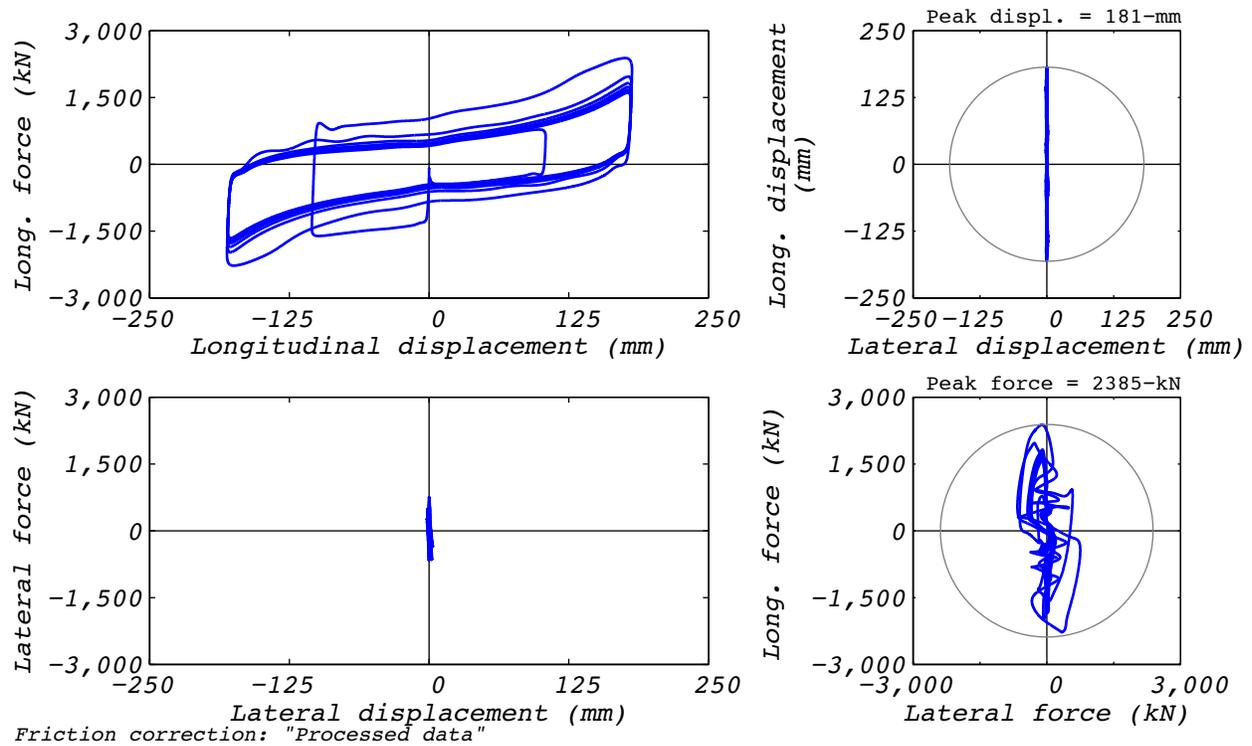
**Figure D.16-2 Test run no. 16 hysteresis: Longitudinal (180 mm amplitude, 8,663 kN axial load, and 409 mm/s velocity).**
