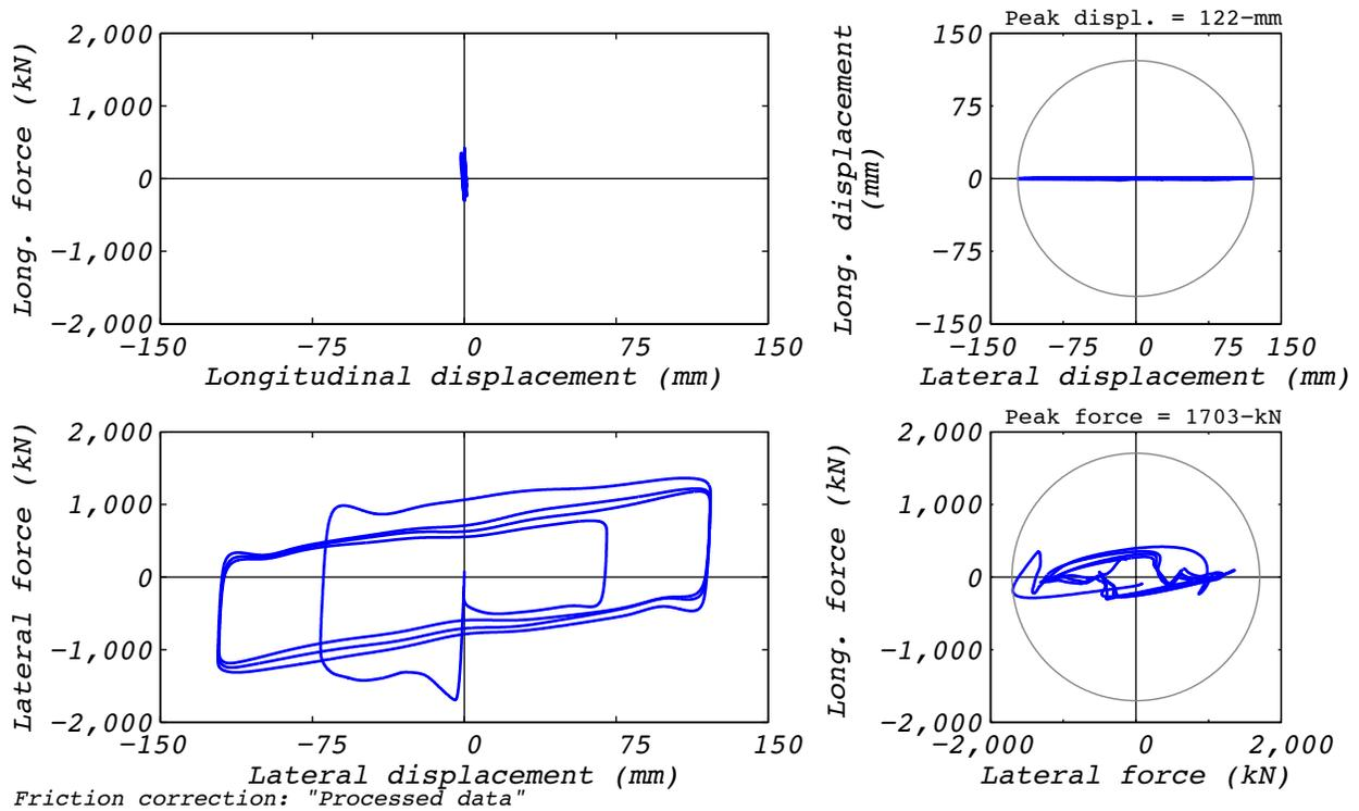
Figure D.32-2 Test run no. 60 hysteresis: Transverse (120 mm amplitude, 8,663 kN axial load, and 410 mm/s velocity).
