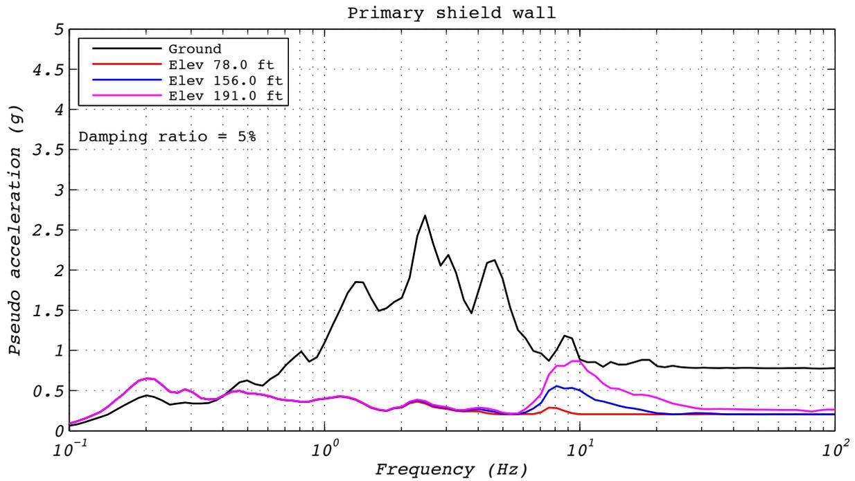
**Figure A.15-4 Hybrid test floor spectra for run 55: NRC15, 2D with experimental bearing representing all bearings.**
