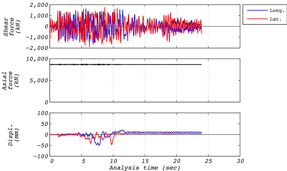
**Figure C.2-3 Hybrid test time history responses for run 18: EUR5, 2D with experimental bearing representing all bearings.**
