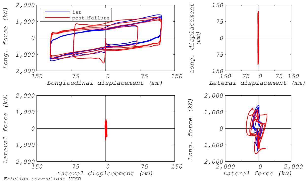
Figure 3.89 EQS-2 bearing response to longitudinal characterization tests.
