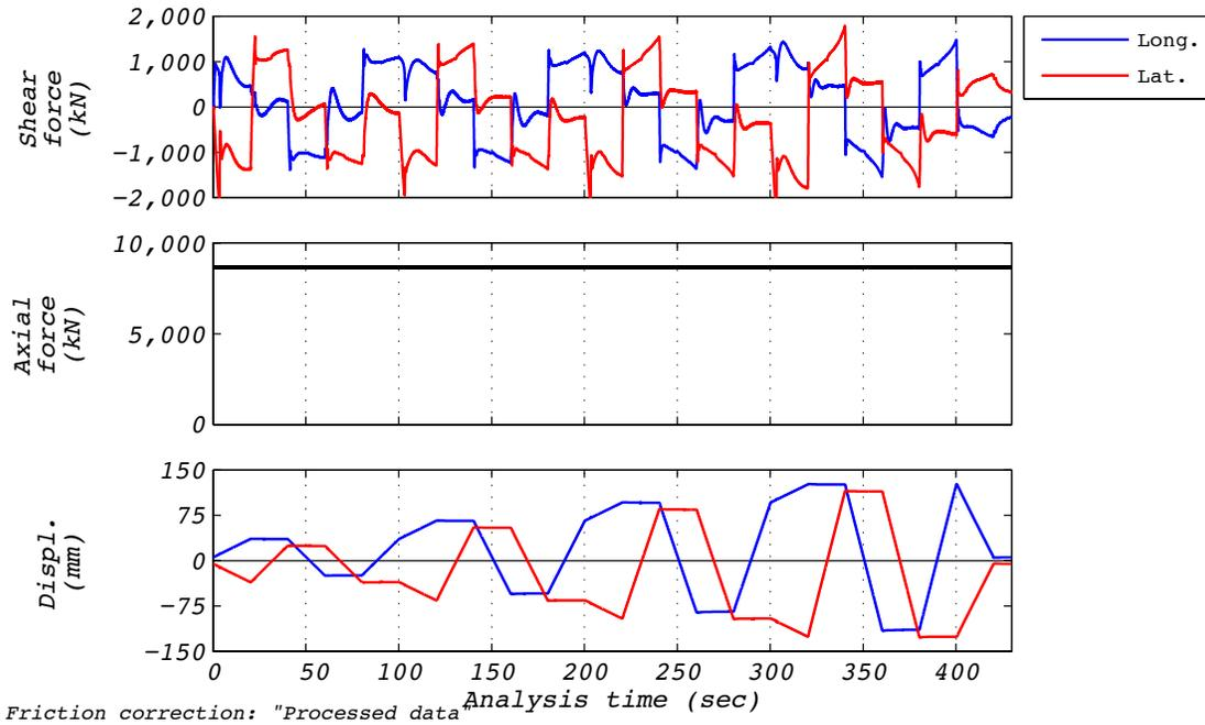
Figure D.22-1 Test run no. 28 time history: Square orbit (Varying amplitude, 8,663 kN axial load, and varying velocity).
