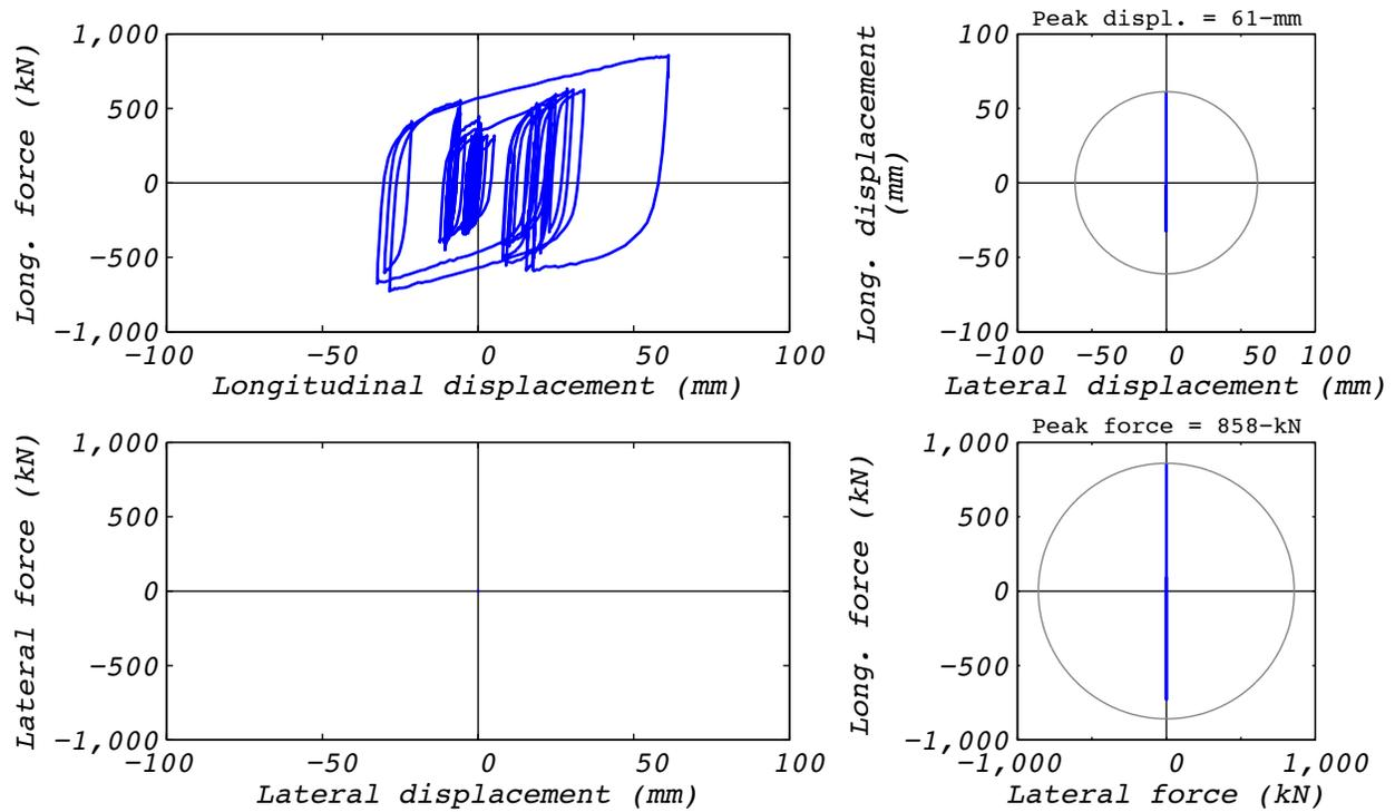
**Figure A.8-2 Hybrid test bearing response for run 44: EUR5, 1D with experimental bearing representing all bearings.**
