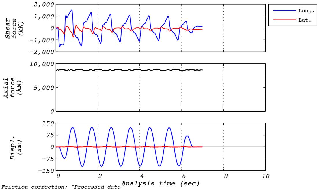
Figure D.19-1 Test run no. 25 time history: Longitudinal (120 mm amplitude, 8,663 kN axial load, and 820 mm/s velocity).
