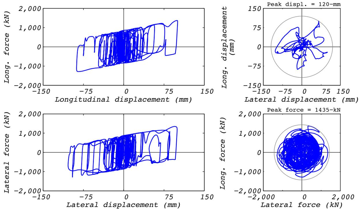
Figure C.21-1 Analytical bearing response for run 54A: NRC2, 2D with a single analytical bearing.
