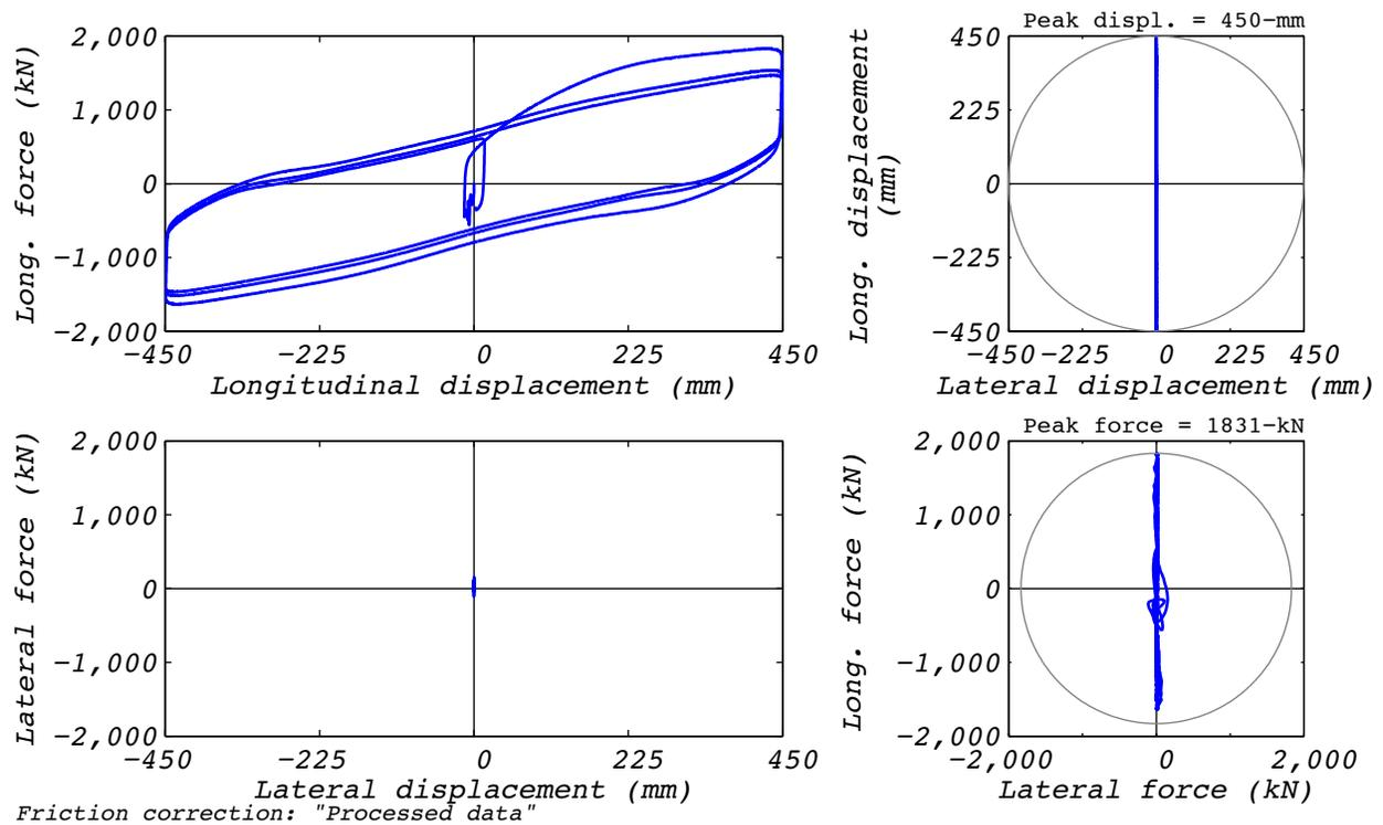
Figure B.21-2 Test run no. 64 hysteresis: Longitudinal (448 mm amplitude, 8,663 kN axial load, and 28 mm/s velocity).
