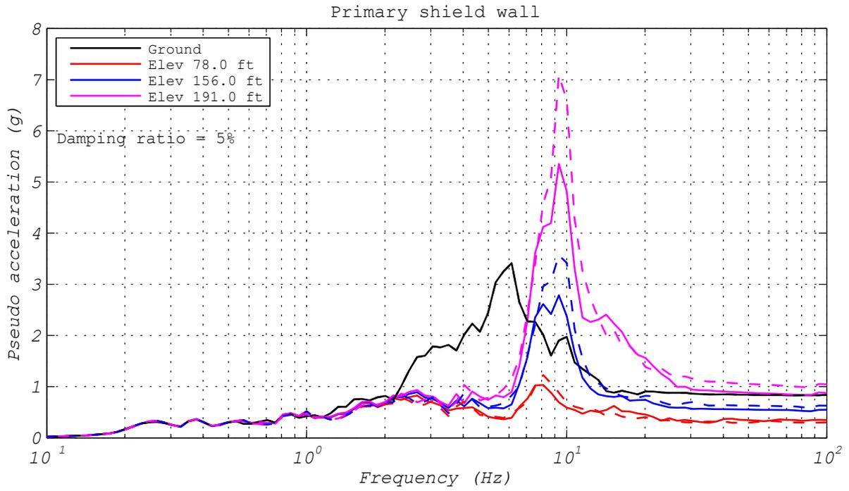
**Figure 3.63** EQS bearing: response spectra comparison of responses to ground motion NRC2 executed 25 times slower than real time (1D and 2D analyses).
