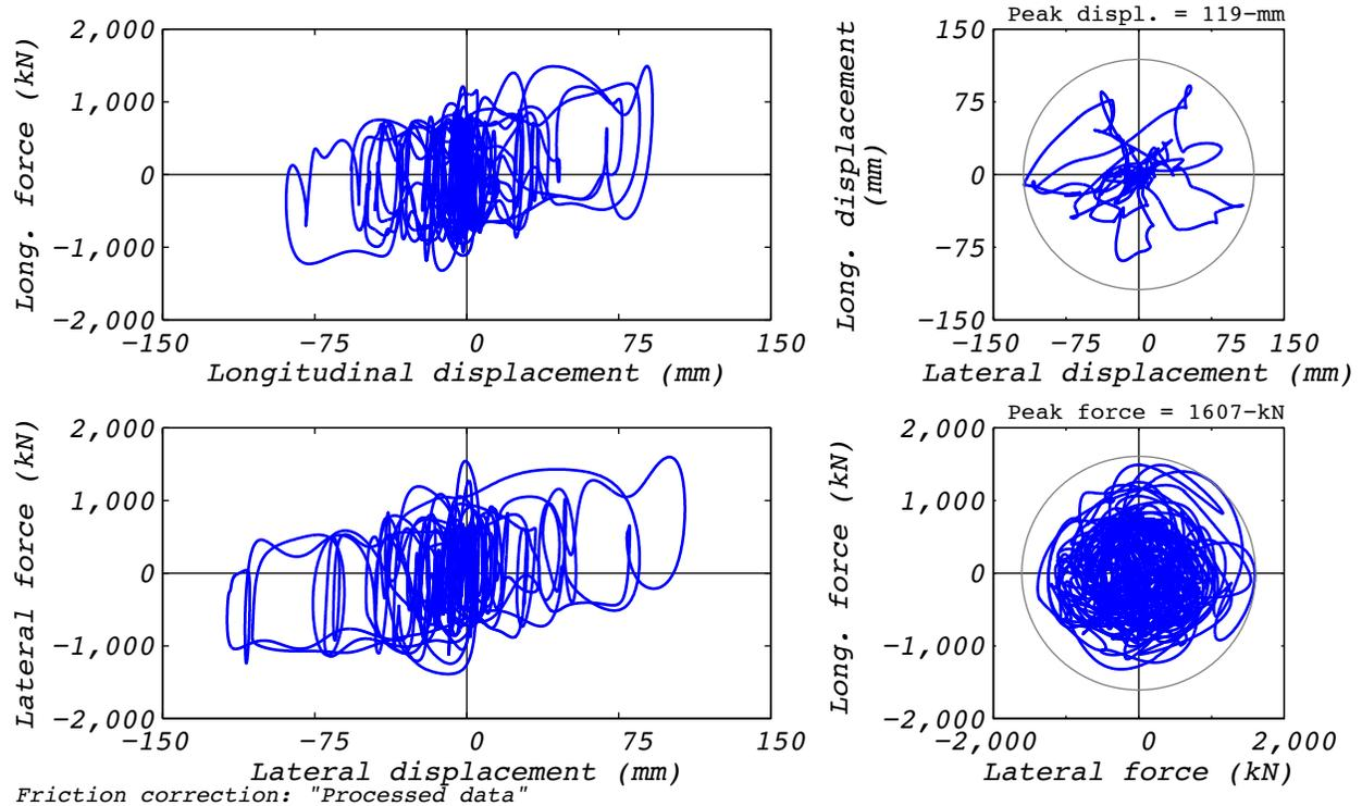
**Figure C.23-1 Bearing response for real-time reproduction of hybrid test run 54: NRC2, 2D with experimental bearing representing all bearings.**
