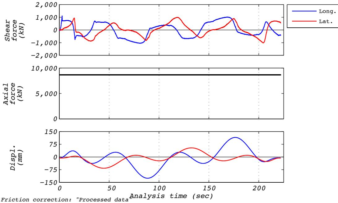
Figure D.27-1 Test run no. 33 time history: Clover leaf orbit (120 mm amplitude, 8,663 kN axial load, and varying velocity).
