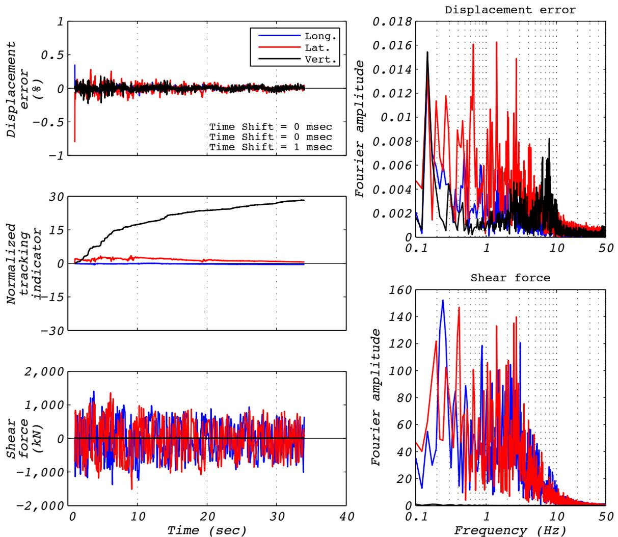
Figure C.13-1 Hybrid test performance metrics for run 49: NRC2, 3D with 5 groups of bearings and the experimental bearing representing the no. 3 corner group.
