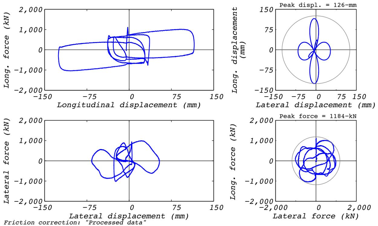
Figure D.27-2 Test run no. 33 hysteresis: Clover leaf orbit (120 mm amplitude, 8,663 kN axial load, and varying velocity).
