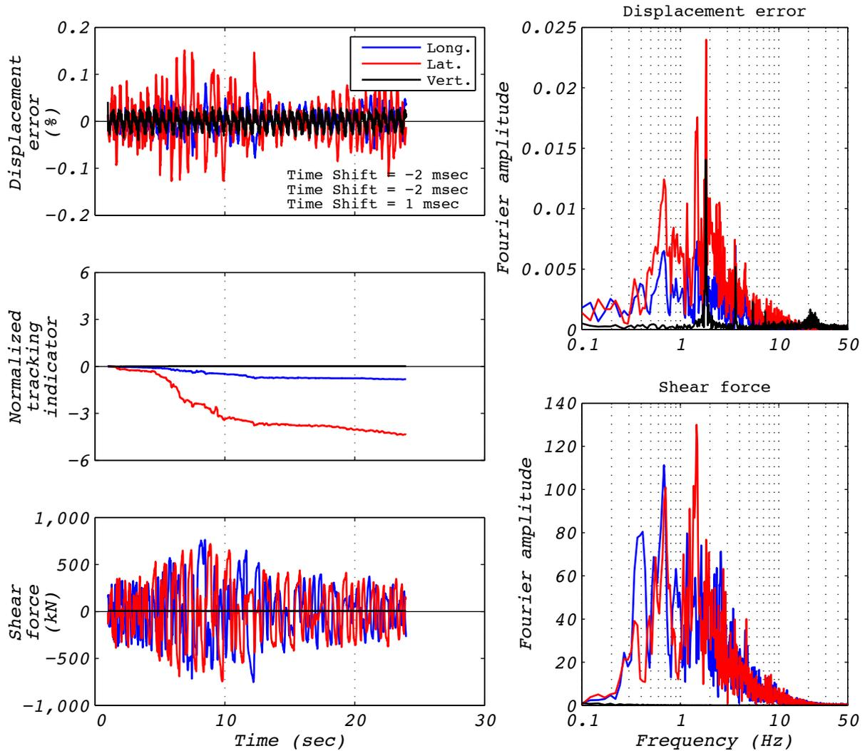
Figure A.21-1 Hybrid test performance metrics for run 78: EUR5, 3D with experimental bearing representing all bearings.
