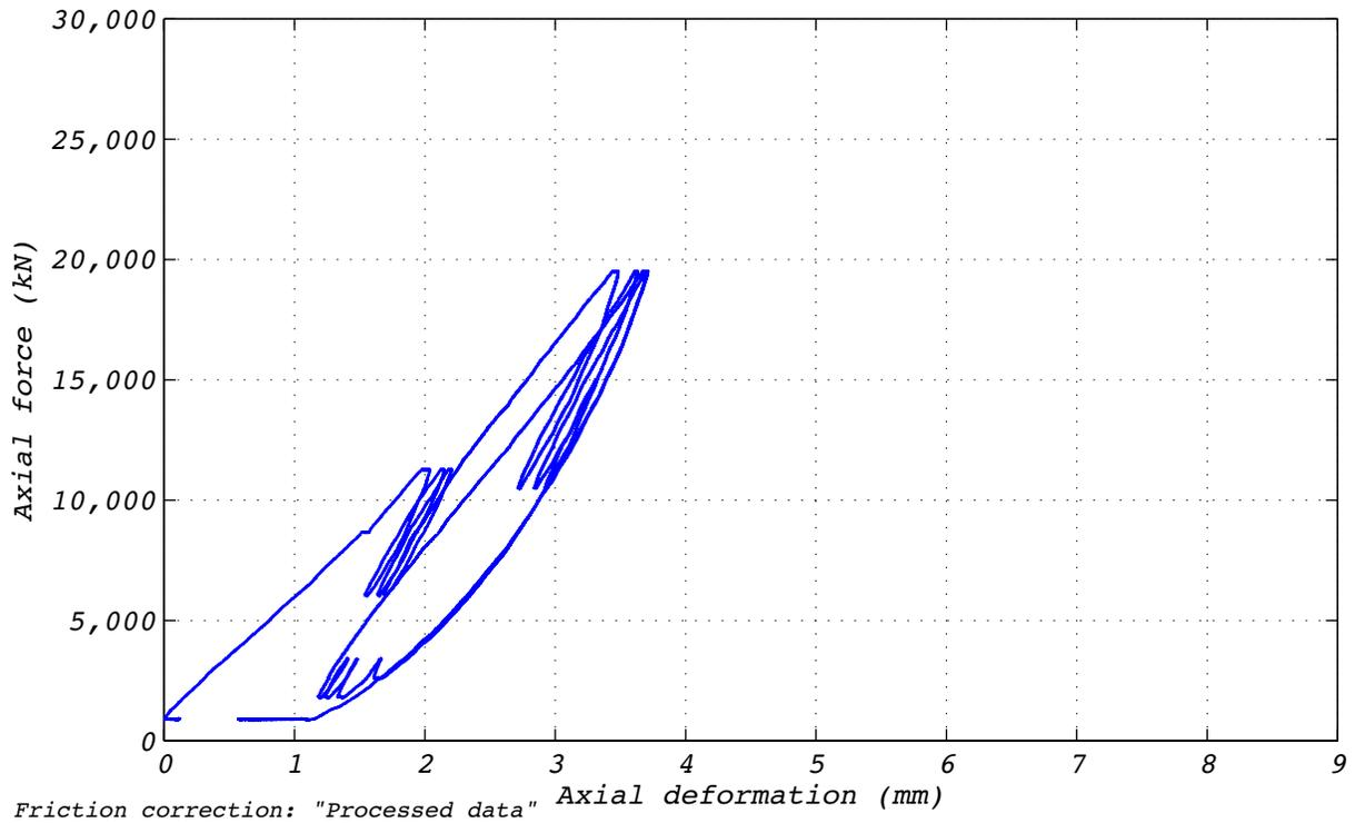
Figure D.3-2 Test run no. 3 hysteresis: Axial (120 mm displacement and varying axial load).
