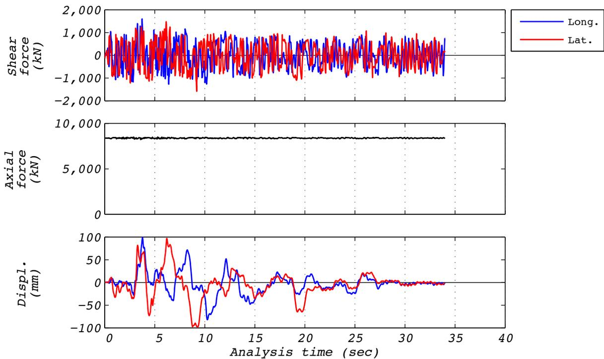
**Figure C.11-3 Hybrid test time history responses for run 47: NRC2, 3D with 5 groups of bearings and the experimental bearing representing the center group.**
