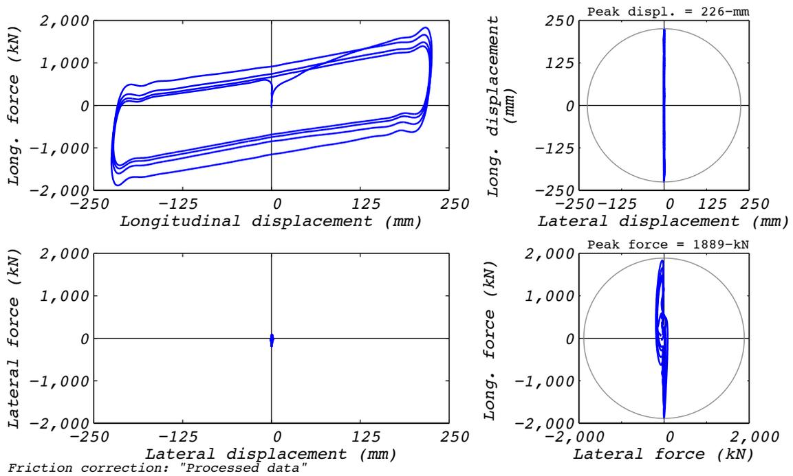
Figure B.32-2 Test run no. 75 hysteresis: Longitudinal (224 mm amplitude, 25,002 kN axial load, and 373 mm/s velocity).
