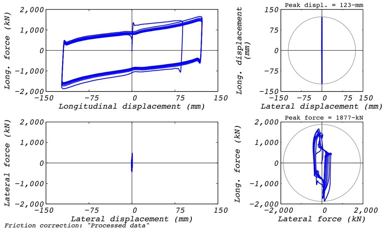
Figure D.9-2 Test run no. 9 hysteresis: Longitudinal (120 mm amplitude, 10,000 kN axial load, and 410 mm/s velocity).
