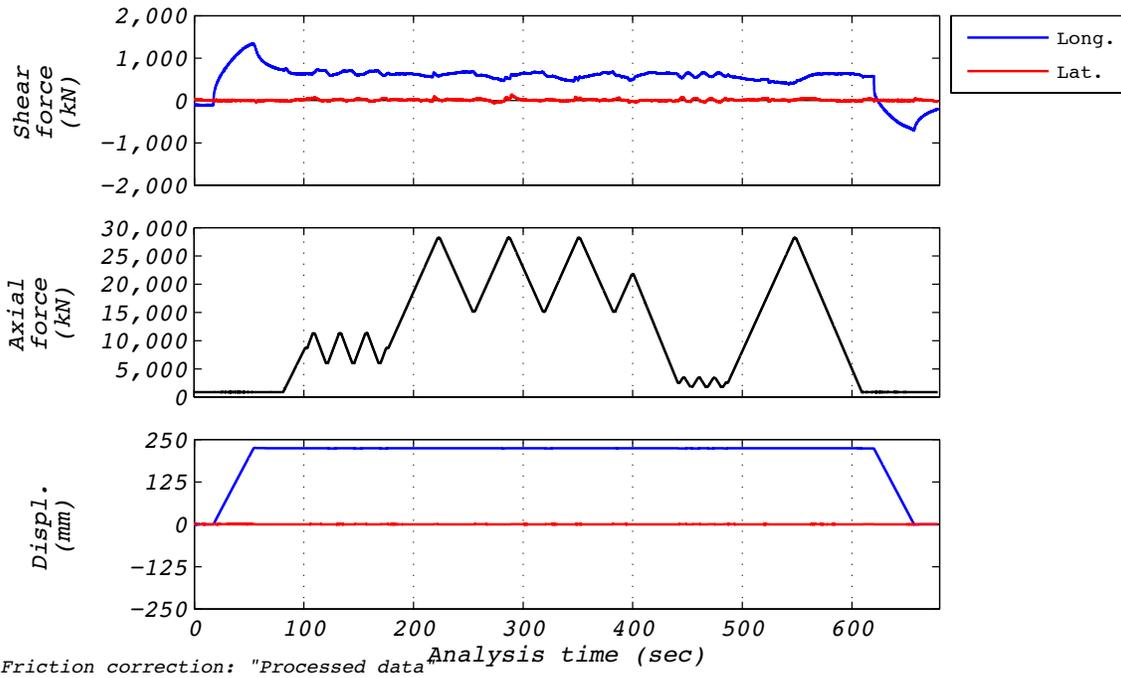
Figure B.8-1 Test run no. 17 time history: Axial (224 mm amplitude and varying axial load).
