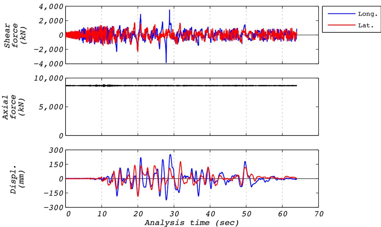
**Figure C.24-3 Hybrid test time history responses for run 58: NRC10, 2D with experimental bearing representing all bearings.**
