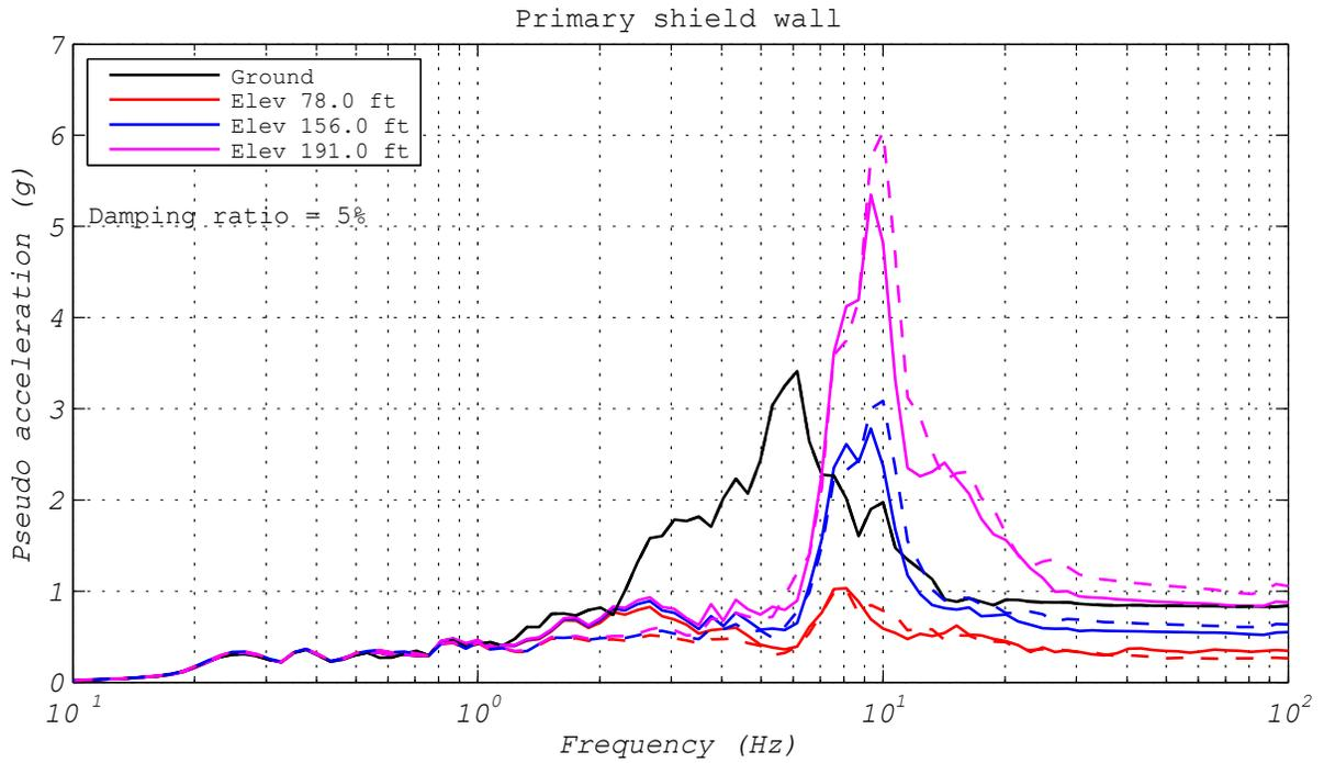
**Figure 3.75 EQS bearing: response spectra comparison of responses to loading rates (ground motion NRC2, 1D analysis).**
