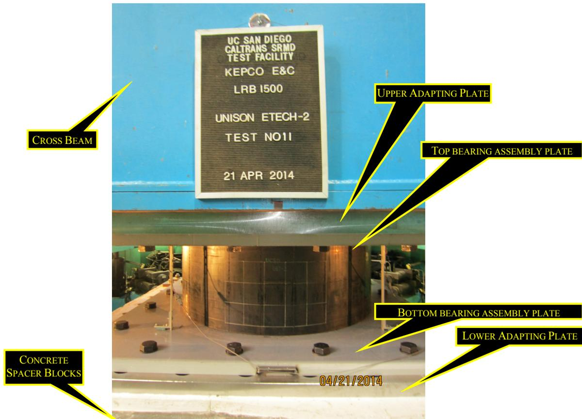
Figure 3.21 Overview of the typical test set-up.
