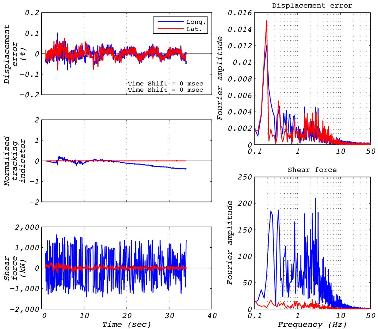
Figure C.6-1 Hybrid test performance metrics for run 22: NRC2, 1D with experimental bearing representing all bearings.
