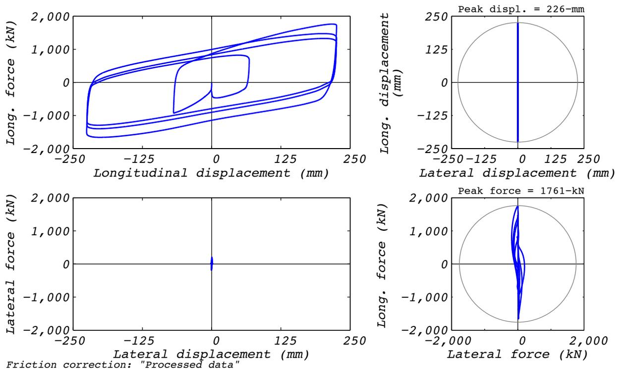
Figure B.19-2 Test run no. 59 hysteresis: Longitudinal (224 mm amplitude, 8,663 kN axial load, and 586 mm/s velocity).
