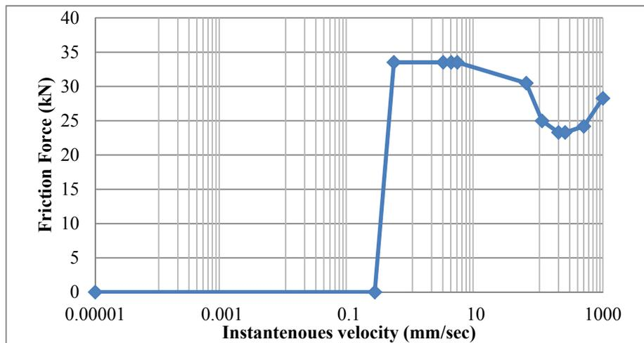
**Figure 3.13 Friction force for different instantaneous velocity values.**
