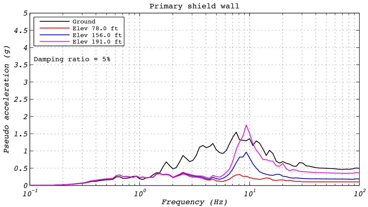
**Figure A.4-4 Hybrid test floor spectra for run 37: EUR5, 1D with experimental bearing representing all bearings.**
