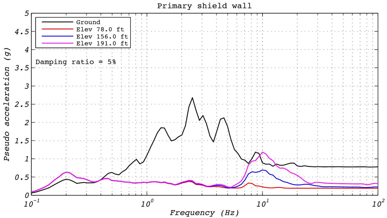
**Figure A.16-3 Floor spectra for analytical run 55A: NRC15, 2D with a single analytical bearing.**
