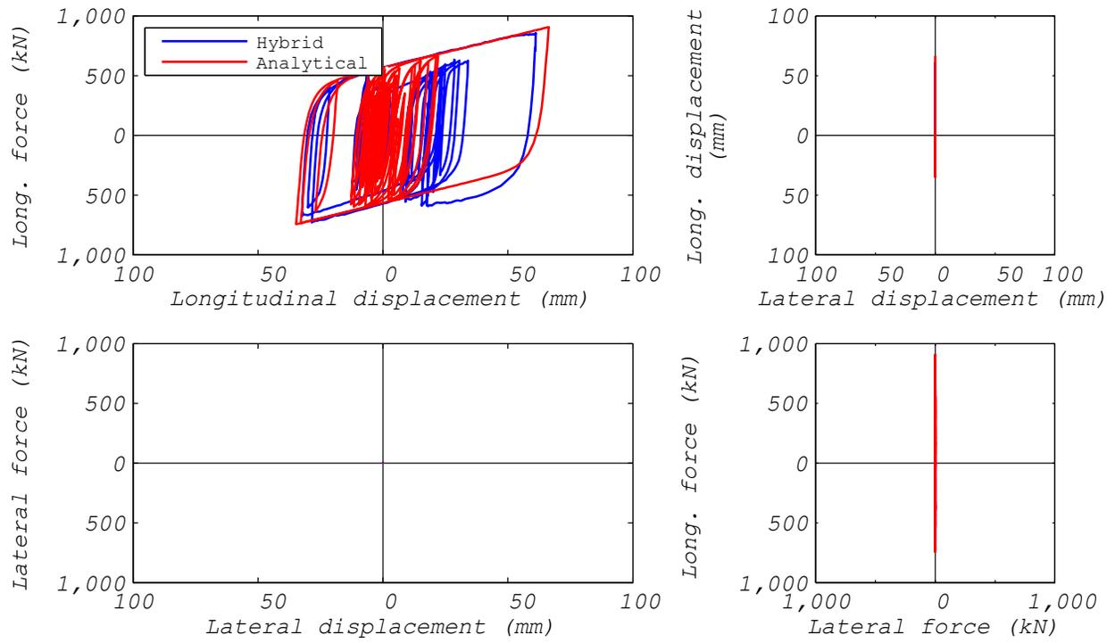
**Figure 3.52** LPRB bearing: comparison of hybrid simulation and analytical estimation bearing responses (ground motion EUR5, 1D analysis).
