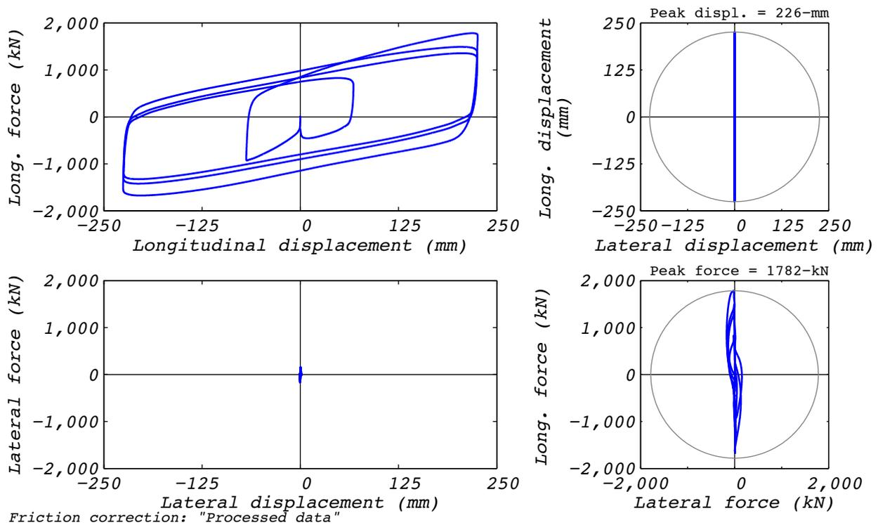
Figure B.2-2 Test run no. 9 hysteresis: Longitudinal (224 mm amplitude, 8,663 kN axial load, and 586 mm/s velocity).
