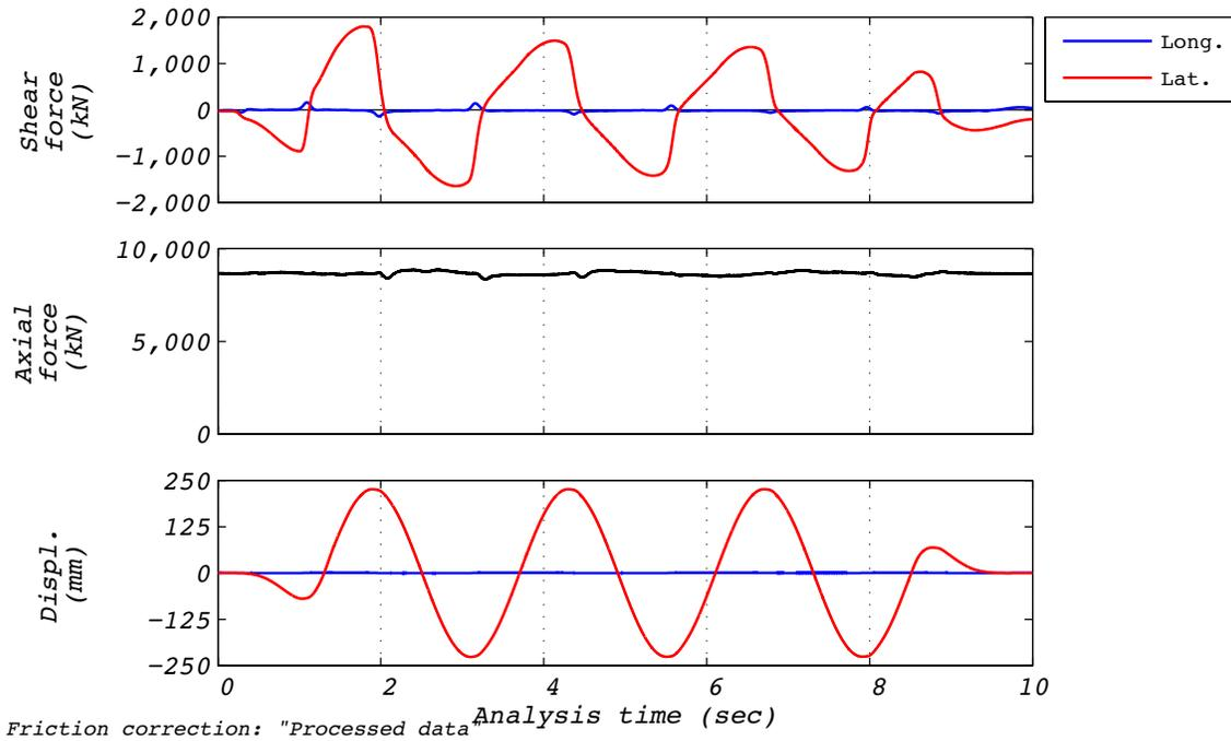
Figure B.27-1 Test run no. 70 time history: Transverse (224 mm amplitude, 8,663 kN axial load, and 586 mm/s velocity).
