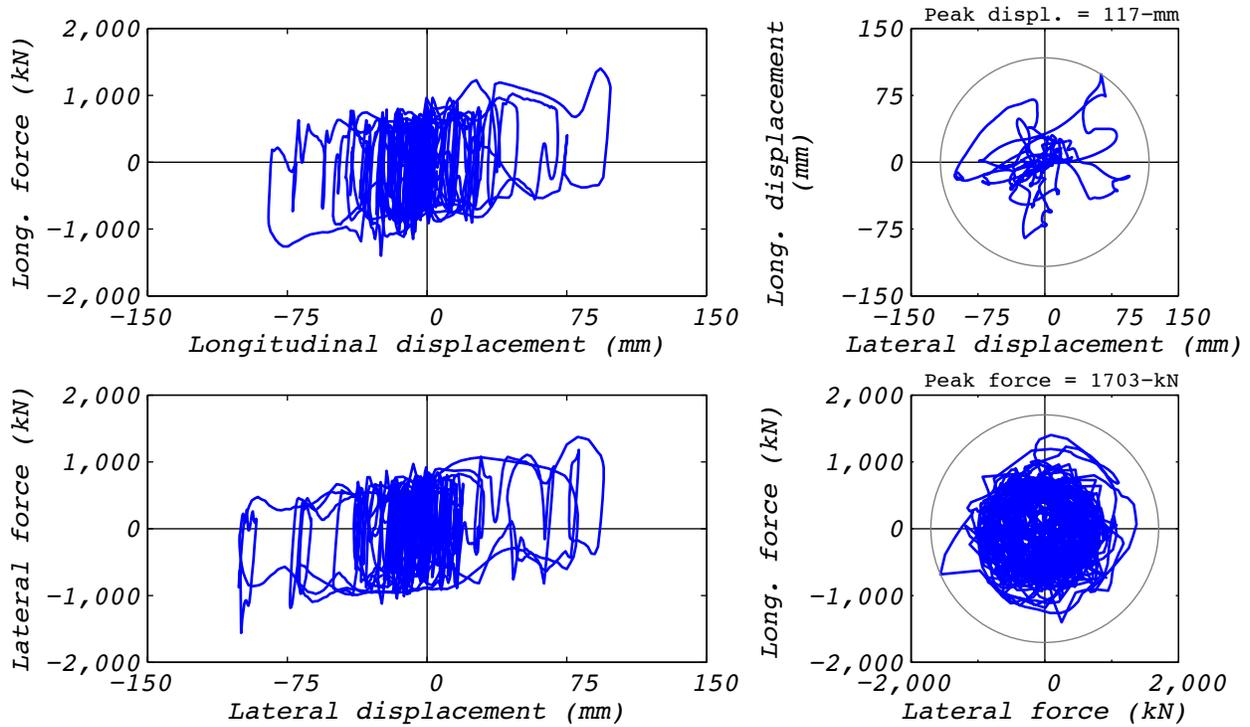
Figure C.14-2 Hybrid test bearing response for run 50: NRC2, 3D with 5 groups and the experimental bearing representing the no. 3 corner group.
