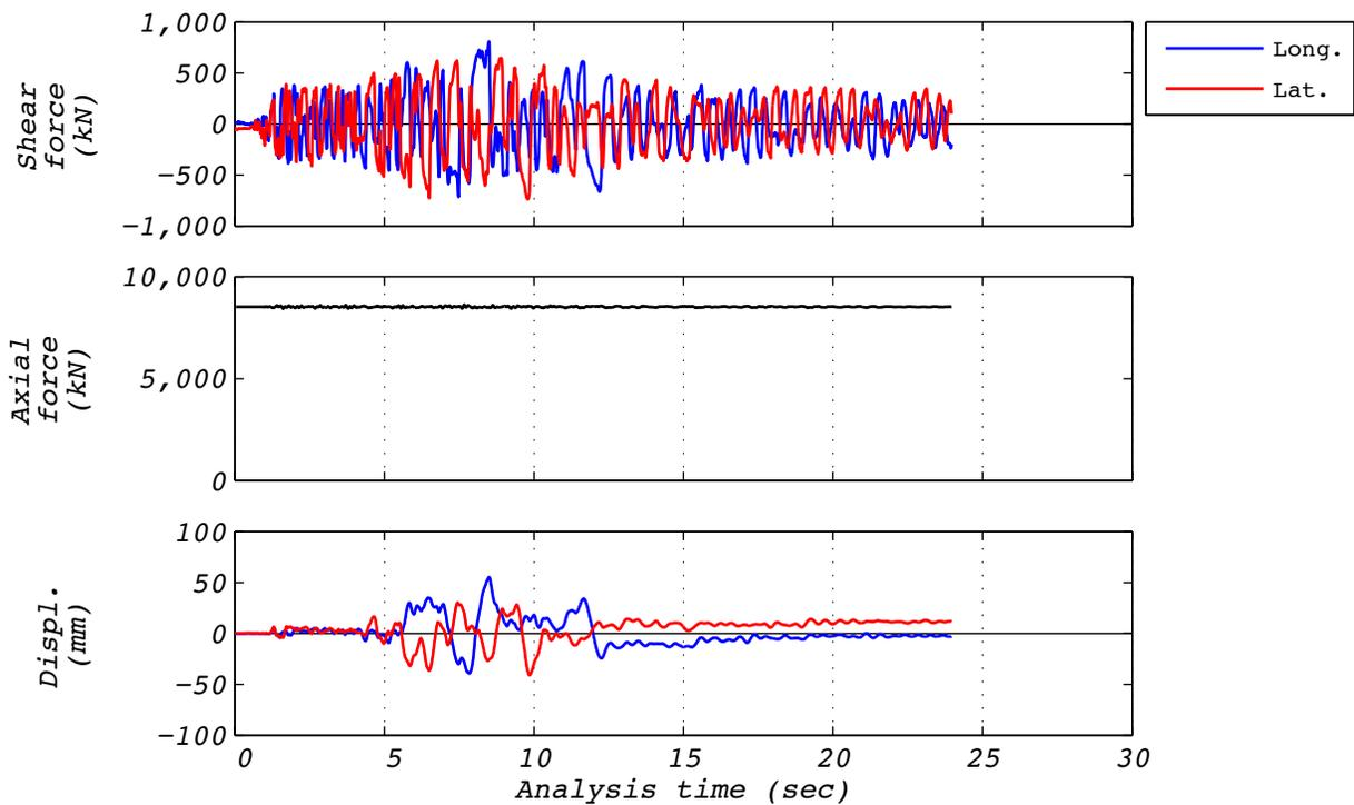
**Figure A.22-3 Hybrid test time history responses for run 79: EUR5, 3D with 5 groups of bearings and the experimental bearing representing the center group.**
