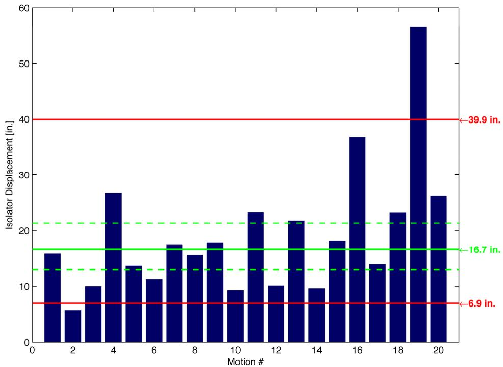
**Figure 3.30** Analytically determined peak lateral displacement demands for the NRC hazard level [1973] based on an LPRB isolator (green lines = median with 95% confidence interval, red lines = 5<sup>th</sup> and 95<sup>th</sup> percentile).
