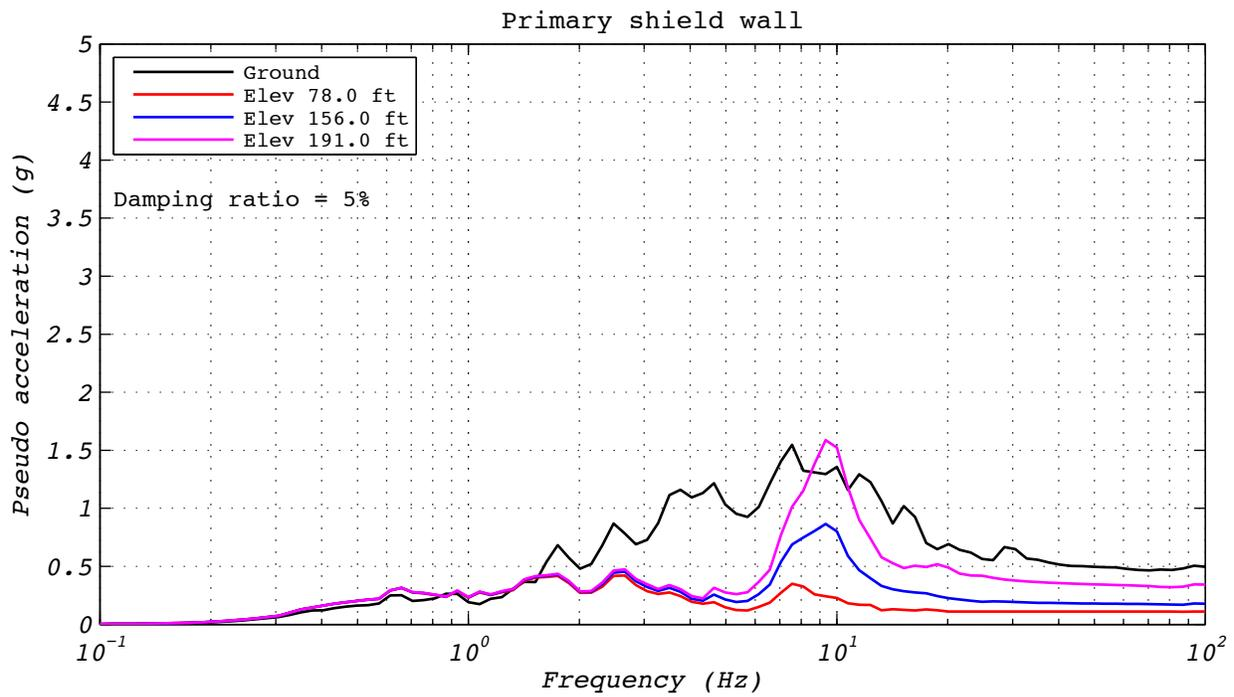
**Figure A.9-3 Floor spectra for analytical run 44A: EUR5, 1D with a single analytical bearing.**
