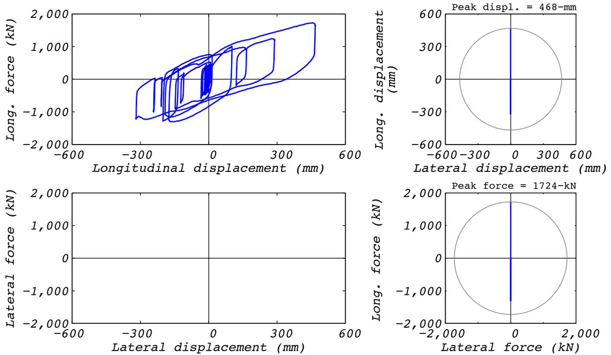
**Figure A.13-2 Hybrid test bearing response for run 47: NRC15, 1D with experimental bearing representing all bearings.**
