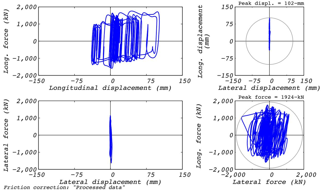
Figure C.7-1 Bearing response for real-time reproduction of hybrid test run 22: NRC2, 1D with experimental bearing representing all bearings.
