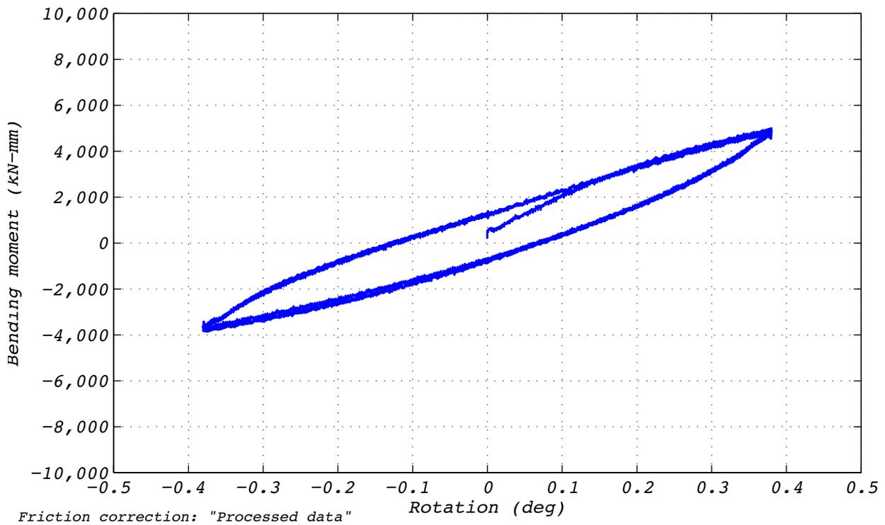
Figure D.6-2 Test run no. 6 hysteresis: Transverse rotation (0 mm displacement and 8,663 kN axial load).
