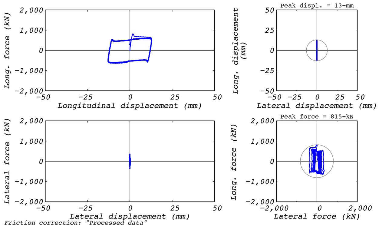
Figure D.30-2 Test run no. 36 hysteresis: Longitudinal (13 mm amplitude, 8,663 kN axial load, and 4 mm/s velocity).
