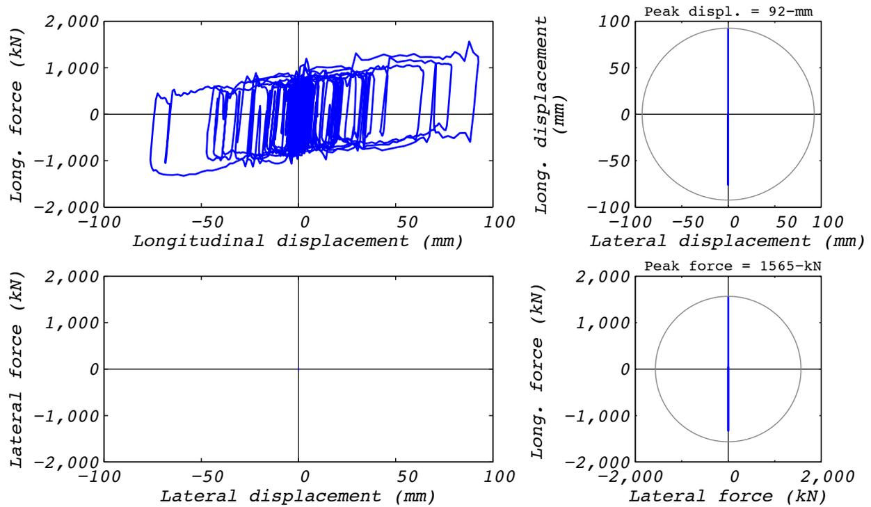
**Figure C.16-2 Hybrid test bearing response for run 52: NRC2, 1D with experimental bearing representing all bearings.**
