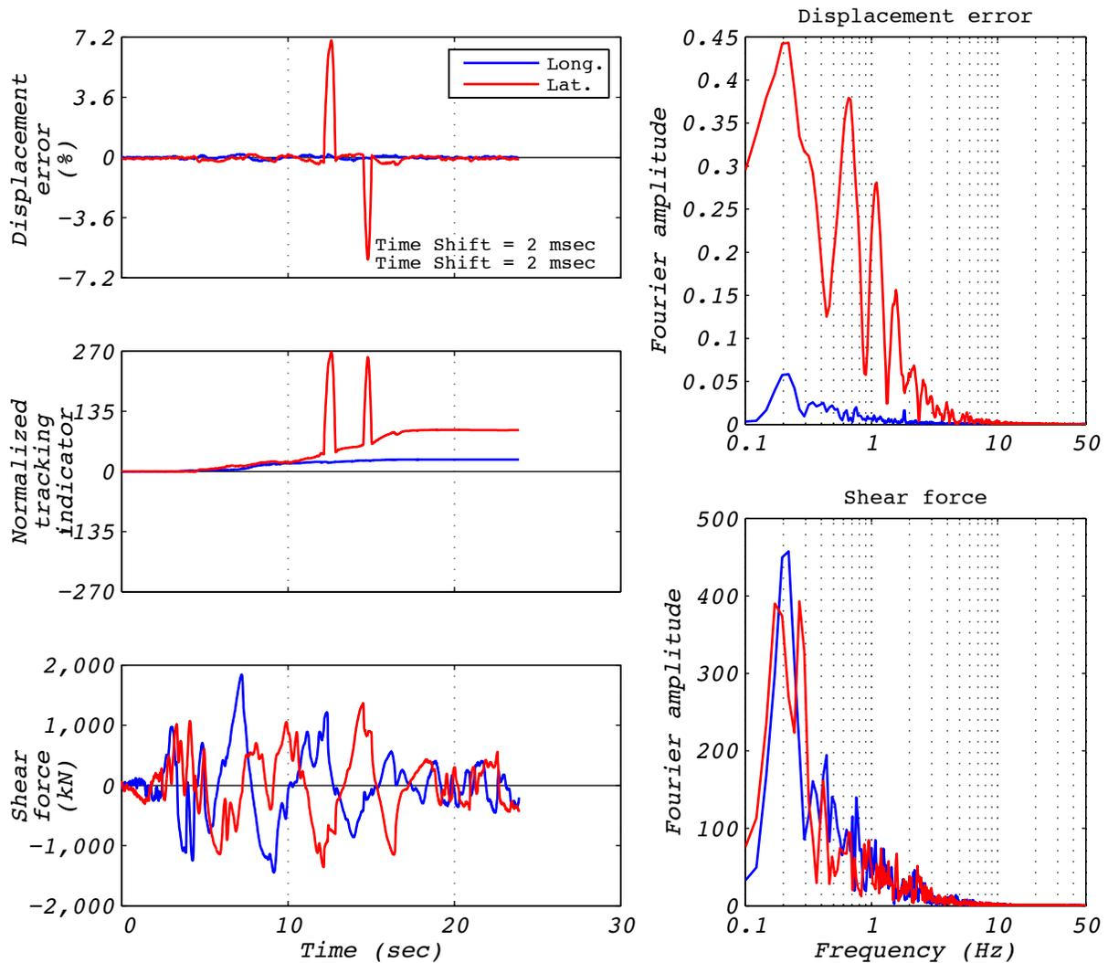
Figure A.12-1 Hybrid test performance metrics for run 46: NRC15, 2D with experimental bearing representing all bearings.
