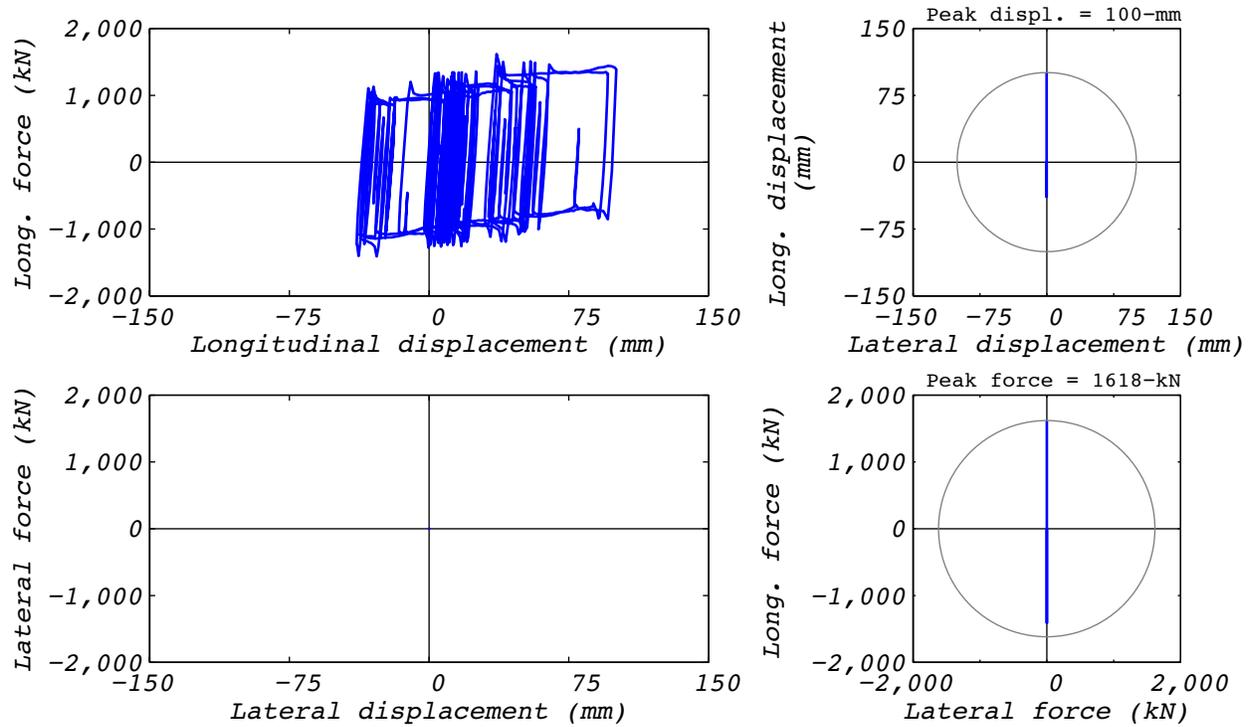
**Figure C.6-2 Hybrid test bearing response for run 22: NRC2, 1D with experimental bearing representing all bearings.**
