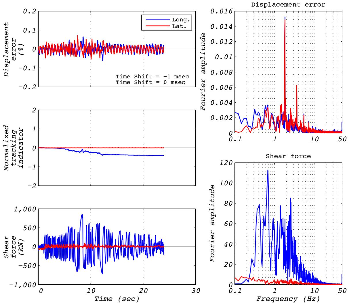
Figure A.7-1 Hybrid test performance metrics for run 43: EUR5, 1D with experimental bearing representing all bearings.
