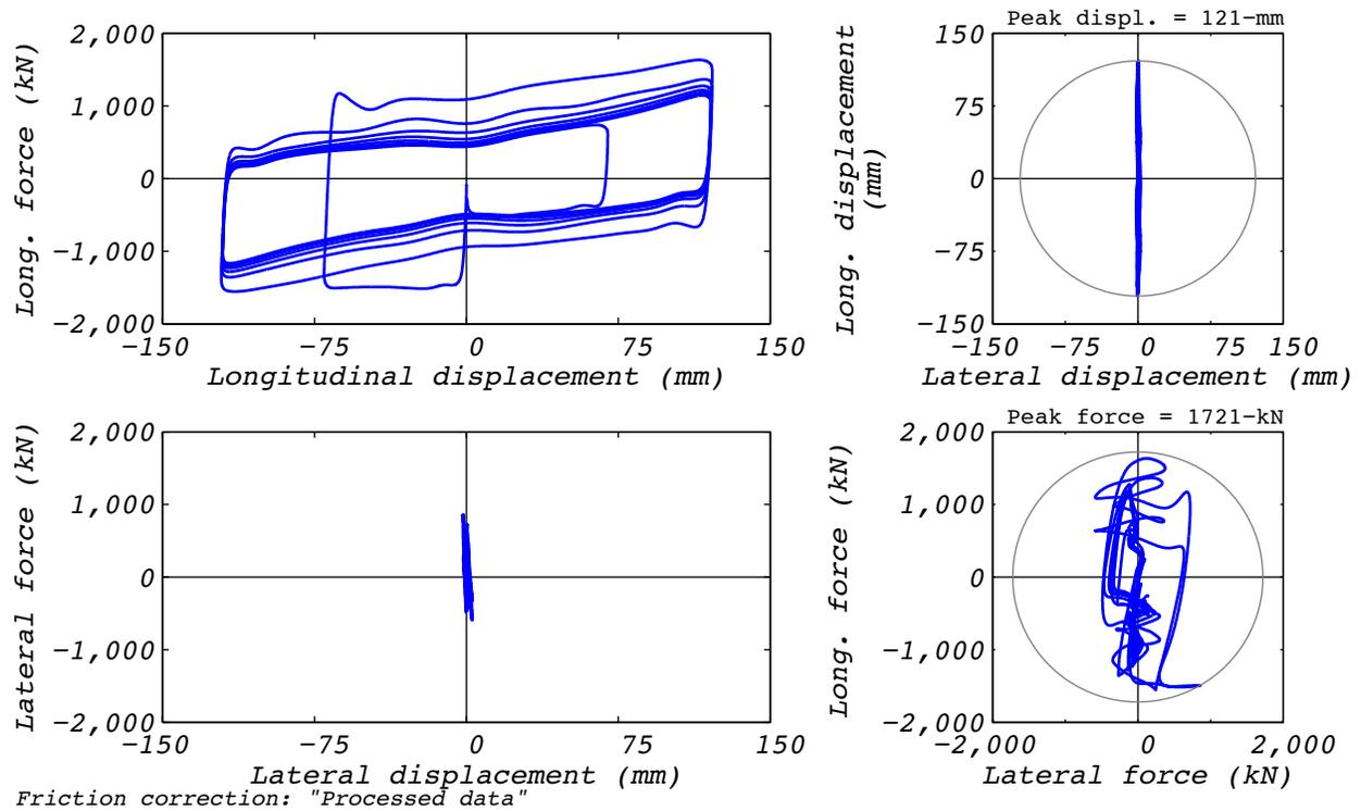
Figure D.18-2 Test run no. 24 hysteresis: Longitudinal (120 mm amplitude, 8,663 kN axial load, and 410 mm/s velocity).
