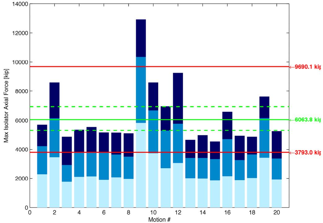
**Figure 3.29** Analytically determined peak axial force demands for the EUR hazard level [2012] based on an LPRB isolator (green lines = median with 95% confidence interval, red lines = 5<sup>th</sup> and 95<sup>th</sup> percentile).
