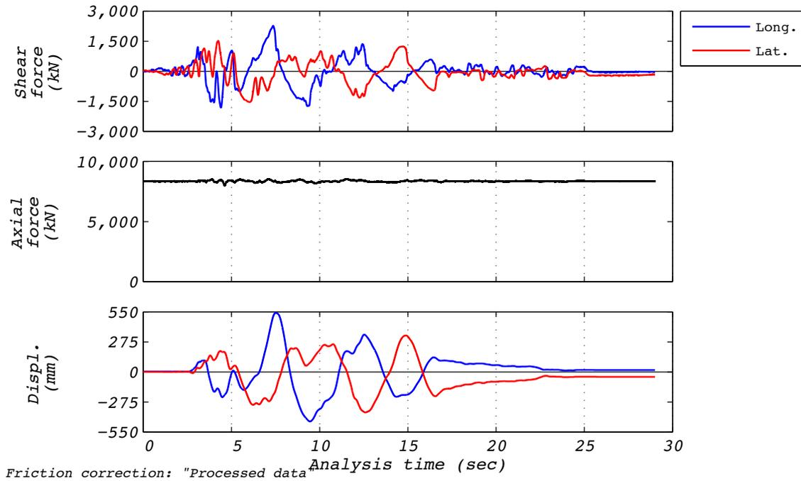
Figure B.35-1 Test run no. 87 time history: Longitudinal (444 mm amplitude, 8,663 kN axial load, and 485 mm/s velocity).
