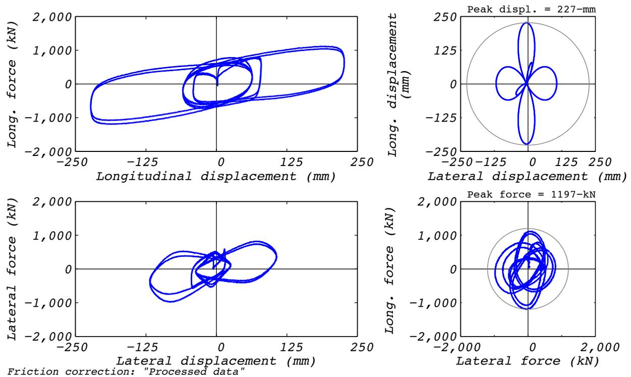
Figure B.18-2 Test run no. 57 hysteresis: Clover leaf orbit (224 mm amplitude, 8,664 kN axial load, and varying velocity).
