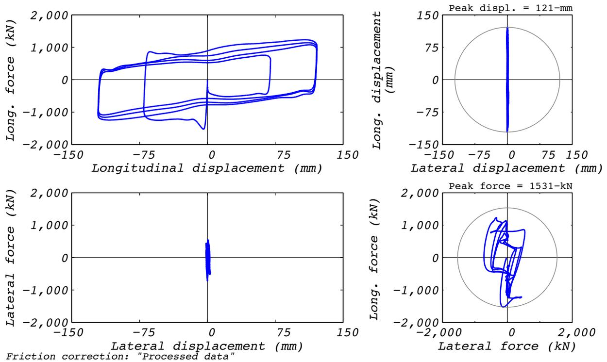
Figure D.31-2 Test run no. 59 hysteresis: Longitudinal (120 mm amplitude, 8,663 kN axial load, and 410 mm/s velocity).
