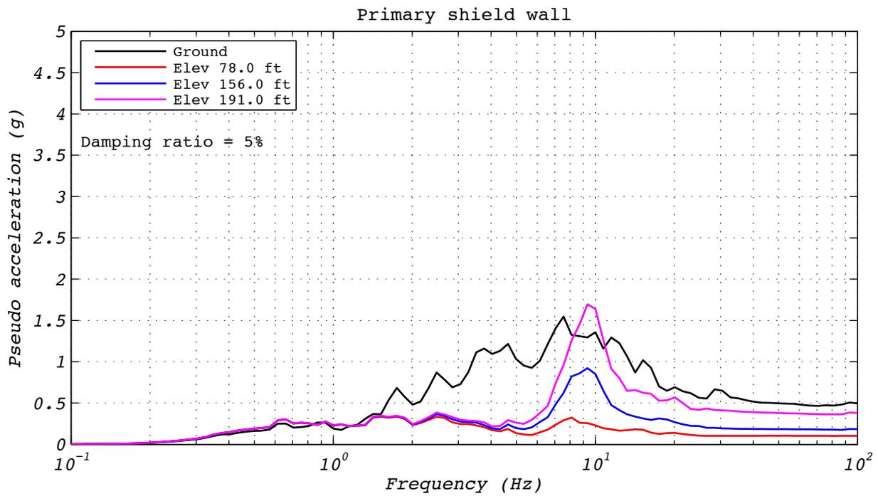
**Figure A.6-4 Hybrid test floor spectra for run 42: EUR5, 1D with experimental bearing representing all bearings.**
