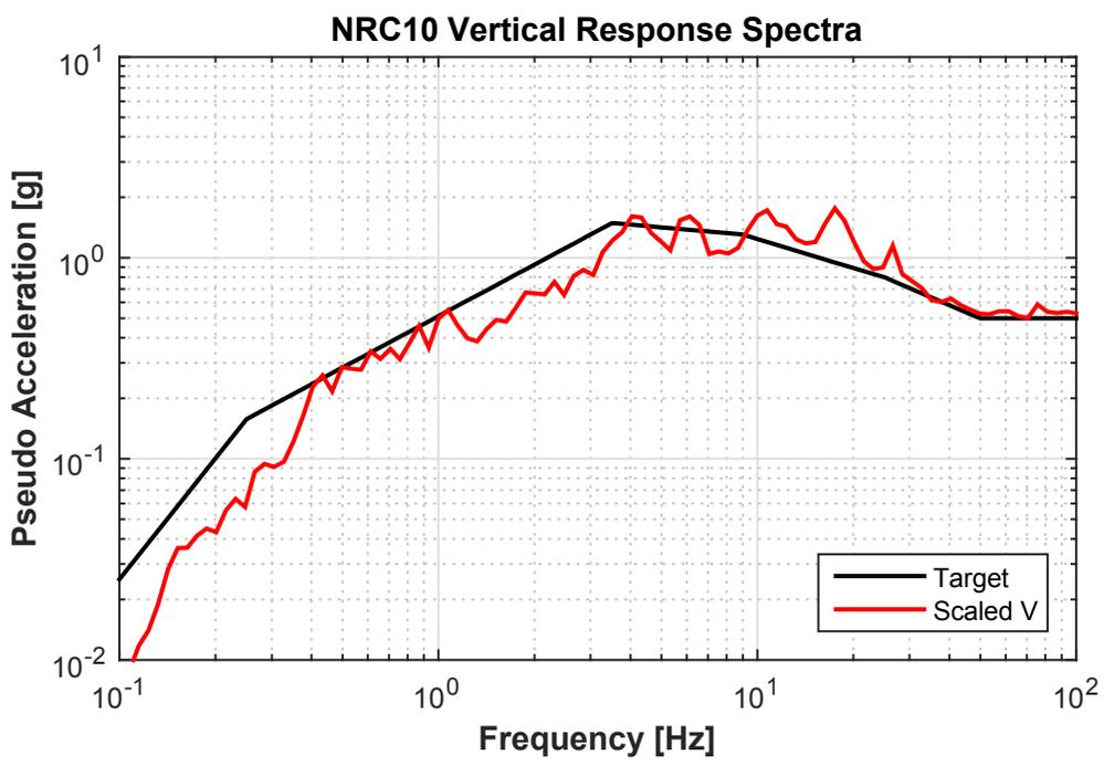
Figure 3.38 Response spectra of the NRC10 ground motion characterizing the NRC hazard level [1973].
