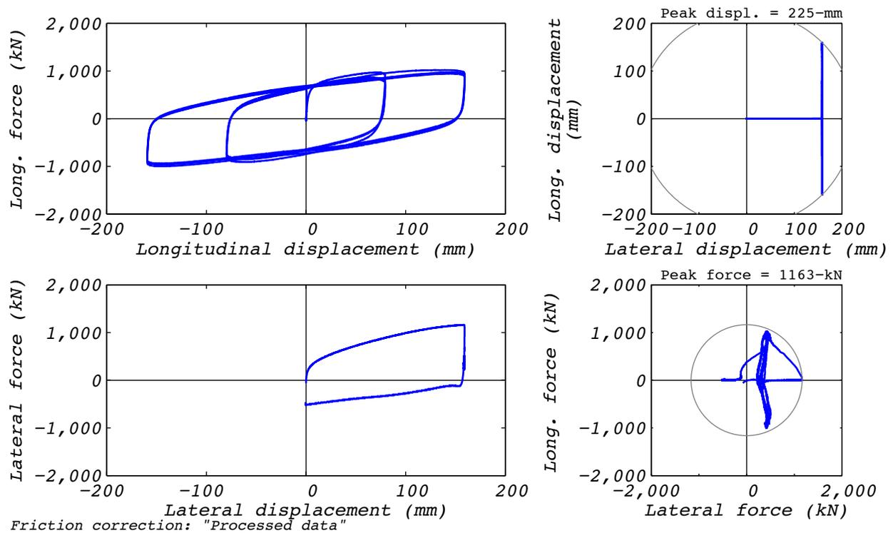
Figure B.20-2 Test run no. 62 hysteresis: Bidirectional (224 mm amplitude, 8,663 kN axial load, and 28 mm/s velocity).
