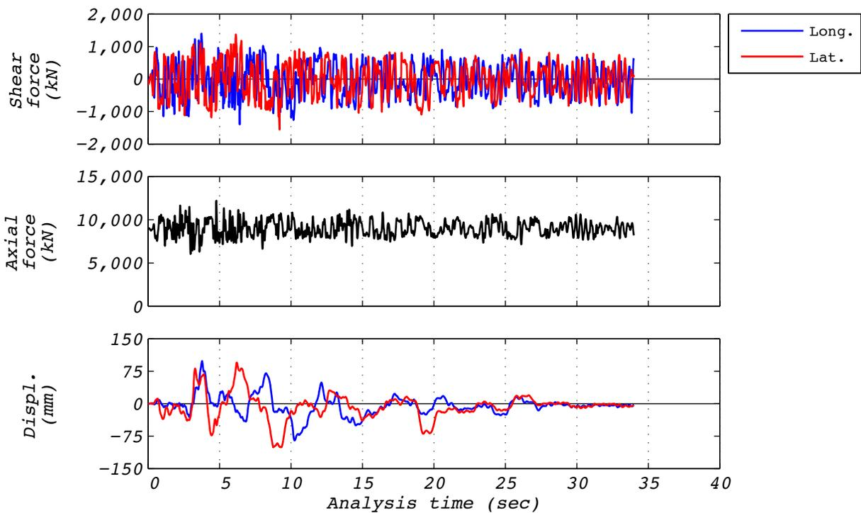
Figure C.14-3 Hybrid test time history responses for run 50: NRC2, 3D with 5 groups and the experimental bearing representing the no. 3 corner group.
