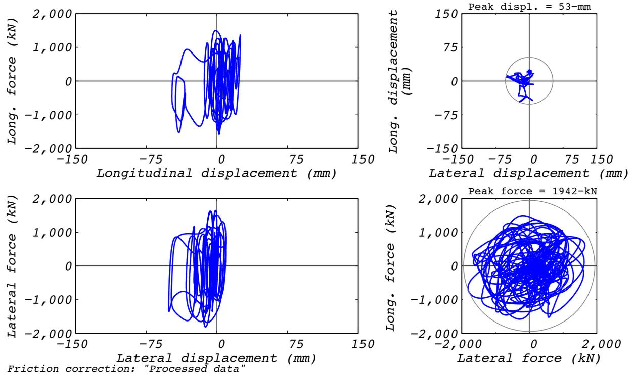
Figure C.4-1 Bearing response for real-time reproduction of hybrid test run 18: EUR5, 2D with experimental bearing representing all bearings.
