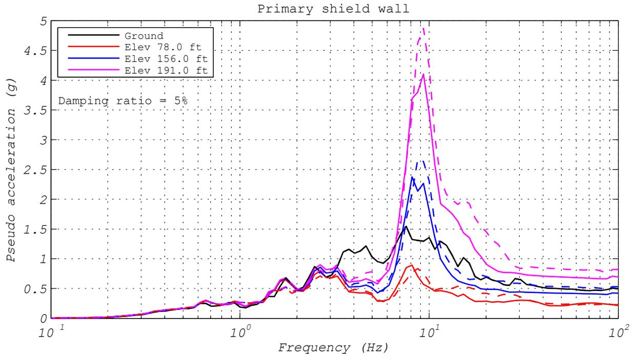
**Figure 3.61** EQS bearing: response spectra comparison of responses to ground motion EUR5 (1D and 2D analyses).
