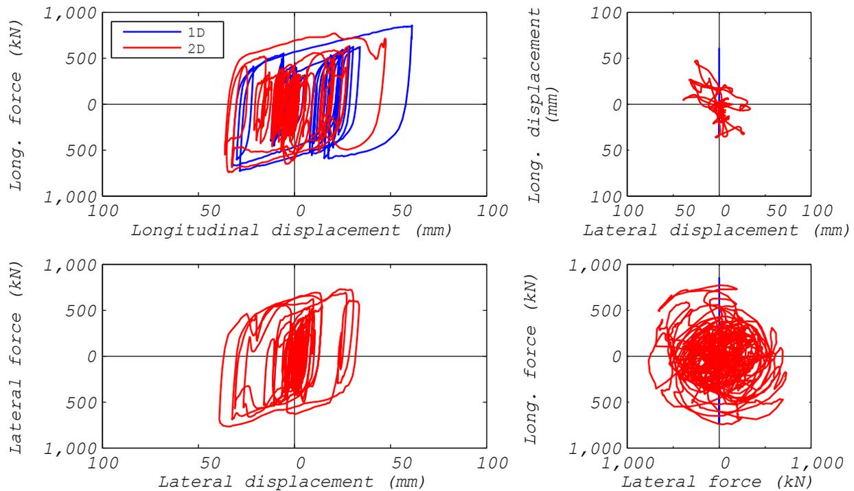
**Figure 3.40** LPRB bearing: comparison of bearing responses to ground motion EUR5 (1D and 2D analyses).
