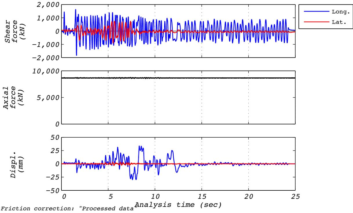
**Figure C.22-2 Time history responses for real-time reproduction of hybrid test run 53: EUR5, 1D with experimental bearing representing all bearings.**
