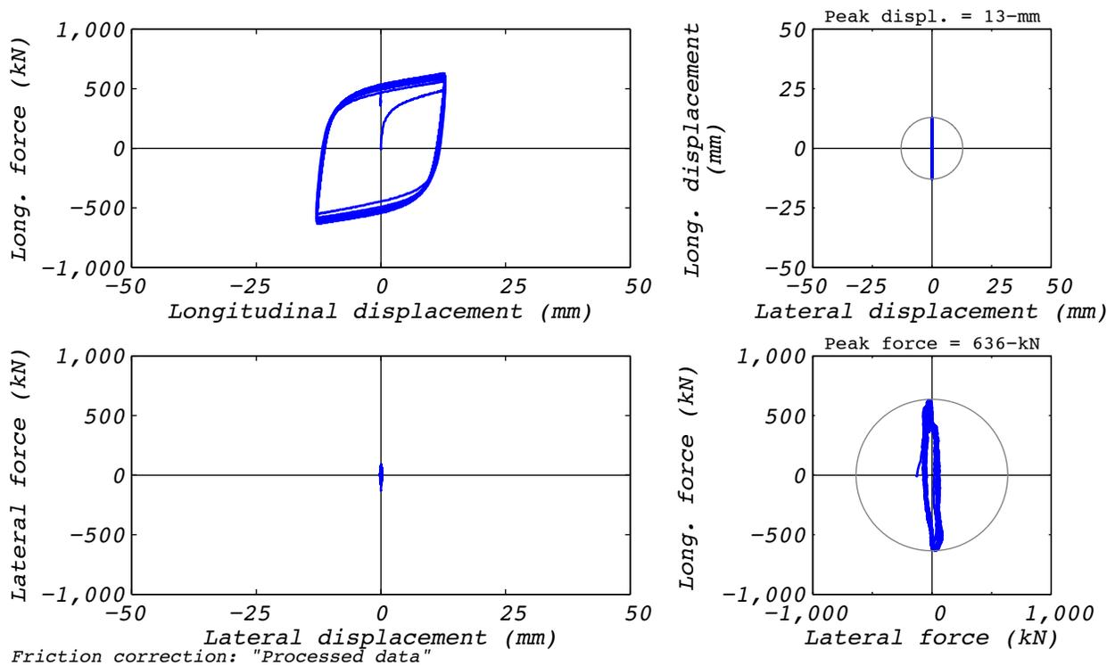
Figure B.34-2 Test run no. 81 hysteresis: Longitudinal (13 mm amplitude, 8,663 kN axial load, and 4 mm/s velocity).
