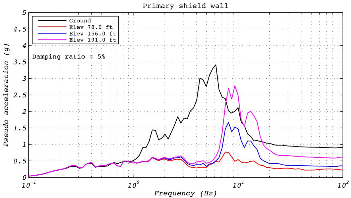
**Figure C.13-4 Hybrid test floor spectra for run 49: NRC2, 3D with 5 groups of bearings and the experimental bearing representing the no. 3 corner group.**
