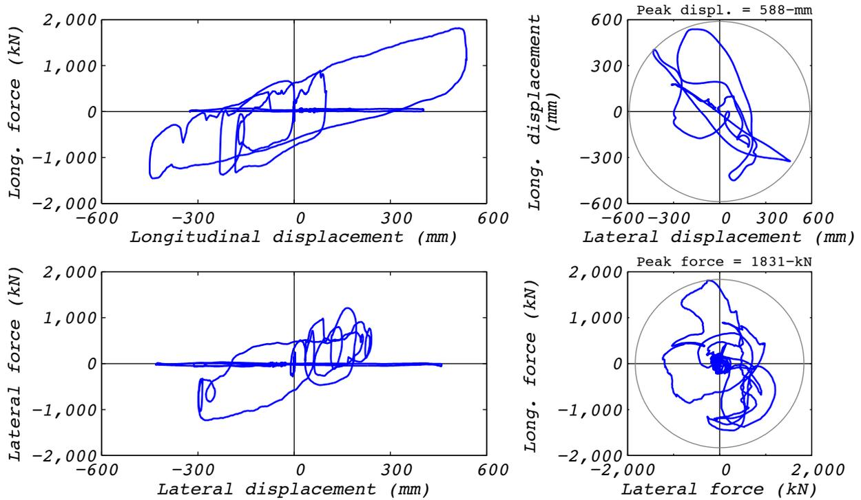
**Figure A.29-2 Hybrid test bearing response for run 88: NRC15, 3D with 5 groups and the experimental bearing representing the no. 3 corner group.**
