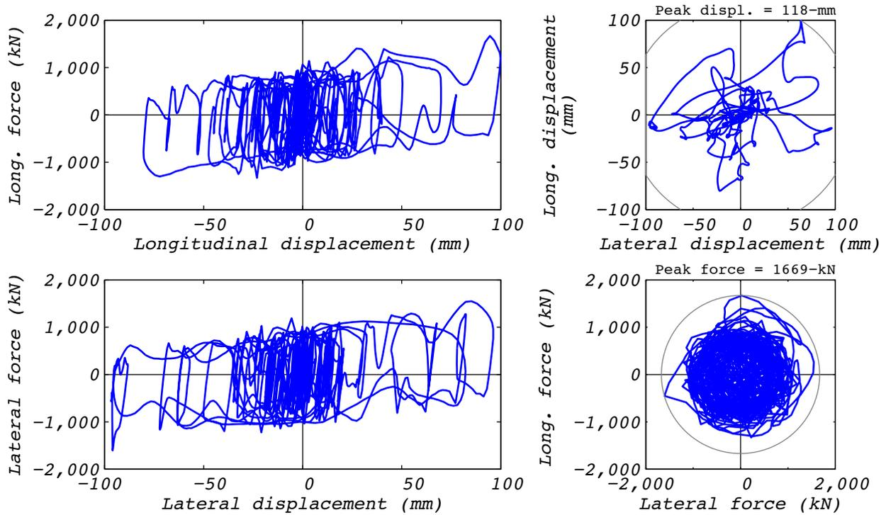
**Figure C.10-2 Hybrid test bearing response for run 46: NRC2, 3D with 5 groups of bearings and the experimental bearing representing the center group.**
