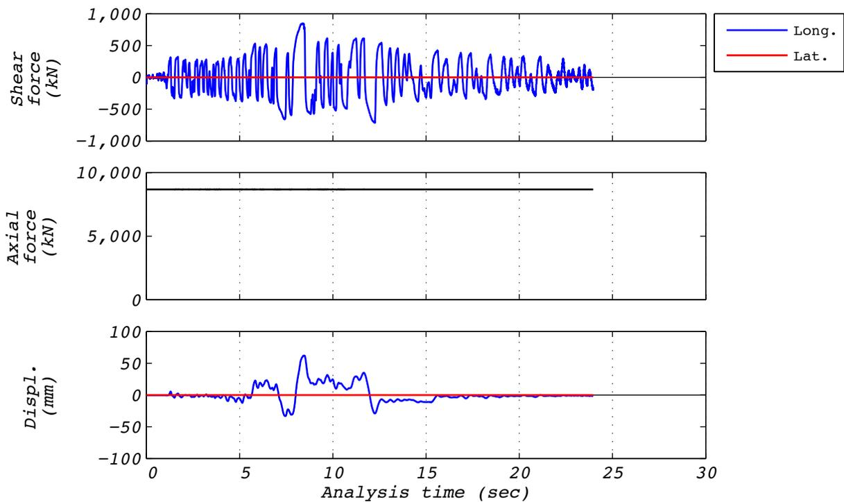
**Figure A.7-3 Hybrid test time history responses for run 43: EUR5, 1D with experimental bearing representing all bearings.**
