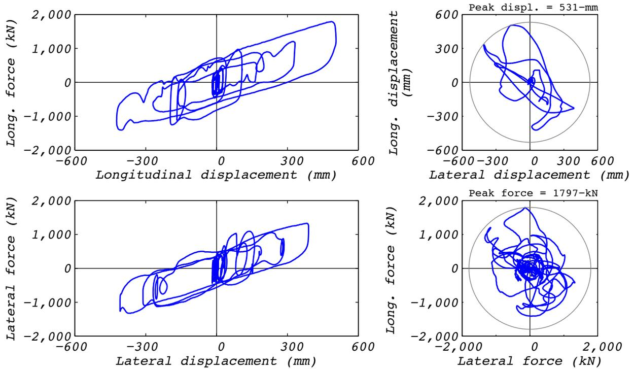
**Figure A.15-2 Hybrid test bearing response for run 55: NRC15, 2D with experimental bearing representing all bearings.**
