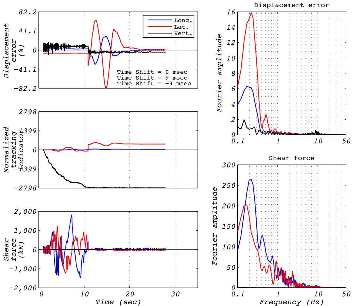
Figure A.29-1 Hybrid test performance metrics for run 88: NRC15, 3D with 5 groups of bearings and the experimental bearing representing the no. 3 corner group.
