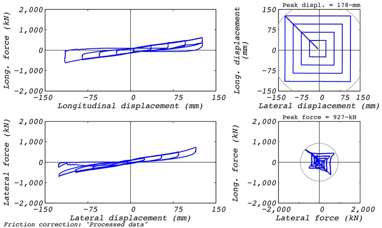
Figure D.23-2 Test run no. 29 hysteresis: Square orbit (Varying amplitude, 178 kN axial load, and varying velocity).
