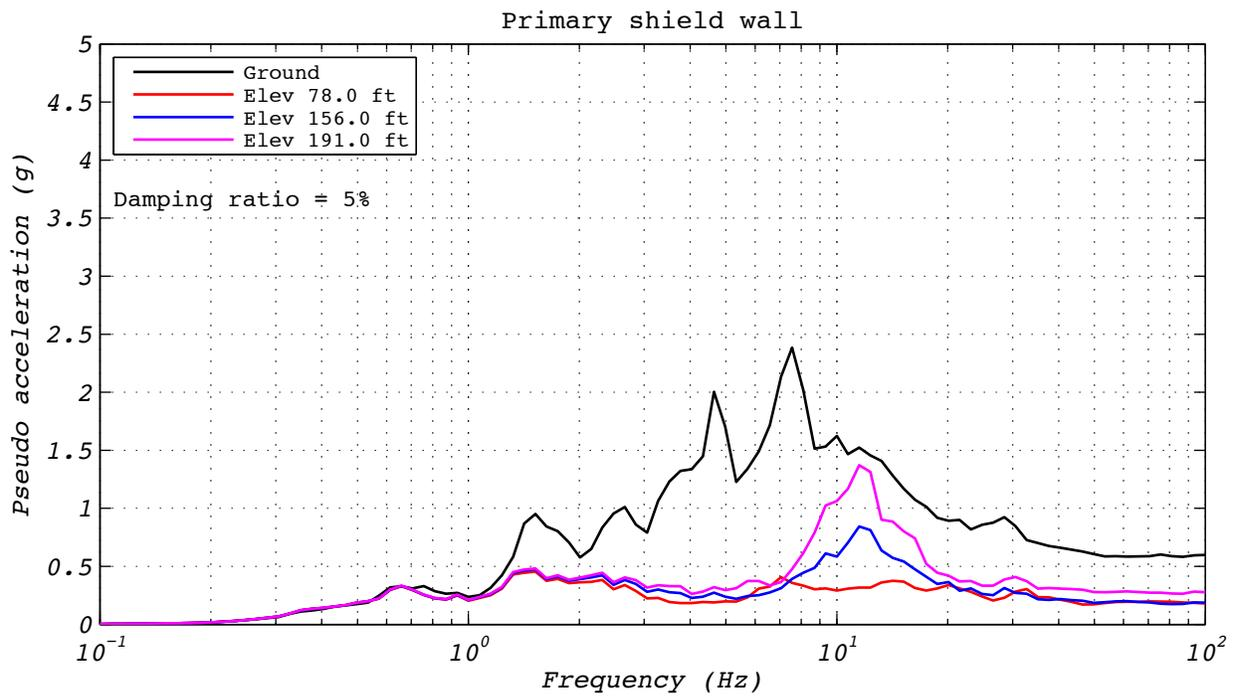
**Figure A.22-4 Hybrid test floor spectra for run 79: EUR5, 3D with 5 groups of bearings and the experimental bearing representing the center group.**
