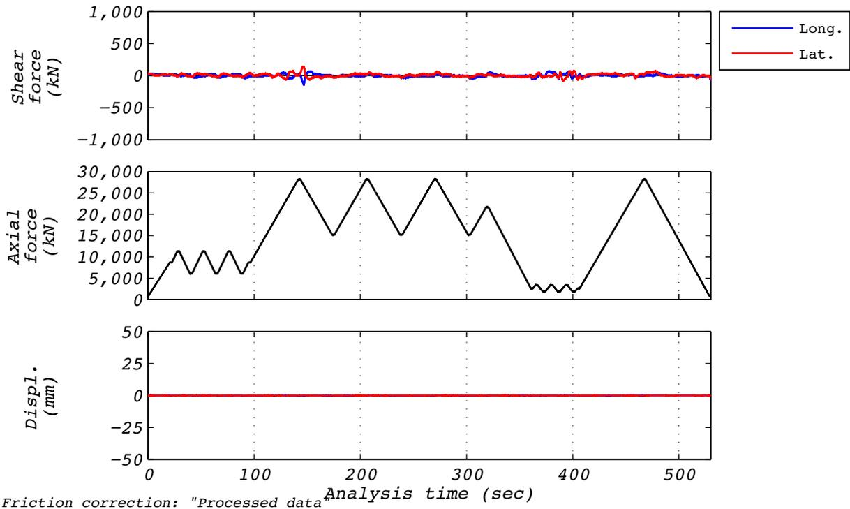
Figure B.1-1 Test run no. 8 time history: Axial compression (0 mm amplitude and varying axial load).
