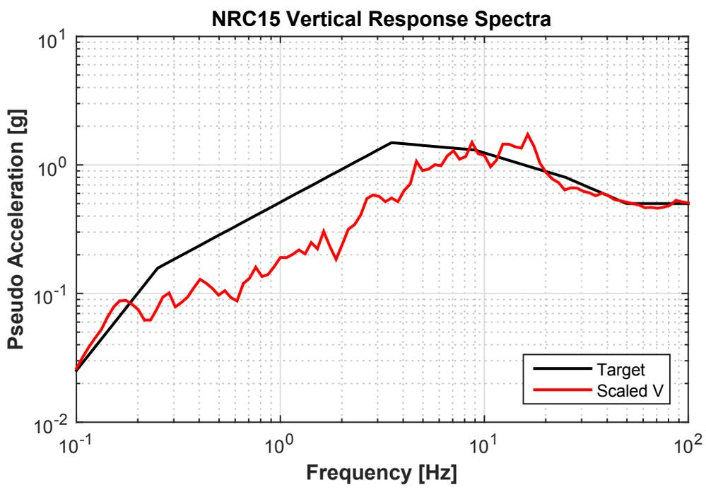
Figure 3.39 Response spectra of the NRC15 ground motion characterizing the NRC hazard level [1973].
