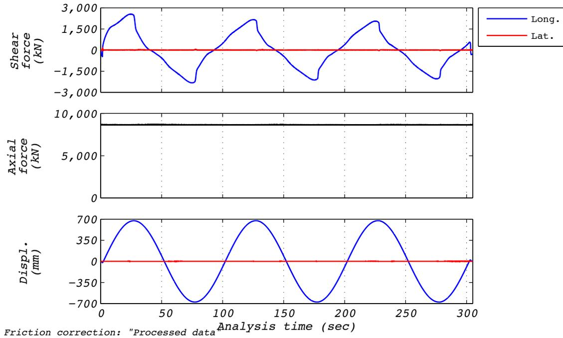
Figure B.22-1 Test run no. 65 time history: Longitudinal (896 mm amplitude, 8,663 kN axial load, and 56 mm/s velocity).
