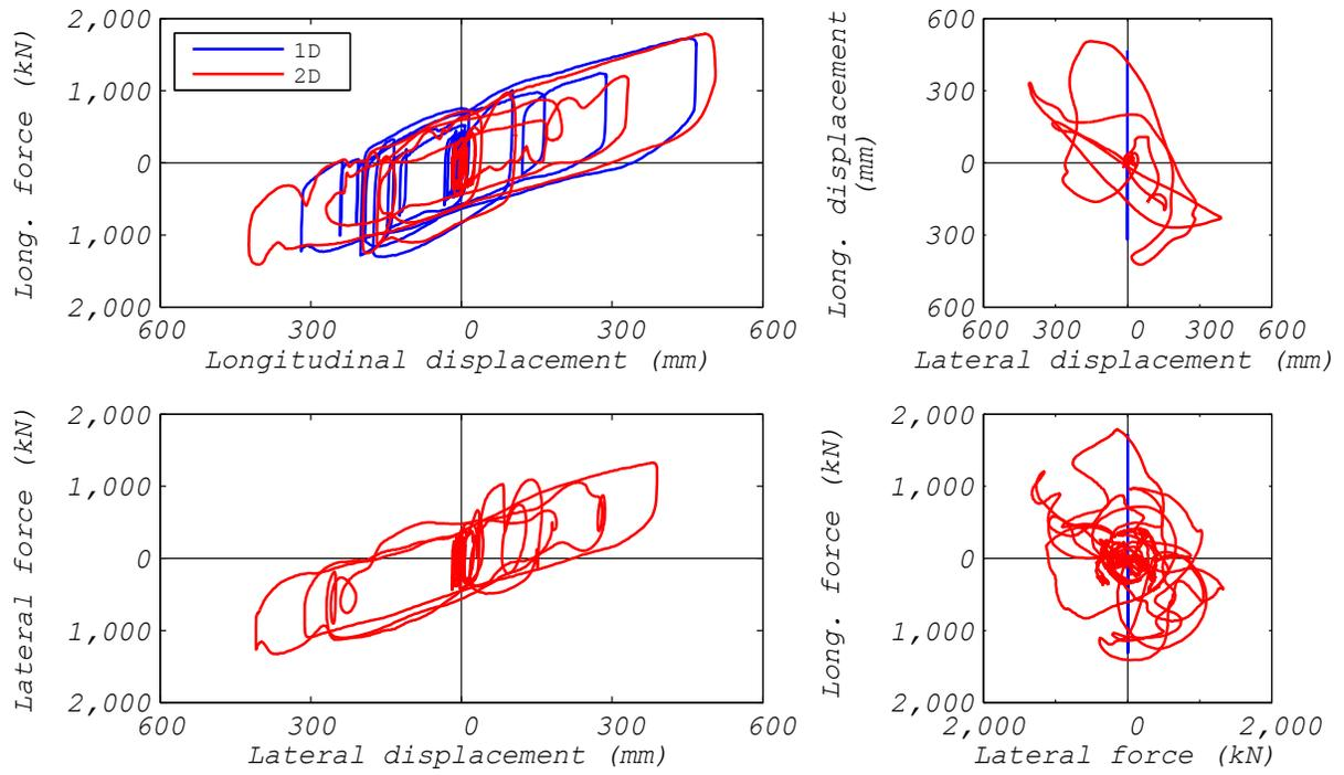
**Figure 3.42** LPRB bearing: comparison of bearing responses to ground motion NRC15 (1D and 2D analyses).
