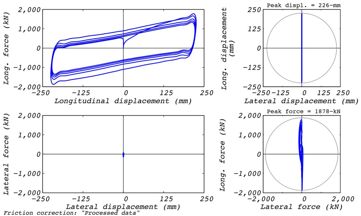
Figure B.28-2 Test run no. 71 hysteresis: Longitudinal (224 mm amplitude, 8,663 kN axial load, and 373 mm/s velocity).
