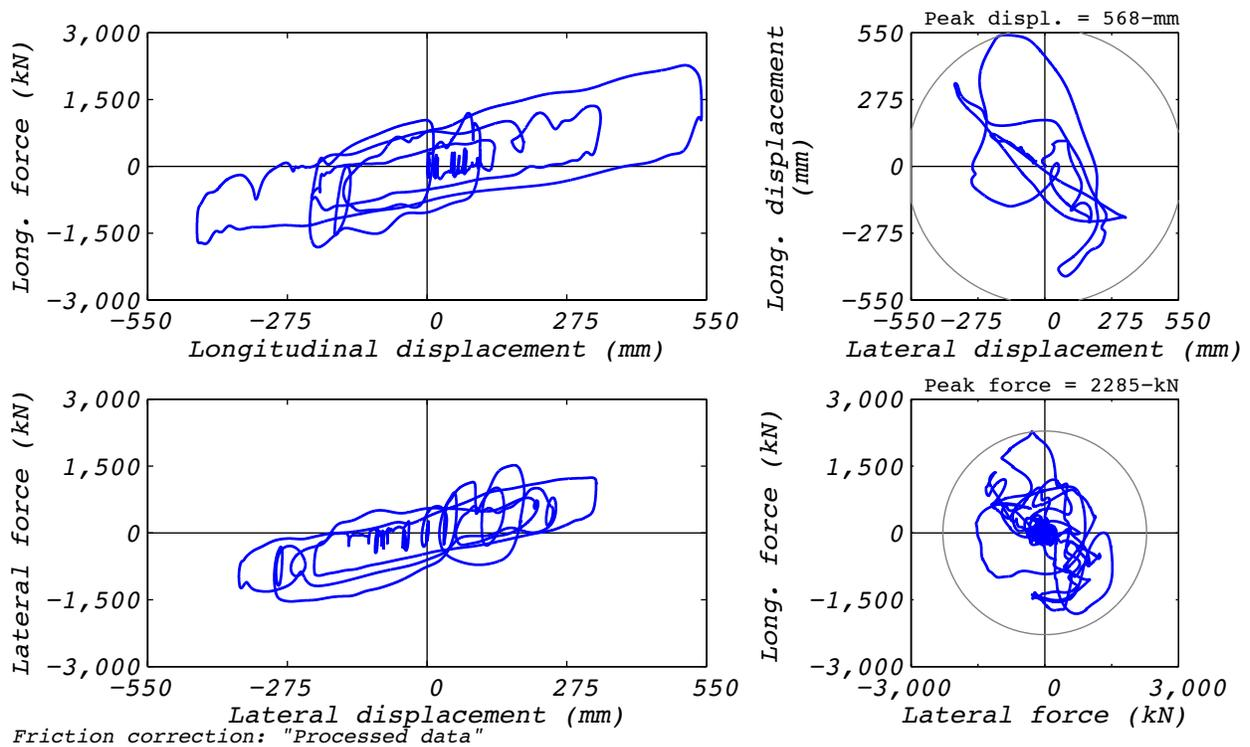
Figure B.35-2 Test run no. 87 hysteresis: Longitudinal (444 mm amplitude, 8,663 kN axial load, and 485 mm/s velocity).
