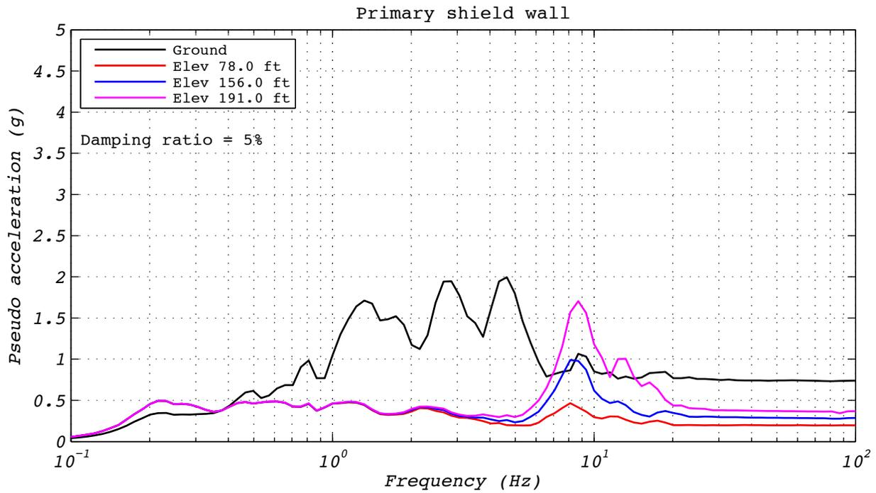
**Figure A.13-4 Hybrid test floor spectra for run 47: NRC15, 1D with experimental bearing representing all bearings.**
