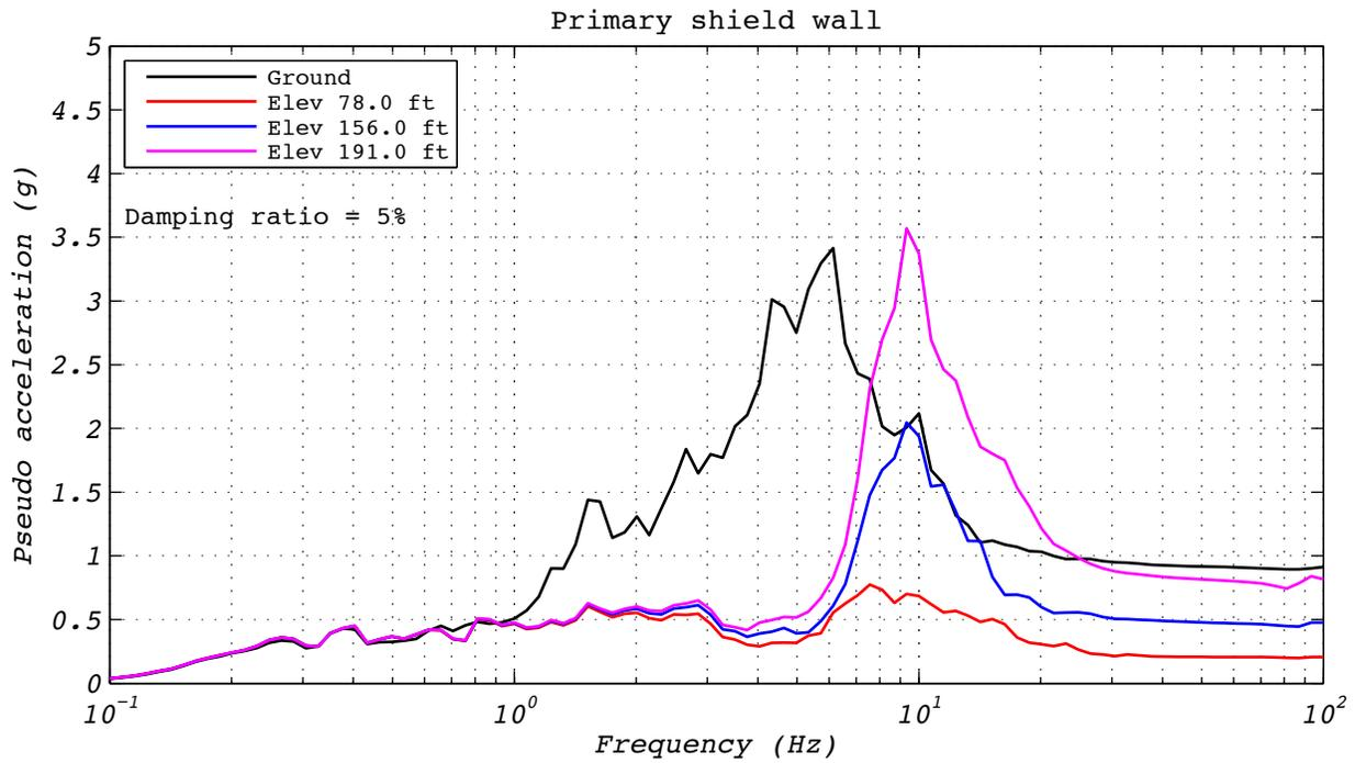
**Figure C.15-4 Hybrid test floor spectra for run 51: NRC2, 3D with 5 groups of bearings and the experimental bearing representing the no. 3 corner group.**
