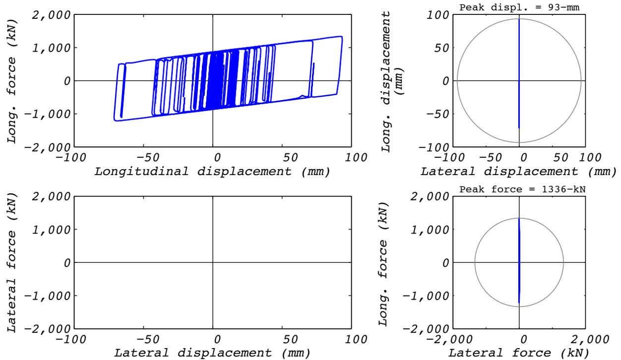
Figure C.17-1 Analytical bearing response for run 52A: NRC2, 1D with a single analytical bearing.
