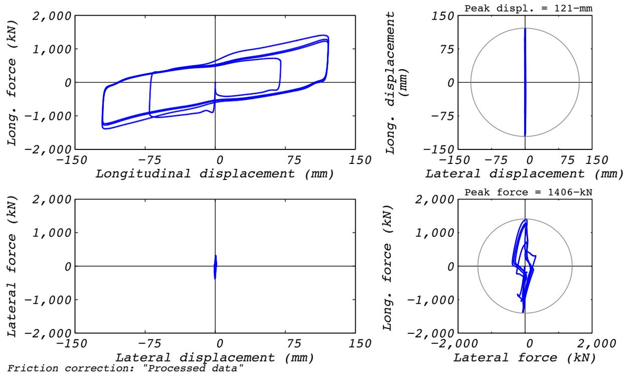
Figure D.24-2 Test run no. 30 hysteresis: Longitudinal (120 mm amplitude, 8,663 kN axial load, and 410 mm/s velocity).
