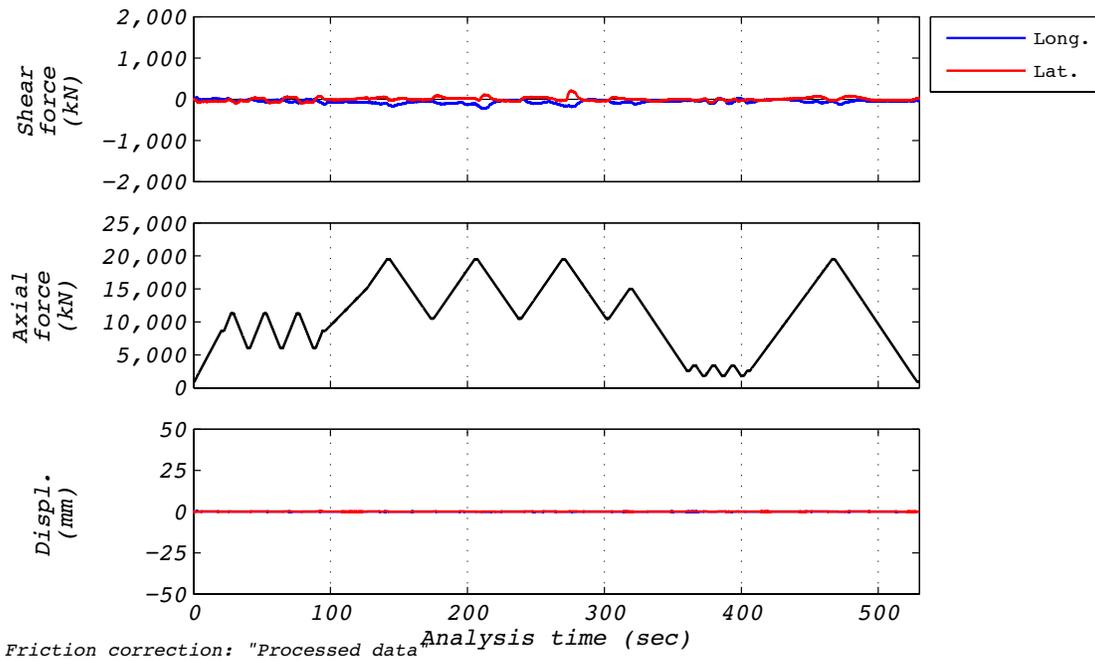
Figure D.2-1 Test run no. 2 time history: Axial (0 mm displacement and varying axial load).
