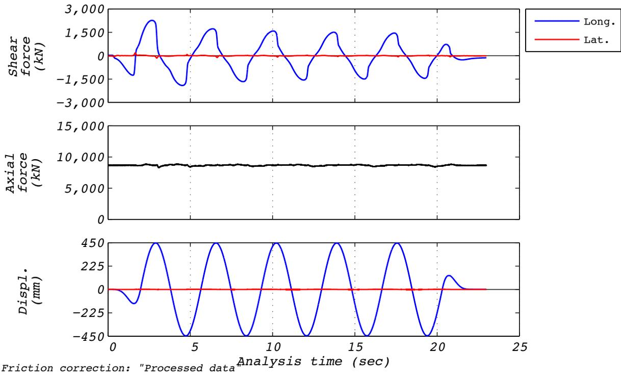
**Figure A.28-2 Time history responses for real-time displacement history from hybrid test run 84: NRC15, 3D with 5 groups of bearings and the experimental bearing representing the center group.**
