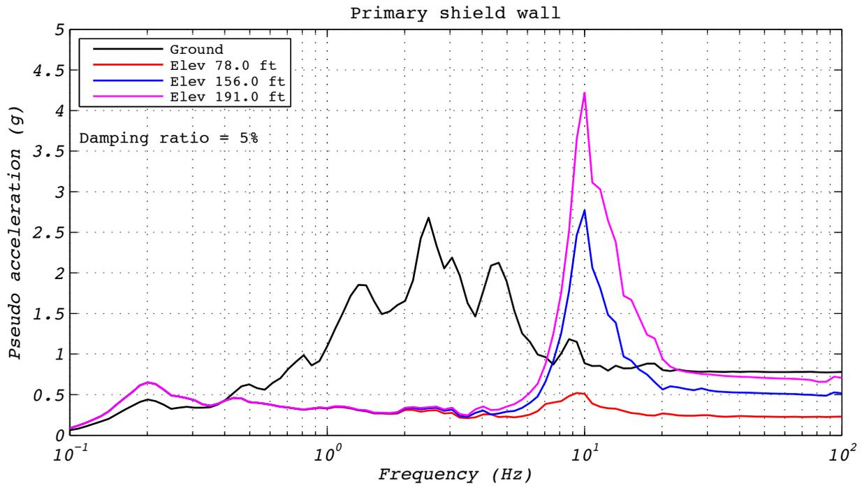
**Figure A.30-4 Hybrid test floor spectra for run 89: NRC15, 3D with 5 groups of bearings and the experimental bearing representing the no. 3 corner group.**
