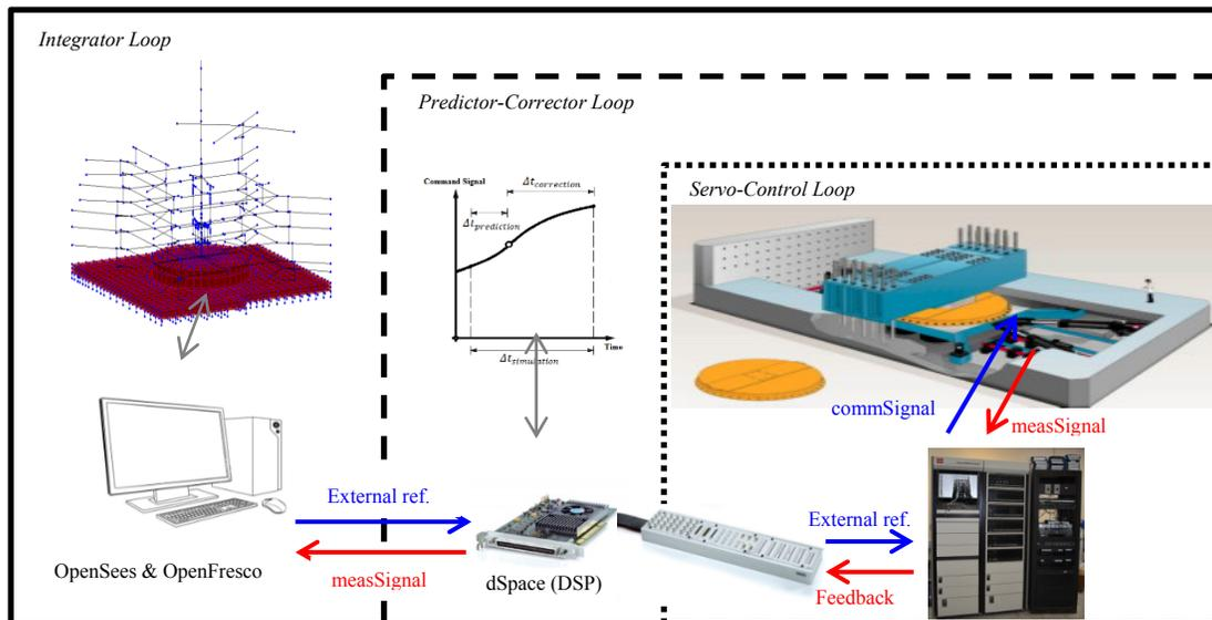
Figure 3.4 dSpace experimental control.
