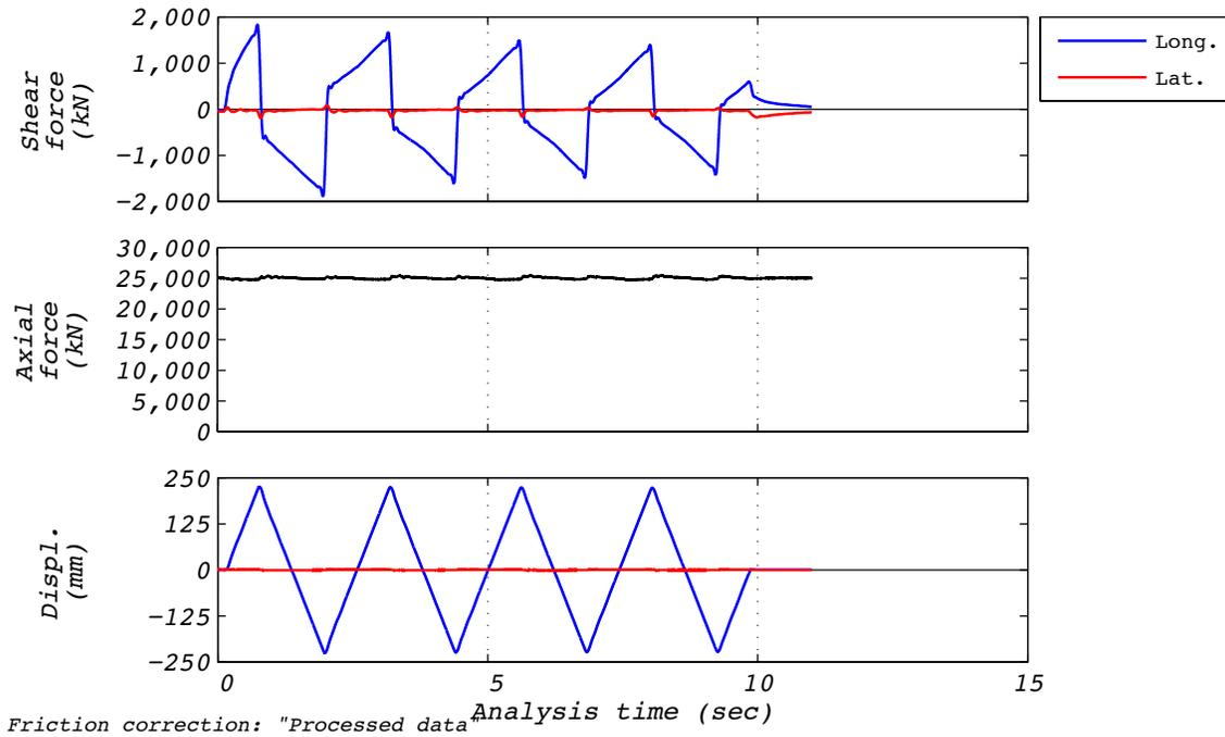
Figure B.32-1 Test run no. 75 time history: Longitudinal (224 mm amplitude, 25,002 kN axial load, and 373 mm/s velocity).
