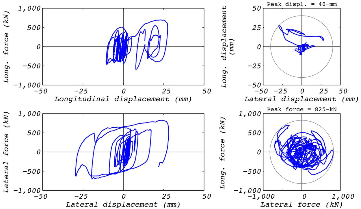
**Figure A.18-2 Hybrid test bearing response for run 60: EUR5, 2D with experimental bearing representing one of 527 bearings.**
