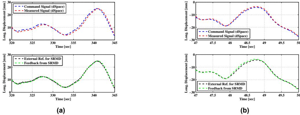
Figure 3.11 Tracking signal for delay: (a) no feed-forward and (b) with feed-forward.
