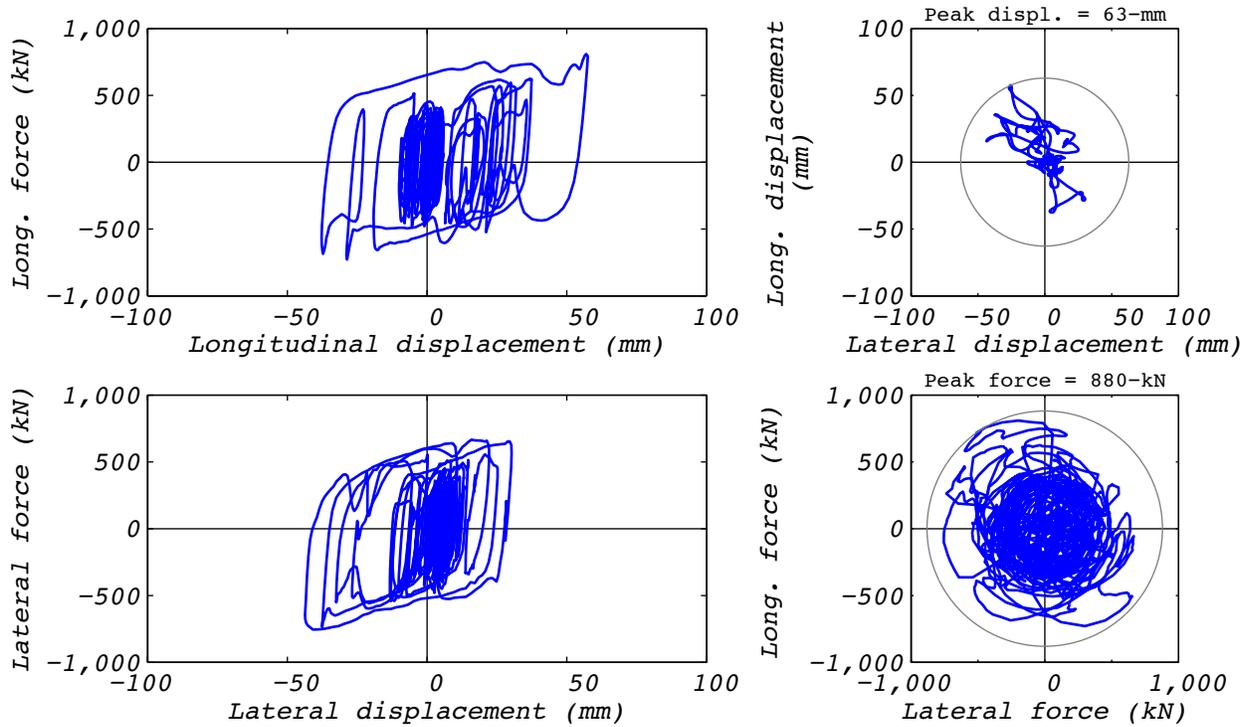
**Figure A.25-2 Hybrid test bearing response for run 83: EUR5, 3D with 5 groups and the experimental bearing representing the no. 3 corner group.**
