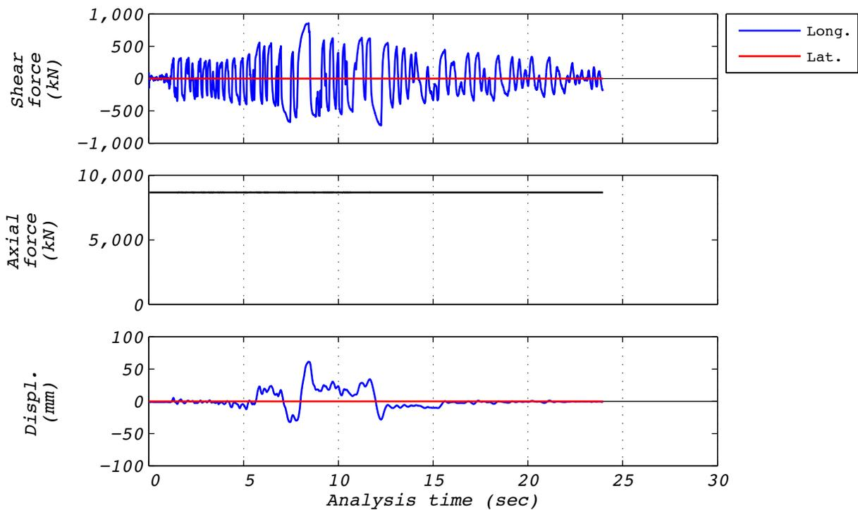
**Figure A.8-3 Hybrid test time history responses for run 44: EUR5, 1D with experimental bearing representing all bearings.**
