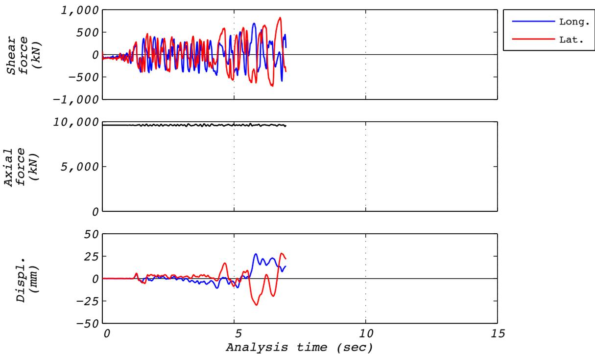
**Figure A.18-3 Hybrid test time history responses for run 60: EUR5, 2D with experimental bearing representing one of 527 bearings.**
