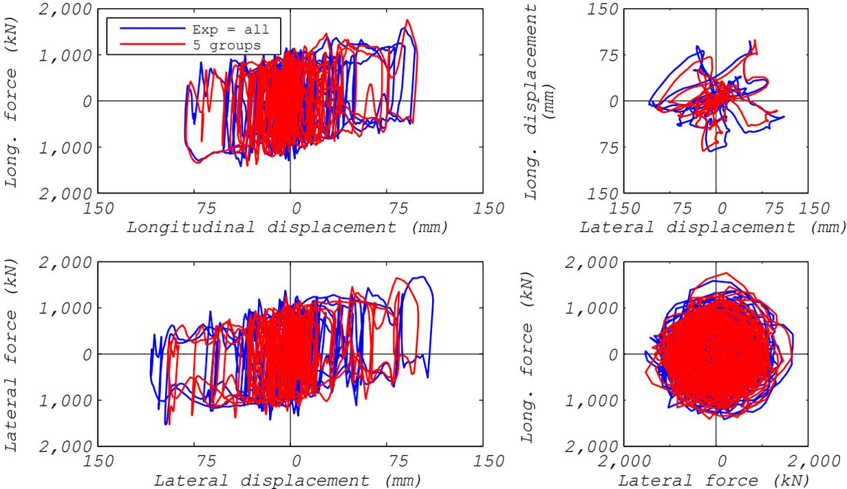
**Figure 3.70 EQS bearing: comparison of bearing responses to bearing layout discretization (ground motion NRC2, 2D analysis).**
