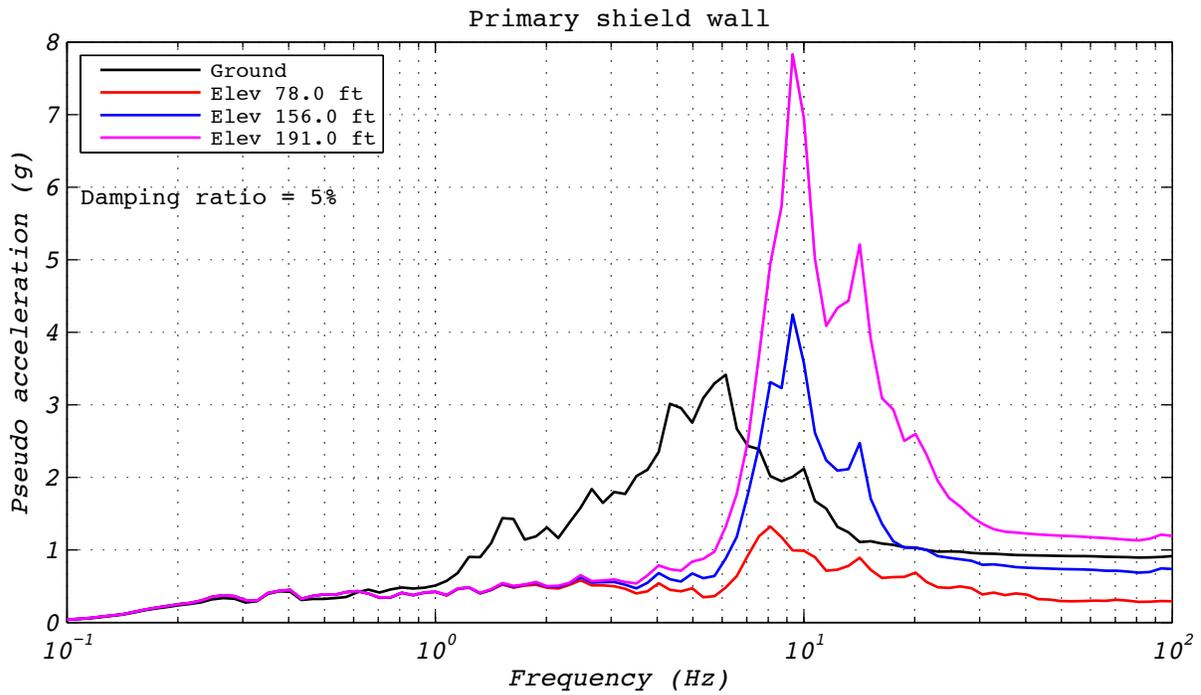
**Figure C.20-4 Hybrid test floor spectra for run 54: NRC2, 2D with experimental bearing representing all bearings.**
