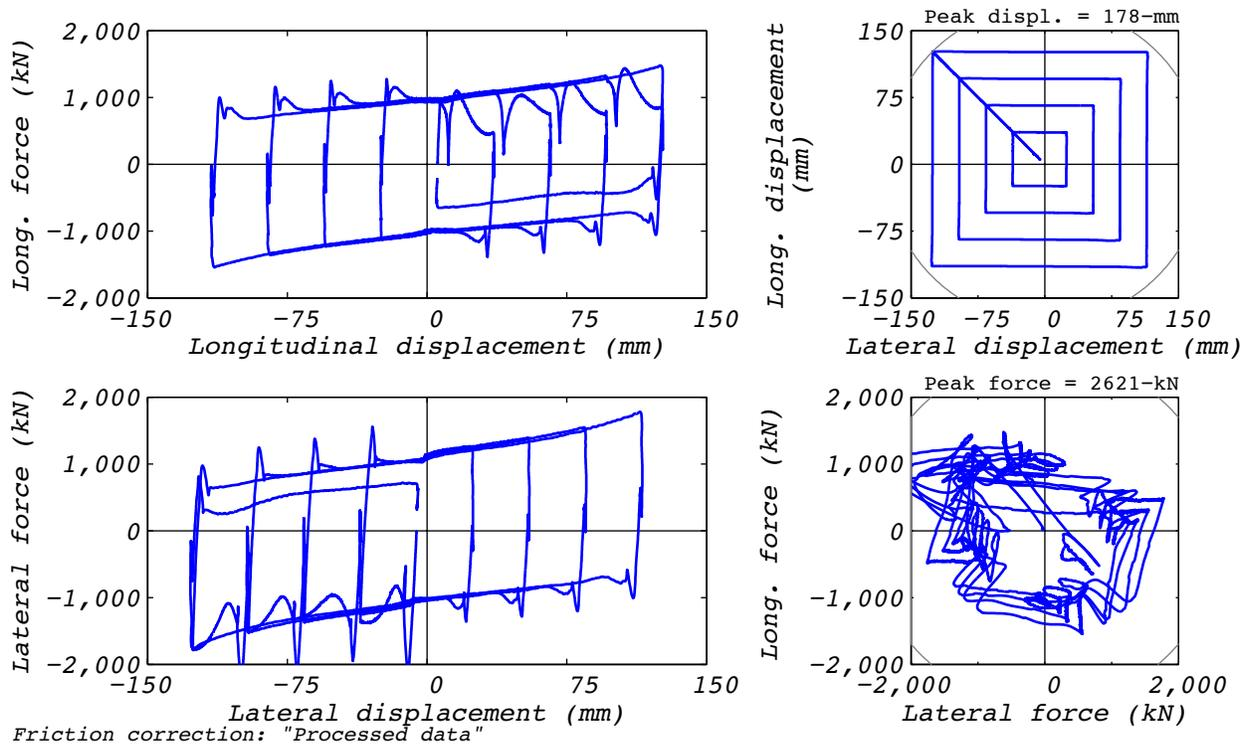
Figure D.22-2 Test run no. 28 hysteresis: Square orbit (Varying amplitude, 8,663 kN axial load, and varying velocity).
