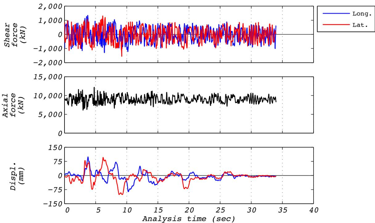
Figure C.12-3 Hybrid test time history responses for run 48: NRC2, 3D with 5 groups and the experimental bearing representing the no. 3 corner group.
