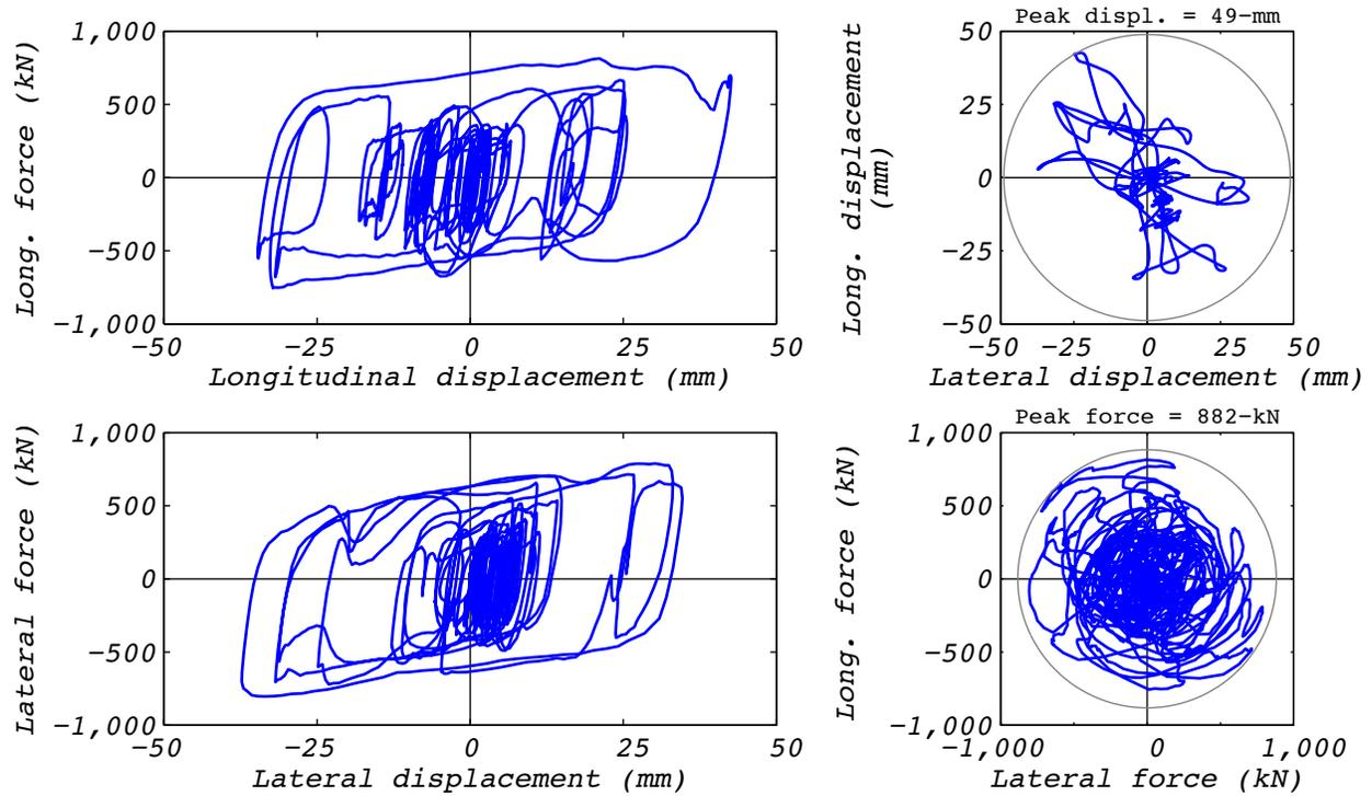
**Figure A.3-2 Hybrid test bearing response for run 26: EUR5, 2D with experimental bearing representing all bearings.**
