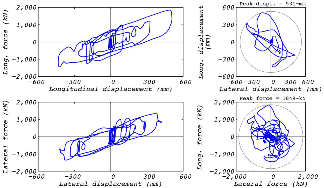
**Figure A.12-2 Hybrid test bearing response for run 46: NRC15, 2D with experimental bearing representing all bearings.**
