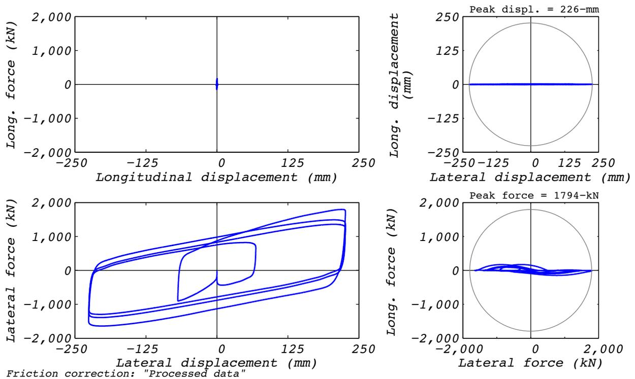
Figure B.10-2 Test run no. 23 hysteresis: Transverse (224 mm amplitude, 8,663 kN axial load, and 586 mm/s velocity).
