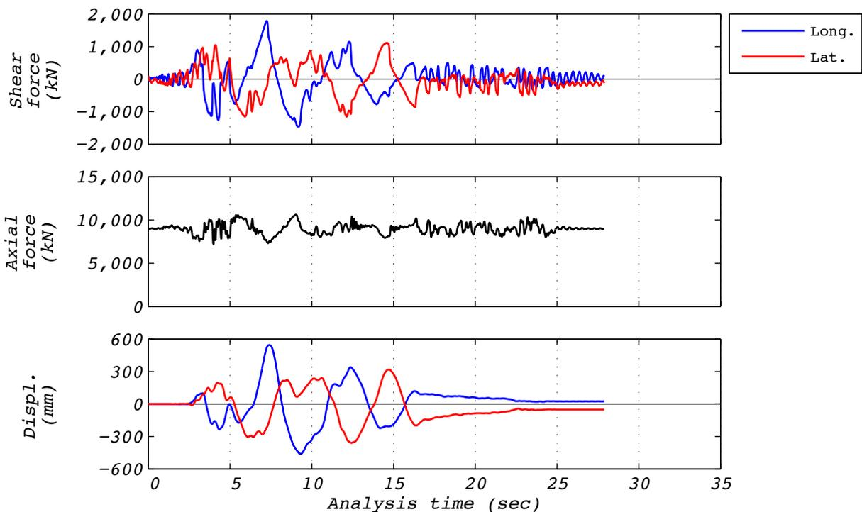
**Figure A.27-3 Hybrid test time history responses for run 85: NRC15, 3D with 5 groups and the experimental bearing representing the no. 3 corner group.**
