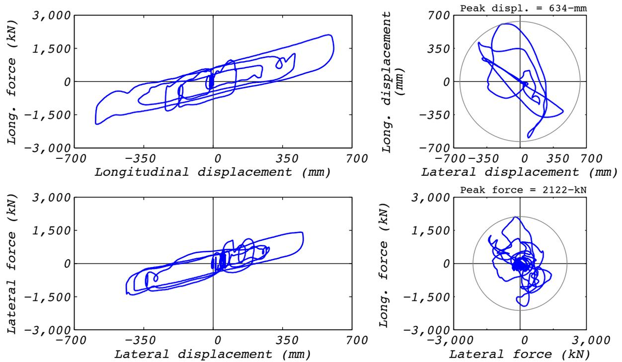
Figure A.20-2 Hybrid test bearing response for run 63: NRC15, 2D with five groups of bearings.
