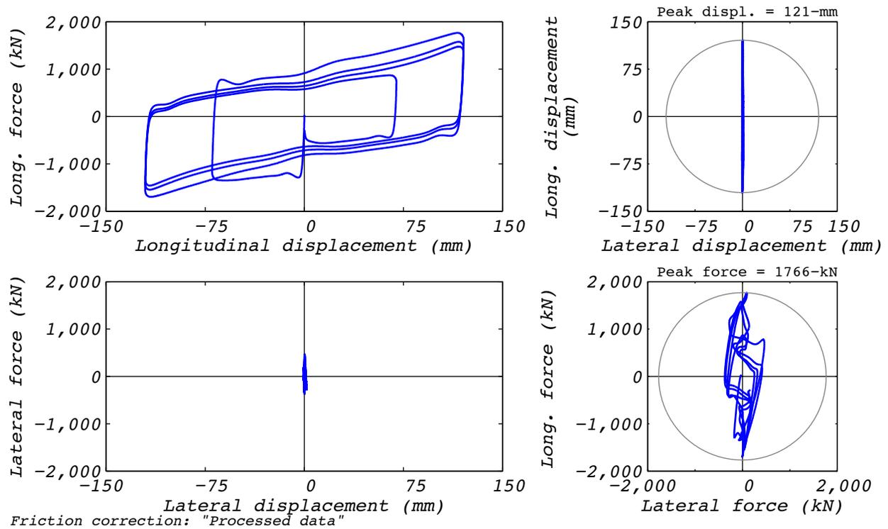
Figure D.1-2 Test run no. 1 hysteresis: Longitudinal (120 mm amplitude, 8,663 kN axial load, and 410 mm/s velocity).
