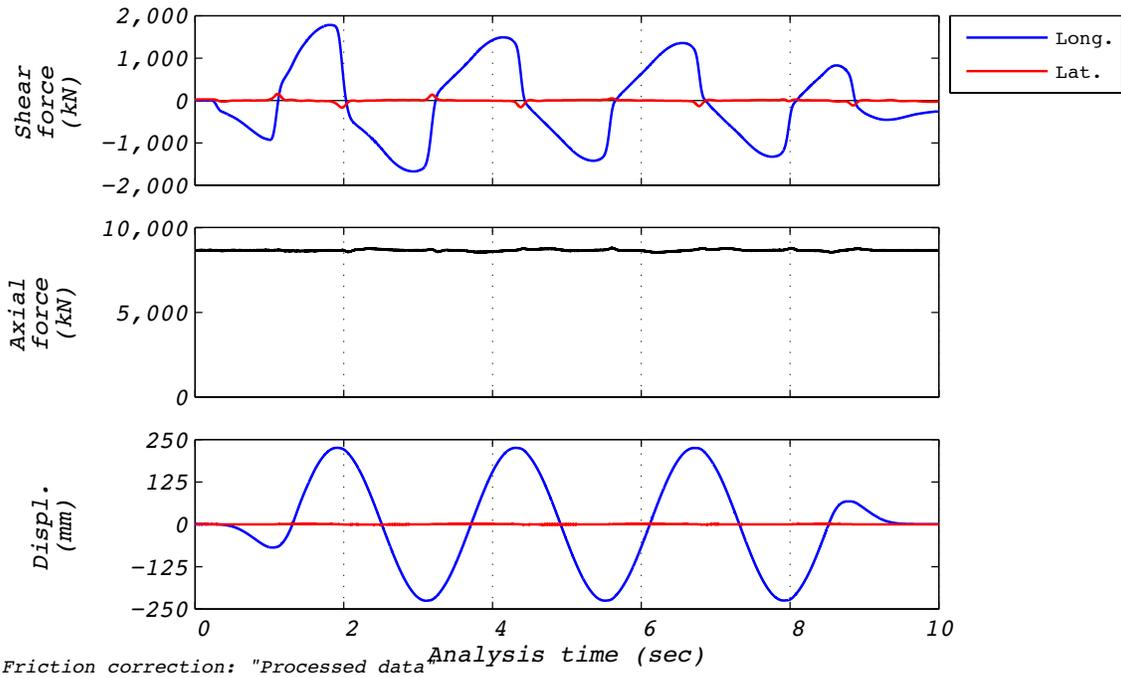
Figure B.2-1 Test run no. 9 time history: Longitudinal (224 mm amplitude, 8,663 kN axial load, and 586 mm/s velocity).
