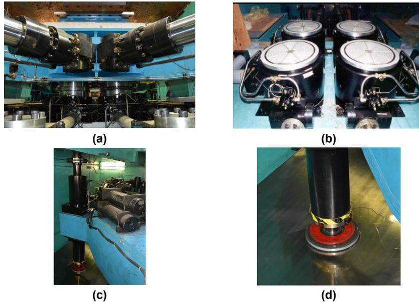
**Figure 3.14** Machine contact surfaces: (a) and (b) are the vertical actuators; (c) and (d) are the outriggers.
