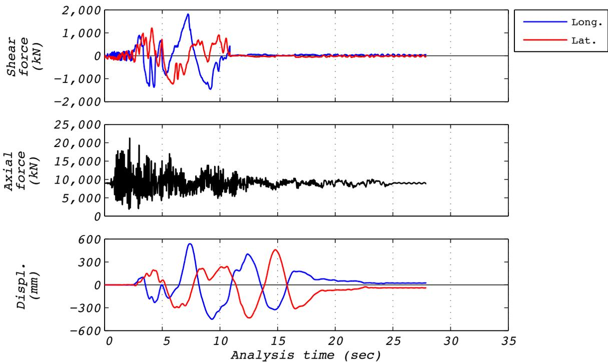
**Figure A.29-3 Hybrid test time history responses for run 88: NRC15, 3D with 5 groups and the experimental bearing representing the no. 3 corner group.**
