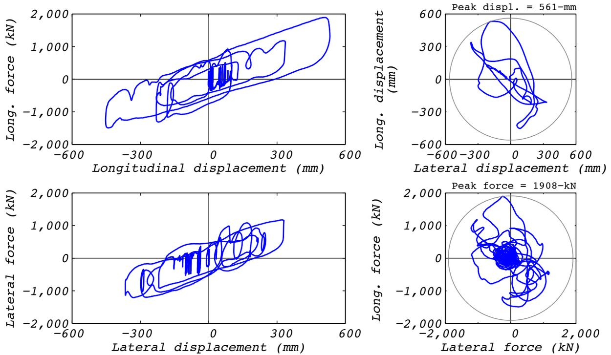
**Figure A.26-2 Hybrid test bearing response for run 84: NRC15, 3D with 5 groups of bearings and the experimental bearing representing the center group.**
