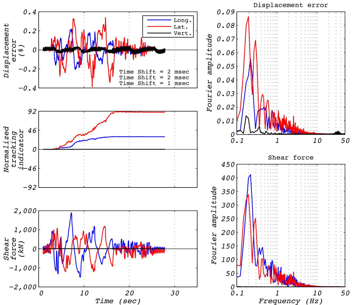
Figure A.26-1 Hybrid test performance metrics for run 84: NRC15, 3D with 5 groups of bearings and the experimental bearing representing the center group.
