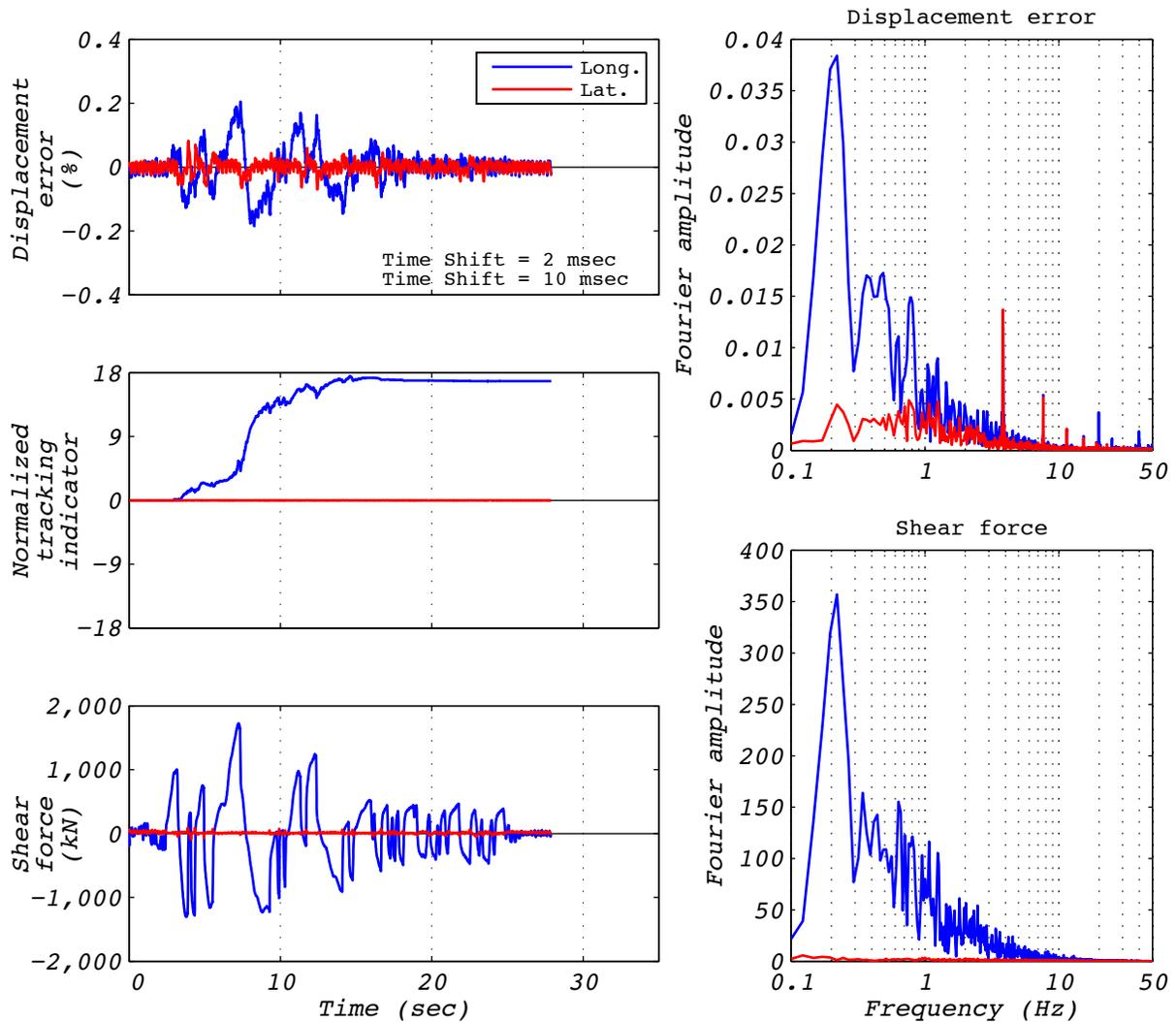
Figure A.13-1 Hybrid test performance metrics for run 47: NRC15, 1D with experimental bearing representing all bearings.
