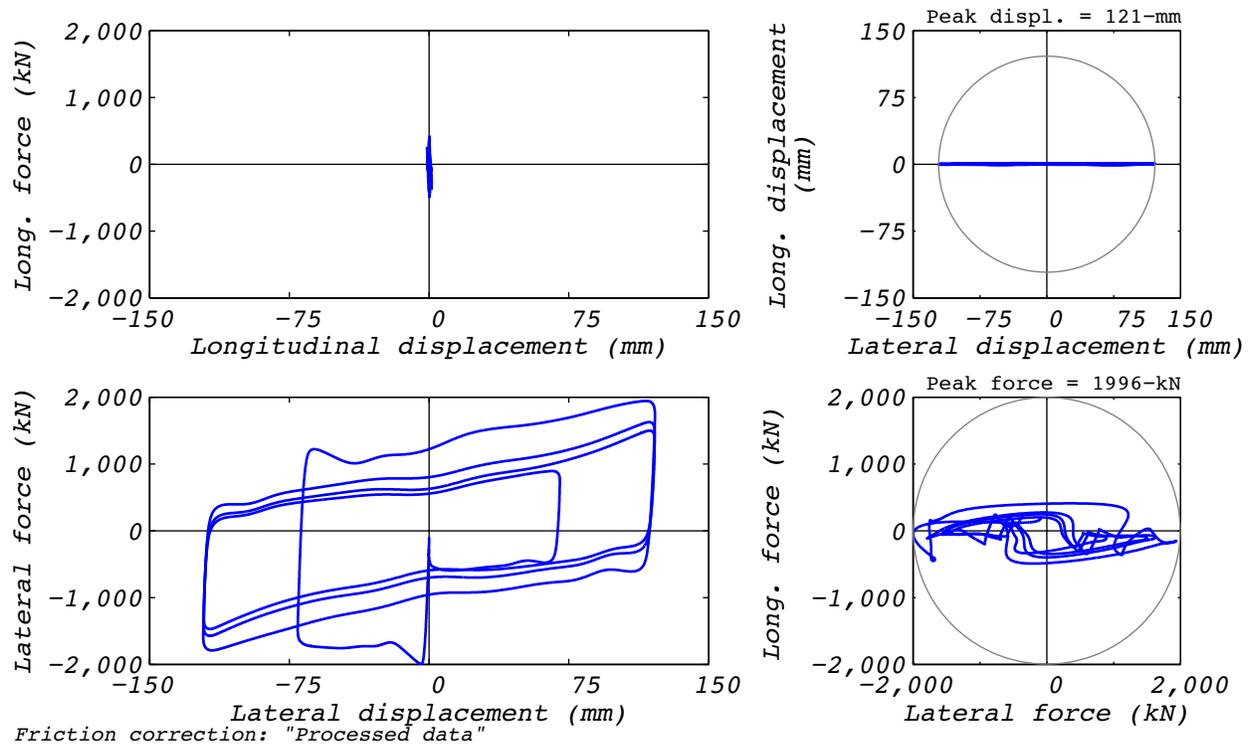
Figure D.10-2 Test run no. 10 hysteresis: Transverse (120 mm amplitude, 8,663 kN axial load, and 410 mm/s velocity).
