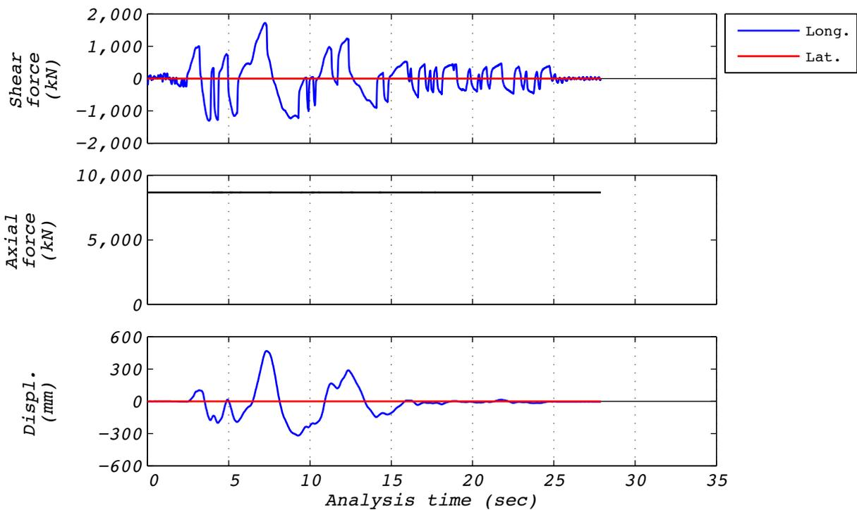
**Figure A.13-3 Hybrid test time history responses for run 47: NRC15, 1D with experimental bearing representing all bearings.**
