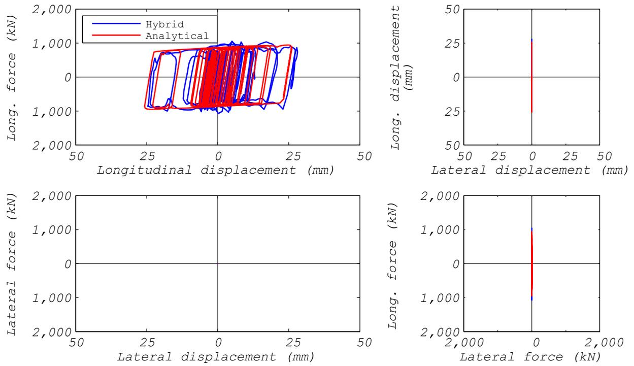
**Figure 3.76 EQS bearing: comparison of hybrid simulation and analytical estimation responses (ground motion EUR5, 1D analysis).**
