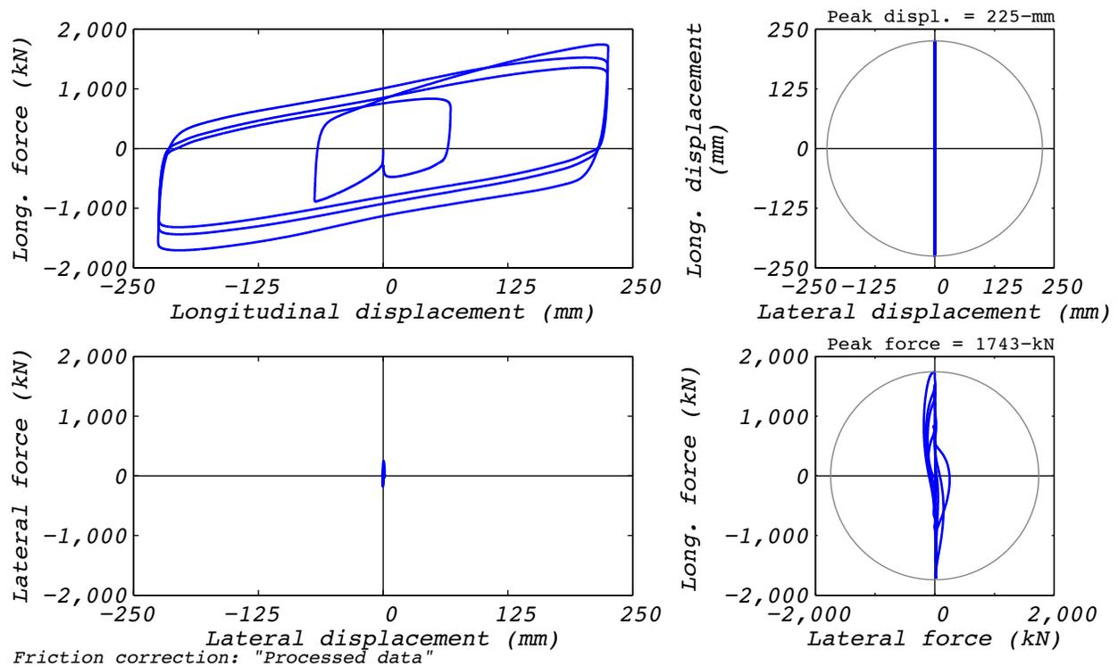
Figure B.16-2 Test run no. 54 hysteresis: Longitudinal (224 mm amplitude, 8,663 kN axial load, and 586 mm/s velocity).
