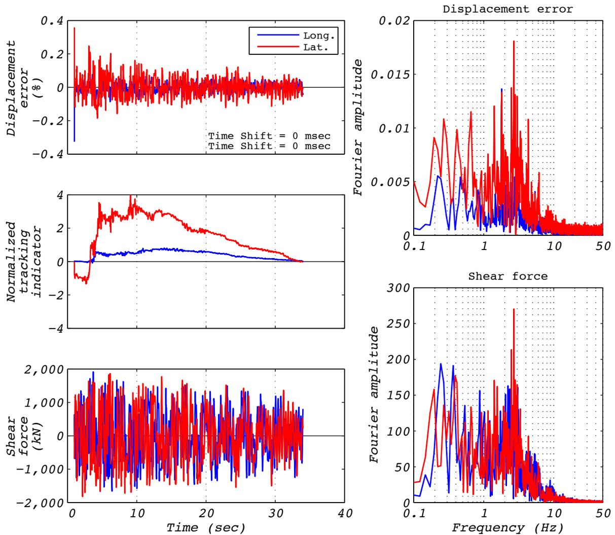
Figure C.5-1 Hybrid test performance metrics for run 21: NRC2, 2D with experimental bearing representing all bearings.
