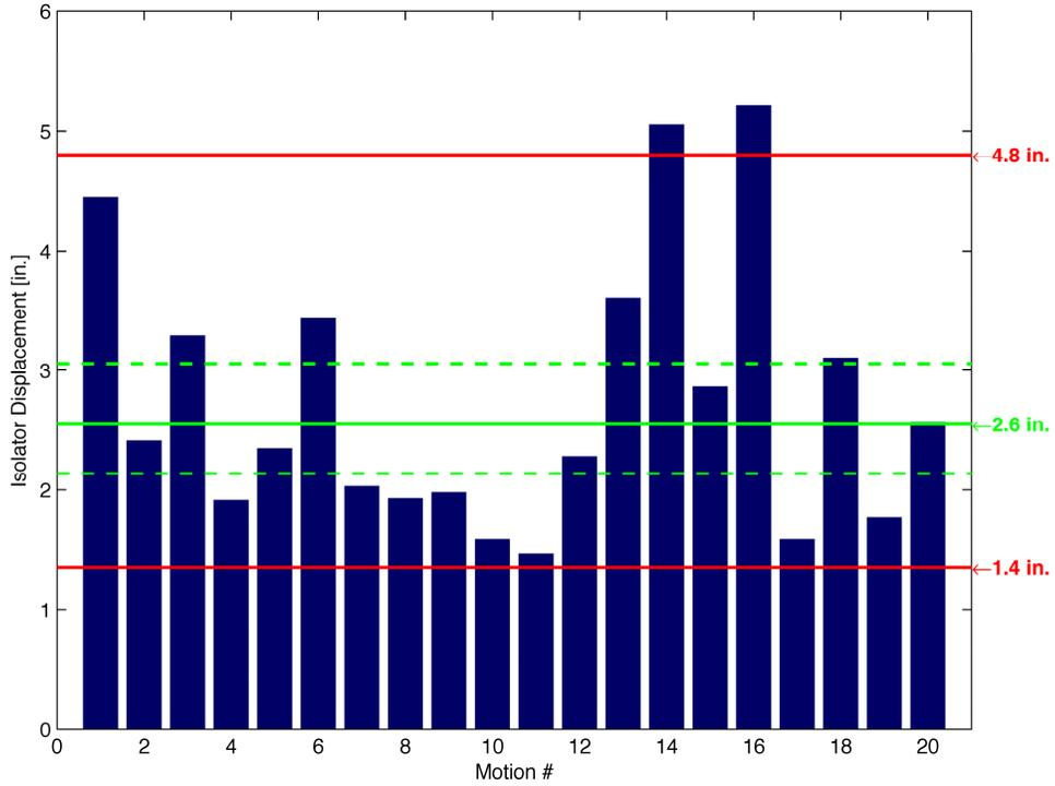
**Figure 3.32** Analytically determined peak lateral displacement demands for the EUR hazard level [2012] based on an FPSB isolator (green lines = median with 95% confidence interval, red lines = 5<sup>th</sup> and 95<sup>th</sup> percentile).
