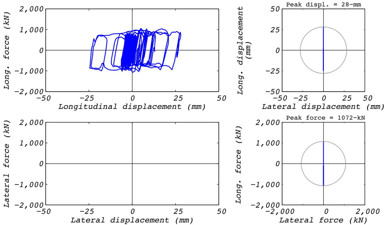
**Figure C.18-2 Hybrid test bearing response for run 53: EUR5, 1D with experimental bearing representing all bearings.**
