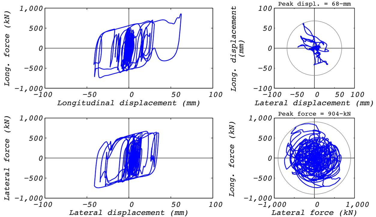
Figure A.11-1 Analytical bearing response for run 45A: EUR5, 2D with a single analytical bearing.
