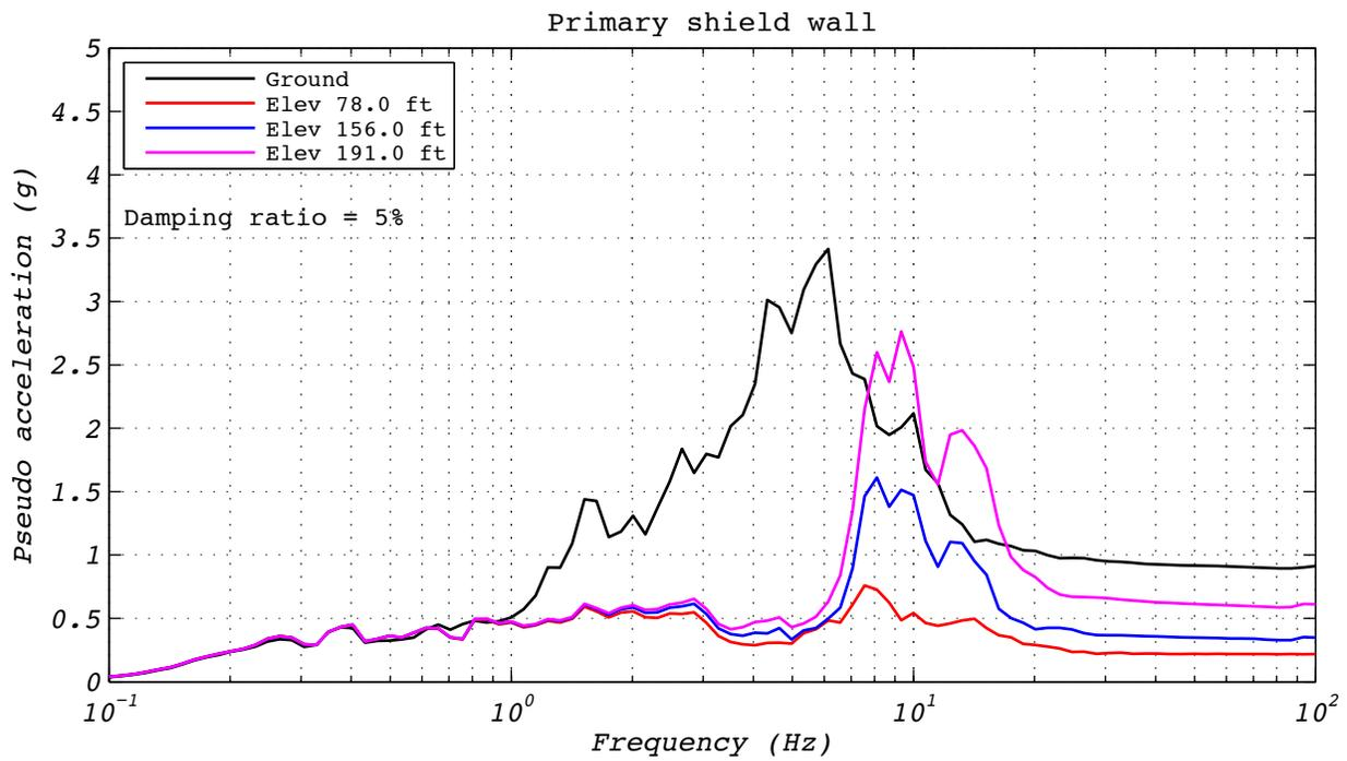
**Figure C.14-4 Hybrid test floor spectra for run 50: NRC2, 3D with 5 groups of bearings and the experimental bearing representing the no. 3 corner group.**
