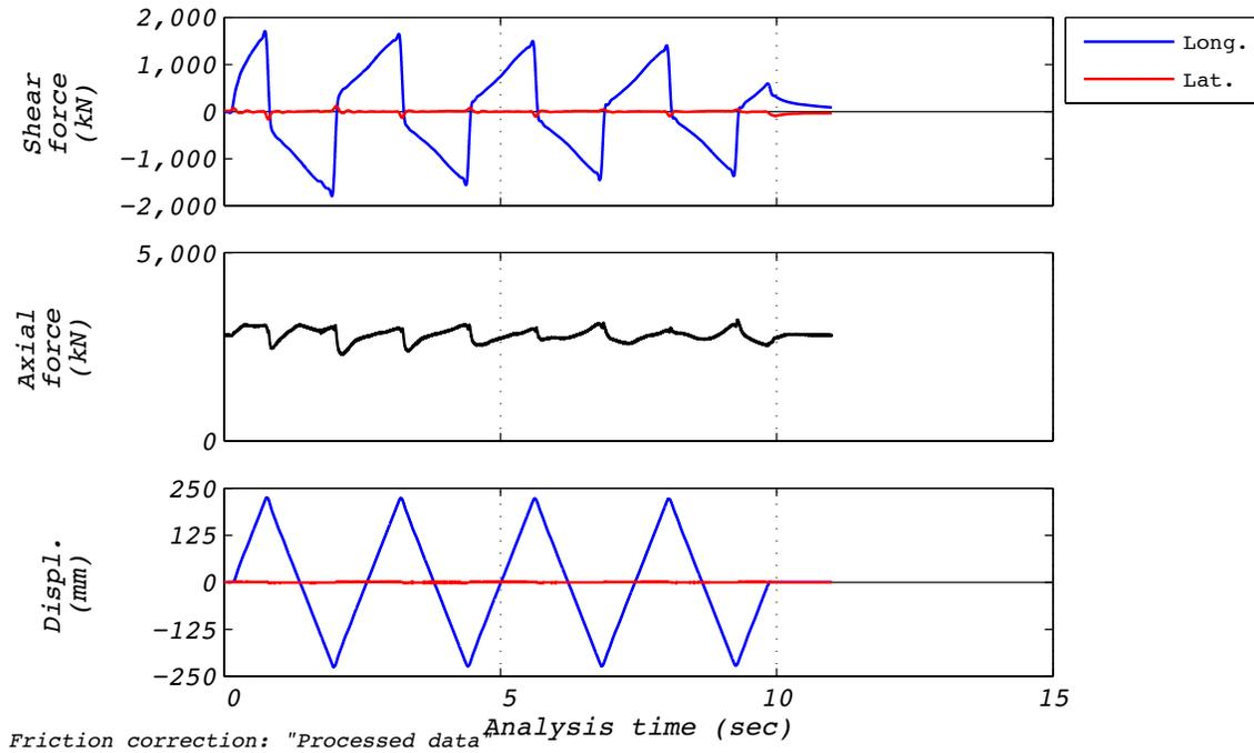
Figure B.33-1 Test run no. 76 time history: Longitudinal (224 mm amplitude, 2,807 kN axial load, and 373 mm/s velocity).
