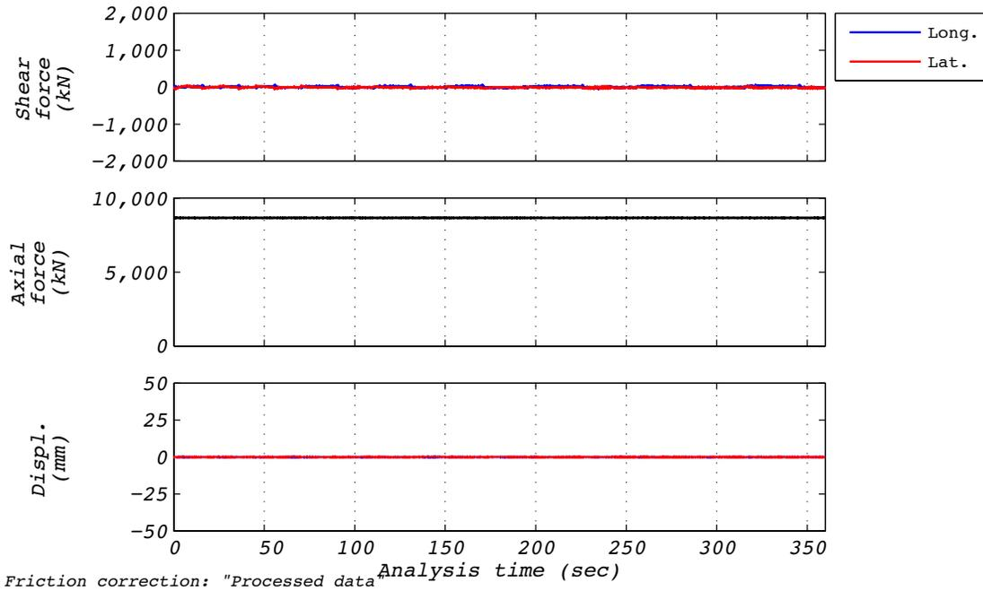
Figure D.8-1 Test run no. 8 time history: Twist (0 mm displacement and 8,663 kN axial load).
