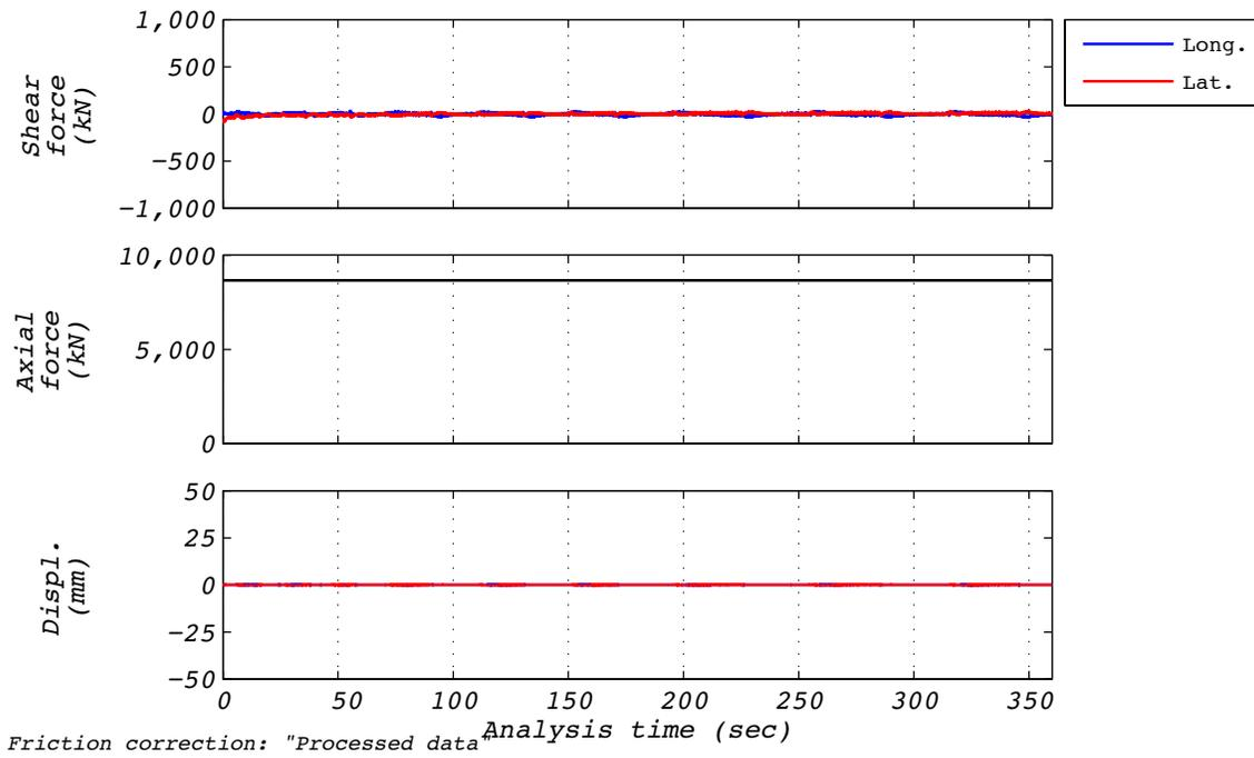
Figure B.15-1 Test run no. 53 time history: Twist (0 mm amplitude and 8,663 kN axial load).
