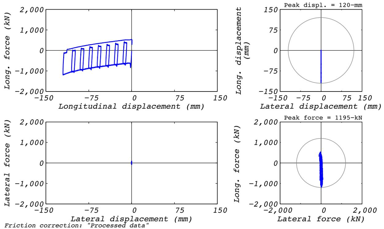
Figure D.28-2 Test run no. 34 hysteresis: Longitudinal (120 mm amplitude, 8,663 kN axial load).
