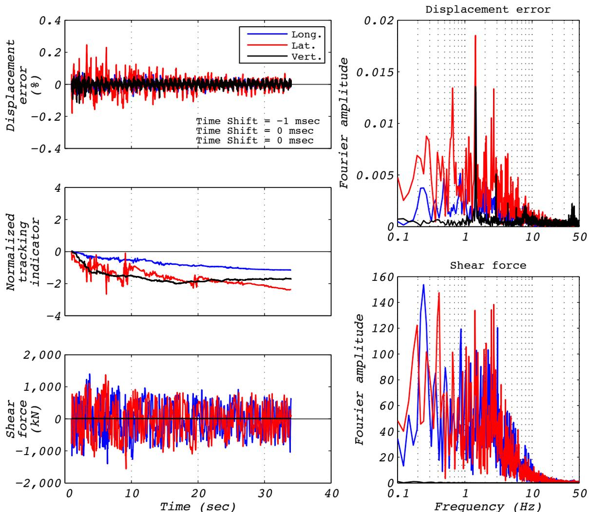
Figure C.14-1 Hybrid test performance metrics for run 50: NRC2, 3D with 5 groups of bearings and the experimental bearing representing the no. 3 corner group.
