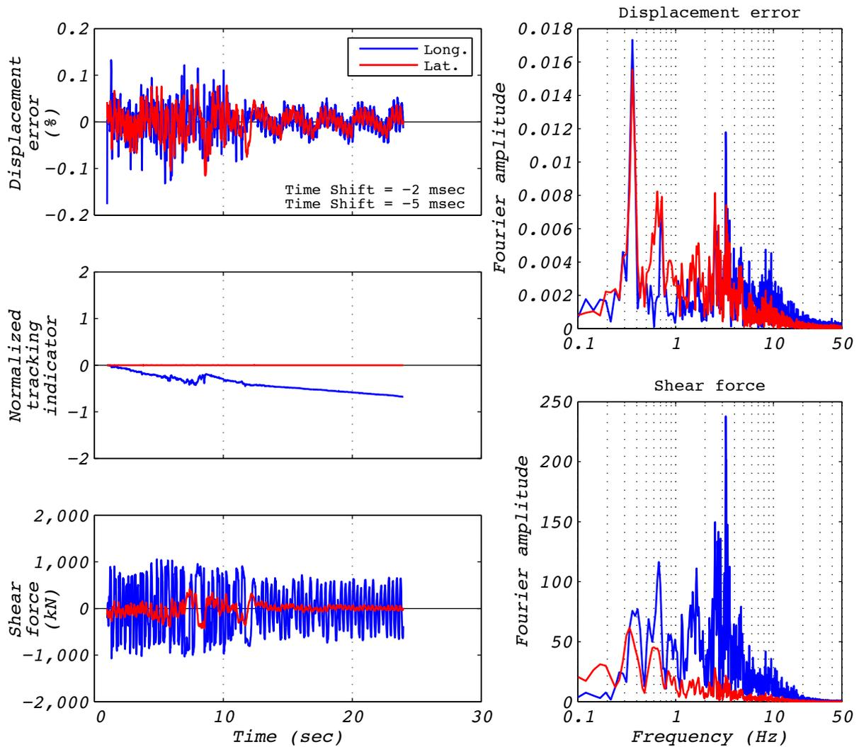
Figure C.18-1 Hybrid test performance metrics for run 53: EUR5, 1D with experimental bearing representing all bearings.
