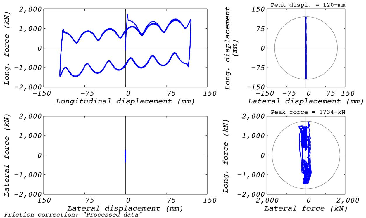
Figure D.21-2 Test run no. 27 hysteresis: Longitudinal (120 mm amplitude, varying axial load, and 410 mm/s velocity).
