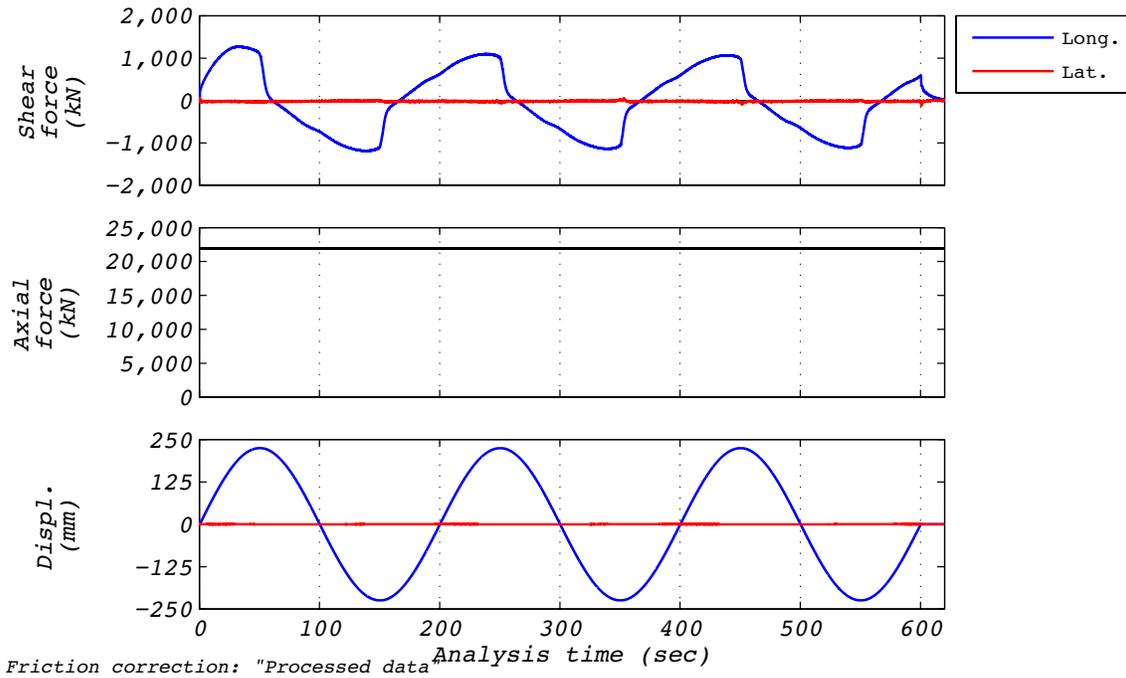
Figure B.26-1 Test run no. 69 time history: Longitudinal (224 mm amplitude, 21,927 kN axial load, and 7 mm/s velocity).
