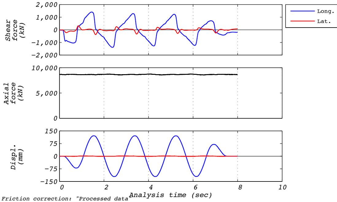
Figure D.24-1 Test run no. 30 time history: Longitudinal (120 mm amplitude, 8,663 kN axial load, and 410 mm/s velocity).
