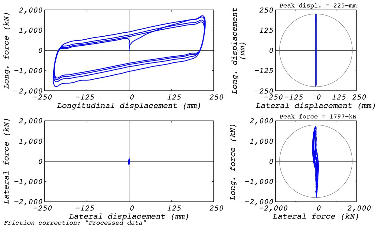
Figure B.33-2 Test run no. 76 hysteresis: Longitudinal (224 mm amplitude, 2,807 kN axial load, and 373 mm/s velocity).
