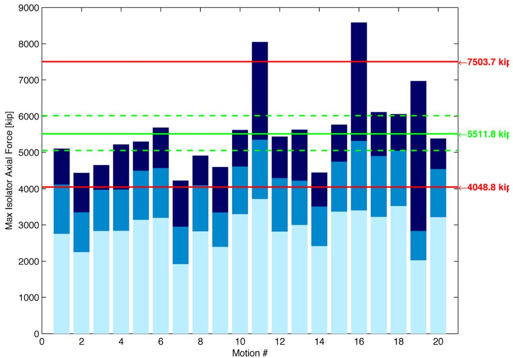
**Figure 3.35** Analytically determined peak axial force demands for the NRC hazard level [1973] based on an FPSB isolator (green lines = median with 95% confidence interval, red lines = 5<sup>th</sup> and 95<sup>th</sup> percentile).
