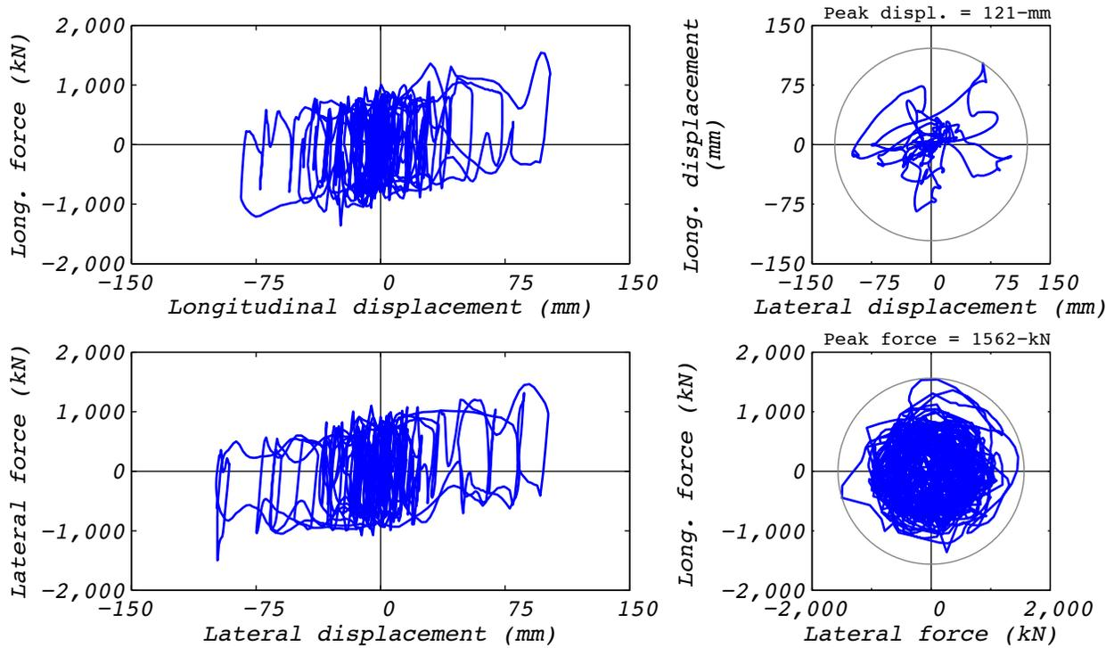
**Figure C.9-2 Hybrid test bearing response for run 44: NRC2, 3D with 5 groups of bearings and the experimental bearing representing the center group.**
