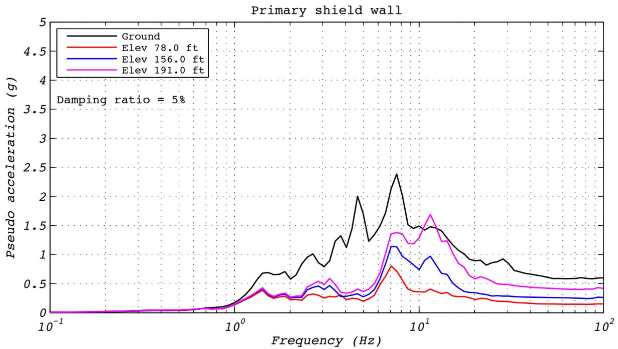
**Figure A.18-4 Hybrid test floor spectra for run 60: EUR5, 2D with experimental bearing representing one of 527 bearings.**
