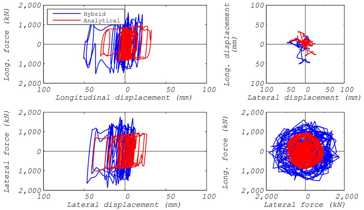
**Figure 3.80** EQS bearing: comparison of hybrid simulation and analytical estimation responses (ground motion EUR5, 2D analysis).
