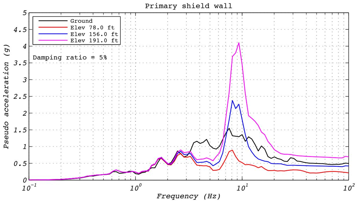
**Figure C.1-4 Hybrid test floor spectra for run 17: EUR5, 1D with experimental bearing representing all bearings.**
