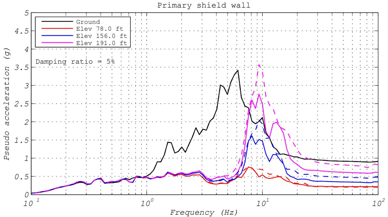
**Figure 3.67** EQS bearing: response spectra comparison of responses to a ground motion with and without vertical excitation (ground motion NRC2, 2D and 3D analyses).
