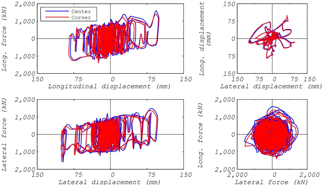
**Figure 3.68 EQS bearing: comparison of bearing responses depending on the location of the bearing (ground motion NRC2, 2D analysis).**
