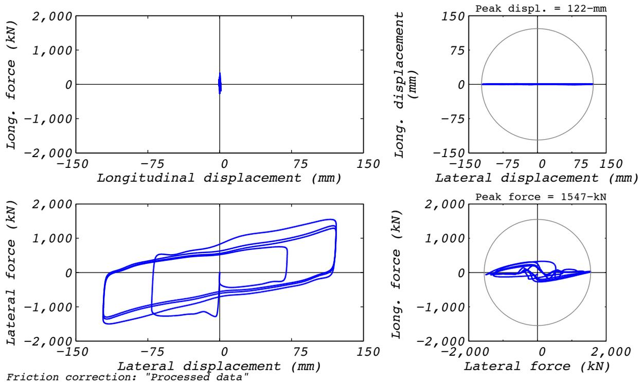
Figure D.26-2 Test run no. 32 hysteresis: Transverse (120 mm amplitude, 8,663 kN axial load, and 410 mm/s velocity).
