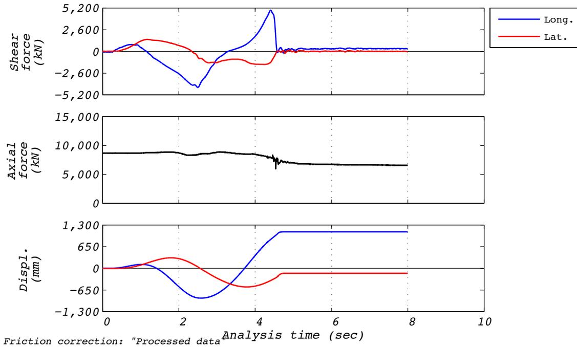
Figure B.23-1 Test run no. 66 time history: Bearing response during failure test (varying amplitude and 8,663 kN axial load).
