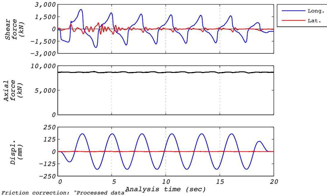
**Figure D.16-1 Test run no. 16 time history: Longitudinal (180 mm amplitude, 8,663 kN axial load, and 409 mm/s velocity).**
