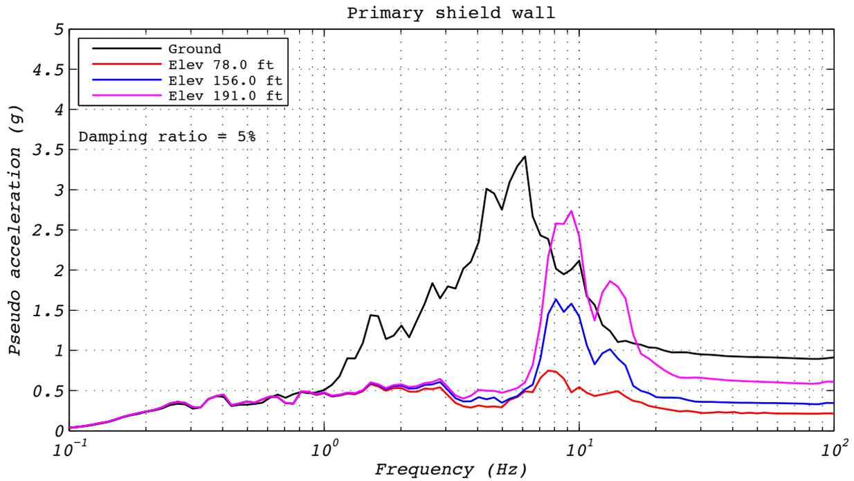
**Figure C.11-4 Hybrid test floor spectra for run 47: NRC2, 3D with 5 groups of bearings and the experimental bearing representing the center group.**
