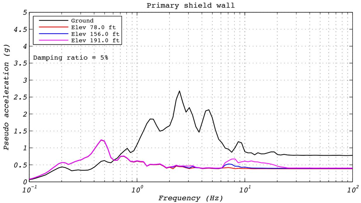
Figure A.19-4 Hybrid test floor spectra for run 61: NRC15, 2D with experimental bearing representing one of 527.
