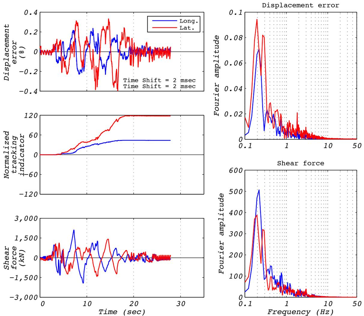
Figure A.20-1 Hybrid test performance metrics for run 63: NRC15, 2D with five groups of bearings.
