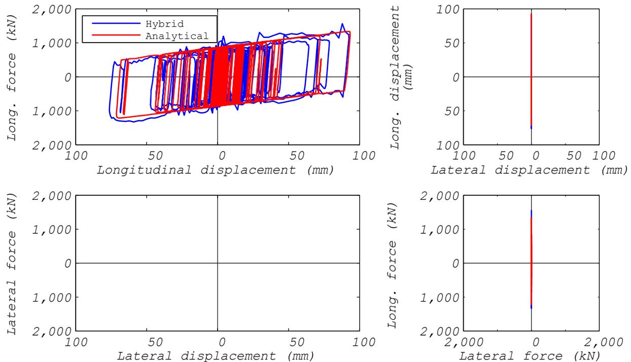
**Figure 3.78** EQS bearing: comparison of hybrid simulation and analytical estimation responses (ground motion NRC2, 1D analysis).
