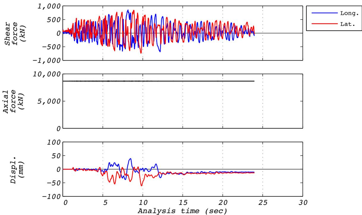
**Figure A.2-3 Hybrid test time history responses for run 25: EUR5, 2D with experimental bearing representing all bearings.**
