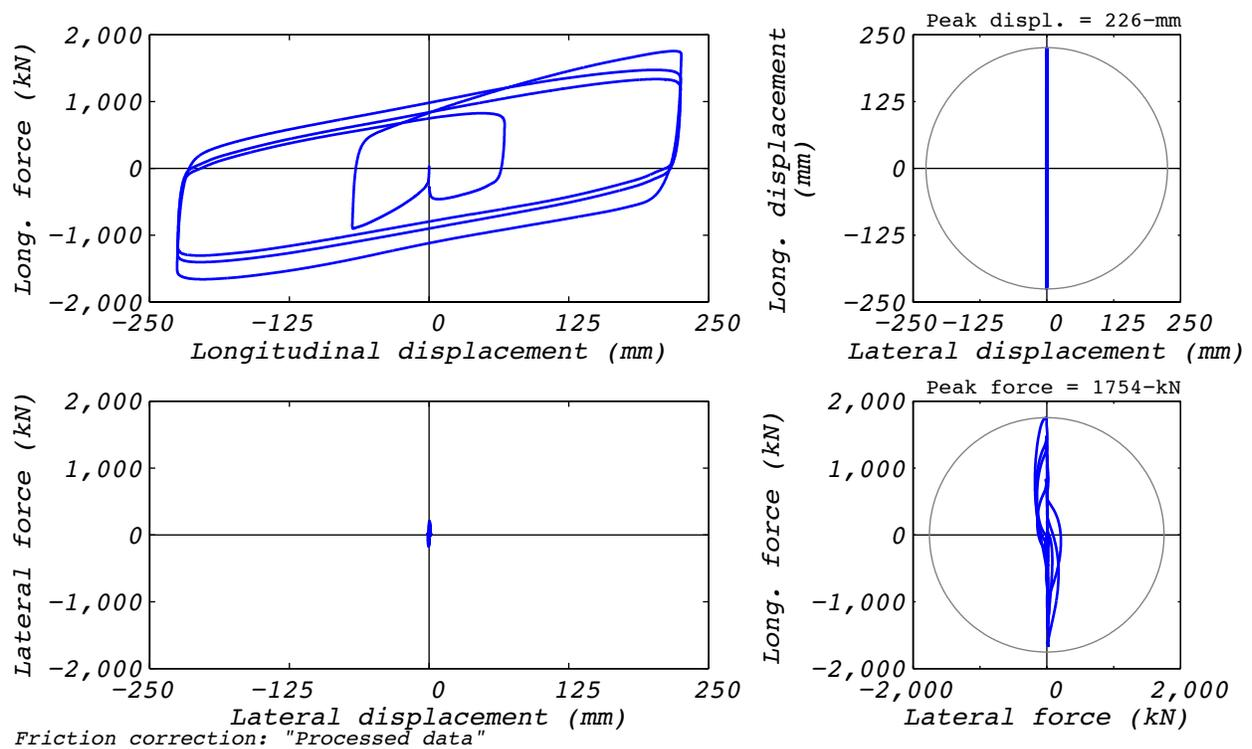
Figure B.11-2 Test run no. 35 hysteresis: Longitudinal (224 mm amplitude, 8,663 kN axial load, and 586 mm/s velocity).
