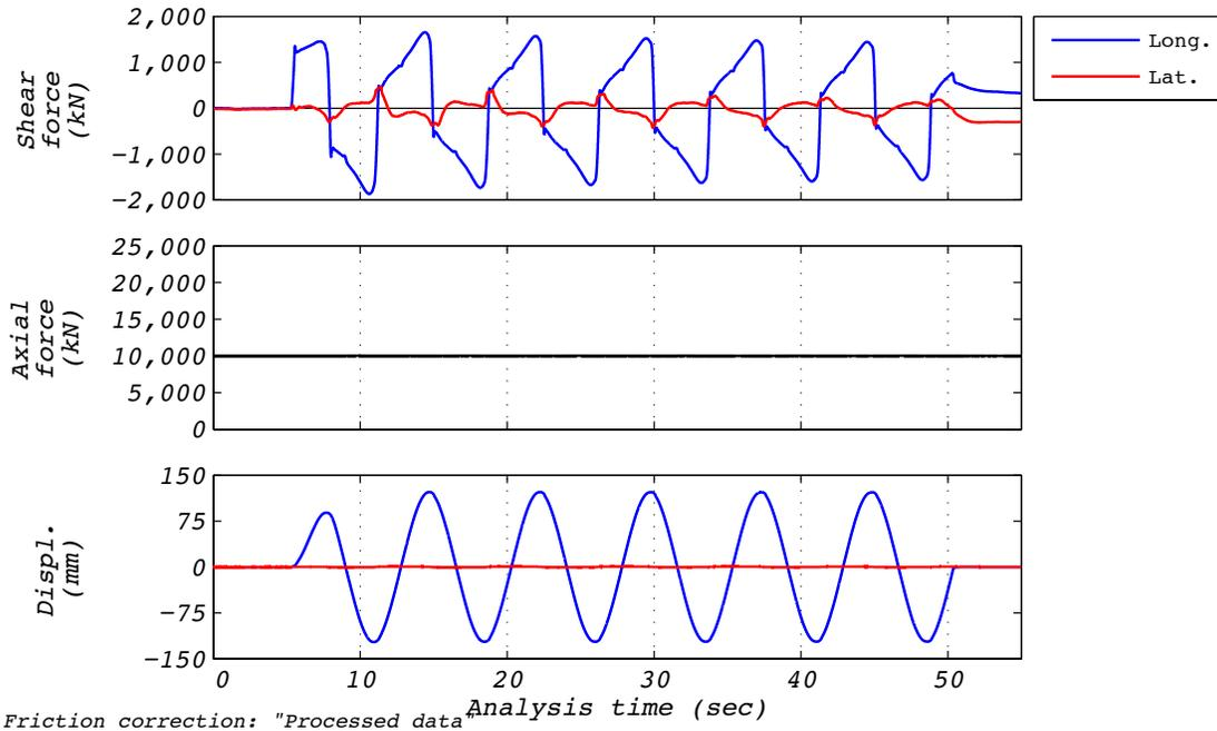
Figure D.9-1 Test run no. 9 time history: Longitudinal (120 mm amplitude, 10,000 kN axial load, and 410 mm/s velocity).
