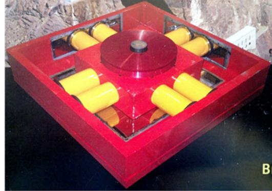
Figure 3.19 RJ-Watson EQS sliding isolator.
