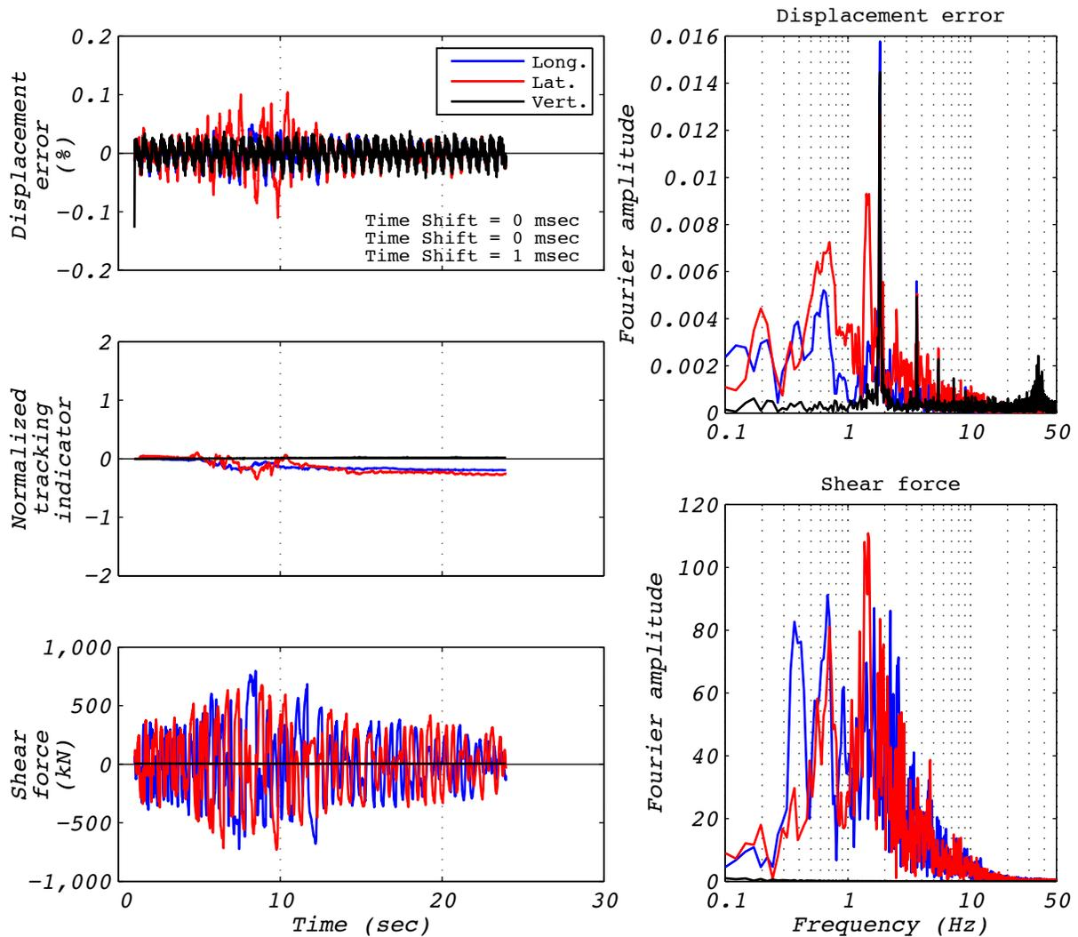
Figure A.24-1 Hybrid test performance metrics for run 82: EUR5, 3D with 5 groups of bearings and the experimental bearing representing the center group.
