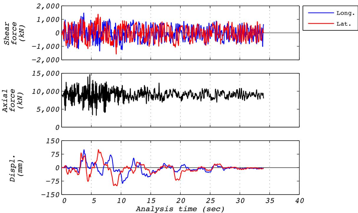
Figure C.15-3 Hybrid test time history responses for run 51: NRC2, 3D with 5 groups and the experimental bearing representing the no. 3 corner group.
