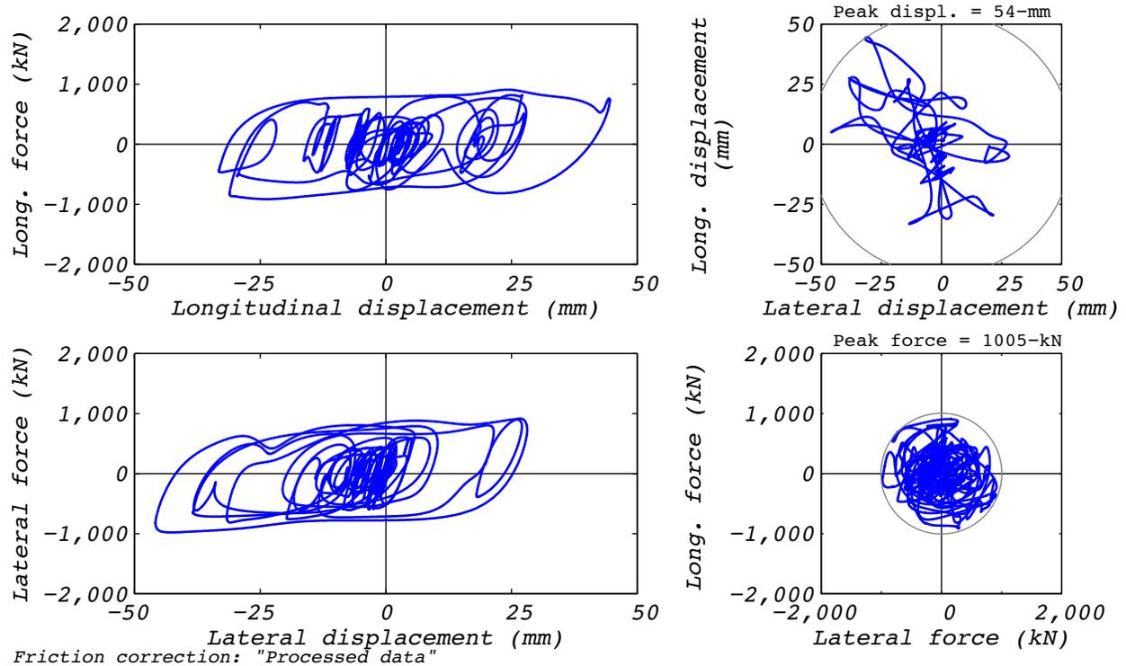
**Figure A.5-1 Bearing response for real-time reproduction of hybrid test run 26: EUR5, 2D with experimental bearing representing all bearings.**
