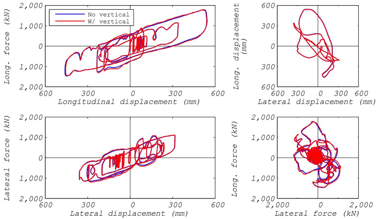
**Figure 3.44** LPRB bearing: comparison of bearing responses to a ground motion with and without vertical excitation (ground motion NRC15, 2D and 3D analyses).
