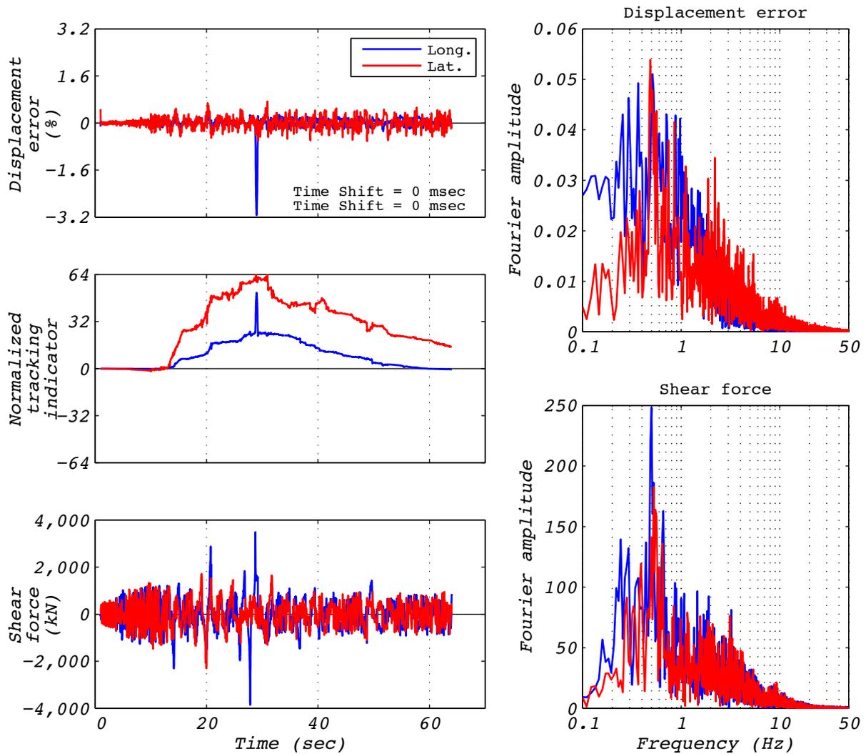
Figure C.24-1 Hybrid test performance metrics for run 58: NRC10, 2D with experimental bearing representing all bearings.
