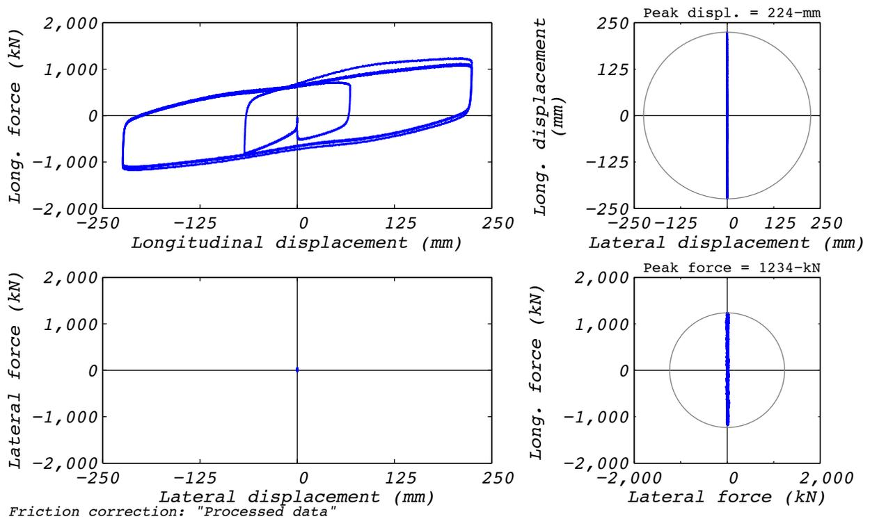
Figure B.3-2 Test run no. 12 hysteresis: Longitudinal (224 mm amplitude, 21,927 kN axial load, and 7 mm/s velocity).
