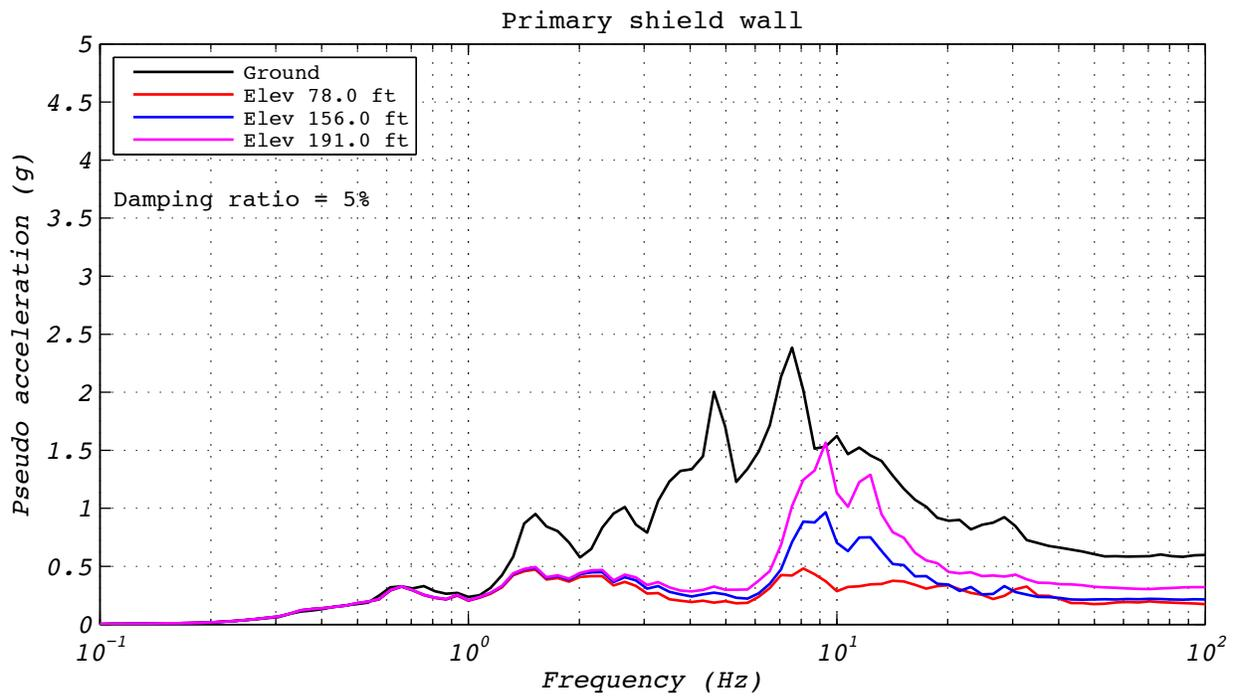
**Figure A.25-4 Hybrid test floor spectra for run 83: EUR5, 3D with 5 groups of bearings and the experimental bearing representing the no. 3 corner group.**
