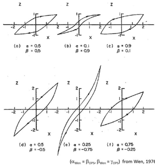
Figure 3.18 Possible hysteresis loops for different Bouc-Wen model parameters.
