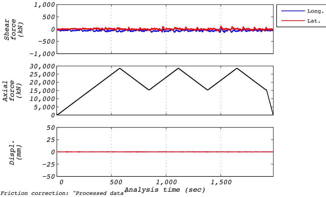
Figure B.4-1 Test run no. 13 time history: Axial (0 mm amplitude and varying axial load).
