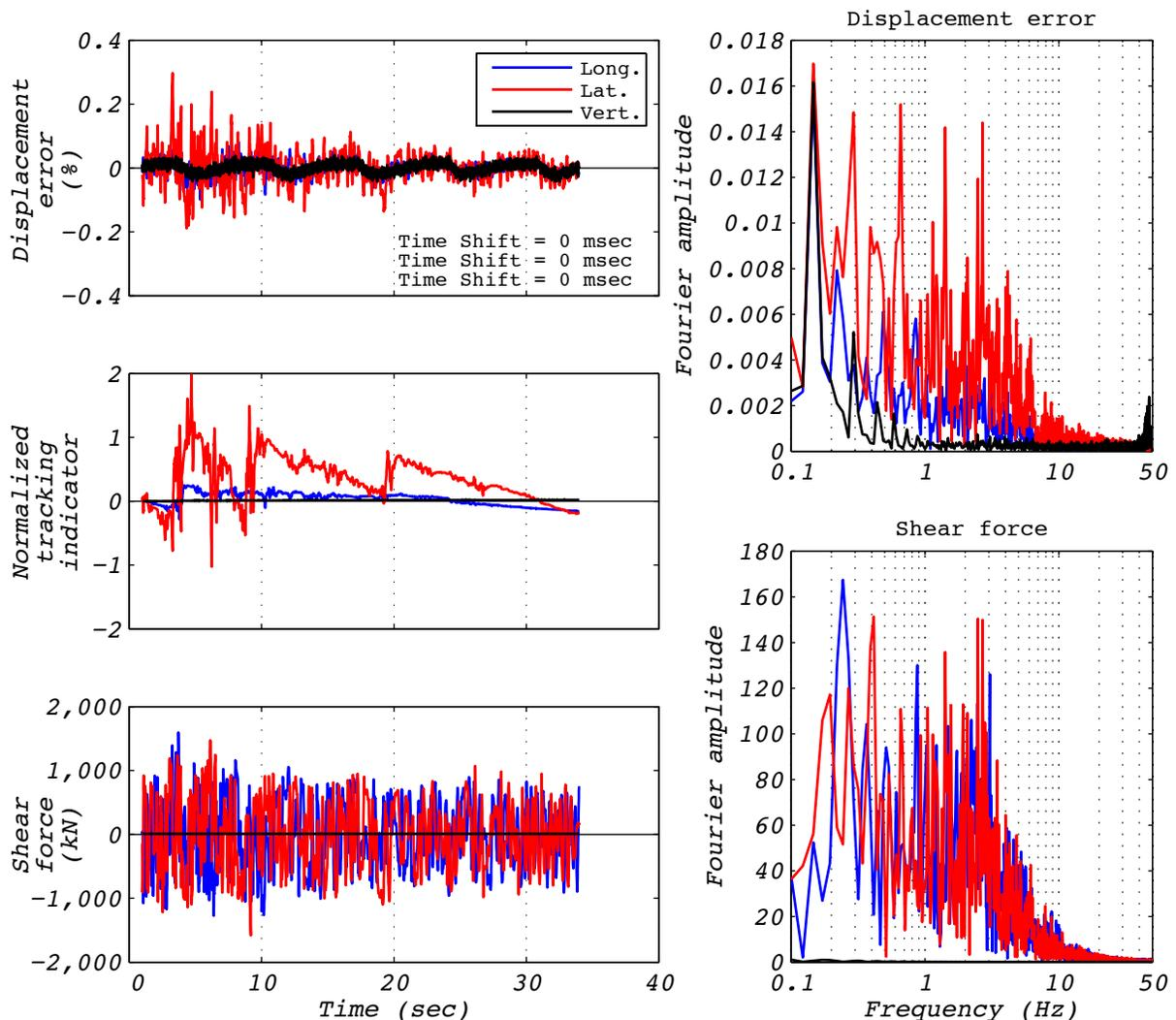
**Figure C.11-1 Hybrid test performance metrics for run 47: NRC2, 3D with 5 groups of bearings and the experimental bearing representing the center group.**
