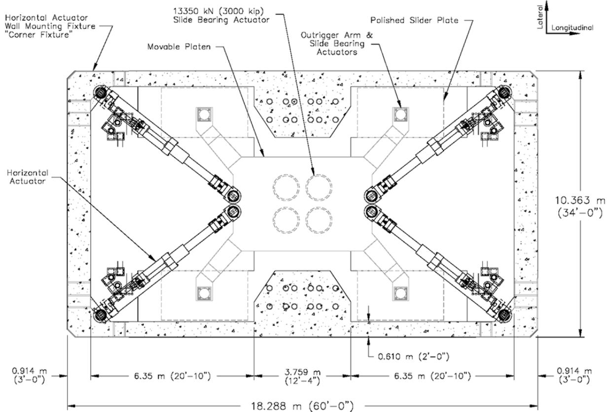
Figure 3.2 SRMD plan view.
