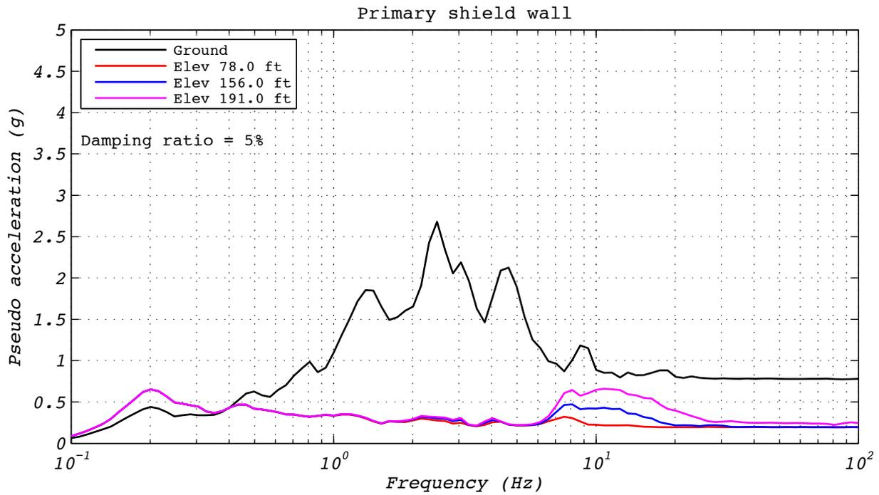
**Figure A.26-4 Hybrid test floor spectra for run 84: NRC15, 3D with 5 groups of bearings and the experimental bearing representing the center group.**
