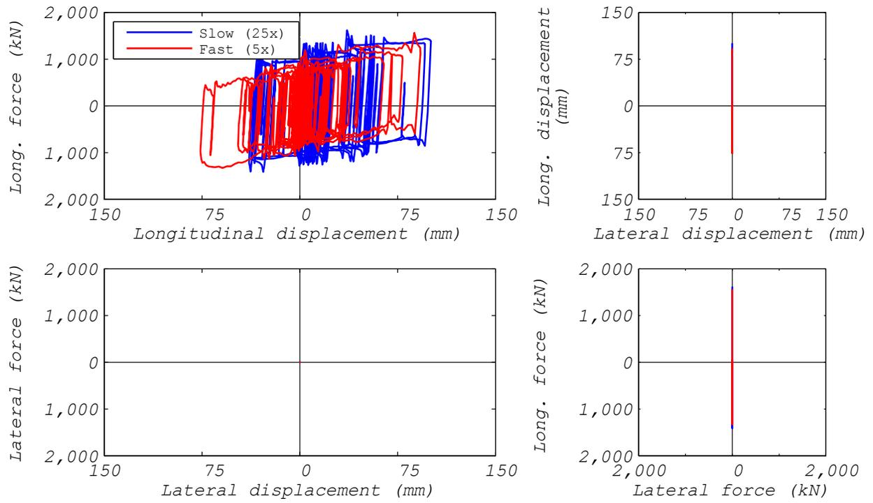
**Figure 3.74** EQS bearing: comparison of bearing responses to loading rates (ground motion NRC2, 1D analysis).
