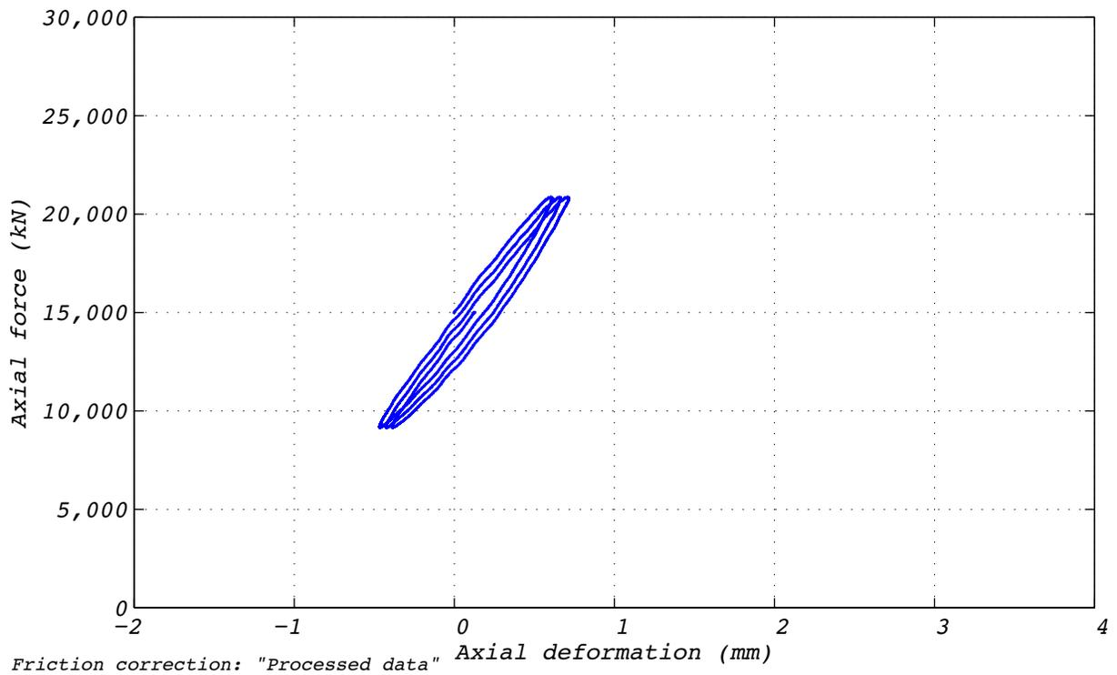
Figure D.5-2 Test run no. 5 hysteresis: Axial (0 mm displacement and varying axial load).
