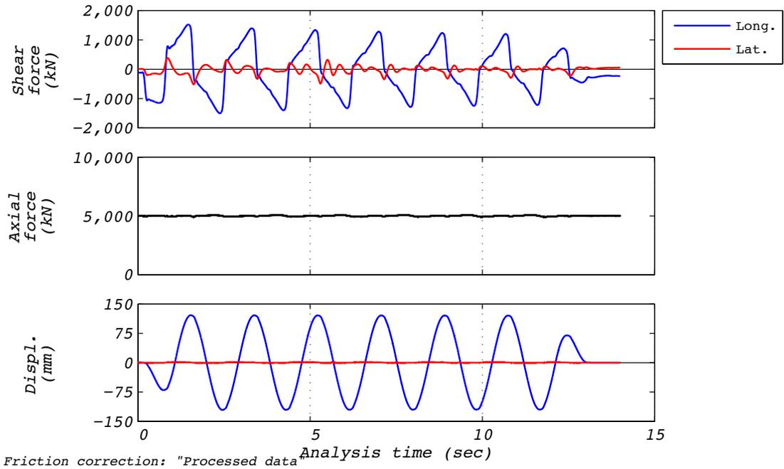
Figure D.13-1 Test run no. 13 time history: Longitudinal (120 mm amplitude, 5,000 kN axial load, and 410 mm/s velocity).
