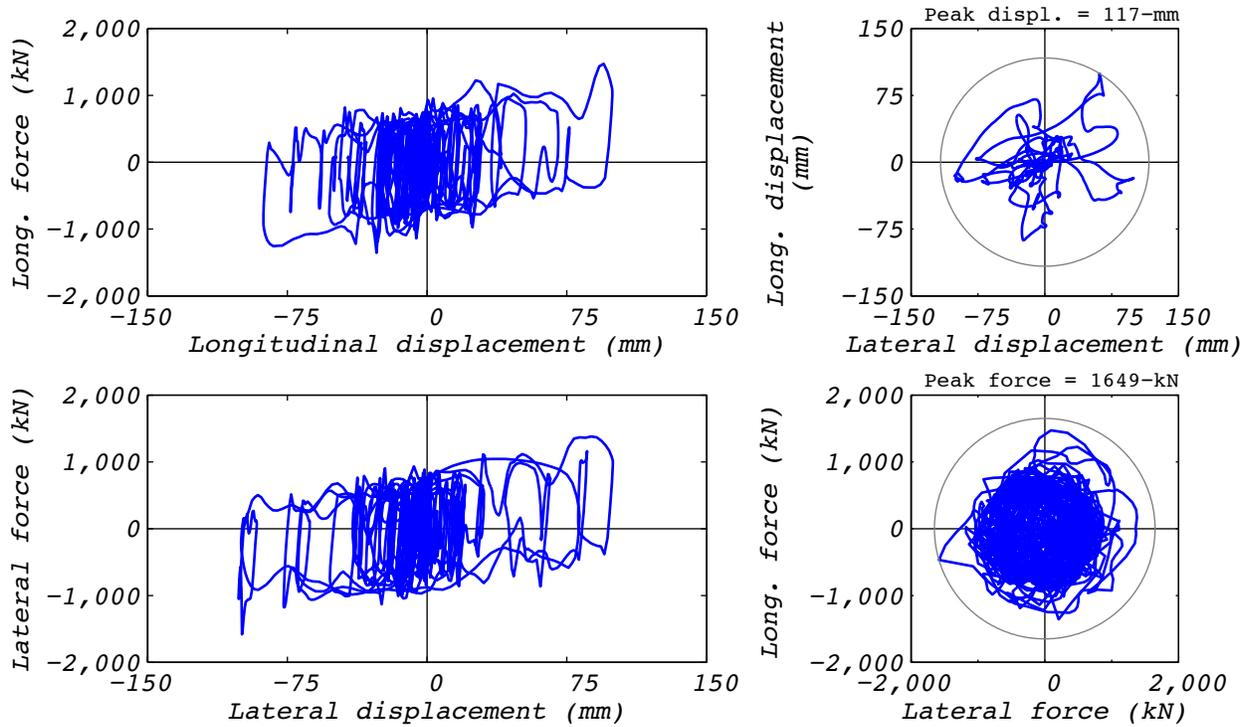
Figure C.15-2 Hybrid test bearing response for run 51: NRC2, 3D with 5 groups and the experimental bearing representing the no. 3 corner group.
