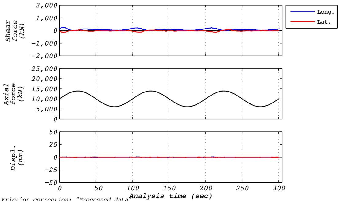
Figure D.4-1 Test run no. 4 time history: Axial (0 mm displacement and varying axial load).
