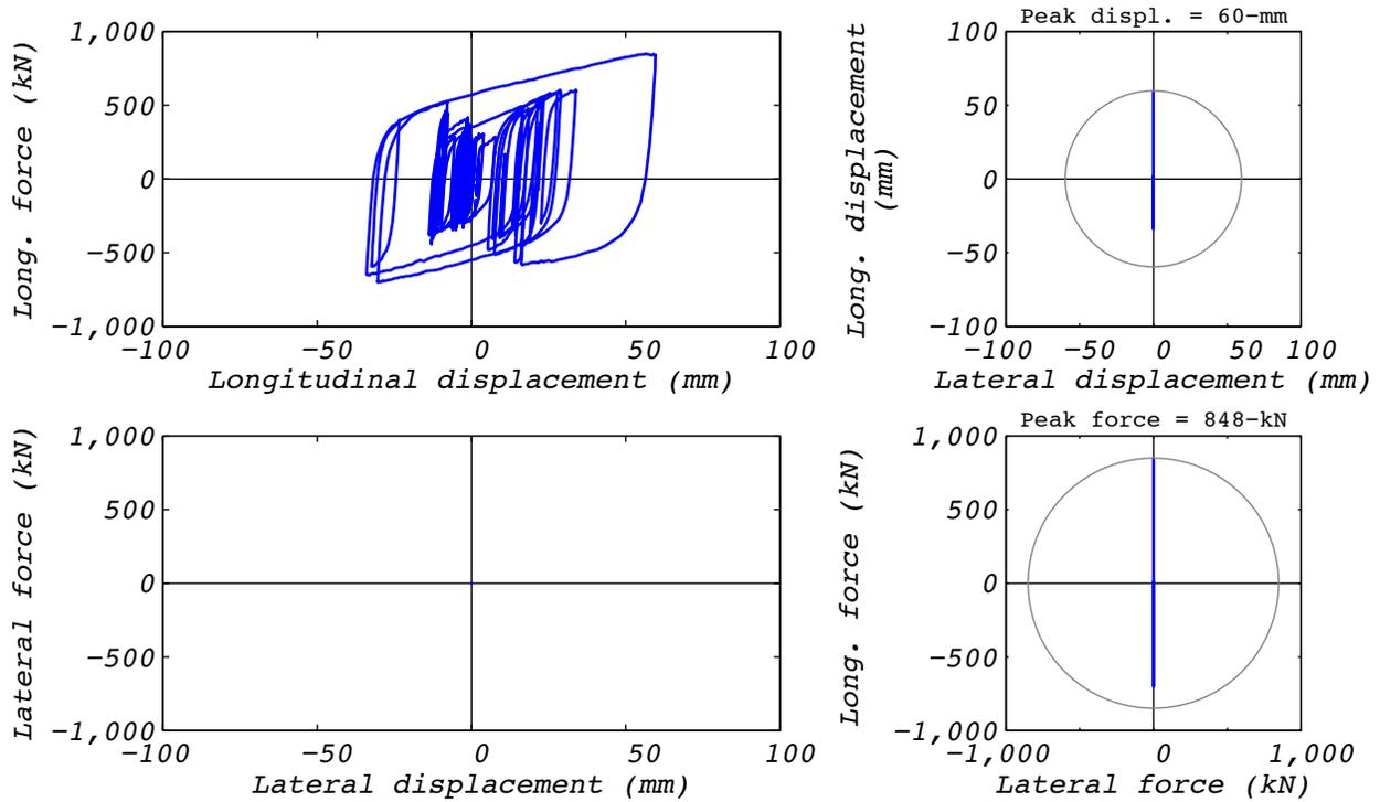
**Figure A.6-2 Hybrid test bearing response for run 42: EUR5, 1D with experimental bearing representing all bearings.**
