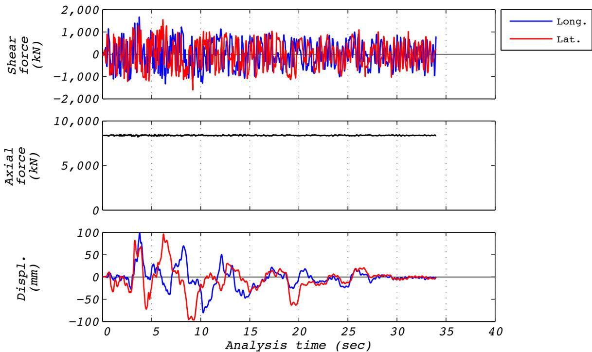
**Figure C.10-3 Hybrid test time history responses for run 46: NRC2, 3D with 5 groups of bearings and the experimental bearing representing the center group.**
