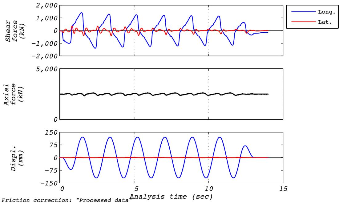
**Figure D.12-1 Test run no. 12 time history: Longitudinal (120 mm amplitude, 2,500 kN axial load, and 410 mm/s velocity).**
