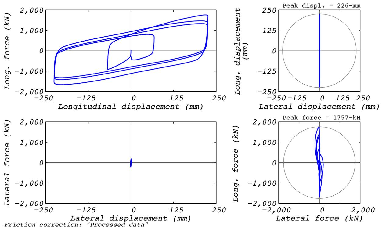
Figure B.24-2 Test run no. 67 hysteresis: Longitudinal (224 mm amplitude, 8,663 kN axial load, 586 mm/s velocity).
