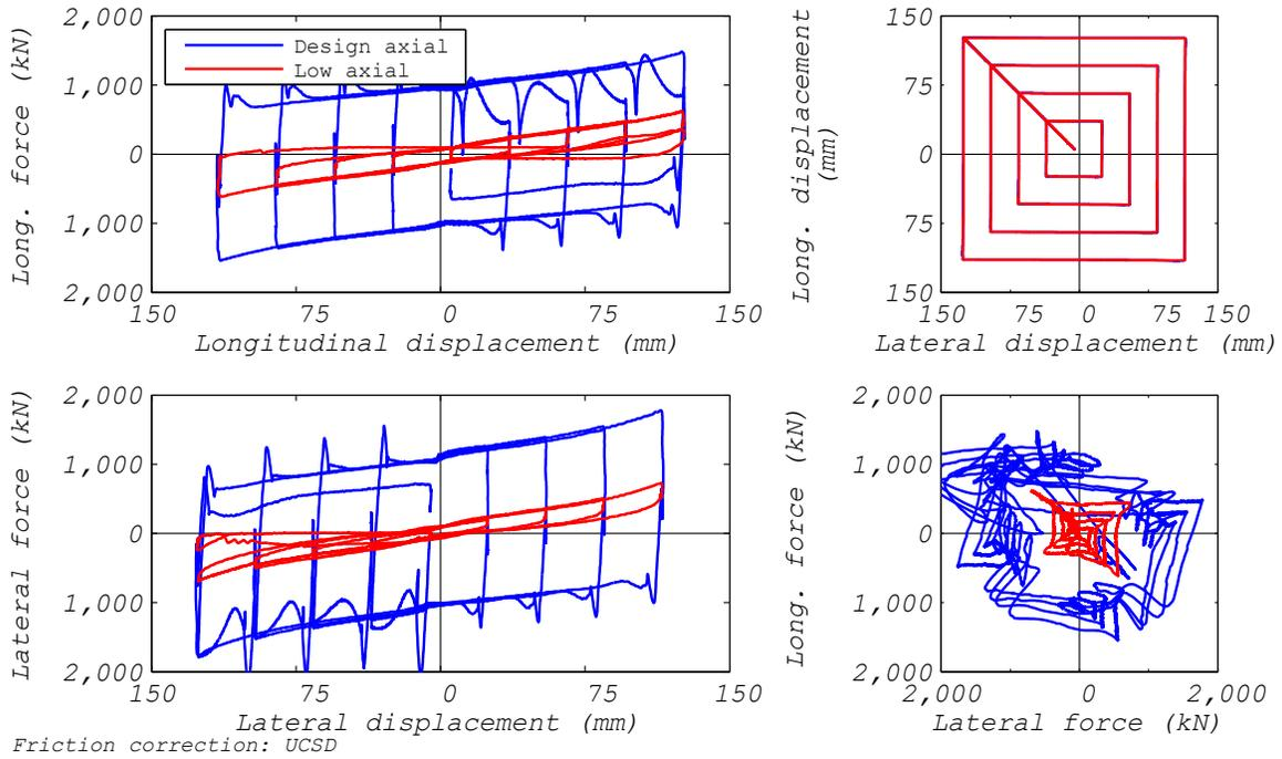
**Figure 3.86 EQS-1 bearing response to square orbits.**
