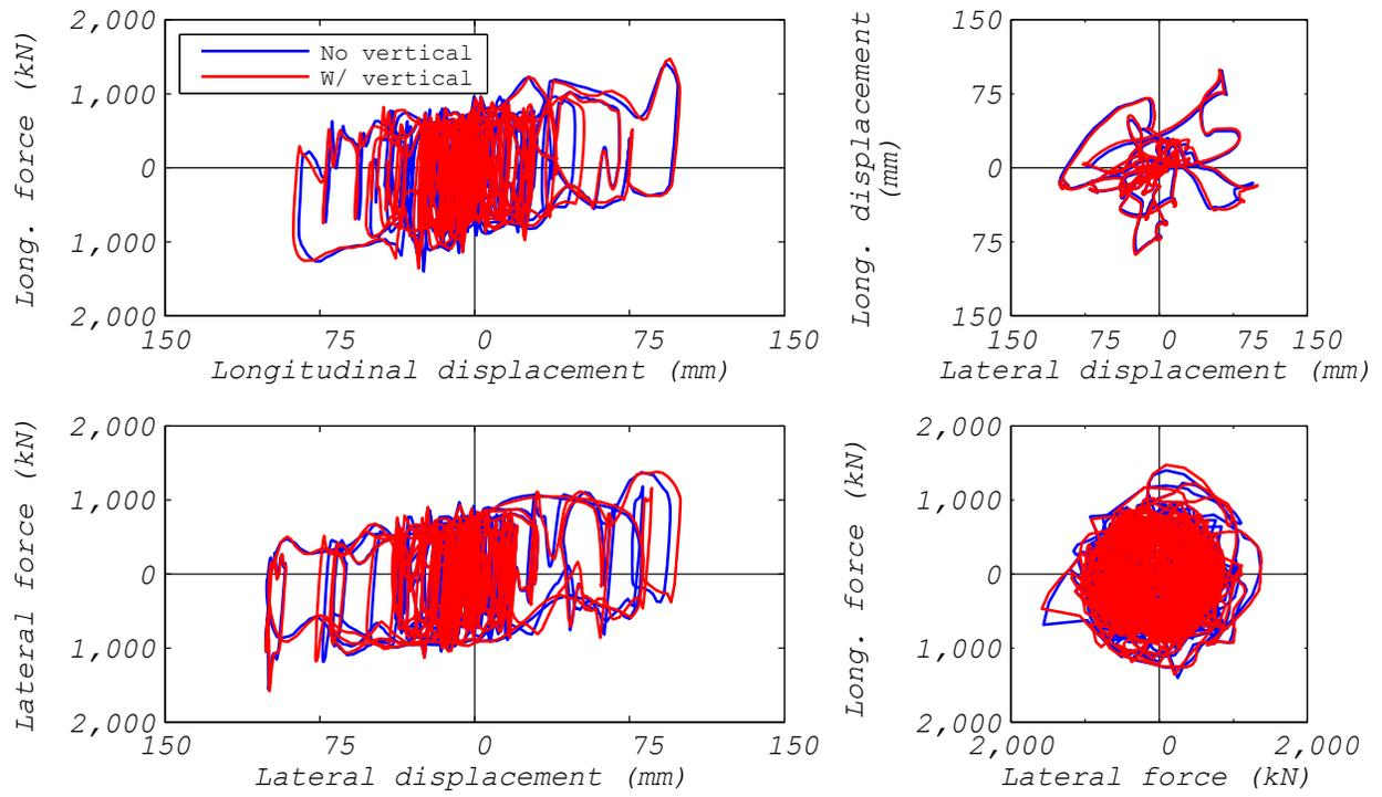
**Figure 3.66** EQS bearing: comparison of bearing responses to a ground motion with and without vertical excitation (ground motion NRC2, 2D and 3D analyses).
