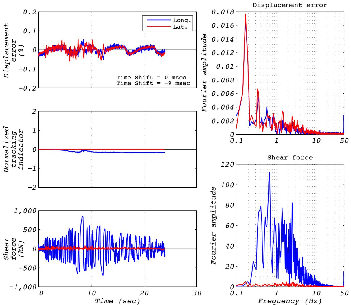
Figure A.6-1 Hybrid test performance metrics for run 42: EUR5, 1D with experimental bearing representing all bearings.
