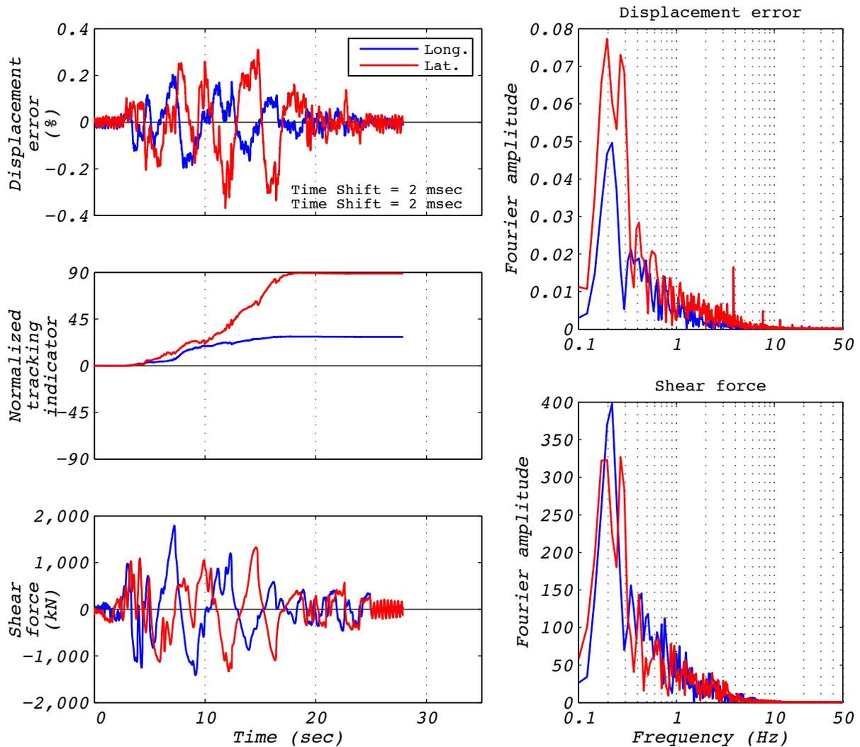
Figure A.15-1 Hybrid test performance metrics for run 55: NRC15, 2D with experimental bearing representing all bearings.
