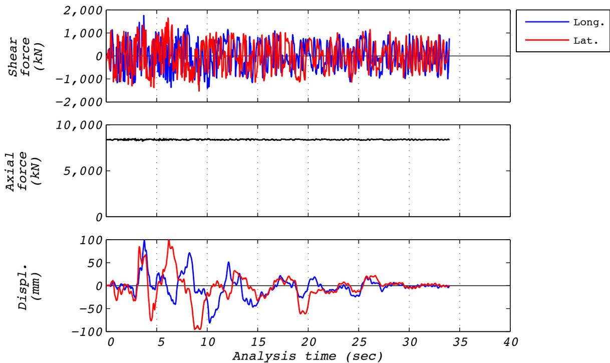
**Figure C.8-3 Hybrid test time history responses for run 43: NRC2, 3D with 5 groups of bearings and the experimental bearing representing the center group.**
