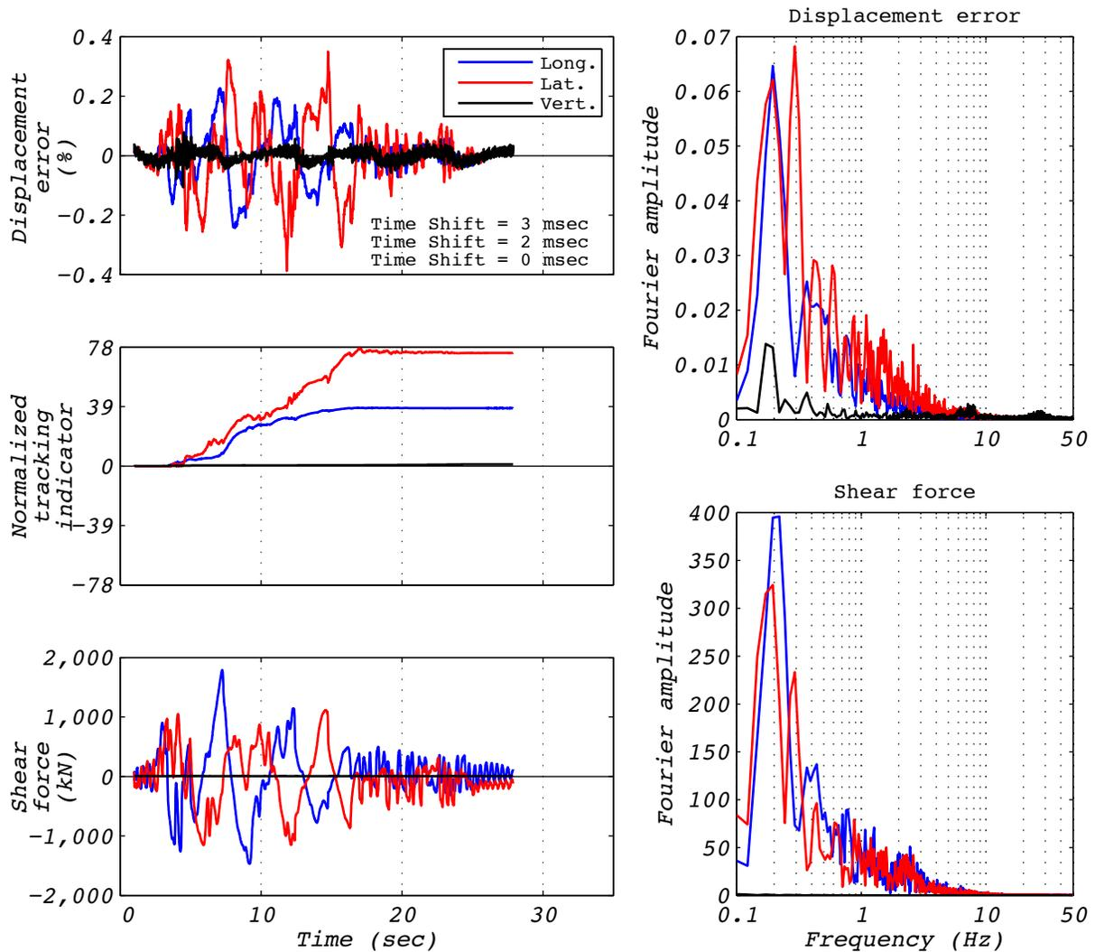
Figure A.27-1 Hybrid test performance metrics for run 85: NRC15, 3D with 5 groups of bearings and the experimental bearing representing the no. 3 corner group.
