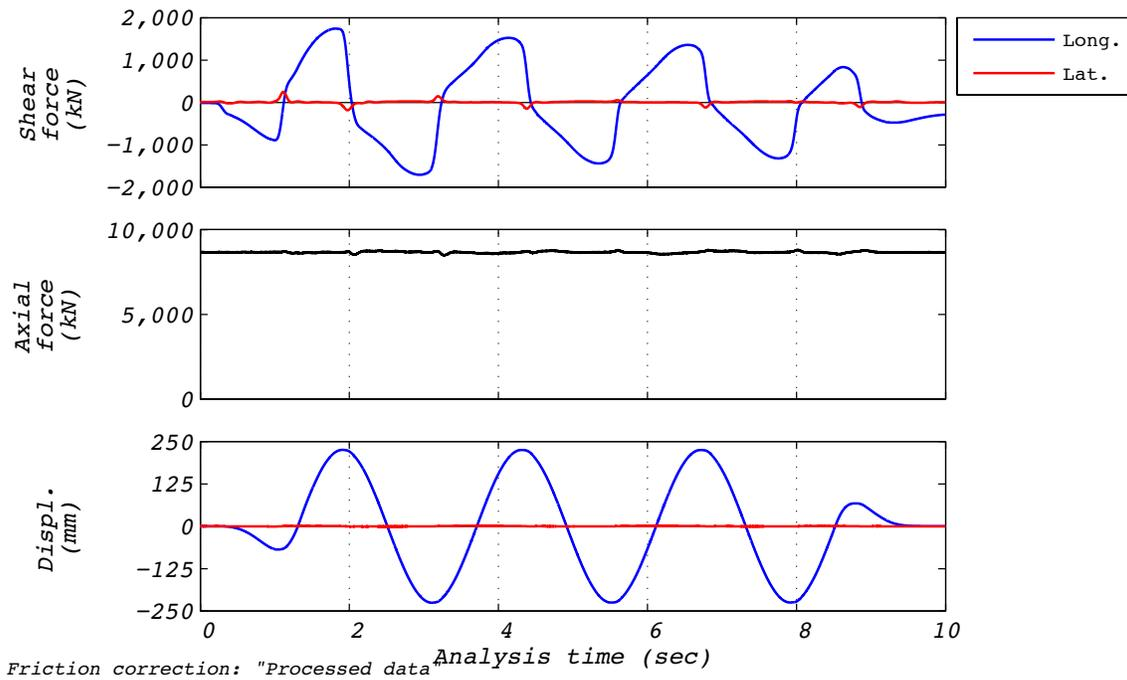
Figure B.16-1 Test run no. 54 time history: Longitudinal (224 mm amplitude, 8,663 kN axial load, and 586 mm/s velocity).
