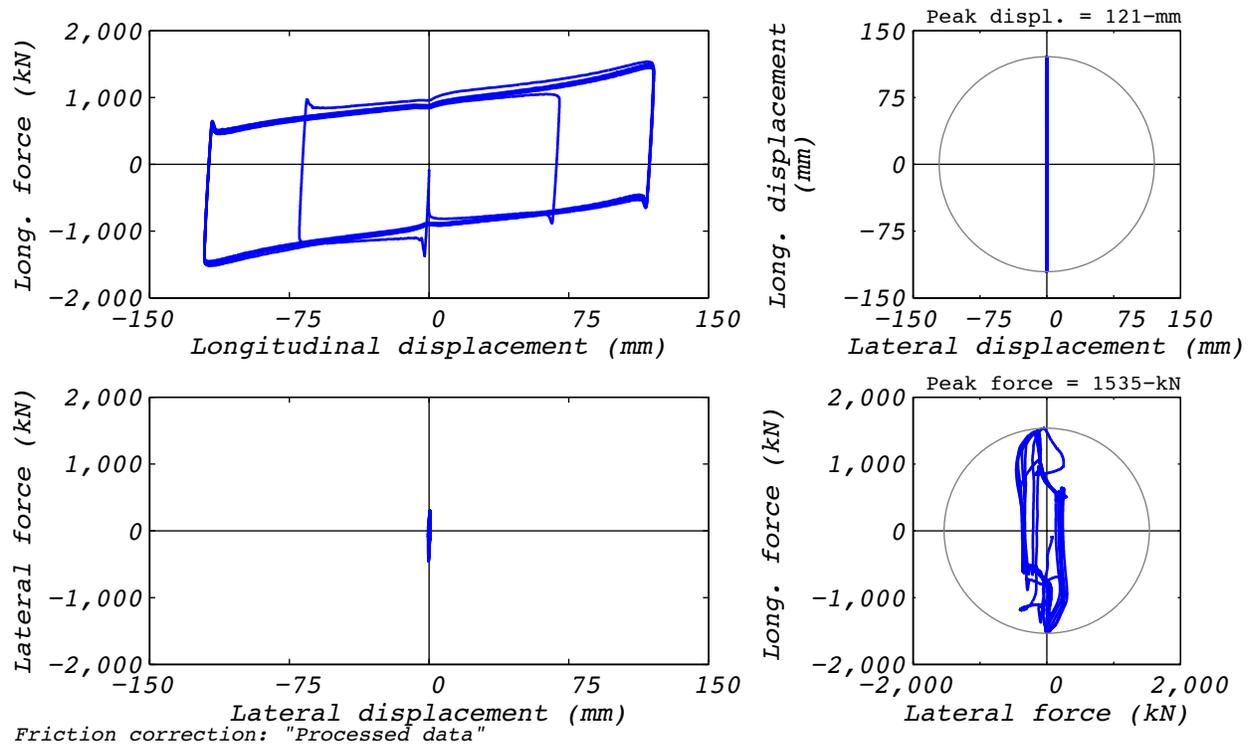
Figure D.15-2 Test run no. 15 hysteresis: Longitudinal (120 mm amplitude, 8,663 kN axial load, and 41 mm/s velocity).
