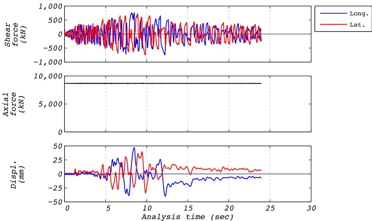
**Figure A.21-3 Hybrid test time history responses for run 78: EUR5, 3D with experimental bearing representing all bearings.**
