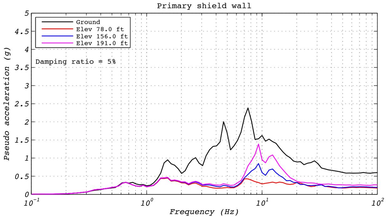
**Figure A.24-4 Hybrid test floor spectra for run 82: EUR5, 3D with 5 groups of bearings and the experimental bearing representing the center group.**
