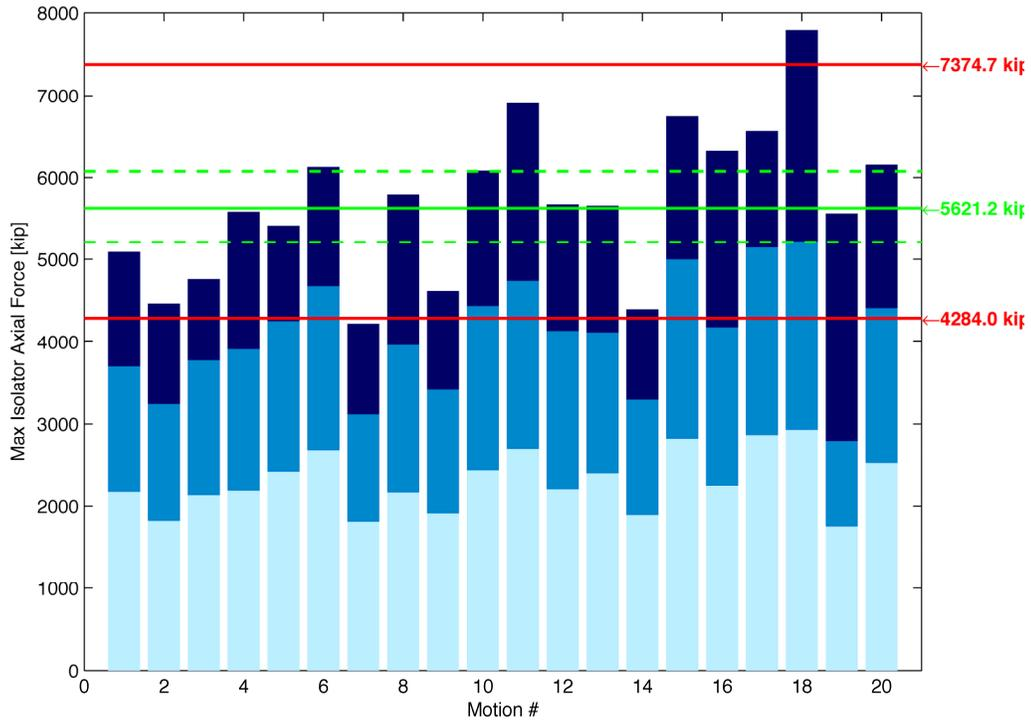
**Figure 3.31 Analytically based peak axial force demands for the NRC hazard level [1973] based on an LPRB isolator (green lines = median with 95% confidence interval, red lines = 5<sup>th</sup> and 95<sup>th</sup> percentile).**
