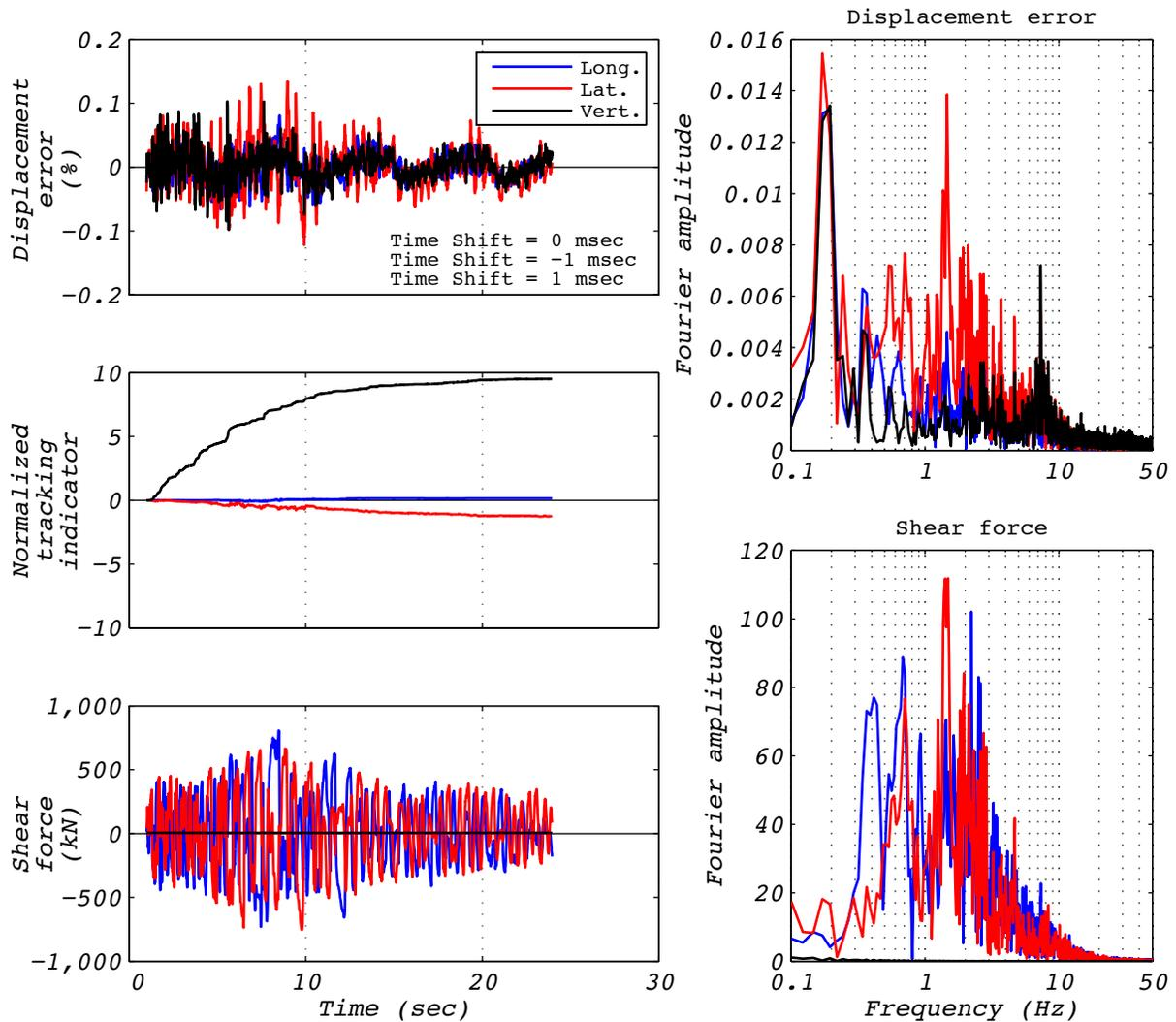
Figure A.25-1 Hybrid test performance metrics for run 83: EUR5, 3D with 5 groups of bearings and the experimental bearing representing the no. 3 corner group.
