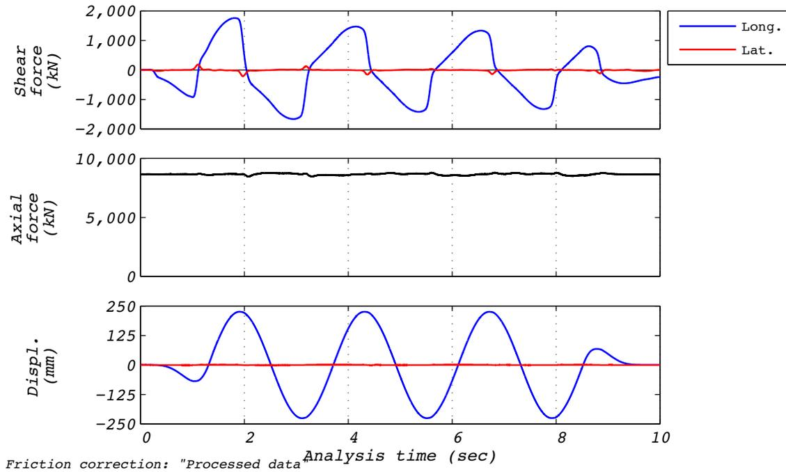
Figure B.24-1 Test run no. 67 time history: Longitudinal (224 mm amplitude, 8,663 kN axial load, 586 mm/s velocity).
