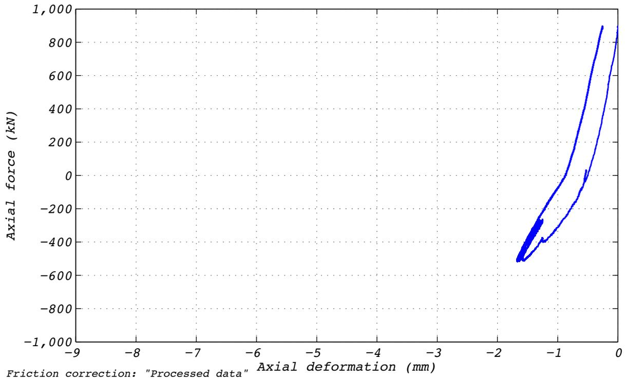
Figure B.5-2 Test run no. 14 hysteresis: Axial (0mm amplitude and tensile axial load).
