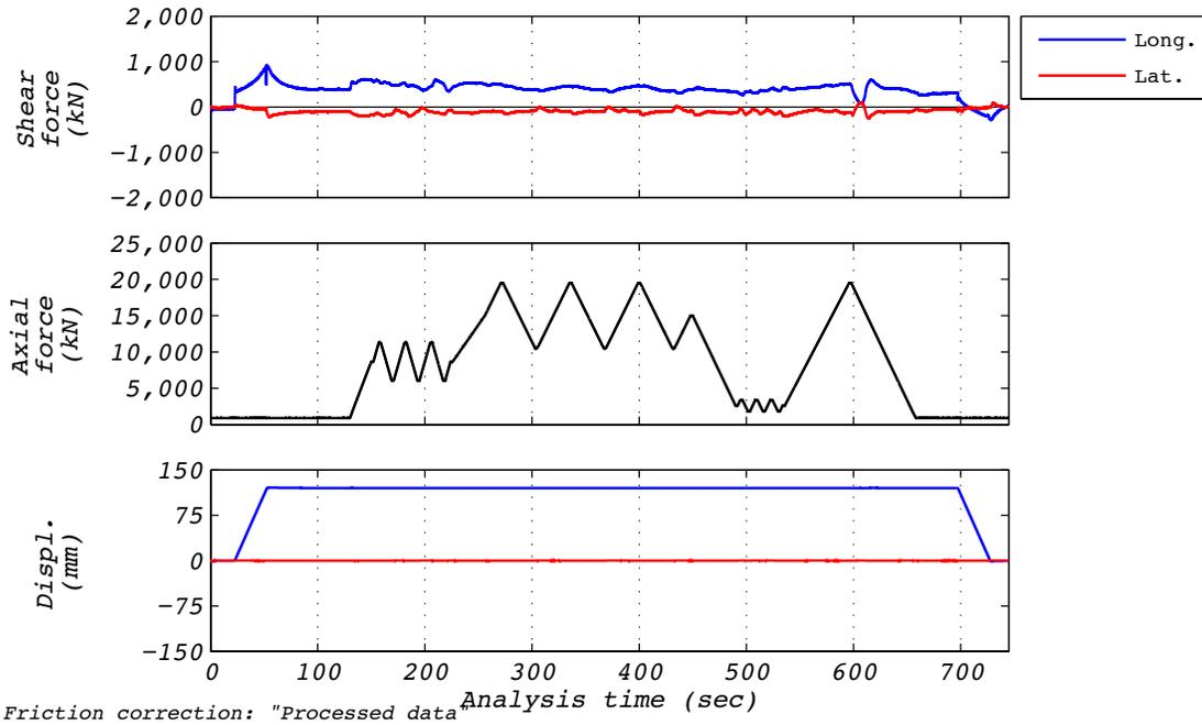
Figure D.3-1 Test run no. 3 time history: Axial (120 mm displacement and varying axial load).
