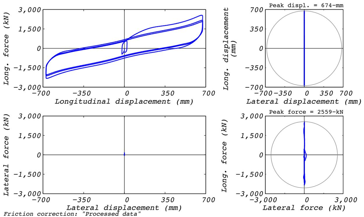
Figure B.22-2 Test run no. 65 hysteresis: Longitudinal (896 mm amplitude, 8,663 kN axial load, and 56 mm/s velocity).
