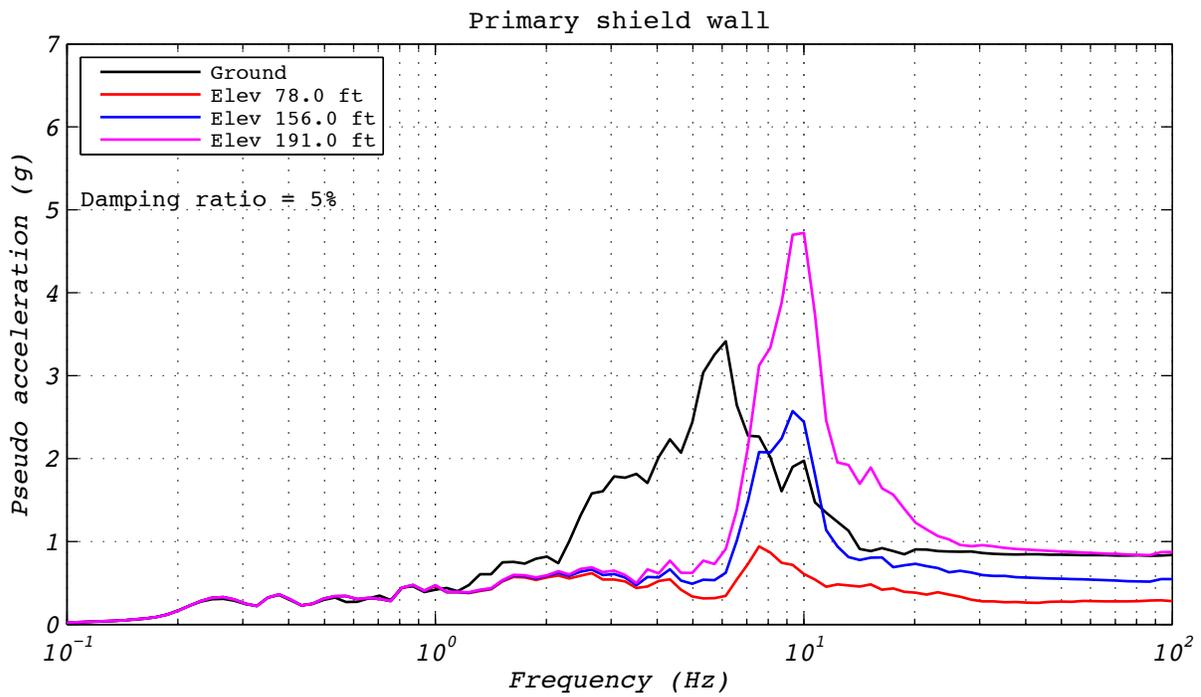
**Figure C.17-3 Floor spectra for analytical run 52A: NRC2, 1D with a single analytical bearing.**
