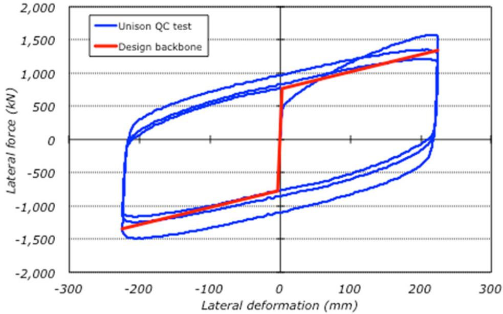
Figure 2.2 LPRB lateral quality-control test and design envelope.
