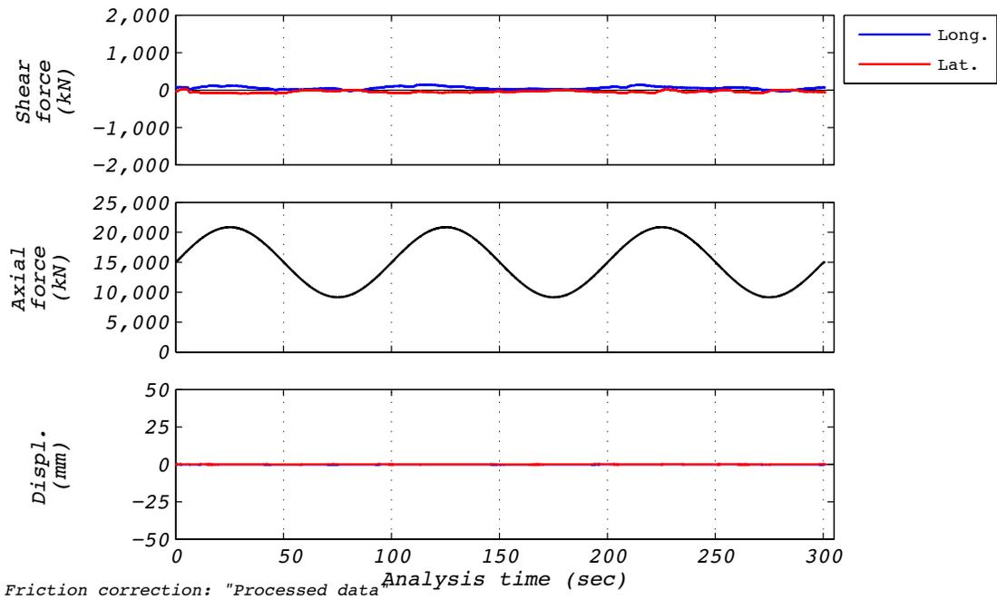
Figure D.5-1 Test run no. 5 time history: Axial (0 mm displacement and varying axial load).
