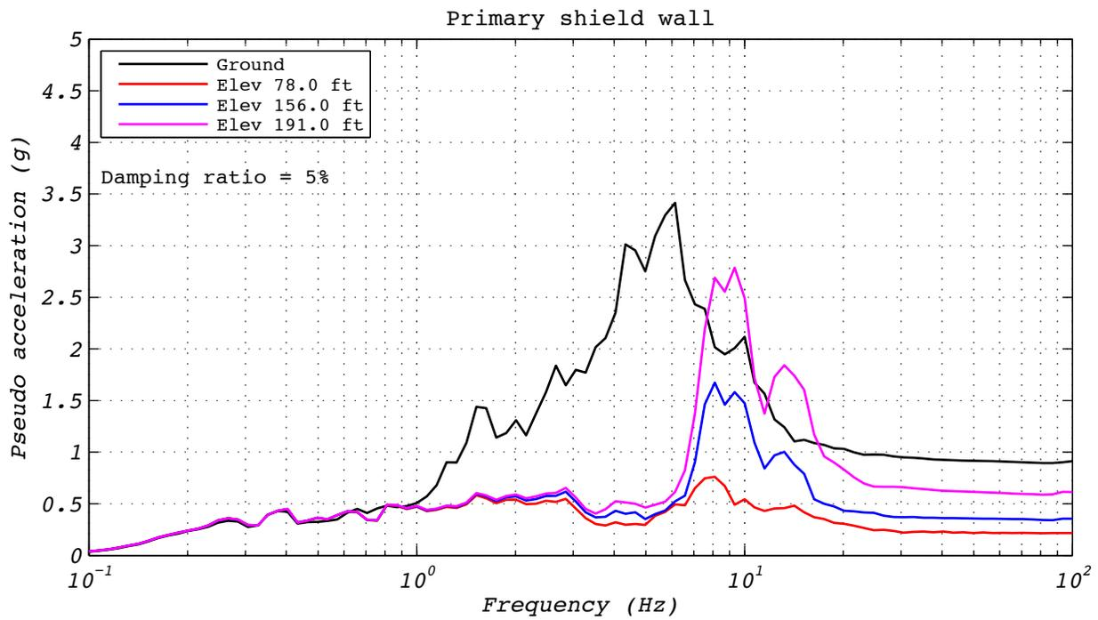
**Figure C.10-4 Hybrid test floor spectra for run 46: NRC2, 3D with 5 groups of bearings and the experimental bearing representing the center group.**
