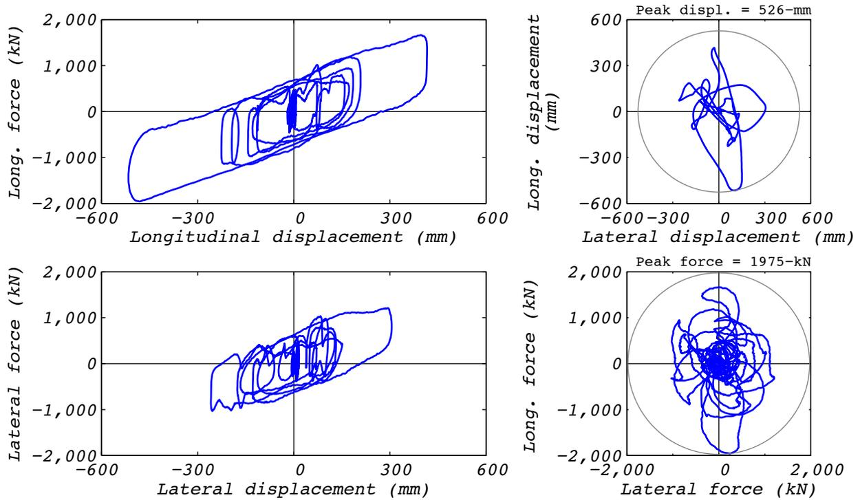
Figure A.19-2 Hybrid test bearing response for run 61: NRC15, 2D with experimental bearing representing one of 527.
