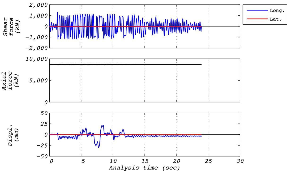
**Figure C.1-3 Hybrid test time history responses metrics for run 17: EUR5, 1D with experimental bearing representing all bearings.**
