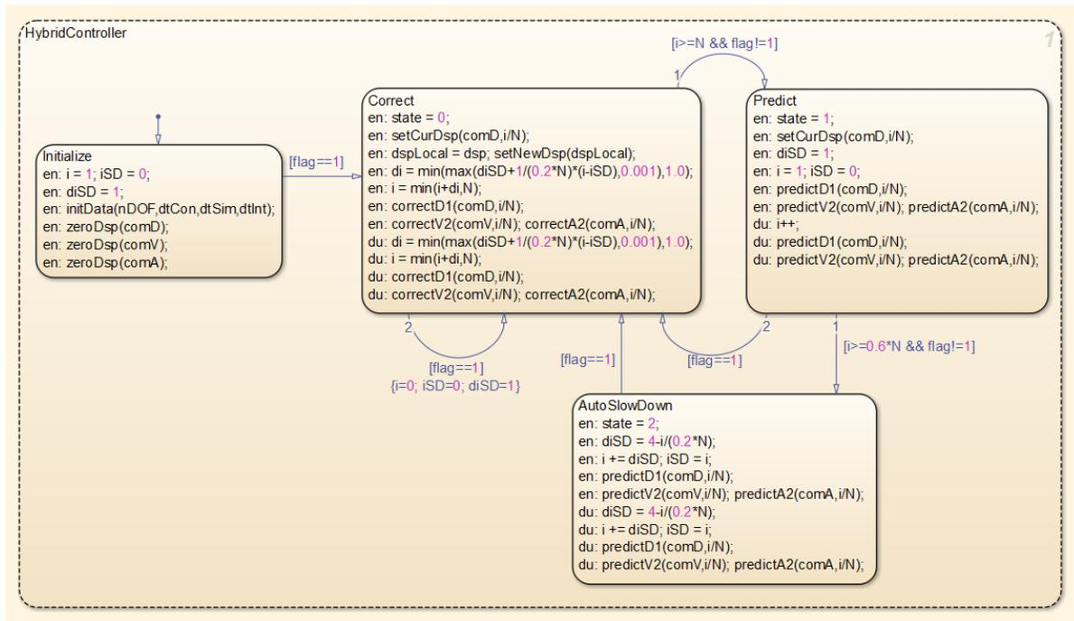
Figure 3.7 Predictor-corrector [Schellenberg et al. 2009].
