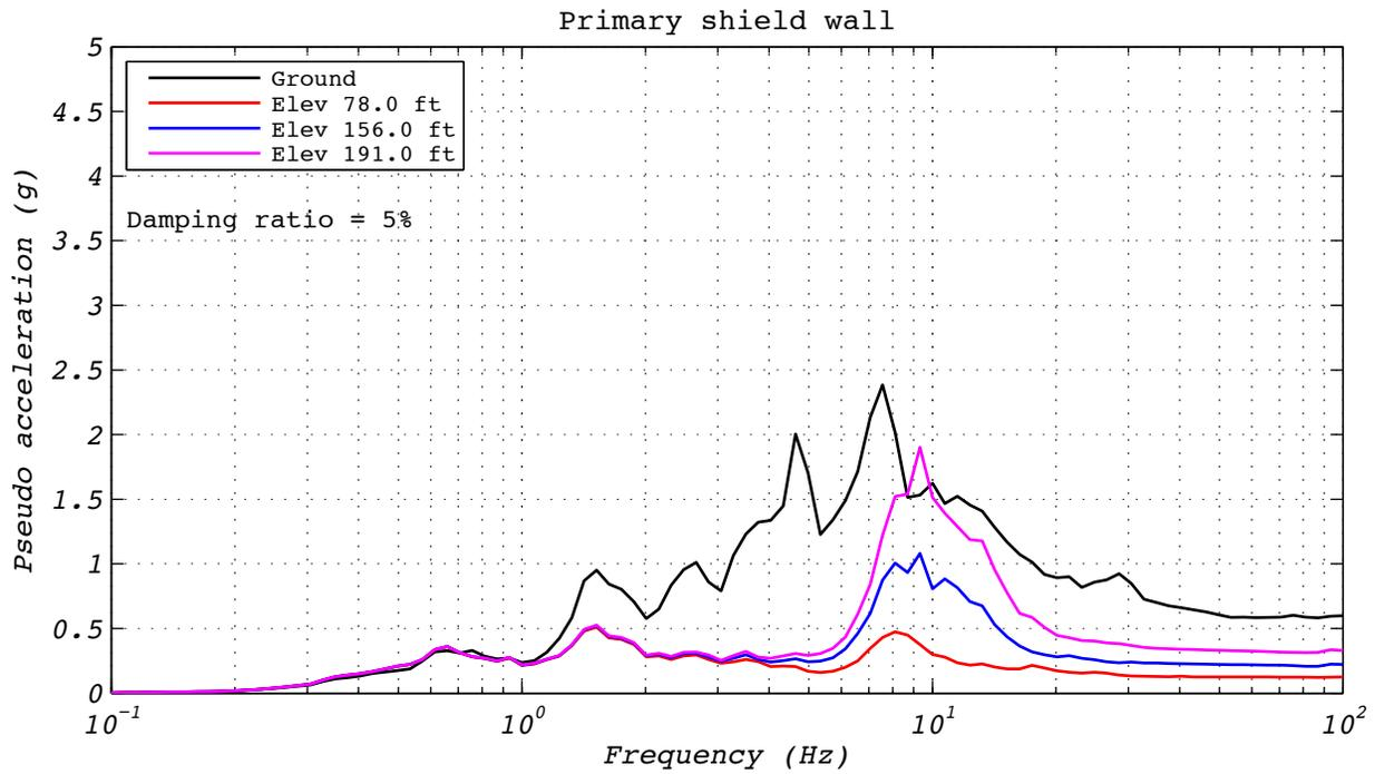
**Figure A.3-4 Hybrid test floor spectra for run 26: EUR5, 2D with experimental bearing representing all bearings.**
