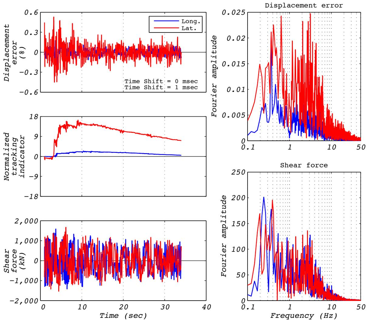
Figure C.20-1 Hybrid test performance metrics for run 54: NRC2, 2D with experimental bearing representing all bearings.
