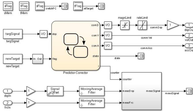
**Figure 3.9 Applying the limits on the command signals.**
