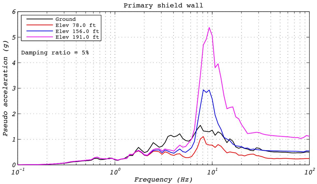
**Figure C.18-4 Hybrid test floor spectra for run 53: EUR5, 1D with experimental bearing representing all bearings.**
