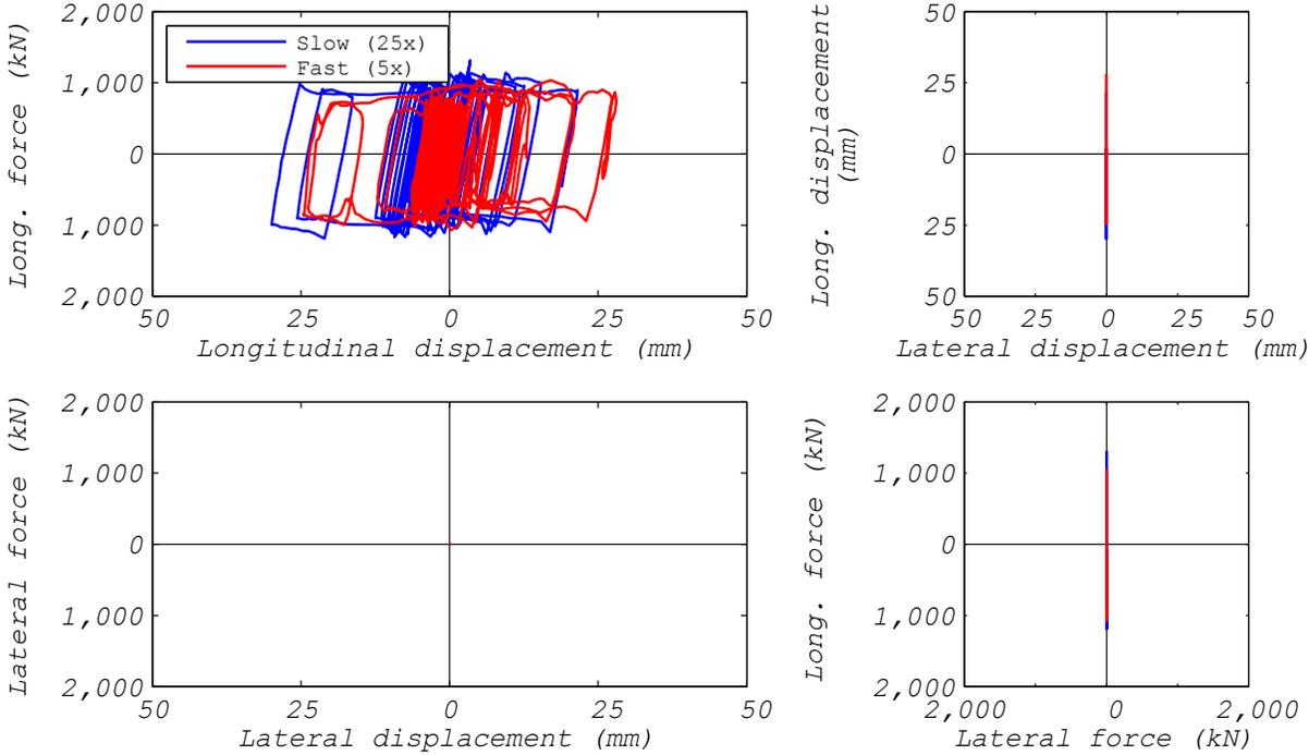
**Figure 3.72 EQS bearing: comparison of bearing responses to loading rates (ground motion EUR5, 1D analysis).**
