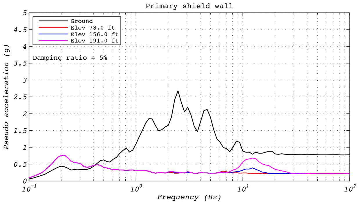
**Figure A.20-4 Hybrid test floor spectra for run 63: NRC15, 2D with five groups of bearings.**
