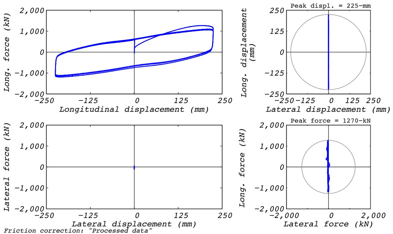
Figure B.26-2 Test run no. 69 hysteresis: Longitudinal (224 mm amplitude, 21,927 kN axial load, and 7 mm/s velocity).
