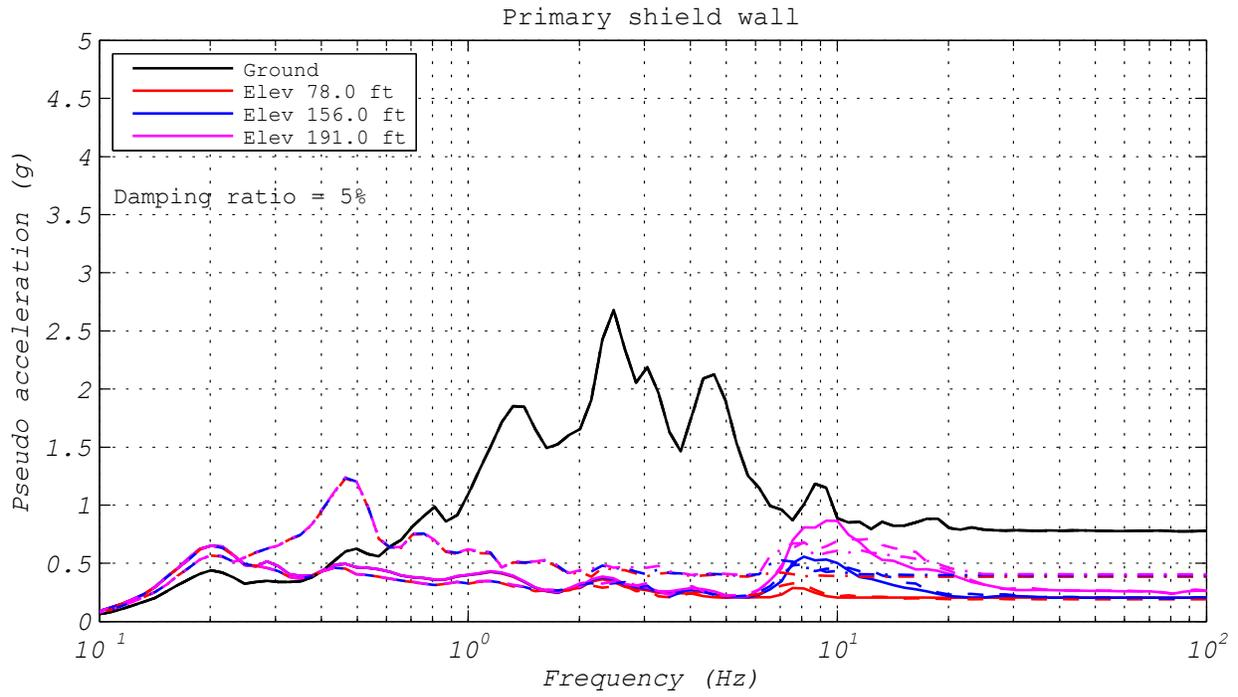
Figure 3.51 LPRB bearing: response spectra comparison of responses to bearing layout discretization (ground motion NRC15, 2D analysis).
