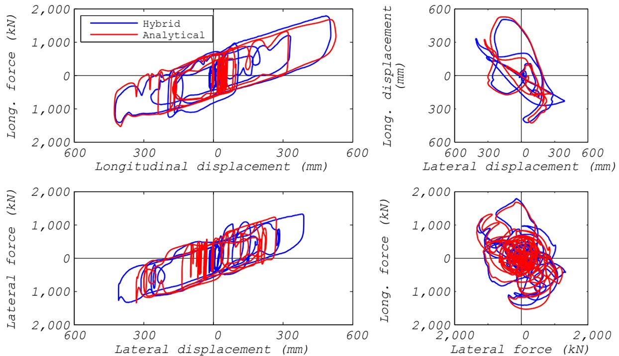
**Figure 3.58** LPRB bearing: comparison of hybrid simulation and analytical estimation bearing responses (ground motion NRC15, 2D analysis).
