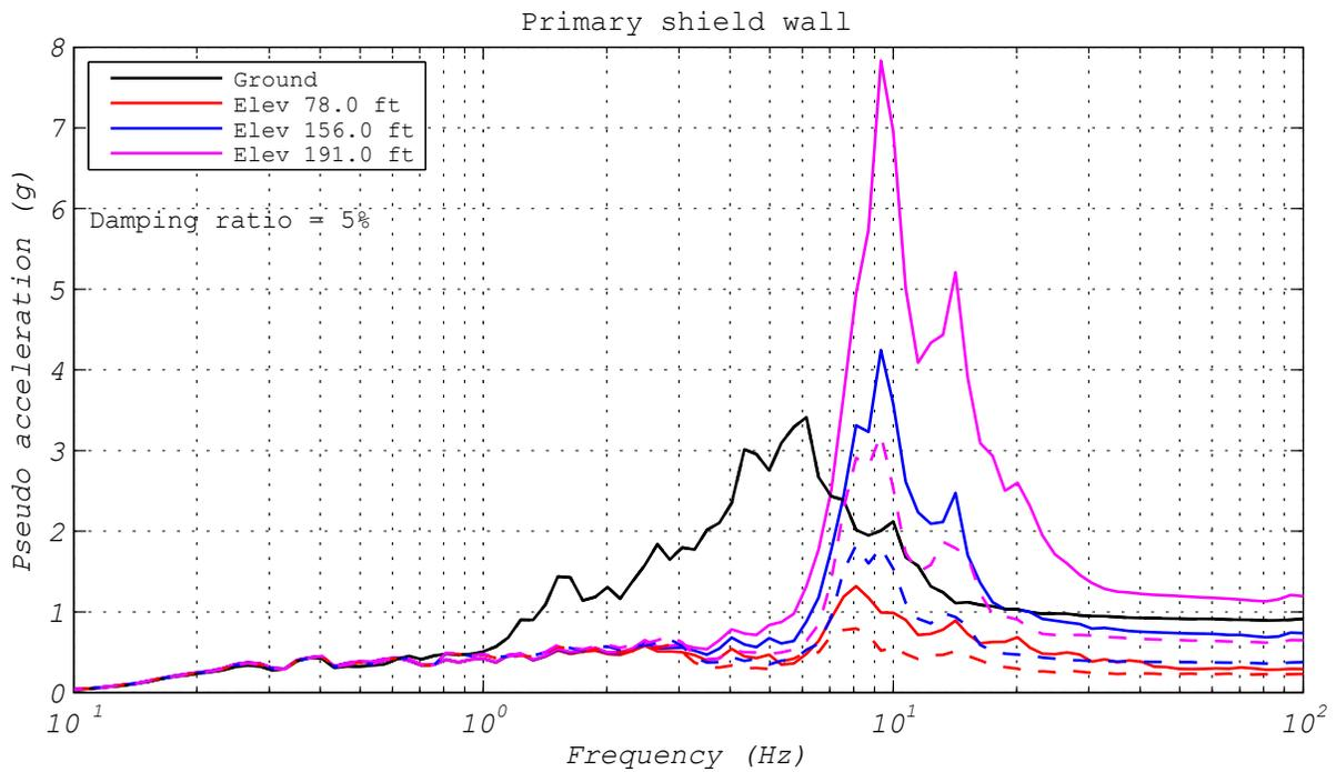
**Figure 3.71** EQS bearing: response spectra comparison of responses to bearing layout discretization (ground motion NRC2, 2D analysis).
