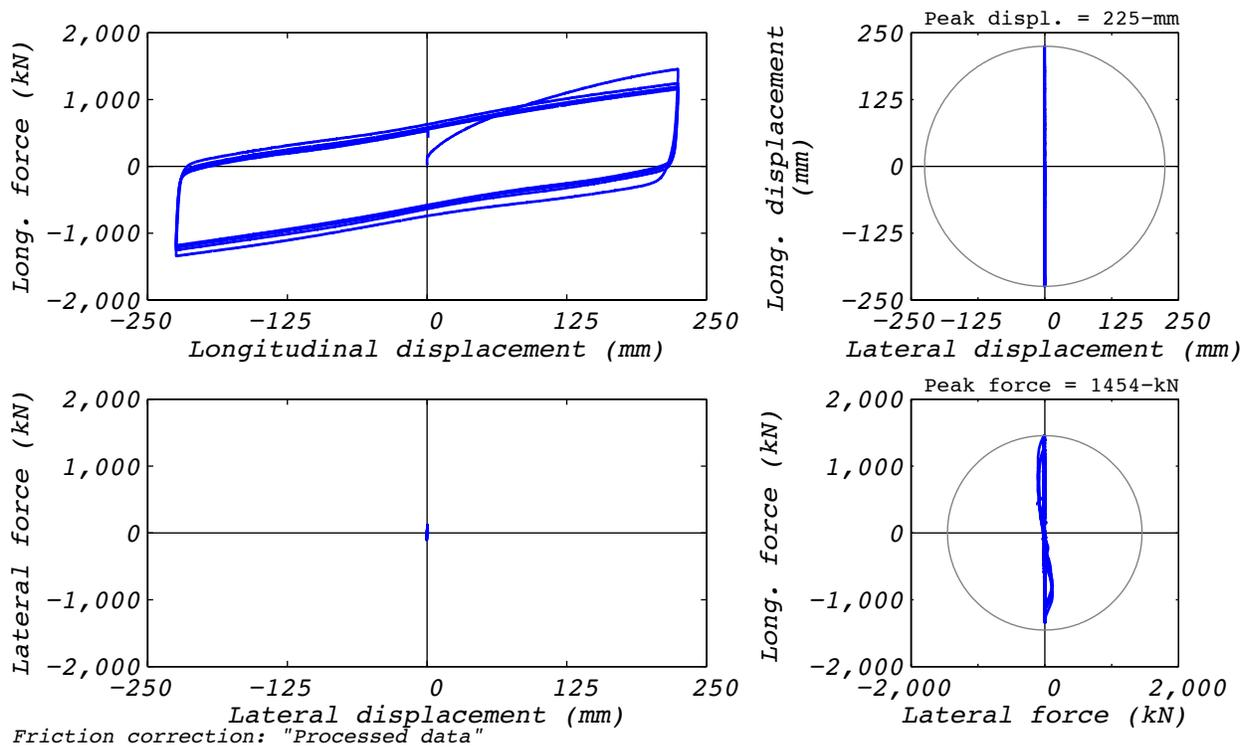
Figure B.29-2 Test run no. 72 hysteresis: Longitudinal (224 mm amplitude, 8,663 kN axial load, and 9 mm/s velocity).
