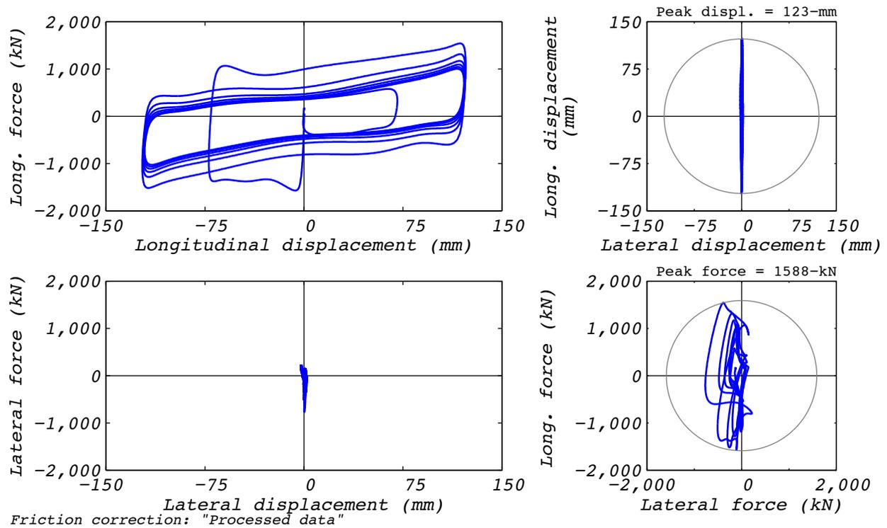
Figure D.19-2 Test run no. 25 hysteresis: Longitudinal (120 mm amplitude, 8,663 kN axial load, and 820 mm/s velocity).
