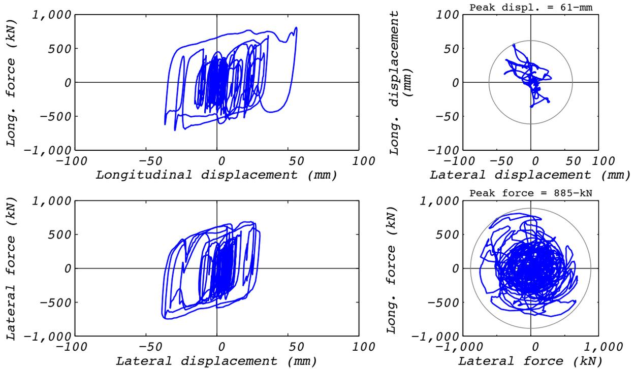
**Figure A.23-2 Hybrid test bearing response for run 80: EUR5, 3D with 5 groups of bearings and the experimental bearing representing the center group.**
