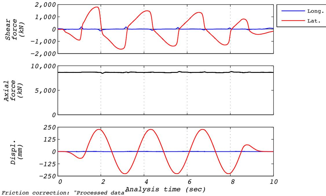
Figure B.10-1 Test run no. 23 time history: Transverse (224 mm amplitude, 8,663 kN axial load, and 586 mm/s velocity).
