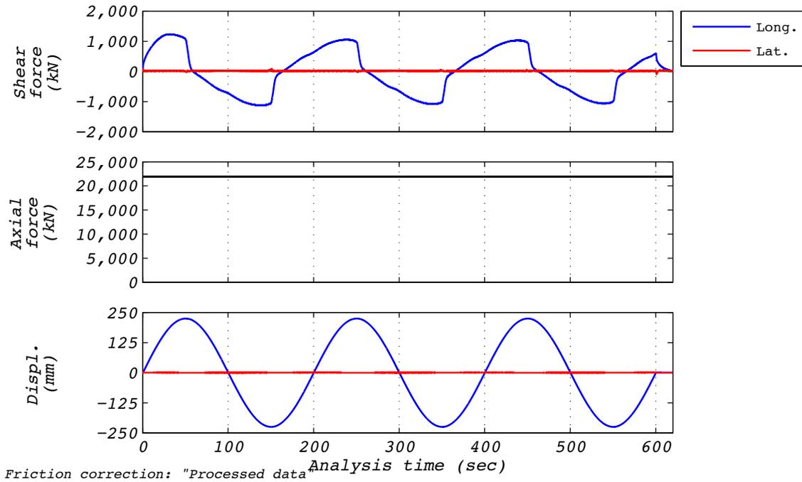
Figure B.17-1 Test run no. 56 time history: Longitudinal (224 mm amplitude, 8,663 kN axial load, and 7 mm/s velocity).
