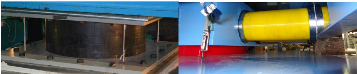
Figure 3.23 LVDTs used to measure vertical deformation of the bearings.
