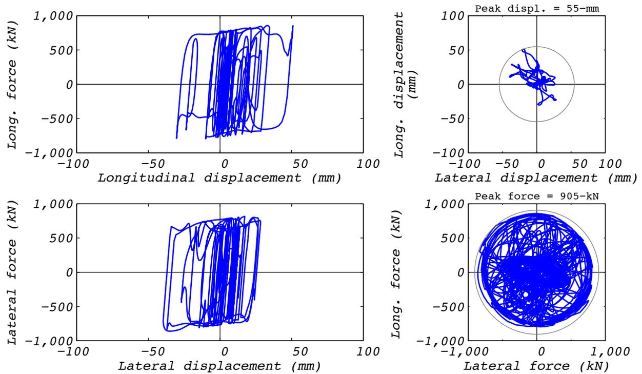
**Figure A.2 Hybrid test bearing response for run 24: EUR5, 2D with experimental bearing representing all bearings.**
