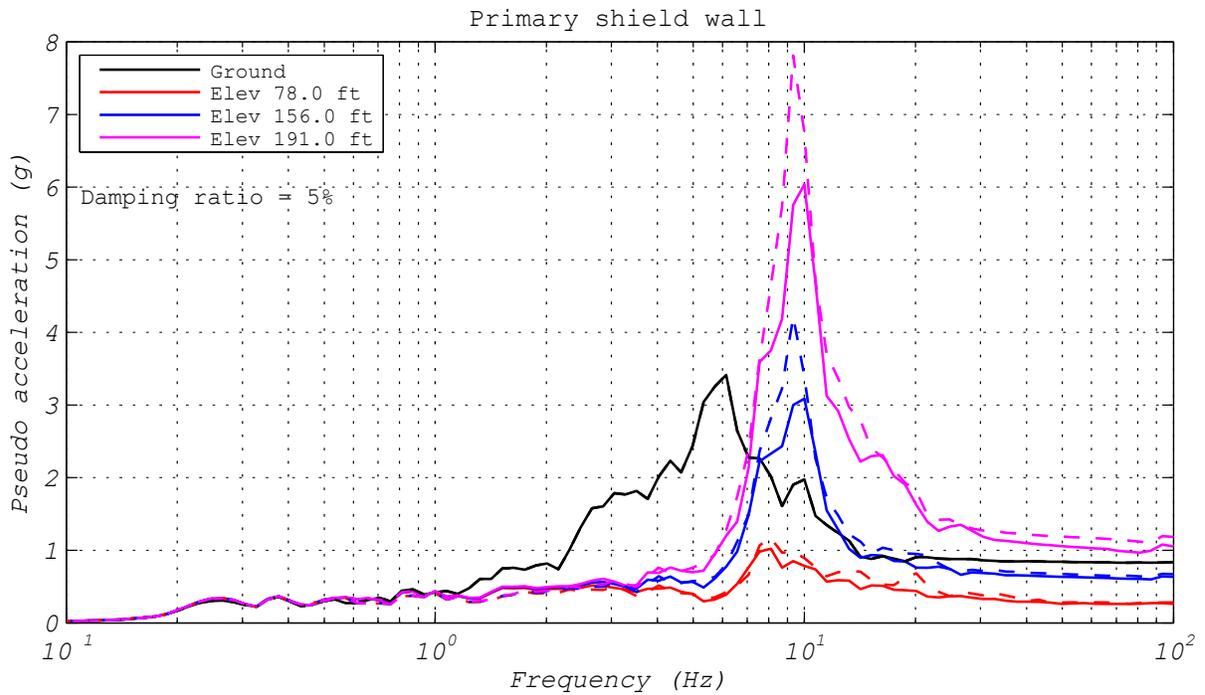
**Figure 3.65** EQS bearing: response spectra comparison of responses to ground motion NRC2 executed five-times slower than real time (1D and 2D analyses).
