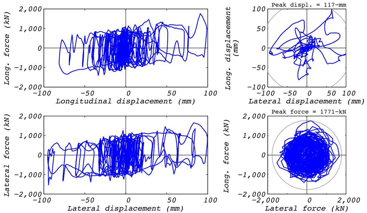
**Figure C.8-2 Hybrid test bearing response for run 43: NRC2, 3D with 5 groups of bearings and the experimental bearing representing the center group.**
