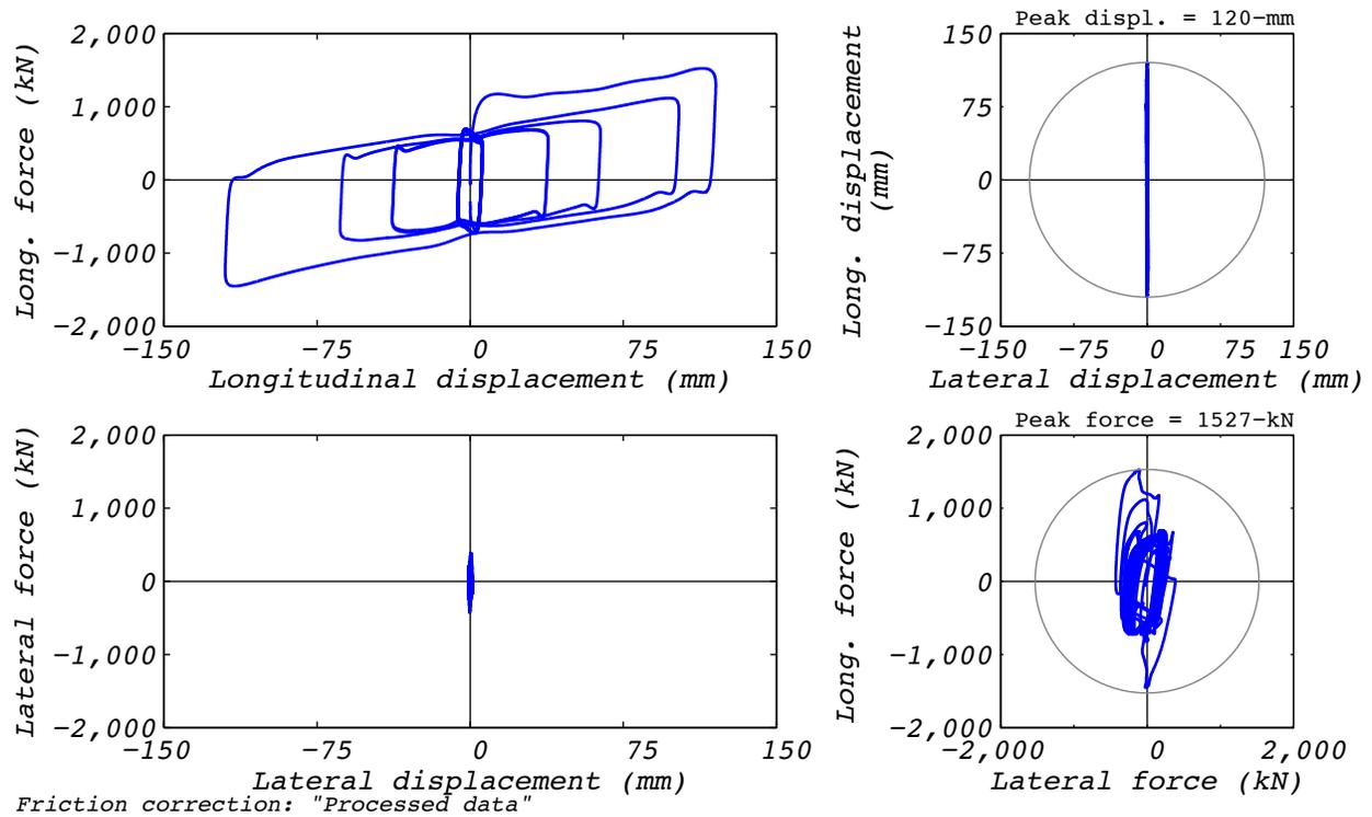
Figure D.29-2 Test run no. 35 hysteresis: Longitudinal (varying amplitude, 8,663 kN axial load, and varying frequency).
