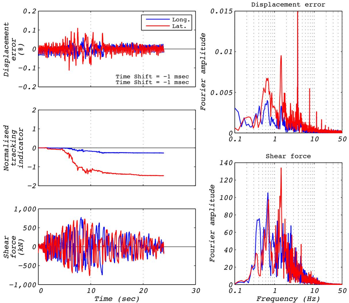
Figure A.10-1 Hybrid test performance metrics for run 45: EUR5, 2D with experimental bearing representing all bearings.
