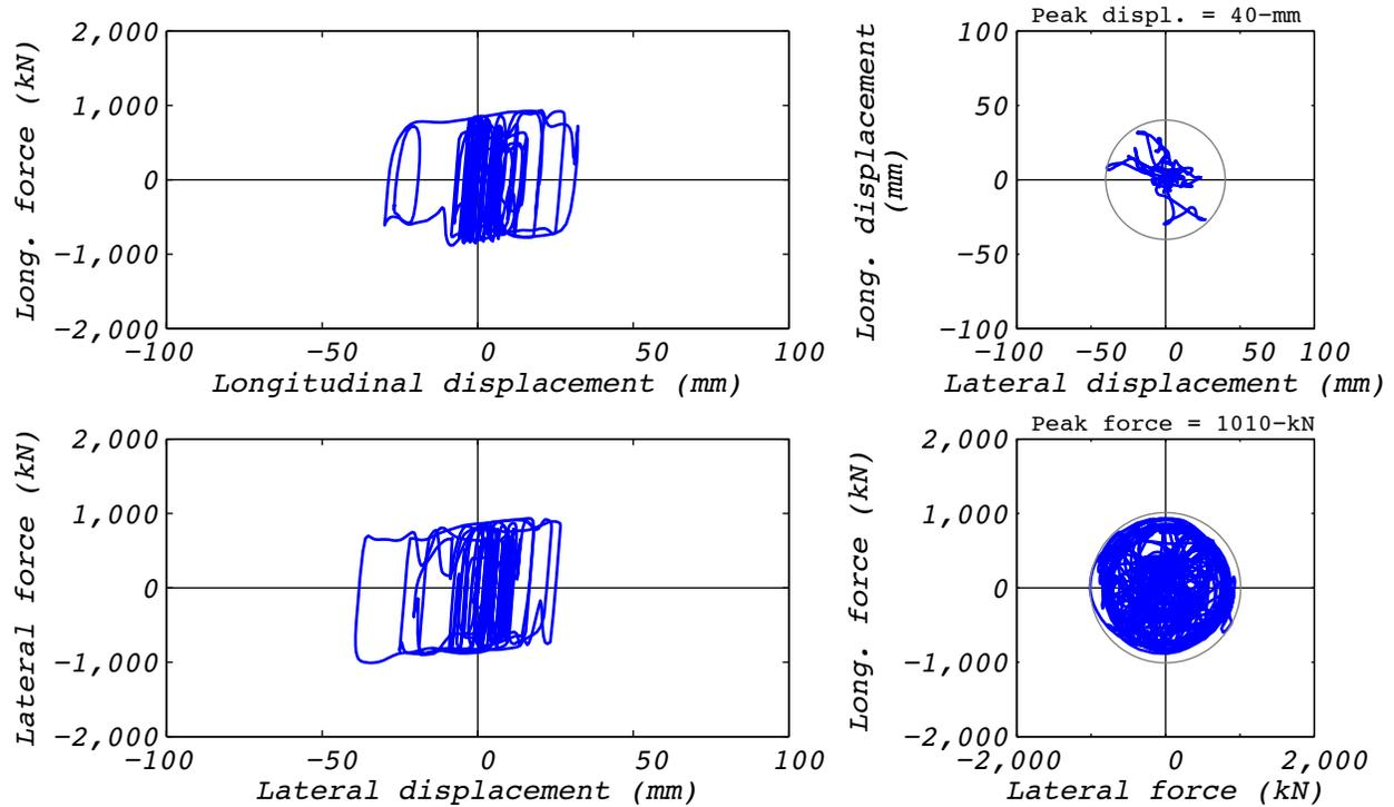
Figure C.3-1 Analytical bearing response for run 18A: EUR5, 2D with a single analytical bearing.
