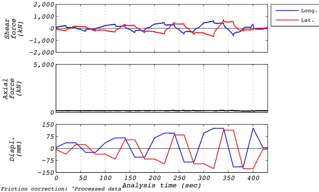
Figure D.23-1 Test run no. 29 time history: Square orbit (Varying amplitude, 178 kN axial load, and varying velocity).
