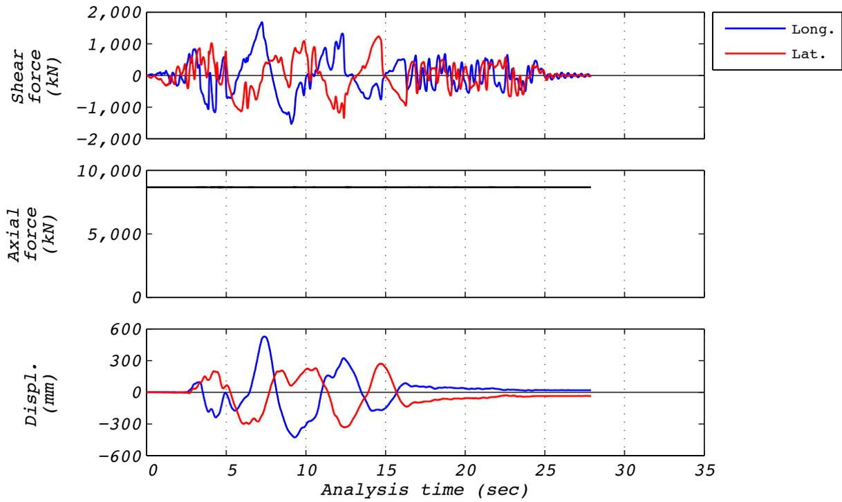
**Figure A.16-2 Analytical time history responses for run 55A: NRC15, 2D with a single analytical bearing.**
