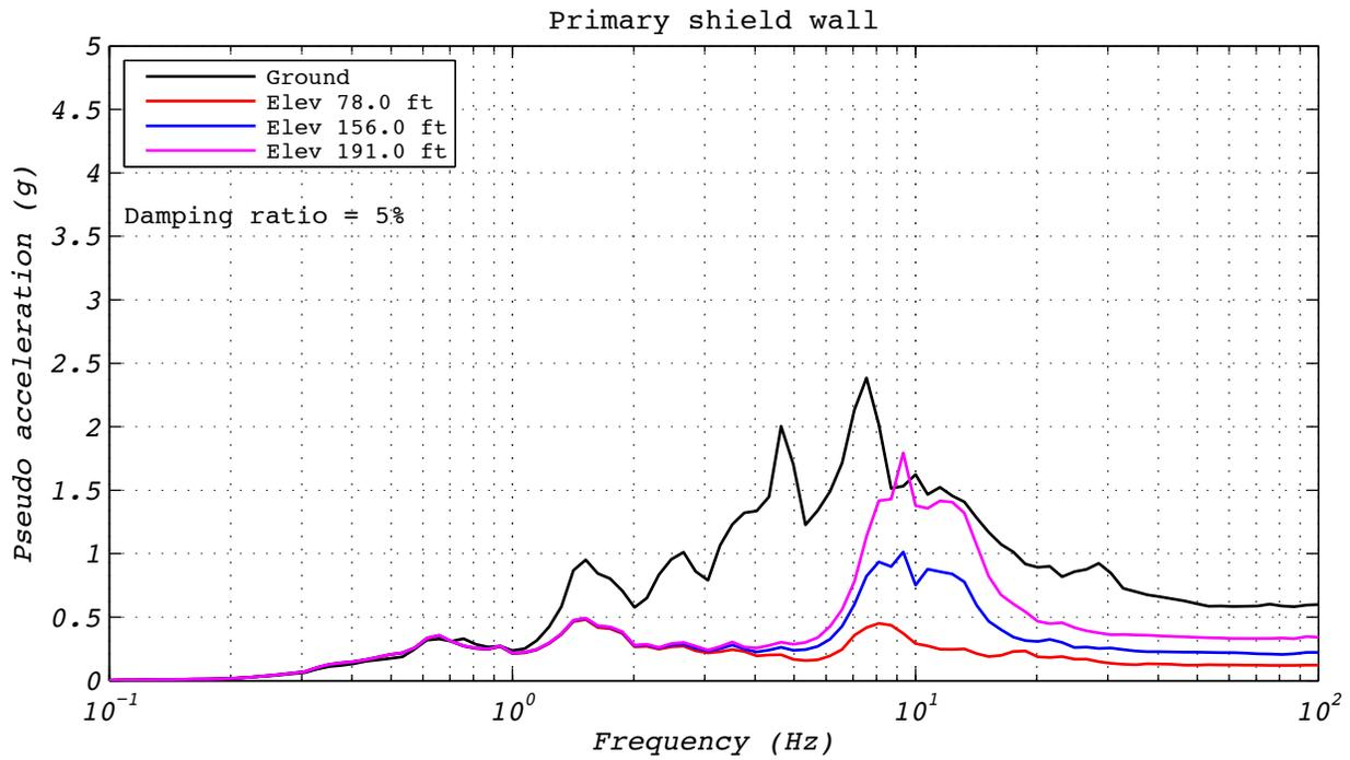
**Figure A.10-4 Hybrid test floor spectra for run 45: EUR5, 2D with experimental bearing representing all bearings.**
