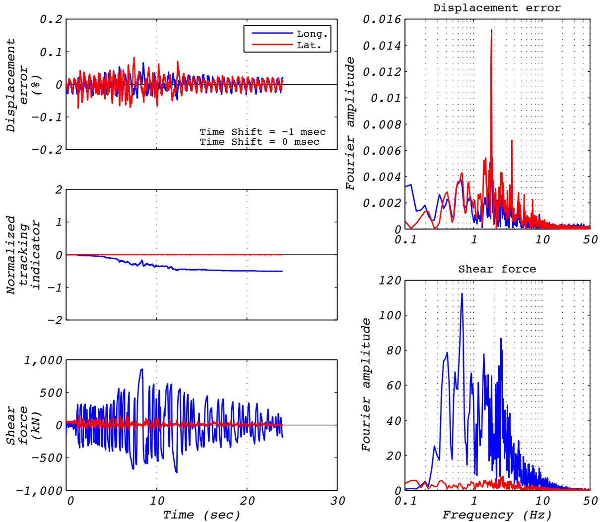
Figure A.8-1 Hybrid test performance metrics for run 44: EUR5, 1D with experimental bearing representing all bearings.
