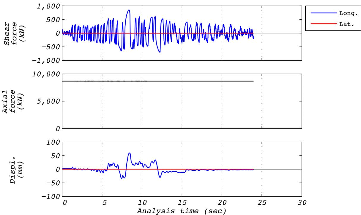
**Figure A.6-3 Hybrid test time history responses for run 42: EUR5, 1D with experimental bearing representing all bearings.**
