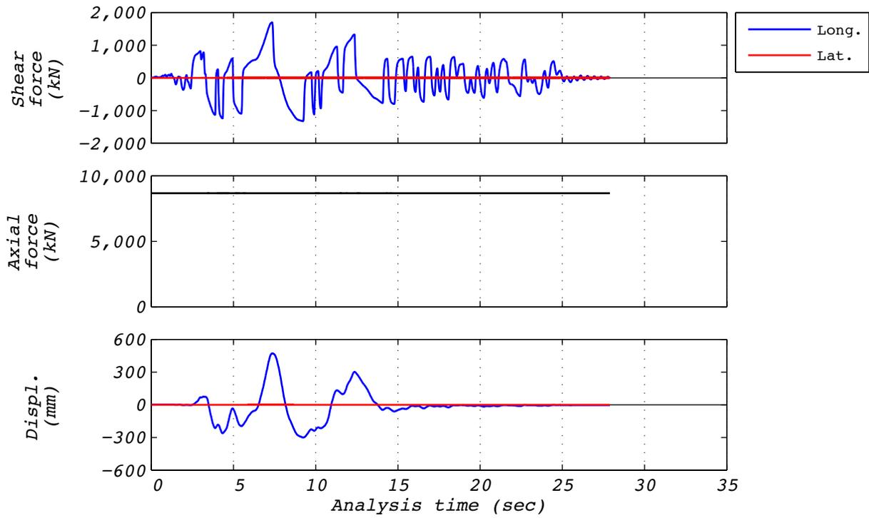
**Figure A.14-2 Analytical time history responses for run 47A: NRC15, 1D with a single analytical bearing.**
