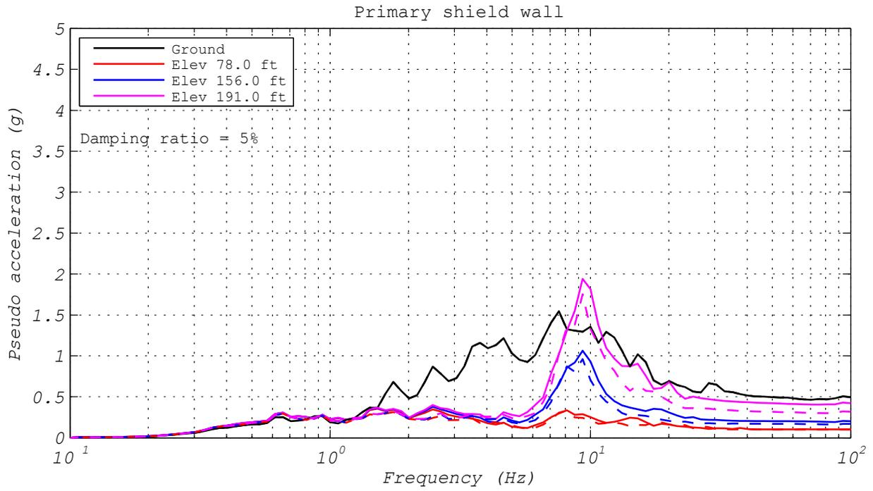
**Figure 3.41** LPRB bearing: response spectra comparison of response to ground motion EUR5 (1D and 2D analyses).
