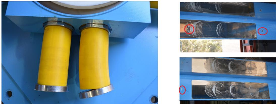
**Figure 3.88 Localized damages in the failed EQS-1 bearing.**
