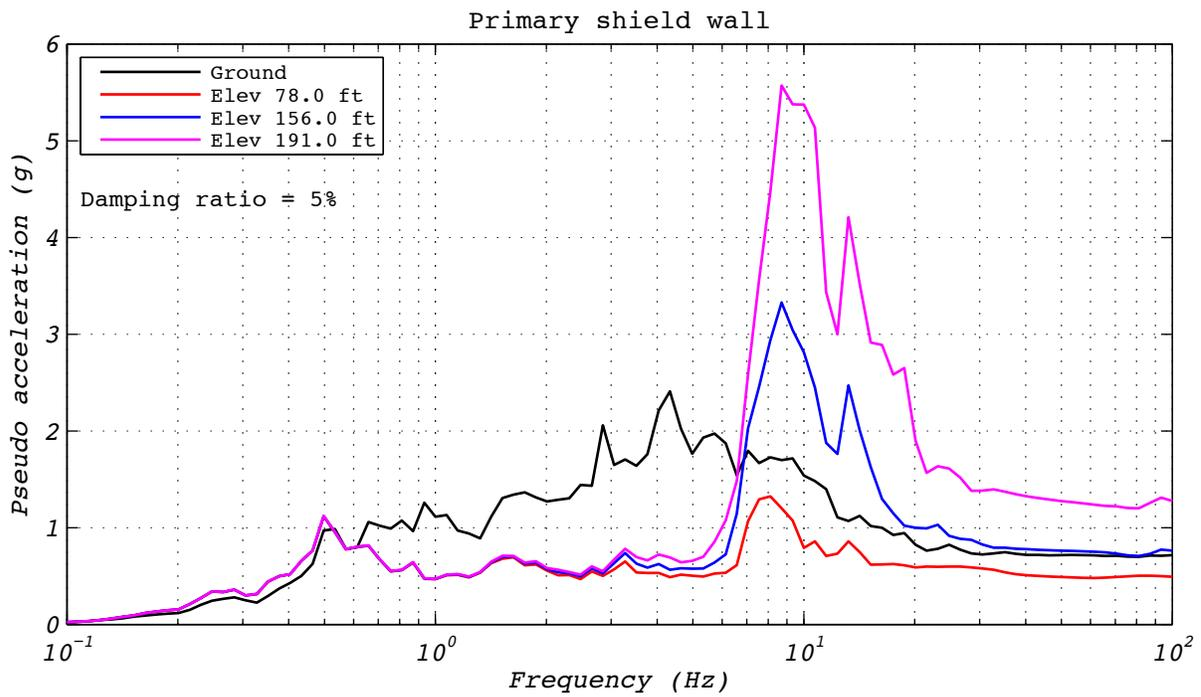
**Figure C.24-4 Hybrid test floor spectra for run 58: NRC10, 2D with experimental bearing representing all bearings.**
