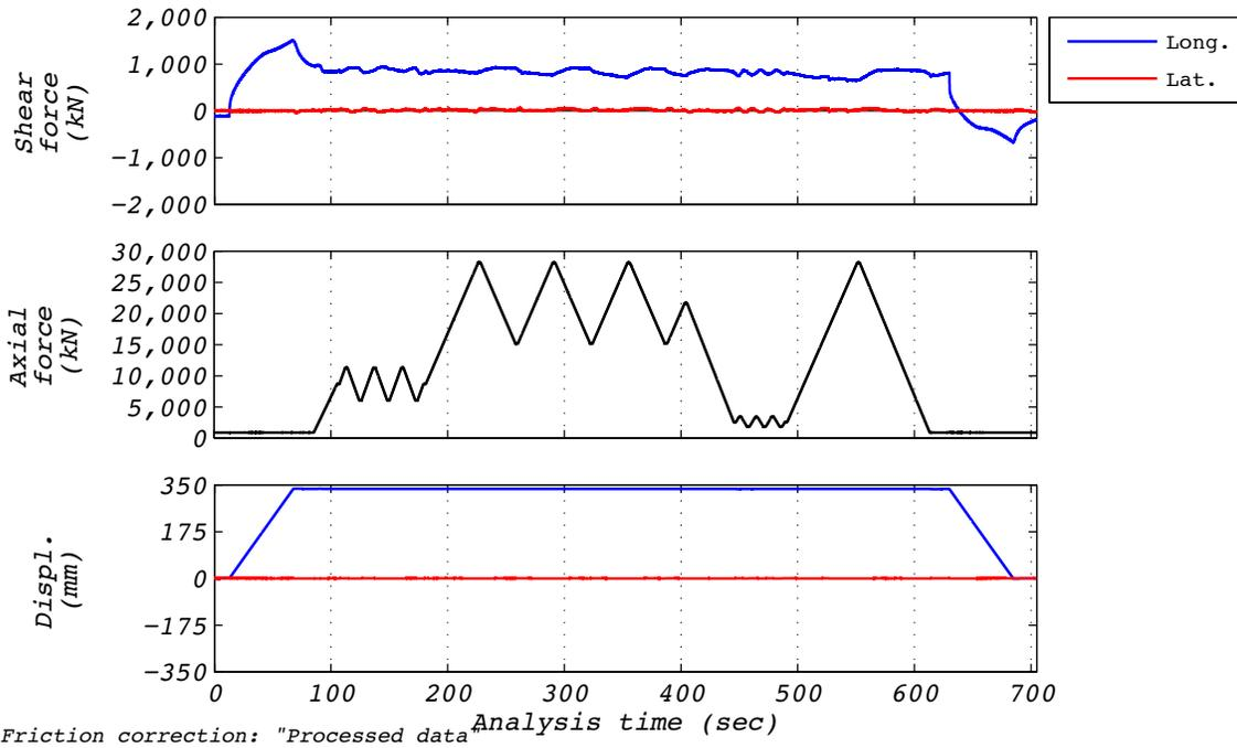
Figure B.9-1 Test run no. 18 time history: Axial (336 mm amplitude and varying axial load).
