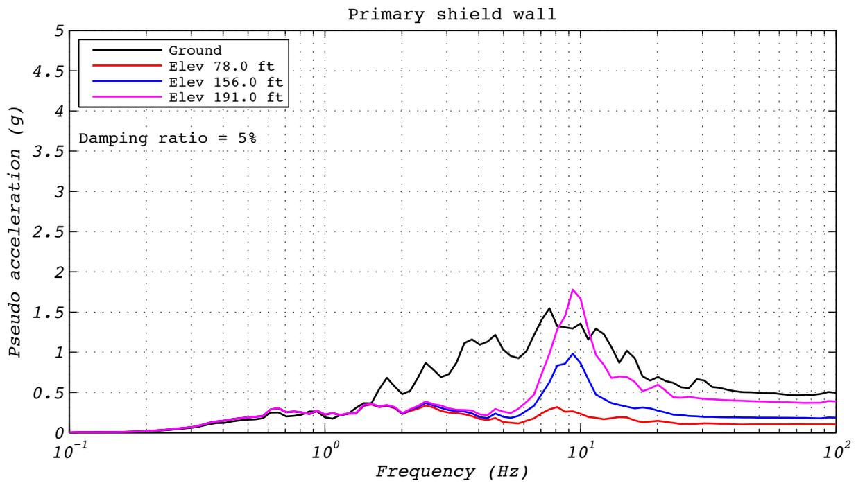
**Figure A.7-4 Hybrid test floor spectra for run 43: EUR5, 1D with experimental bearing representing all bearings.**
