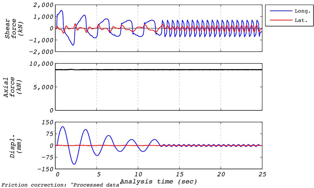
Figure D.29-1 Test run no. 35 time history: Longitudinal (varying amplitude, 8,663 kN axial load, and varying frequency).
