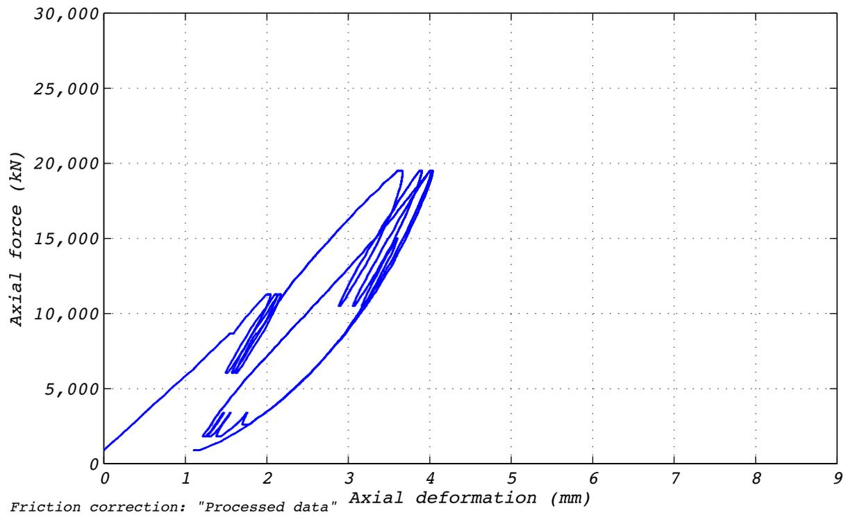
Figure D.25-2 Test run no. 31 hysteresis: Axial (0 mm amplitude and varying axial load).
