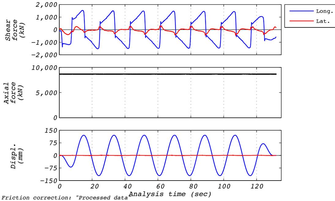
Figure D.15-1 Test run no. 15 time history: Longitudinal (120 mm amplitude, 8,663 kN axial load, and 41 mm/s velocity).
