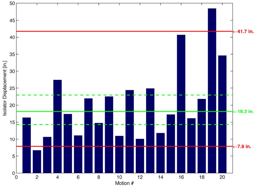
**Figure 3.34** Analytically determined peak lateral displacement demands for the NRC hazard level [1973] based on an FPSB isolator (green lines = median with 95% confidence interval, red lines = 5<sup>th</sup> and 95<sup>th</sup> percentile).
