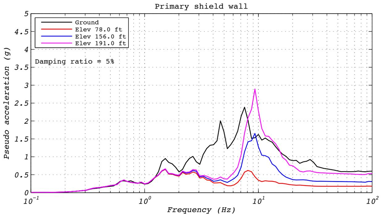
**Figure A.4 Hybrid test floor spectra for run 24: EUR5, 2D with experimental bearing representing all bearings.**
