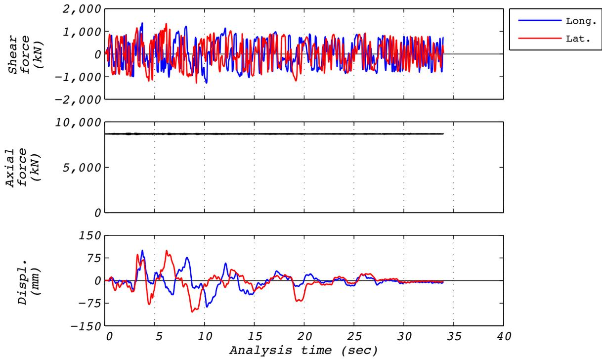
**Figure C.21-2 Analytical time history responses for run 54A: NRC2, 2D with a single analytical bearing.**
