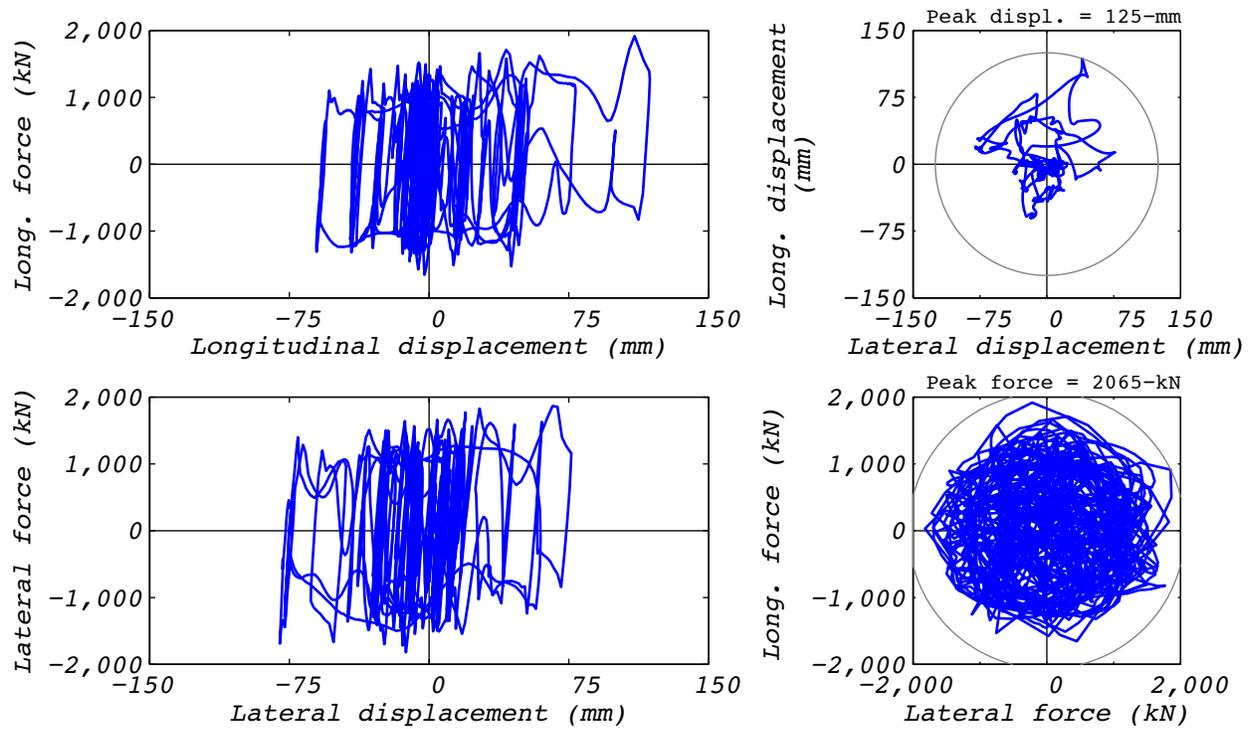
**Figure C.5-2 Hybrid test bearing response for run 21: NRC2, 2D with experimental bearing representing all bearings.**
