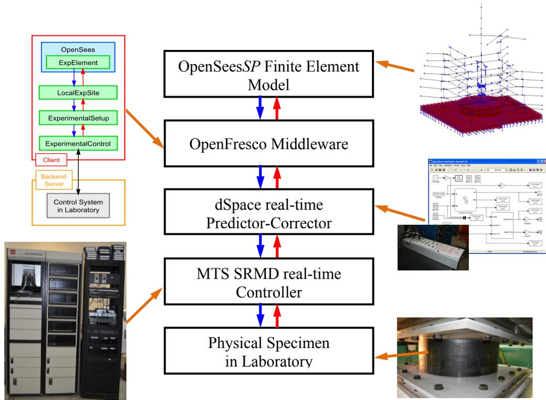
Figure 3.16 Schematic of the test set-up.
