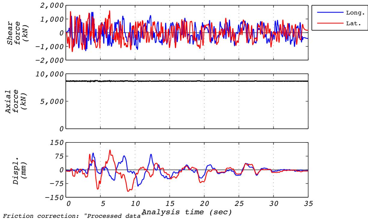
**Figure C.23-2 Time history responses for real-time reproduction of hybrid test run 54: NRC2, 2D with experimental bearing representing all bearings.**
