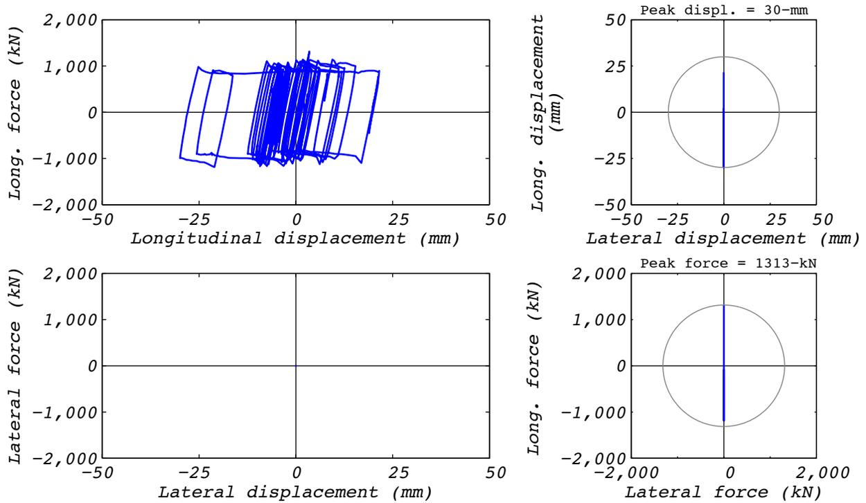
**Figure C.1-2 Hybrid test bearing response for run 17: EUR5, 1D with experimental bearing representing all bearings.**
