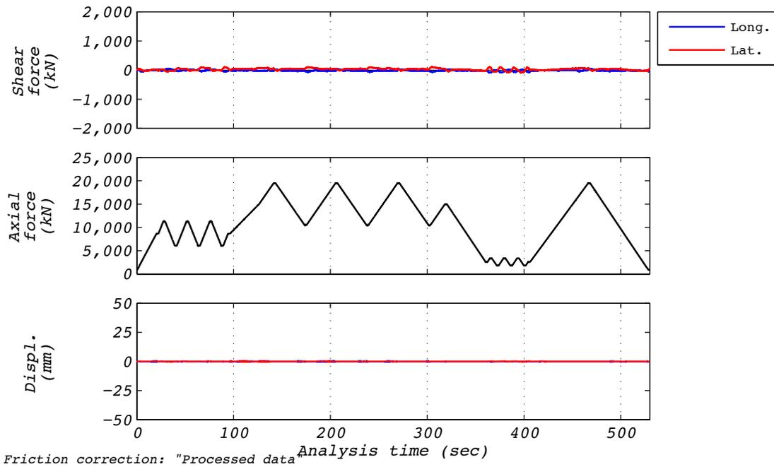
Figure D.25-1 Test run no. 31 time history: Axial (0 mm amplitude and varying axial load).
