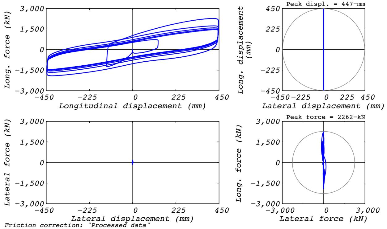
**Figure A.28-1 Bearing response for real-time displacement history from hybrid test run 84: NRC15, 3D with 5 groups of bearings and the experimental bearing representing the center group.**
