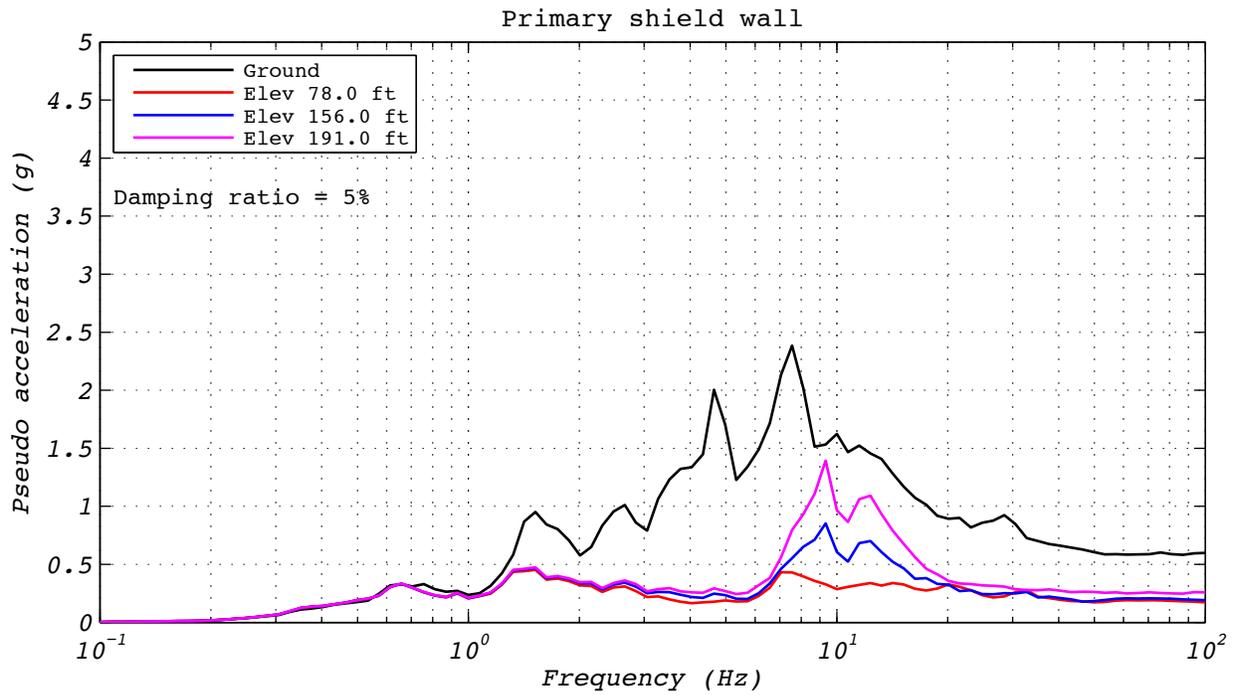
**Figure A.23-4 Hybrid test floor spectra for run 80: EUR5, 3D with 5 groups of bearings and the experimental bearing representing the center group.**
