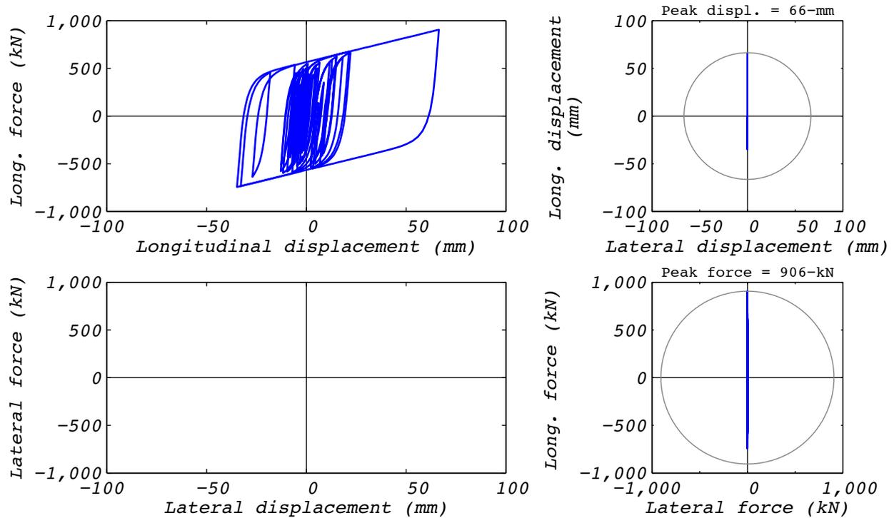
Figure A.9-1 Analytical bearing response for run 44A: EUR5, 1D with a single analytical bearing.
