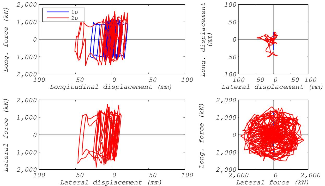
Figure 3.60 EQS bearing: comparison of bearing responses to ground motion EUR5 executed 25 times slower than real time(1D and 2D analyses).
