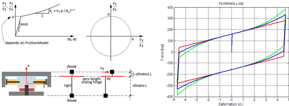
Figure 3.20 New EQS isolator element in OpenSees.
