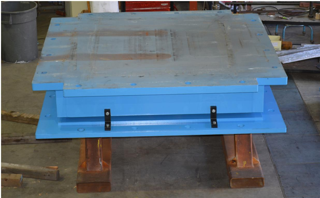
**Figure 3.27** ESCO RTS bearing pre-test condition.
