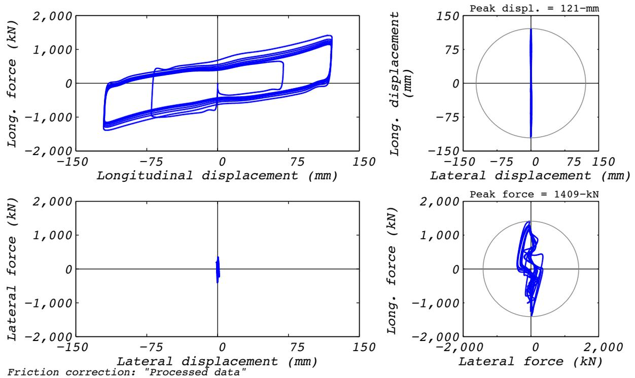
**Figure D.12-2 Test run no. 12 hysteresis: Longitudinal (120 mm amplitude, 2,500 kN axial load, and 410 mm/s velocity).**
