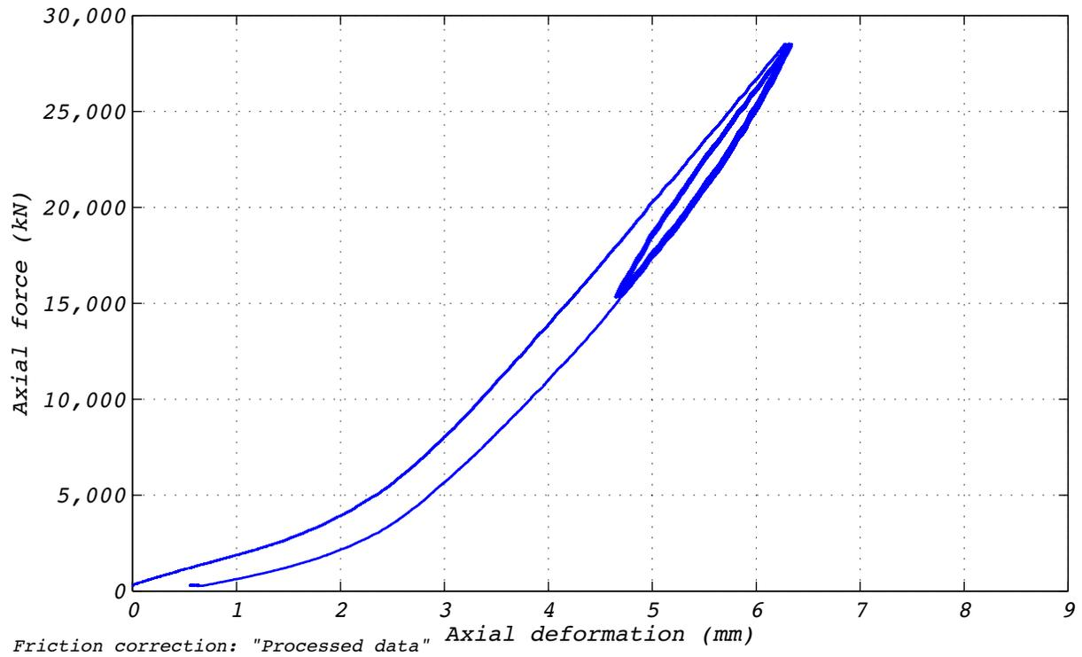
Figure B.25-2 Test run no. 68 hysteresis: Axial (0 mm amplitude, varying axial load).
