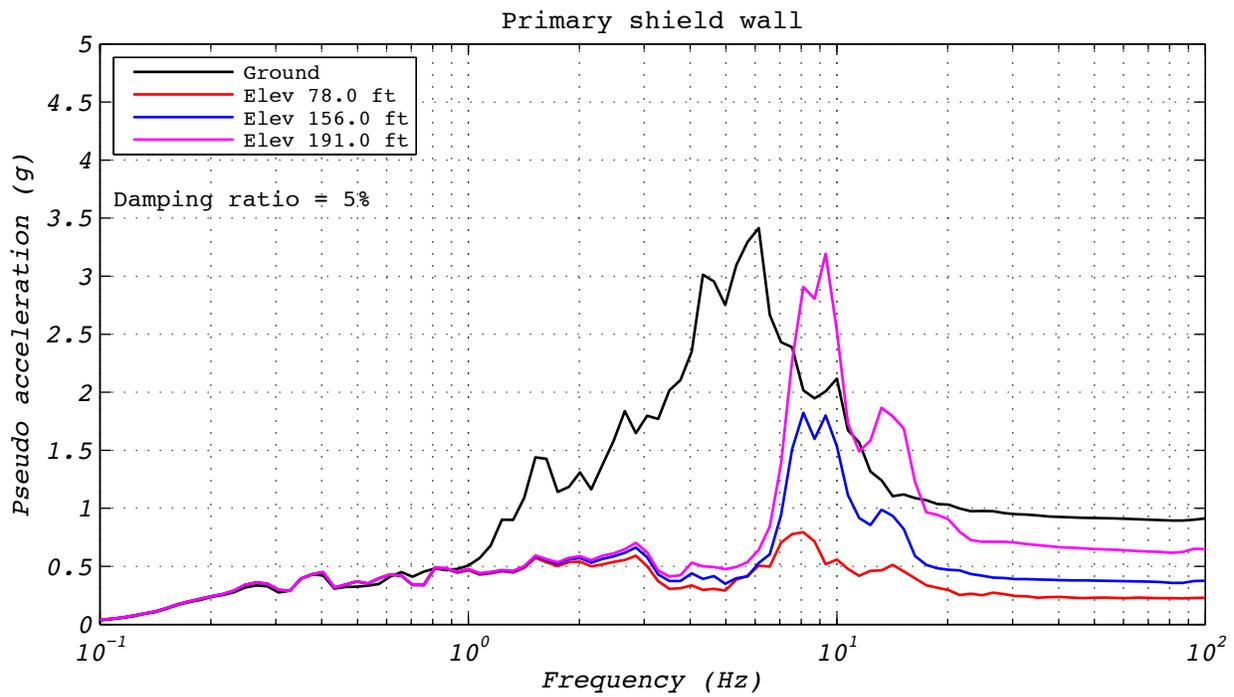
**Figure C.8-4 Hybrid test floor spectra for run 43: NRC2, 3D with 5 groups of bearings and the experimental bearing representing the center group.**
