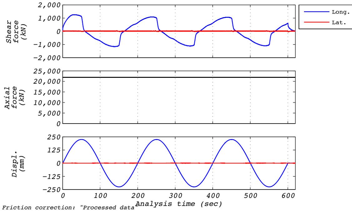
Figure B.12-1 Test run no. 41 time history: Longitudinal (224 mm amplitude, 8,663 kN axial load, and 7 mm/s velocity).
