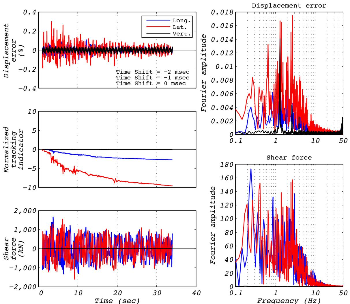
Figure C.10-1 Hybrid test performance metrics for run 46: NRC2, 3D with 5 groups of bearings and the experimental bearing representing the center group.
