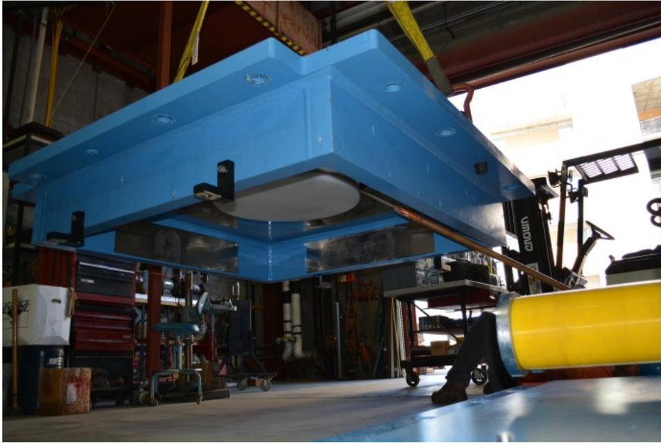
**Figure 3.90** Bonding between sliding surface and sliding pad for EQS-2 bearing with a pry-bar unable to separate the two.
