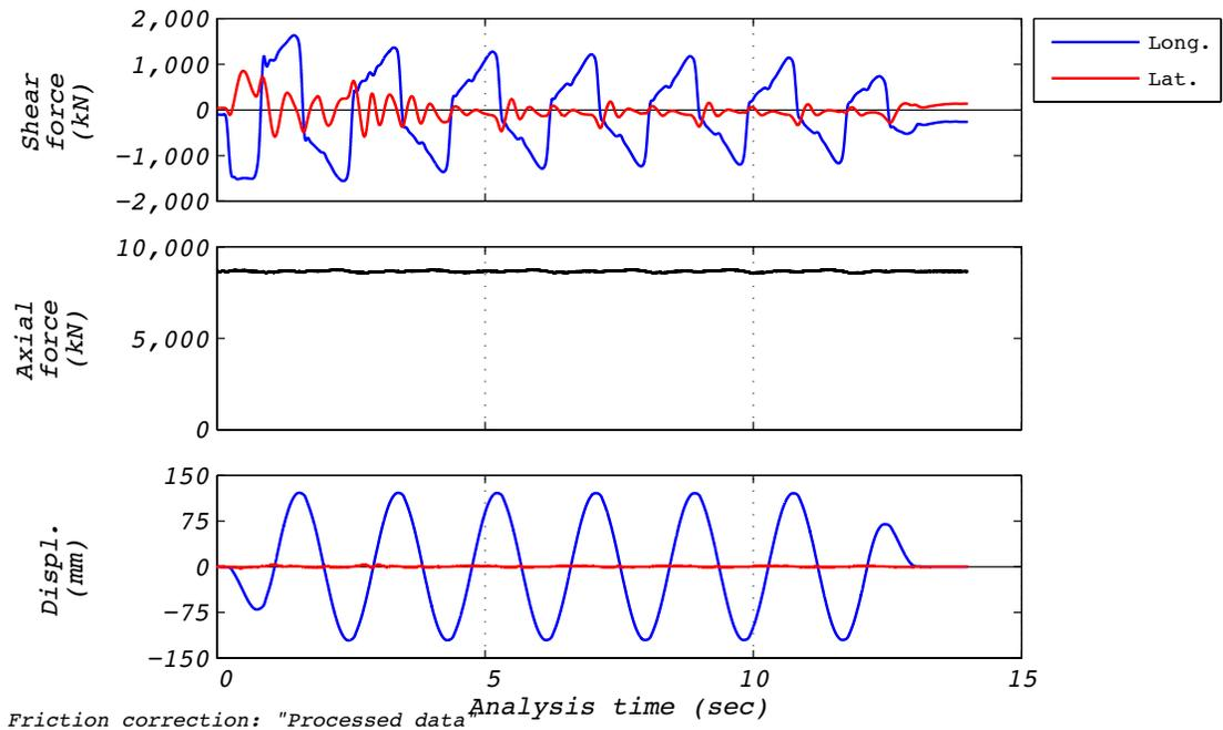
Figure D.18-1 Test run no. 24 time history: Longitudinal (120 mm amplitude, 8,663 kN axial load, and 410 mm/s velocity).
