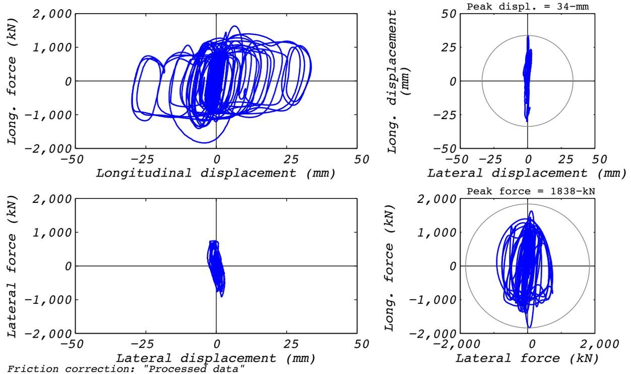
**Figure C.22-1 Bearing response for real-time reproduction of hybrid test run 53: EUR5, 1D with experimental bearing representing all bearings.**
