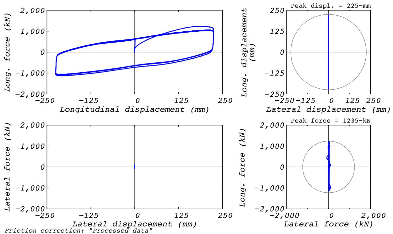
Figure B.17-2 Test run no. 56 hysteresis: Longitudinal (224 mm amplitude, 8,663 kN axial load, and 7 mm/s velocity).
