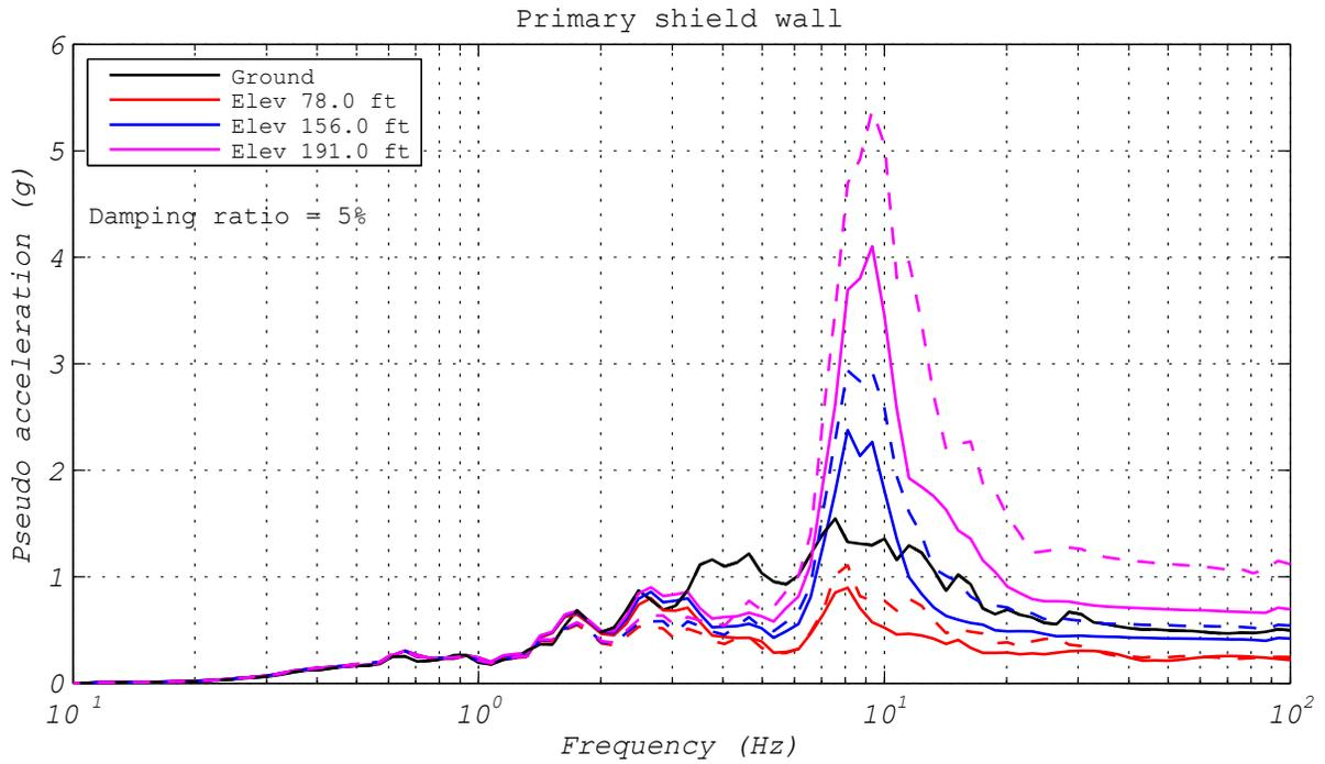
**Figure 3.73** EQS bearing: response spectra comparison of responses to loading rates (ground motion EUR5, 1D analysis).
