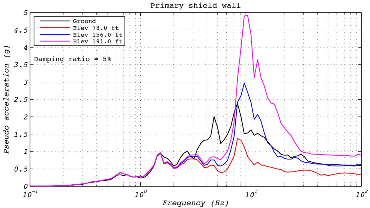
**Figure C.2-4 Hybrid test floor spectra for run 18: EUR5, 2D with experimental bearing representing all bearings.**
