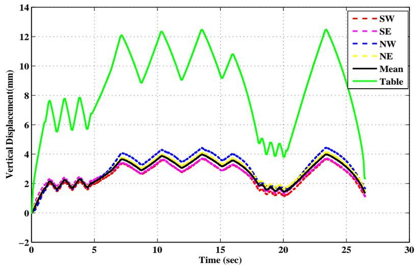
Figure 3.22 Vertical displacement of the SRMD and LVDTs.
