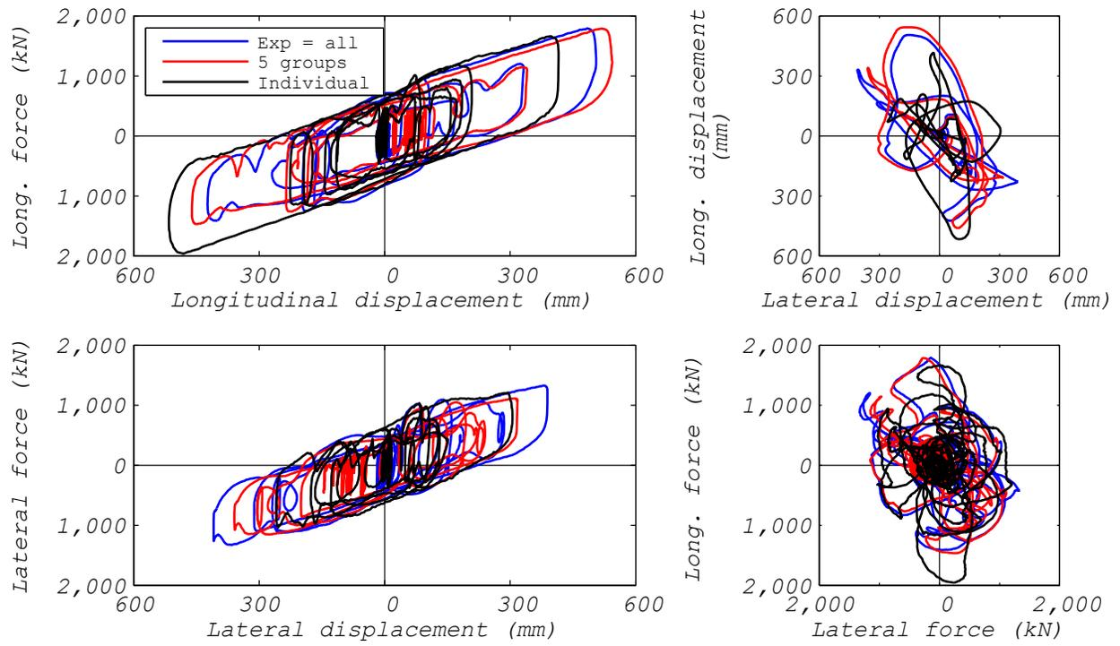
**Figure 3.50** LPRB bearing: comparison of bearing responses to bearing layout discretization (ground motion NRC15, 2D analysis).
