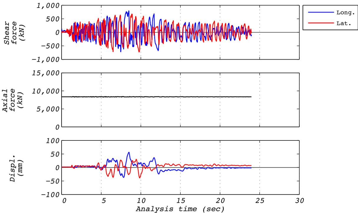
**Figure A.24-3 Hybrid test time history responses for run 82: EUR5, 3D with 5 groups of bearings and the experimental bearing representing the center group.**
