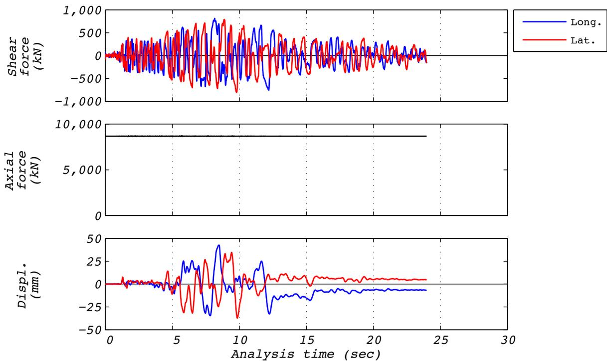
**Figure A.3-3 Hybrid test time history responses for run 26: EUR5, 2D with experimental bearing representing all bearings.**
