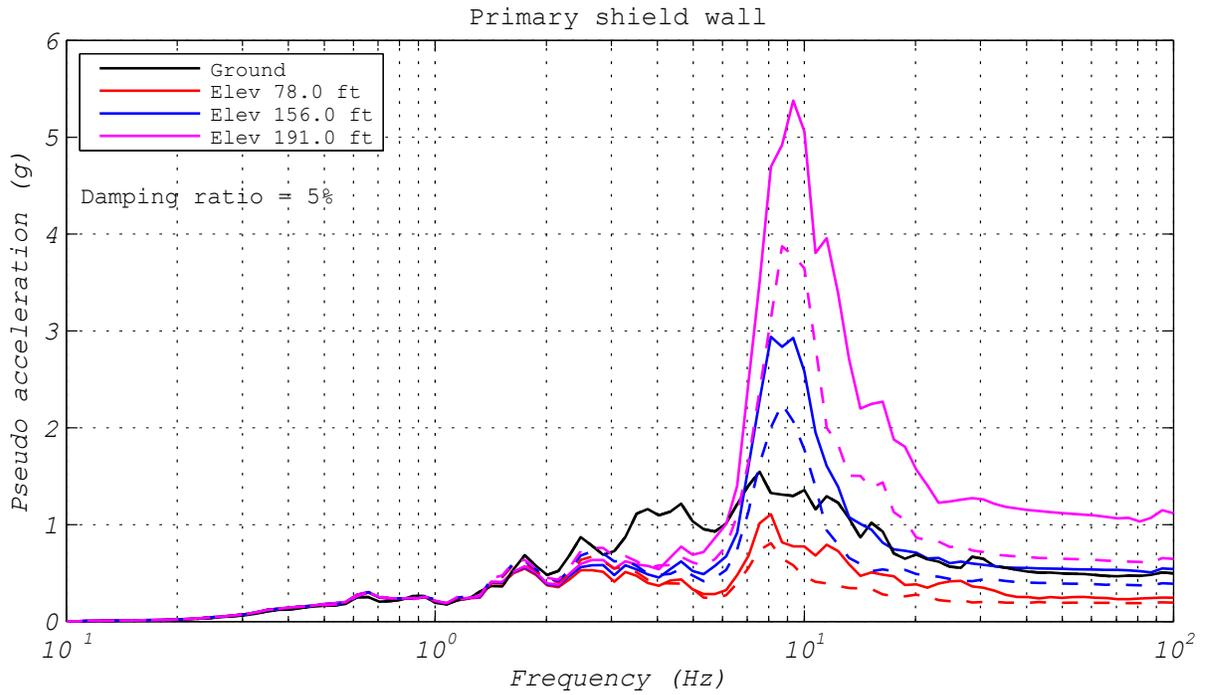
**Figure 3.77** EQS bearing: response spectra comparison of hybrid simulation and analytical estimation responses (ground motion EUR5, 1D analysis).
