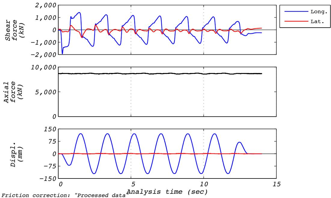
Figure D.20-1 Test run no. 26 time history: Longitudinal (120 mm amplitude, 8,663 kN axial load, and 410 mm/s velocity).
