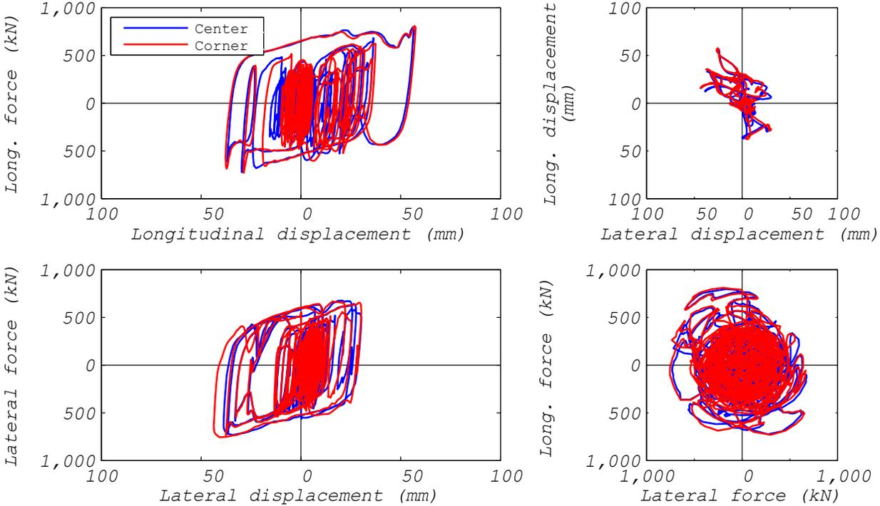
**Figure 3.46** LPRB bearing: comparison of bearing responses depending on the location of the bearing (ground motion EUR5, 3D analysis).
