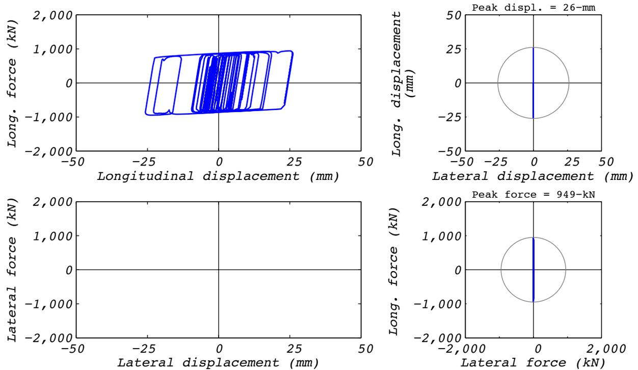
Figure C.19-1 Analytical bearing response for run 53A: EUR5, 1D with a single analytical bearing.
