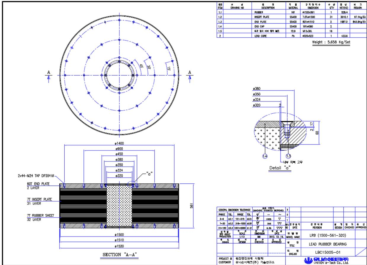
Figure 2.1 LPRB manufacturing specifications (courtesy of Unison eTech).
