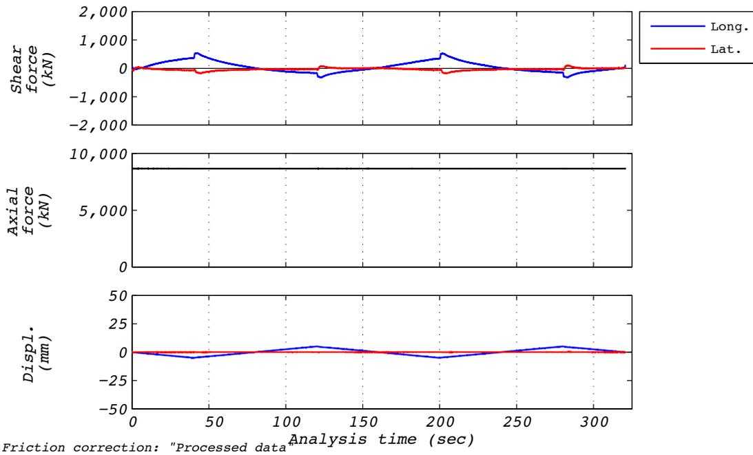
Figure D.6-1 Test run no. 6 time history: Transverse rotation (0 mm displacement and 8,663 kN axial load).
