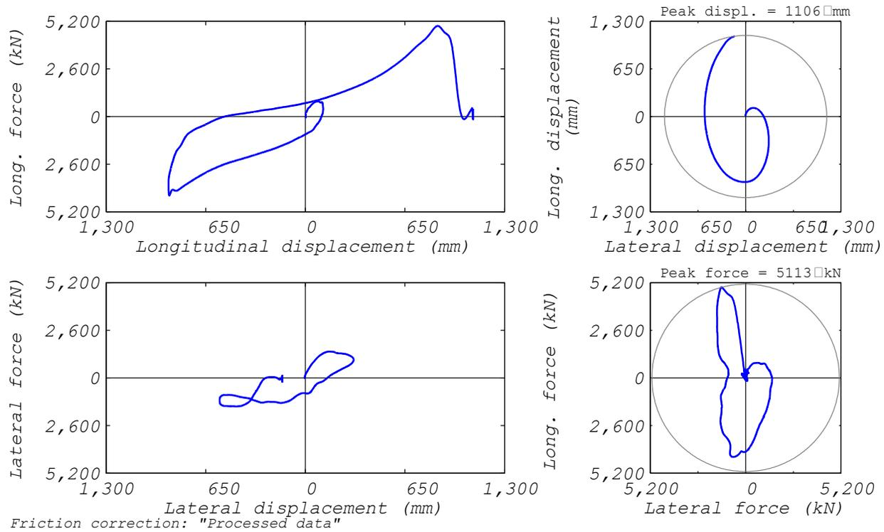
**Figure 3.85 Bearing response during failure test (UET-2): Run 66 with 8663 kN axial load.**
