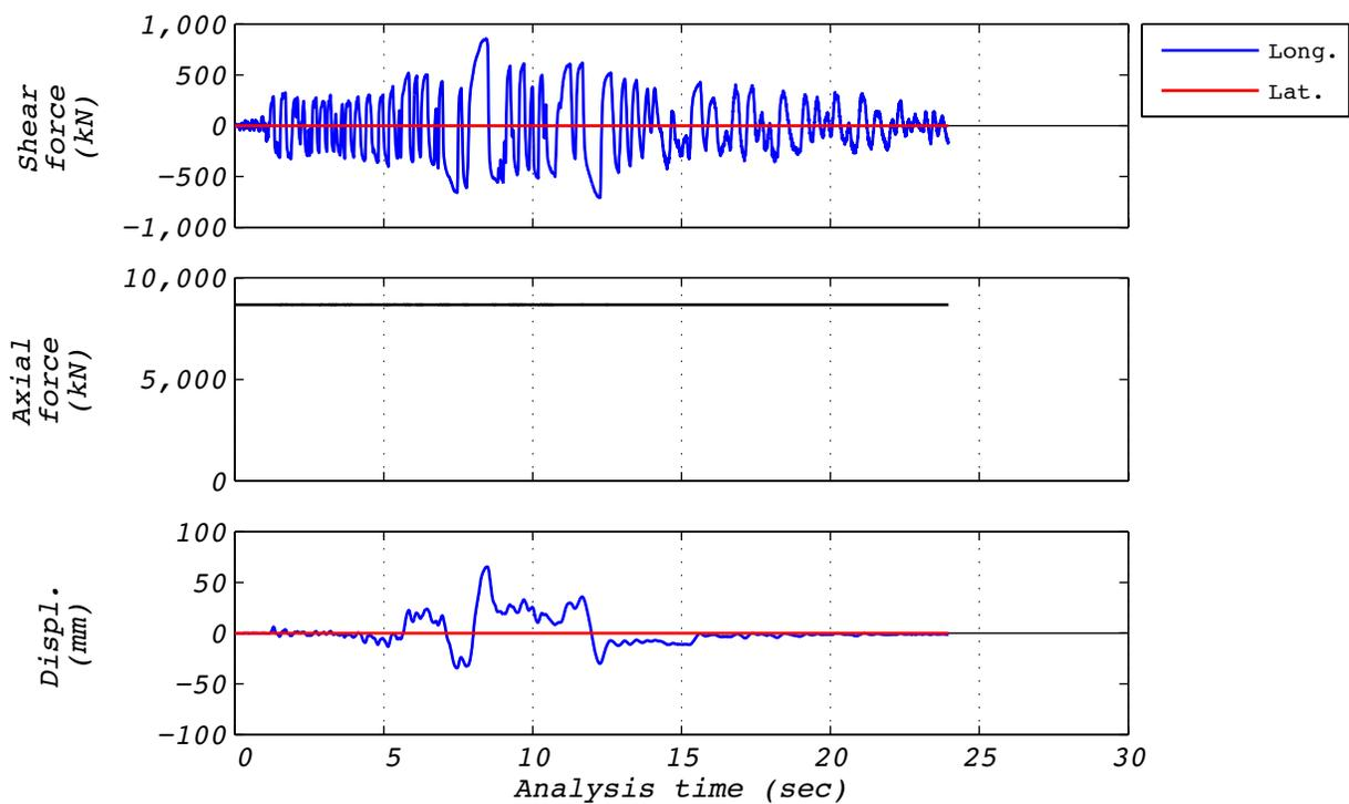
**Figure A.4-3 Hybrid test bearing response for run 37: EUR5, 1D with experimental bearing representing all bearings.**
