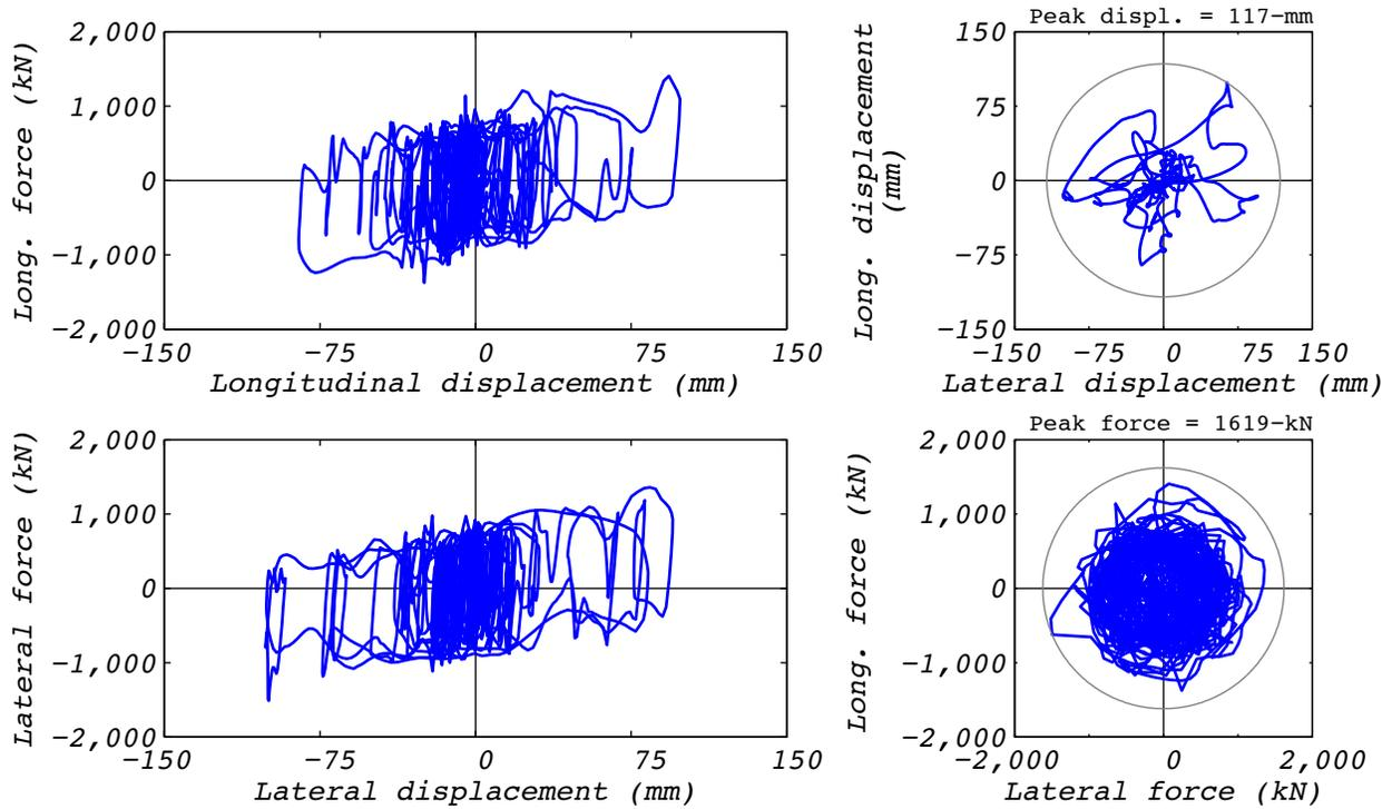
**Figure C.13-2 Hybrid test bearing response for run 49: NRC2, 3D with 5 groups and the experimental bearing representing the no. 3 corner group.**
