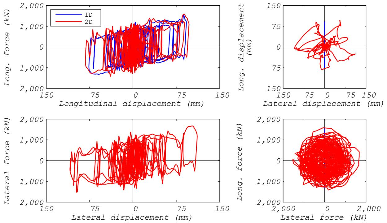
**Figure 3.64** EQS bearing: comparison of bearing responses to ground motion NRC2 executed five times slower than real time (1D and 2D analyses).
