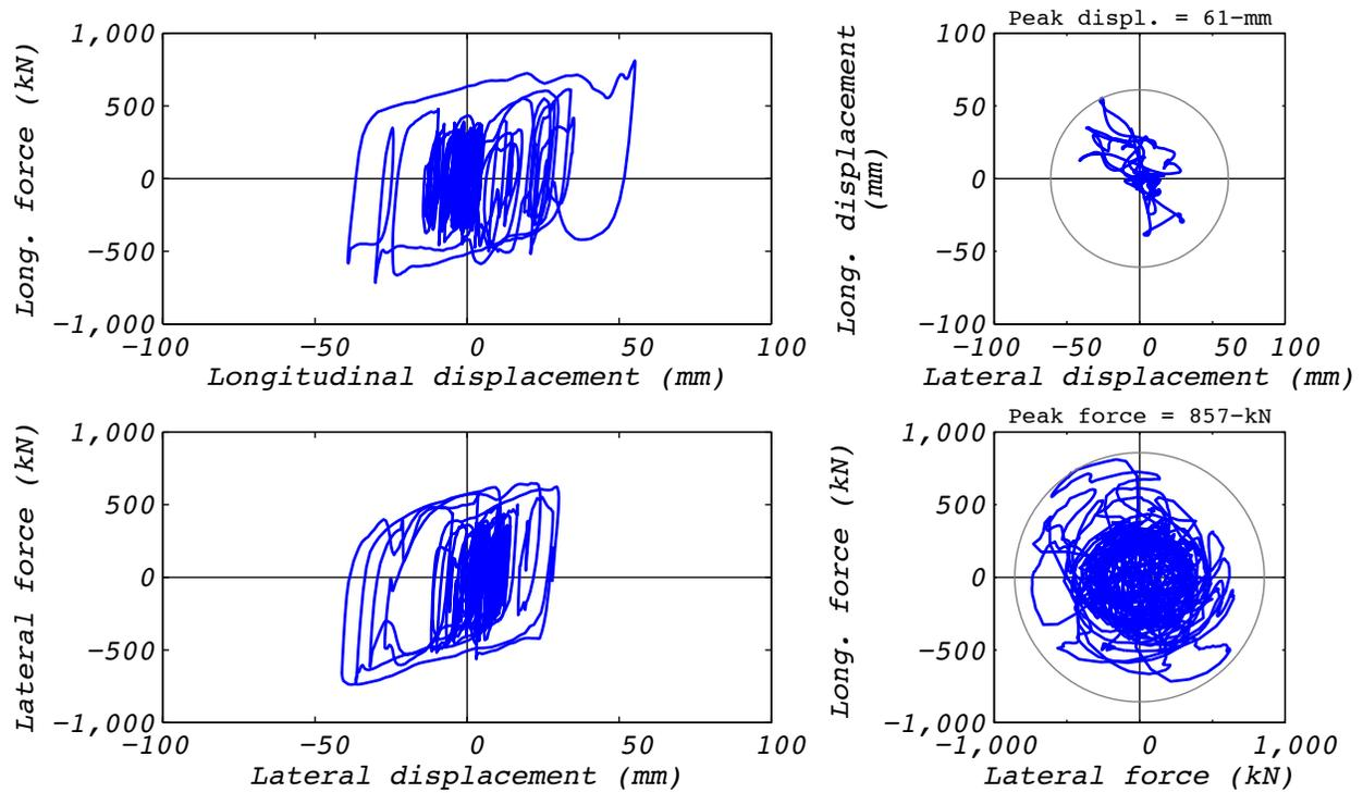
**Figure A.22-2 Hybrid test bearing response for run 79: EUR5, 3D with 5 groups of bearings and the experimental bearing representing the center group.**
