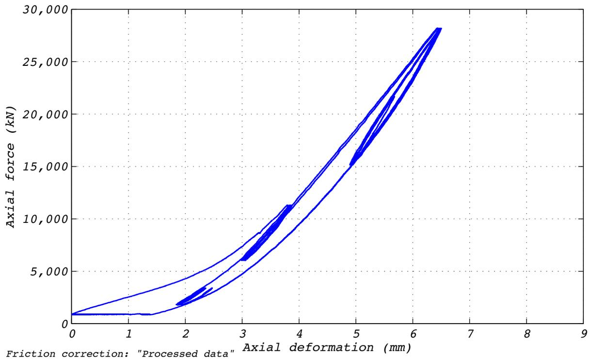
Figure B.7-2 Test run no. 16 hysteresis: Axial (112 mm amplitude and varying axial load).
