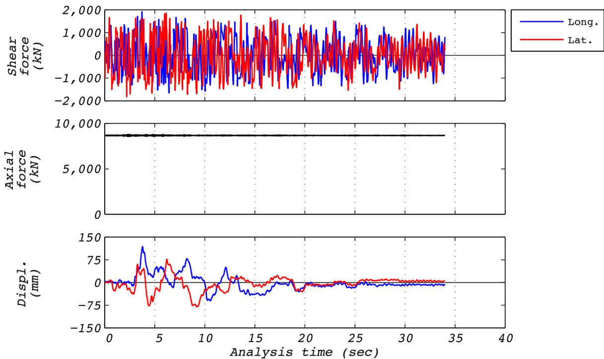
**Figure C.5-3 Hybrid test time history responses for run 21 NRC2, 2D with experimental bearing representing all bearings.**
