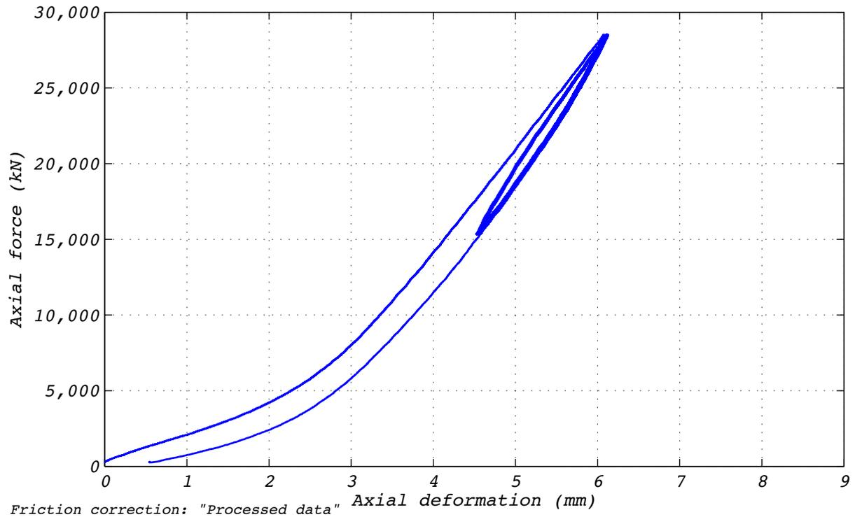
Figure B.4-2 Test run no. 13 hysteresis: Axial (0 mm amplitude and varying axial load).
