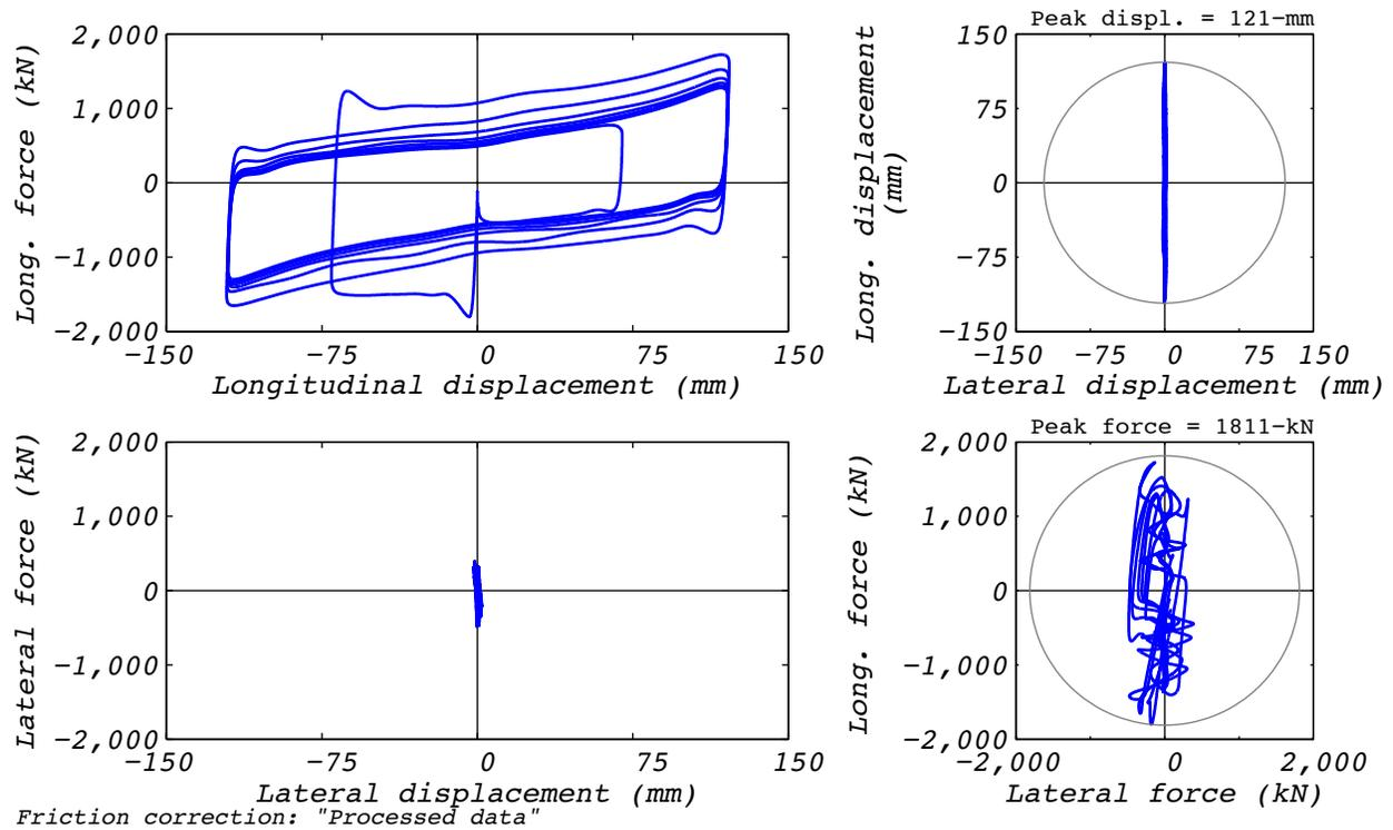
Figure D.14-2 Test run no. 14 hysteresis: Longitudinal (120 mm amplitude, 15,000 kN axial load, and 410 mm/s velocity).
