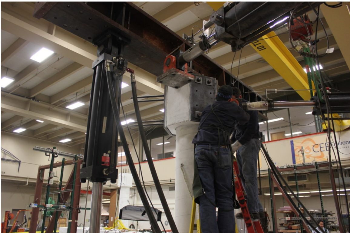
Figure D.12 Attaching the two horizontal actuators to the column head to complete the last step of the test set-up procedure.
