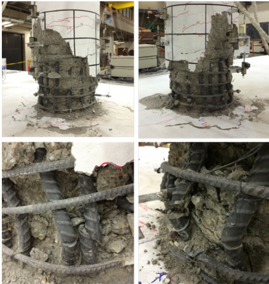
Figure 5.6 Final damaged state of the as-built Specimen No. 1 column: all the rebar were exposed and buckled, and six rebar ruptured.
