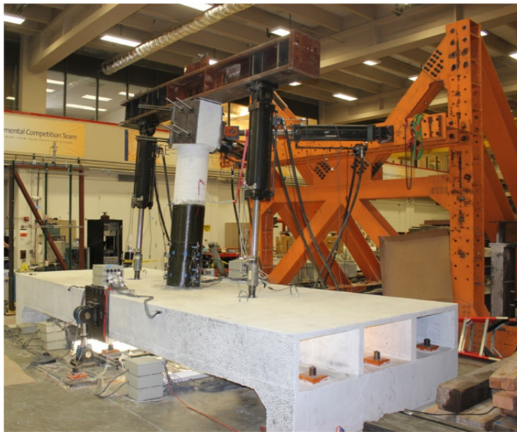
Figure 6.12 Overview of repaired Specimen No. 1 cyclic loading test set-up when loading is in progress and applied in transverse direction.
