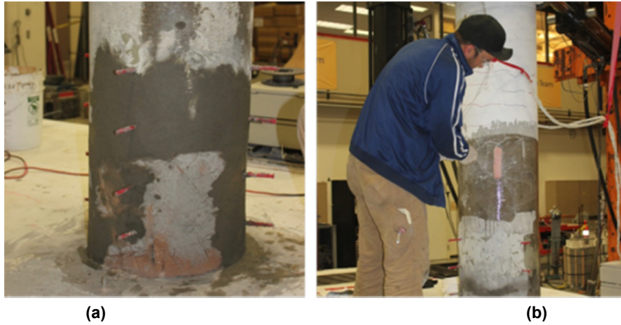
Figure 6.9 (a) A final layer of high strength mortar was applied to patch any remaining voids; and (b) applying a primer epoxy coat to the surface before applying the CFRP sheets.
