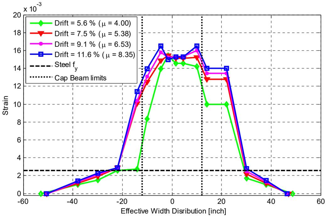
**Figure 3.67** Strain distribution in the tension side at Section B for the four large-scale transverse direction only HS test runs at the positive loading peak (expressed in terms of drift ratio and  $\mu$ ).
