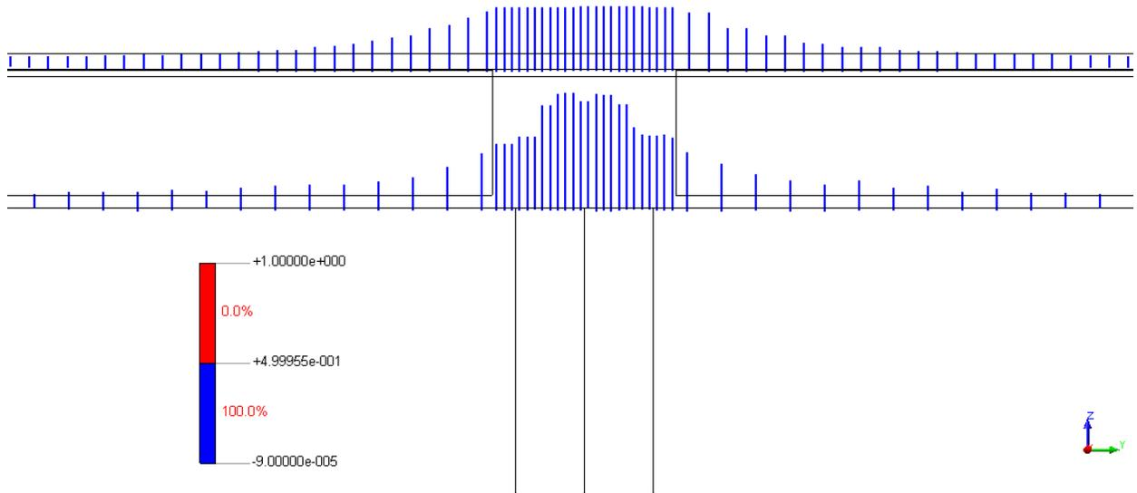
**Figure 5.4** Side view of the tensile strain distribution in the bent cap beam and the adjacent slab transverse reinforcement under combined vertical and lateral loading for bridge 1 (identified in Figure 5.1 and Figure 5.2).
