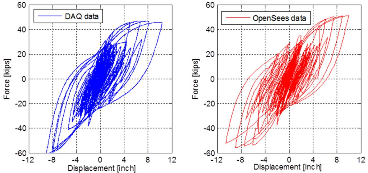
**Figure 3.26** Comparison of force-displacement relationship for all HS test runs as obtained from the observed data acquisition (DAQ) experimental test data and the recorded OpenSees data in the transverse direction.
