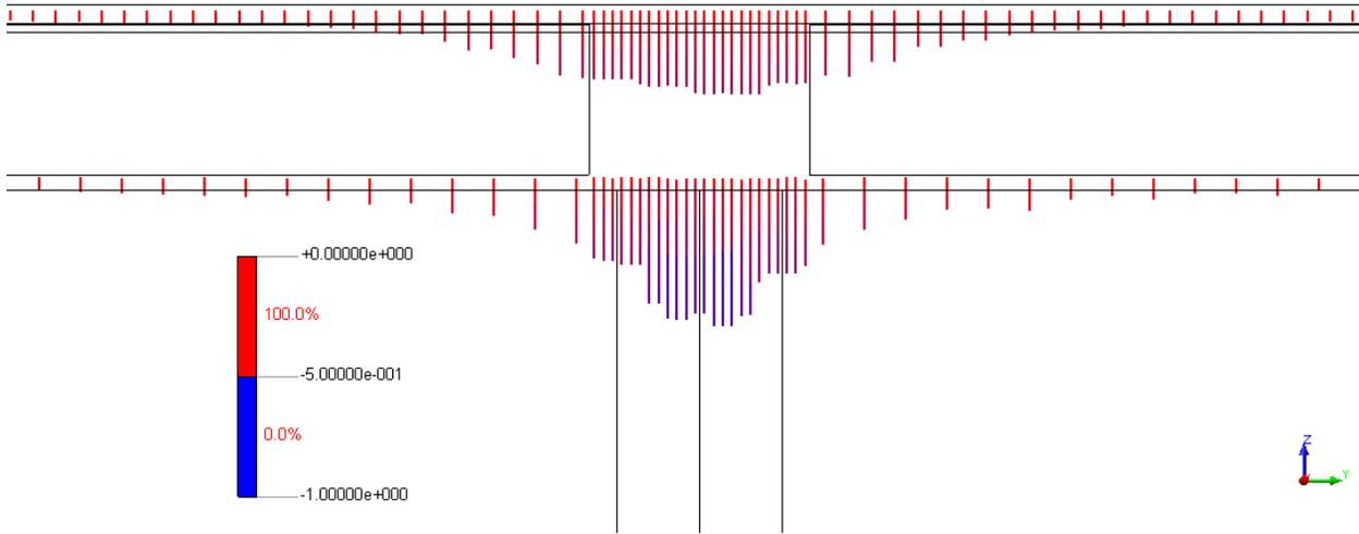
**Figure 5.5** Side view of the compression strain distribution in the bent cap beam and the adjacent slab transverse reinforcement under combined vertical and lateral loading for bridge 1 (identified in Figure 5.1 and Figure 5.2).
