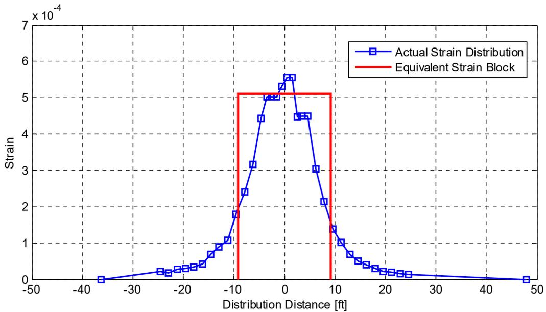
**Figure 5.8** Tensile strain distribution in the bent cap and deck slab transverse reinforcement at Section 2 (identified in Figure 5.2) under combined gravity and lateral transverse load as obtained from DIANA FE linear elastic model.
