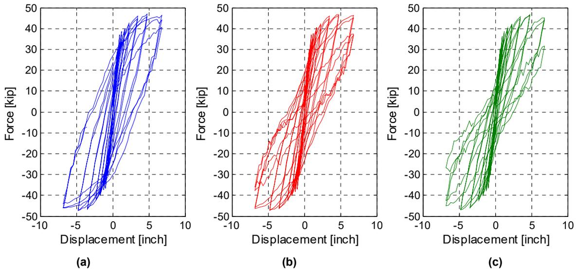
**Figure 4.25** Force-displacement relationships in the longitudinal direction from the calibrated inelastic FE model for three bent cap cases: (a) 8 #5 top and bottom original design; (b) 8 #4 top and bottom design 1; and (c) 8 #3 top and bottom design 2.
