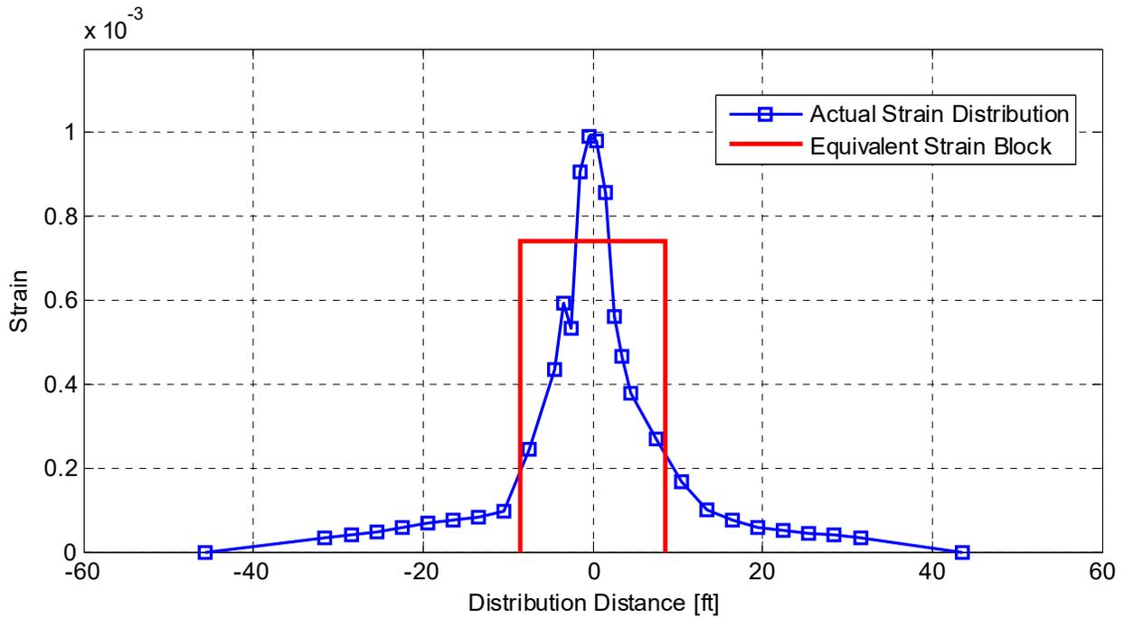
**Figure 5.6** Tensile strain distribution in the bent cap and soffit slab transverse reinforcement at Section 1 (identified in Figure 5.2) under combined gravity and lateral transverse load as obtained from DIANA FE linear elastic model.
