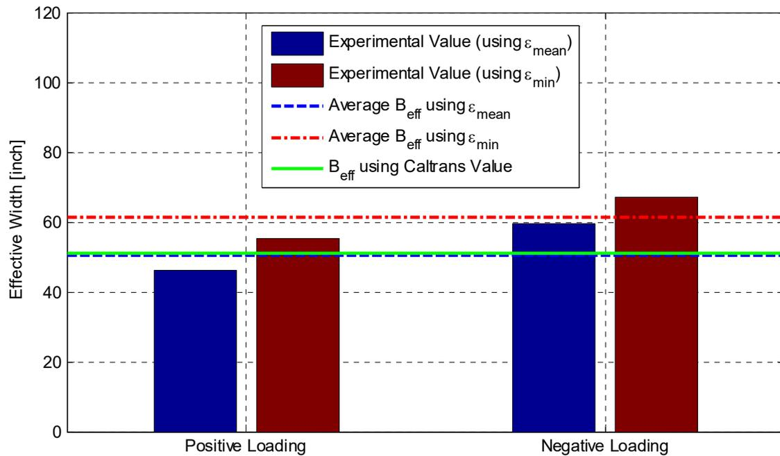
**Figure 3.83 Mean effective width from HS test runs from positive and negative loading (bar chart) and overall average effective width from all HS test runs (dashed lines) at Section D as compared to Caltrans SDC effective width value.**
