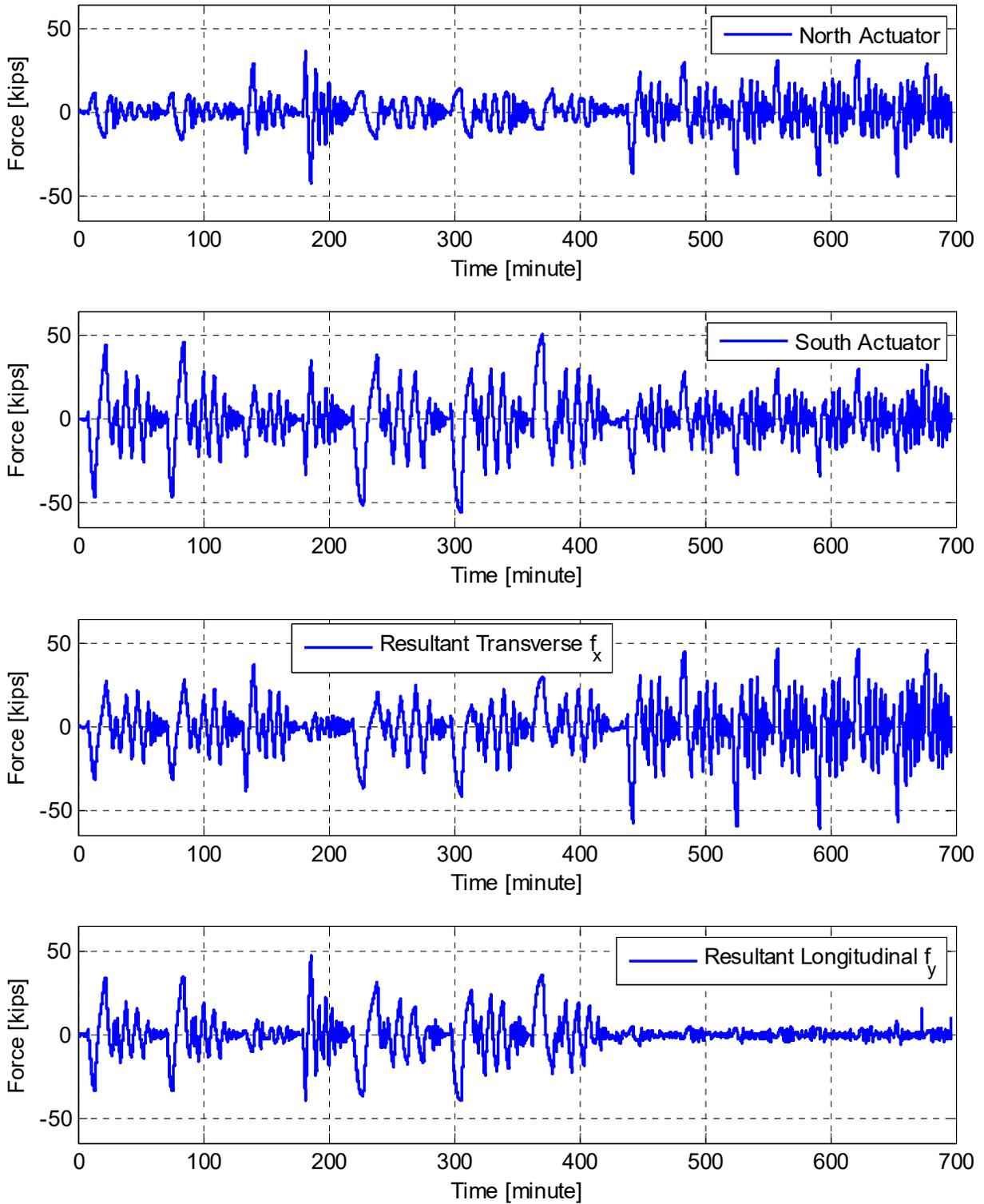
**Figure 3.17** History of north and south lateral actuators load cells measurements and the corresponding resultant forces in the transverse ( $f_x$ ) and the longitudinal ( $f_y$ ) directions for all 15 HS test runs of Specimen No. 2.
