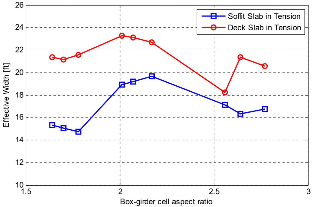
**Figure 5.22** Variation of bent cap effective width in tension at each of the soffit slab (Section 1 in Figure 5.2) and the deck slab (Section 2 in Figure 5.2) with respect to the box-girder cells aspect ratio.
