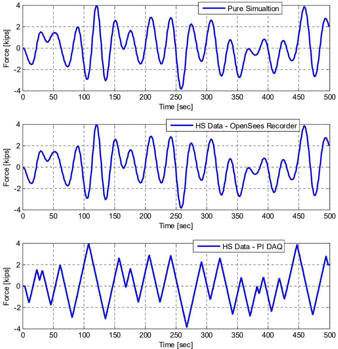
**Figure 2.17 Comparison of the force history obtained from the pure simulation, the received feedback at OpenSees, and multiple of the actual actuator displacement feedback as force as obtained from HS tests using single free actuator.**
