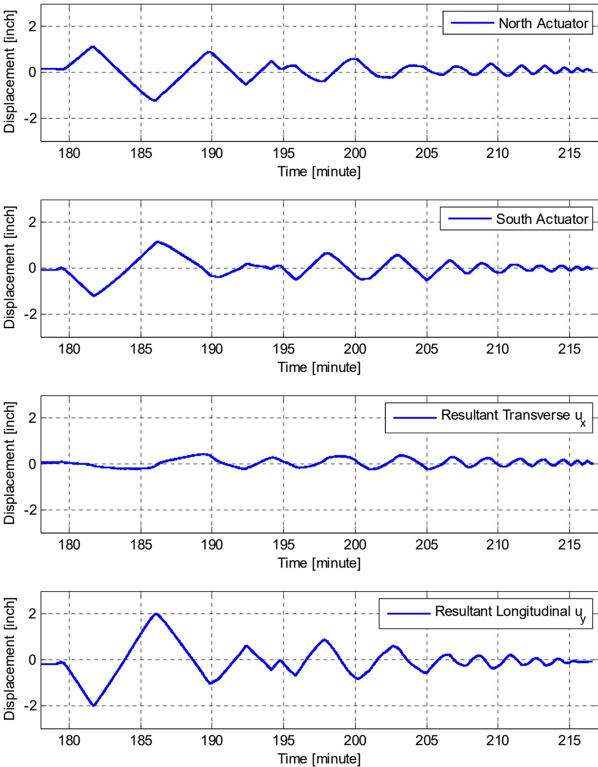
**Figure 3.14** Zoomed-in view of the history of north and south lateral actuators temposonics measurements and the corresponding resultant displacements in transverse ( $u_x$ ) and longitudinal ( $u_y$ ) directions for the 50% scale longitudinal-only HS test.
