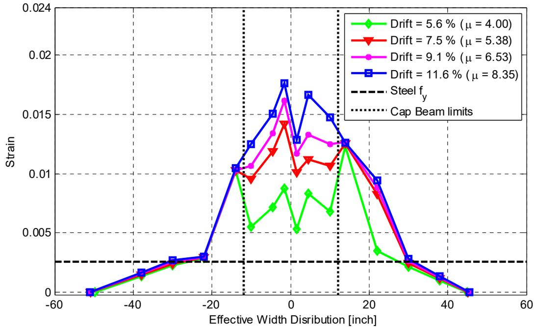
**Figure 3.73** Strain distribution in the tension side at Section D for the four large-scale transverse direction only HS test runs at the positive loading peak (expressed in terms of drift ratio and  $\mu$ ).
