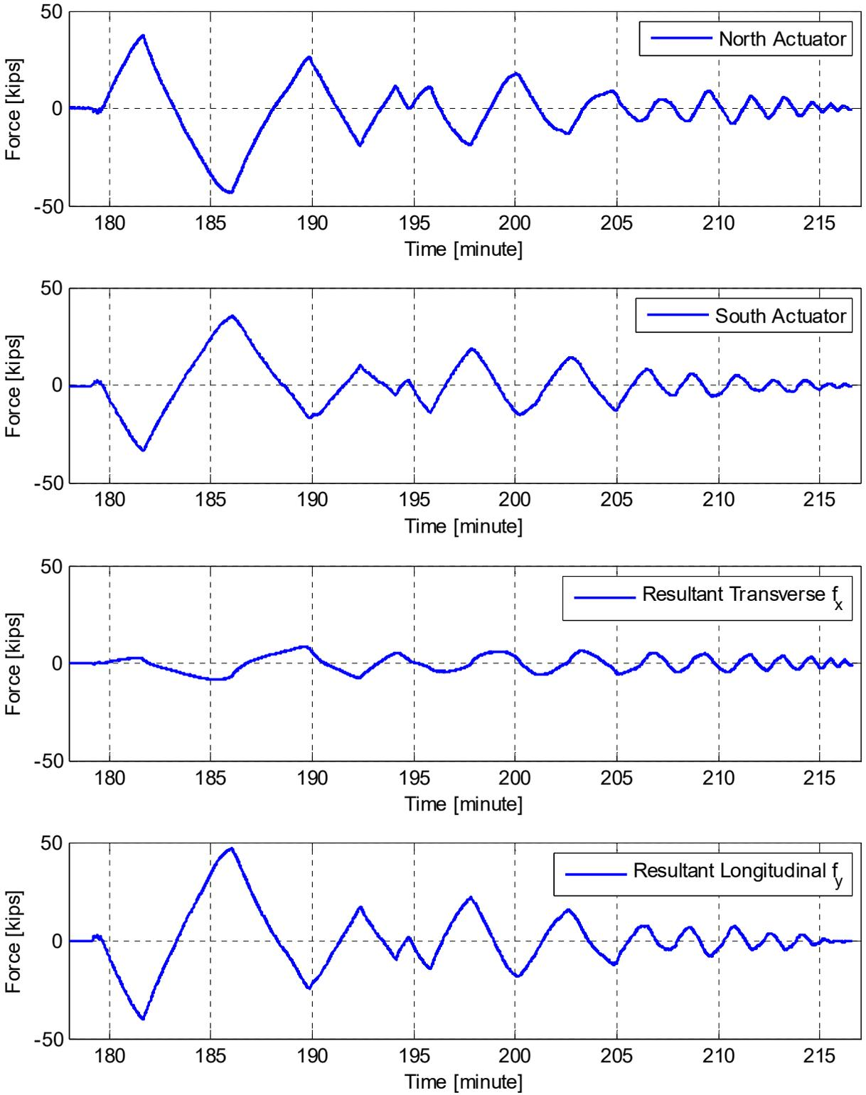
**Figure 3.20** Zoomed-in view of the history of north and south lateral actuators load cells measurements and the corresponding resultant forces in the transverse ( $f_x$ ) and the longitudinal ( $f_y$ ) directions for the 50%-scale longitudinal direction only HS test.
