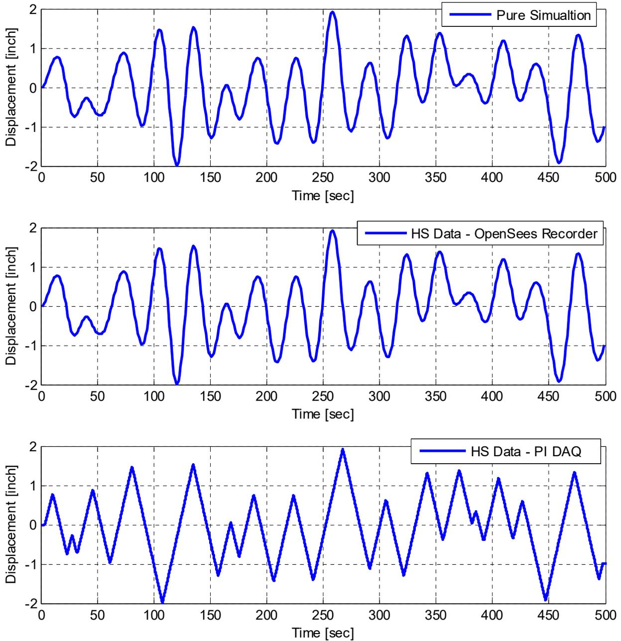
**Figure 2.16 Comparison of the displacement history obtained from the pure simulation, the computed OpenSees command for HS, and the actual actuators motion obtained from HS tests using single free actuator.**
