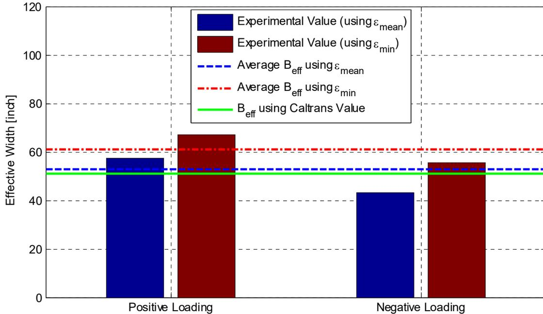
**Figure 3.79** Mean effective width from HS test runs from positive and negative loading (bar chart) and overall average effective width from all HS test runs (dashed lines) at Section B as compared to Caltrans SDC effective width value.
