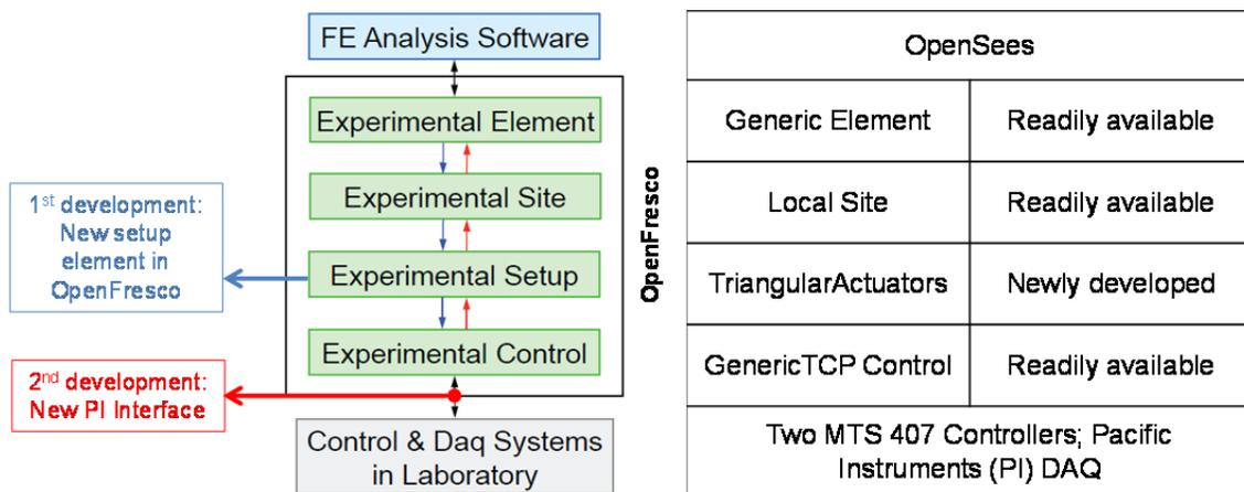
**Figure 2.7** Overview of the HSS using OpenFresco and the new HSS developments.
