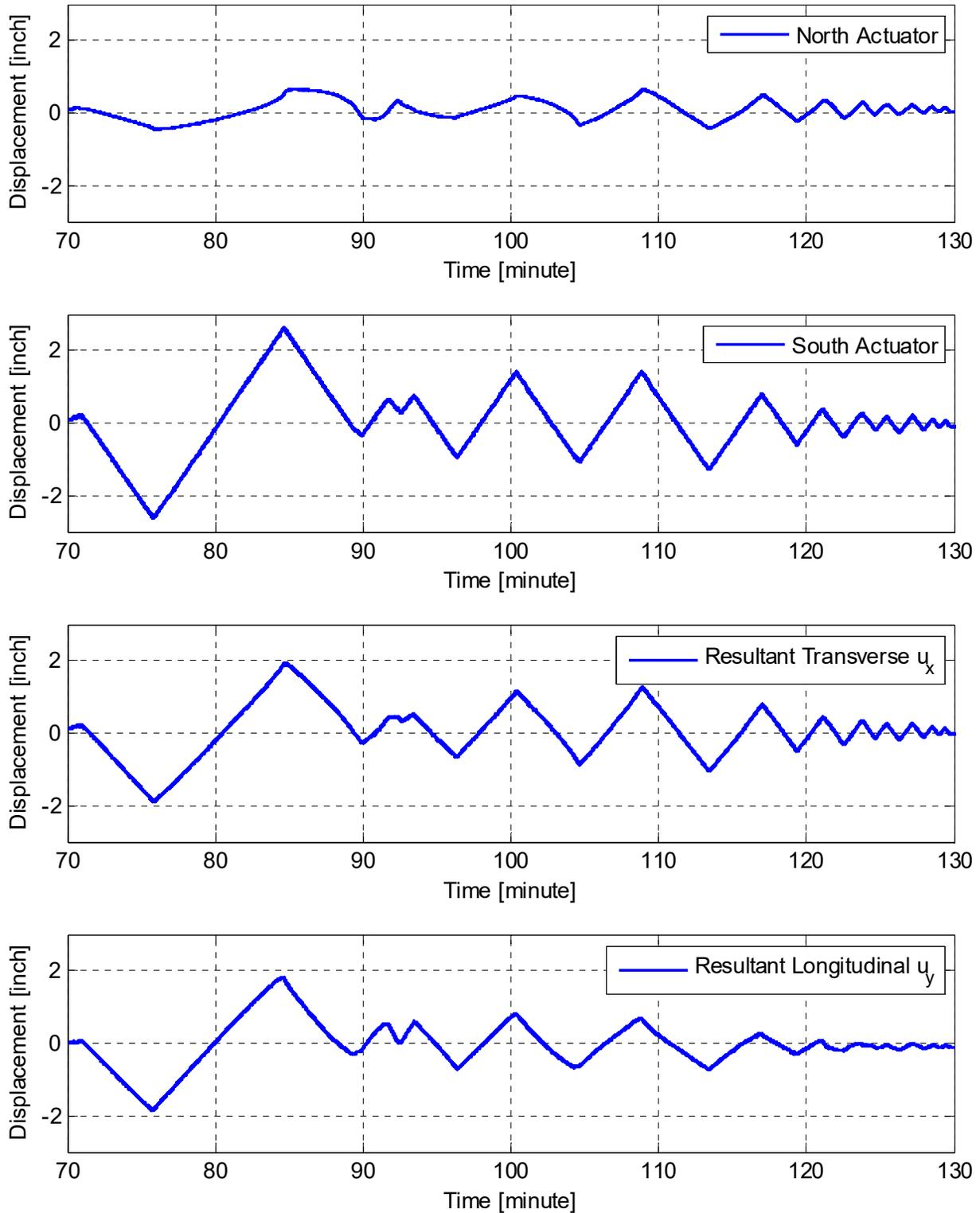
**Figure 3.12** Zoomed-in view of the history of north and south lateral actuators temposonics measurements and the corresponding resultant displacements in transverse ( $u_x$ ) and longitudinal ( $u_y$ ) directions for the 50% scale bi-directional HS test.
