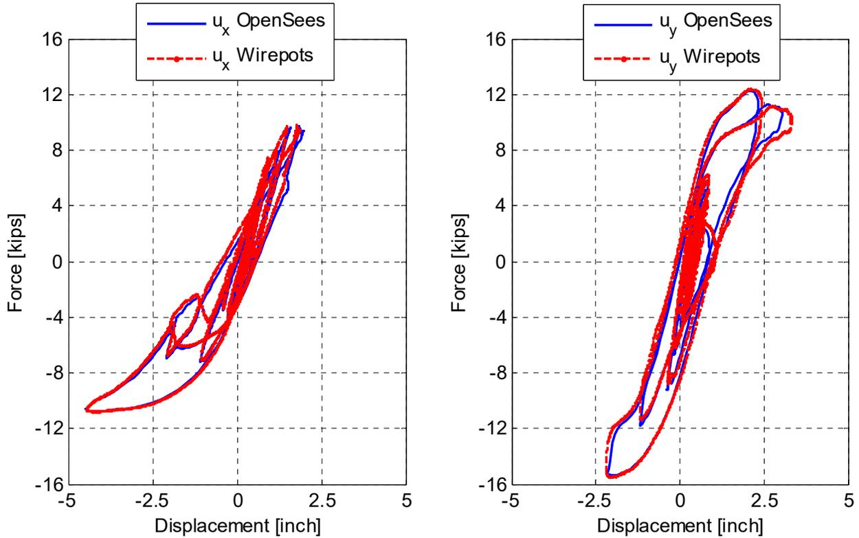
**Figure 2.40** Comparison of force-displacement relationship in transverse (left) and longitudinal (right) directions from the recorded OpenSees data and actual load cells and wirepots DAQ data for the repaired Specimen No. 1 80% Rinaldi bi-directional HS test.
