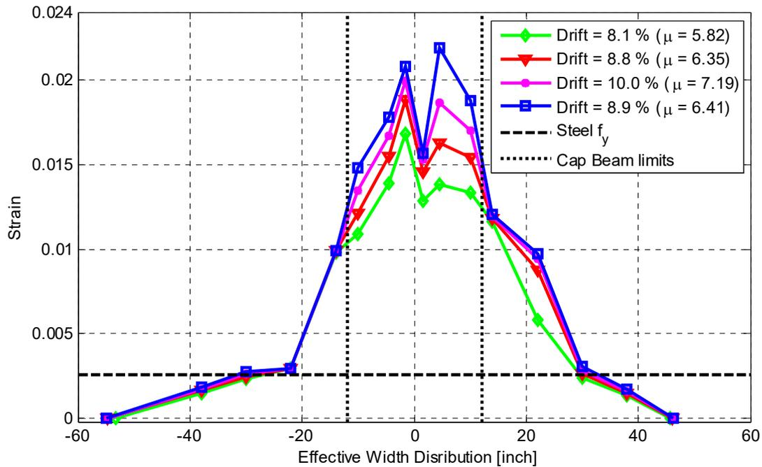
**Figure 3.75** Strain distribution in the tension side at Section B for the four large-scale transverse direction only HS test runs at the negative loading peak (expressed in terms of drift ratio and  $\mu$ ).
