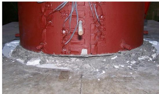
Figure 3.22 Crushed mortar bed at the end of testing of Unit 1B.
