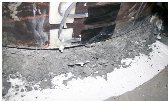
**Figure 3.18** Crushed mortar bed at the end of testing of Unit 1A.
