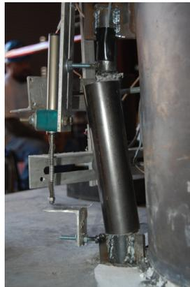
**Figure 3.19** Unit 1A buckling-restrained energy dissipators: (a) south-east energy dissipator hysteretic loops up to 5% drift ratio; (b) north-west energy dissipator hysteretic loops up to 5% drift ratio; and (c) distortion of external energy dissipators.
