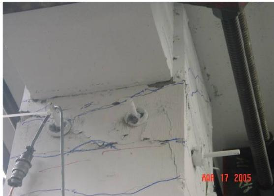
(a) Beam-to-column joint (HS), LPB-10[3]
