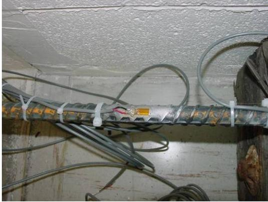
(a) Strain gage on reinforcing steel bar
