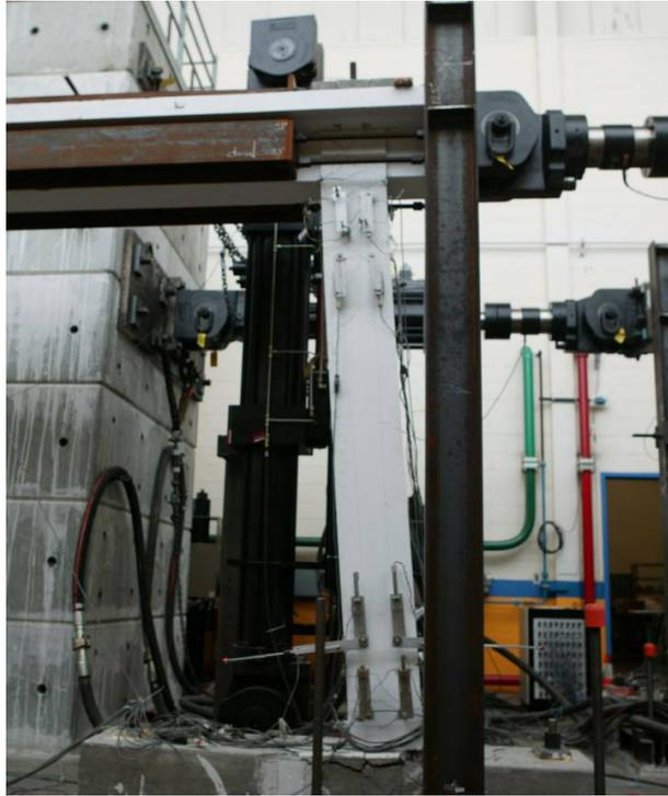
**Fig. 8.24 East column deformed shape at end of phase S-3, LPB-10[3].**
