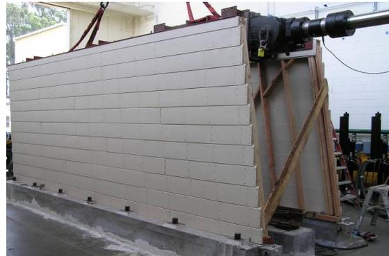
(b) Stair-like deformed shape of shiplap siding (LPG-6)
