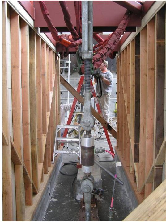
(b) Post-tensioned high-strength steel rod monitored using load cell
