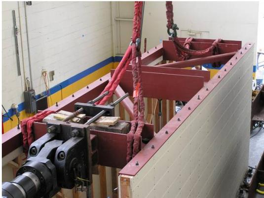
(c) Horizontal loading steel frame
