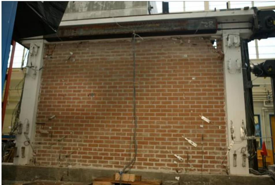
(b) Photograph of instrumented URM infilled frame
