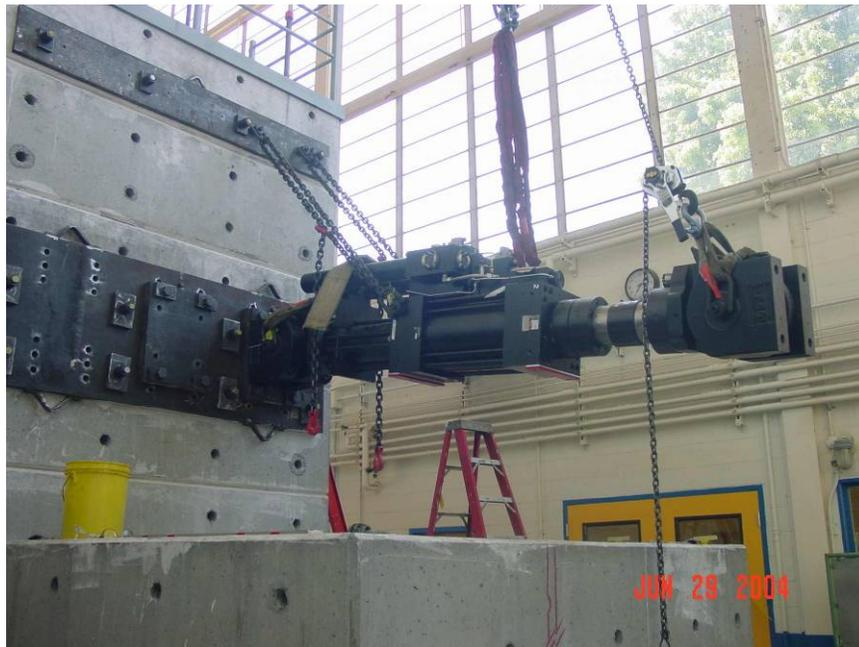
**Fig. 4.14 A 220-kip (979 kN) actuator mounted on RRW.**
