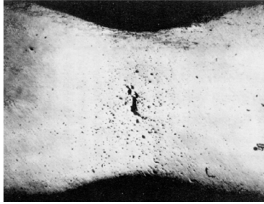
Figure 3.1 Void accumulation in a tensile specimen (Puttick, 1959)
