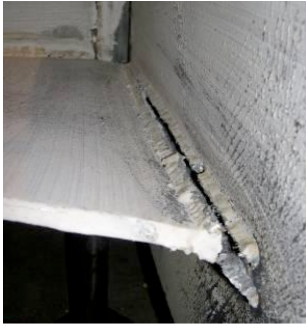
(a) Crack initiation and propagation
