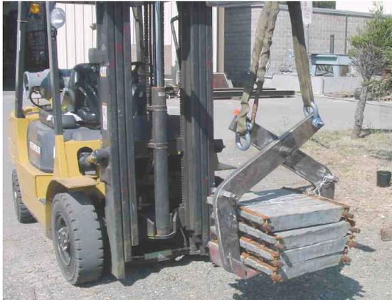
(c) Steel tong designed and constructed to facilitate safe transfer of lead ingots
