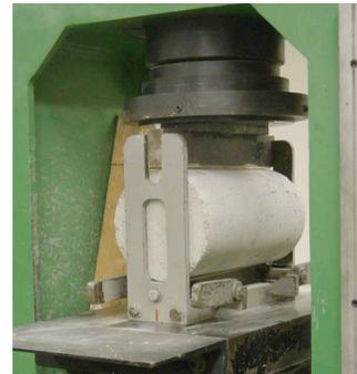
**Fig. 4.2 Concrete split tension test setup.**
