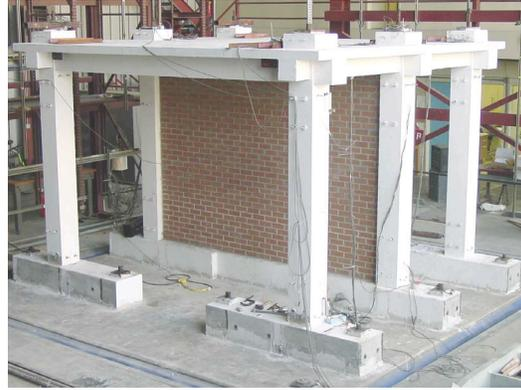
(j) Test structure after completion of URM infill wall
