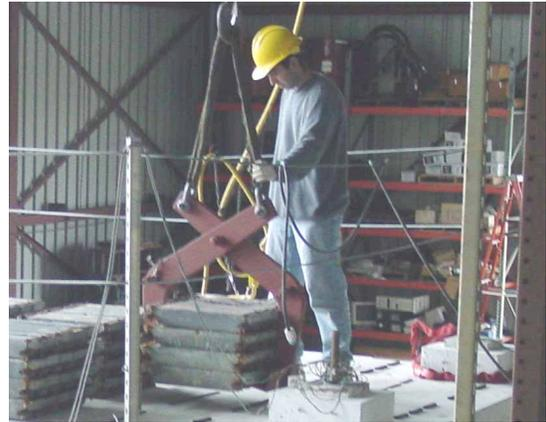
(d) Positioning lead assembly on prescribed locations using crane
