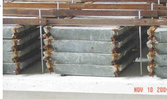
(b) Lead ingots attached to RC slab of test structure
