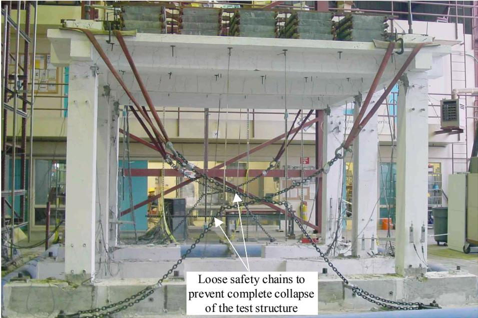
**Fig. 6.38 State of test structure at end of stage three of experiments.**
