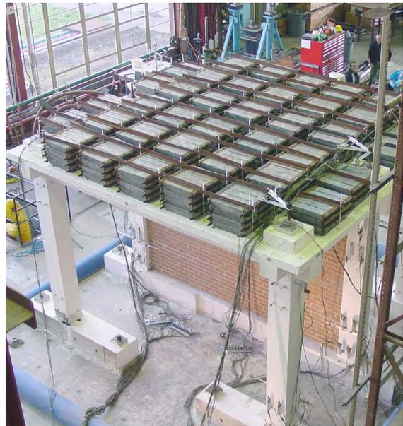
(f) Test structure after completion of mass-stacking procedure (top view)
