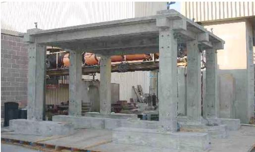
(e) Test structure after stripping forms
