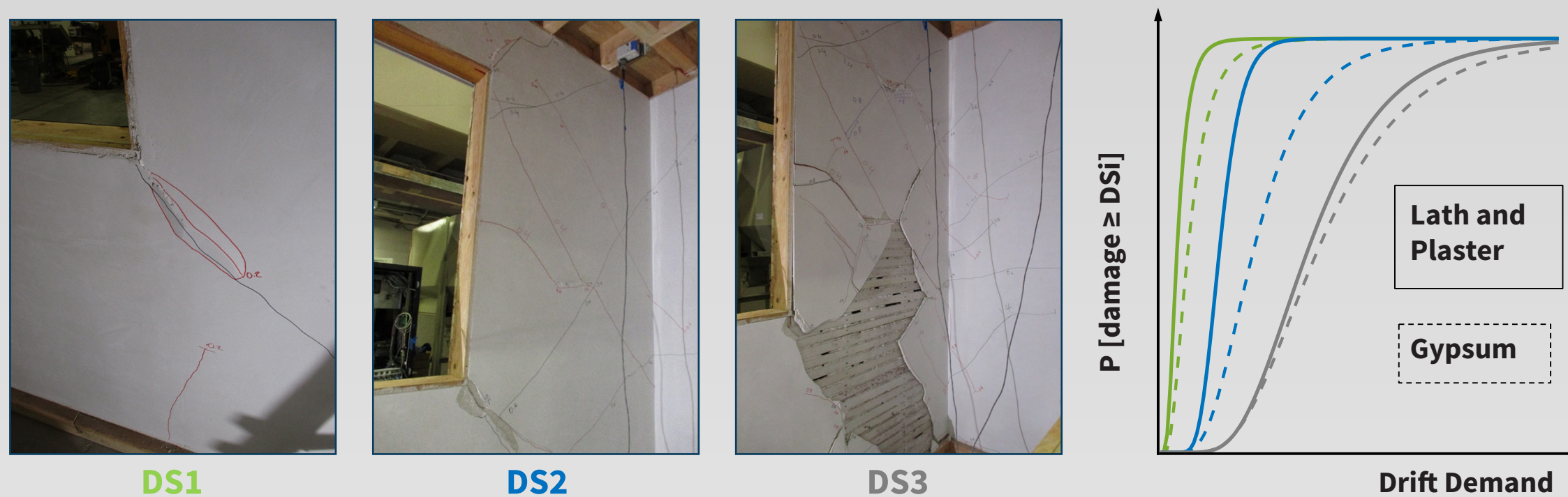
Use of experimental data to improve damage fragilities for plaster on wood lath interior
