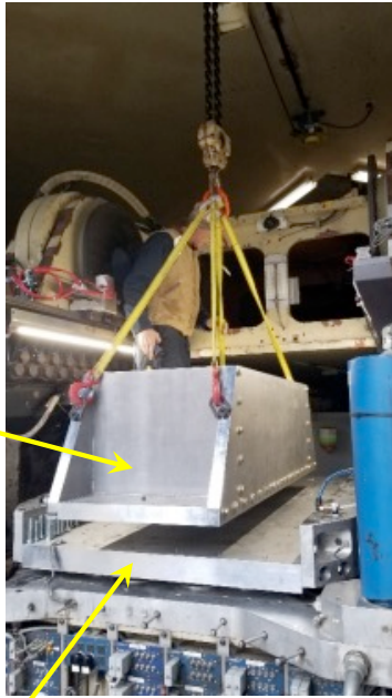
New strong floor, capable of accommodating various smaller boxes
